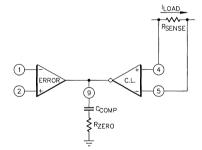
Figure 4. Current Limit Compensation in Comon With Error Amp
