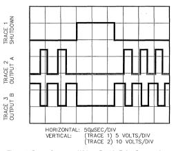
Figure 6. Output Sequence Without Double Pulse Suppression
