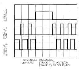
Figure 7. Output Sequence With Double Pulse Suppression
