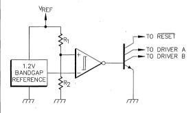
Figure 16. The Undervoltage Lockout Circuit Contains a Bandgap Reference and Comparator Which Becomes Active at V<sub>nee</sub>=3 V<sub>ne</sub>∞2.1 Volts
