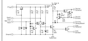
Figure 2. Partial Schematic Diagram SG1627 Driver Circuit
