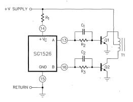
Figure 20. Basic Connections For a Push-Pull Grounded-Emitter Configuration
