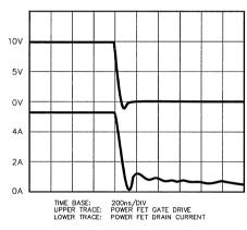
Figure 13. SG1525A/Power Fet Turn-Off Wave Forms
