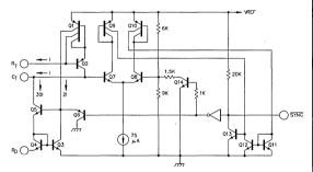
Figure 17. The SG1526 Oscillator Provides Deadband Control By Rationing The Charging Currents to C<sub>+</sub>
