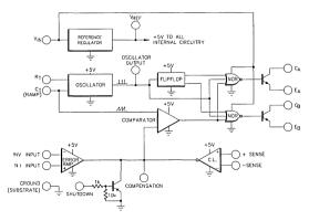
Figure 1. SG1524B Pulse Width Modulator Block Diagram
