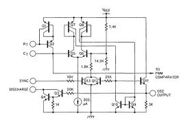
Figure 10. SG1525A/1527A Oscillator Schematic Diagram
