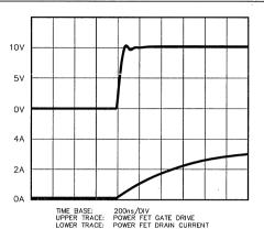
Figure 12. SG1525A/Power Fet Turn-On Wave Forms
