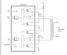
Figure 5. The Low Impedence of the SG1627 in Both On and Off States Allows Direct Transformer Drive With a Minimum of External Components
