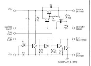
Figure 7. SG1629 Floating Switch Driver Schematic Diagram
