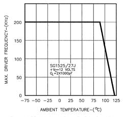
Figure 14. SG1525A/1527A Power Fet Drive Capability
