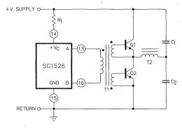
Figure 22. Low Power Transformers are Driven Directly by the Output Terminals
