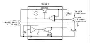
Figure 6. SG1629 Floating Switch Driver Block Diagram
