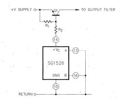
Figure 21. For Single-Ended Configurations the  $\rm V_c$  Terminal is Alternately Switched to Ground by the Driver Pull-Up Transistors
