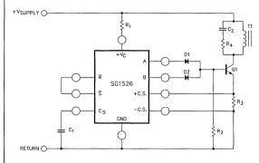
Figure 24. Using the SG1526 in a Flyback Converter With Current Limiting
