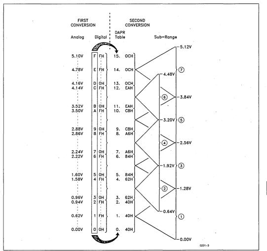
Figure 2. A/D Converter Sub-Ranges
