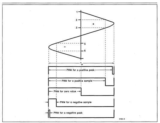
Figure 5. Synthesis of a Sine-Wave Using PWM
