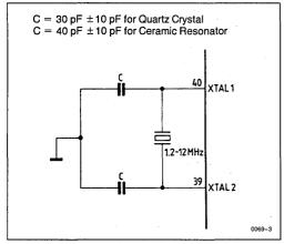
Figure 6. Recommended Oscillator Circuit
