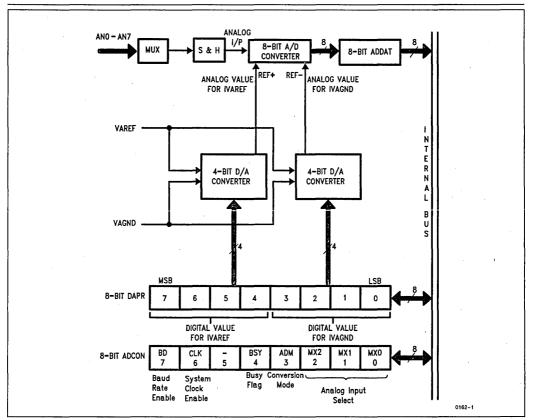
Figure 1. Block Diagram of A/D Converter
