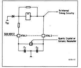
Figure 3-21. On-Chip Oscillator Circuitry
