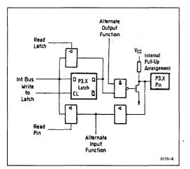
Figure 3-5. Port 3 Circuit
