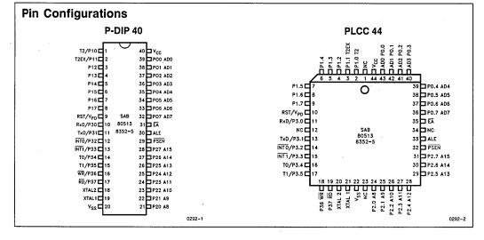
The SAB 80513 and SAB 8352-5 are new members of the Siemens SAB 8051 family of 8-bit microcontrollers. It is fabricated in N-channel, silicon-gate Siemens MYMOS technology.
