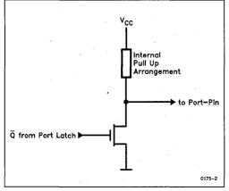
Figure 3-2. Basic Output Driver Circuit of Ports 1 through 5
