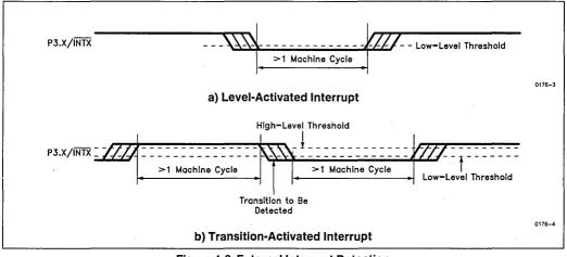
Figure 4-6. External Interrupt Detection
