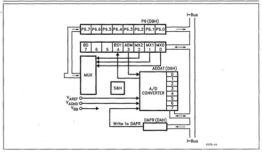
Figure 3-17. A/D Converter Control Register
