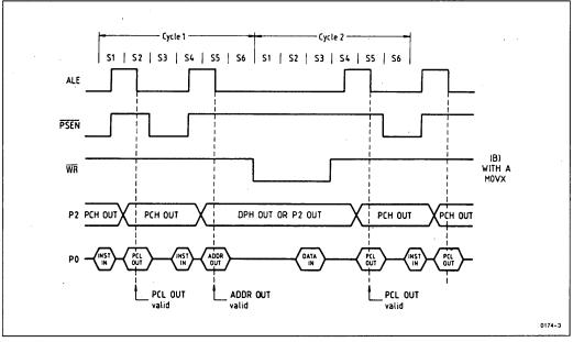
Figure 2-8C. External Data Memory Write
