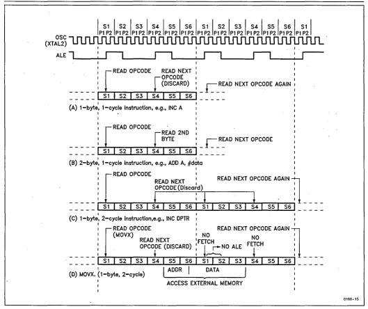
Figure 15. State Sequences in SAB-51 Devices
