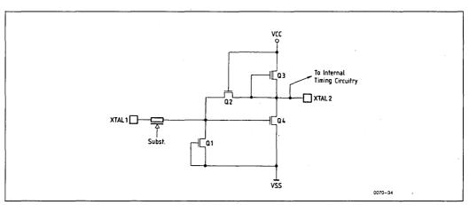
Figure 44. On-Chip Oscillator Circuitry
