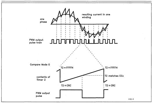
Figure 4. Pulse Width Modulation Using Timer 2 Cycle
