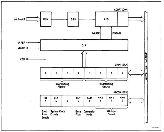
Figure 32. A/D Converter Block Diagram
