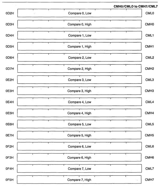
16-bit Compare registers. The compare function of each register controls one output line at port 4 (see Table 4). These registers can individually be assigned either to Timer 2 or to the Compare Timer. When operated with the Compare timer, shadow latches are used to latch the contents at timer overflow.
