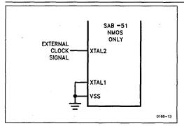
Figure 14. Using an External Clock
