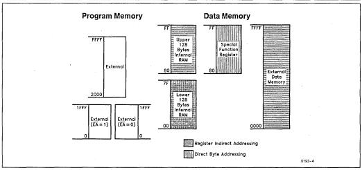
Figure 2. Memory Mapping of the SAB 80C517
