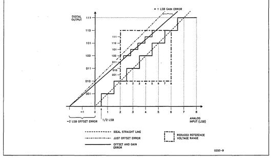
Figure 6. Offset and Gain Error in a Reduced Reference Voltage Range
