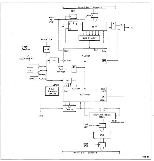
Figure 31c. Serial Port Mode 3, Functional Diagram
