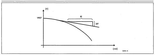
Figure 4. Definition of the Reference Supply Impedance
