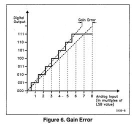
This error can be adjusted by changing the reference voltage or adjusting the input voltage division. The temperature drift of the gain error is generally smaller than that of the offset error.
