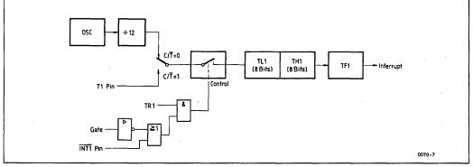
Figure 16. Timer/Counter 1 Mode 1: 16-Bit Counter
