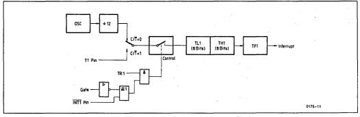
Figure 3-14. Timer/Counter 0/1, Mode 1: 16-Bit Counter
