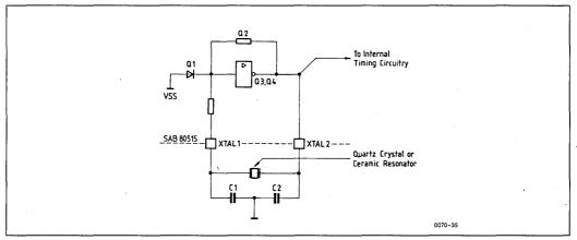
Figure 45. Using the On-Chip Oscillator
