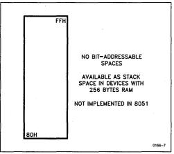
Figure 8. The Upper 128 Bytes of Internal RAM
