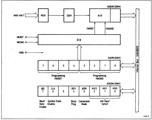
Figure 4. A/D Converter Block Diagram
