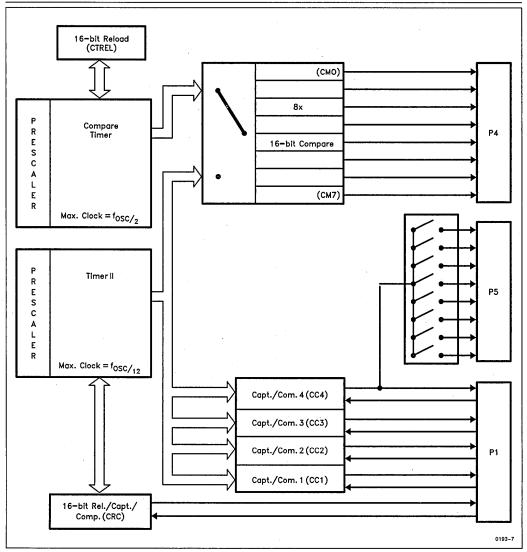
Figure 5. Block Diagram of the Compare/Capture-Unit
