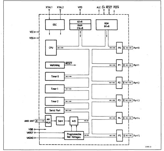
Figure 1. Block Diagram
