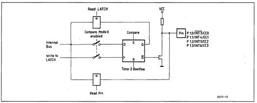
Figure 22. Functional Diagram of Port Latches P1.0 to P1.3 in Compare Mode 0
