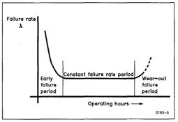
Figure 3. Reliability "Bath-Tub" Curve
