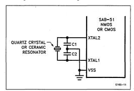
Figure 13. Using the On-Chip Oscillator
