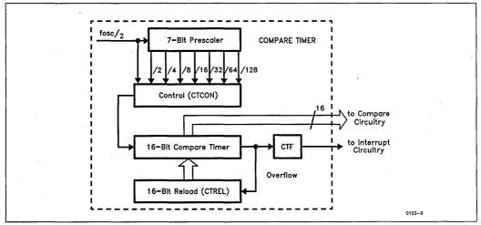
Figure 7. Block Diagram of the Compare Timer
