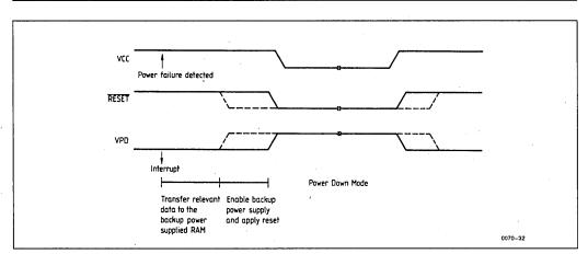
Figure 42. Reset and RAM Backup Power Timing
