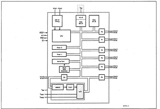
Figure 2-1. Functional Block Diagram
