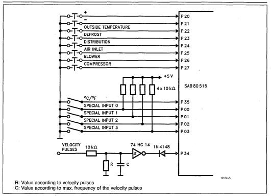
Figure 5. Inputs for Keys, Switches and Speed
