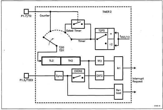
Figure 6. Block Diagram of Timer 2
