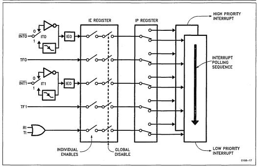
Figure 19. 8052 Interrupt Control System
