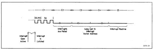
Figure 41. Interrupt Response Timing Diagram
