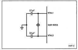
Figure 2. Crystal Oscillator Mode
