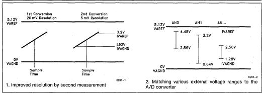
Figure 1. Increase in A/D Converter Resolution
