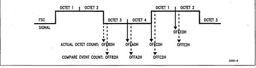
Figure 5. Octet Placement in FSC Signal
