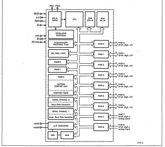
Figure 1. Block Diagram SAB 80C517
