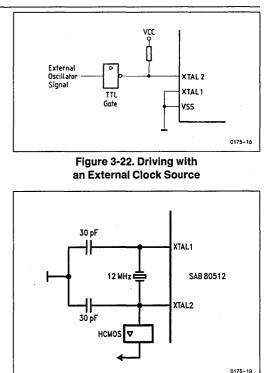
Figure 3-23. Generating a System Clock from the Oscillator Circuit
