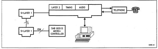
Figure 8. NT—Simulator Application Using the SAB 80515/5353 as a Terminal
