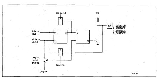
Figure 23. Functional Diagram of Port Latches P1.0 to P1.3 in Compare Mode 1
