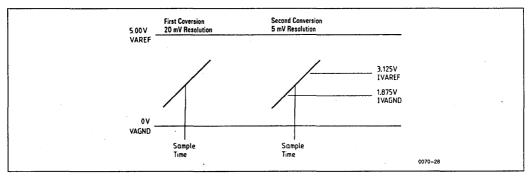
Figure 35b. Increasing the Resolution of the A/D Result by Doing a Second Conversion
