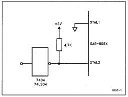
Figure 1. Driving from External Source
