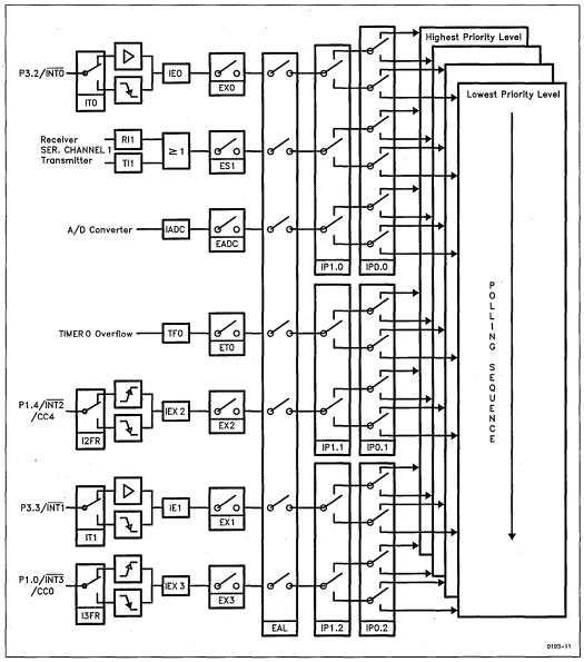
Figure 9. Interrupt Structure of the SAB 80C517
