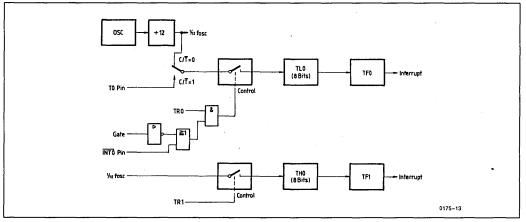
Figure 3-16. Timer/Counter 0 Mode 3: Two 8-Bit Counters
