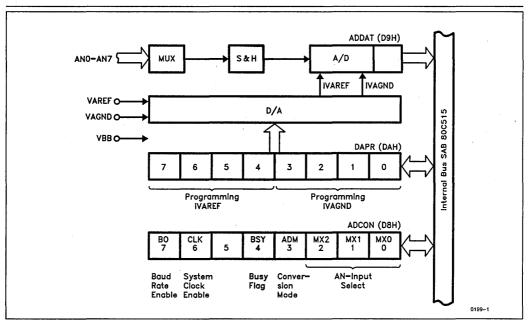
Figure 1. A/D Converter Block Diagram
