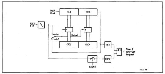
Figure 21. Timer 2 in Reload Mode
