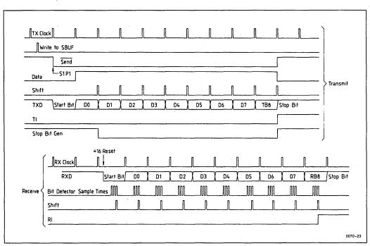
Figure 31b. Serial Port Mode 2, Timing
