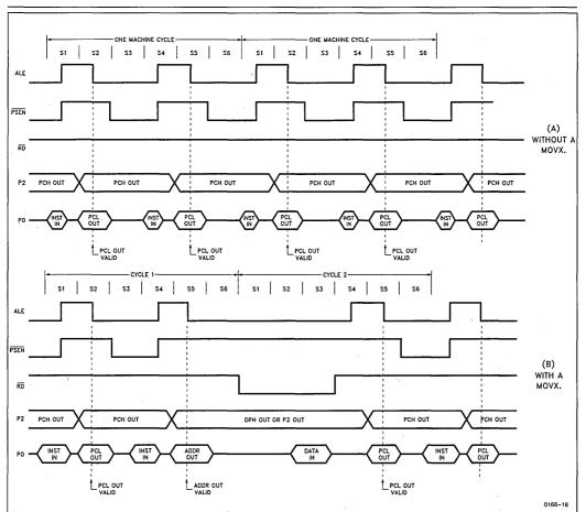
Figure 16. Bus Cycles in SAB-51 Devices Executing from External Program Memory
