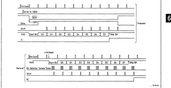
Figure 3-9. Serial Port Mode 1, Timing
