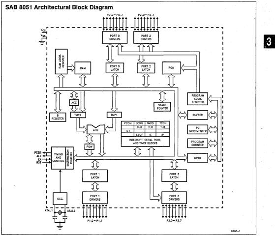
Figure 1. SAB 8051 Architectural Block Diagram
