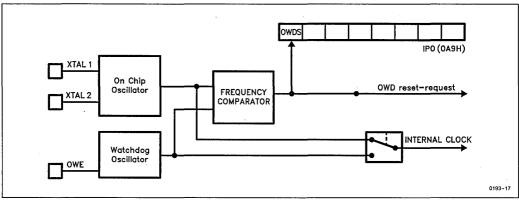
Figure 13. Functional Block Diagram of the Oscillator Watchdog
