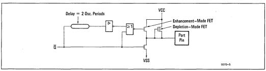
Figure 12. Ports 1 to 5 Internal Pullup Configurations
