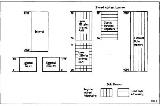
Figure 4. Program and Internal Data Memory Address Spaces
