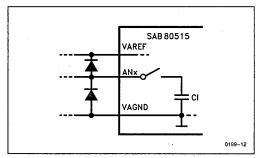
Figure 11. Protection Diodes for Analog Inputs
