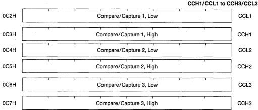
16-bit dual function Compare/Capture-Registers. The compare function of each register controls one port output line (see Table 4) on port 1. These registers exclusively operate with Timer 2 as a time-base. On a compare match an interrupt is requested.
