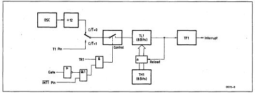
Figure 17. Timer/Counter 1 Mode 2: 8-Bit Auto-Reload
