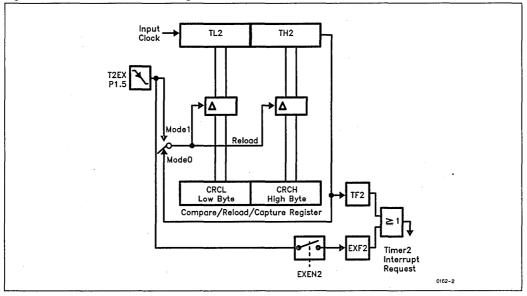
Figure 2. Timer 2 in Reload Mode
