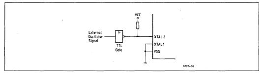
Figure 46. Driving with an External Clock Source
