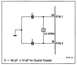
Figure 3-20. Recommended Oscillator Circuit
