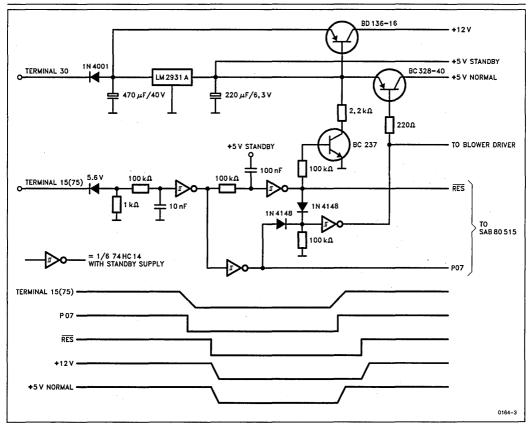
Figure 3. Voltage Supply, Reset Logic
