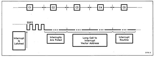
Figure 4-5. Interrupt Response Timing Diagram
