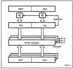
Figure 2. PWM Using the PTRA Unit
