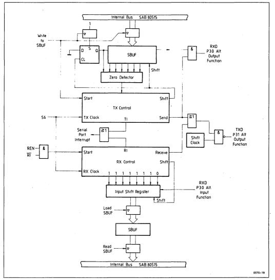
Figure 29a. Serial Port Mode 0, Function Diagram
