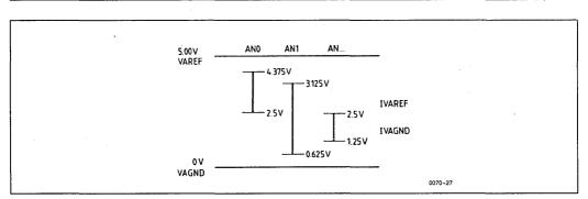
Figure 35a. Adjusting the Internal Reference Voltages to the Range of the External Analog Voltages
