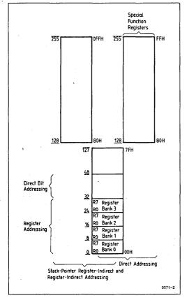
Figure 49. Internal Data Memory Address Space
