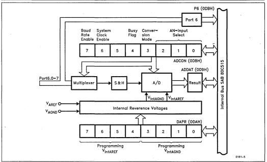
Figure 3. Block Diagram of the A/D Converter
