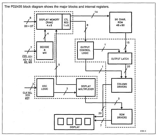
Figure 3. PD2435 Block Diagram
