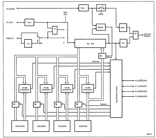
Figure 4. Block Diagram of the PTRA Unit
