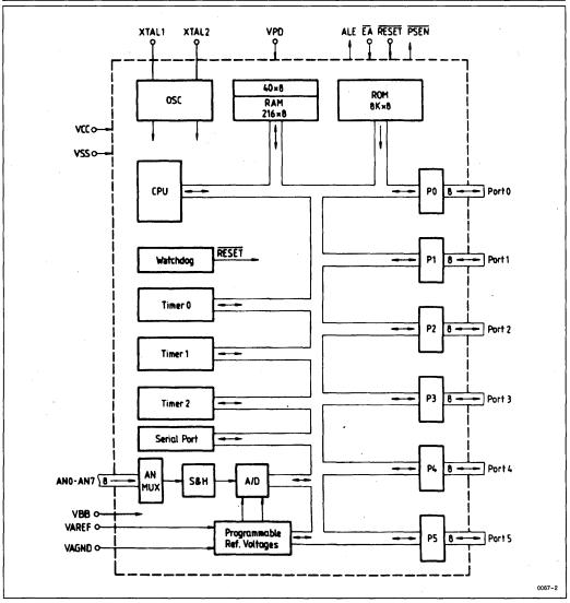
Figure 2. Block Diagram
