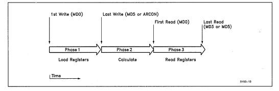
To start an operation, register MD0 to MD5 (or ARCON) must be written to in a certain sequence according to Table 6 or 7. The order the registers are accessed determines the type of the operation. A shift operation is started by a final write operation to register ARCON (see also the register description).
