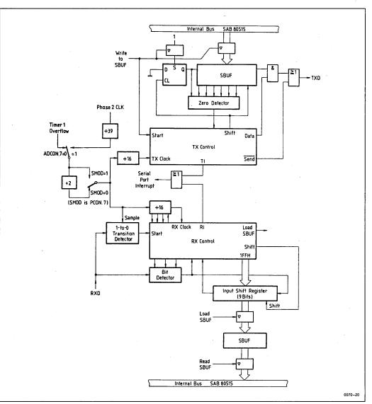
Figure 30a. Serial Port Mode 1, Functional Diagram
