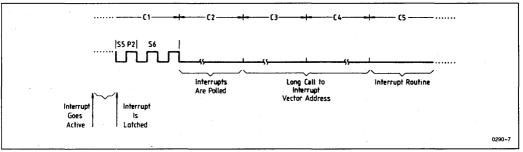
Figure 6. Interrupt Response Timing Diagram
