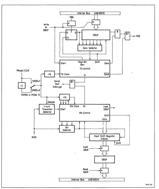
Figure 31a. Serial Port Mode 2, Functional Diagram
