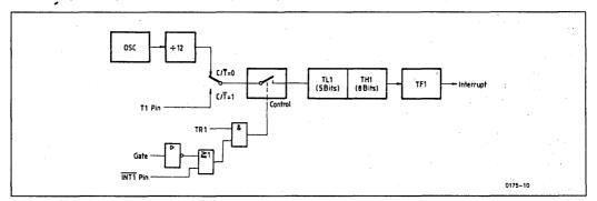
Figure 3-13. Timer/Counter 0/1, Mode 0: 13-Bit Counter
