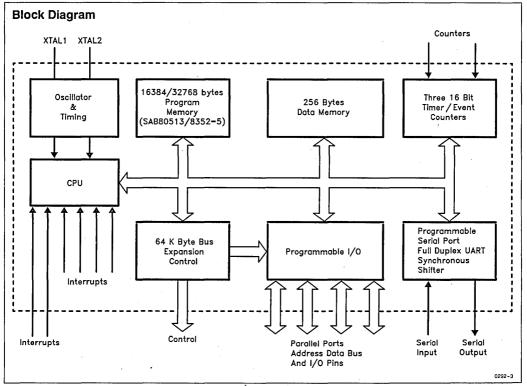
The SAB 80513 and the SAB 8352-5 are standalone, high-performance single-chip microcontrollers based on the SAB 8051 architecture. They maintain all features of the SAB 8051A and SAB 8052B (including timer 2 of the SAB 8052B) and are thus fully compatible with both the SAB 8051A and SAB 8052B.
