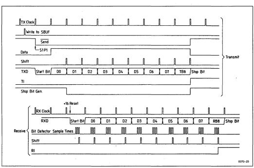
Figure 31d. Serial Port Mode 3, Timing
