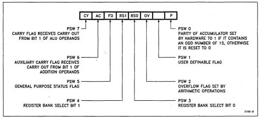
Figure 10. PSW (Program Status Word) Register SAB-51 Devices
