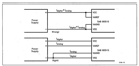
**Figure 9. Power Supply Connections**
