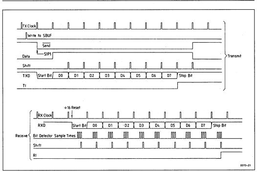
Figure 30b. Serial Port Mode 1, Timing
