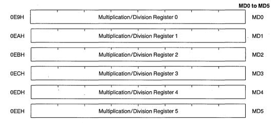
Operand registers of the MDU must be loaded in a certain sequence to start a MDU-operation (see Table 6 or 7). Registers also contain result and remainder after operation. MD0 is the first byte to be written in any operation. Writing to MD5 completes the trigger-procedure of multiplication and division.
