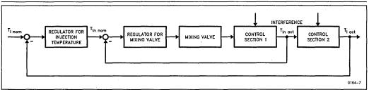
Figure 7. Block Diagram of Temperature Regulation
