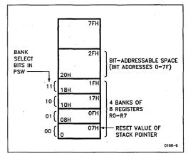
Figure 7. The Lower 128 Bytes of Internal RAM
