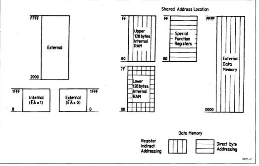
Figure 48. Program Memory and Data Memory Address Spaces
