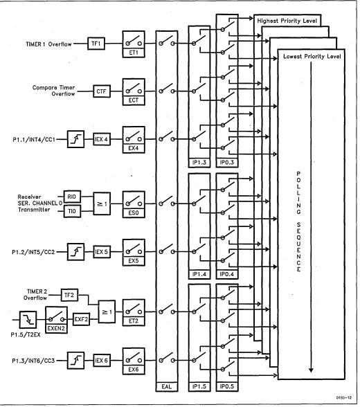
Figure 9. Interrupt Structure of the SAB 80C517 (Continued)
