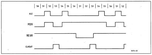
Figure 43. System Clock Timing
