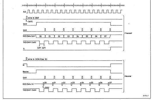
Figure 3-8. Serial Port Mode 0, Timing
