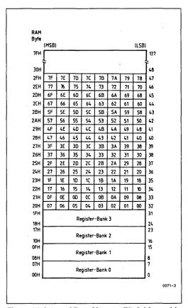
Figure 50. Internal Data Memory Bit-Addressable Locations
