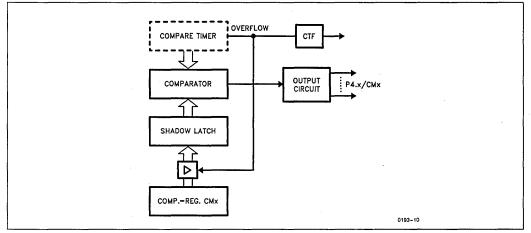
Figure 8. Compare-Mode 0 with Registers CM0 to CM7
