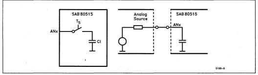
Figure 7. Analog Interface, an RC Network
