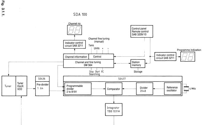
It is electrically programmable and converts the tuning information to a frequency information which determines the dividing factor of the PLL-divider and which is serially transfered to the PLL-circuit. The total channel numbers are stored in the station memory, i.e., each address of the memory corresponds to a TV station.
