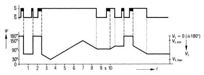
Fig. 6.1.3. Influencing the phase angle by touching the sensor
