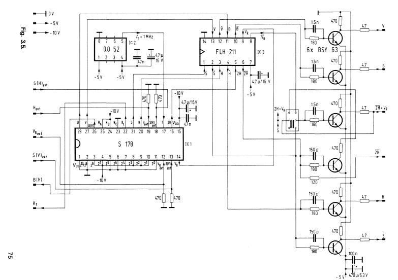
All important pulses are generated either as pulse composition (synchroneous pulse composition S, blanking pulse composition B) or as separate pulses (V, H,  $\overline{2H}$ ,  $2H + V_R$ ). They are available at transistor output stages driven by the TTL-IC FLH 211. Besides that the horizontal blanking pulses B (H) and the clamping pulses K<sub>t</sub> are generated. The fan out for the output stage of these two pulses is one TTL-input each.
