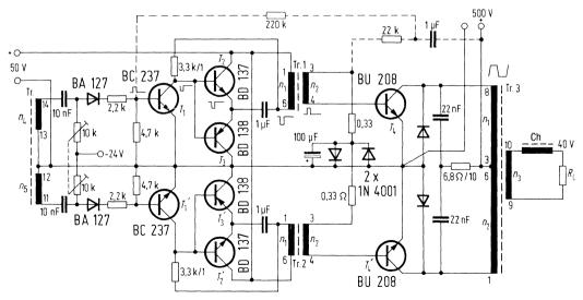
The pulse duration can be adjusted by resistor  $R_1$  if a control voltage is applied. For variable blanking intervals the resistance of  $R_1$  or the  $\pm 24$  V-supply-voltage has to be changed.
