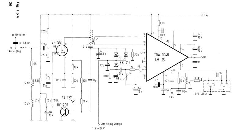
signal level at the capacitance diode of the oscillator circuit is kept constant to a value of approx. 800 mV<sub>pp</sub> by means of the internally controlled oscillator.
