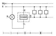
Fig. 6.1.2. Arrangement of parallel-connected control devices
