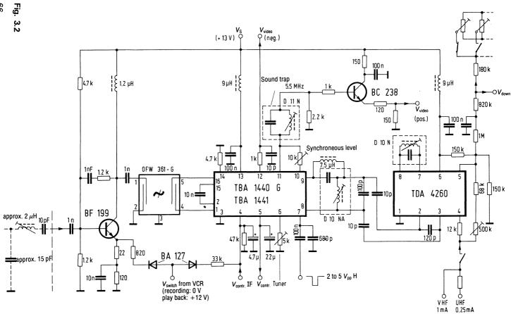
TBA1440 to a gain minimum by an impressed IF control-voltage of approx. 3 V. Because of the internal control amplifier the tuner is also downward-controlled.
