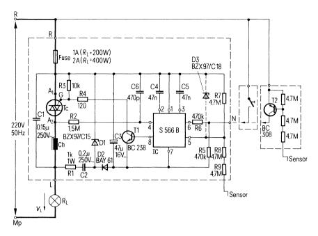
**Fig. 6.1.1.** Circuit of the electronic sensor dimmer using the new MOS IC type S 566 B. Attention has to be paid in that the correct connections are made, i.e. R to the hot lead, and L to the lamp.
