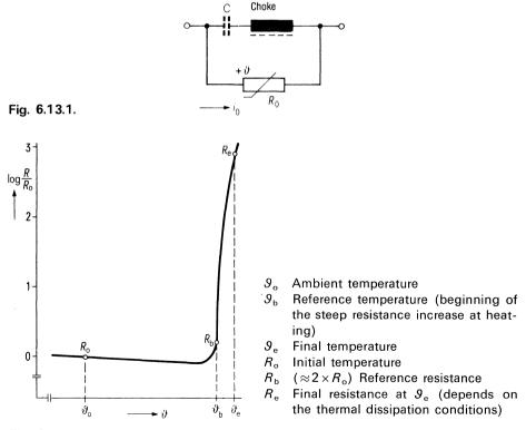
reference temperature  $\mathcal{P}_{b}$ . Its resistance increases rapidly in that the current drops to a very small value. The final resistance  $R_{e}$  which will be adopted depends on the heat dissipation conditions. It is, in this case, rising at least to the power of two decades of the initial resistance  $R_{o}$ . The power to maintain the highly resistive balance is about 1 W.
