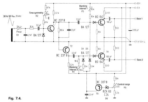
The blanking intervals are adjusted by potentiometers R3 and R4. The differentiated pulses are amplified by the Darlington transistors T3 and T4 and applied in push-pull to base 1 and 2 of the output-stage transistors, whereby the two 100  $\mu F$  – electrolytic – capacitors transmit the control and turn-off currents.
