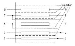
Winding schematic for transformer Tr 3 Potcore: 87 mm  $\emptyset \times 70$  mm, L = 1 mm (inside) B 65713 - A0000 - R027 Coil former: B 65714-A1001-T 001
