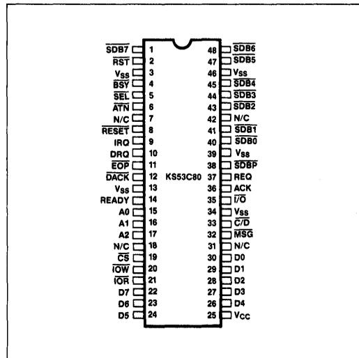
Figure 3. Physical Layout of the KS53C80 SCSI Bus Controller (DIP-48 Version)
