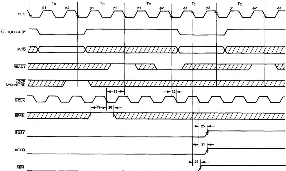
Figure 18. MULTIBUS® Release due to CBRQ Active
