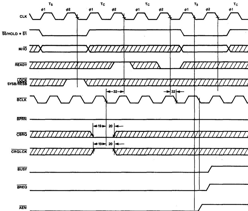
Figure 19. MULTIBUS® Acquisition During 80286 INTA Cycles
