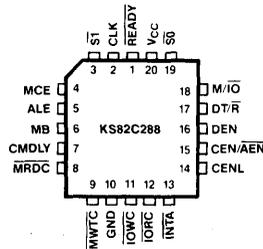
Figure 2b. KS82C288 DIP Pin Diagram
