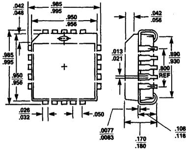
Figure 17. 68-Pin PLCC Package
