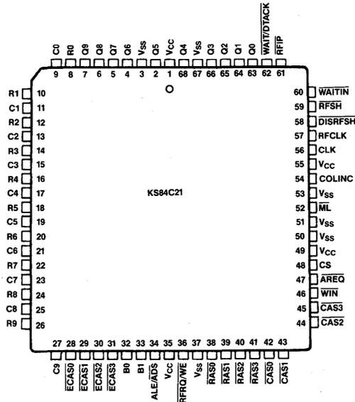
Figure 3. Pin Configuration of the KS84C22 DRAM Controller
