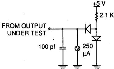
Figure 14: STANDARD TEST LOAD
