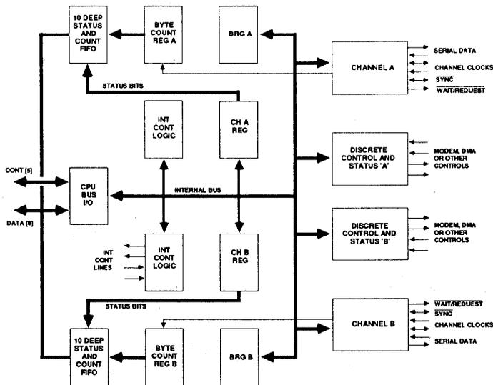
Figure 1 : KS85C30 BLOCK DIAGRAM
