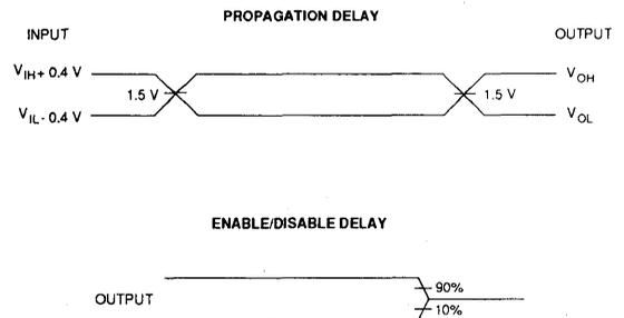
A.C. Testing: All input signals must switch between  $V_{IL} + 0.4$  V and  $V_{IH} - 0.4$  V. TR and TF must be  $\leq 15$  ns.
