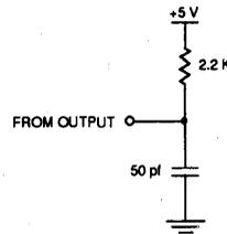
Figure 15: OPEN-DRAIN TEST LOAD
