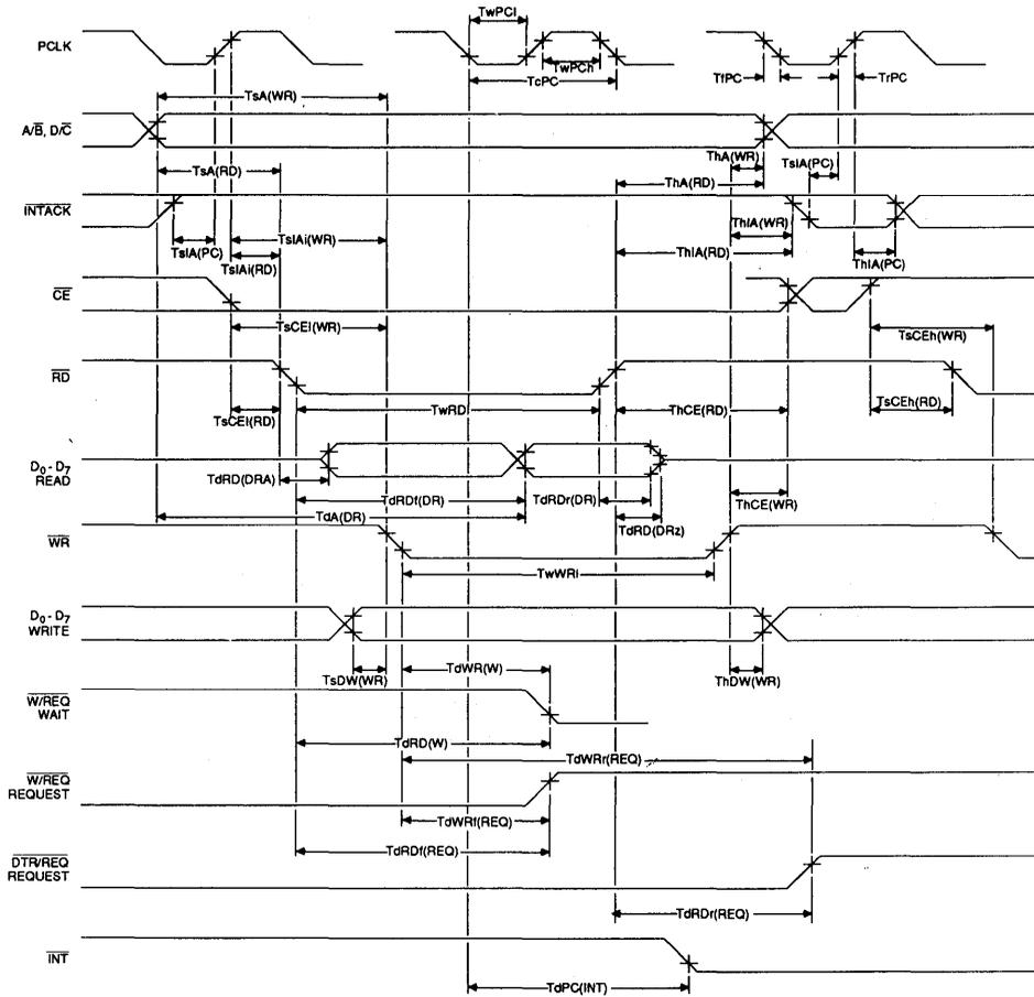
**Note:** Addresses on A/B and D/C and the status on INTACK must remain stable throughout the cycle. If CE falls after RD or WR falls, or if it rises before RD or WR rises, the effective RD or WR is shortened. Data must be valid before the falling edge of WR.
