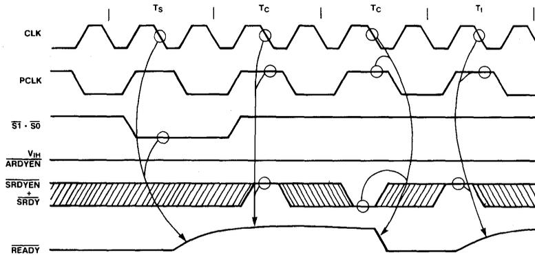
Figure 7. Asynchronous READY Operation
