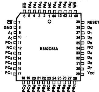
Figure 1a: 44-Pin PLCC Configuration
