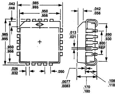
**Figure 28. 84-Pin PLCC Package**
