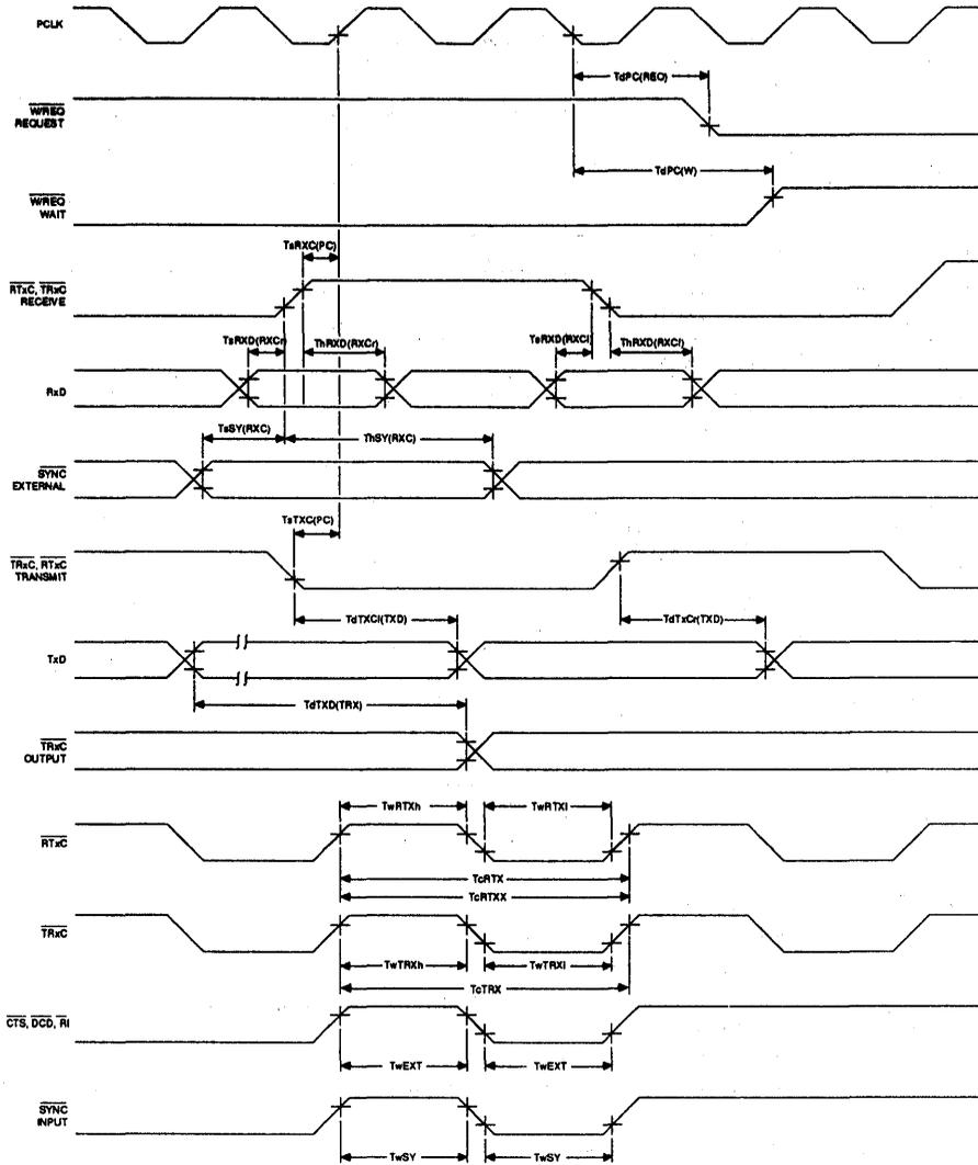
Table 9 : AC CHARACTERISTICS, SYSTEM TIMING ( $T_A = 0^\circ\text{C}$  to  $70^\circ\text{C}$ ,  $V_{DD} = 5V \pm 5\%$ )
