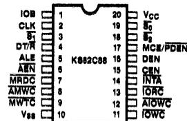
Figure 1b: 20-Pin DIP Configuration
