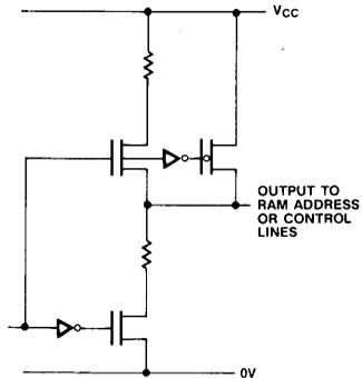
Figure 8. Mode 1, Interleave, Address Latch
