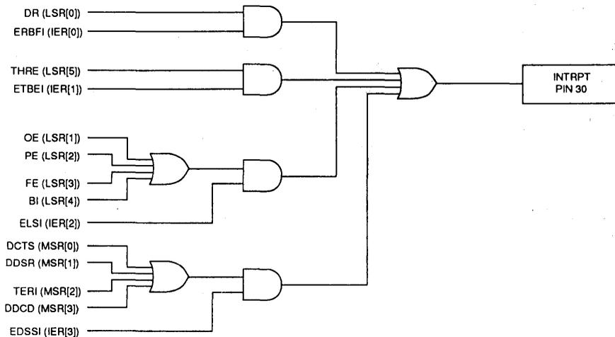
Figure 6 : 82C50A INTERRUPT CONTROL STRUCTURE
