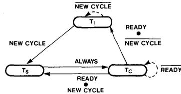
Internal CPU processor clock phases correspond to the bus state phases.
