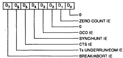
Figure 9 : READ REGISTER BIT FUNCTIONS
