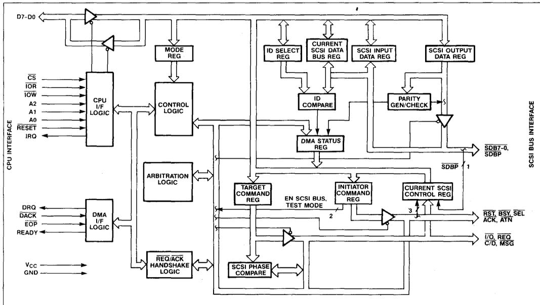
Figure 1. Functional Block Diagram of KS53C80
