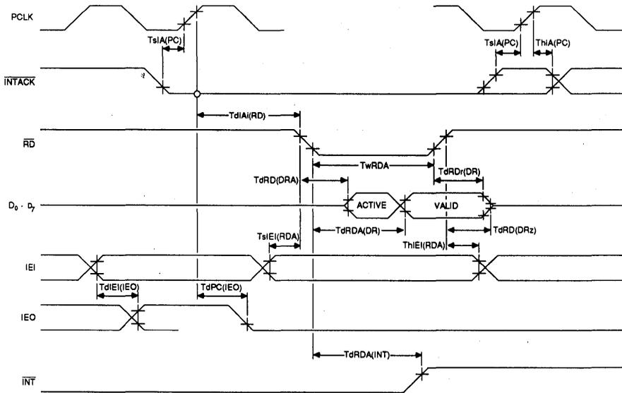
**Note:** Between the time INTACK goes Low and the falling edge of RD, the internal and external IEI/IEO daisy chains settle. If there is an interrupt pending in the SCC and IEI is High when RD falls, the Acknowledge cycle is intended for the SCC. In this case, the SCC may be programmed to respond to RD Low by placing its interrupt vector on D<sub>0</sub>-D<sub>7</sub> and it then sets the appropriate Interrupt-Under-Service latch internally.
