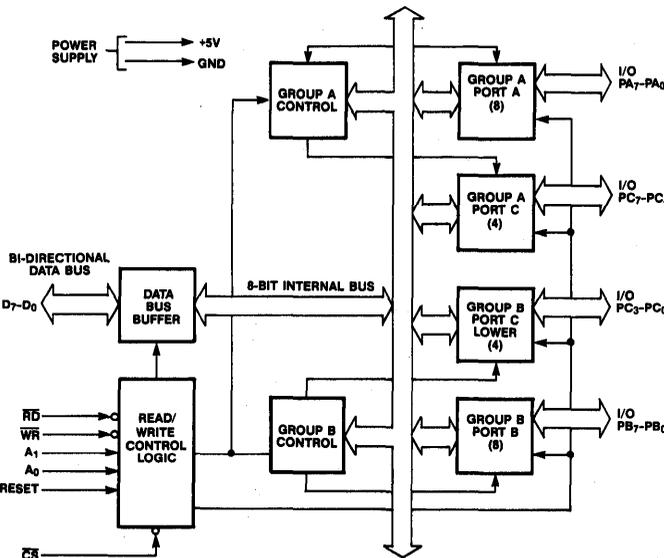
Figure 2: KS82C55A Block Diagram
