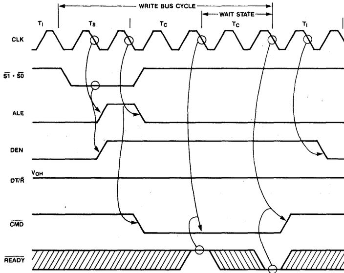
Figure 8. Write-Write Bus Cycles with MB = 0
