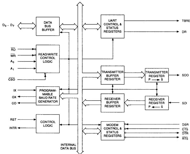
Figure 1 : KS82C52 BLOCK DIAGRAM
