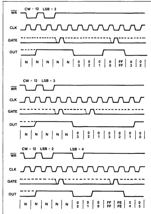
After a Control Word and initial count have been written, the Counter is loaded on the next CLK pulse. OUT goes low N CLK pulses after the initial count is written, which allows the Counter to be synchronized by software.
