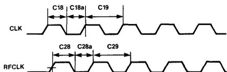
Figure 11. KS84C31/32 Static Column Operation Mode 1
