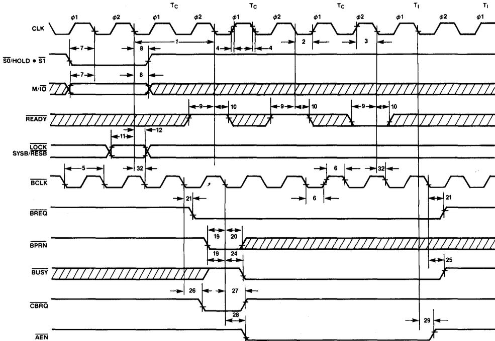
Figure 17. MULTIBUS® Release due to BPRN Inactive
