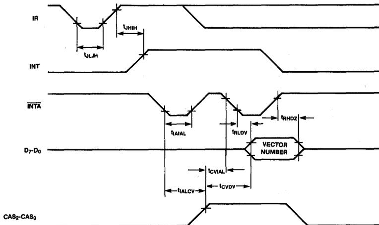
Note that IR input should remain at a high level until the leading edge of the first  $\overline{INTA}$  pulse.
