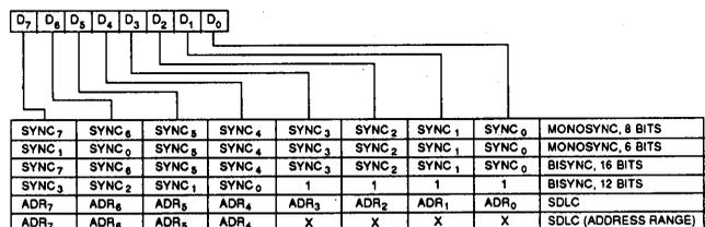
Figure 10 : WRITE REGISTER BIT FUNCTIONS
