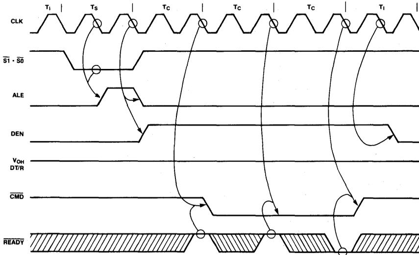
The MB control input affects the timing of the command and DEN outputs. These outputs are automatically delayed in Multibus 1 mode to satisfy three requirements:
