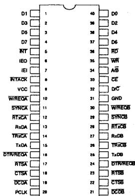
Figure 2b: 40-PIN DIP CONFIGURATION
