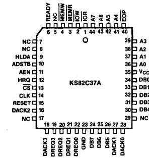
Figure 2: 44 Pin PLCC Configuration
