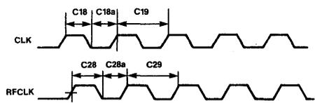
Figure 14. Internal Refresh — Interleave Access
