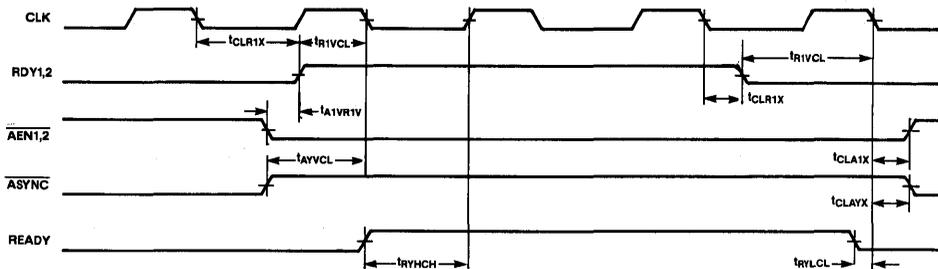
Figure 5: AC Testing I/O Waveform
