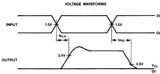
AC Testing inputs are driven at 3.0V for a logic "1" and 0.0V for a logic "0". Timing measurements are made at 2.4V for a logic "1" and 0.8V for a logic "0" at the outputs.
