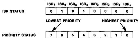
BEFORE ROTATE: IR<sub>4</sub> is the highest priority requiring service
