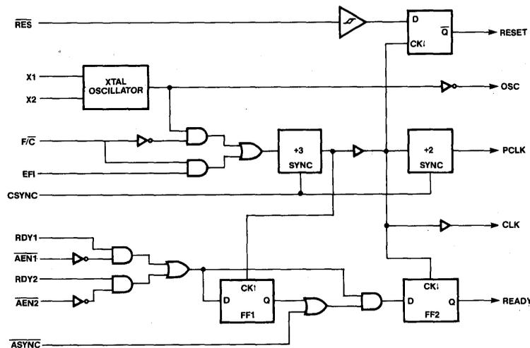
Figure 2: KS82C84A Block Diagram
