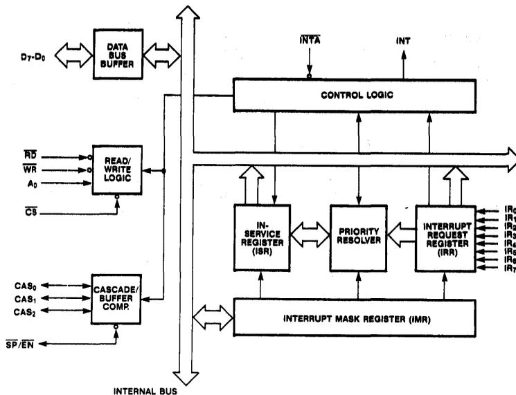
Figure 1: Block Diagram of KS82C59A
