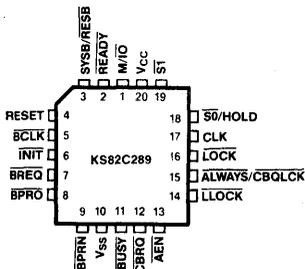
Figure 2b: 20-pin DIP Configuration
