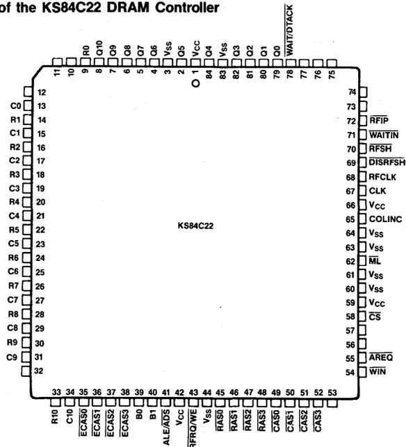
Table 1 shows detailed pin allocations for the KS84C21, while Table 2 shows the KS84C22. Table 3 provides the input/output signal definitions.
