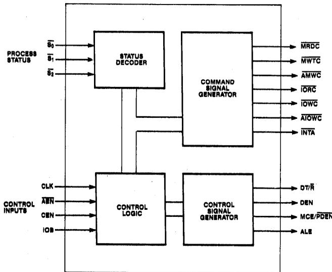
Figure 2: KS82C88 Block Diagram
