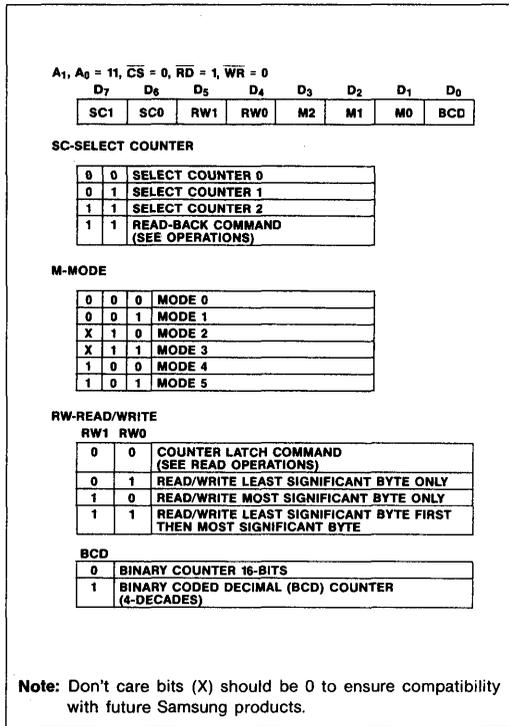
If a Counter is programmed as a 16 bit counter, the Control Register should not be accessed between writing the first and second byte count. Otherwise, the Counter will be loaded incorrectly.
