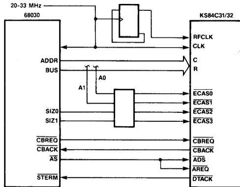
Figure 18. 68040 or Similar CPU or Cache Interface KS84C31/32 Interface Timing with Nibble Mode Burst Access
