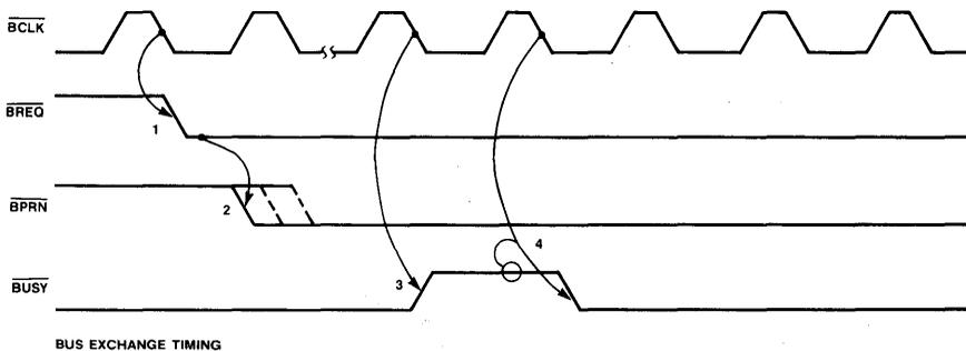
A multi-master bus request is initiated when two conditions occur. 1) a processor signals the status for memory read, memory write, I/O read, I/O write, or interrupt acknowledge. 2) an  $\text{SYSB}/\overline{\text{RESB}}$  (high) at the end of  $T_S$ .
