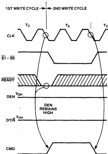
Bus cycles can occur back-to-back with no  $T_1$  bus states between  $T_C$  and  $T_S$ . Back-to-back cycles do not affect the timing of the command and control outputs. Command and control outputs always match the states shown for the same clock edge (within  $T_S$ ,  $T_C$ ) or falling bus state of a bus cycle.
