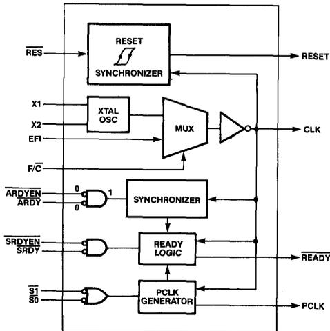
Figure 1. KS82C284 Block Diagram
