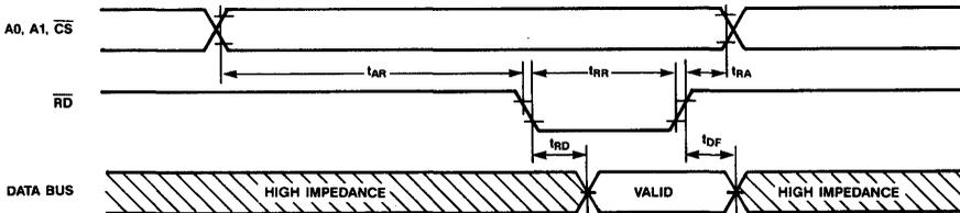
Figure 24: AC Testing I/O Waveform
