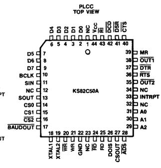
Figure 3: PLCC Pin Assignments
