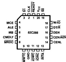
Figure 2a. KS82C288 PLCC Pin Configuration
