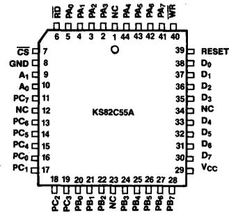
Figure 1a: 44-Pin PLCC Configuration
