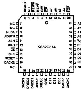
Figure 2: 44 Pin PLCC Configuration
