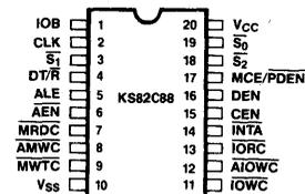
Figure 1b: 20-Pin DIP Configuration
