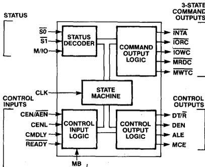
Figure 1. KS82C288 Block Diagram
