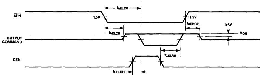
Note: CEN must be LOW or valid prior to  $S_2$  to prevent the command from being generated.
