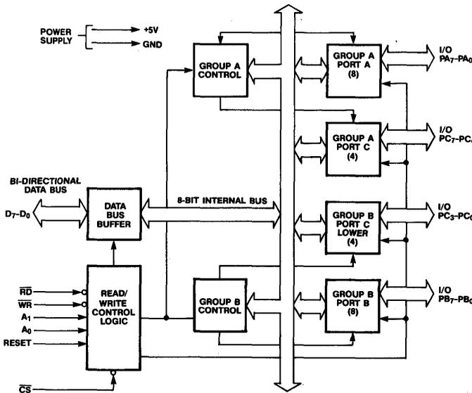
Figure 2: KS82C55A Block Diagram
