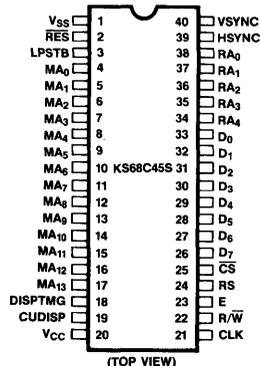
Figure 2: Pin Arrangement
