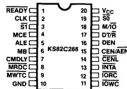
Figure 2b. KS82C288 Pin Configuration
