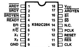
Figure 2b. KS82C284 Pin Diagram
