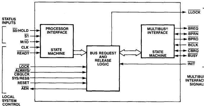
Figure 1. KS82C289 Block Diagram
