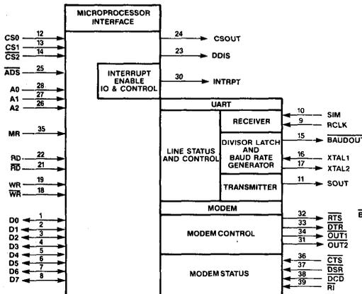
Figure 1: Pin Functions
