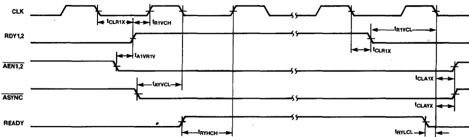
c) Ready Signals (for Synchronous Devices)
