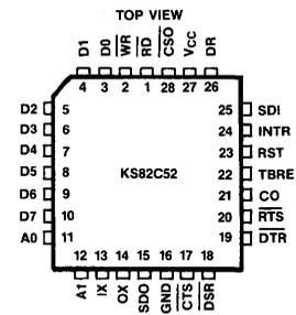
Figure 2a: PLCC Pin Assignments
