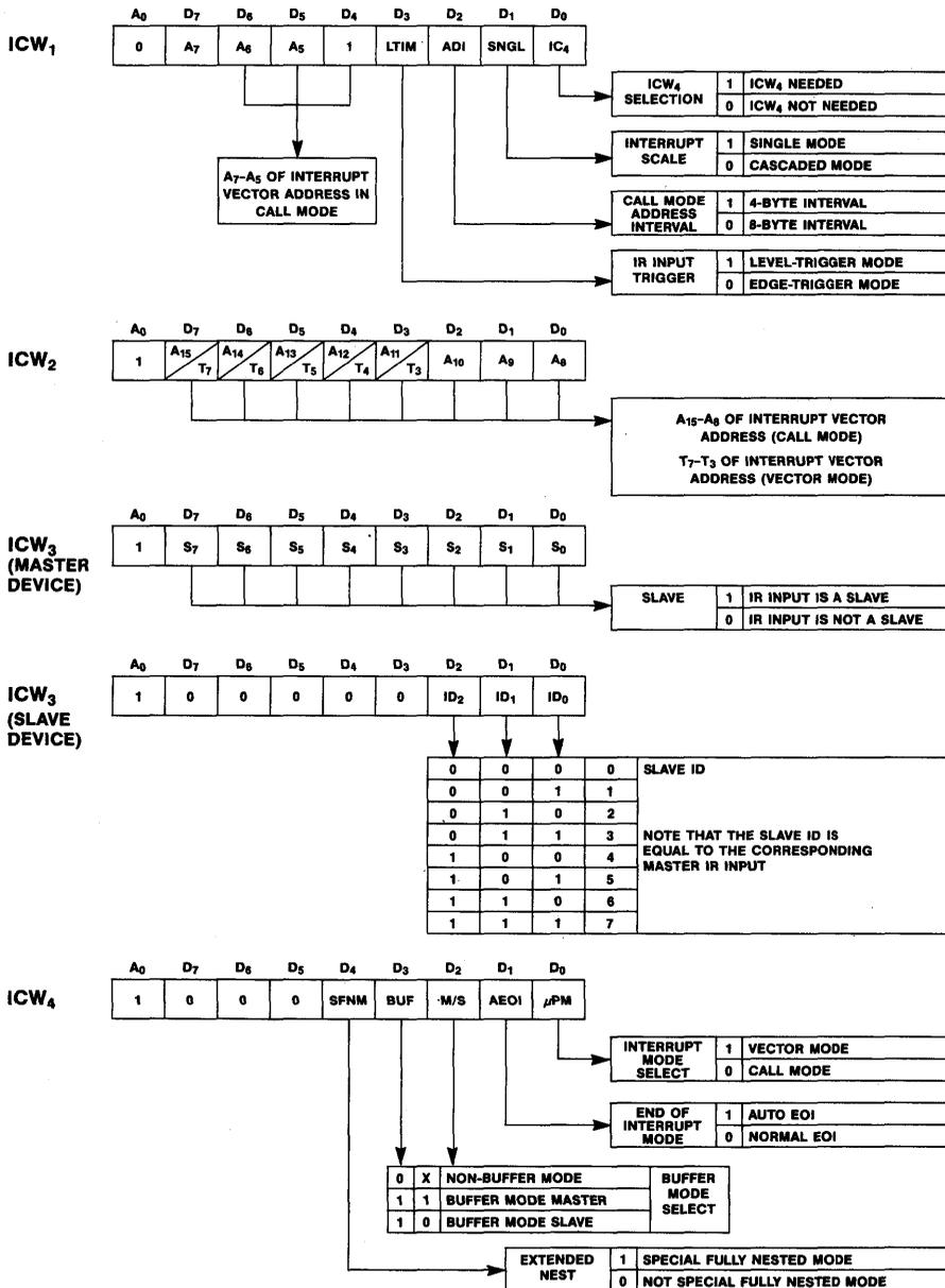
Figure 12. Operation Command Word Format
