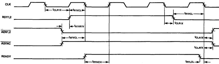
Figure 5: AC Testing I/O Waveform
