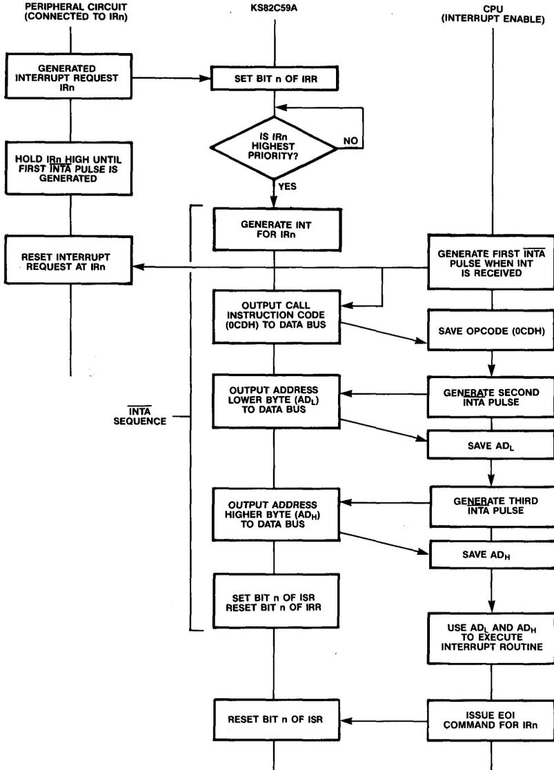
Figure 5: CALL Mode Operation (Cascaded KS82C59A Systems)
