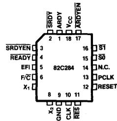
Figure 2a. KS82C284 PLCC Pin Diagram
