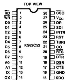
Figure 2b: DIP Pin Assignments
