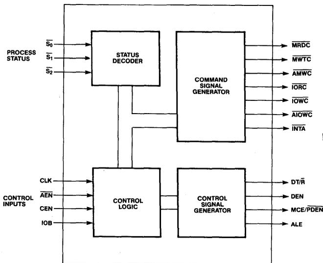
Figure 2: KS82C88 Block Diagram
