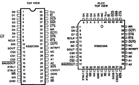
Figure 2: DIP Pin Assignments
