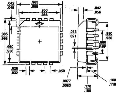
Figure 17. 68-Pin PLCC Package
