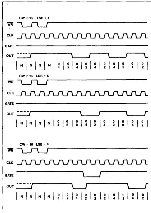
Note: A gate transition should not occur one clock cycle prior to reaching the terminal count (TC).
