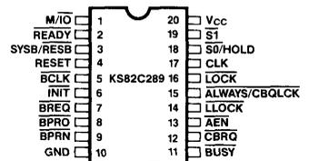
Figure 2b. KS82C289 Pin Diagram
