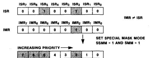
Interrupt request IR<sub>6</sub> and IR<sub>7</sub> cannot be accepted when IMR ≠ ISR, even with the Special Mask Mode set
