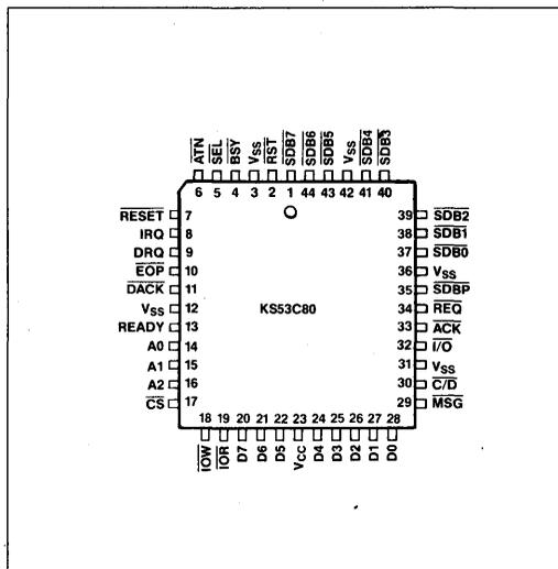
Figure 2. Physical Layout of the KS53C80 SCSI Bus Controller (PLCC Version)
