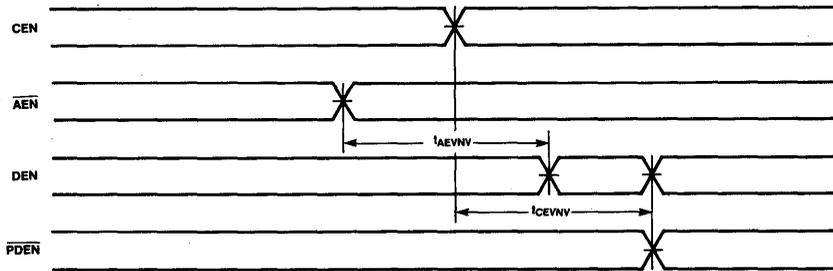
c) Address Enable Timing (3-State Enable/Disable)
