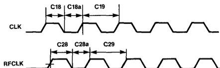
Figure 14. Internal Refresh — Interleave Access
