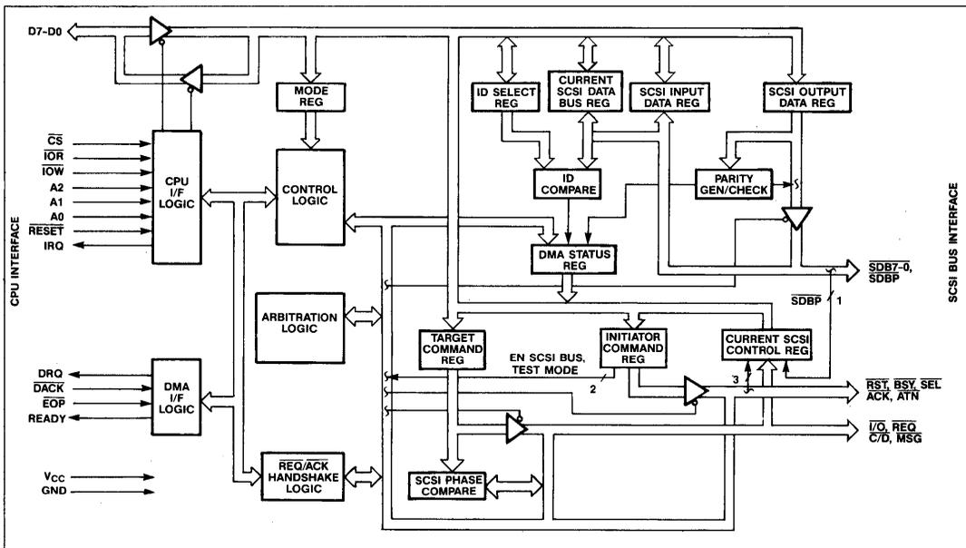
Figure 1. Functional Block Diagram of KS53C80
