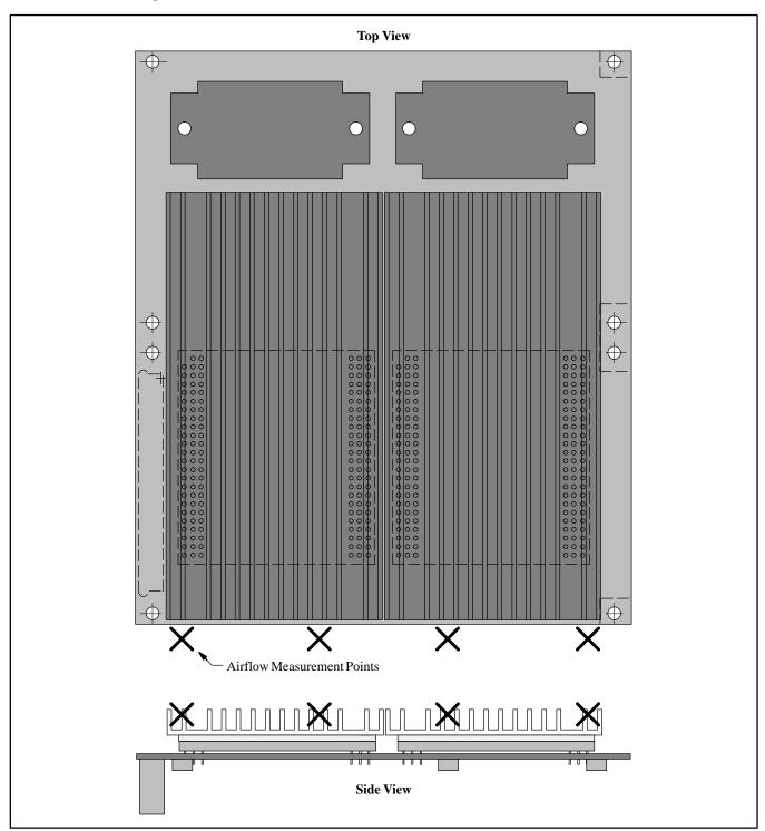
Figure 8. RT6226M Airflow Measurement
