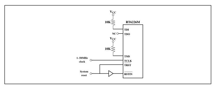
Figure 5. Scan Pin Connections
