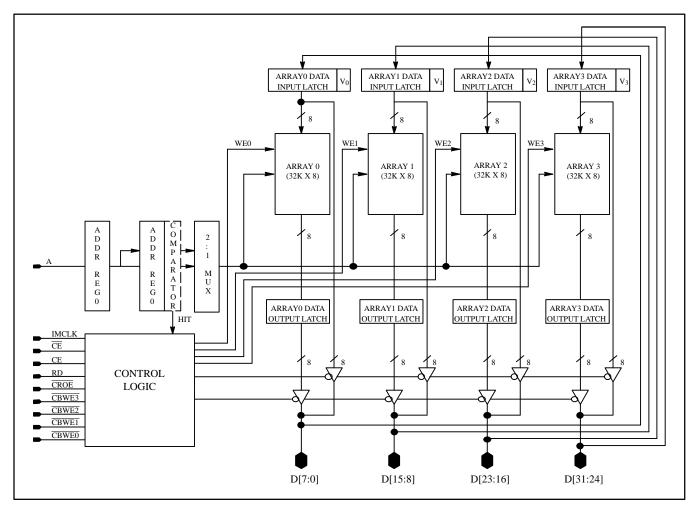
Figure 4. RT628 Block Diagram
