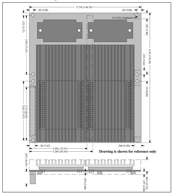
Figure 6. RT6226M Mechanical Dimensions
