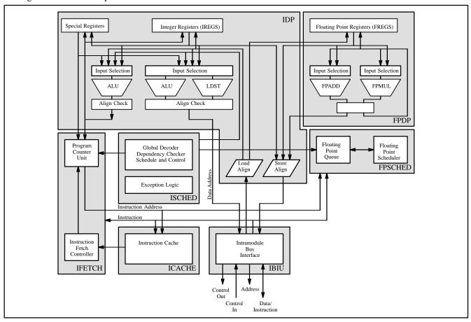
Figure 2. RT620C CPU Logic Block Diagram
