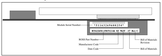
Figure 7. RT6226M Module Labeling
