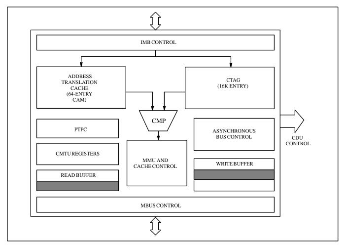
Figure 3. RT626 CMTU Block Diagram
