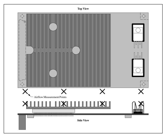
Figure 8. RT6224K Airflow Measurement
