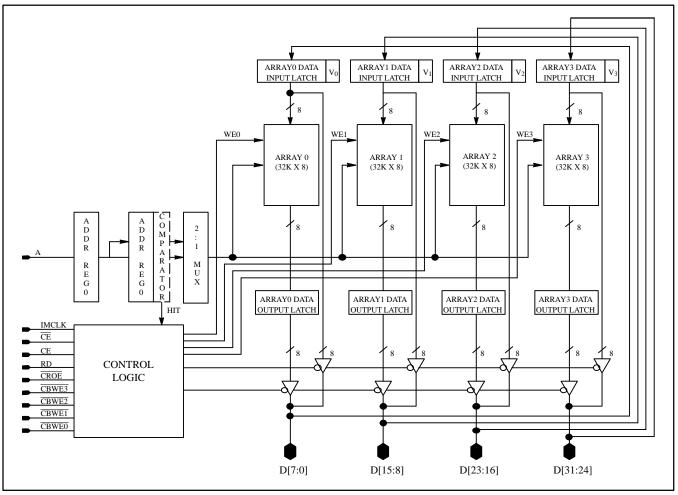
Figure 4. RT628 Block Diagram
