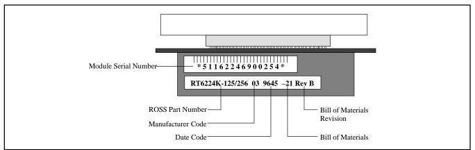
Figure 7. RT6224K Module Labeling
