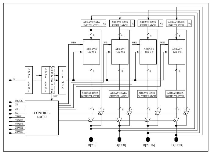
Figure 4. RT627 Block Diagram
