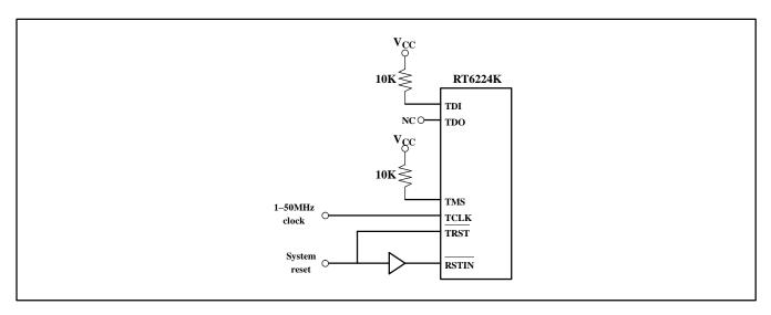
Figure 5. Scan Pin Connections
