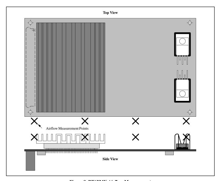
Figure 8. RT6224K Airflow Measurement
