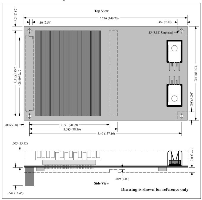
Figure 6. RT6224K Mechanical Dimensions
