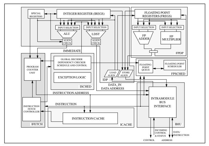
Figure 2. RT620 CPU Logic Block Diagram
