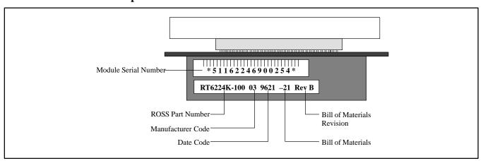
Figure 7. RT6224K Module Labeling
