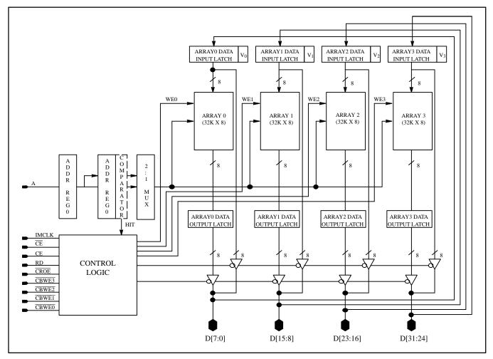
Figure 4. RT628 Block Diagram
