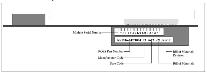
Figure 7. RS1916 Module Labeling
