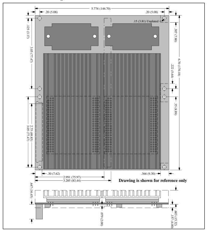
Figure 6. RS1916 Mechanical Dimensions
