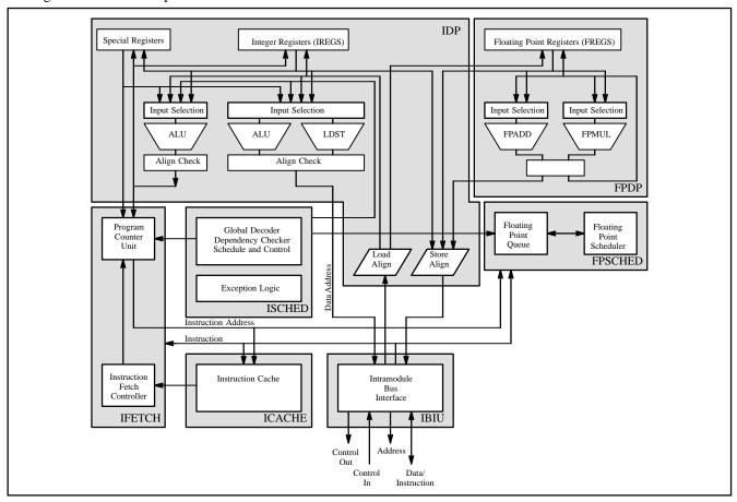
Figure 2. RT620C CPU Logic Block Diagram
