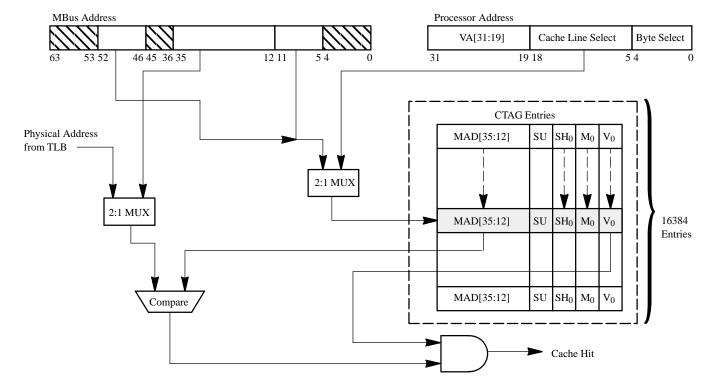
Figure 11. RT626 Cache TAG (CTAG) Comparison (512-Kbyte Cache)
