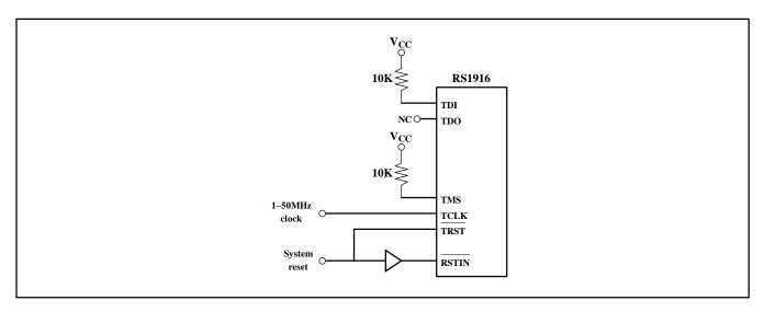
Figure 5. Scan Pin Connections
