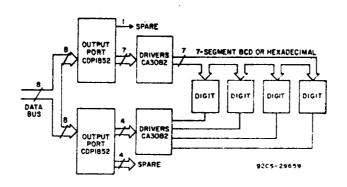
Fig. 8 - Handling segment information in software by means of an output port and lookup table.
