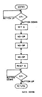
Fig. 22 - Primitive programming technique for puise generation.
