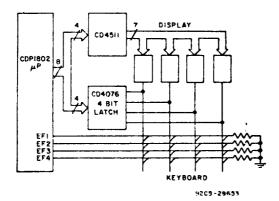
Fig. 19 - System Improvement made by combining keyboard scan and display multiplexing signals.
