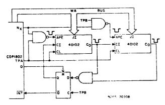
Fig. 24 - System for pulse generation using an external counter.
