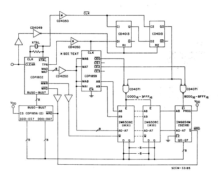
Fig. 2 - CDP1802 Synchronous RAM/ROM System
