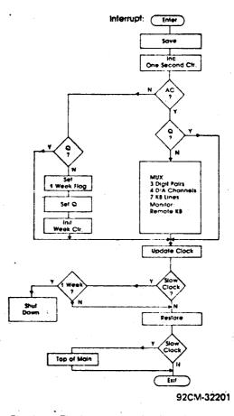
Fig. 4— The interrupt-routine flowchart. The interrupt service routine increments the seconds counter and updates the clock. It also multiplexes the display and the analog values and scans and monitors the keyboards. If ac power fails, the CPU switches to a low-frequency clock and battery power.
