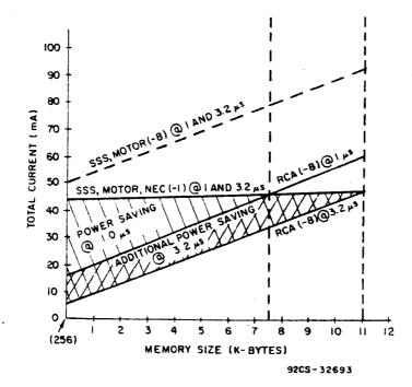
Fig. 1 - Power savings for small and medium systems (using the MWS5101EL-8).
