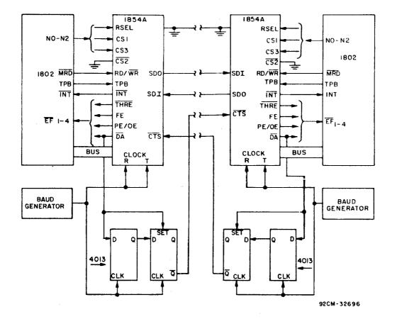
Asynchronous full duplex data communication between two independent COSMAC systems can be achieved using two 1854A UART's wired as shown. Baud rate generators must be the same frequency for both systems.
