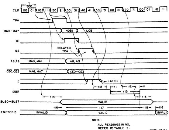
Fig. 3(b) - WRITE Timing -/60 -
