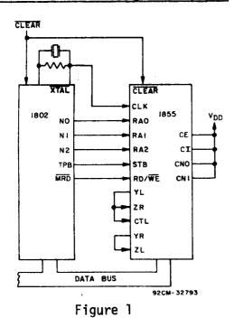
Figure 1 shows the pin connections for using the 1855 with the 1802/ 1804. A subroutine for performing an 8x8 multiply is listed in Program #2. The overhead of register initializing is about the same as in the 1st program, however, the actual 13 instruction subroutine must be executed only once since the MDU does all the shifting and adding.
