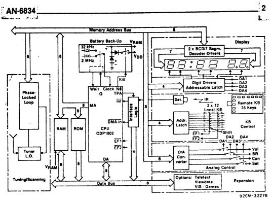
Fig. 1 — The microprocessor-control system. The user interacts with the controller by means of either the local 2 x 12 keyset or the 35-key remote unit. Clock and program information is shown on the six-digit display. Exact tuning is accomplished through the phase-locked loop. The battery backup system keeps the clock running and stored information intact in the event of a power failure.
