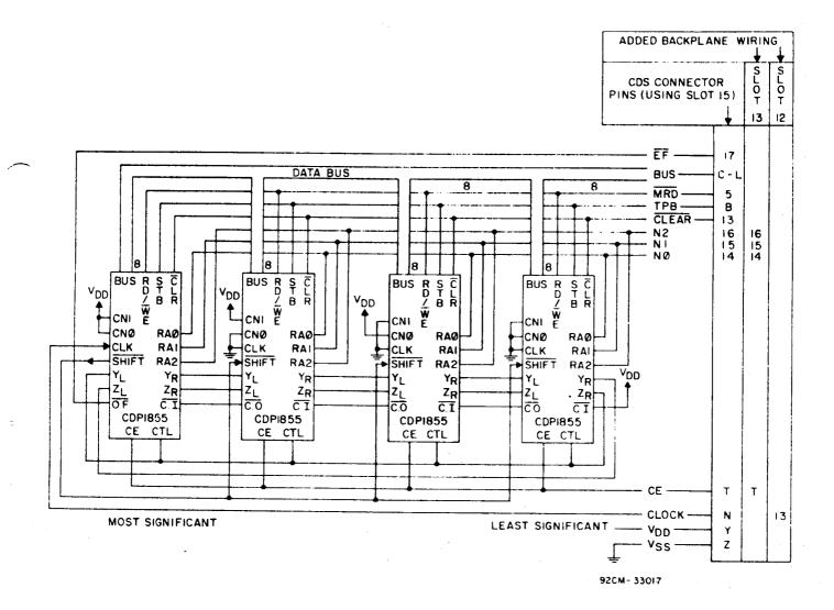
Figure 1 - Cascaded CDP1855 configuration for CDS Interface.
