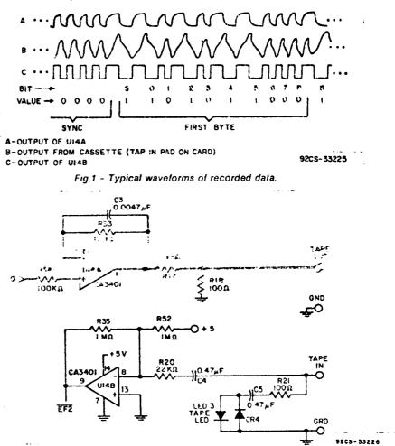
Fig.2 - Schematic diagram for COSMAC cassette tape 1/O interface.
