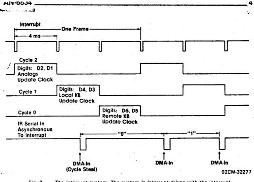
Fig. 2 — The interrupt system. The system is interrupt driven with the interrupt service routine split and time multiplexed. Remote infrared control pulses are received in real time through direct memory access without interfering with ongoing processing.
