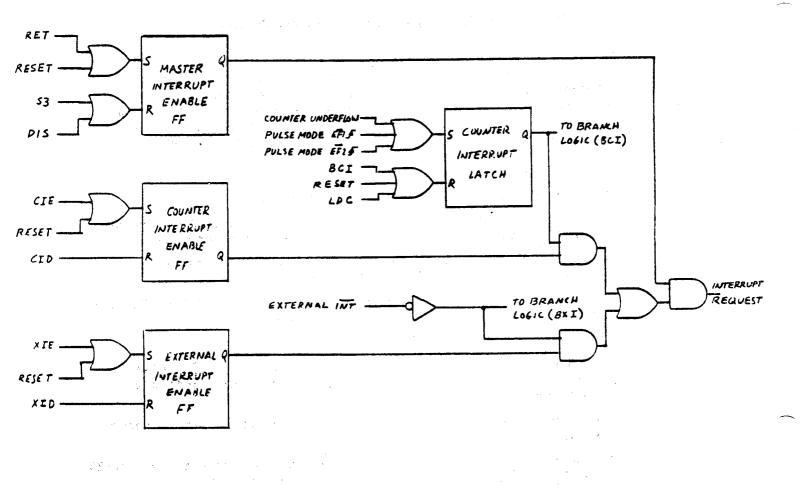
Fig. 1 - CDP1805 Interrupt Control Logic
