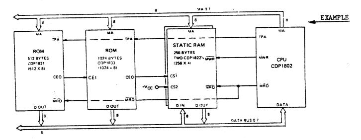
The above diagram shows a typical system with RAM and ROM memory. The customer desires memory mapping as follows:
