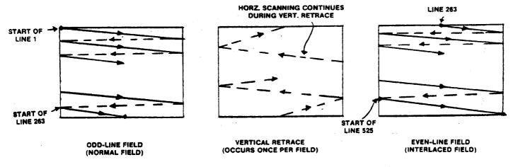
FIG. 3-2 TO 1 ODD-LINE INTERLACE SCANNING
