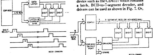
Fig. 5 - Typical multiplexed display system.
