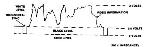
FIG. 5C-STANDARD VIDEO SIGNAL LEVELS
