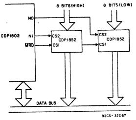
Fig. 1—Basic 16-bit Input circuit.
