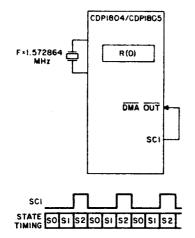
SCI FORCES DMA REQUEST EVERY THIRD MACHINE CYCLE. EACH DMA CYCLE INCREMENTS R(0). FOR FREQUENCY SHOWN, R(0) OVERFLOWS ONCE PER SECOND, WHICH CAN BE CHECKEO BY SOFTWARE.
