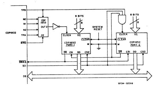
Fig. 2—Circuit for automatic input of a 16-bit value to memory.
