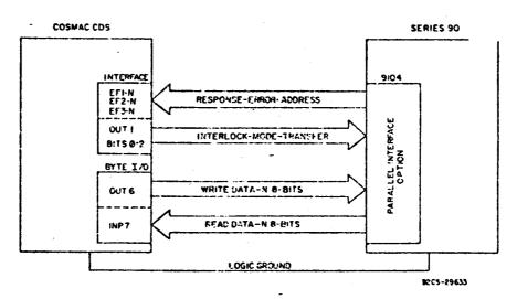
Fig. 1 - COSMAC-Series 90 block diagram.
