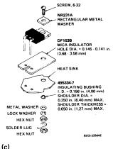
Fig. 710—Mounting arrangements for VERSAWATT transistors: (a) and (b) methods of mounting in-line-lead types; (c) chassis mounting.
