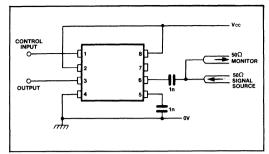
Fig.5 Toggle frequency test circuit
