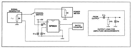
Fig.4 Test circuit
