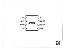
Fig.1 Pin connections - top view
