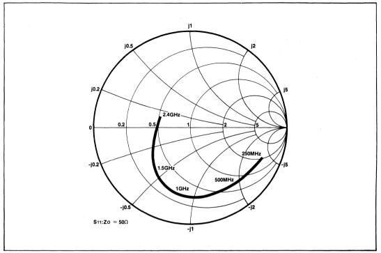
Fig.5 Typical input impedance
