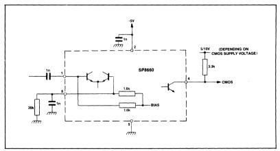
Fig.6 Typical application showing interfacing
