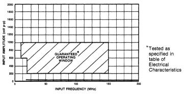
Fig.3 Typical input characteristics SP8629
