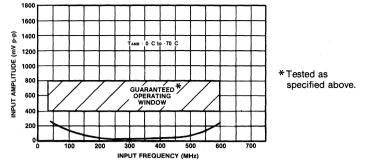
Fig.4 Typical input characteristics SP8735
