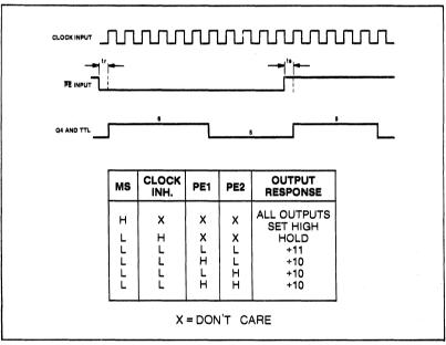
Fig.3 Truth table and timing diagram SP8680
