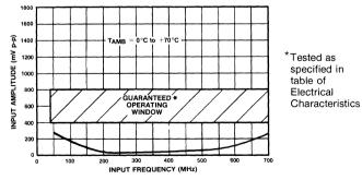
Fig.3 Typical input characteristics SP8634
