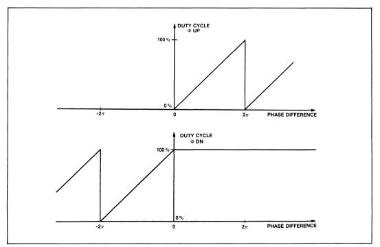
Fig.9 Phase comparator output characteristics
