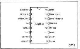
Fig.1 Pin connections (plastic DIL - top view)
