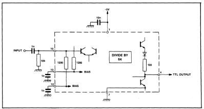
Fig.6 Typical applications circuit showing interfacing
