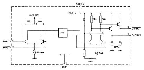
Fig.2 SP8834B block diagram
