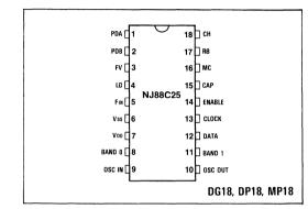
Fig.1 Pin connections - top view
