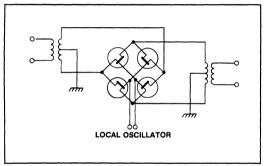
Fig.11 Quad MOSFET commutative mixer
