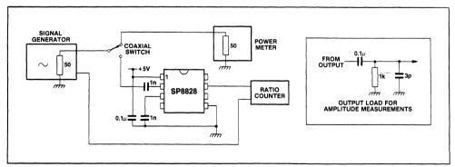
Fig.4 Test circuit
