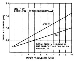
Fig.3 Typical supply current versus input frequency
