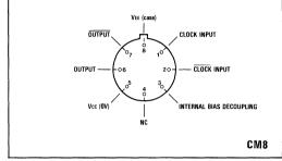
Fig.1 Pin connections - bottom view
