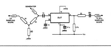
Fig.6 Test circuit
