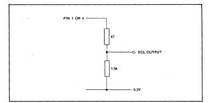
Fig.7 Interfacing to ECL 10K
