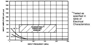
Fig.6 Typical input characteristics SP86790/1
