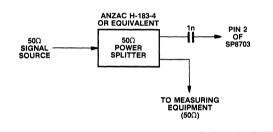
Fig.5 Input voltage measurement method
