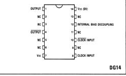
Fig.1 Pin connections - top view
