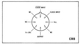
Fig.1 Pin connections - bottom view
