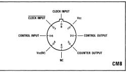
Fig.1 Pin connections - top view
