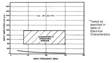
Fig.3 Typical input characteristic of SP8660A
