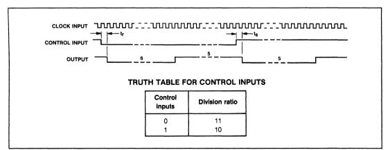
Fig.3 Timing diagram SP8799A
