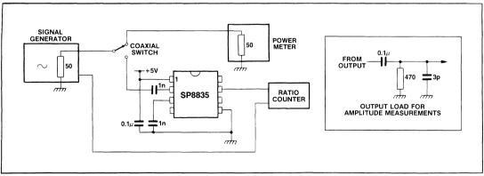
Fig.4 Test circuit
