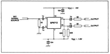
Fig.6 Operation on split supply voltages
