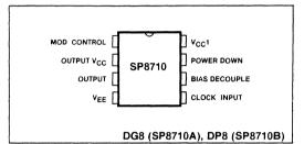
Fig.1 Pin connections - top view
