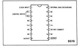
Fig.1 Pin connections - top view
