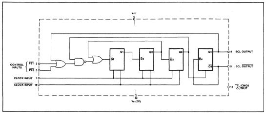
Fig.3 Functional diagram (SP8691)
