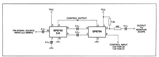
Fig.4 Test circuit
