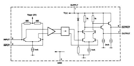
Fig.2 SP8824 block diagram
