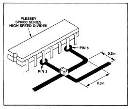
Fig.3 Coupling between parallel tracks
