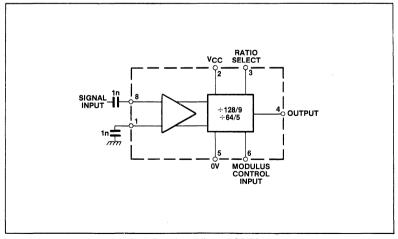
Fig.2 Functional diagram SP8704
