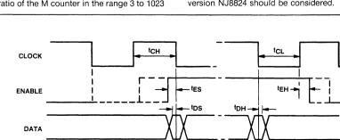
Fig.5 Timing diagram showing timing periods required for correct operation
