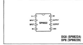
Fig.1 Pin connections - top view
