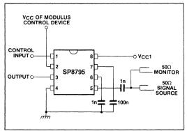
Fig.6 Toggle frequency test circuit
