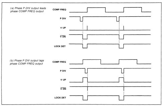
Fig.8 Phase comparator waveforms
