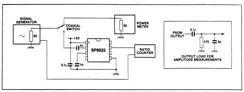
Fig.4 Test circuit
