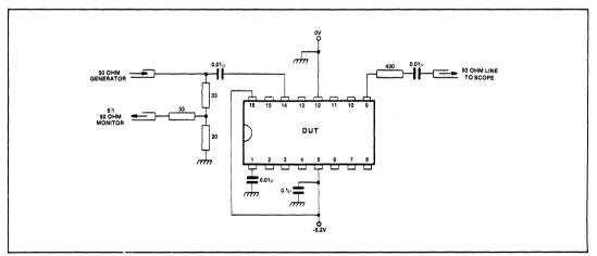
Fig.5 SP8634/5/7 high frequency test circuit
