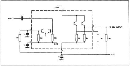
Fig.6 Typical application showing interfacing
