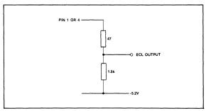
Fig.7 Interfacing to ECL 10K
