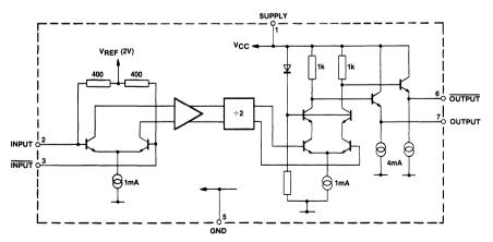
Fig.2 SP8822 block diagram
