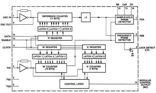
Fig.2 Block diagram. Pin numbers for MP package are shown in brackets.
