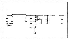
Fig.10 Transmission line VCO using a shortened  $\lambda/4$  line capacitively loaded
