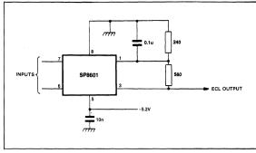
Fig.7 Interfacing to ECL
