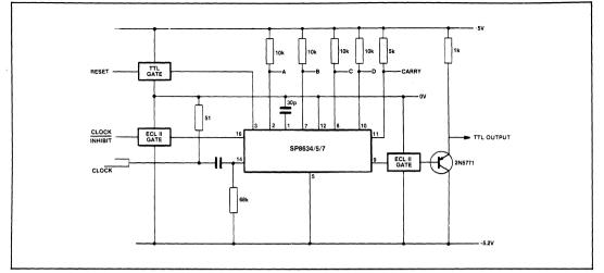
Fig.6 Typical application configuration
