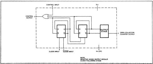
Fig.2 Functional diagram
