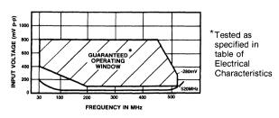
Fig.4 Typical input characteristics
