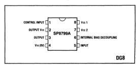
Fig.1 Pin connections - top view
