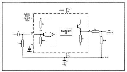
Fig.8 Typical application showing interfacing
