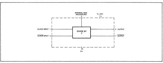
Fig.2 Functional diagram
