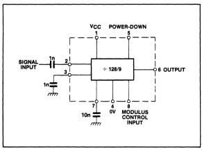
Fig.2 Functional diagram
