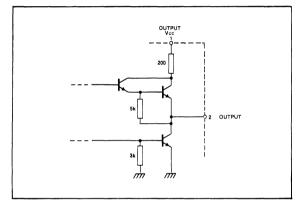
Fig.10 Output circuit diagram
