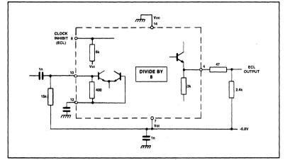
Fig.8 Typical application showing interfacing
