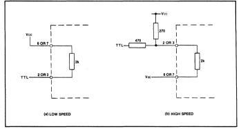
Fig.8 TTL interface to PE1 and PE2
