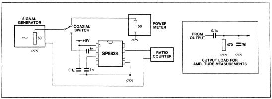
Fig.4 Test circuit
