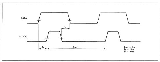
Fig.3 Clock and data timing requirements
