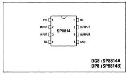
Fig.1 Pin connections - top view
