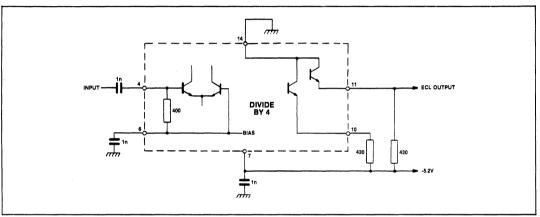
Fig.8 Typical application showing interfacing
