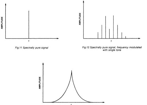
Fig.13 Spectrally pure signal, frequency modulated by noise
