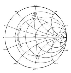
Fig.8 Series reactance to parallel admittance conversion
