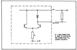
Fig.6 TTL output circuit
