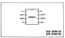
Fig.1 Pin connections - top view
