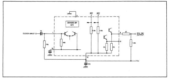
Fig.7 Typical applications circuit showing interfacing
