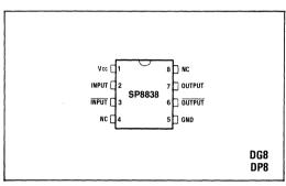
Fig.1 Pin connections - top view
