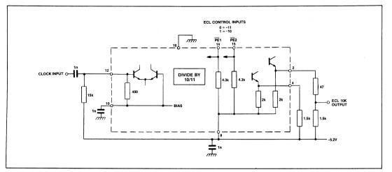
Fig.7 Typical application showing interfacing
