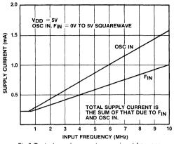
Fig.3 Typical supply current versus input frequency
