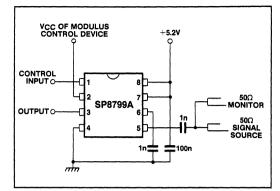
Fig.6 Toggle frequency test circuit
