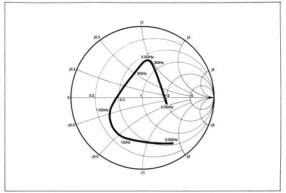
Fig.5 Typical input impedance
