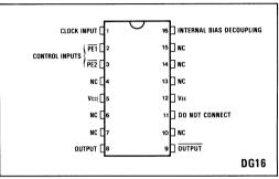
Fig.1 Pin connections - top view
