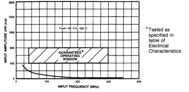
Fig.4 Typical input characteristics SP8720A
