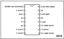
Fig.1 Pin connections - top view
