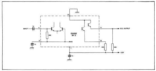
Fig.8 Typical application showing interfacing
