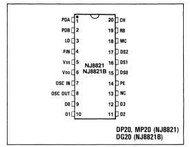
Fig.1 Pin connections
