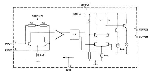
Fig.2 SP8818 block diagram
