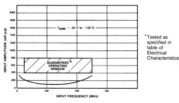
Fig.3 Typical input characteristics of SP8600A
