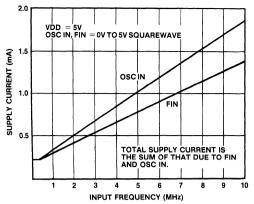
Fig.3 Typical supply current versus input frequency
