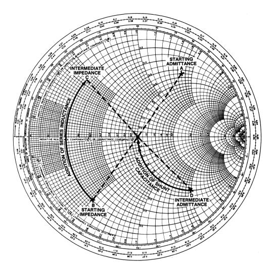
Fig.10 Matching design using the Smith Chart
