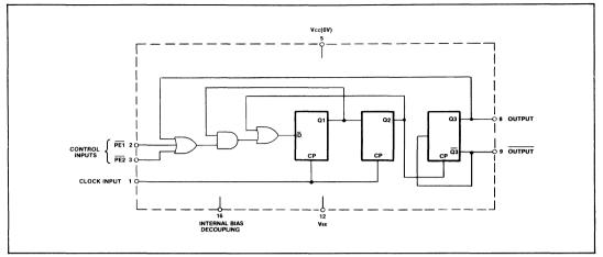
Fig.3 Functional diagram (SP8741)
