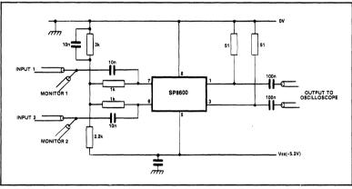
Fig.5 Test circuit
