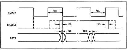
Fig.5 Timing diagram showing timing periods required for correct operation
