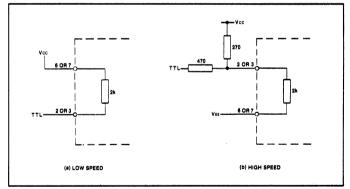
Fig.9 TTL interface to PE1 and PE2
