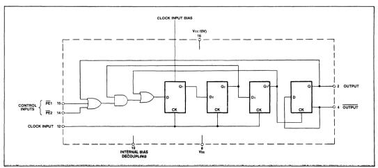
Fig.2 Functional diagram
