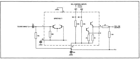
Fig.9 Typical applications circuit showing interfacing
