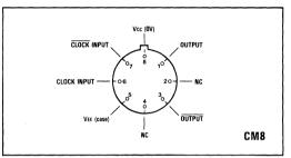
Fig.1 Pin connections - bottom view
