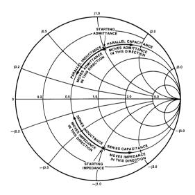
Fig.9 Effects of series and shunt reactance
