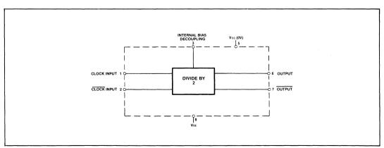
Fig.2 Functional diagram
