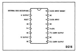
Fig.1 Pin connections - top view
