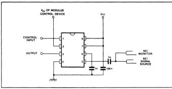
Fig.6 Toggle frequency test circuit
