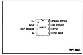
Fig.1 Pin connections - top view
