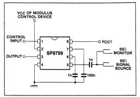
Fig.6 Toggle frequency test circuit
