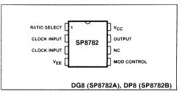
Fig.1 Pin connections - top view
