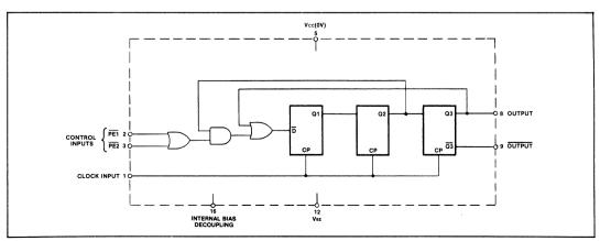
Fig.2 Functional diagram (SP8740)
