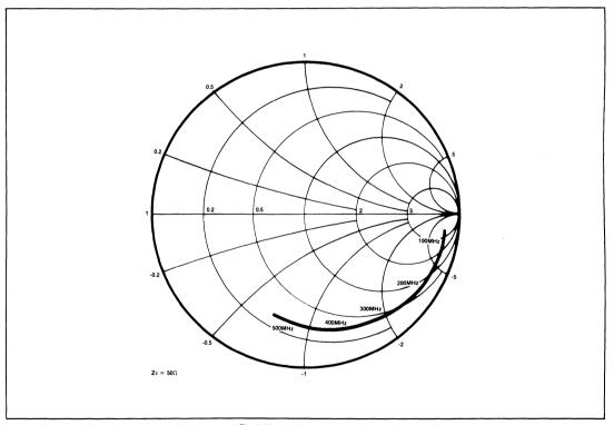
Fig.6 Typical input impedance
