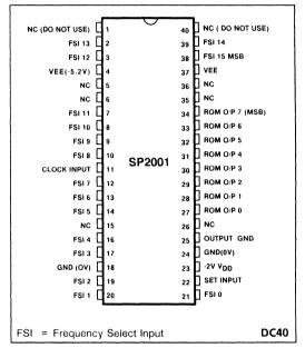
Fig.1 Pin connections - top view
