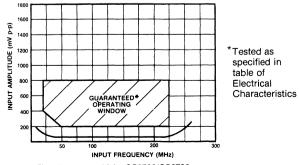
Fig.4 Input sensitivity SP8792/SP8793
