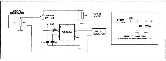
Fig.4 Test circuit
