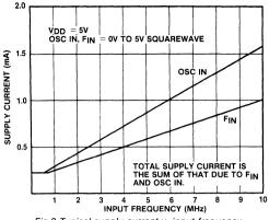
Fig.3 Typical supply current v. input frequency
