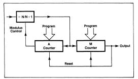
Fig.5 Two modulus divider
