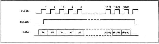
Fig.6 Timing diagram showing programming details
