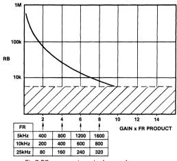
Fig.7 RB versus gain and reference frequency
