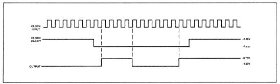
Fig.4 Timing diagram (N.B. output waveform is asymmetric)
