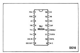
Fig.1 Pin connections - top view, not to scale
