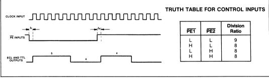
Fig.5 Timing diagram SP8691
