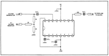
Fig.8 SP8735 high frequency test circuit
