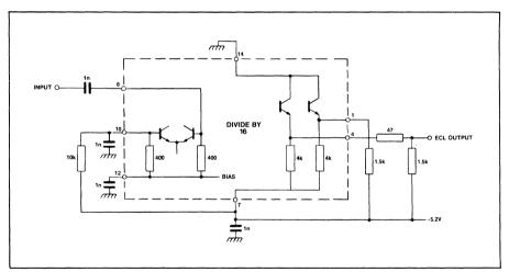
Fig.6 Typical application showing interfacing
