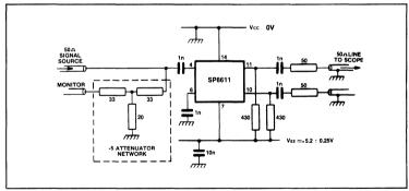
Fig.5 Toggle frequency test circuit
