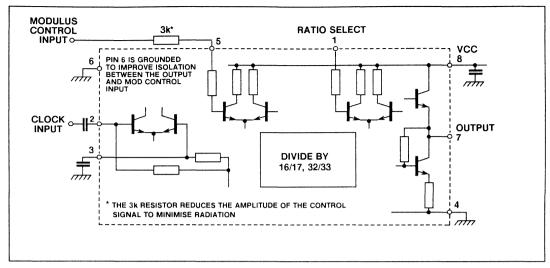
Fig.3 Typical applications showing interfacing
