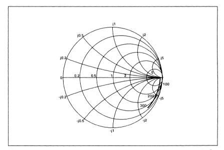
Fig.4 Typical Input Impedance. Test conditions:supply voltage 5V, ambient temperature 25°C, frequencies in MHz, impedances normalised to 50 Ohms
