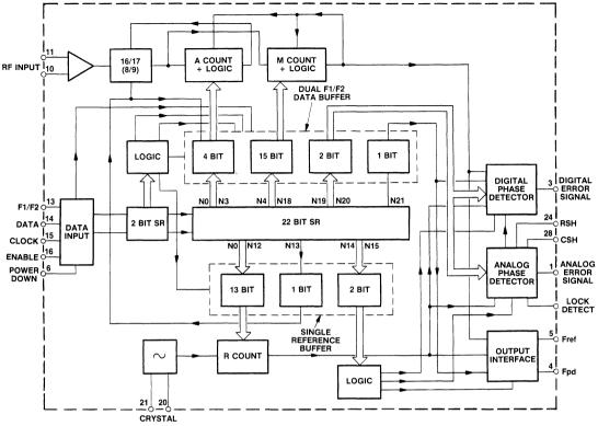
Fig.2 SP8850 block diagram
