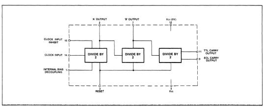
Fig.2 Functional diagram
