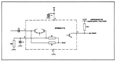
Fig.6 Typical application showing interfacing
