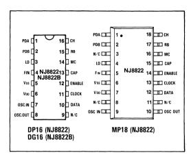
Fig. I Pin connections - top view, not to scale
