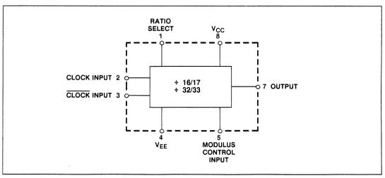
Fig.2 SP8782 functional diagram
