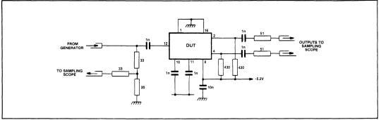
Fig.6 Toggle frequency test circuit
