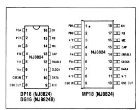
Fig. I Pin connections - top view, not to scale
