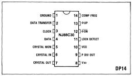
Fig.1 Pin connections (plastic DIL - top view)
