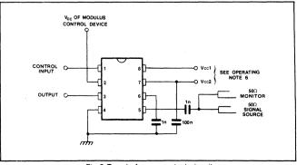
Fig.6 Toggle frequency test circuit
