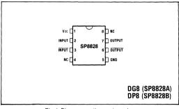
Fig.1 Pin connections - top view
