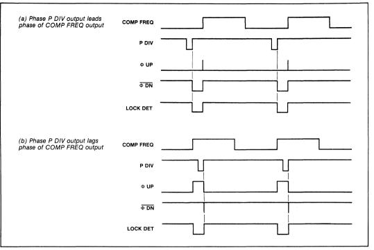
Fig.8 Phase comparator waveforms
