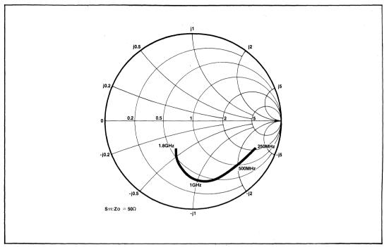
Fig.5 Typical input impedance
