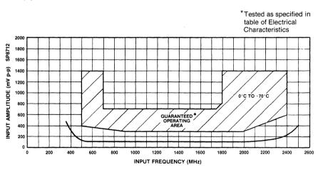
Fig.3 Typical input characteristics SP8712
