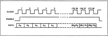
Fig.6 Timing diagram showing programming details
