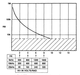
Fig.8 RB versus gain and reference frequency
