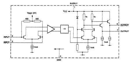
Fig.2 SP8828 block diagram
