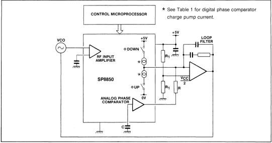
Fig.4 Typical application diagram
