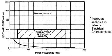
Fig.6 Typical input characteristics SP8740/1A
