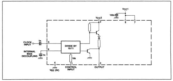
Fig.2 Function diagram SP8799A
