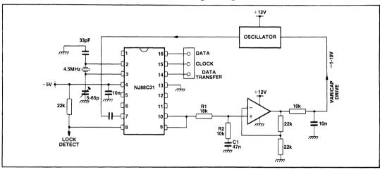
Fig.10 Typical application for DP16 device
