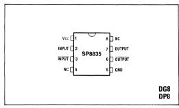
Fig.1 Pin connections - top view
