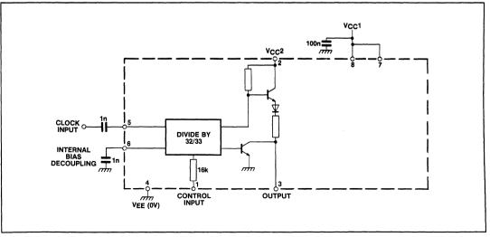
Fig.2 Function diagram SP8795A
