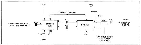
Fig.4 Test circuit
