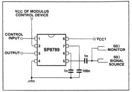
Fig.6 Toggle frequency test circuit
