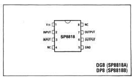
Fig.1 Pin connections - top view
