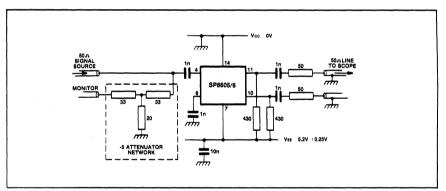
Fig.5 Toggle frequency test circuit
