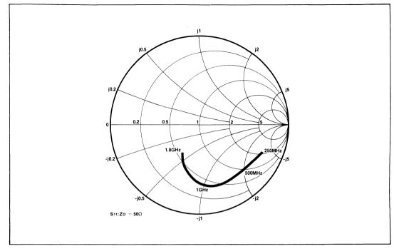
Fig.5 Typical input impedance
