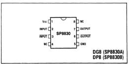
Fig.1 Pin connections - top view
