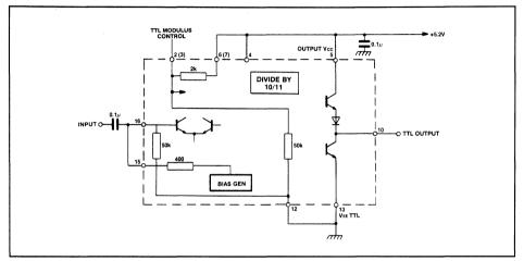
Fig.7 Typical application showing interfacing
