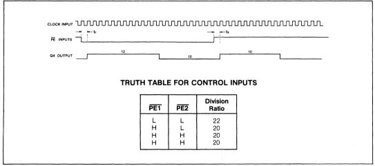
Fig.3 Timing diagram
