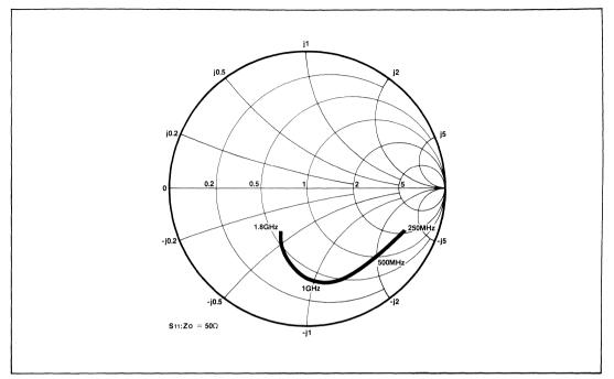
Fig.5 Typical input impedance
