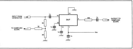
Fig.5 Test circuit
