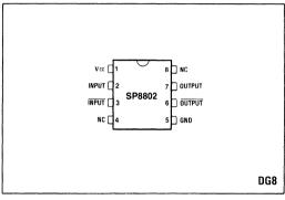
Fig.1 Pin connections - top view
