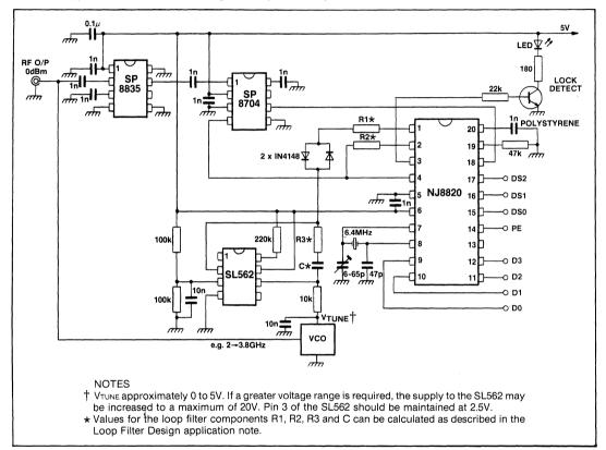
Fig.2 3.5GHz synthesiser using SP8835, SP8703, NJ8820 and SL562
