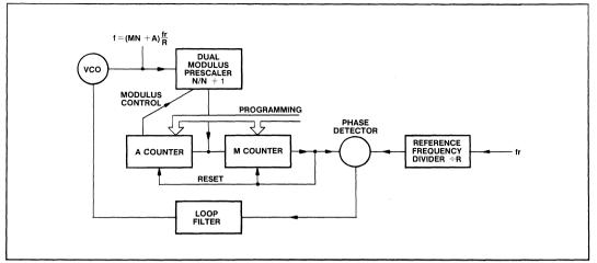
Fig.7 Dual modulus prescaling
