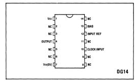
Fig.1 Pin connections - top view
