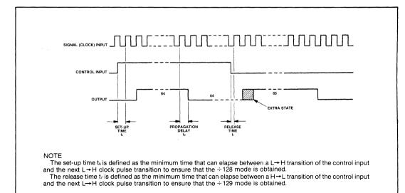
Fig.3 Timing diagram
