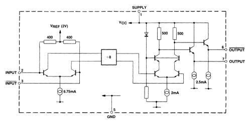
Fig.2 SP8838B block diagram
