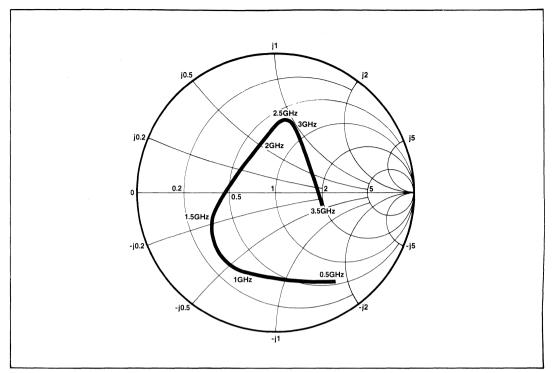
Fig.5 Typical input impedance
