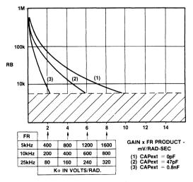
Fig.8 RB v. gain and reference frequency
