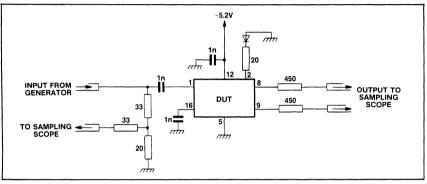
Fig.8 Test circuit
