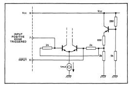
Fig.9 Input circuit diagram
