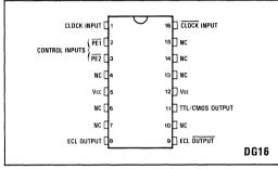
Fig.1 Pin connections - top view
