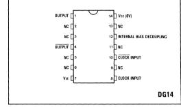
Fig.1 Pin connections - top view
