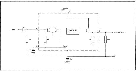
Fig.6 Typical application showing interfacing
