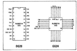
Fig.1 Pin connections
