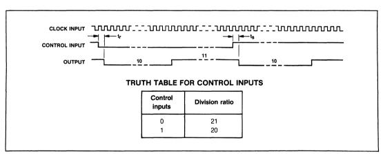
Fig.3 Timing diagram SP8789A
