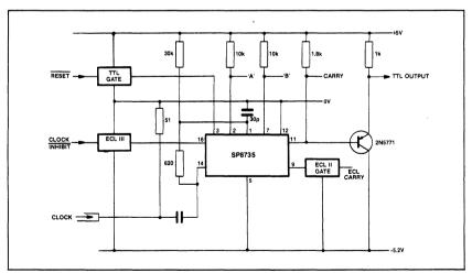
Fig.9 Typical application showing interfacing
