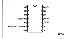
Fig.1 Pin connections - top view
