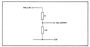
Fig.8 Interfacing to ECL 10K
