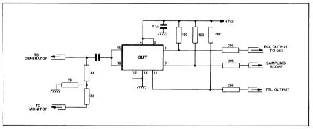
Fig.5 Test circuit
