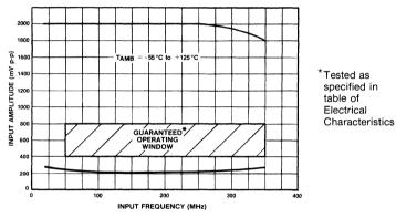
Fig.3 Typical input characteristic of SP8643A
