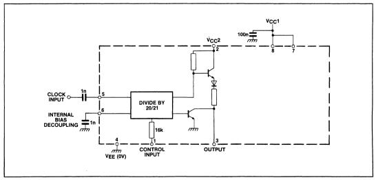
Fig.2 Function diagram SP8789A
