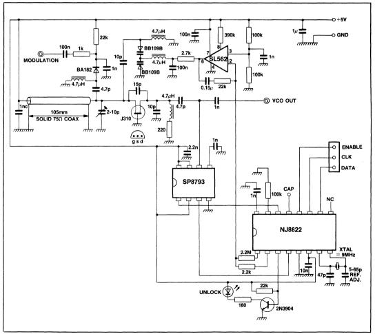
Fig.1 NJ8822 serially programmable VHF synthesiser
