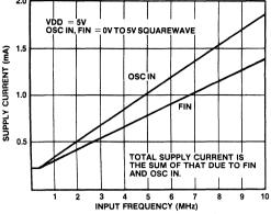
Fig.3 Typical supply current versus input frequency
