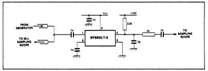
Fig.5 Test circuit
