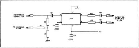
Fig.5 Test circuit
