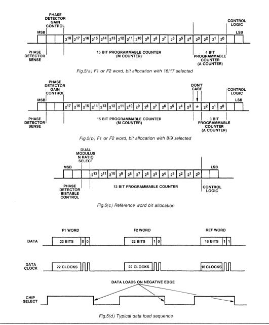
Fig.5 Data format diagrams
