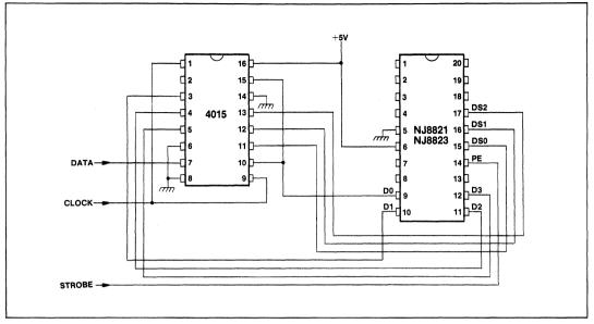
Fig.11 NJ8821/23 serial mode connections
