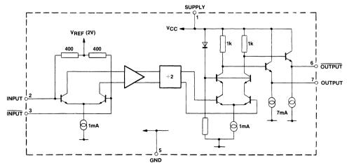
Fig.2 SP8812 block diagram
