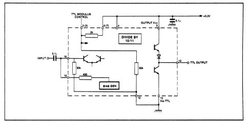
Fig.8 Typical application showing interfacing
