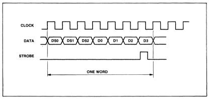
Fig.12 Serial data timing
