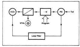
Fig.4 Mixing in the loop
