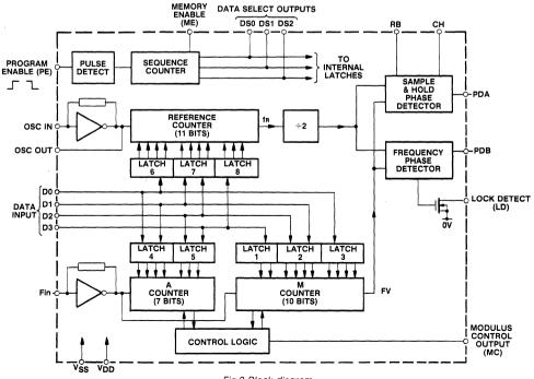
Fig.2 Block diagram
