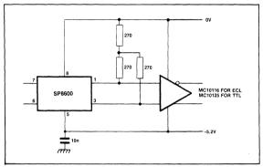
Fig.7 Interfacing to ECL and Schottky TTL
