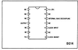
Fig.1 Pin connections - top view
