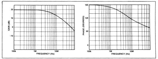
Fig.6 Gain phase characteristics of reference oscillator inverter
