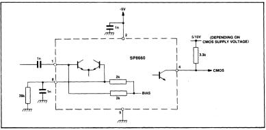
Fig.6 Typical application showing interfacing
