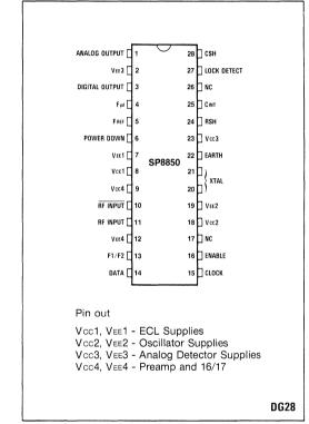
Fig.1 Pin connections - top view
