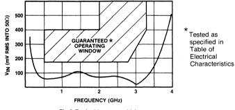
Fig.3 Typical input sensitivity
