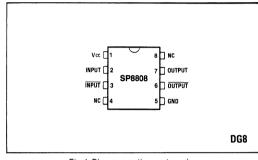
Fig.1 Pin connections - top view
