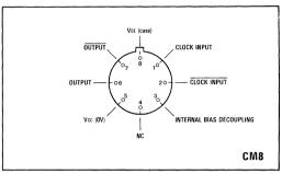
Fig.1 Pin connections - bottom view
