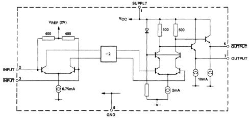
Fig.2 SP8802A block diagram
