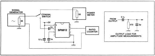
Fig.4 Test circuit
