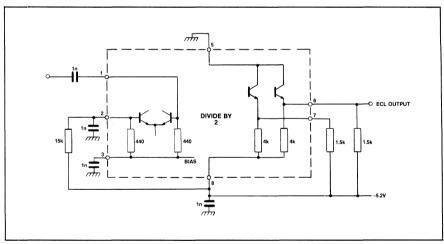
Fig.6 Typical application showing interfacing
