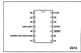
Fig.1 Pin connections - top view
