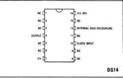
Fig.1 Pin connections - top view
