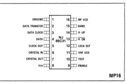
Fig.2 Pin connections (miniature plastic DIL - top view)
