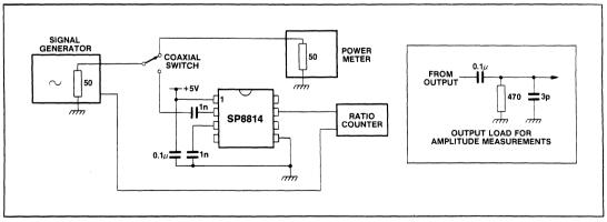
Fig.4 Test circuit
