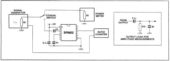
Fig.4 Test circuit
