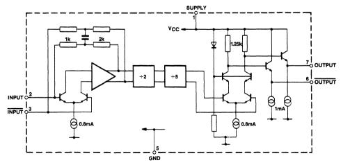
Fig.2 SP8830 block diagram
