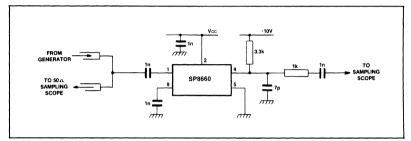
Fig.5 Test circuit
