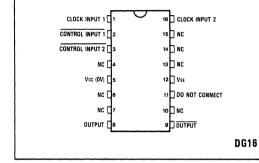
Fig.1 Pin connections - top view
