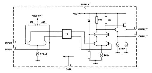
Fig.2 SP8808A block diagram
