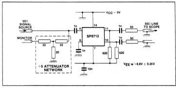
Fig.5 Toggle frequency test circuit
