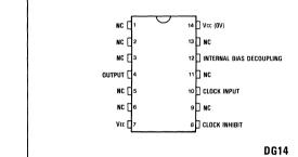
Fig.1 Pin connections - top view
