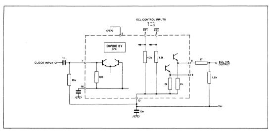
Fig.7 Typical applications circuit showing interfacing
