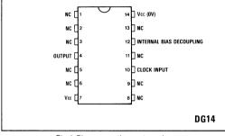
Fig.1 Pin connections - top view
