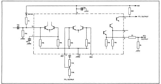
Fig.9 Typical application showing interfacing
