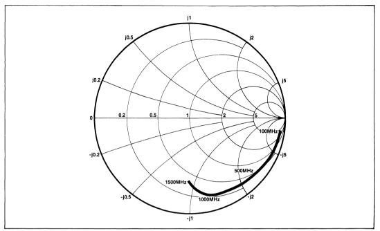
Fig.5 Typical input impedance
