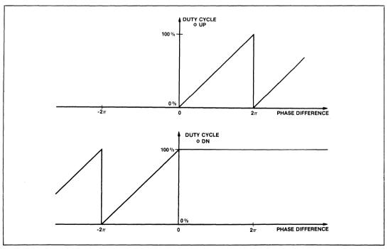
Fig.9 Phase comparator output characteristics
