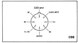
Fig.1 Pin connections - bottom view
