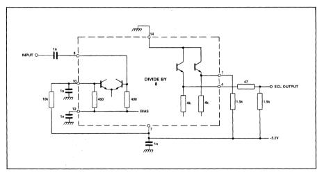
Fig.6 Typical application showing interfacing
