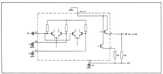
Fig.7 Typical application circuit showing interfacing
