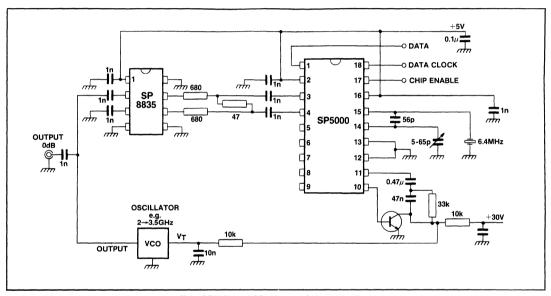
Fig.1 SP8835 and SP5000 - 3.5GHz synthesiser
