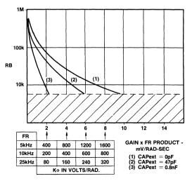
Fig.8 RB v. gain and reference frequency
