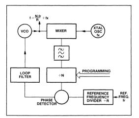
Fig.6 Mixing in the loop
