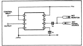
Fig.5 Toggle frequency test circuit
