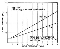
Fig.3 Typical supply current v. input frequency
