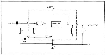
Fig.6 Typical application showing interfacing
