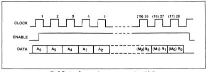
Fig.6 Timing diagram showing programming details
