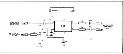
Fig.6 Test circuit
