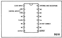
Fig.1 Pin connections - top view
