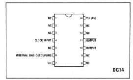
Fig.1 Pin connections - top view
