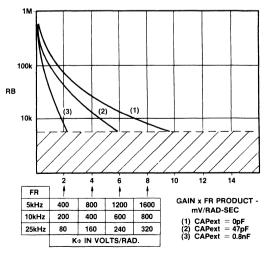
Fig.8 RB v. gain and reference frequency
