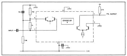
Fig.6 Typical application showing interfacing
