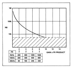
Fig.9 RB versus gain and reference frequency
