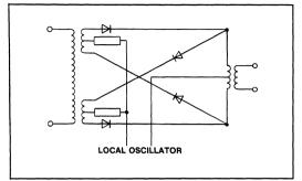
Fig.10 Resistive loaded high intercept point mixer
