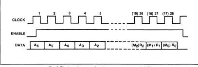
Fig.6 Timing diagram showing programming details
