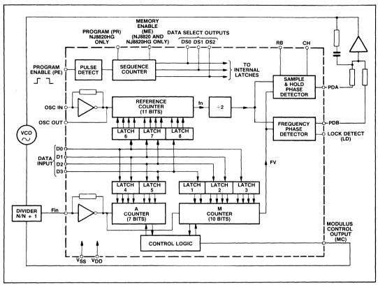
Fig.8 The phase lock loop
