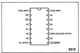
Fig.1 Pin connections - top view
