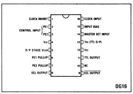
Fig.1 Pin connections - top view
