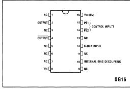
Fig.1 Pin connections - top view
