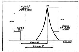
Fig.1 Phase noise and adjacent channel rejection
