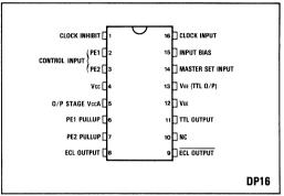
Fig.1 Pin connections - top view
