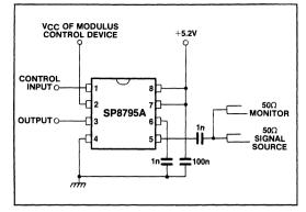
Fig.6 Toggle frequency test circuit
