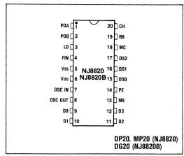
Fig.1 Pin connections
