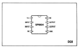
Fig.1 Pin connections - top view
