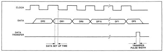
Fig.5 Input data timing diagram
