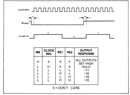
Fig.4 Truth table and timing diagram SP8680
