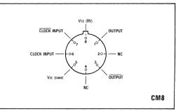
Fig.1 Pin connections - bottom view
