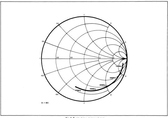
Fig.6 Typical input impedance
