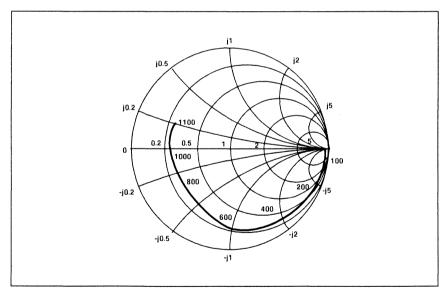
Fig.4 Typical input Impedance. Test conditions: supply voltage 5V, ambient temperature 25°C, frequencies in MHz, impedancies normalised to 50 Ohms
