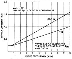
Fig.3 Typical supply current versus input frequency
