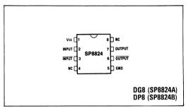
Fig.1 Pin connections - top view
