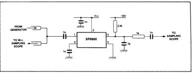
Fig.5 Test circuit
