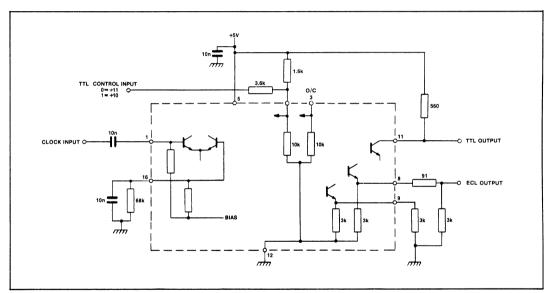
Fig.9 Typical applications circuit showing interfacing
