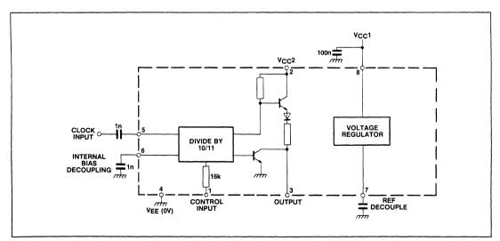
Fig.2 Functional diagram SP8799
