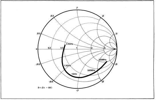
Fig.5 Typical input impedance
