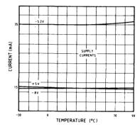
Fig. 7/ Supply current variation with temperature
