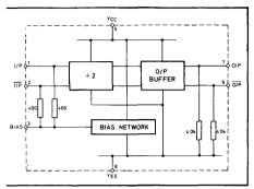
Fig. 2 SP8607 block diagram
