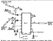
k Only one generator should be connected to either the VHF or UHF inputs. The input not in use may be left open circuit. All capacitors are 1nF unless otherwise stated.
