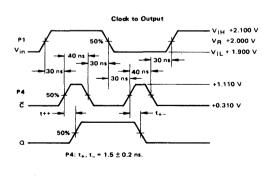
FIGURE 3 – PROPAGATION DELAY  $(\tau_{\mathbf{pd}})$  versus INPUT PULSE AMPLITUDE AND CONSTANT OVERDRIVE
