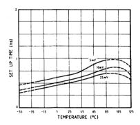
Fig. 9 Set-up time as a function of temperature
