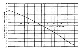
Fig. 6 Crystal frequency v. supply voltage
