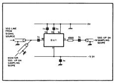
Fig. 4 Test circuit
