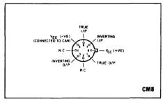
Fig. 1 Pin connections (bottom view)
