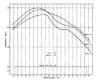
Fig. 5 Maximum input frequency v. temperature
