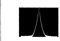
B.W. = 10 kHz Scan Width - 50 kHz/div Center Frequency = 100 MHz Vertical Scale = 10 dB/div
