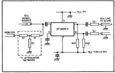
Fig. 3 Toggle frequency test circuit
