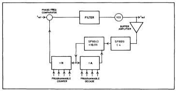
Fig. 6 A 1.5GHz synthesiser loop
