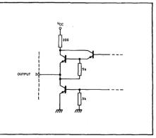
Fig. 7 Output circuit diagram
