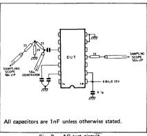
Fig. 3 - AC test circuit
