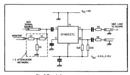
Fig. 3 Toggle frequency test circuit
