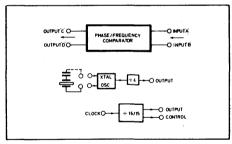
Fig. 2 SP8760 block diagram
