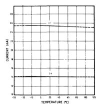
Fig. 15 Supply current as a function of temperature
