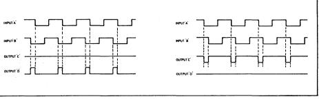
Fig. 3 Phase/frequency comparator waveforms
