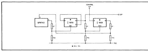
Fig.7 A  $\div$  32/33 application. Control loop delay time approx. 56ns.
