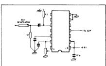
Capacitors are 1 nf unless otherwise stated. Values should be increased if operation below 10 MHz is desired.
