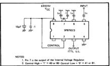
Fig. 3 - SP8792/3 Application Diagram
