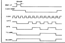
Fig.6 Output waveforms
