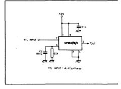
Fig. 3 High frequency, single-ended input
