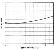
Fig. 7e Input to 10 output delay as a function ot temperature
