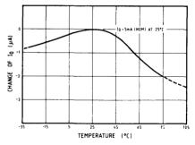
Fig. 7M Analogue output current variation with temperature
