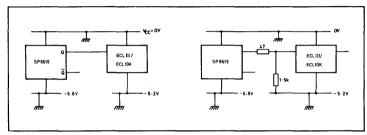
Fig. 5 Interfacing SP8619 series to ECL 10K and ECL III
