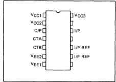
Fig. 1 - Pin Configuration
