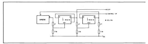
Fig. 6 Divide by 6/8 Control loop delay time approximately 20ns at 300MHz I/P frequency
