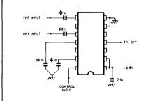
\*Connections to these pins should be made to have the minimum series inductance. Capacitors should be of a type suitable for use at 1GHz.
