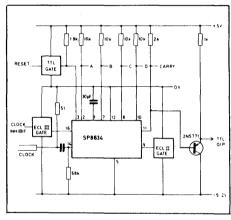
Fig. 5 Typical application configuration
