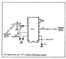
Fig. 3 - AC test circuit
