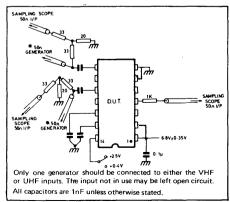
Fig. 3 AC test circuit
