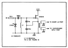
Fig. 18 Voltage controlled oscillator for 27MHz CB synthesiser
