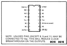
Fig. 1 Pin connections
