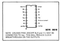
Fig. 1 Pin connections
