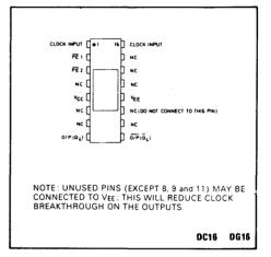
Fig. 1 Pin connections (top)
