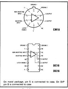
Fig. 1 Pin connections
