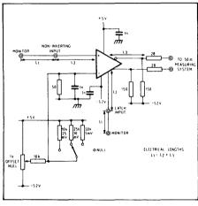
Fig. 4 SP9685/9687 test circuit
