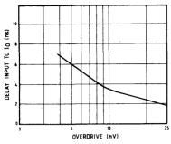
Fig. 7a input to 10 output delay v. overdrive
