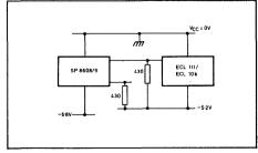
Fig. 5 Interfacing SP8608/9 series to ECL 10K and ECL III
