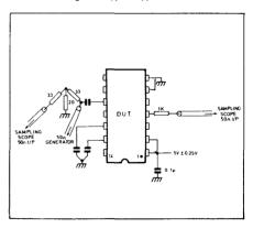
Fig. 3 - AC test circuit
