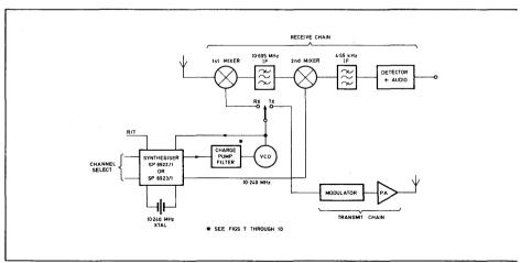
Fig. 4 Double conversion transceiver
