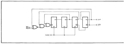
Fig. 2 SP8743 logic diagram
