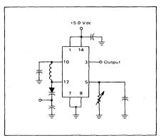
Figure 12 shows the SP1648 operating from +5.0 Vdc and +9.0 Vdc power supplies. This permits a higher voltage swing and higher output power than is possible from the PECL output (pin 3). Plots of output power versus total collector load resistance at pin 1 are given in Figures 13 and 14 for 100 MHz and 10 MHz operation. The total collector load includes R in parallel with Rp of L1 and C1 at resonance. The optimum value for R at 100 MHz is approximately 850 ohms.
