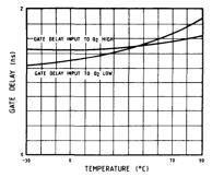
Fig. 7i Gate input to Q1 - Q4 delay variation with temperature
