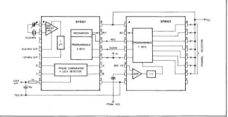
Fig. 2 SP8921/SP8922 interconnections (10.695MHz receive offset)
