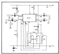
Fig. 5 Test circuit for dynamic measurements
