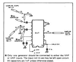
Fig. 3 AC test circuit
