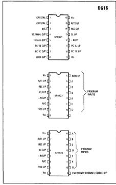
Fig. 1 Pin connections (top view)
