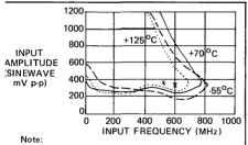
The above graphs are with the TTL output connected. Sensitivity in the 300 to 500 MHz frequency range is improved by 100mV peak to peak when pin 13 is disconnected.
