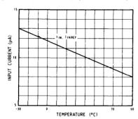
Fig. 7k Input current variation with temperature
