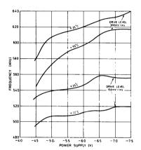
Fig. 6 Max. operating frequency v. power supply voltage for a typical SP8630B
