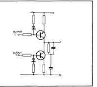
Fig. 5 Low voltage charge pump and filter
