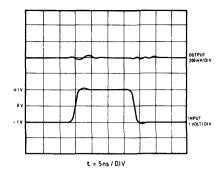
Fig. 18 Common mode pulse response
