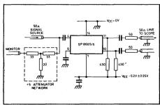
Fig. 3 Toggle frequency test circuit
