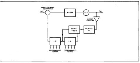
Fig.6 A 1.5GHz synthesiser loop
