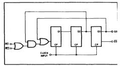
Fig. 2 Logic diagram SP8740
