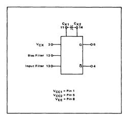
The SP1658 is a voltage-controlled multivibrator which provides appropriate level shifting to produce an output compatible with PECL. III and PECL. 10,000 logic levels. Frequency control is accomplished through the use of voltage-variable current sources which control the slew rate of a single external capacitor.
