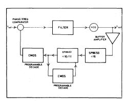
Fig. 5 A low power synthesiser loop
