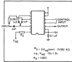
Fig. 6. - Application Circuit
