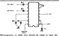
minimum series inductance. Capacitors should be of a type suitable for use at 1GHz.
