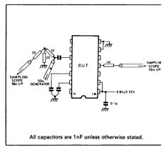
Fig. 2 AC test circuit
