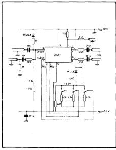
Fig. 5 Test circuit for dynamic measurements
