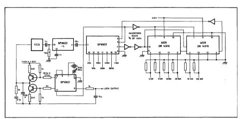
Fig. 19 200 MHz general purpose binary programmed synthesiser with 25KHz resolution using SP8921/22
