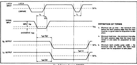
Fig. 3 Timing diagram SP9750
