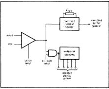
Fig. 2 Block diagram of SP9750
