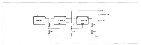
Fig. 6 Divide by 10/12. Control loop delay time approximately 33 ns
