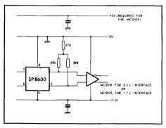
Fig. 7 ECL and Schottky TTL interfacing
