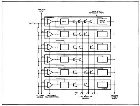
Fig. 6 Block diagram of 4-bit LSB stage showing top six levels
