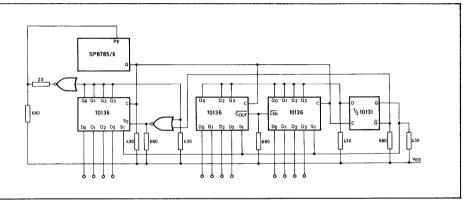
Fig. 7 1.3 GHz variable divider (200-2000 in steps of 2)
