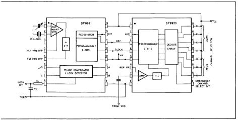
Fig. 3 SP8921/SP8923 interconnections (10.695MHz receive offset)
