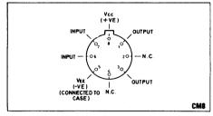
Fig. 1 Pin connections (bottom view)
