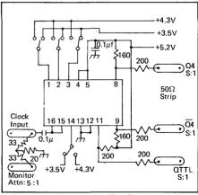
Fig. 5 - Dynamic Test Circuit
