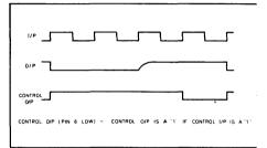
Fig. 4 SP8790 waveforms
