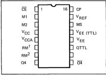
Fig. 1 - Pin Connections (Top View)
