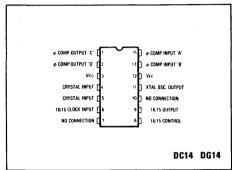
Fig. 1 Pin connections
