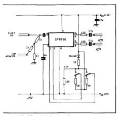
Fig.5 Test circuit for dynamic measurements
