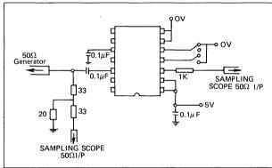
Fig. 5 - Test Circuit
