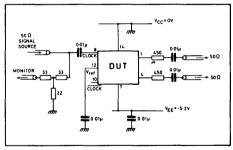
Fig. 3 Toggle frequency test circuit
