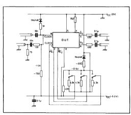
Fig. 5 Test circuit for dynamic measurements
