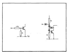
Fig. 4 Phase comp./divider control inputs
