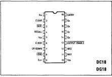
Fig. 1 Pin connections (top)
