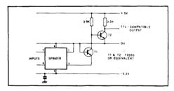
Fig. 10 High fanout TTL interface
