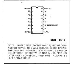
Fig. 1 Pin connections (top)
