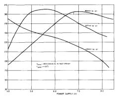
Fig. 5 Maximum frequency v. power supply voltage at single input drive levels of 400, 600 and 800 mV (typical device)
