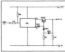
Fig. 7 TTL to ECL and ECL/TTL interfaces (for SP8725 device and TTL operating from the same supply rails)
