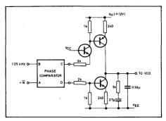
Fig. 10 Filter D. Current pump output voltage range  $V_H - 1.5V$  for  $V_H$  greater than 12V
