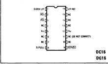
Fig. 1 Pin connections (top view)
