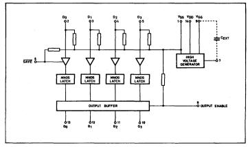
Fig. 2 Block diagram of MN9102
