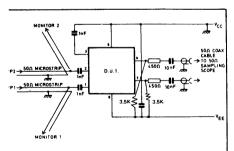
Note: The values of the coupling and decoupling capacitors used are uncritical but they should be of a type and value suitable for the frequencies involved.
