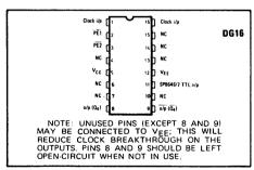
Fig. 1 Pin connections (top)
