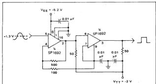
FIGURE 4 - 200 MHz SCHMITT TRIGGER
