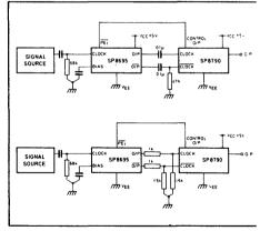
Fig. 6 Methods of preventing self-oscillation
