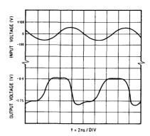
Fig. 7j Response to 100MHz sine wave
