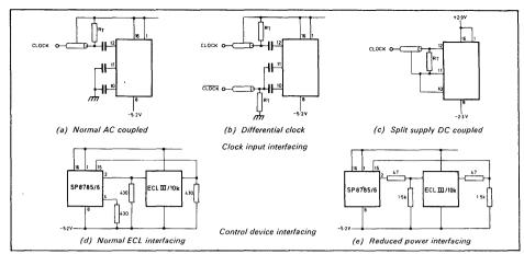
Fig. 3 Interface circuit configurations
