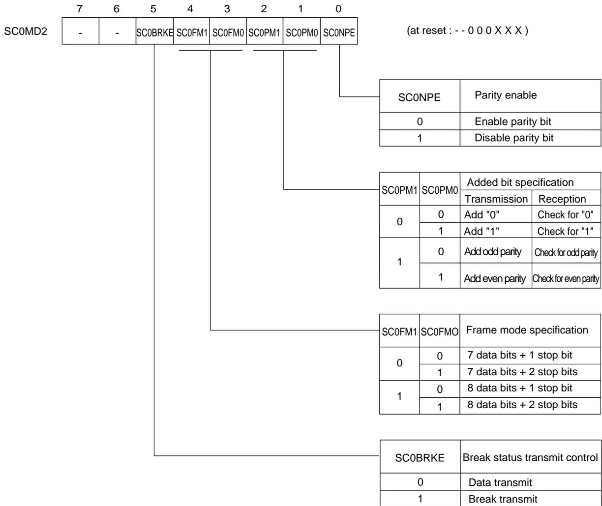
Figure 10-2-5 Serial Interface 0 Mode Register 2 (SC0MD2 : x'03F52', R/W)
