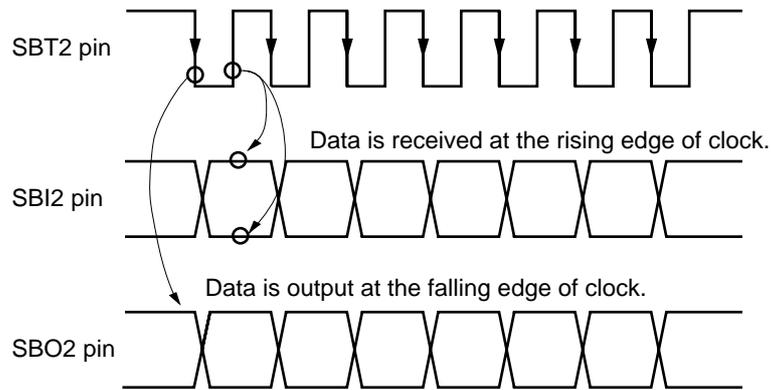
**Figure 12-3-8 Transmission / Reception Timing**
