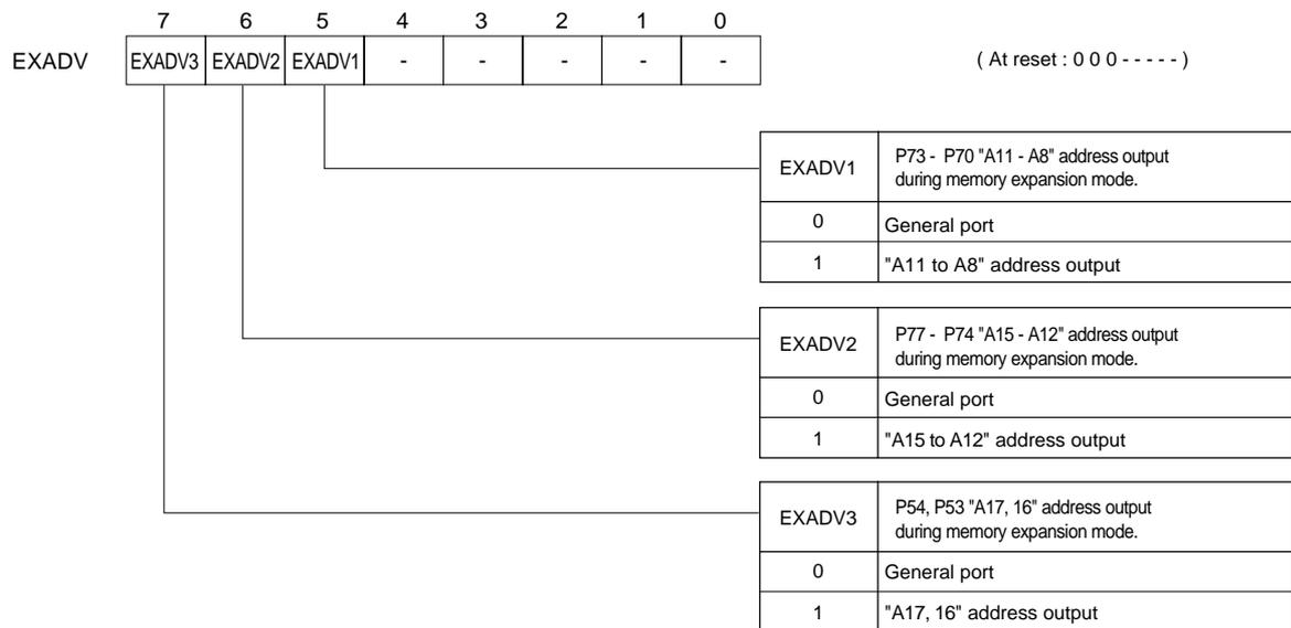
**Figure 2-3-3 Expansion Address Control Register (EXADV : x'03F0E', R/W)**
