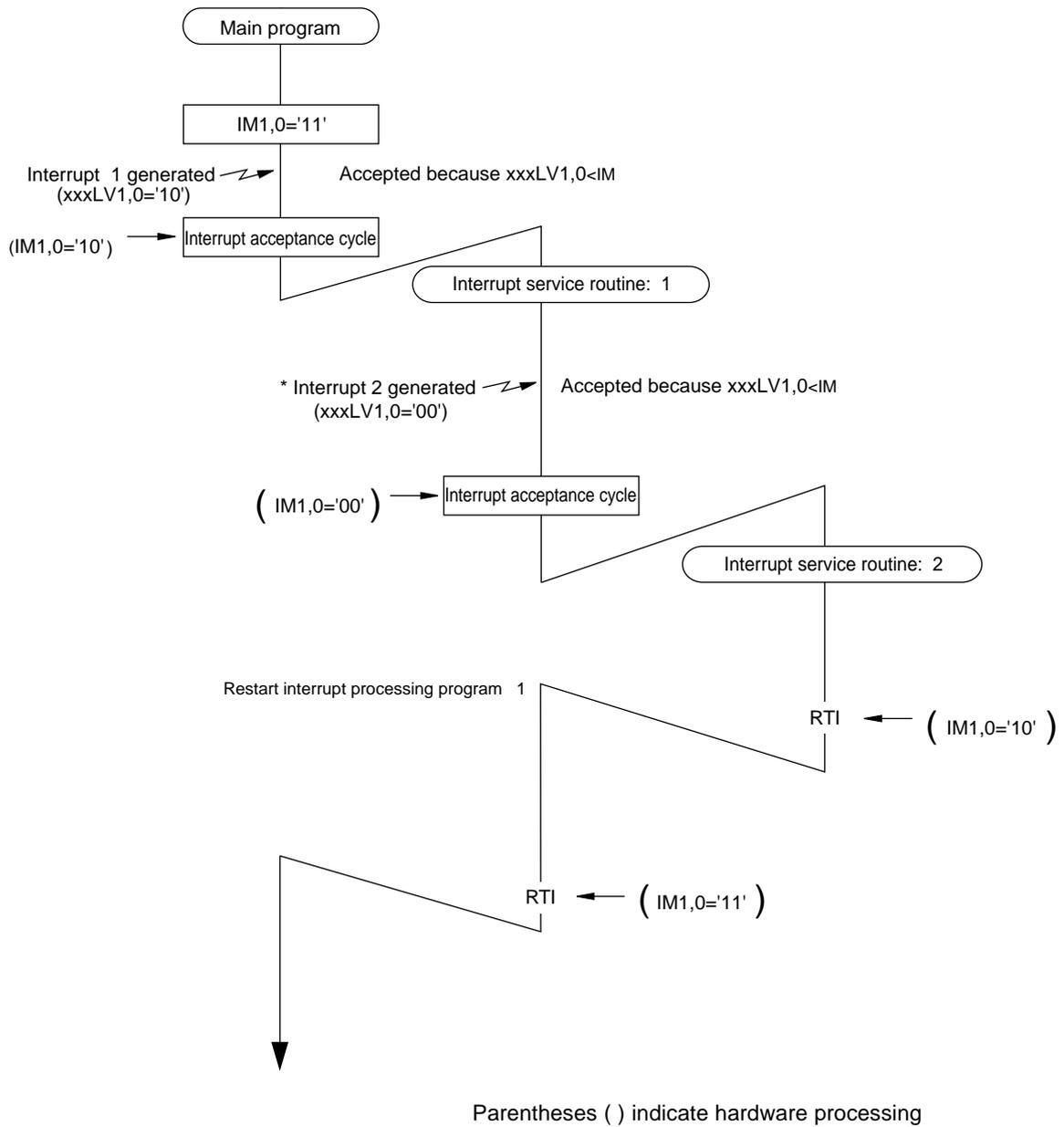
**Figure 3-1-7 Processing Sequence with Multiple Interrupts Enabled**
