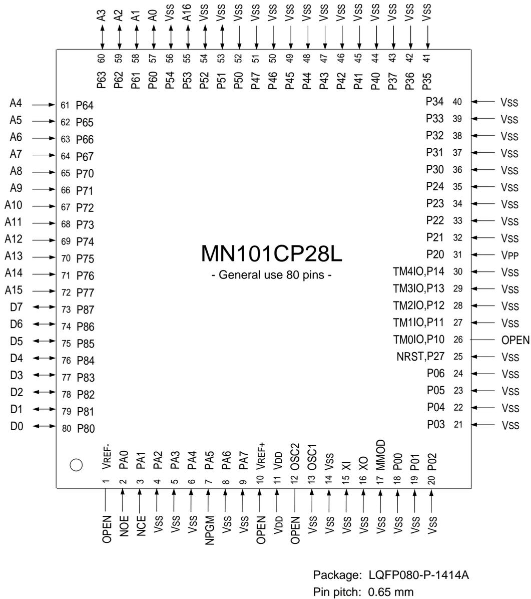
Figure 15-1-2 MN101CP28LAL EPROM Programming Adapter Connection
