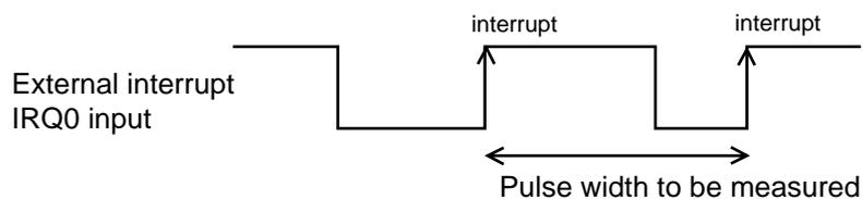
**Figure 6-8-2 Pulse Width Measurement of External Interrupt 0**
