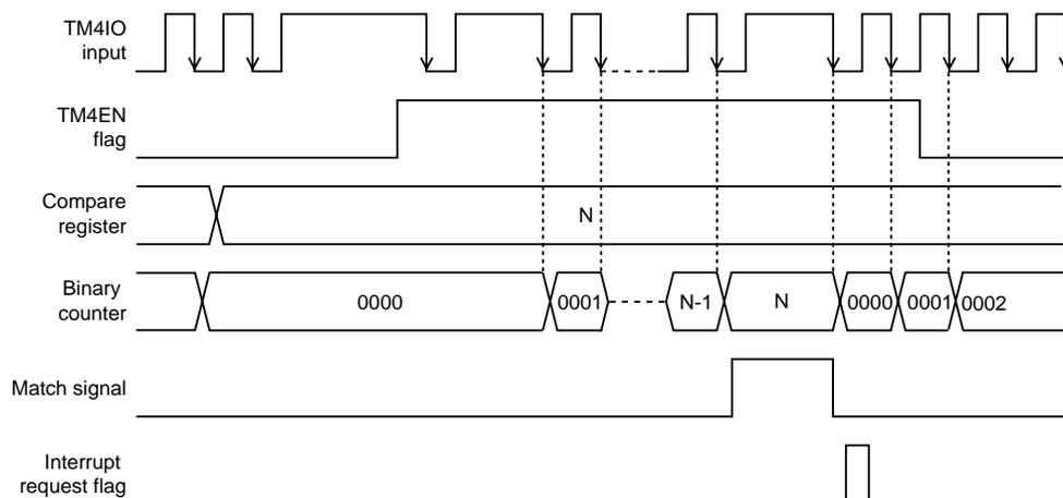
**Figure 6-4-1 Count Timing TM4IO Input (Timer 4)**
