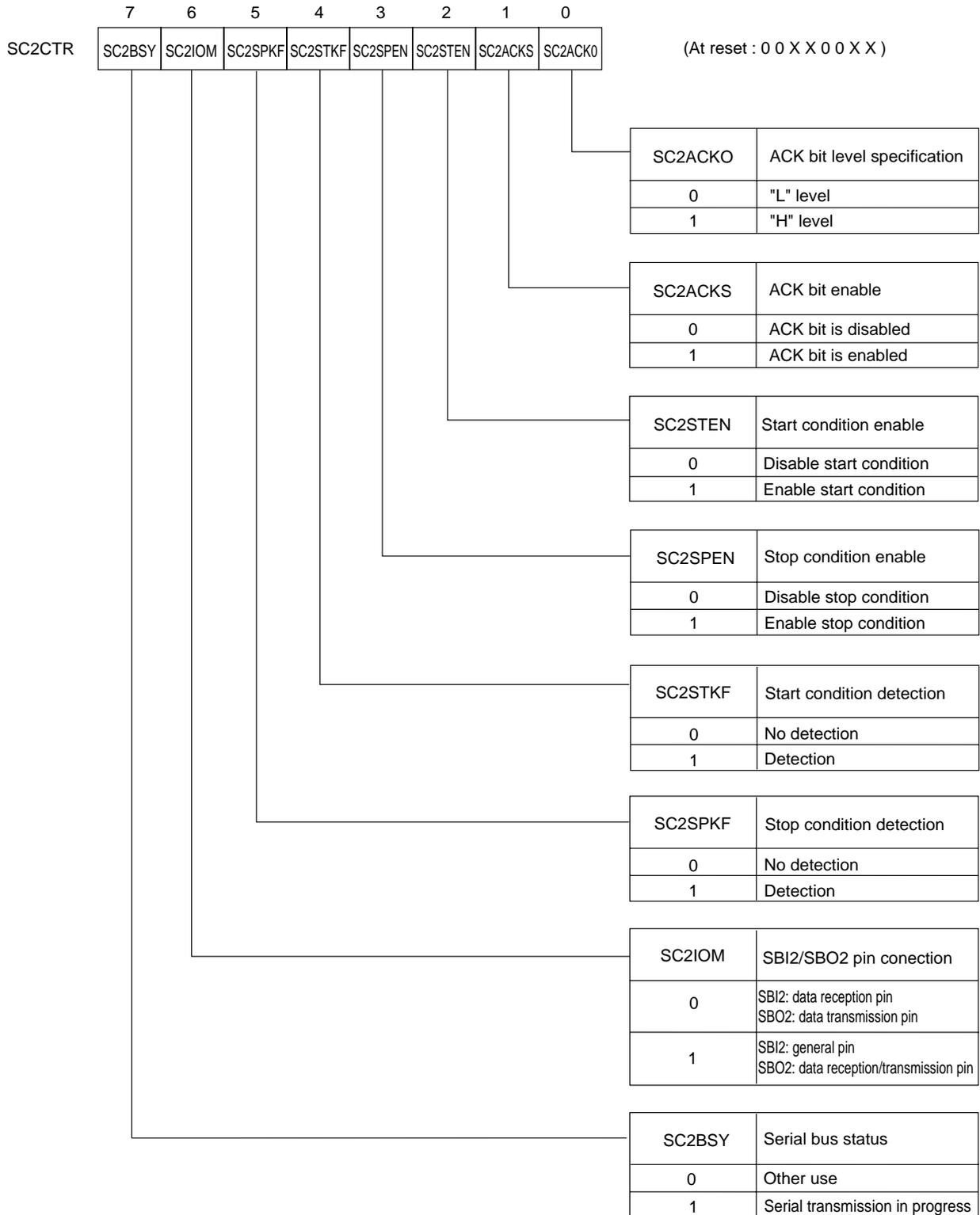
Figure 12-2-4 Serial Interface 2 Control Register (SC2CTR : x'03F5C', R/W)
