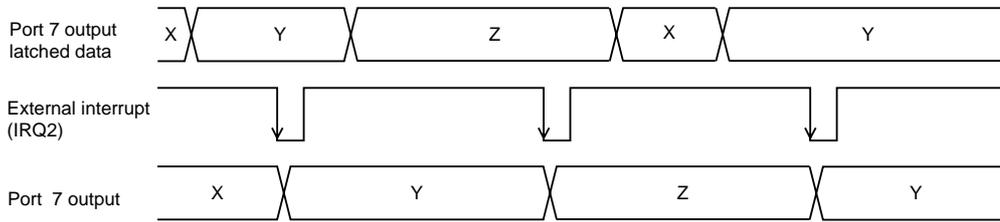
**Figure 4-12-2 Synchronous Output Timing by Event Generation (IRQ2)**
