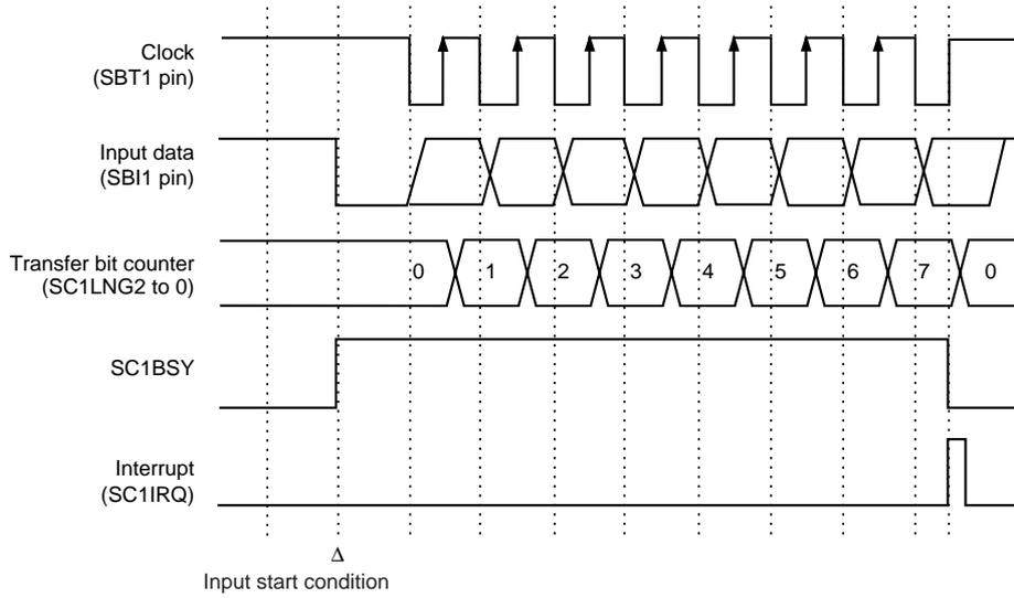
Figure 11-3-5 Reception Timing (at rising edge, start condition is enabled)
