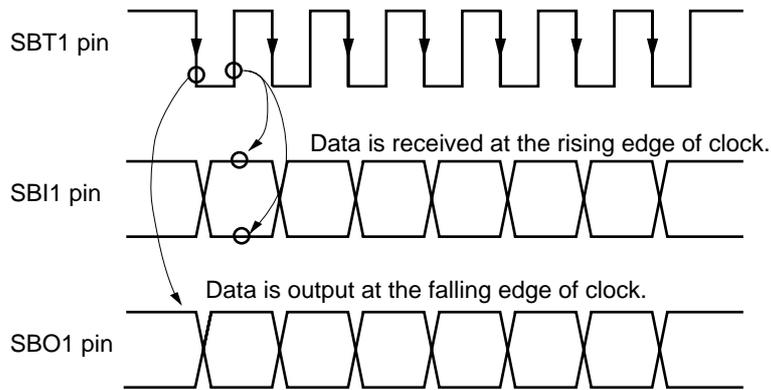
**Figure 11-3-9 Transmission / Reception Timing**
