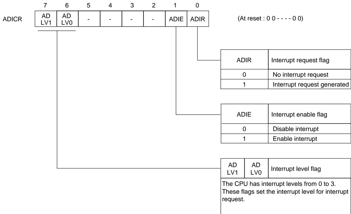
Figure 3-2-17 A/D Conversion Interrupt Control Register (ADICR : x'03FEA', R/W)
