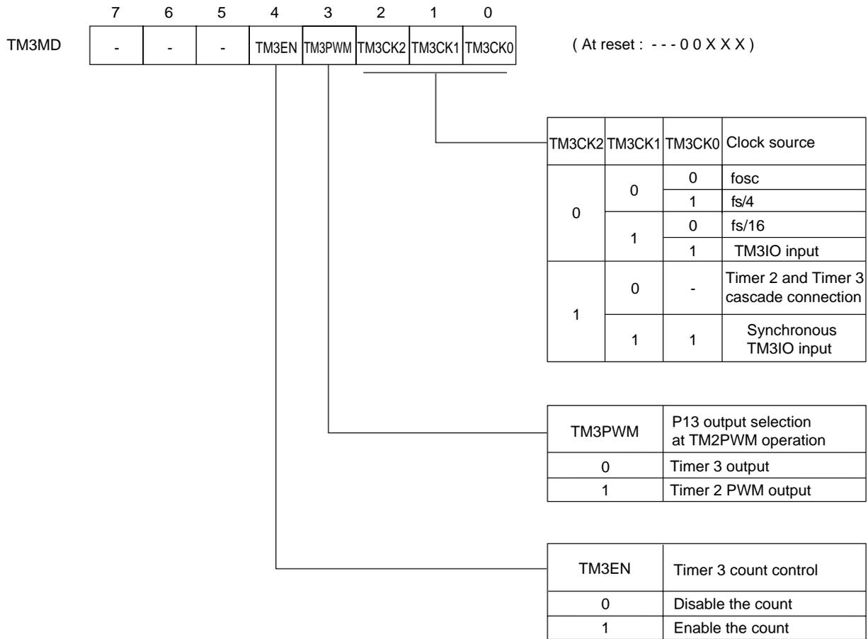
Figure 5-2-12 Timer 3 Mode Register (TM3MD : x'03F83', R/W)
