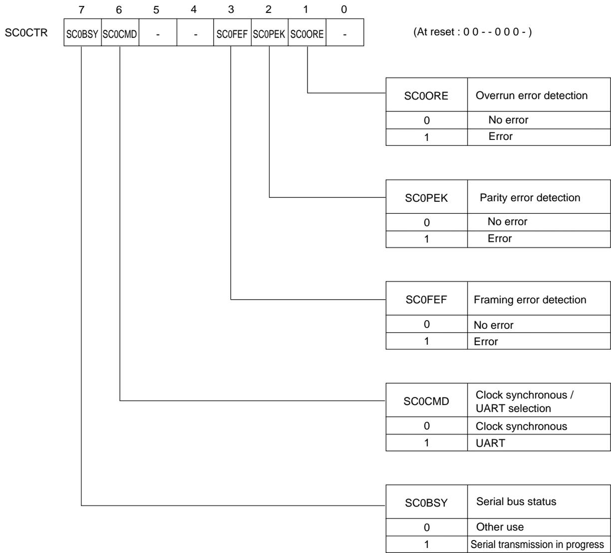
**Figure 10-2-7 Serial Interface 0 Control Register (SC0CTR : x'03F54', R/W)**
