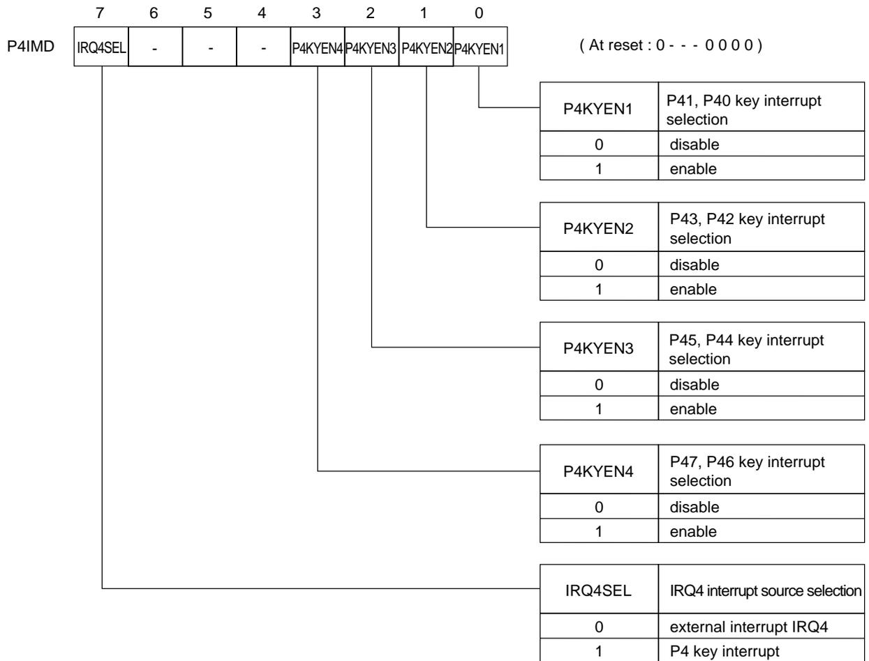
Key interrupt control register (P4IMD: x'03F3C', R/W)
