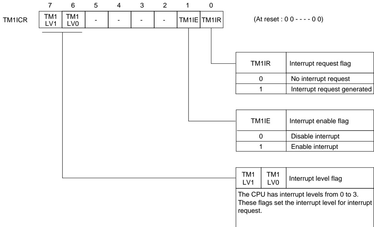
Figure 3-2-8 Timer 1 Interrupt Control Register (TM1ICR : x'03FE5', R/W)
