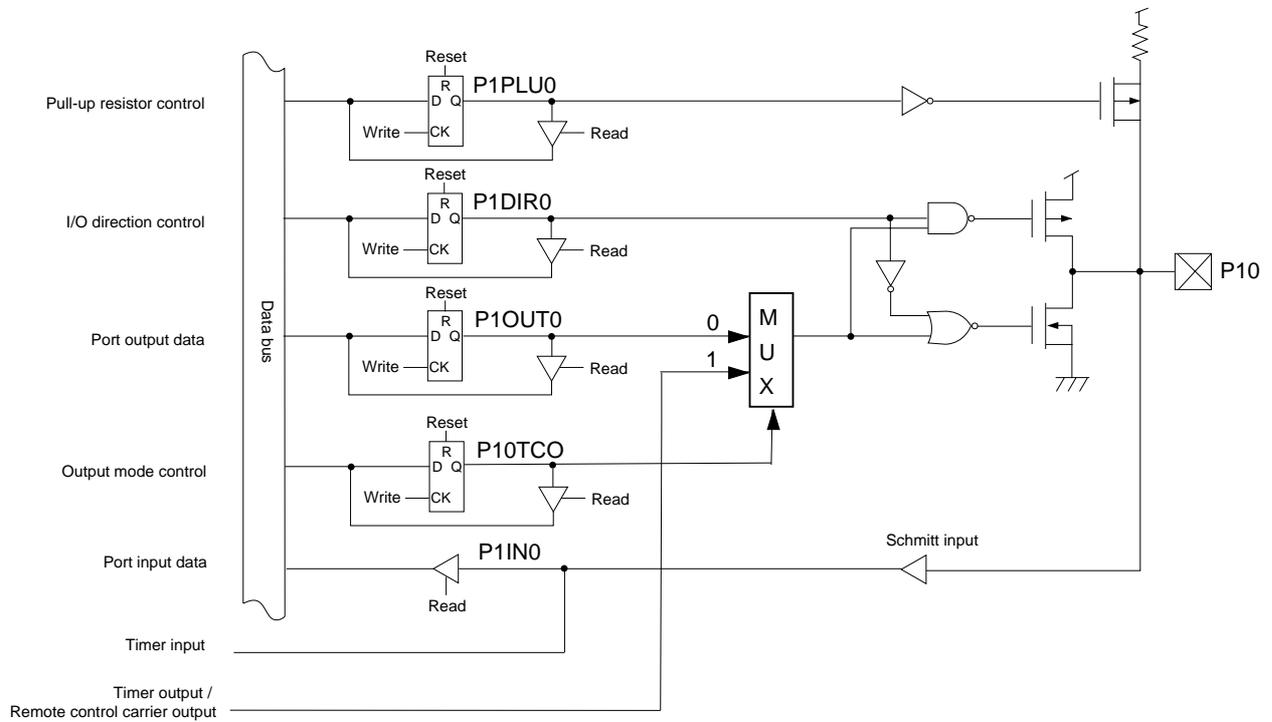
\* The TM0RM flag of the RMCTR register switches the remote control output and the timer output.
