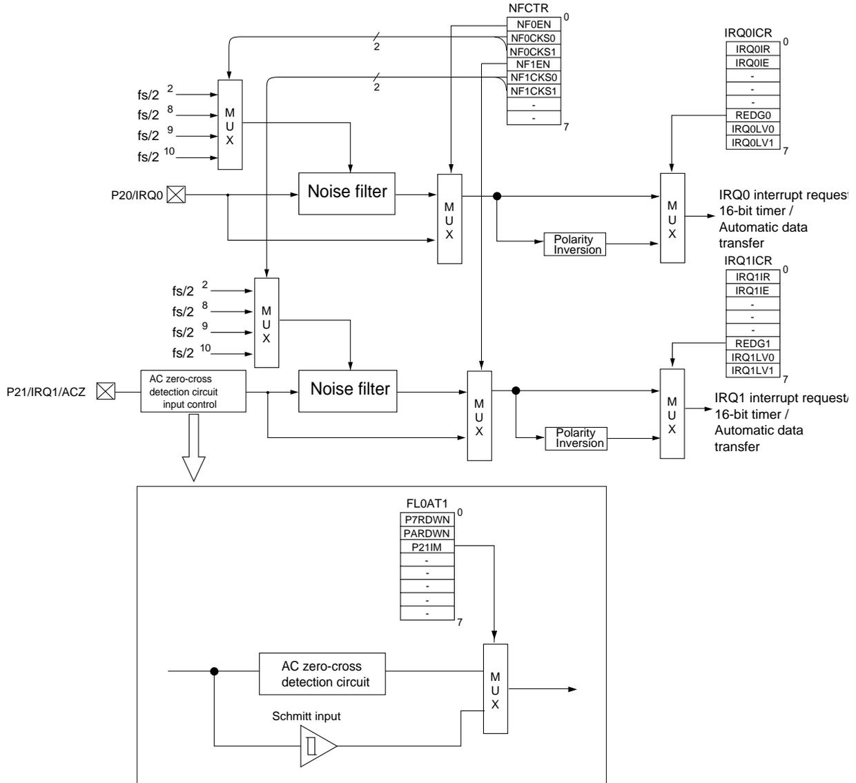
Figure 3-3-1 External Interrupt 0 Interface and External Interrupt 1 Interface Block Diagram
