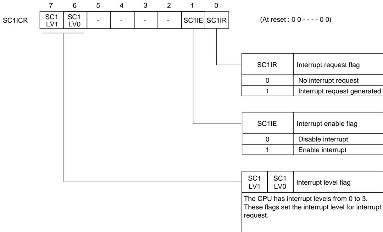
Figure 3-2-15 Serial interface 1 Interrupt Control Register (SC1ICR : x'03FF1', R/W)
