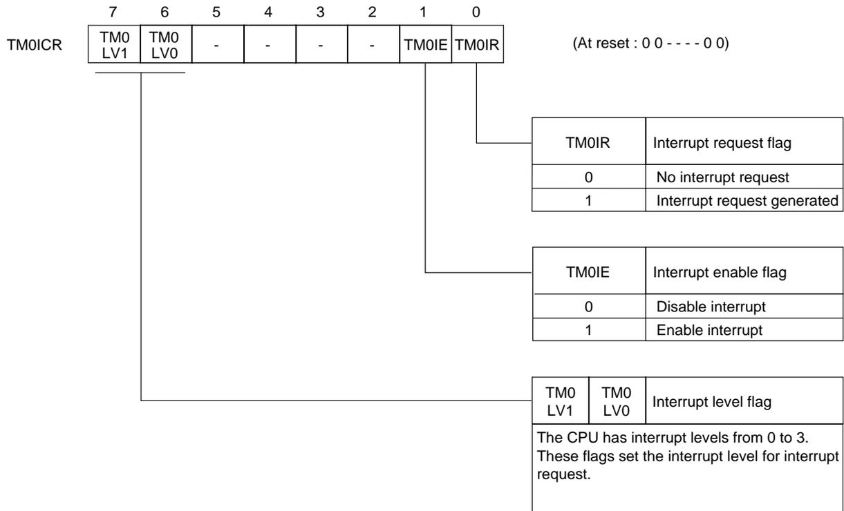
Figure 3-2-7 Timer 0 Interrupt Control Register (TM0ICR : x'03FE4', R/W)
