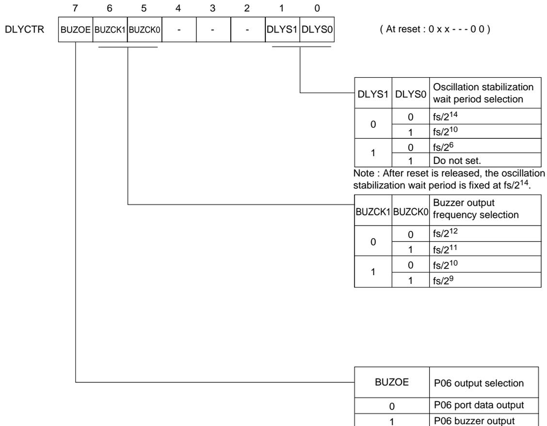
**Figure 9-2-1 Oscillation Stabilization Wait Timer Control Register**
