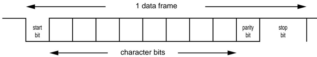
**Figure 10-3-11 UART Serial Interface Transmission / Reception Data Format**
