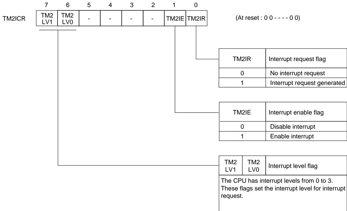
Figure 3-2-9 Timer 2 Interrupt Control Register (TM2ICR : x'03FE6', R/W)
