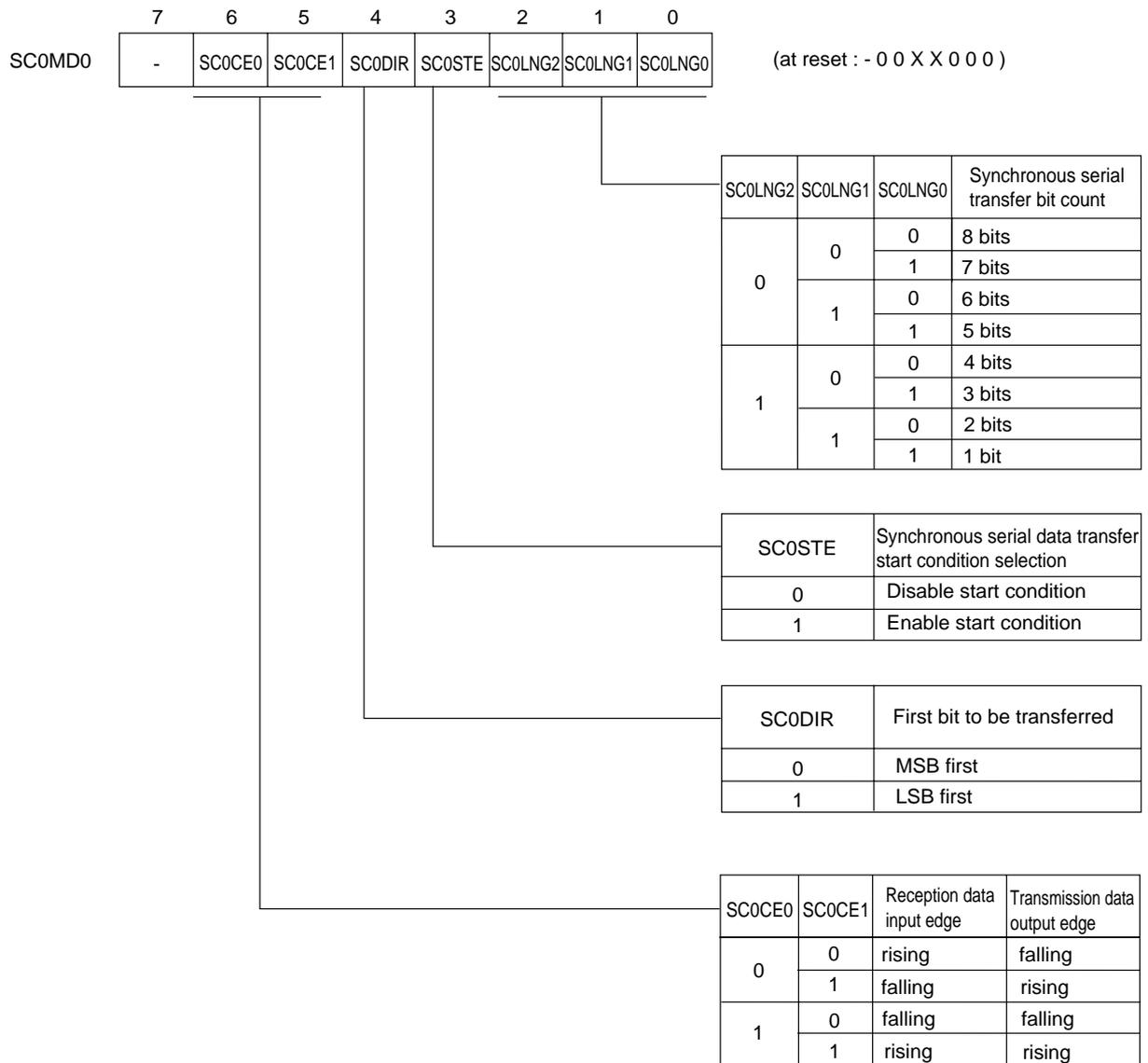
Figure 10-2-3 Serial Interface 0 Mode Register 0 (SC0MD0 : x'03F50', R/W)
