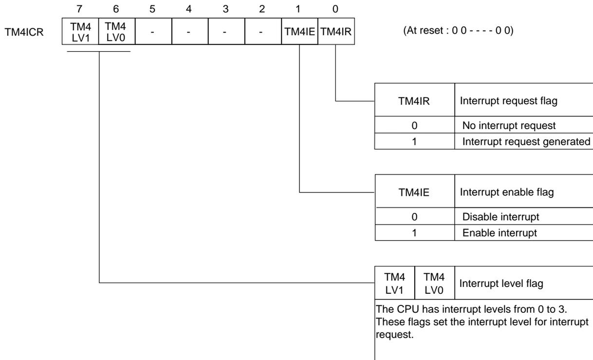
Figure 3-2-11 Timer 4 Interrupt Control Register (TM4ICR : x'03FEF', R/W)
