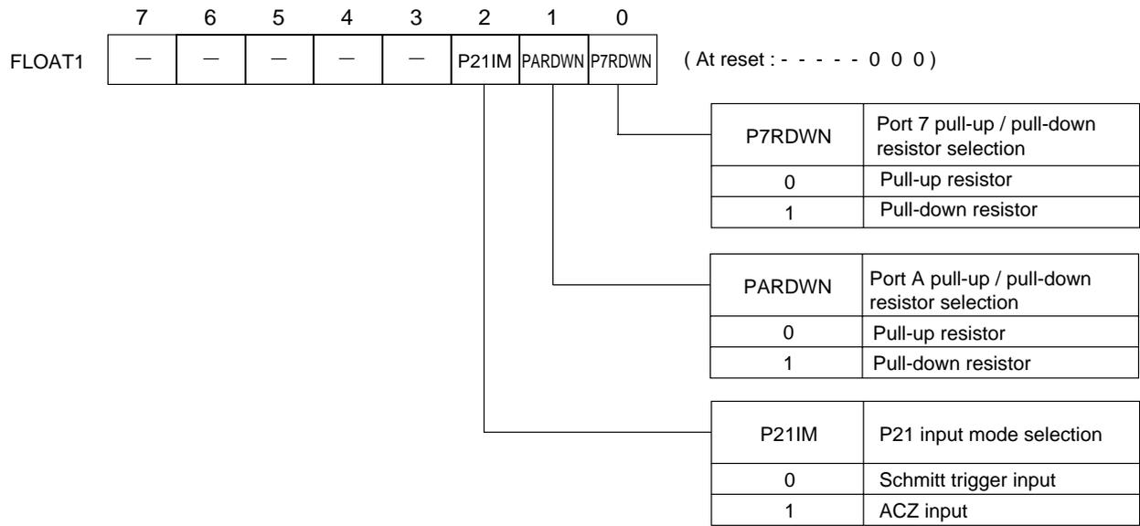
Pin control register 1 (FLOAT1 : X'03F4B', R/W)
