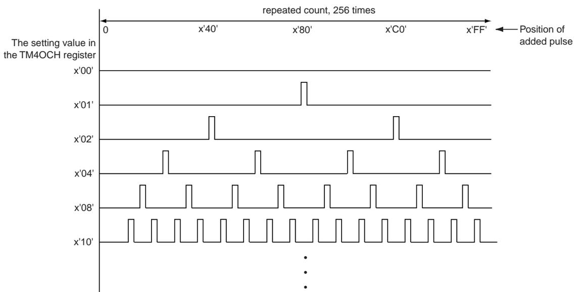
Figure 6-6-2 The Setting Value in The TM4OCH Register and The Position of The Added Pulse
