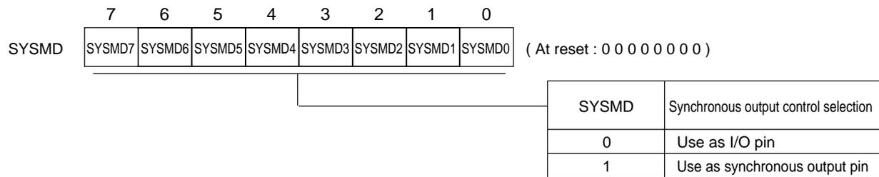
Synchronous output control register (SYSMO : X'03F1F', R/W)
