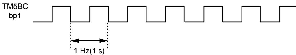
**Figure 7-3-1 Waveform of TM5BC Register bp1 (Timer 5)**
