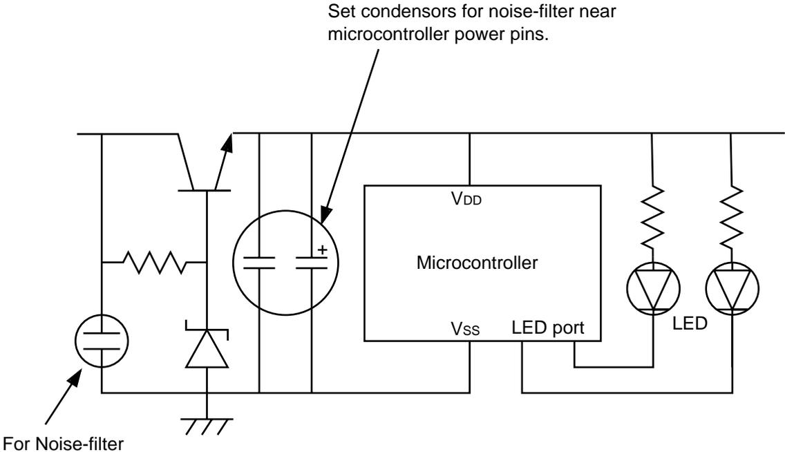
Figure 1-7-7 An Example for Emitter Follower Type Power Supply Circuit
