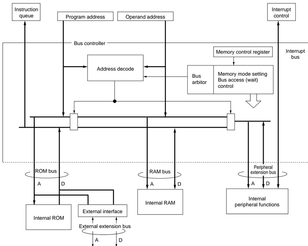
**Figure 2-3-1 Functional Block Diagram of the Bus Controller**
