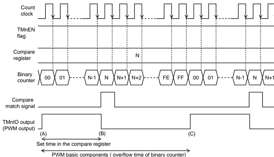
**Figure 5-6-1 Count Timing of PWM Output (at Normal)**
