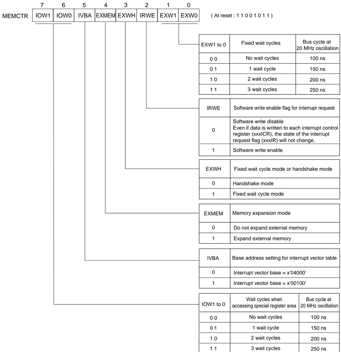
Figure 2-3-2 Memory Control Register (MEMCTR: x'3F01' R/W)
