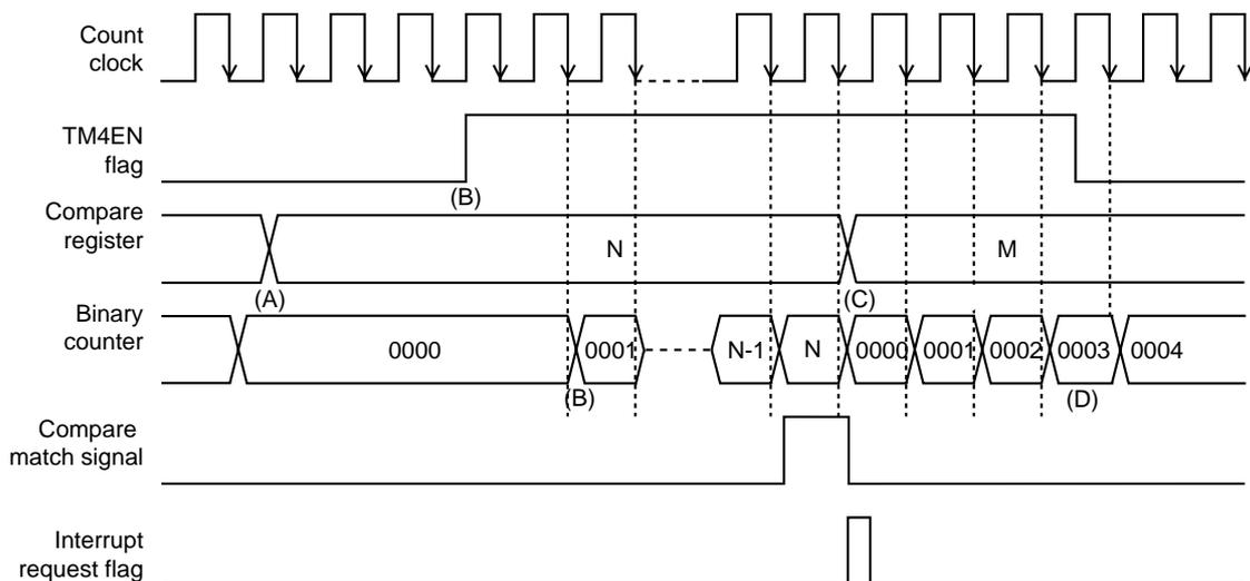
**Figure 6-3-1 Count Timing of Timer Operation (Timer 4)**
