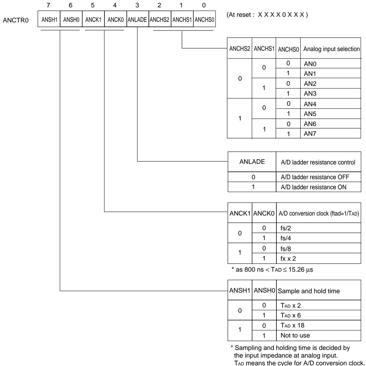
Figure 14-2-1 A/D Converter Control Register 0 (ANCTR0 : x'03F90', R/W)
