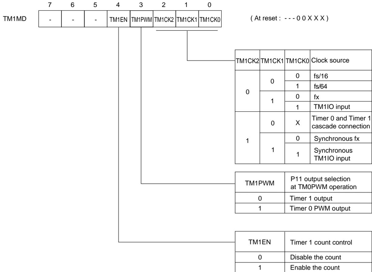
Figure 5-2-10 Timer 1 Mode Register (TM1MD : x'03F81', R/W)
