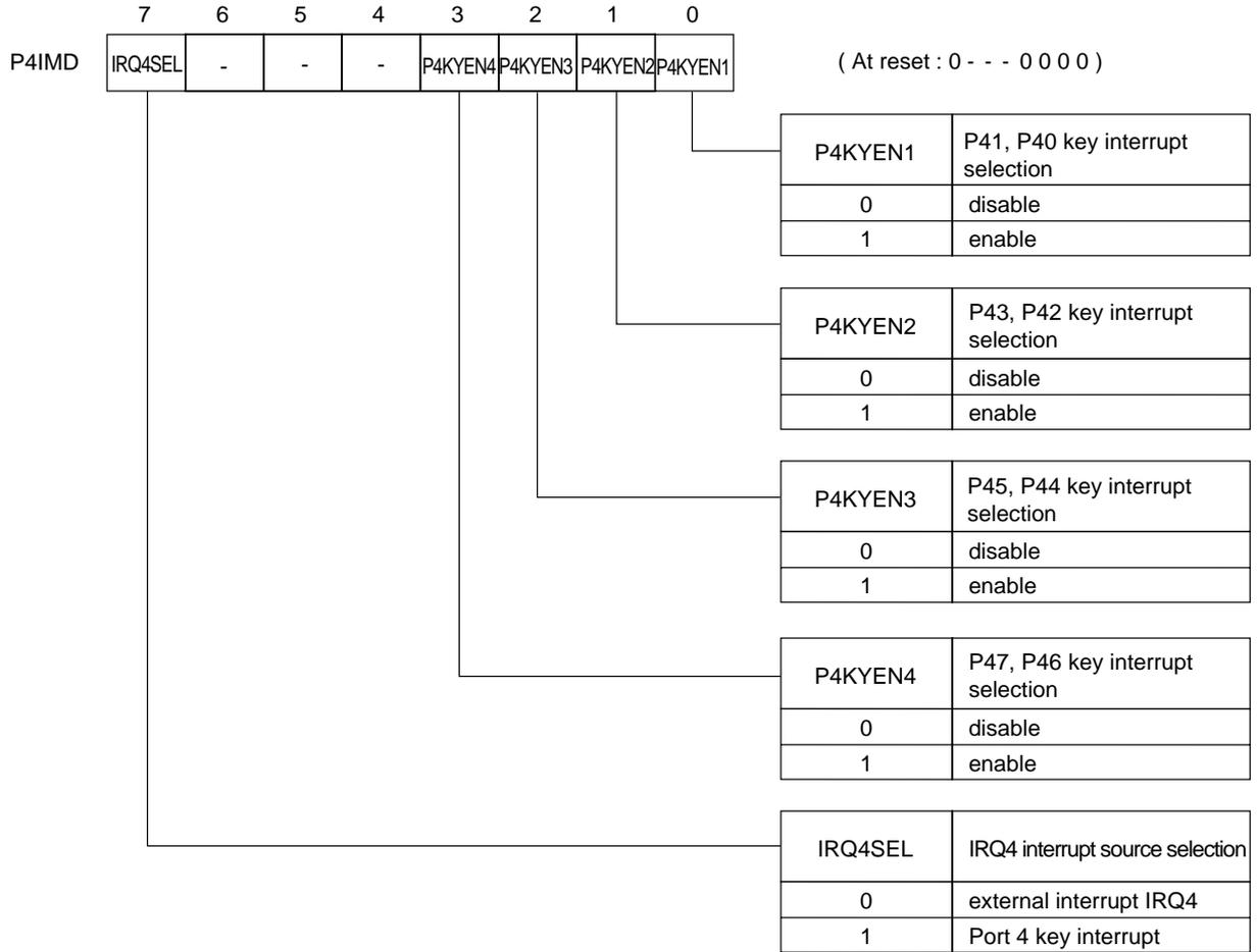
Figure 3-3-6 Port 4 Key Interrupt Control Register (P4IMD : x'03F3C', R/W)
