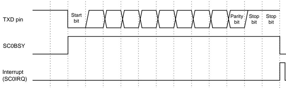
**Figure 10-3-12 Transmission Timing (parity bit is enabled)**
