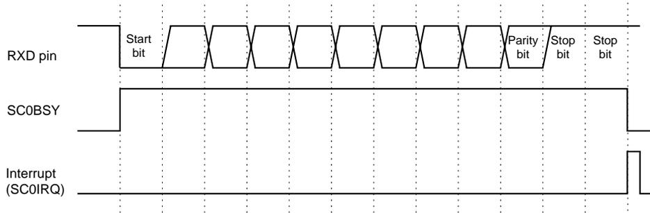
Figure 10-3-14 Reception Timing (parity bit is enabled)
