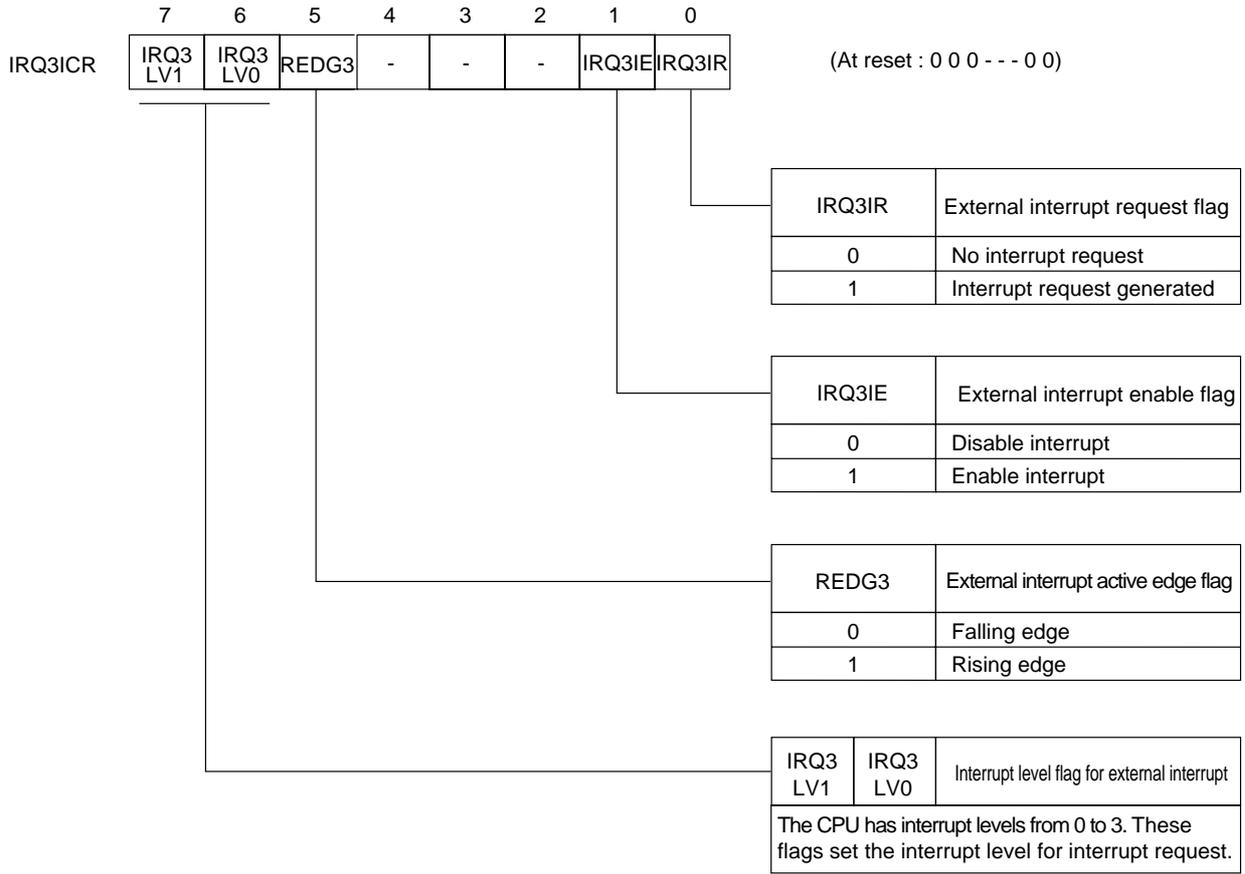
Figure 3-2-5 External Interrupt 3 Control Register (IRQ3ICR : x'03FEC', R/W)
