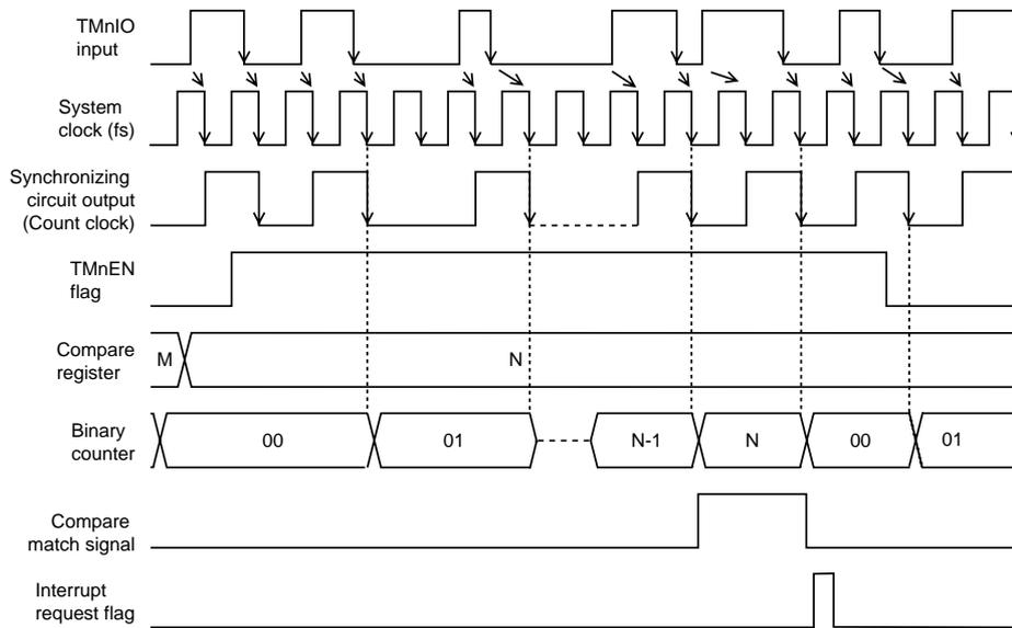
Figure 5-4-2 Count Timing of Synchronous TMnIO Input (Timers 0 to 3)
