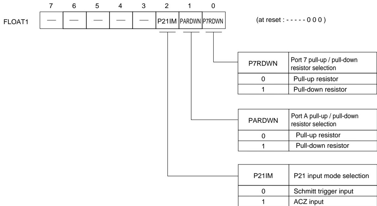
Figure 3-3-5 Pin Control Register 1 (FLOAT1 : x'03F4B', R/W)
