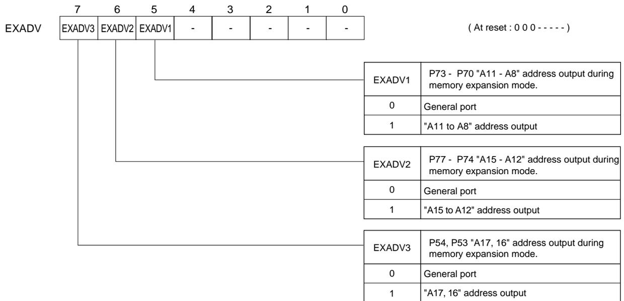
Expansion address output control register (EXADV: x'03F0E', R/W)
