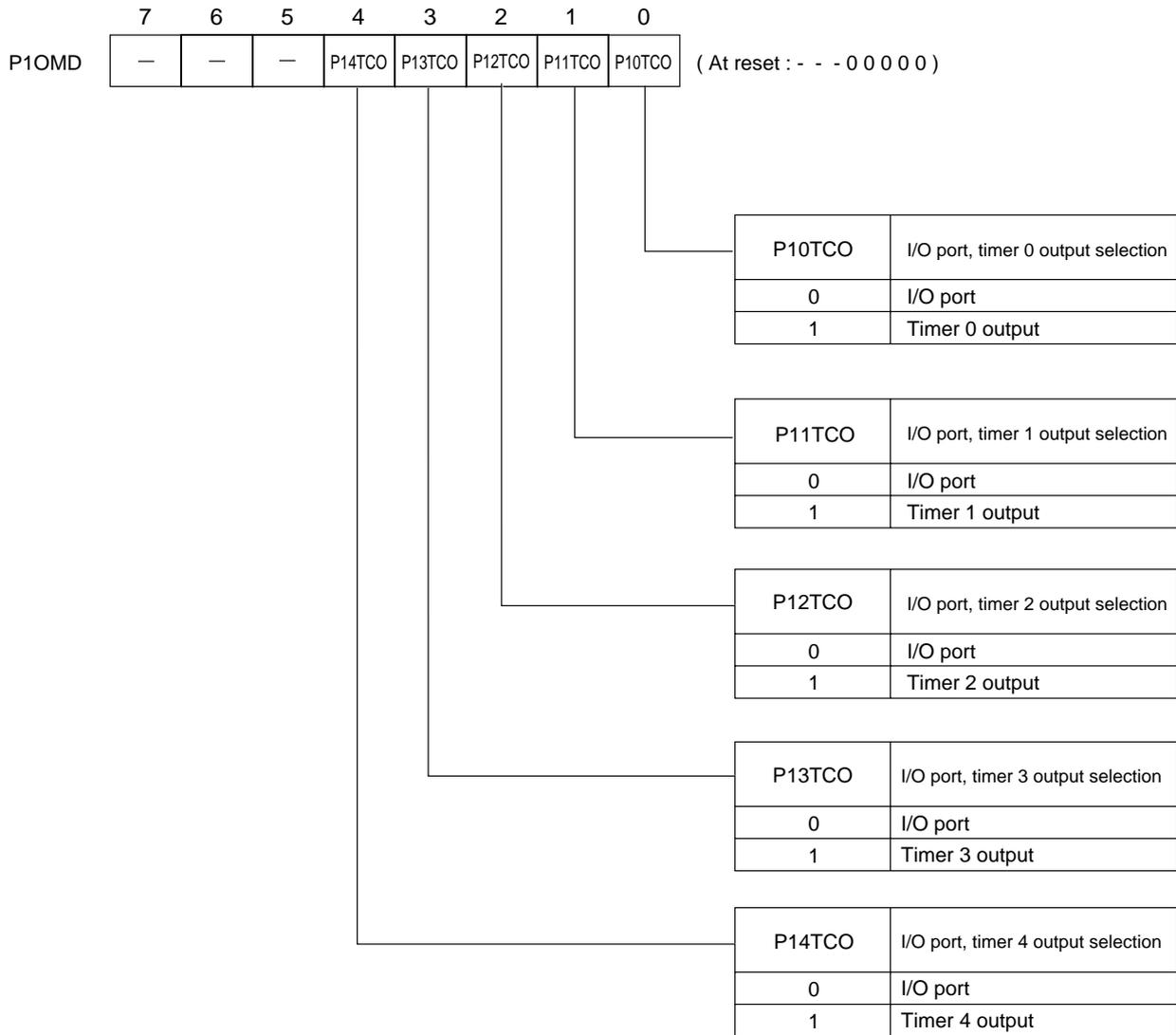
Port 1 output mode register (P1OMD : x'03F39', R/W)
