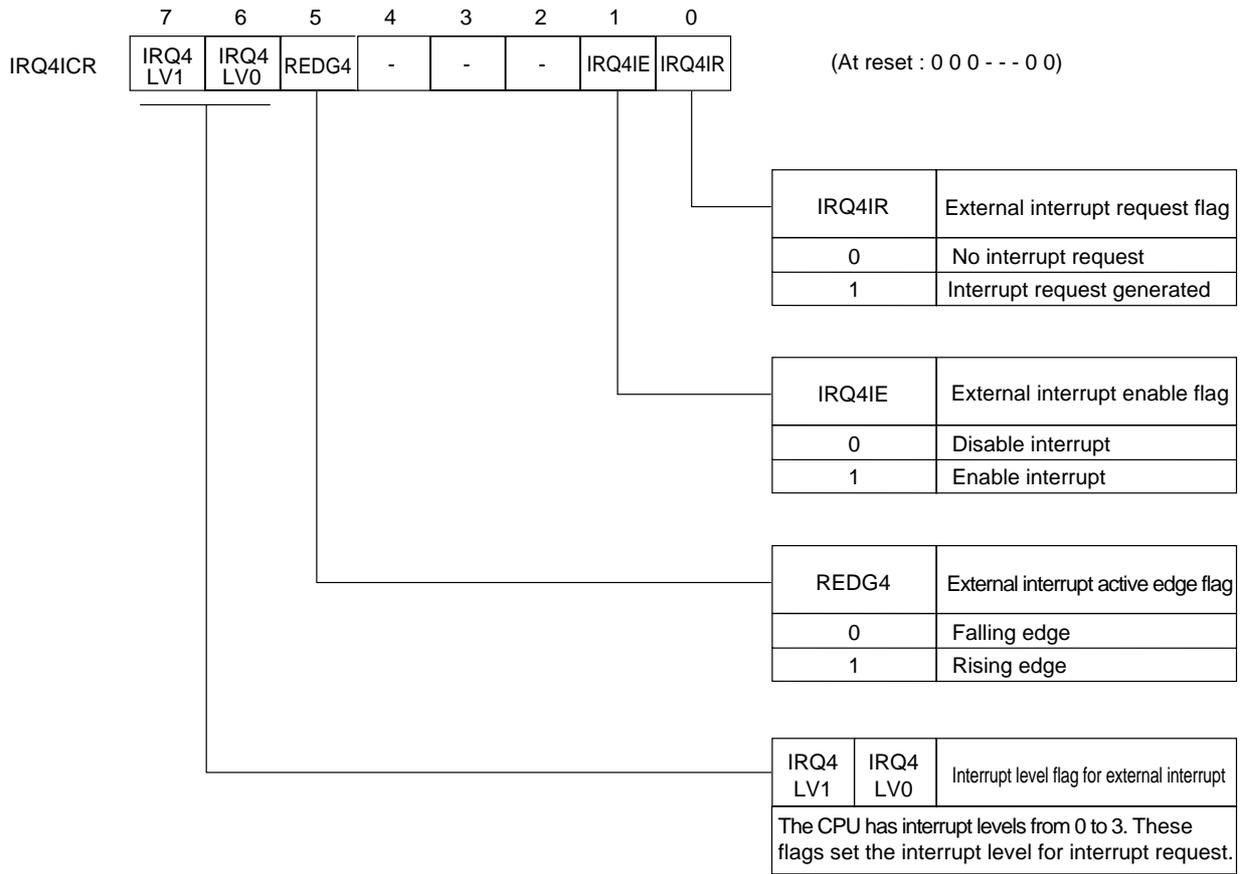
Figure 3-2-6 External Interrupt 4 Control Register (IRQ4ICR : x'03FED', R/W)
