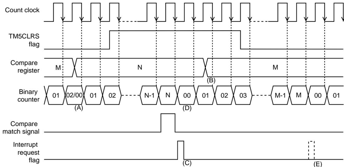
**Figure 7-3-2 Count Timing of Timer Operation (Timer 5)**
