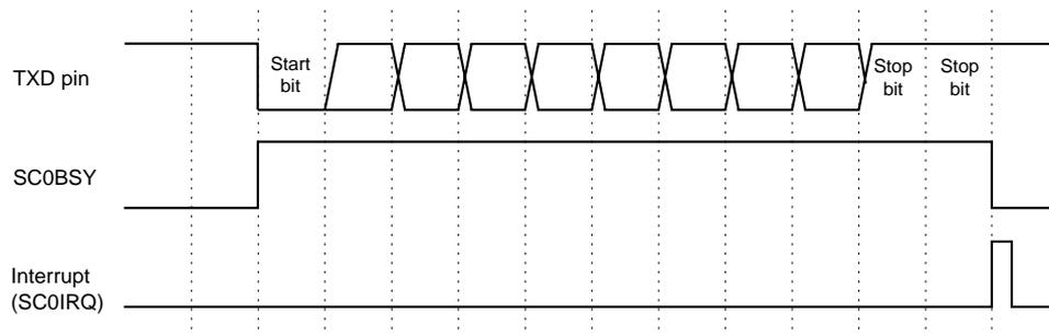
**Figure 10-3-13 Transmission Timing (parity bit is disabled)**
