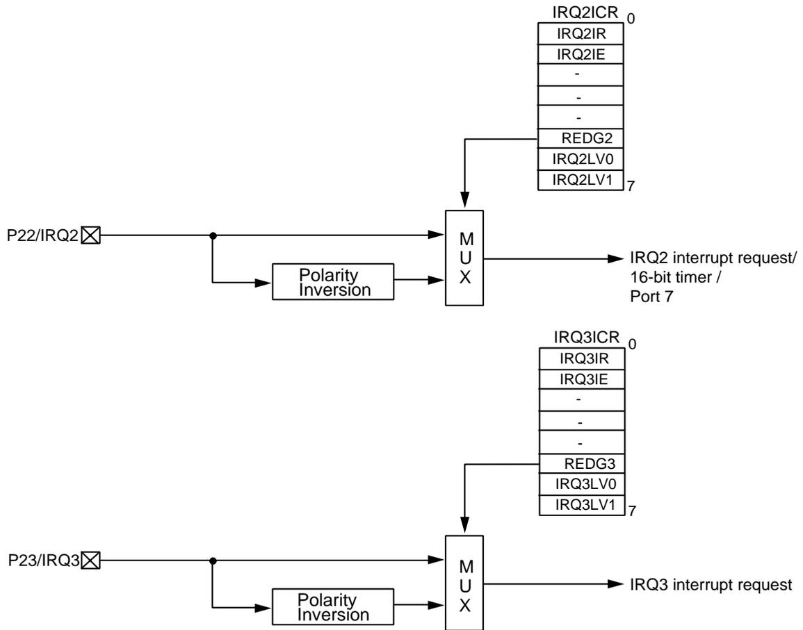
Figure 3-3-2 External Interrupt 2 Interface, External Interrupt 3 Interface
