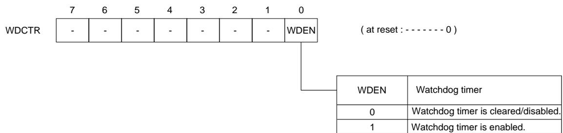
**Figure 8-2-1 Watchdog Timer Control Register (WDCTR : x'03F02', R/W)**
