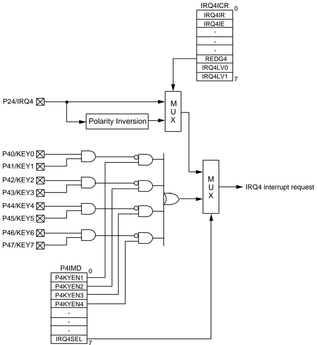
Figure 3-3-3 External Interrupt 4 Interface Block Diagram
