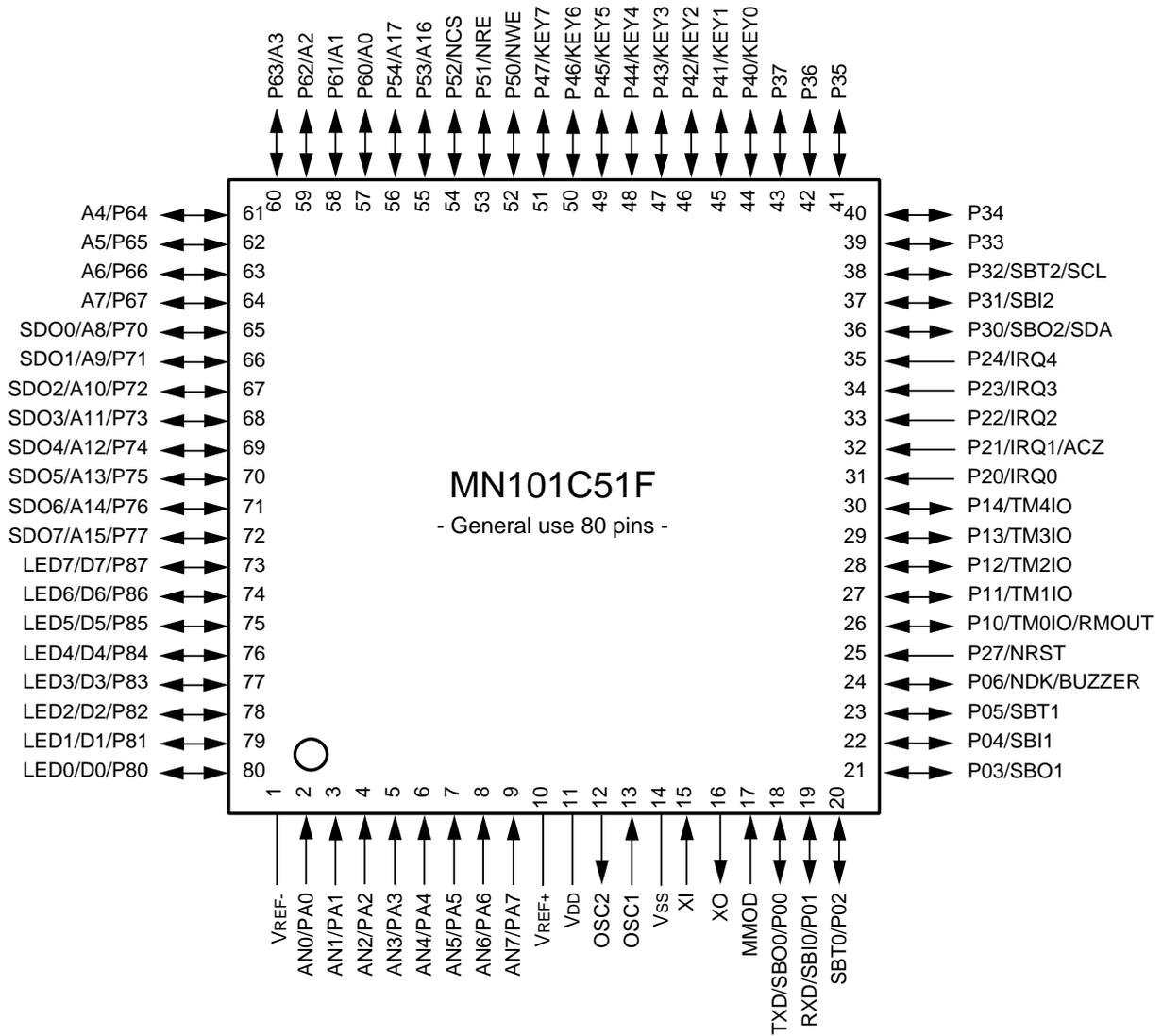
Figure 1-3-1 Pin Configuration ( 80LQFP : Top view )
