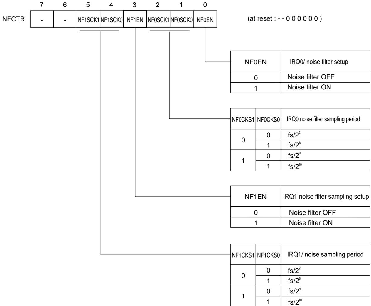
Figure 3-3-4 Noise Filter Control Register (NFCTR : x'03F8A', R/W)
