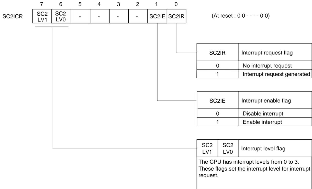
Figure 3-2-16 Serial interface 2 Interrupt Control Register (SC2ICR : x'03FF2', R/W)
