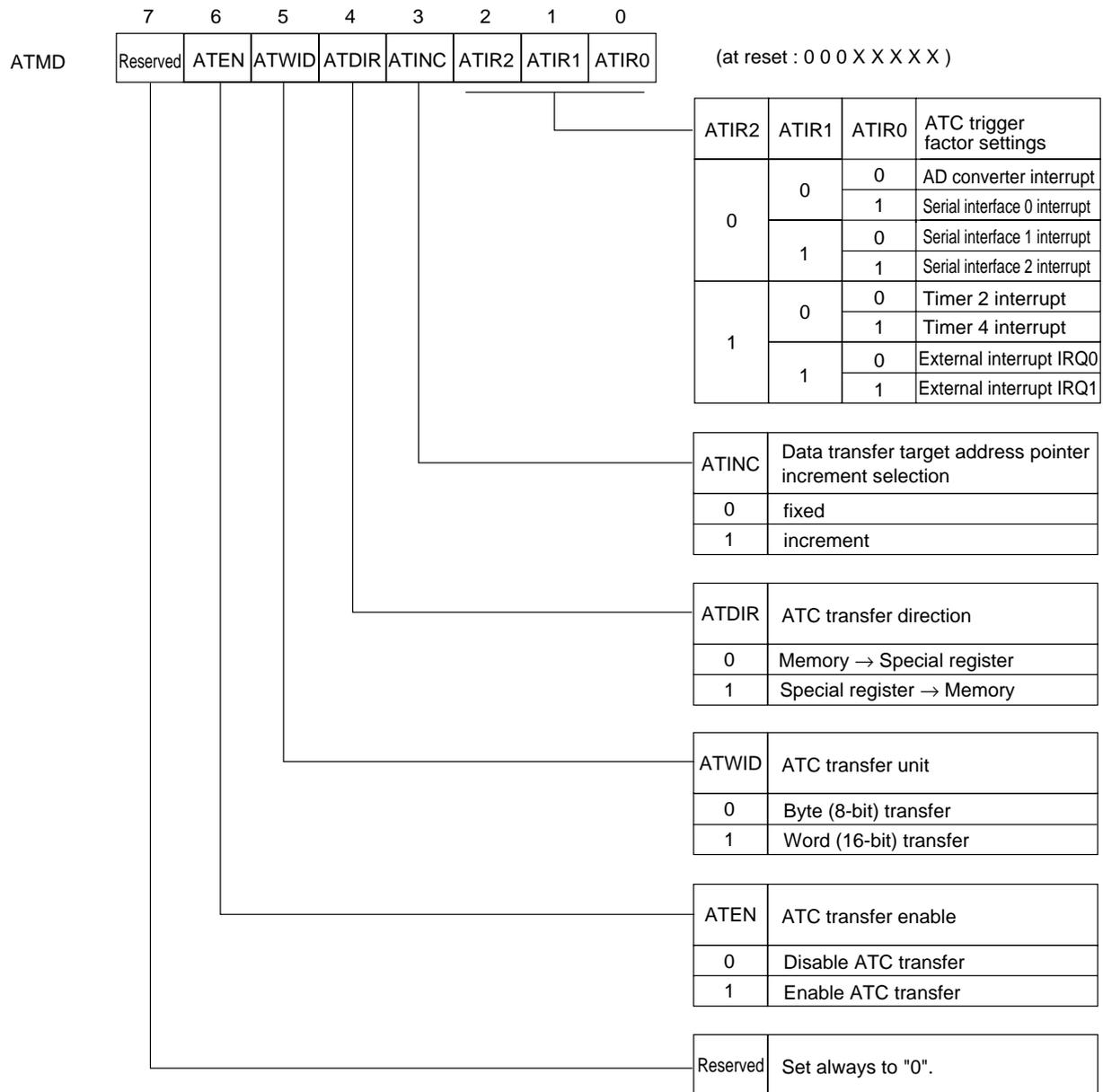
Figure 13-2-1 ATC Register (ATMD : x'03FA0', R/W)
