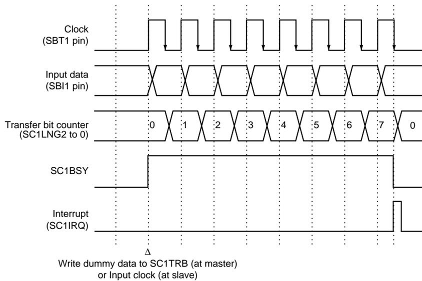
**Figure 11-3-8 Reception Timing (at falling edge, start condition is disabled)**
