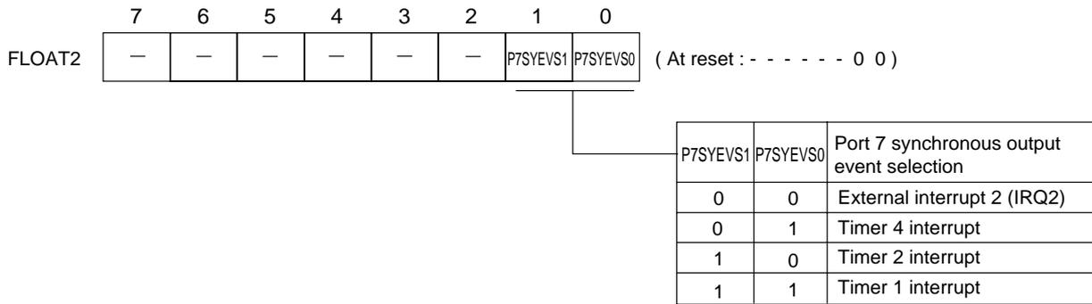
Pin control register 2 (FLOAT2 : x'03F4C', R/W)
