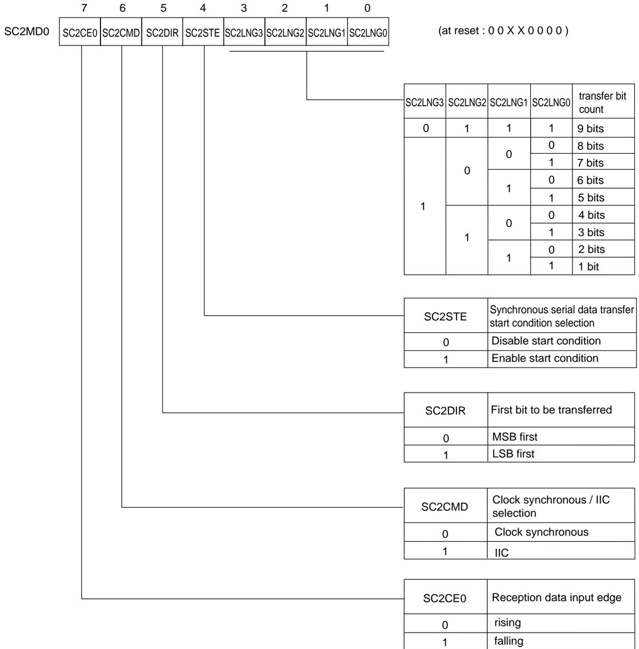
Figure 12-2-2 Serial Interface 2 Mode Register 0 (SC2MD0 : x'03F5A', R/W)
