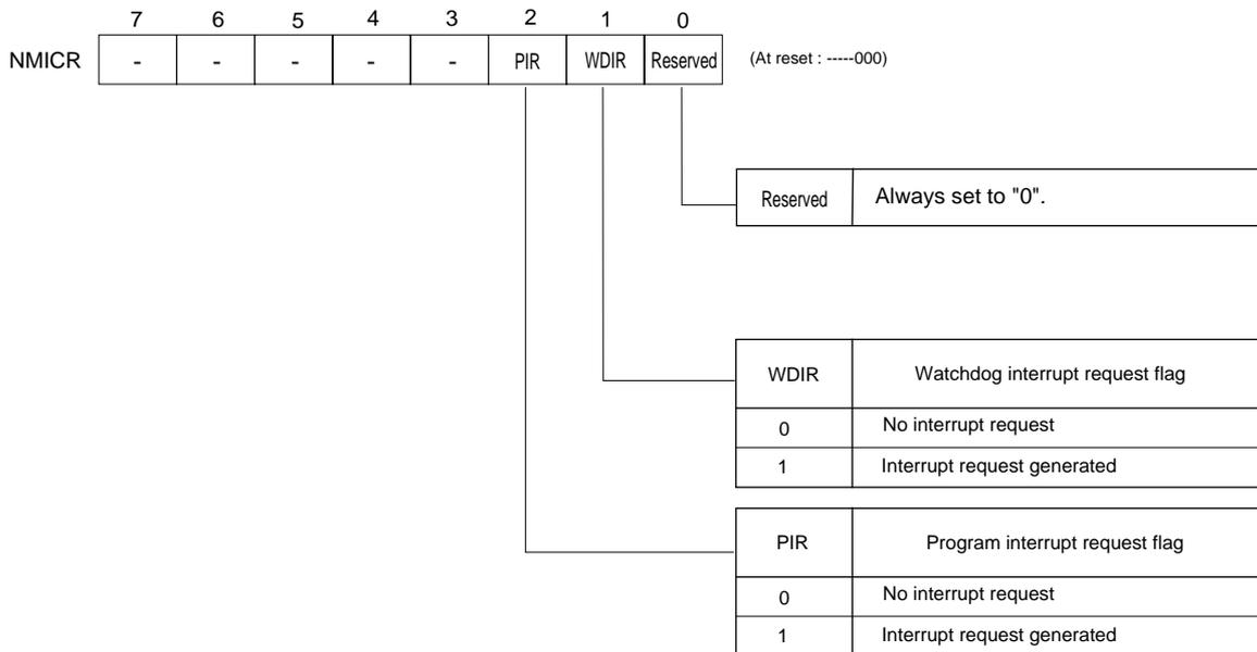
**Figure 3-2-1 Non-Maskable Interrupt Control Register (NMICR:x'03FE1', R/W)**
