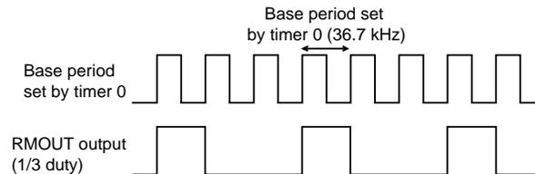
**Figure 5-10-3 Output Wave Form of RMOUT Output Pin**
