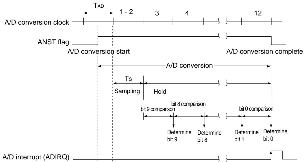
\* This example is as sampling and hold time is  $T_{AD} \times 2$ .
