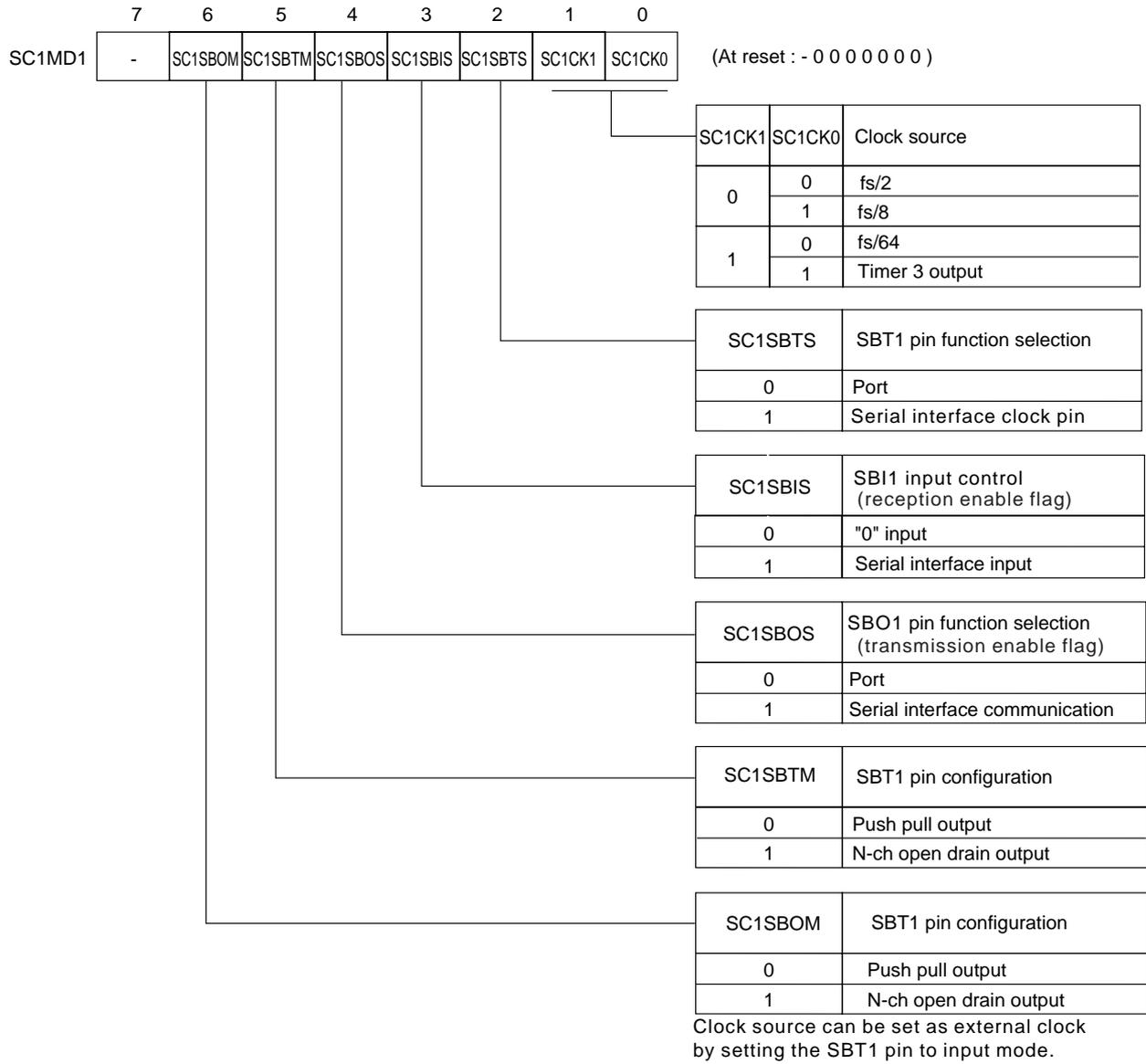
Figure 11-2-3 Serial Interface 1 Mode Register 1 (SC1MD1 : x'03F58', R/W)
