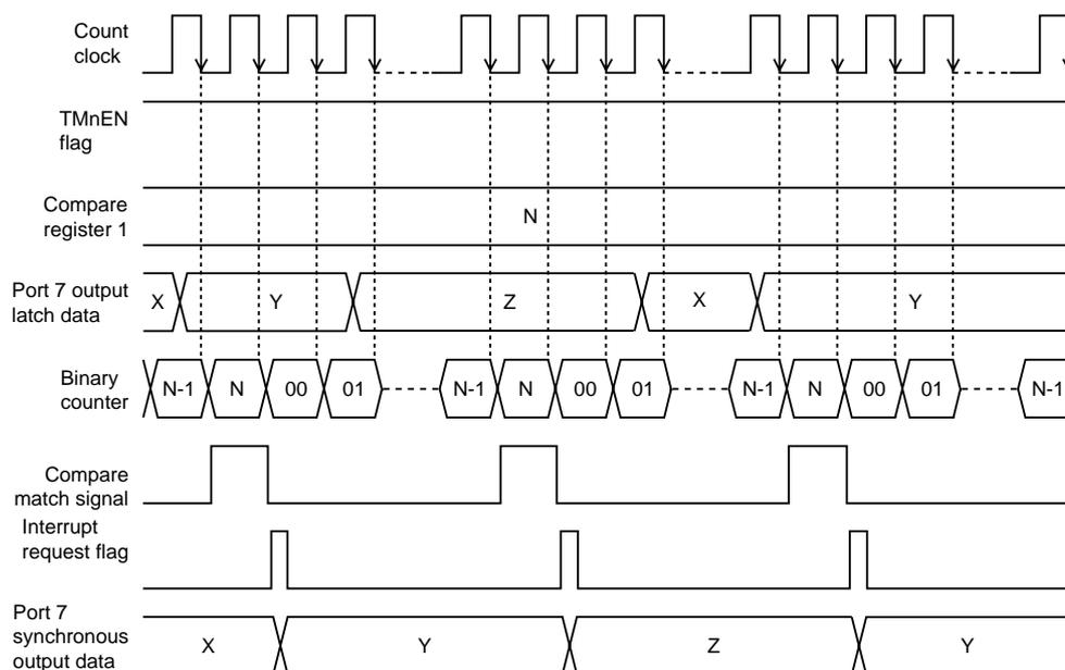
**Figure 5-7-1 Count Timing of Synchronous Output (Timer 1, Timer 2)**
