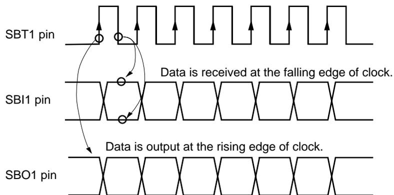
**Figure 11-3-10 Transmission / Reception Timing**
