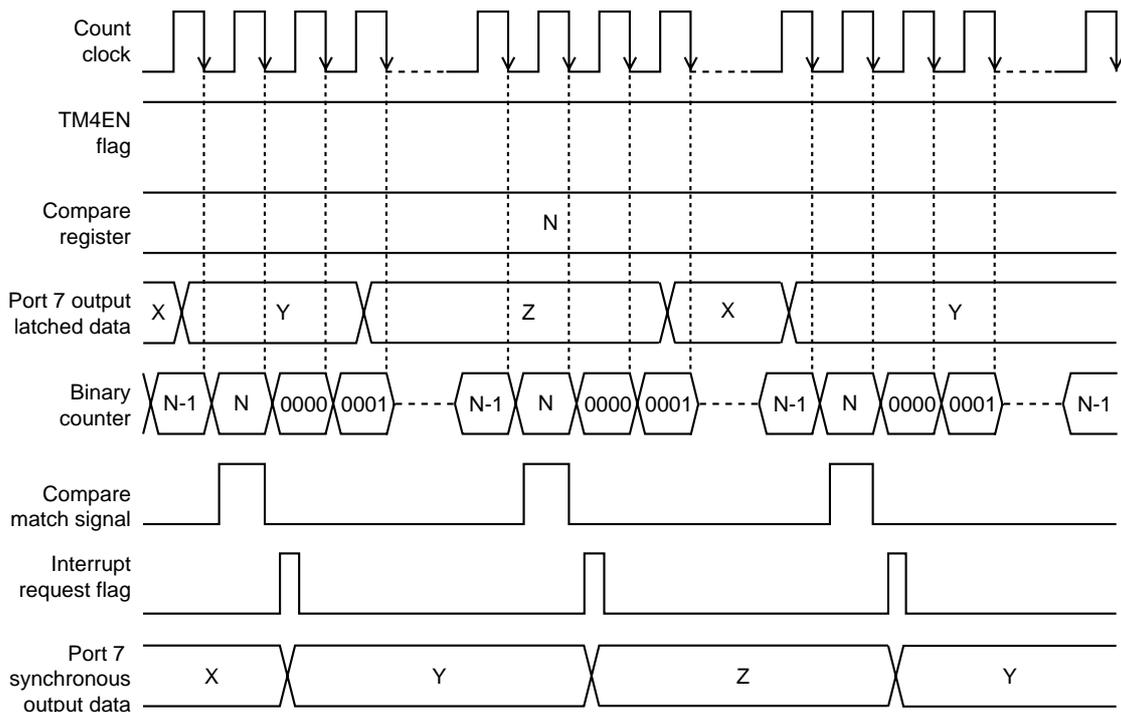
**Figure 6-7-1 Count Timing of Synchronous Output (Timer 4)**
