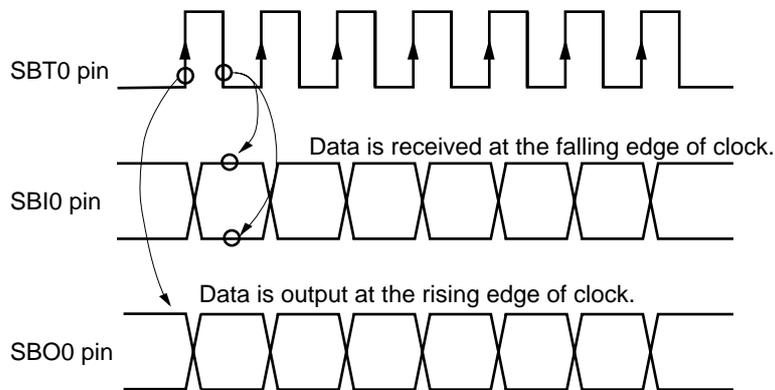
**Figure 10-3-10 Transmission / Reception Timing**
