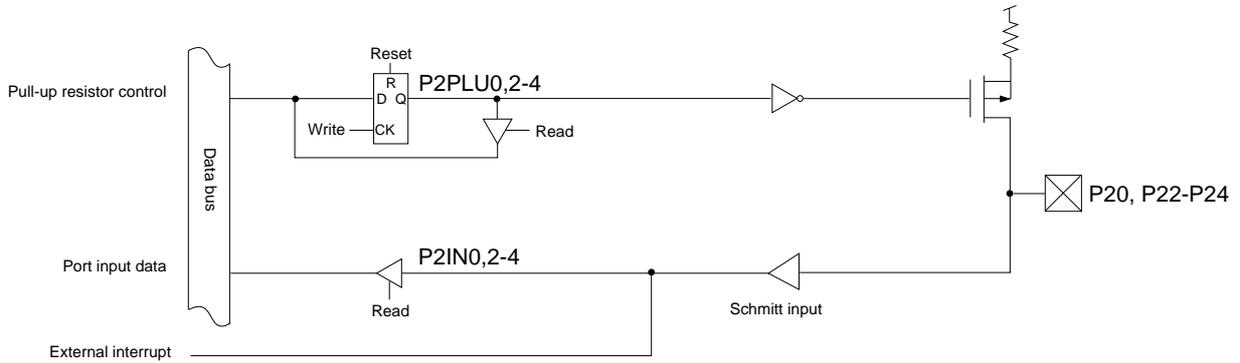
Figure 4-4-2 Block Diagram (P20, P22 to P24)
