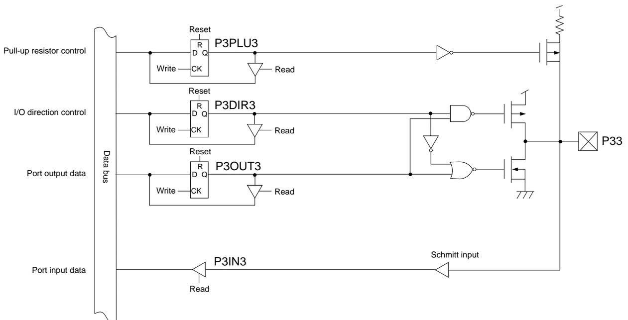
Figure 4-5-5 Block diagram (P33)
