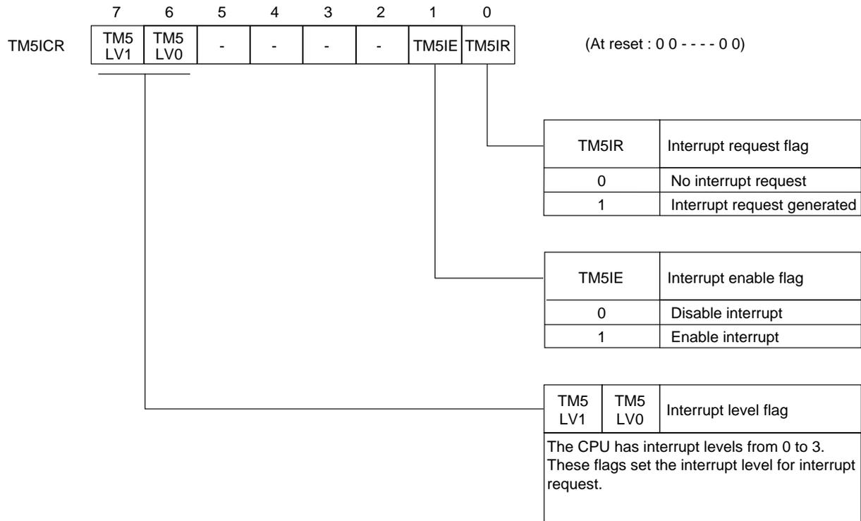
Figure 3-2-12 Timer 5 Interrupt Control Register (TM5ICR : x'03FF0', R/W)
