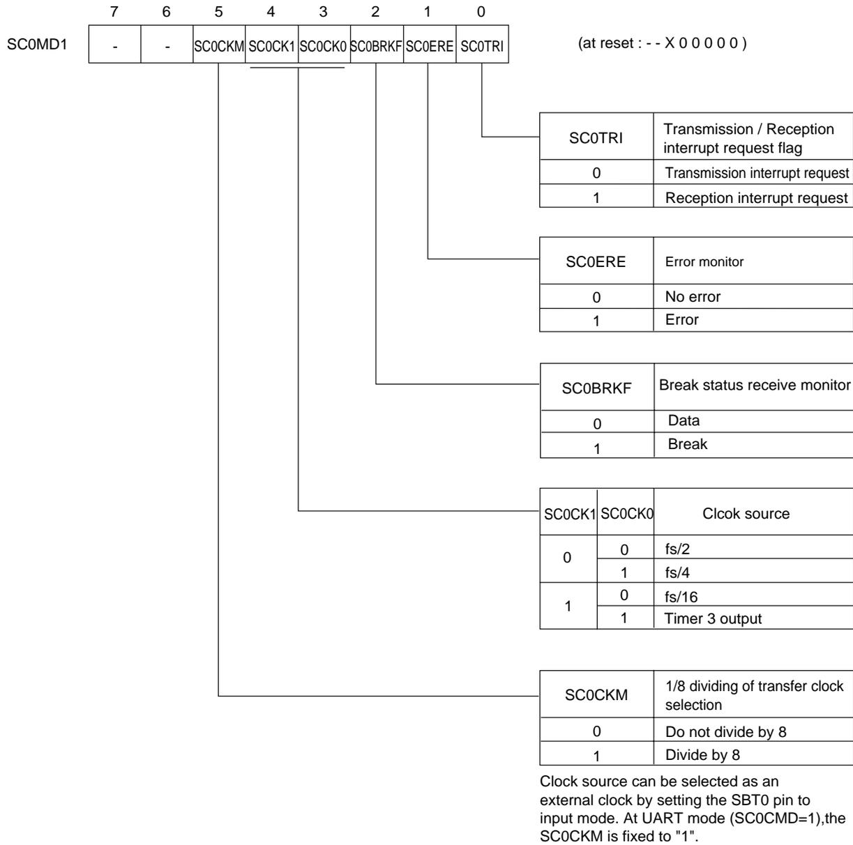
Figure 10-2-4 Serial Interface 0 Mode Register 1 (SC0MD1 : x'03F51', R/W)
