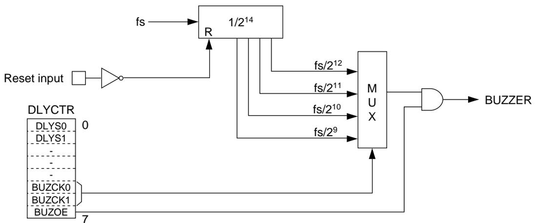
Figure 9-1-1 Block Diagram (Buzzer)
