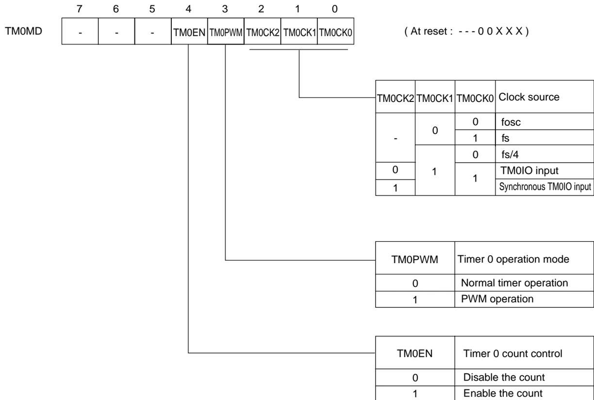
Figure 5-2-9 Timer 0 Mode Register (TM0MD : x'03F80', R/W)
