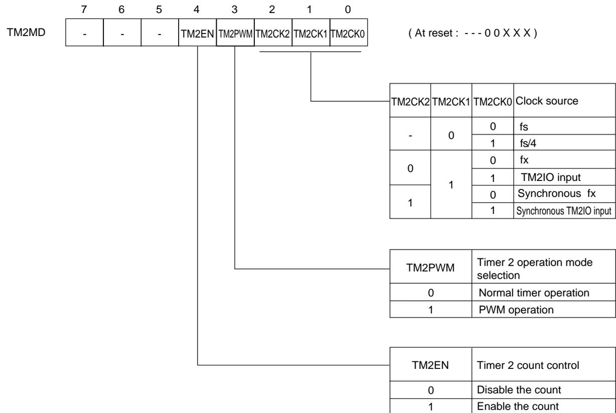
**Figure 5-2-11 Timer 2 Mode Register (TM2MD : x'03F82', R/W)**
