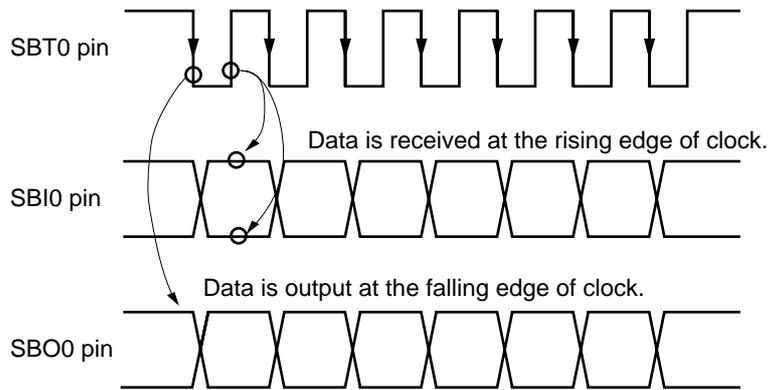
**Figure 10-3-9 Transmission / Reception Timing**
