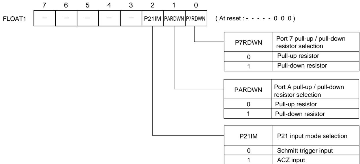
Pin control register 1 (FLOAT1 : X'03F4B', R/W)
