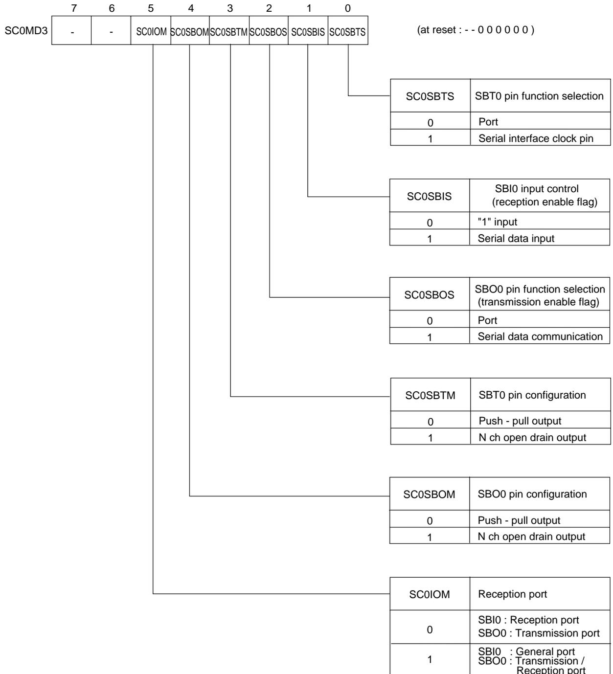
Figure 10-2-6 Serial Interface 0 Mode Register 3 (SC0MD3 : x'03F53', R/W)
