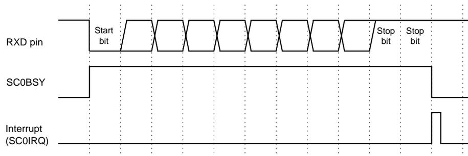
Figure 10-3-15 Reception Timing (parity bit is disabled)
