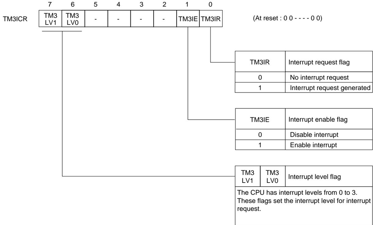
Figure 3-2-10 Timer 3 Interrupt Control Register (TM3ICR : x'03FEE', R/W)
