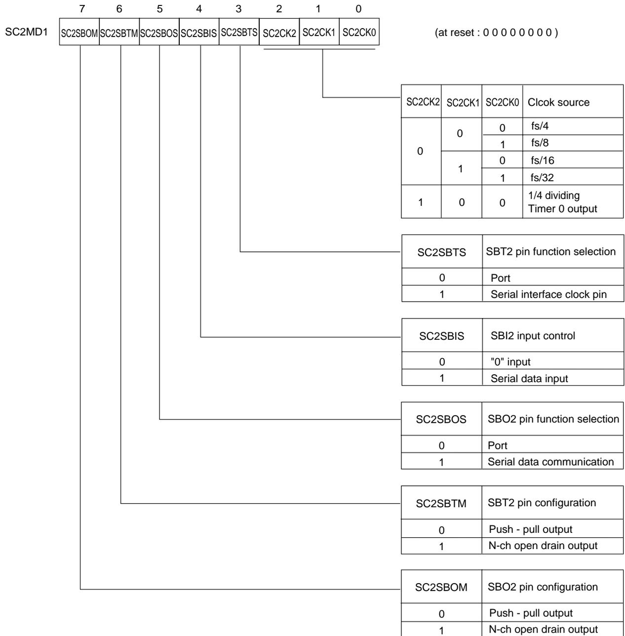
Clock source can be selected as an external clock by setting the SBT2 pin to input mode.
