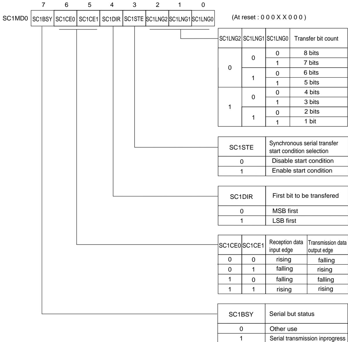
Figure 11-2-2 Serial Interface 1 Mode Register 0 (SC1MD0 : x'03F57', R/W)
