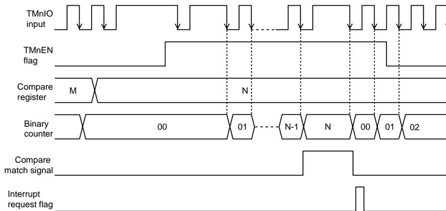
**Figure 5-4-1 Count Timing of TMnIO Input (Timers 0 to 3)**
