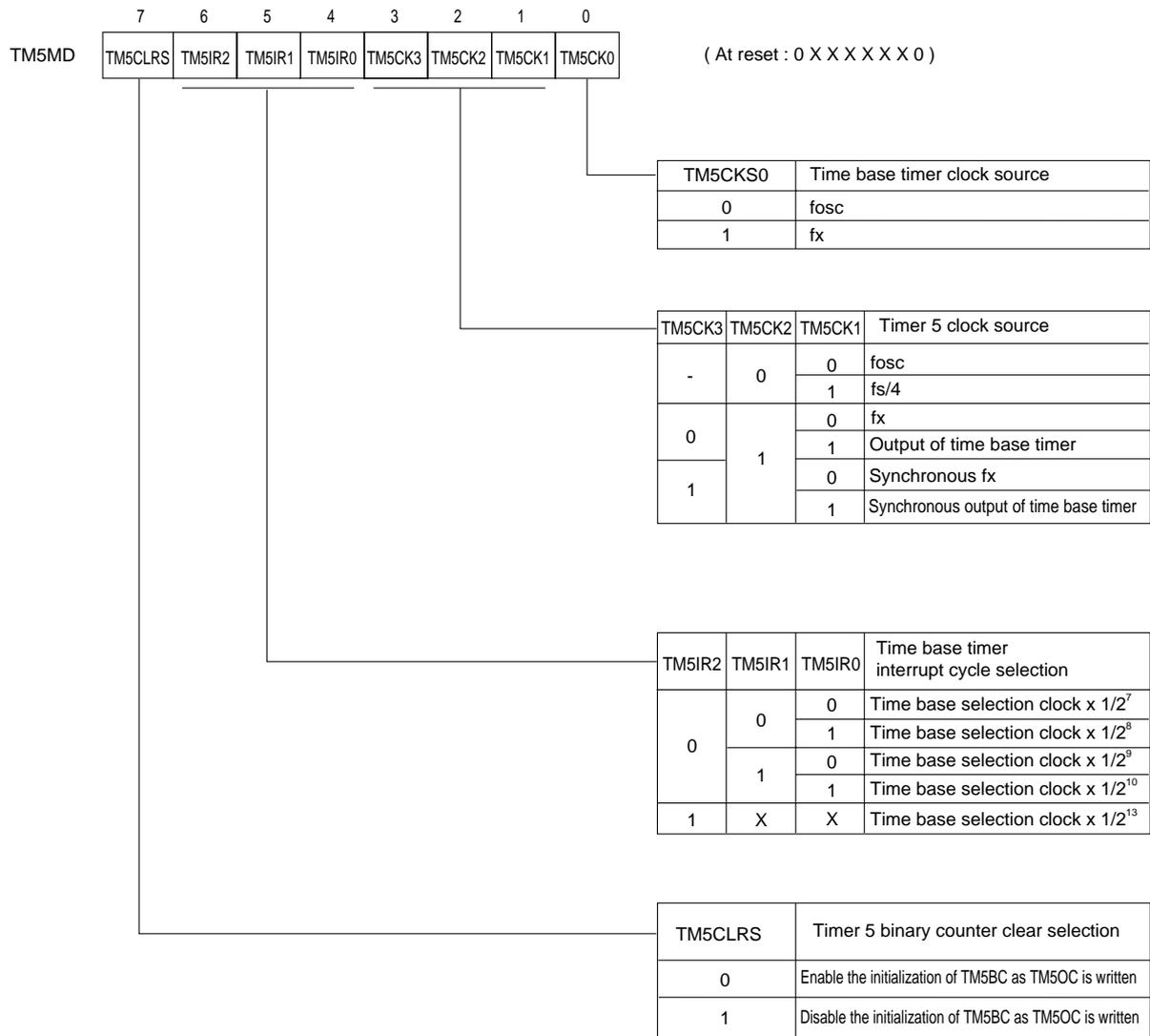
Figure 7-2-3 Timer 5 Mode Register (TM5MD : x'03F88', R/W)
