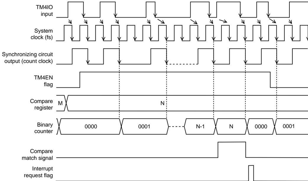
Figure 6-4-2 Count Timing of Synchronous TM4IO Input (Timer 4)
