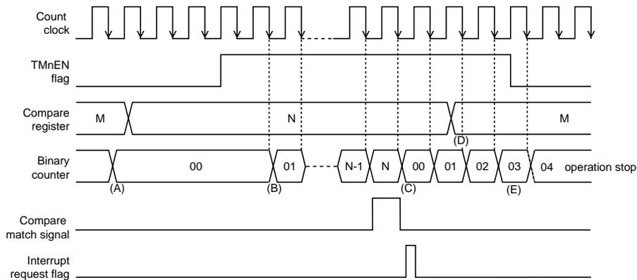
**Figure 5-3-1 Count Timing of Timer Operation (Timers 0, 1, 2 and 3)**
