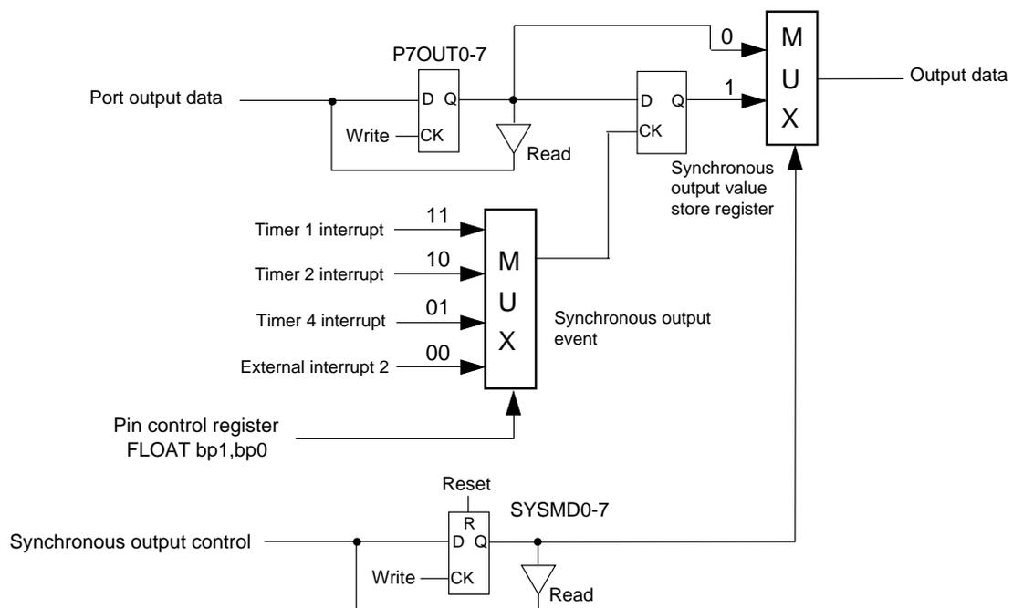
Figure 4-12-1 Synchronous Output Control Block Diagram
