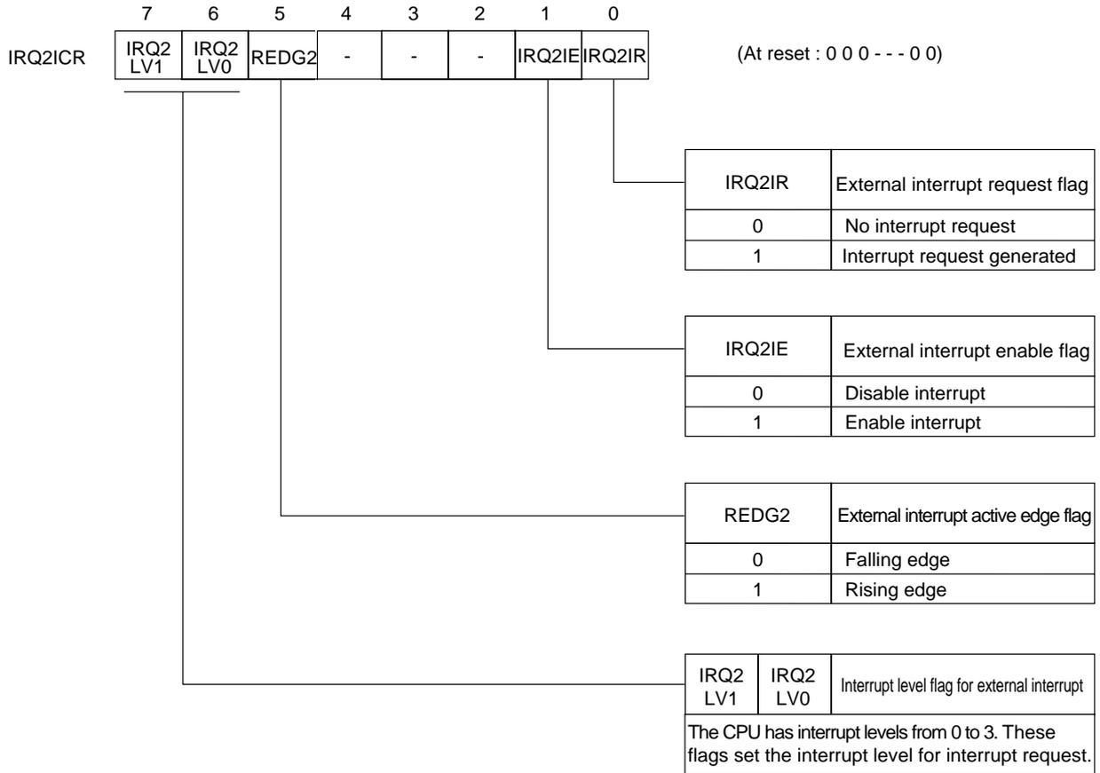
Figure 3-2-4 External Interrupt 2 Control Register (IRQ2ICR : x'03FEB', R/W)
