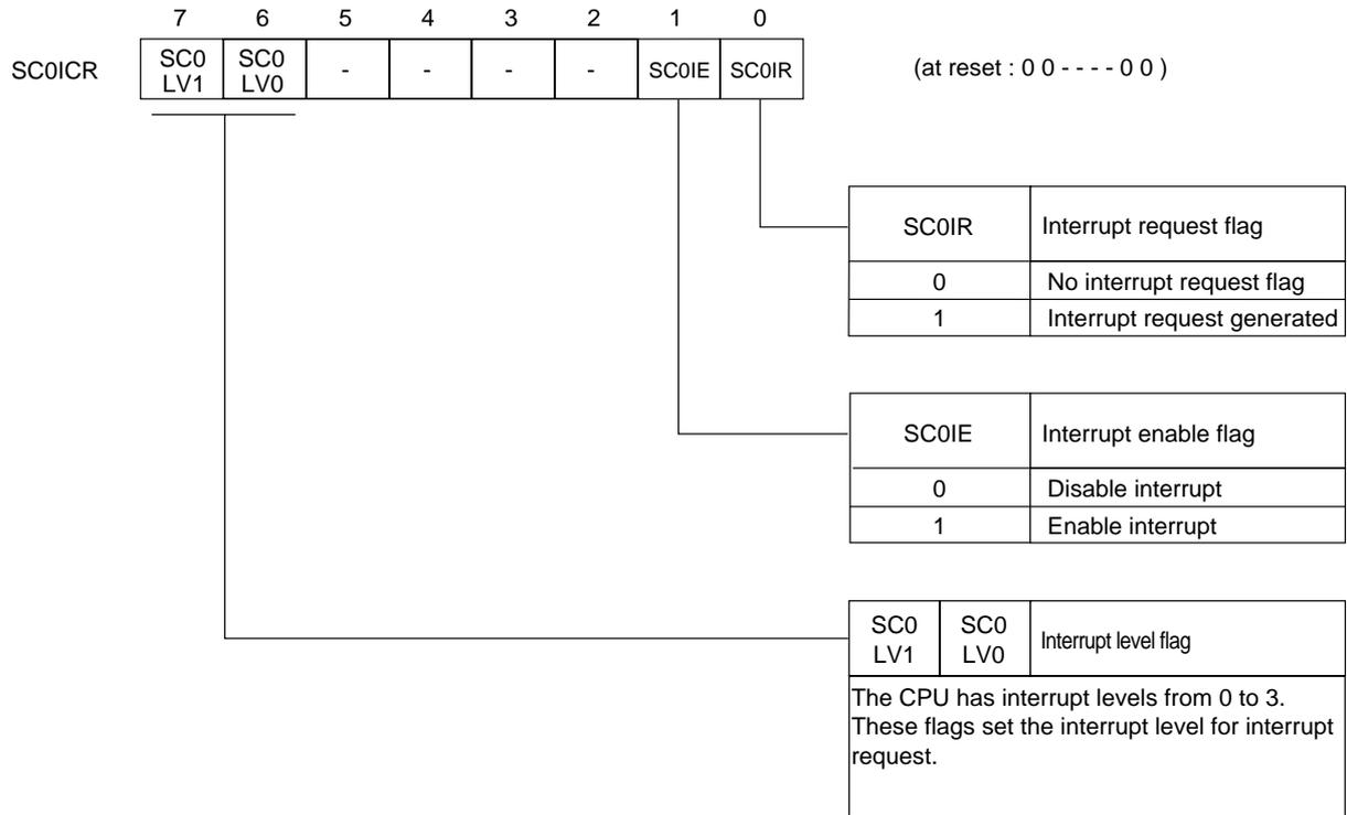
Figure 3-2-14 Serial interface 0 Interrupt Control Register (SC0ICR : x'03FE8', R/W)
