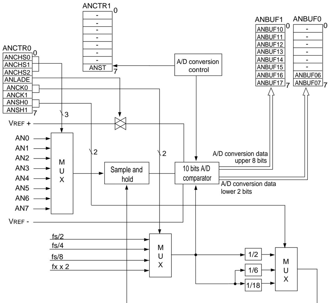
Figure 14-1-1 A/D Converter Block Diagram
