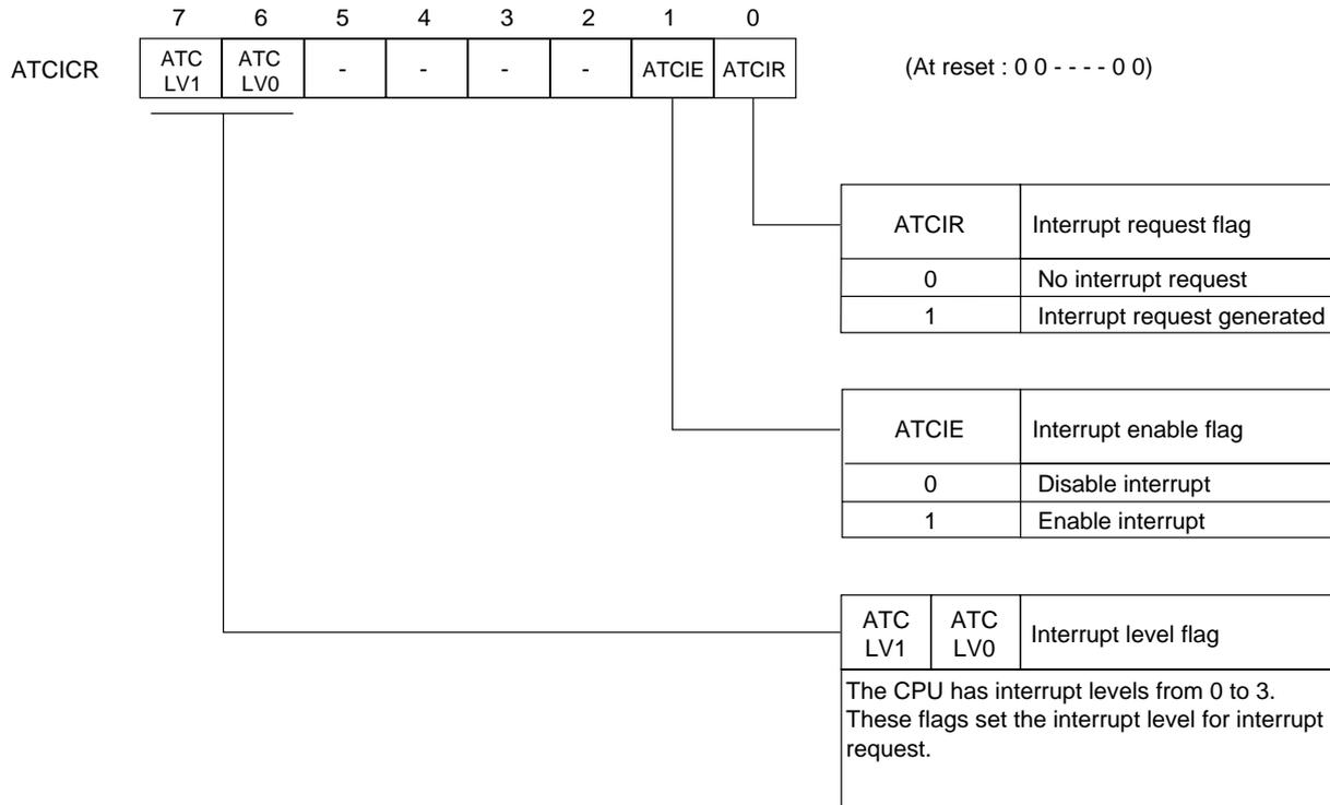
Figure 3-2-18 ATC Interrupt Control Register (ATCICR : x'03FE9', R/W)
