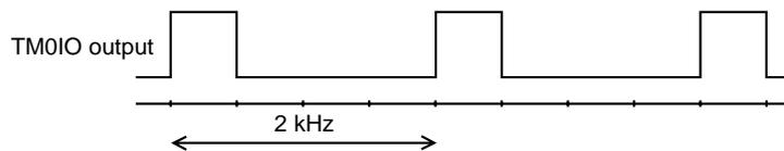
**Figure 5-6-4 Output Waveform of TM0IO Output Pin**
