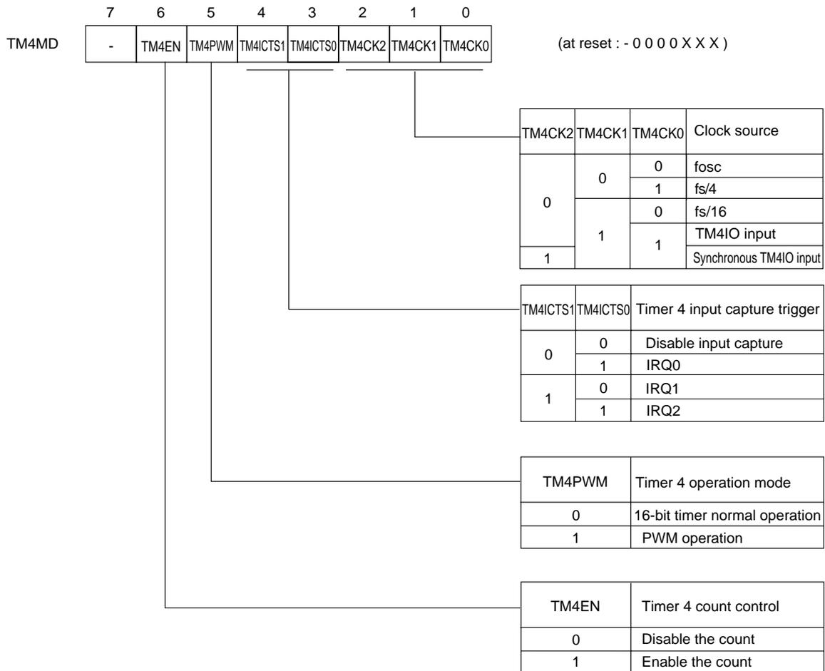
Figure 6-2-7 Timer 4 Mode Register (TM4MD : x'03F84', R/W)
