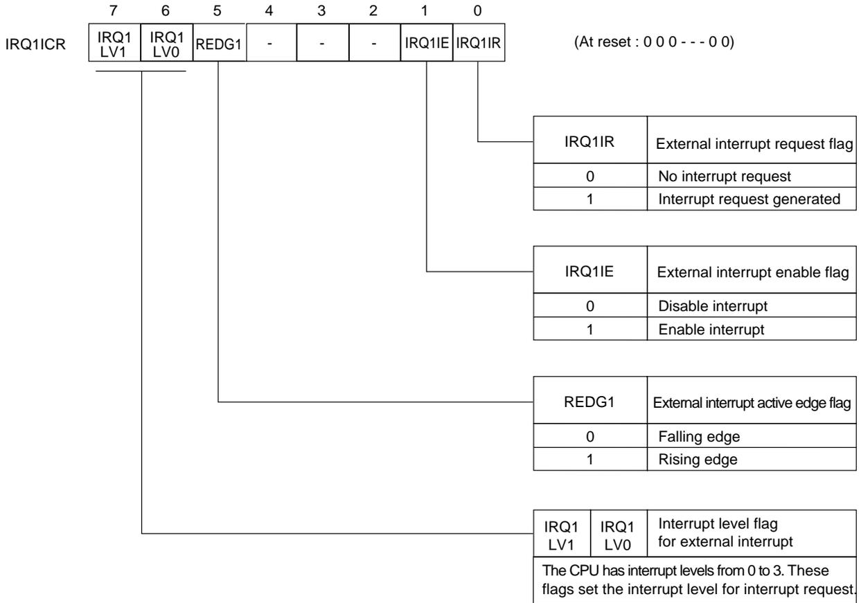
Figure 3-2-3 External Interrupt 1 Control Register (IRQ1ICR : x'03FE3', R/W)
