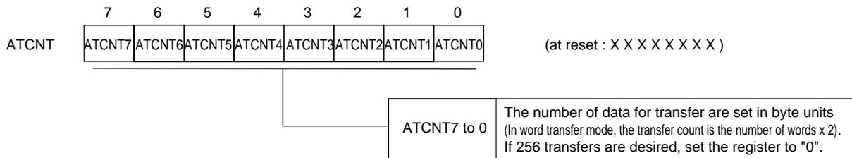
**Figure 13-2-2 Transfer Data Counter (ATCNT : x'03FA1', R/W)**
