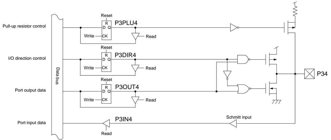
Figure 4-5-6 Block Diagram (P34)
