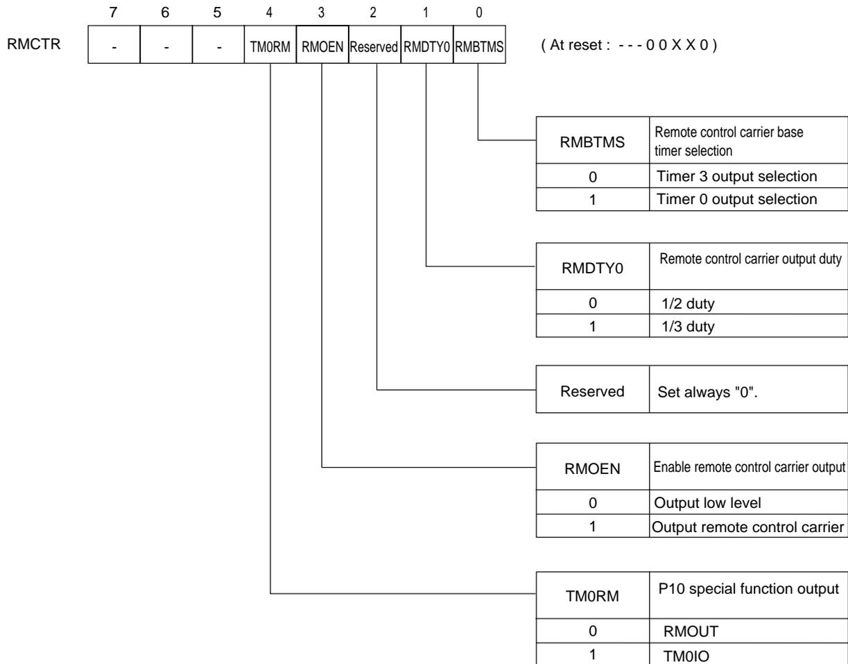
Figure 5-2-13 Remote Control Carrier Output Control Register (RMCTR : x'03F89', R/W)
