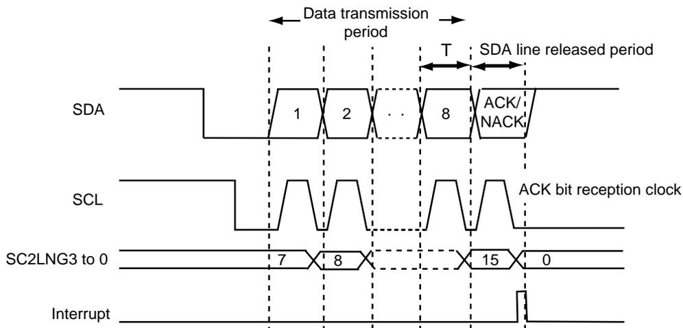
Figure 12-3-10 ACK Bit Reception Timing after Transmission of 8-Bit Data
