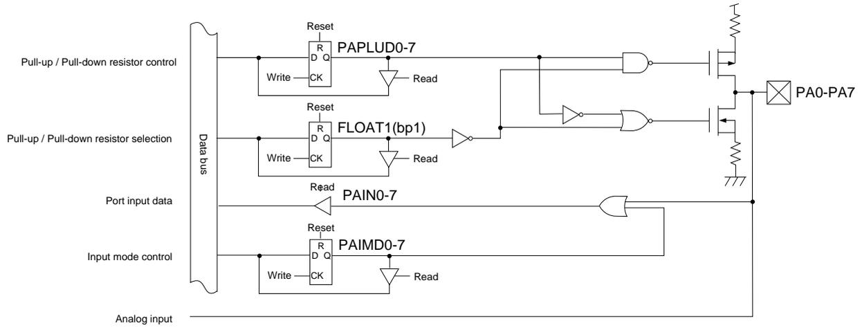
**Figure 4-11-3 Block Diagram (PA0 to PA7)**
