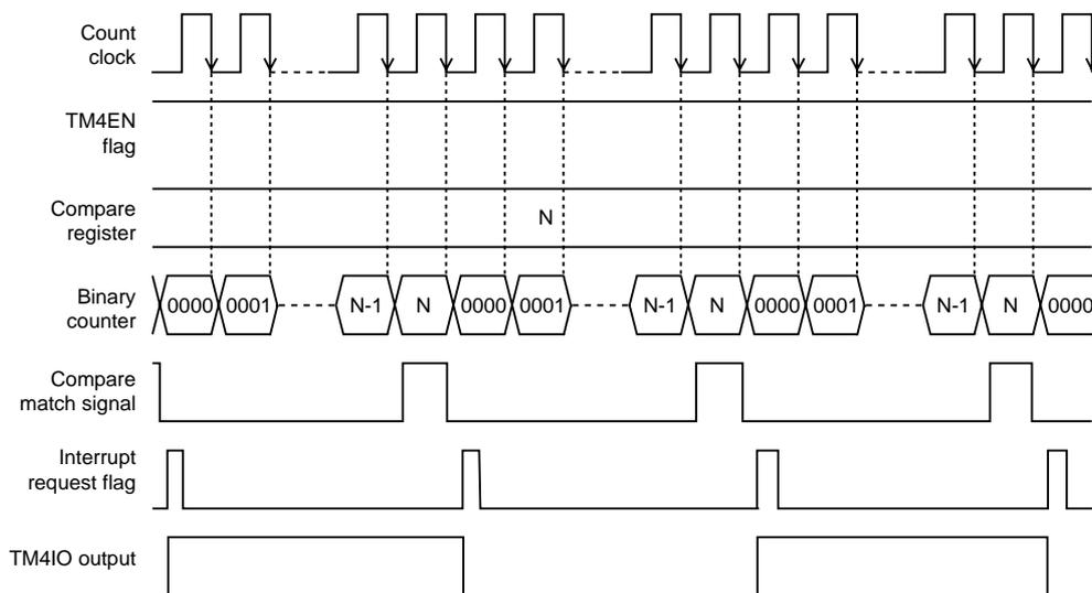
**Figure 6-5-1 Count Timing of Timer Pulse Output (Timer 4)**
