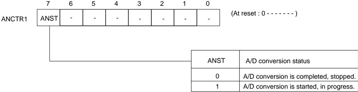
Figure 14-2-2 A/D Converter Control Register 1 (ANCTR1 : x'03F91', R/W)
