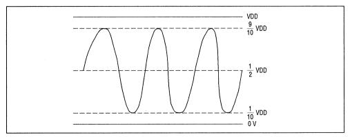
Figure 10 Waveform When the Maximum Amplitude Level of the Input Waveform is about 80% of the Dynamic Range
