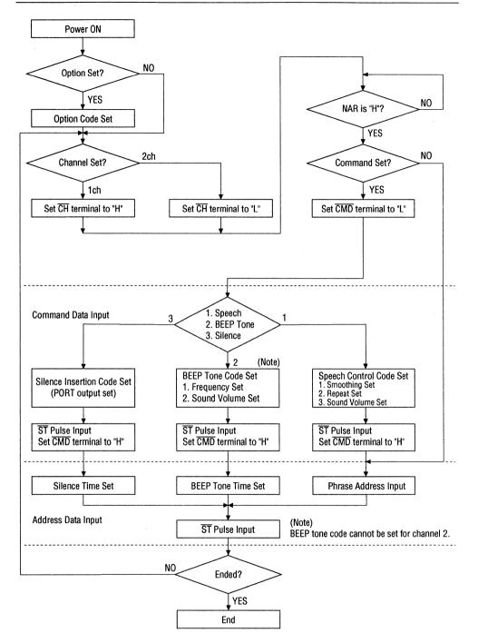
Figure 4.4 Parallel Input Flow Chart when External Command Is Used.
