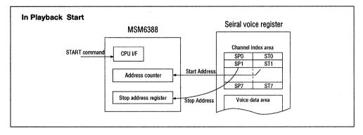
When STOP command is inputted, the playback finishes. The MSM6388 does not exchange the data with the channel index area.
