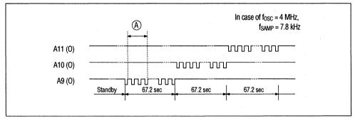
Figure 15 Address Timing for 256 x 4-Bit DRAM
