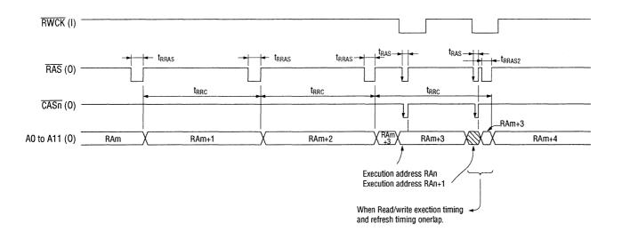
DRAM Drive Timing (When execution timing and refresh timing overlap)
