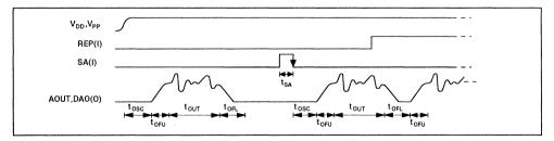
Note: When REP pin is merely set to "H" level, the speech is not output.
