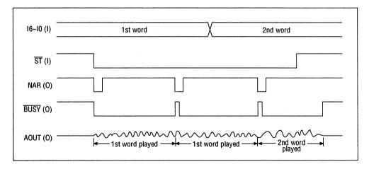
Figure 4 Timing of SW Input Interface (repeated play)
