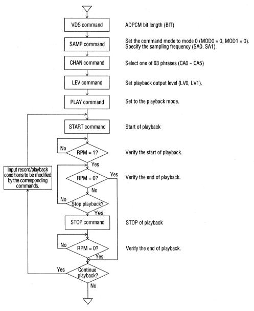
This flow chart can apply to the playback operation in the direct record/playback mode, excluding that the command mode is set to mode 2 by the SAMP command and one of 64 phrases (ch00–ch3F) can be selected by the CHAN command in the direct record/playback mode.
