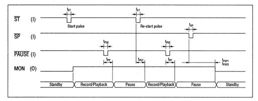
Note: t<sub>PSP1</sub>------ for recording or playback with the PDMD pin = "H" t<sub>PSP2</sub>------ for recording or playback with the PDMD pin = "L"
