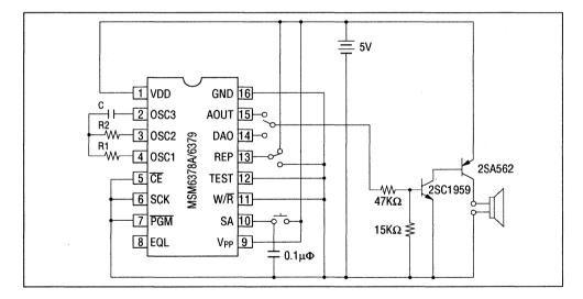
Note: If 5V or less is used, change the constant used to divide the resistor in the output stage.
