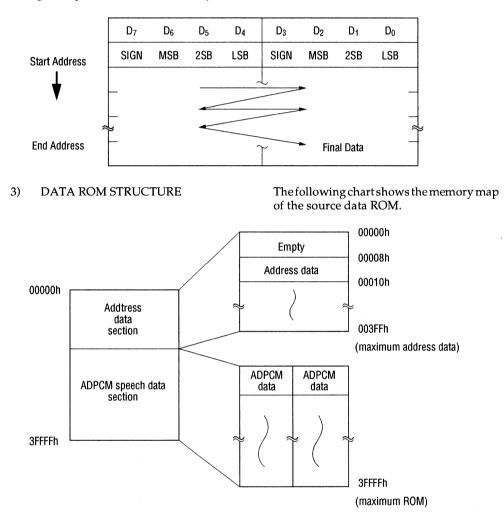
When the maximum 127 phrases are selected in address data section, the data is written up to ROM address 003FFh. When 1 phrase is selected, address data is written from ROM address 00008h to 0000Fh, and the rest is used as the ADPCM data section.
