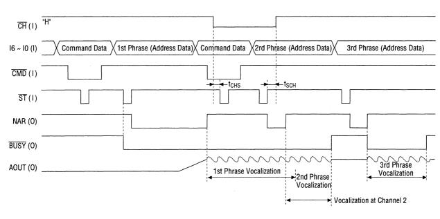
Since command data is maintained independently at channels 1 and 2, If speech is started up at channel 1 without a command setting, speech is vocalized by the same command set at the 1st phrase.
