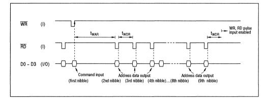
Note 1: In the BUSY bit of the status register, input the command after checking that it is not in the BUSY state.
