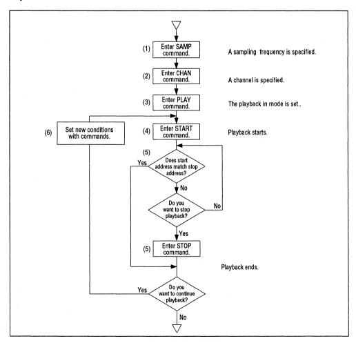
Playback flowchart when the LSI is connected to a microcontroller interface
