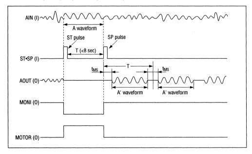
4) After inputting SP pulse, ST pulse is input 8 sec. later. Same as 2).
