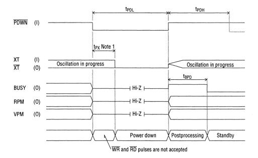
**Note 1:** When an external clock is used, apply a low level to the  $\overline{\text{PDWN}}$  pin and then continue to apply the external clock to the XT pin for t<sub>PX</sub>.
