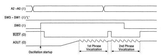
Figure 5.3 Complete SW Input Interface Vocalization Timing
