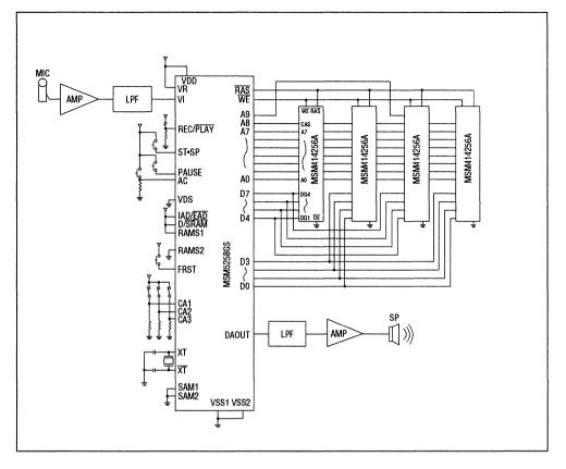
Figure 27 Application Note for 1M-bit DRAM
