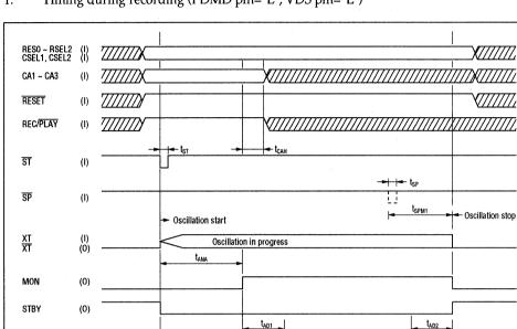
1. Timing during recording (PDMD pin="L", VDS pin="L")
