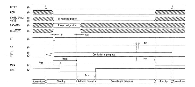
Timing for Voice Activated Recording (PDMD Pin = High)
