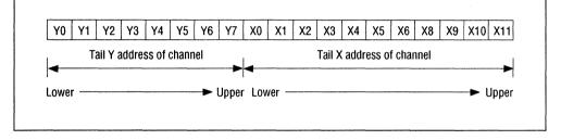
The X addresses of the voice data area are 008h-FFFh (when connecting the serial voice register for 4Mbit).
