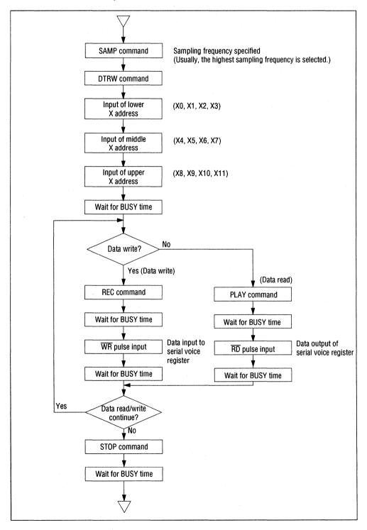
Method of record/playback by input /output of voice data from the data bus (EXT command)
