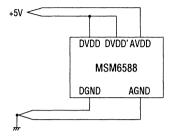
It is not permitted to have two power supplies for the analog section and the logic section separately because it may cause a latch-up.
