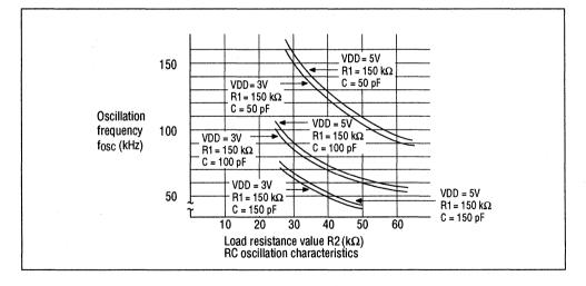
Figure 12 RC Oscillation Frequency
