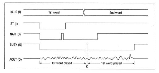
Figure 2 Timing of CPU Interface ( $\overline{ST} > 800 \ \mu S$ )
