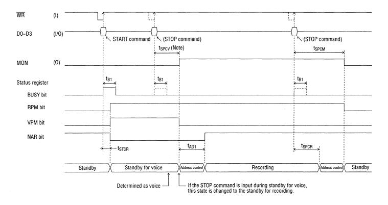
Note:  $t_{scv}$  varies depending on the recording mode (flex recording or direct recording).
