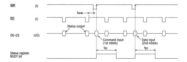
The LEV command is used to specify the playback level. See the timing diagram for DC level transition by the LEV command.
