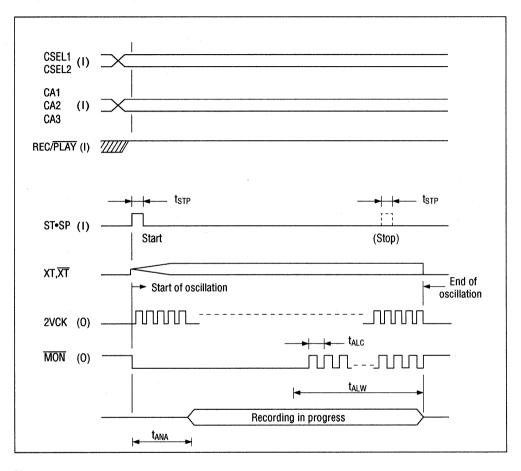
Note: When the remaining capacity of available memory of the selected channels falls to 128K-bit (last four seconds) during recording, a 4Hz clock is output from the MON pin. (f<sub>sam</sub>=8kHz)
