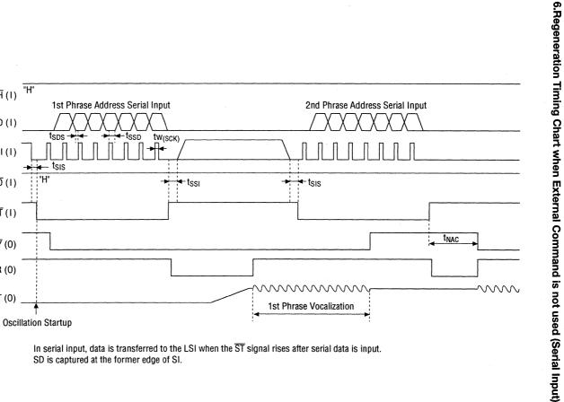
In serial input, data is transferred to the LSI when the ST signal rises after serial data is input. SD is captured at the former edge of SI.
