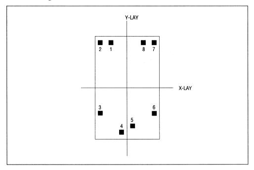
Pad Positions (the die center is located at X=0, Y=0)
