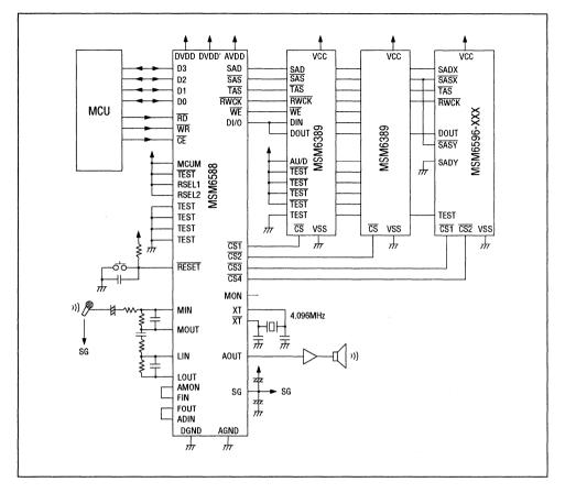
Note: MSM6588 can not control the Serial voice ROM without use of Serial voice registers.
