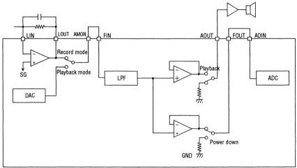
Note: This diagram shows the state of each switch during the recording operation.
