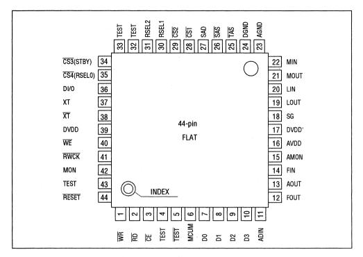
Selection of stand-alone mode or microcontroller interface mode is controlled by the level of the MCUM pin. MCUM="H": microcontroller interface mode
