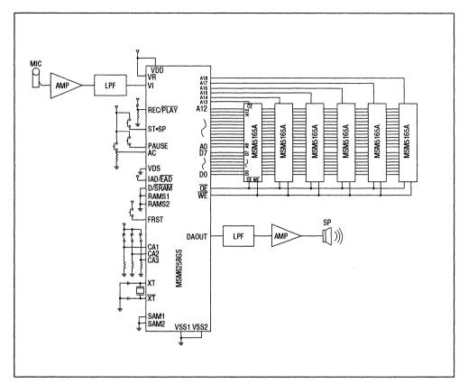
Figure 23 Application Note for 64K SRAM
