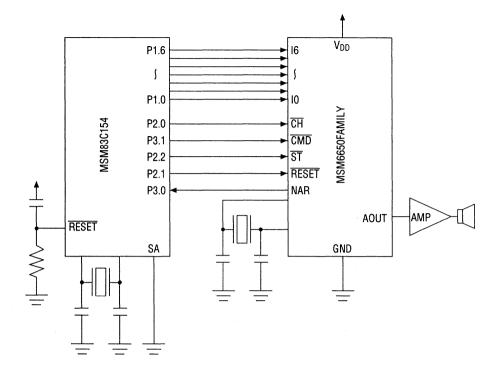
Example of Application Circuit at Parallel Input Interface
