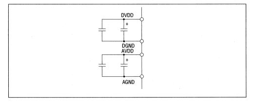
Note: The voltages of AVDD and DVDD should rise from 0V to 4V within 2ms when the power is risen.
