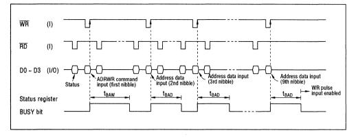
Note 1: In the BUSY bit of the status register, input the command after checking that it is not in the BUSY state.Note 2: Next, input the address data into 2nd through 9th nibble command, but after checking that the status is
