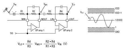
During the time the recording operation is performed, the output  $V_{LO}$  of OP amp 2 is connected to the input FIN of the built-in LPF. The FIN allowable input voltage ( $V_{FIN}$ ) ranges from 1V to ( $V_{DD} - 1$ )V. Therefore, the amplification ratio must be adjusted so that the  $V_{LO}$  amplitude can be within the FIN allowable input voltage range.
