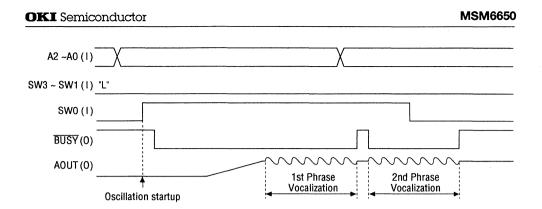
Figure 4.3 Complete SW Input Interface Repeat Vocalization Timing
