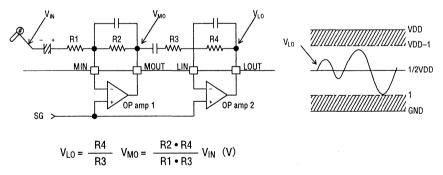
During the time the recording operation is performed, the output  $V_{LO}$  of OP amp 2 is connected to the input FIN of the built-in LPF. The FIN allowable input voltage ( $V_{FIN}$ ) ranges from 1V to ( $V_{DD} - 1$ )V. Therefore, the amplification ratio must be adjusted so that the  $V_{LO}$  amplitude can be within the FIN allowable input voltage range.
