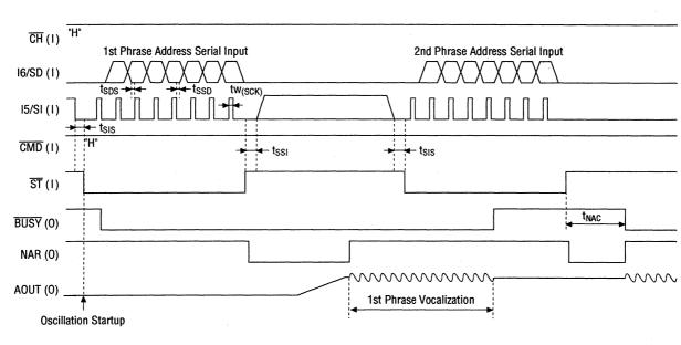
In serial input, data is transferred to the LSI when the  $\overline{ST}$  signal rises after serial data is input. SD is captured at the end before SI.
