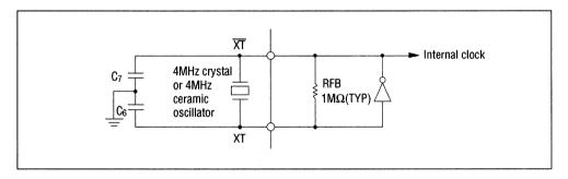
Figure 5 Oscillation Circuit
