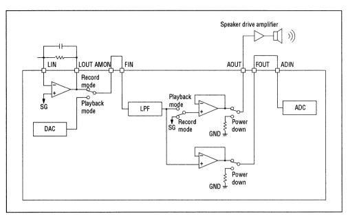
Note: Switches in the figure denote the state during record operation.
