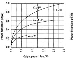
Power dissipation vs output power (example)
