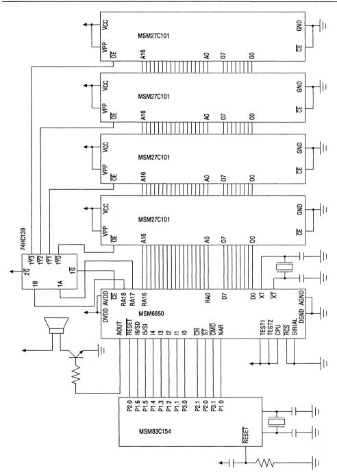
Application circuit example when four 1 M-bit EPROMs are used (parallel input interface).
