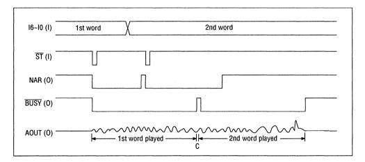
Figure 1 Timing of CPU Interface (ST ≤ 350µs)
