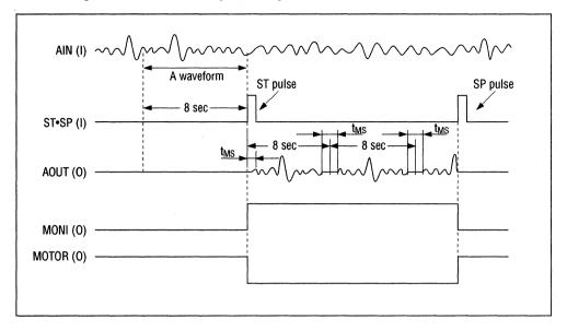
2) After power is turned on, ST pulse is input 8 sec. later.
