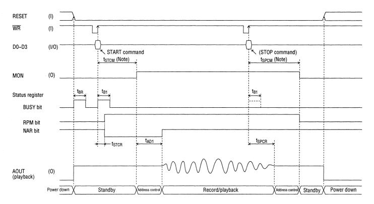
Note: tSTCM and tSPCM vary depending on the control mode for record/playback and on record or playback mode.
