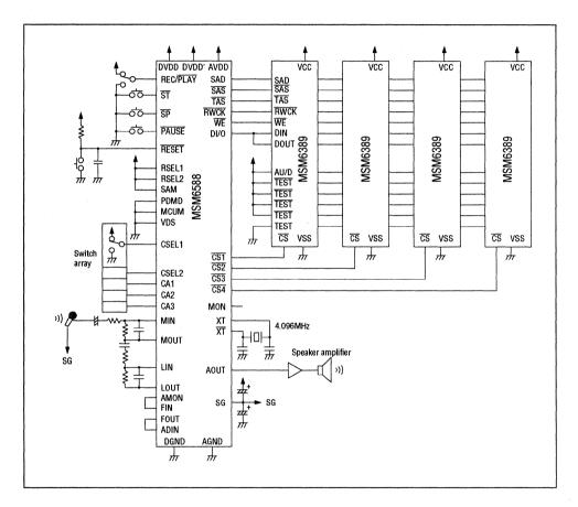
Figure 1 Example of Application Circuit in Stand-alone Mode and with 1Mbit Serial Voice Registers
