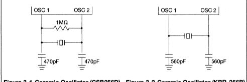
Figure 3-1 Ceramic Oscillator (CSB256D) Figure 3-2 Ceramic Oscillator (KBR-256B) Connection Circuit Connection Circuit
