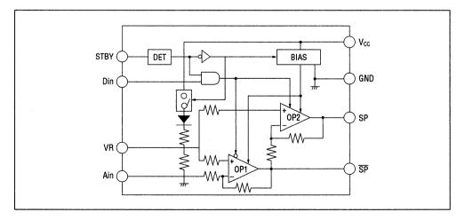
Note: MSC1191: Standby mode is activated by "H" level to the input STBY MSC1192: Standby mode is activated by "L" level to the input STBY
