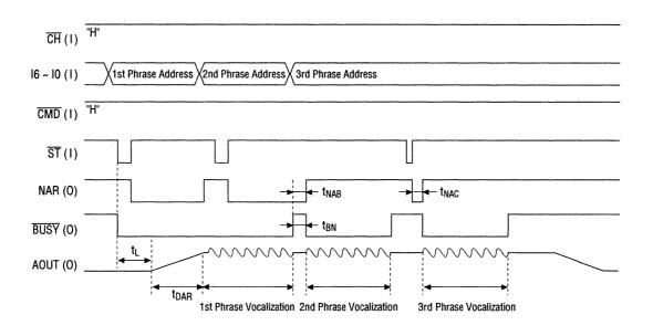
4. Channel 1 Regeneration Timing Chart when External Command Is Used (Parallel Input)
