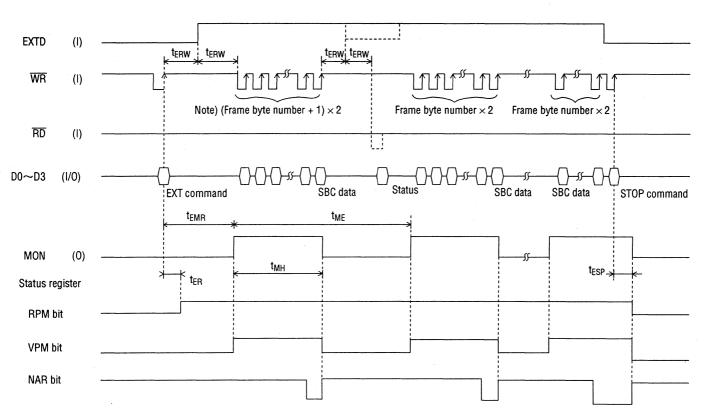
Note) During playback, the 1st frame writes (byte number in a frame + 1 byte), and the following frames writes the byte number of each frame.
