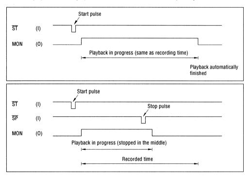
By maintaining the  $\overline{ST}$  pin at "L" level, repeated playback is possible.
