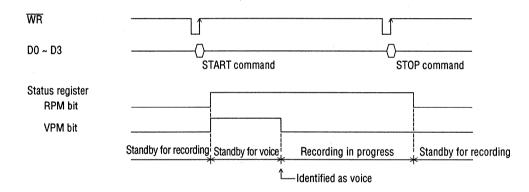
When the STOP command is input during standby for voice, standby for voice will be finished and changed to standby for recording,
