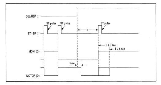
Note 1: If T is 8 sec. or longer, MOTOR rises at the same time when ST pulse is input. Note 2: If T is 8 sec. or shorter, MOTOR rises 8 seconds after DEL/REP is selected.
