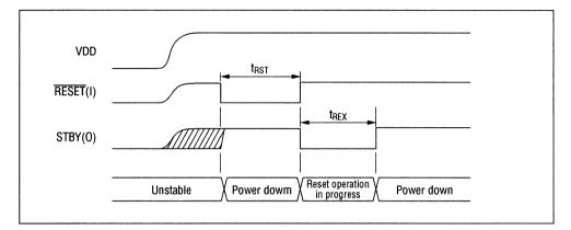
2. Stand-alone mode when the PDMD pin is "H" and in microcontroller interface mode.
