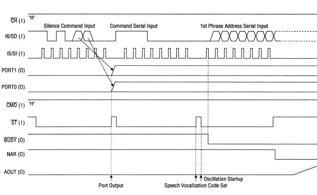
In serial input, port output can be set by a command setting. Since a port output command and internal command are shared, if a command is set for port output, set the command for speech again to input address data. If address data is input without setting the command, the LSI recognizes it as silence insertion code.
