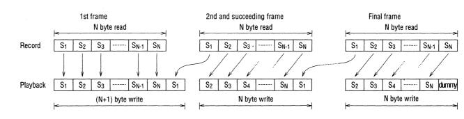
N: SBC data amount at one frame Sn: SBC data at n byte at any frame
