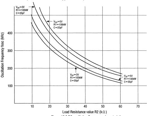
Figure 13.2 RC oscillation Frequency eharacteristics
