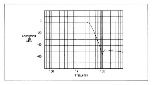
Figure 8 Low-pass Filter Characteristics (fs=8 kHz)
