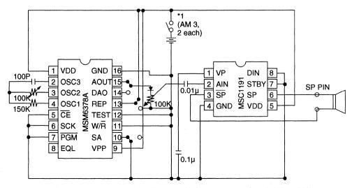
\* Note: The guaranteed voltage of LPF output of MSM6378 ranges from 2.7 V  $\sim$  5.5 V.
