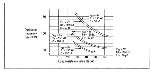
Figure 12 RC Oscillation Frequency Characteristics
