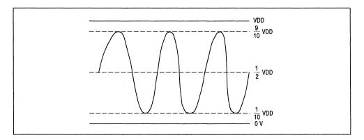
Figure 6 Waveform When the Maximum Amplitude Level of the Input Waveform is about 80% of the Dynamic Range.
