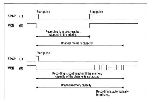
Note: As mentioned above, the memory capacity of the external serial registers is divided by the number of phrases and is assigned as the channel memory capacity. During recording, ADPCM data is written, starting from the first address of the memory of the specified channel. When recording is terminated in the middle of the channel memory capacity by a stop pulse, the subsequent memory area remains unused.
