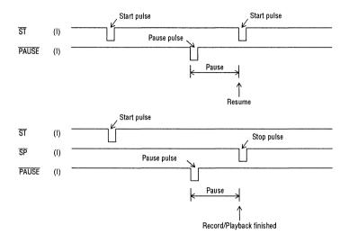
When record/playback is resumed after temporary stop, the voice activating circuit is not operated and recording is started when a start low pulse is applied to SP pin.
