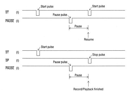
When record/playback is resumed after temporary stop, the voice activating circuit is not operated and recording is started when a start low pulse is applied to SP pin.
