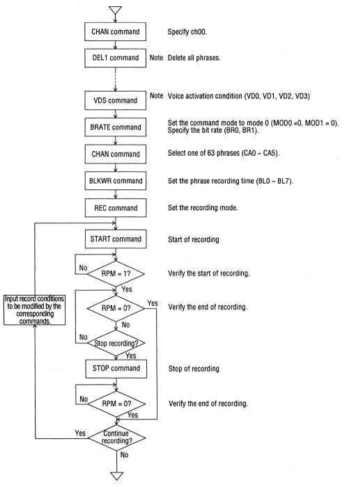
Note: Setting of the command mode by BRATE command is deleted in this flow chart.
