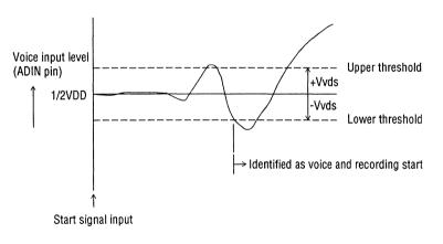
Specify the enable/disable of the voice activated recording function and the voice detection level by VD0 and VD1 bit data of the VDS command as shown in the following table.
