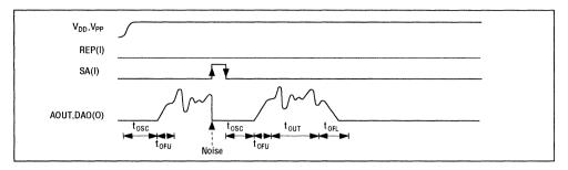
Note: When SA pin goes to "H" level during playback, speech is stopped and a noise is output.
