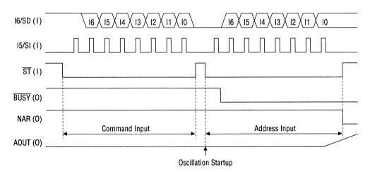
Figure 4.2 Command, Address Input Timing (Serial Input)
