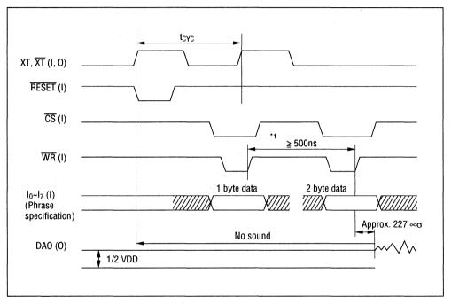
Note: Phrase selection is from channel 1 to channel 4 continuously. \*1 An interval of 75 T<sub>CYC</sub> (max.) is needed between phrases.
