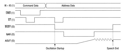
Figure 4.1 Command, Address Input Timing (Parallel Input)
