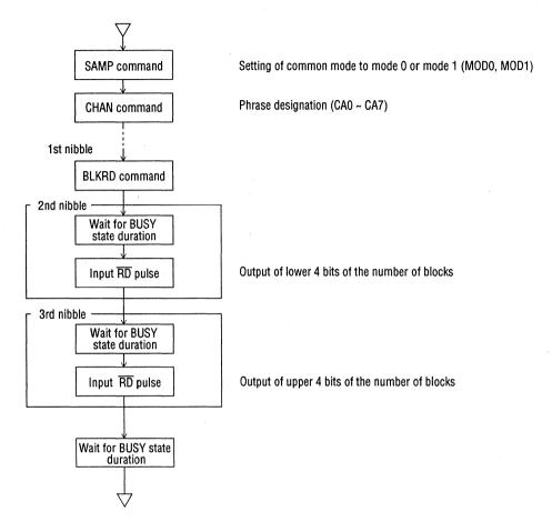
During execution of the BLKRD command, verification of the status register cannot be performed by input of the RD pulse. When inputting the RD pulse for the 2nd nibble or 3rd nibble or inputting the next command after the BLKRD command, input the RD pulse either after the waiting time longer than the BUSY state duration or after verifying that the BUSY status is not present via the BUSY pin.
