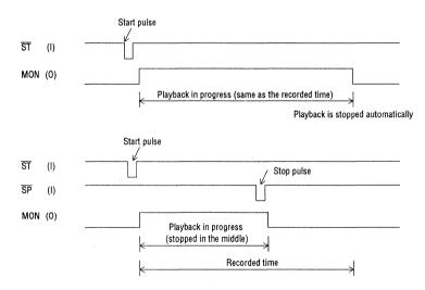
By maintaining the ST pin at a low level, repeated playback is possible.
