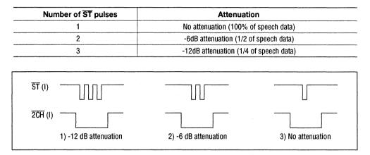
Figure 7 Input Timing of 2-Channel Mixing
