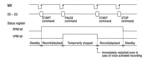
When the STOP command is input during temporarily stopped state, the record/playback operation is finished and the MSM6788 is placed in the standby state.
