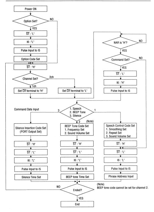
Figure 5.4 Parallel Input Flow Chart when External Command is used.
