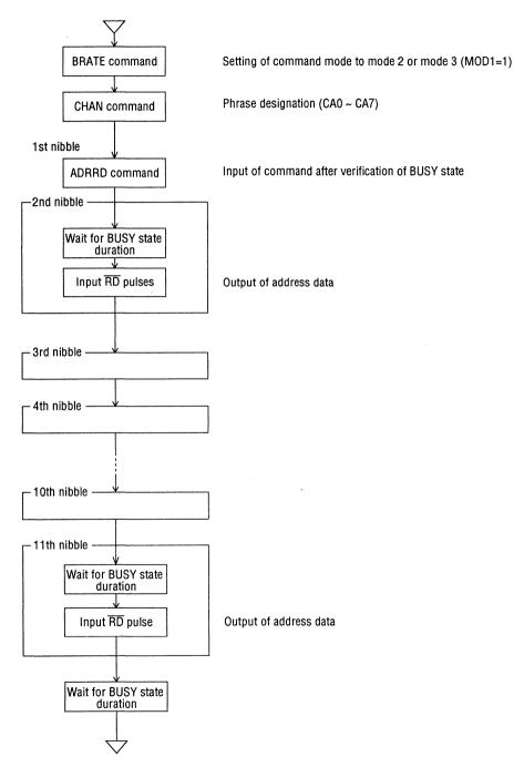
During execution of the ADRRD command, verification of the status register cannot be performed by input of the RD pulse. When inputting the RD pulse for the 2nd nibble to 11th nibbles or inputting the next command after the ADRRD command, input the RD pulse either after the waiting time longer than the BUSY state duration or after verifying that the BUSY status is not present via the BUSY pin.
