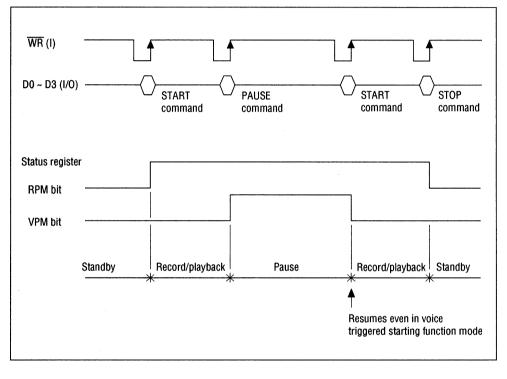
Input of the STOP command during pause, record/playback is finished and the LSI en-
