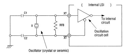
Figue 1 Crystal/Ceramic Oscillation Circuit
