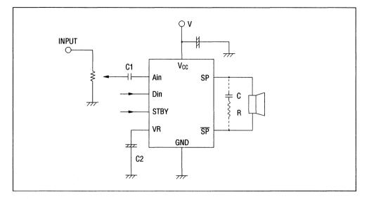
• C1 is the AC coupling capacitance. Low cut off frequency fc can be obtained by the following equation:
