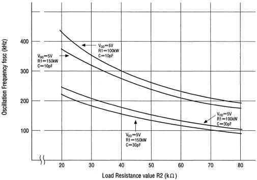
Figure 12.1 RC oscillation Frequency eharacteristics
