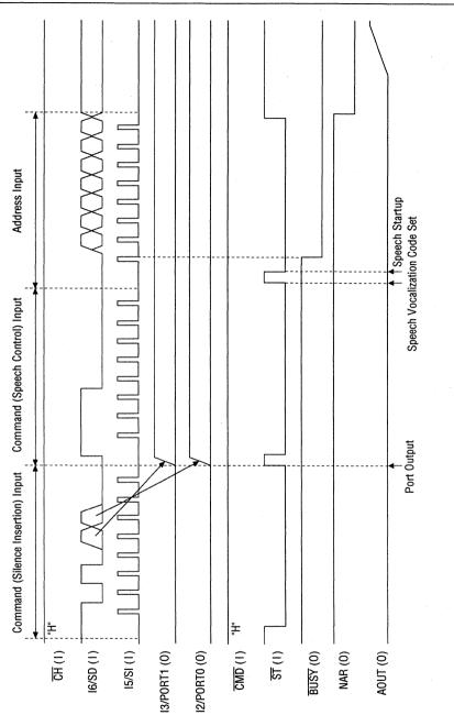
Figure 6.3 Port Output and Command, Address Setting Timing (during Serial Input)
