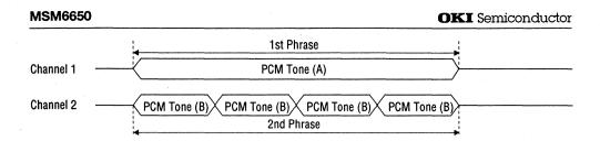
Figure 9.9 Example of Channel Synthesis between PCM Main Melody Tone (A) and PCM Rhythm Tone (B) with 4 Repeats
