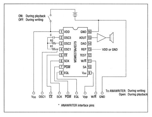
Note: \* Be careful about noise margin for input pins that are open during playback.
