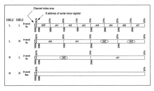
By combining CSEL1, CSEL2, CA1, CA2 and CA3, it is possible to assign (the encircled channels) ch0=16 seconds, ch2=8 seconds and ch3=8 seconds (f<sub>sam</sub>=8kHz, 4 bit ADPCM).
