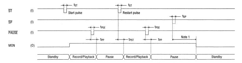
Note 1: This time interval varies depending on the state of PDMD pin and the record/playback mode and is one of t<sub>PMH1</sub>, t<sub>PMH2</sub>, t<sub>PMH3</sub>, t<sub>PML1</sub>, t<sub>PML2</sub> and t<sub>PML3</sub>.
