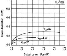
Power dissipation vs output power (example)
