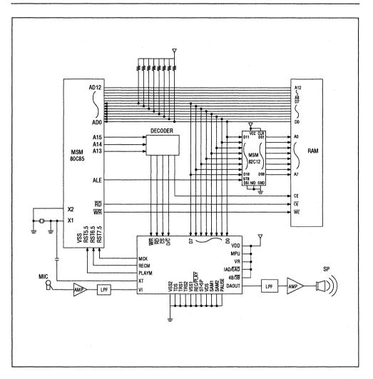
Figure 32 Example of Interface with MSM80C85
