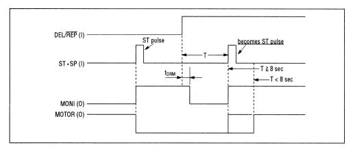
**Note 1:** If T is 8 sec. or longer, MOTOR rises at the same time when ST pulse is input. **Note 2:** If T is 8 sec. or shorter, MOTOR rises 8 seconds after DEL/REP is selected.
