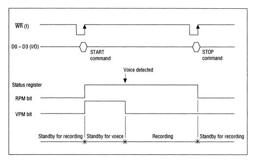
Input of a STOP command during standby for voice causes the LSI to first finish standby
