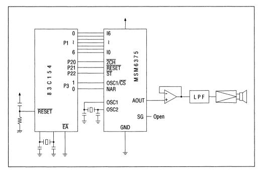
Figure 16 Application Circuit Example in the Case of Selecting XT, DAC and CPU in Option
