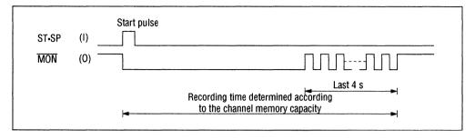
Note: During the last four seconds a clock frequency of 4 Hz described above is output, when the sampling frequency (f<sub>sam</sub>) of 8.0 kHz is selected. The duration of the alarm clock is proportional to the length of the cycle of the sampling frequency and the clock frequency is proportional to the sampling frequency used.
