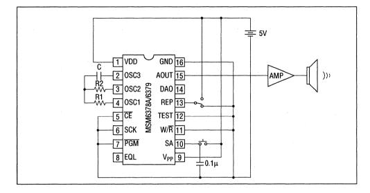
Note: The capacitor connected to the SA pin contributes to noise margin in the case of SA being "open"
