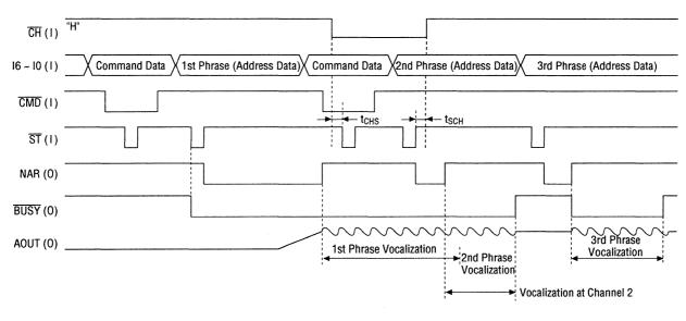
Since command data is maintained independently, if speech is started up at channel 1 without a command setting, speech is vocalized by the same command set at the 1st phrase.
