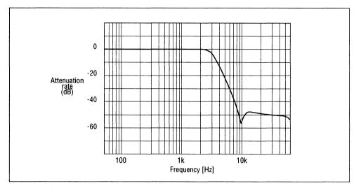
Figure 8 Low-pass Filter Characteristics (fs=8 kHz)
