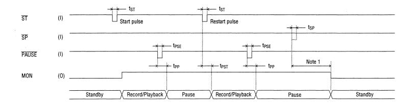
Note 1: This time interval varies depending on the state of PDMD pin and the record/playback mode and is one of t<sub>PMH1</sub>, t<sub>PMH2</sub>, t<sub>PMH3</sub>, t<sub>PML2</sub> and t<sub>PML3</sub>.
