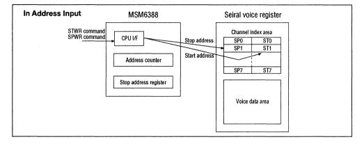
When START command is inputted, the recording is started after the start addresses of channel index area are automatically set
