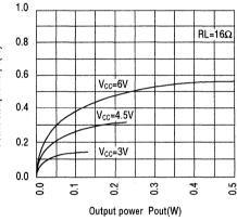
Power dissipation vs output power (example)
