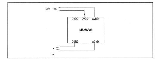
If the analog portion and logic portion are suppled from a separate power source, make sure the voltage difference between both power sources does not exceed  $\pm 3$  volts or latch-up may occur.
