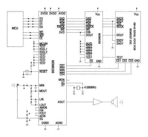
Note: When MSM6597 is driven by MSM6388 or MSM6588, a serial register is required. (MSM6597 can not operate without it.)
