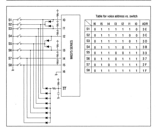
Figure 17 Application Circuit Example to Output the Voice of 8 Words by Switch Interface
