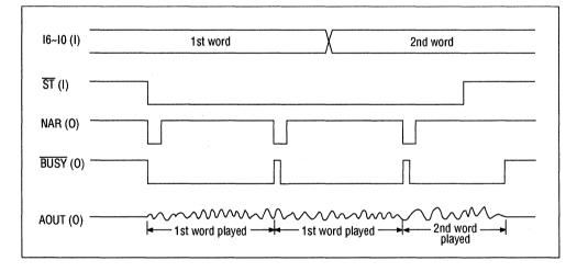
Figure 4 Timing of SW Input Interface (repeated play)
