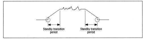
Figure 9 Pop Noise of Low-pass Filter Output
