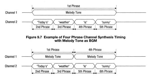
Figure 9.8 Example of Four Phrase Channel Synthesis Timing with Melody Tone and 1st and 4th Phrases as BGM
