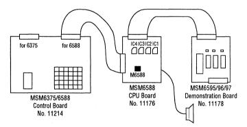
Note: When the serial register is not mounted, to IC1 on the MSM6588 CPU board (No. 11176) the circuit does not operate normally. In the meantime, when the serial register is mounted to IC2 ~ IC4, the normal operation is not obtained either.
