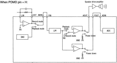
Note: This diagram shows the state of each switch during the recording operation.
