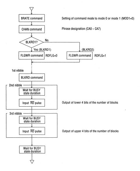
During execution of the BLKRD1, BLKRD2 command, verification of the status register cannot be performed by input of the RD pulse. When inputting the RD pulse for the 2nd nibble or 3rd nibble or inputting the next command after the BLKRD command, input the RD pulse either after the waiting time longer than the BUSY state duration or after verifying that the BUSY status is not present via the BUSY pin.
