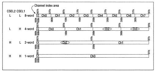
Note: By the combination of CSEL1, CSEL2, CA1, CA2 and CA3, the circled channel memory capacities can be allocated as Ch0=16sec., Ch2=8 sec. and Ch3=8 sec. (@f<sub>sam</sub>=8kHz).
