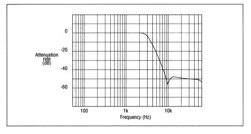
Figure 8 Low-pass Filter Characteristics (fsam=8kHz)
