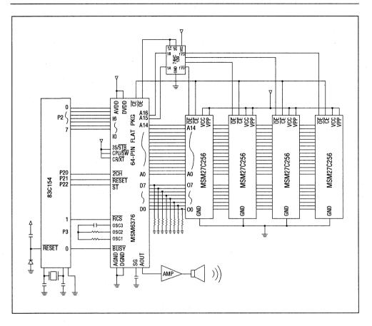
**Note:** Use a CMOS type 27C256 as an EPROM if possible. If an NMOS type 27256 is used, there are some cases where the power voltage variation of the EPROM becomes a source to generate noise.
