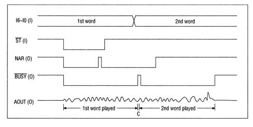
Figure 2 Timing of CPU Interface (800  $\mu$ s <  $\overline{ST}$ )
