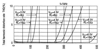
Total harmonic distortion rate vs output power (example)
