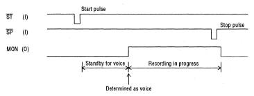
When a low level is applied to the SP pin during standby state for voice, the MSM6688 finishes the standby state for voice and goes to the standby state for recording.
