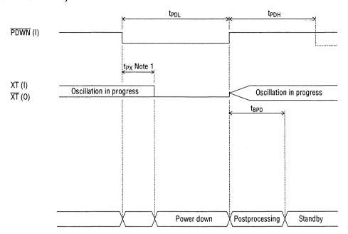
Note 1: When an external clock is used, continue to apply the clock input to the XT terminal during  $t_{PX}$  after the PDWN pin is set to a low level.
