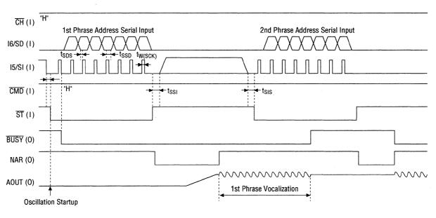
In serial input, data is transferred to the LSI when the ST signal rises after serial data is input. SD is captured at the former edge of SI.
