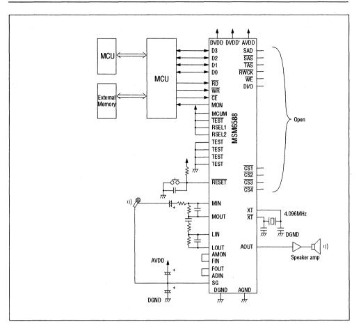
Figure 3 Application Circuit When Playback is Made Using EXT Command
