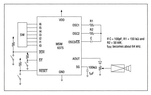
Figure 15 Application Circuit Example in the Case of Selecting RC, LPF and SW in Option
