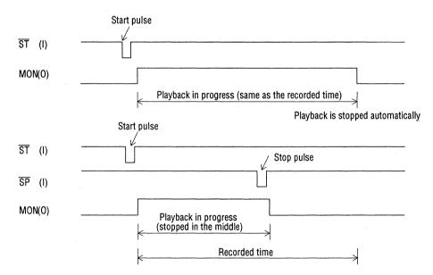
By maintaining the ST pin at a low level, repeated playback is possible.
