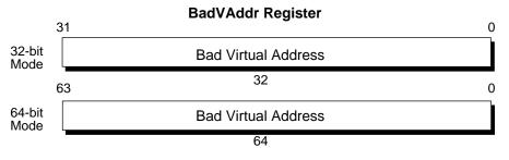
BadVAddr: virtual address at which an address error occurred last or which failed in address translation
