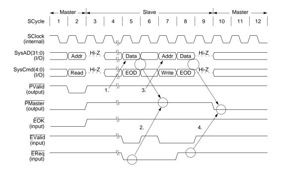
Figure 12-22 External Write Request Following Read Response
