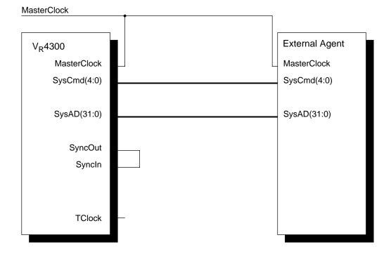
Figure 10-5 Phase-Locked System
