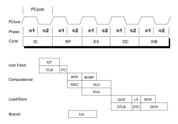
Figure 4-3 Pipeline Operations
