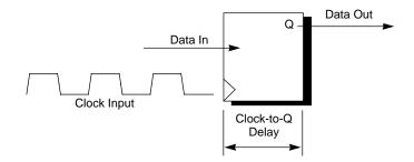
Figure 10-2 Clock-to-Q Delay
