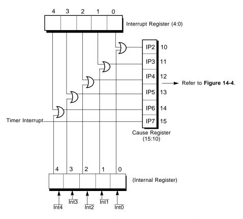
Figure 14-3 Hardware Interrupt Request Signals
