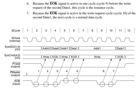
Figure 12-29 Discarding and Re-executing Processor Single Write Request
