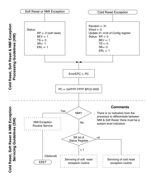
Figure 6-16 Cold Reset, Soft Reset & NMI Exception Handler
