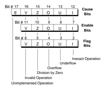
Figure 7-3 Control/Status Register (FCR31) Cause, Enable, and Flag Bit Fields
