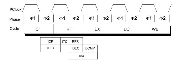
Figure 4-7 Branch on Equal Instruction Pipeline Operations
