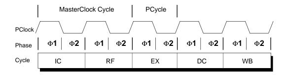
Figure 4-1 Pipeline Stages
