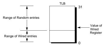
Figure 5-13 Wired Register Boundary
