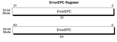
ErrorEPC : Indicates the program counter on cold reset or soft reset, or in case of the NMI exception.
