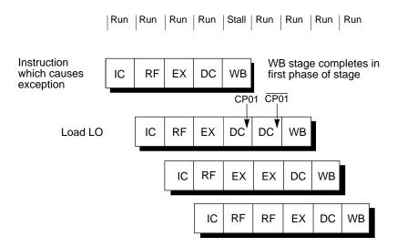
Figure 4-18 Example of a Coprocessor 0 Bypass Interlock (CP0I)
