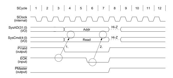
Figure 12-15 Delayed Processor Read Request
