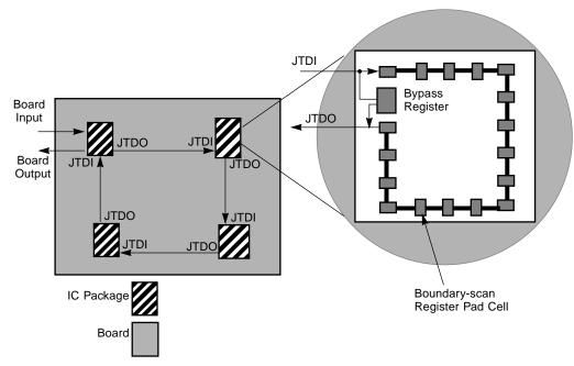
Figure 13-4 Bypass Register Operation
