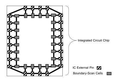
Figure 13-1 JTAG Boundary-Scan Cells
