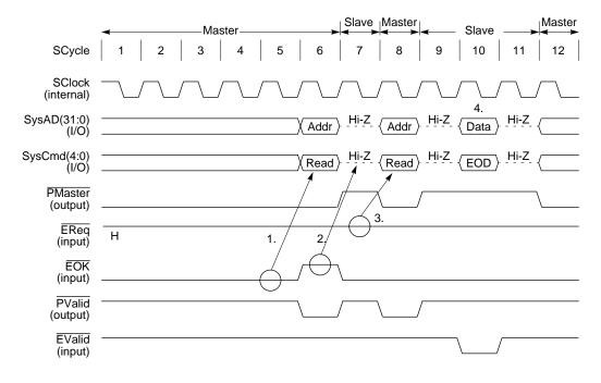
Figure 12-30 Discarding and Re-executing Processor Single Read Request
