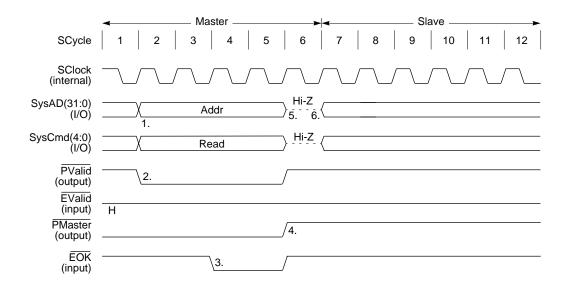
Figure 12-12 Delayed Processor Read Request
