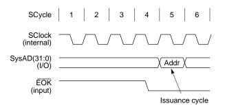
Figure 12-4 EOK Signal Status of Processor Request
