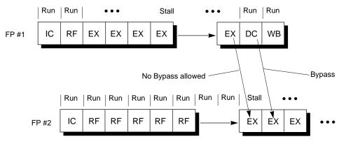
Figure 7-9 DC-to-EX Hardware Interlock Bypass
