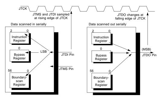
Figure 13-6 JTAG Test Access Port
