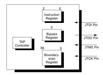
Figure 13-2 JTAG Interface Signals and Registers
