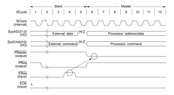
Figure 12-18 Bus Arbitration of Processor
