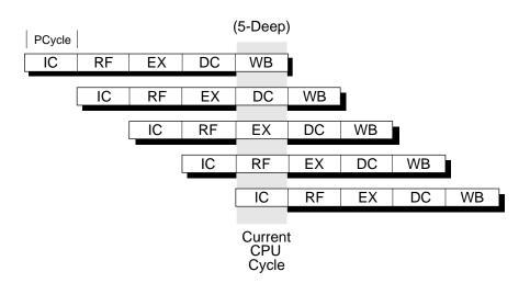
Figure 4-2 outlines the pipeline. The horizontal rows in this figure indicate the execution processes of instructions, and the vertical columns indicate the five processes executed at the same time.
