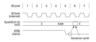
Figure 12-5 Address Cycle Extended by EOK Signal
