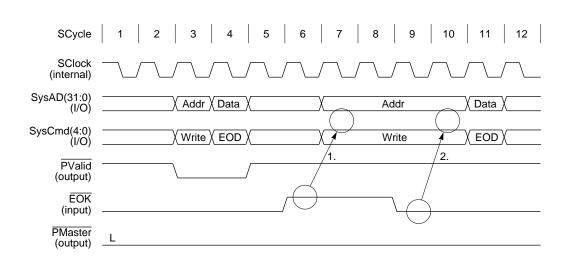
Figure 12-16 Delayed Second Processor Write Request
