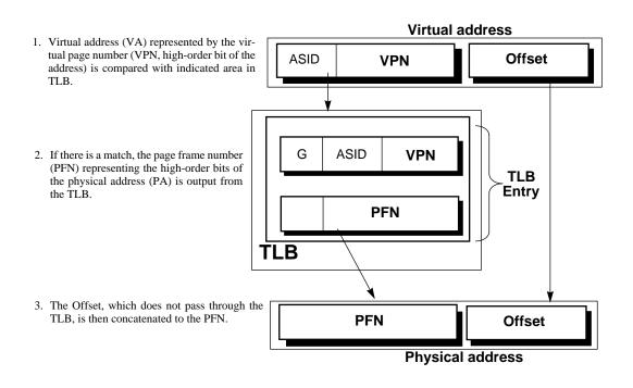
Figure 5-1 Overview of a Virtual-to-Physical Address Translation
