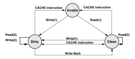
Figure 11-6 Data Cache State Diagram
