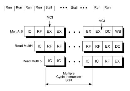
Figure 4-15 Example of a Multicycle Instruction Interlock
