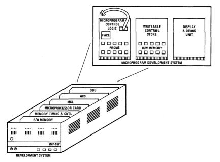
Figure 1. Microprogram Development System, as it would be used with a Development System during Microprogram Development.
