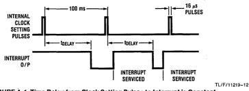
FIGURE A-1. Time Delay from Clock Setting Pulses to Interrupt is Constant
