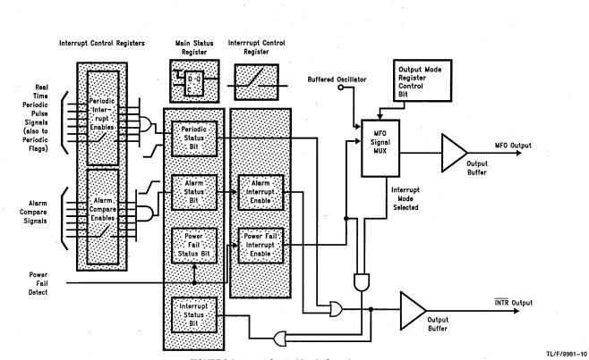
FIGURE 5. Interrupt Control Logic Overview
