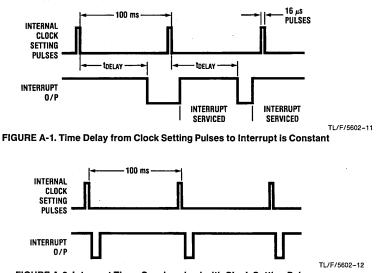
FIGURE A-2. Interrupt Timer Synchronized with Clock Setting Pulses
