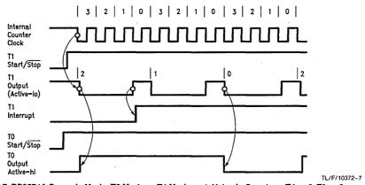
FIGURE 7. DP8571A Cascade Mode, T0 Mode = T1 Mode = 1, Value in Counters: T1 = 3, T0 = 2
