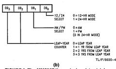
FIGURE 2. The MM58274's control register (a), in response to a nibble written to it, determines mode, starts and stops the clock, and selects interrupt frequency. The status register (b), a read-only register, indicates changes in clock data and signals an interrupt. Both registers reside at address 0<sub>HEX</sub>, which may be offset from location 0<sub>HEX</sub> in a host computer's I/O space.
