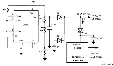
FIGURE 1. Voltage Regulator as a V<sub>CC</sub> Supply for an External Oscillator
