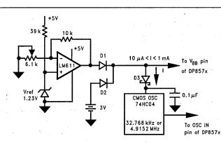
FIGURE 2. LM611 as a V<sub>CC</sub> Supply for an External Oscillator
