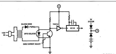
FIGURE 19. Sensing AC Line Failure Using Retriggerable One Shot
