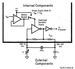
FIGURE 4. Oscillator Circuit Diagram
