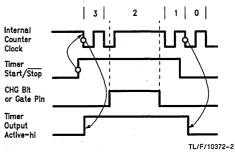
FIGURE 2. Mode 0—Single Pulse Generator
