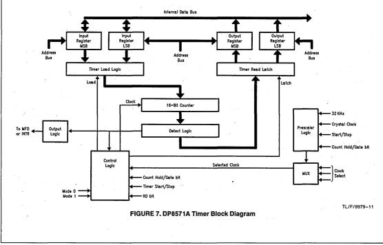
input data registers are loaded into the timer. The output will stay high until the counter reaches zero. At zero the output is reset. The result is an output pulse whose duration is equal to the input clock period times the count value (N) loaded into the input data register. This is shown in *Figure 8*.
