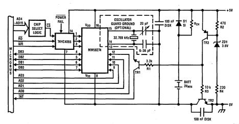
FIGURE 1. MM58274C System Installation
