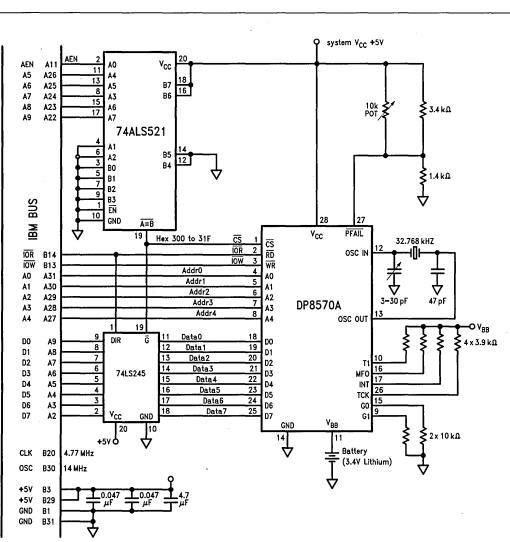
FIGURE 1. DP8570A Timer Clock Peripheral Interface to IBM/XT
