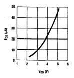
FIGURE 3. Typical I<sub>DD</sub> ( $\mu$ A) vs V<sub>DD</sub> (V) for MM58274C in Standby Mode (T<sub>A</sub> = 25°C)
