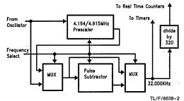
FIGURE 3. Programmable Clock Prescaler Block
