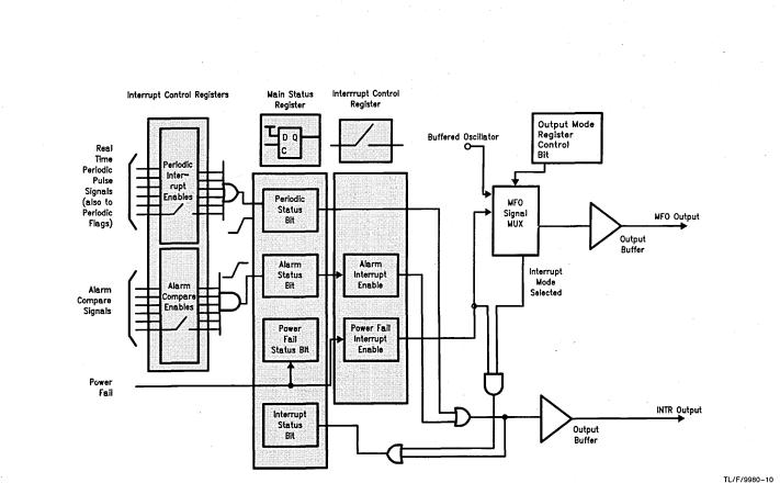
FIGURE 5. Interrupt Control Logic Overview
