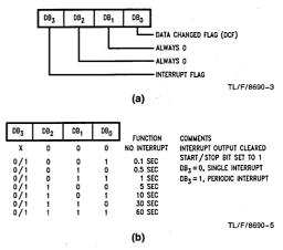
FIGURE 3. The state of bit DB<sub>2</sub> in the control register at address  $0_{HEX}$  selects one of two command registers at address FH<sub>EX</sub>. If the control register's DB<sub>2</sub> equals 0, then F<sub>HEX</sub> becomes the clock-setting register (a). If DB<sub>2</sub> is 1, then F<sub>HEX</sub> becomes the interrupt register (b).
