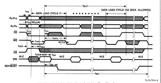
FIGURE 4. NMC98C64 Write Cycle Switching Time Waveforms
