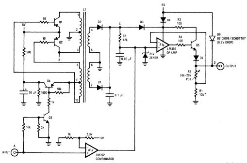
FIGURE 8. V<sub>PP</sub> Pulse Generator Circuit
