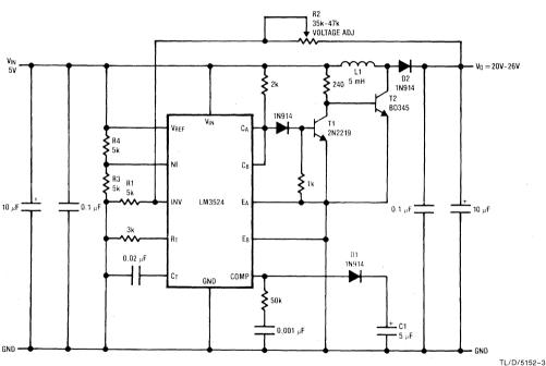
FIGURE 3. A 5V-21V Vpp Voltage Generator Circuit for E<sup>2</sup>PROM Application
