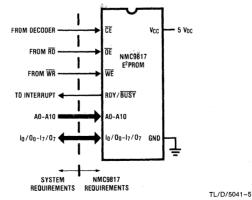
FIGURE 3. Simple NMC9817 Interface Requirements
