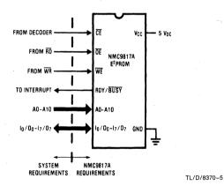
FIGURE 3. Simple NMC9817A Interface Requirements
