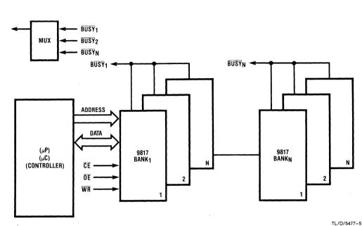
FIGURE 5. A Typical NMC9817 System
