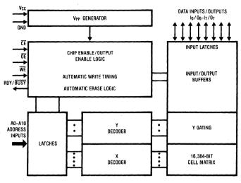
FIGURE 2. Functional Block Diagram
