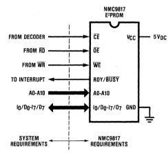
FIGURE 4. Simple NMC9817 Interface Requirements
