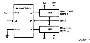
FIGURE 7. Converting Parallel Data into Serial Input for NMC9306/COP494
