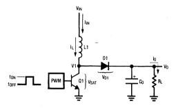
FIGURE 1. Basic Step-Up Switching Regulator
