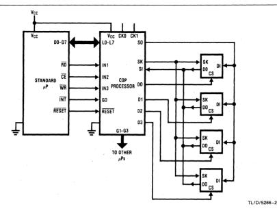
FIGURE 2. NMC9306 — Standard  $\mu P$  Interface Via COP Processor
