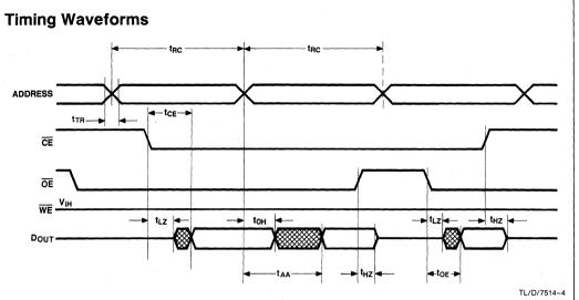
FIGURE 3. NMC98C64 Read Cycle Switching Time Waveforms
