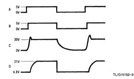
FIGURE 9. Idealized Signals at Various Nodes
