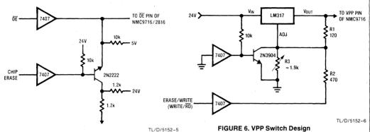
FIGURE 5. OE Chip Erase Control for NMC2816/NMC9716
