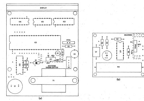
Figure 11. Printed Circuit Board Component Layouts. a) Layout for the Stopwatch/Timer PC board. b) Layout for the Appliance Control PC board.
