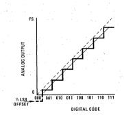
Hysteresis Error in an ADC causes the voltage at which a code transition occurs to be dependent upon the direction from which the transition is approached. This is usually caused by hysteresis in the comparator inside an ADC. Excessive hysteresis may be reduced by design; however, some slight hysteresis is inevitable and may be objectionable in converters if hysteresis approaches ½ LSB.
