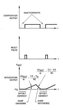
Note. Here the LF13300 always operates as an autozeroed, high input impedance inverting integrator; bipolar input voltages are handled by offsetting the analog ground by 2.2V. MM5330
