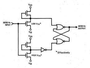
FIGURE 3. 50/60 Hz Input Shaping Circuit
