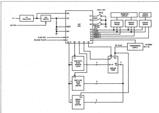
Figure 1. Electronic Speedometer/Odometer
