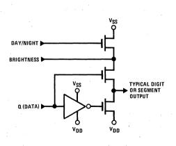
FIGURE 4. Output Circuit
