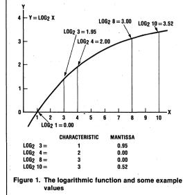
In figure 1 some points on the logarithmic curve are identified and evaluated to the base<sub>2</sub>. Notice that the characteristic in each case represents the highest even power of 2 contained in the value of X. This is readily seen when binary notation is used.
