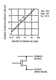
Figure 3. Typical Single Segment Output Buffer
