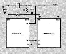
d. Externally Synchronized Oscillator
