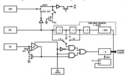
Figure 11. Dual Clock Option Block Diagram
