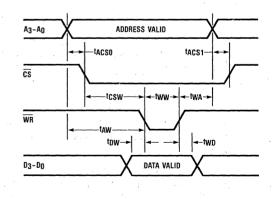
Figure 6. Write Cycle Waveforms
