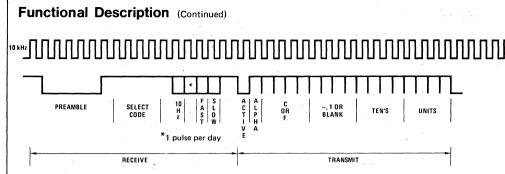
Select code for MM5407 is "1111" 10 Hz is used for generating internal time clock
