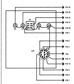
Figure 18. Wiring Diagram for the Switches Mounted in the Case Top.
