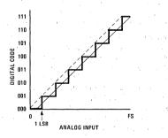
FIGURE 3. ADC Transfer Curve, No Offset
