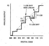
FIGURE 9. Non-Monotonic (Must be  $> \pm \frac{1}{2}$  LSB Non-Linear)
