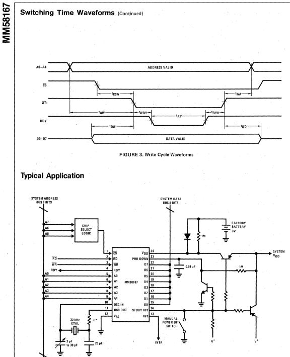
\*R is required for microwatt crystals R=200K
