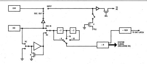
Figure 10a. Oscillator Options Block Diagram Using SKT Instruction
