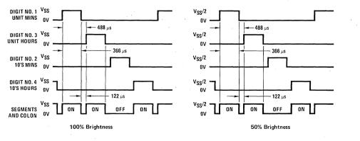
FIGURE 3. MM53110 Output Timing Diagram
