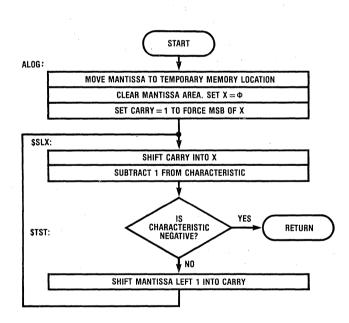
Figure 8. Flow Chart for Conversion to Antilog
