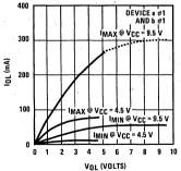
Figure 8. I/O DC Current Characteristics
