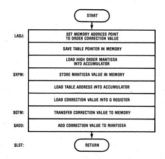
Figure 12. Flow Chart for Correction of a Value Found by Straight Line Approximation
