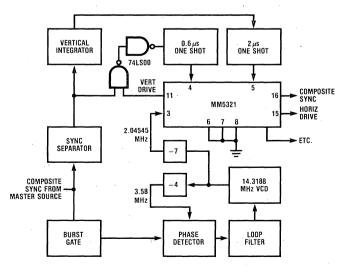
Figure 5. Genlocking with Color-Burst Phaselock
