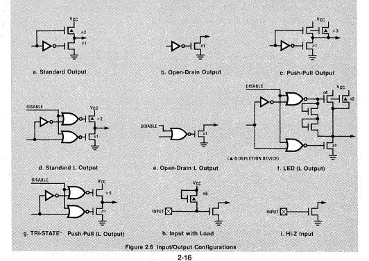
g. TRI-STATE<sup>®</sup> Push-Pull — an enhancement-mode device to ground and V<sub>CC</sub>. These outputs are TRI-STATE outputs, allowing for connection of these outputs to a data bus shared by other bus drivers.
