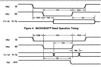
Figure 5. MICROBUS<sup>™</sup> Write Operation Timing
