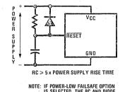
NOTE: IF POWER-LOW FAILSAFE OPTION IS SELECTED, THE RC AND DIODE CIRCUIT IS NOT USED
