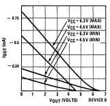
Figure 9b. COP420/COP421 Input/Output Characteristics
