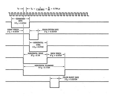
Figure 4. Horizontal Timing Diagram with the Input Clock Equal to 1.260 MHz
