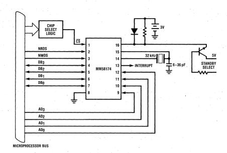
Figure 4. Typical Microprocessor Interface
