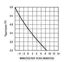
FIGURE 8. Drift vs VBATTERY
