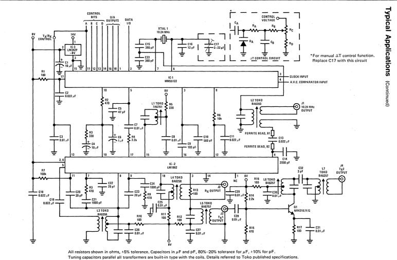
FIGURE 5. LM1862, MM55122 Single Crystal 40-Channel PLL Schematic Diagram
