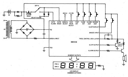
Figure 5. Typical Application (MM7318BN): Clock/Calendar with Battery Back-up
