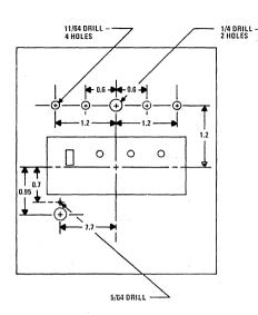
Figure 16. Drilling Guide for the Case Top if the MRC-1-10 Rotary Function Switch is Used. (Dimensions in inches.)
