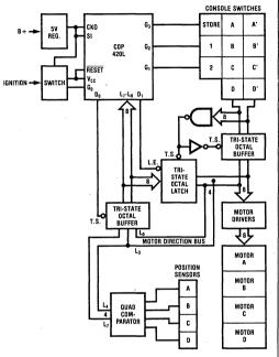
Figure 1. Block Diagram
