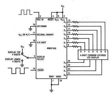
Figure 8. MM57436 as 8-Digit Decimal Down Counter with Extenal Oscillator
