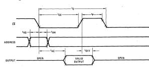
FIGURE 1. AC Electrical Waveforms
