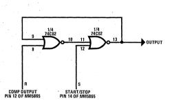
Figure 9. Detail of the 74C02 NOR Latch. The latch interfaces the MM5865 to the CA3059.
