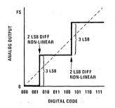
FIGURE 8. ±1 LSB Linear, ±2 LSB Differential Non-Linear
