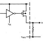
FIGURE 4a. BCD Outputs, MM53100
