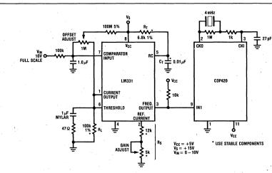
Figure 20. Basic LM331 Connection
