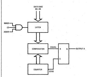
Pulse width modulated output for analog functions 6-bit resolution/63 discrete steps
