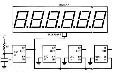
\* The minimum recommended value for R for the oscillator input is 9 k $\Omega$ . An RC time constant of approximately 4.91  $\times$  10<sup>-4</sup> should produce a backplane frequency between 30 Hz and 150 Hz.
