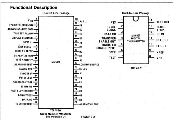
A block diagram of the MM5406 is shown in *Figure 1*. The various display modes and their priorities are listed in Table I. The functions of the setting controls in combination with the selected display mode are listed in Table II. *Figure 2* is a connection diagram and one add-on circuit. The following discussions are based on *Figure 1*.
