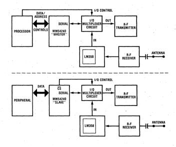
Figure 5. Radio Frequency Transmission Application
