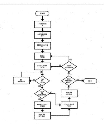
Figure 3. Functions 1 and 2. Pressing START/STOP after FINAL EVENT has been pressed gives Total Elapsed Time in Function 1, Total Accumulated Time in Function 2.
