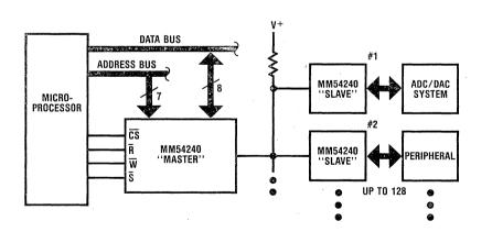
Figure 1. Typical System Block Diagram
