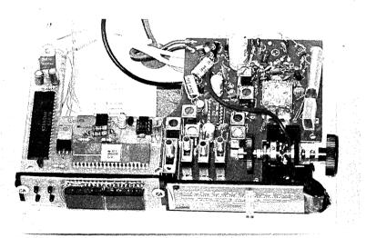
The MM5430, MM5402 Circuit Applied to an Existing Clock Radio Chassis; Note that the Original Dial Pointer is Still Used. MB-19
