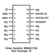
The flip flop sets all data bus bits to a "1" during NRDS time indicating that a register has been updated.
