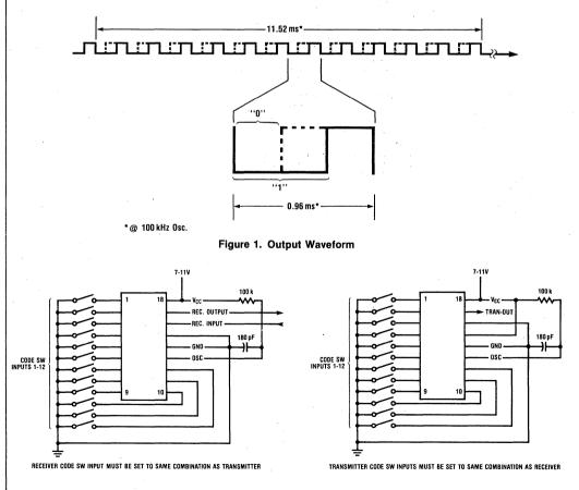
Figure 3. Pin Connections for Transmitter Mode
