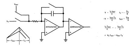
FIGURE 8. Basic Dual Slope
