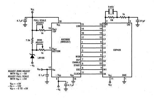
Figure 29. Simple A/D with ADC0800
