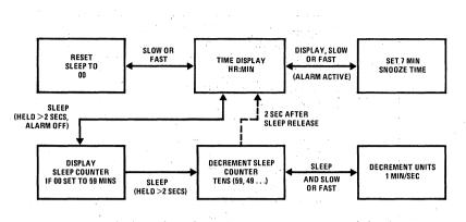
FIGURE 9. Snooze and Sleep Control State Diagram
