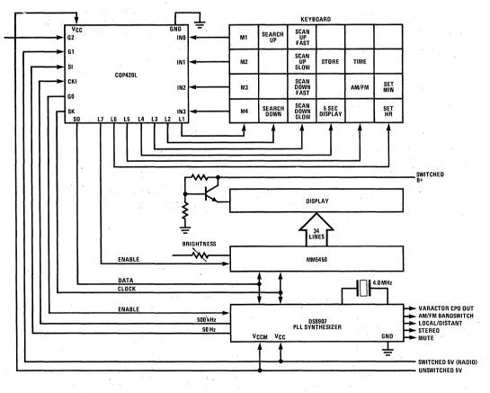
Figure 8. Electronically Tuned Radio System
