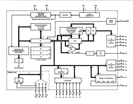
Figure 1. COP444L/445L Block Diagram
