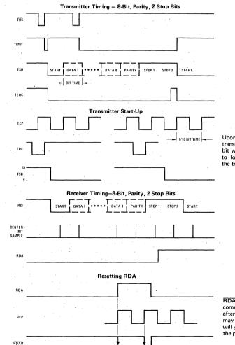
Upon data transmission initiation, or when not transmitting at 100% line utilization, the start bit will be placed on the TSO line at the high to low transition of the TCP clock following the trailing edge of  $\overline{\text{TDS}}$ .
