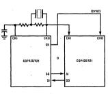
Externally Synchronized Oscillator
