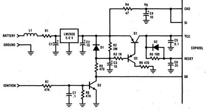
Figure 6. Power Supply Circuitry
