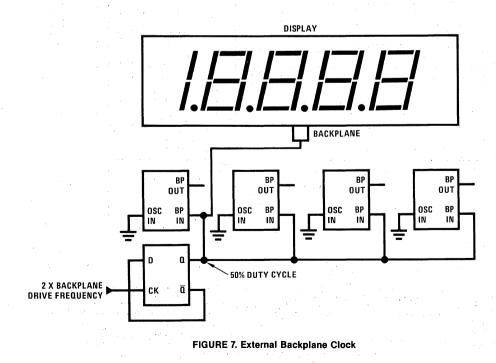
Using an external clock allows synchronizing the display drive with AC power, internal clocks, or DVM integration time to reduce interference from the display.
