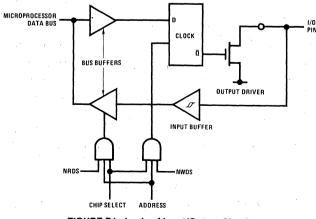
FIGURE B1. Logic of Input/Output Circuitry
