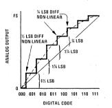
FIGURE 7. 1% LSB Non-Linear, ½ LSB Differential Non-Linearity
