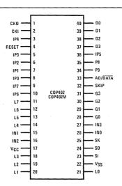
Figure 2. Connection Diagram
