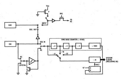
Figure 10b. Oscillator Options Block Diagram Using IT Instruction
