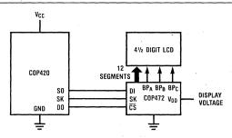
Figure 6. System Diagram - 41/2 Digit Display
