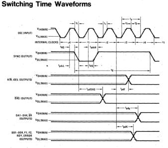
Note 1: See discussion of timing diagrams on page 5. Note 2: Osc. Duty Cycle =  $t_1$  ( $t_1 + t_2$ ) =  $t_1/t_p$ . Note 3: The last four timing diagrams indicate that, if the output changes, it will change within the indicated time. This is not meant to imply that these signals will change every microcycle. The conditions which will cause the various outputs to change are explained in detail in the functional description section of this manual.
