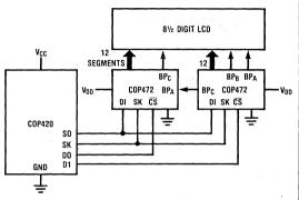
Figure 7. System Diagram - 81/2 Digit Display
