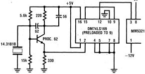
Figure 2. Input Clock Generating Schemes
