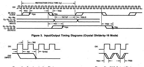
Figure 3a. Synchronization Timing
