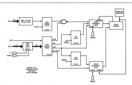
Figure 1. COP410L/411L Hardware Stack Emulator Block Diagram
