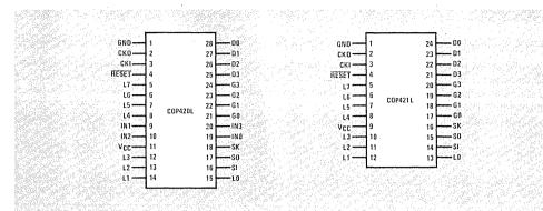
Figure 2.2 COP420/COP421 Connection Diagrams
