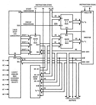
FIGURE 14(a). MM57109 Analog Data Acquisition System Block Diagram
