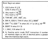
The error flag can be tested by the TERR instruction (which branches if ERROR = 1) or it can be used to clear the external program counter, resulting in a hardware jump to location 0, the error recovery location. In either case, an ECLR instruction must be executed to clear the error flag.
