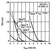
Source Current for L0 through L7 in TRI-STATE\* Configuration (High Current Option)
