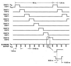
FIGURE 3. Blanking Output
