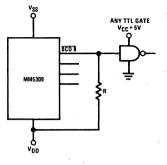
For  $V_{SS} = 5$ ,  $V_{DD} = 12$ , R = 10k For  $V_{SS} = 10$  to 17V,  $V_{DD} = Gnd$ , R = 3k
