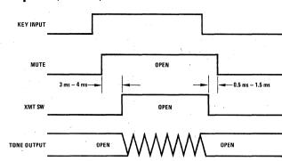
FIGURE 3. Timing Diagram of MUTE and XMT SW in Relation to Key Input and Tone Output
