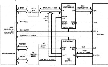
FIGURE 15. MM57109 Microcomputer Interface Using 2 FIFO's
