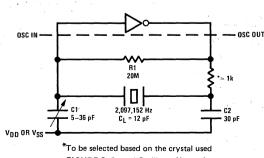
FIGURE 3. Crystal Oscillator Network
