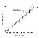
FIGURE 4. Linear, 1 LSB Scale Error
