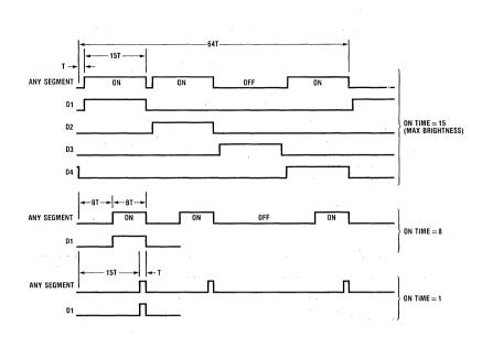
Figure 5. Segment and Digit Output Timing Diagram
