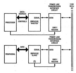
Figure 4. Power Line Transmission Application
