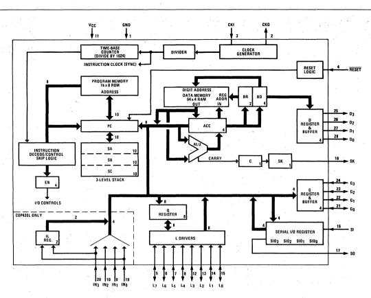
Figure 2. COP420L Block Diagram
