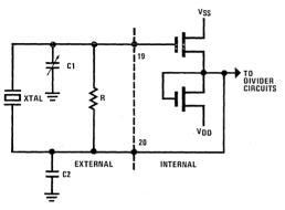
Figure 3. Crystal oscillator connections.
