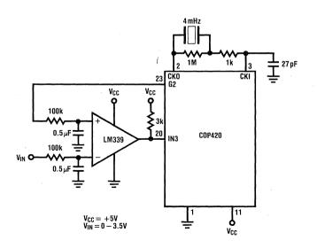
Figure 7. Basic Duty Cycle A/D
