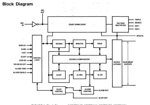
FIGURE 1. Block Diagram of MM58143, MM58144, MM58183, MM58184
