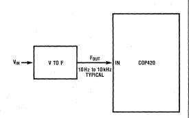
Figure 18. V to F Converter - Basic Concept
