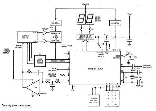
FIGURE 3. Tuning System With Full Keyboard And Remote Control
