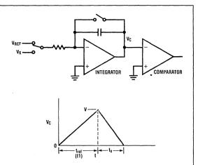
Figure 12. Dual Slope Integration - Basic Concept
