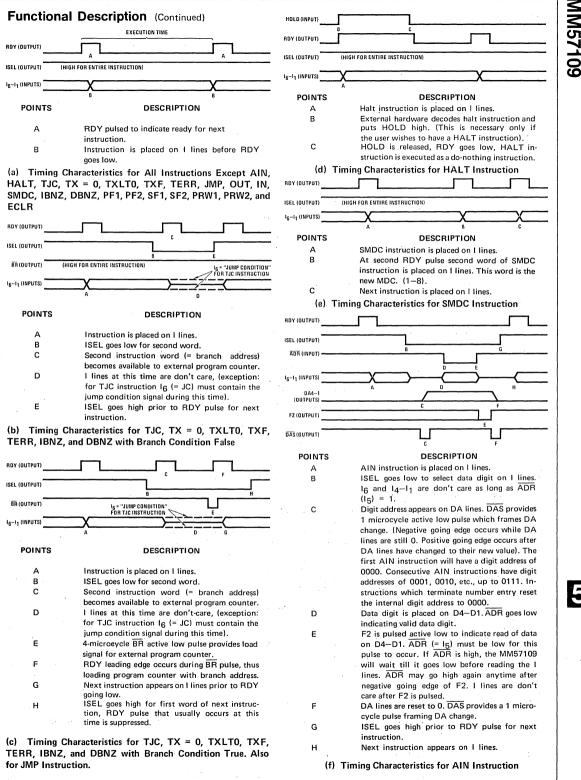
FIGURE 10. Instruction Timing Diagrams
