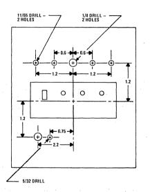
Figure 17. Drilling Guide for the Case Top if the PS-101 Rotary Function Switch is Used. (Dimensions in inches.)
