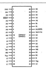
Figure 2. Connection Diagram
