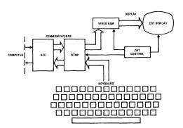
FIGURE 4. Block Diagram of an Interactive Terminal
