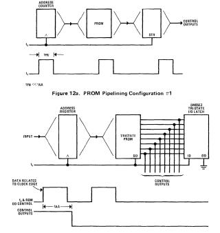
Figure 12b. PROM Pipelining Configuration #2
