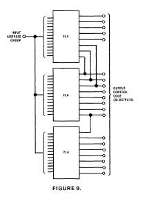
Doing this allows half of the partial product terms to be placed in each of two separate PLA's. PLA's can be connected with common inputs and common outputs. It should be noted that the output code for the common terms must be programmed using a negative true logic for, since this permits "wire-OR'ing" the outputs. This very significant design possibility would not be allowed if standard ROM techniques are used.
