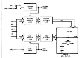
FIGURE 3. Block Diagram of Cell Selection
