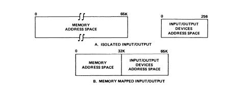
Figure 2. Mapping for Isolated Input/Output and Memory Mapped Input/Output Techniques
