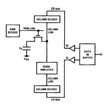
FIGURE 6. Simplified Write Circuitry
