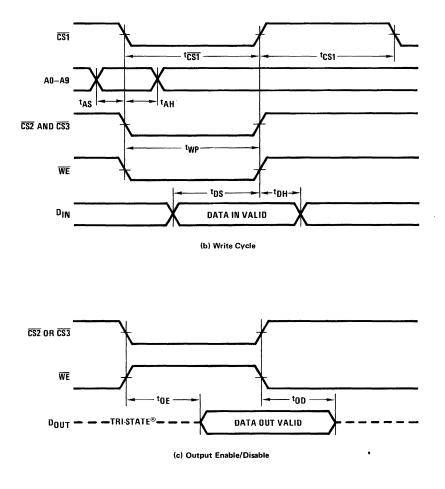
FIGURE 5. MM54C929/MM74C929, MM54C930/MM74C930 Switching Time Waveforms
