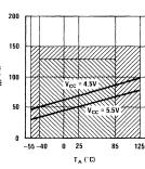
(c) Minimum Write Pulse Width vs Ambient Temperature
