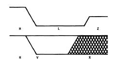
In cases where the exact time of the transition may vary or be unimportant, the transition should be drawn as a series of parallel transition lines. This series of transition lines should span the region in which the transition may occur.
