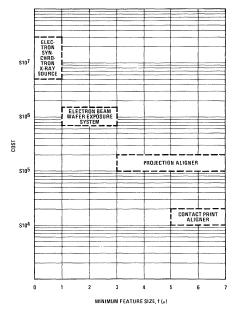
FIGURE 4. Cost of Key Equipment for Various Pattern Definition Technologies and Minimum Feature Sizes
