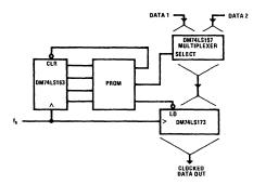
Figure 6. Sequencer Controlling Clocked & Unclocked Devices
