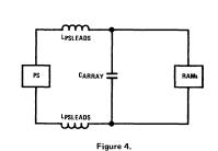
Let the total power supply lead inductance be 50 nH. (We are ignoring the PC trace inductance within the RAM array itself.) What would the voltage step have to be at the RAMs to get  $40 \text{ mA} \times 8$  flowing in 20 ns? The equation is:
