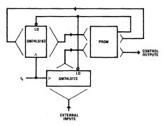
Figure 7. Determination of Next State Using External Inputs
