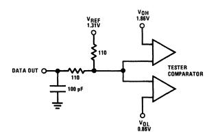
$I_{\text{SOURCE}} = \frac{2.4 - 1.31}{220} = 4.95 \text{ mA}$  $I_{\text{SINK}} = \frac{1.31 - 0.40}{220} = 4.14 \text{ mA}$
