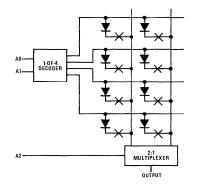
Figure 2. Read Only Device Portrayed as a Diode Array
