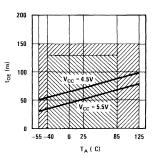
(i) Output Enable Time vs Ambient Temperature
