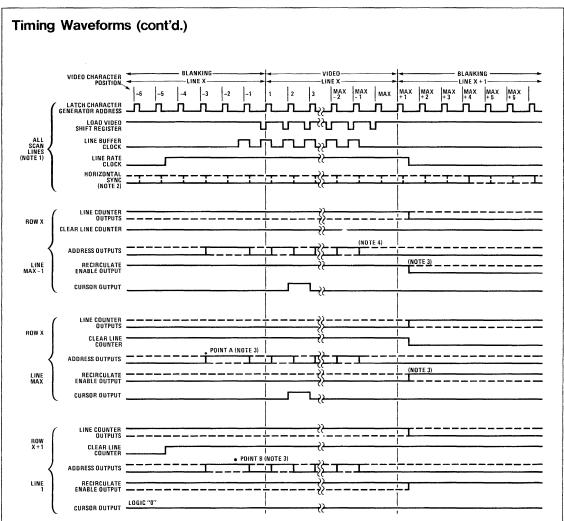
Note 1: The load video shift register output is not active during vertical or horizontal blanking (remains in the logic "1" state during these intervals.
