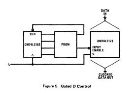
Notice that although the clock is ungated the DM74LS173 need capture data only during the state(s) determined by the contents of the PROM and retains the data until next enabled.
