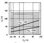
(f) Minimum ST Pulse Width (Positive) vs Ambient Temperature
