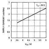
FIGURE 8. Dynamic Current vs Power Supply Voltage (VIH = VCC, VIL = 0V)
