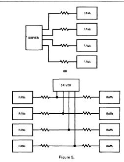
give the best clock waveform at the RAM chips. Its value will probably be between 10 and 51  $\Omega$ . Figure 5 shows the commonly used arrangements.
