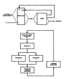
Figure 9. Control Sequence Determined by External Conditions
