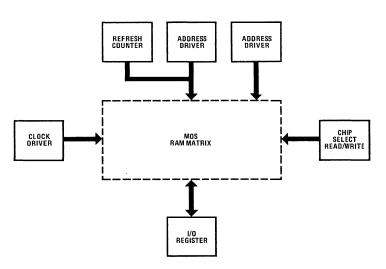
Figure 1. Memory System Block Diagram
