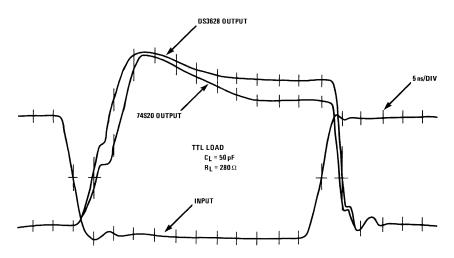
Figure 2. Switching Response with TTL Load
