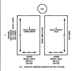
Figure 1. MM5290 Cell Array Diagram
