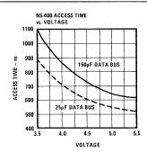
Figure 1. NS400 Access Time vs Voltage
