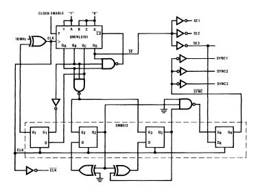
Figure 4. 1 MHz Clock Generator
