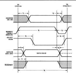
Figure 3. Write Cycle Timing
