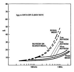
Figure 3. IDD vs Clock or Data Rate @ +70°C
