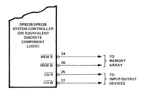
Figure 3. System Control Signals for Isolated Input/Output Addressing
