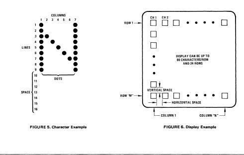
Next, the first line of the first character of the second row is addressed and scanned. This continues until the 9th line plus lines for vertical spacing of the last character in the last row has been scanned. At this time the display field has been written. For a CRT Display, it is necessary to refresh the display. Displays are typically refreshed 30 to 60 times each second. Memory is required to store the character address so that they may be called up when required for refresh.
