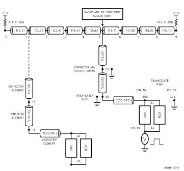
Model of the Futurebus+ backplane with two daughter boards; one in slot 1, and one in slot 5 with an input signal at pin 10.
