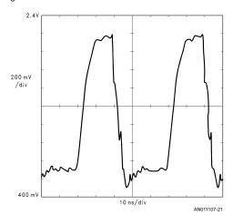
FIGURE 21. Backplane Probed at Driver = Slot 5, 10 pF to 12 pF Loads in Every Slot
