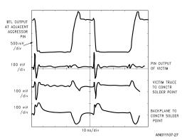
FIGURE 27. Victim Is Only Asserted, 8 Aggressor Channels Switching
