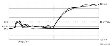
FIGURE 15. Three TDR Waveforms
