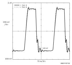
FIGURE 23. Backplane Probed at Driver = Slot 5
