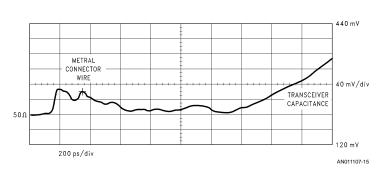
FIGURE 14. TDR Launch into Connector B-b-16 with DS3886 Mounted On Board
