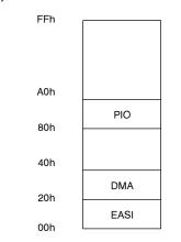
/EASIZ = /A7 \* /A6 \* /A5 \* IOMZ \* BACKZ /DMAZ = /A7 \* /A6 \* A5 \* IOMZ \* BACKZ /PIOZ = A7 \* /A6 \* /A5 \* IOMZ \* BACKZ The other three outputs are used as inverters:
