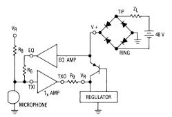
Figure 1. MC34014 Transmit Section
