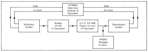
FIGURE 9 - Equipment Setup
