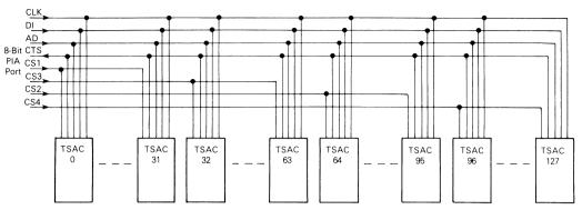
FIGURE 8 - TYPICAL 8-BIT PORT
