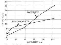
Figure 5. Tip-Ring Voltage versus Loop Current
