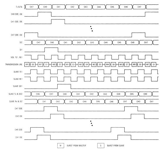
Figure 9. System Timing
