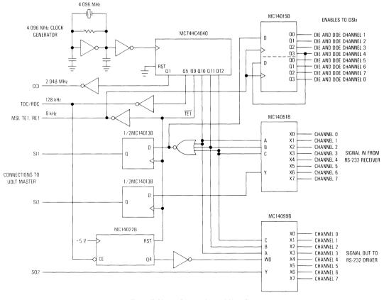
Figure 7. Master Sequencing and Signalling
