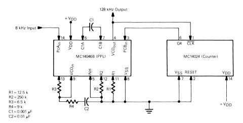
FIGURE 15 - 128 kHz FREQUENCY SYNTHESIZER USING 8 kHz INPUT
