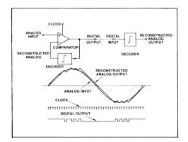
FIGURE 1 — SIMPLE DELTA MODULATION An Analog Input Signal Can Be Digitalized and Transmitted by Synthesizing a Minimum Error Set of Voltage Ramps. The Comparator Clock Establishes the Channel Bandwidth.
