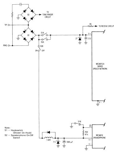
Figure 3. Handset/Speakerphone Power Switching
