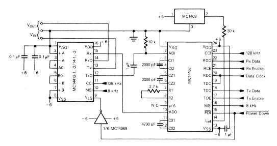
FIGURE 7 — TYPICAL CIRCUIT CONFIGURATION USING THE MC14407 CODEC AND MC14413-1, -2 FILTER (SPLIT SUPPLY)
