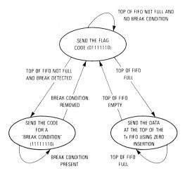
Figure 2A. Synchronous Data Channel Transmitter Operation
