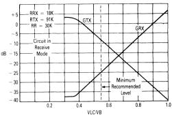
FIGURE 6 — ATTENUATOR GAIN versus ΔVacf
