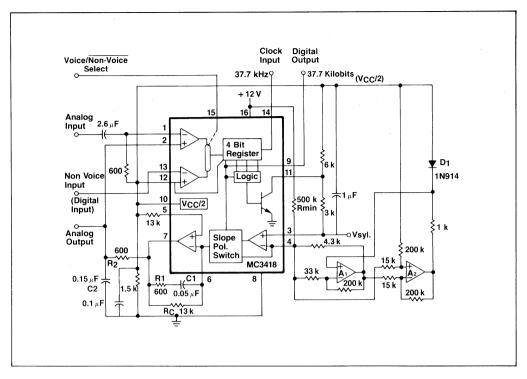
$\label{eq:FIGURE 5} FIGURE 5 - TELEPHONE QUALITY DELTA MODULATOR CODER\\ Both Double Integration and Active Companding Control Are Used to Obtain Improved CVSD Performance.\\ Laser Trimming of the Integrated Circuit Provides Reliable Idle Channel and Step Size Range Characteristics.\\ \end{tabular}$
