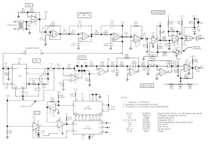
FIGURE 15 - 2400 BPS DPSK DEMODULATOR SYSTEM
