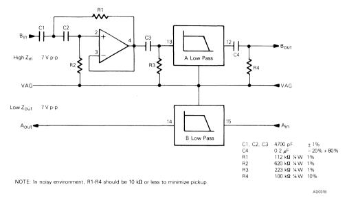
FIGURE 5 - FILTER SCHEMATIC FOR MC145414 WITH 60 Hz REJECT FILTER
