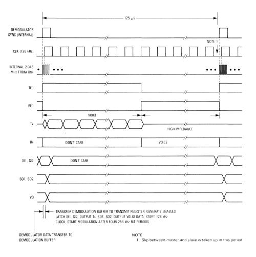
Figure 13. Slave DLT Timing
