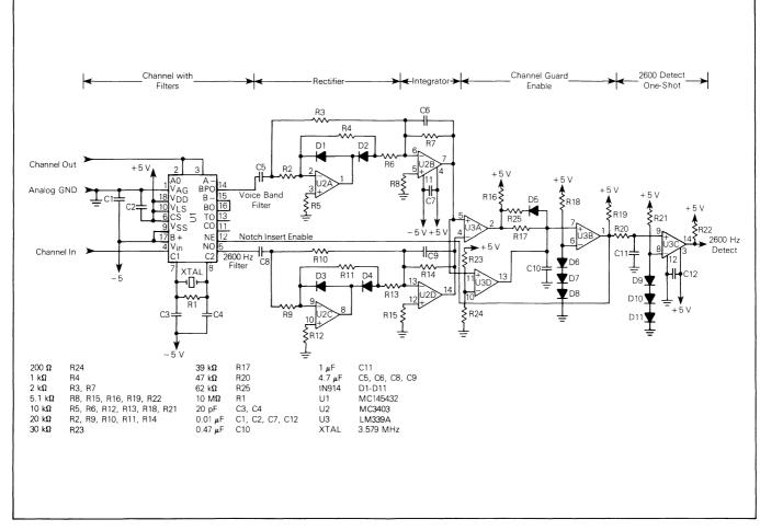
FIGURE 1 - 2600 Hz Guard and Channel Circuit
