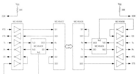
Figure 1. Limited Distance Modem Block Diagram
