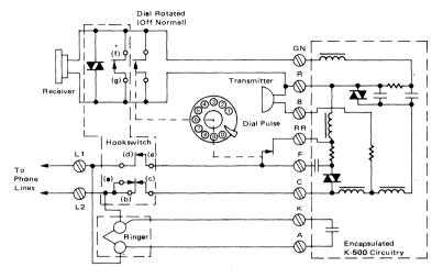
FIGURE 10 - STANDARD K-500 TELEPHONE
