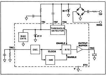
Fig. 5 Tone ringer block diagram.
