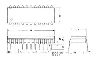
NOTES: 1. LEADS TRUE POSITIONED WITHIN 0.25 mm (0.010) DIA AT SEATING PLANE AT MAXIMUM MATERIAL CONDITION (DIM "D"). 2. DIM "L" TO CENTER OF LEADS WHEN FORMED PARALLEL.
