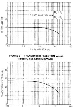
FIGURE 8 — RETURN LOSS versus TIP/RING RESISTOR MISMATCH
