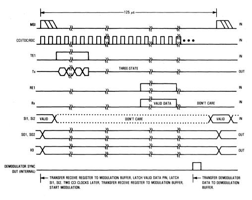
Figure 10. Master UDLT Timing
