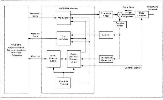
FIGURE 8 - Typical MC6860 Modem System
