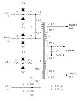
Figure 9. Battery Feed Transformer Configuration
