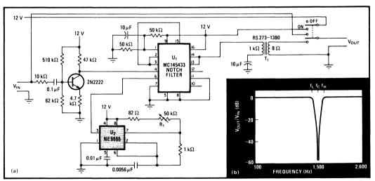
Filtering. Motorola's switched-capacitor notch filter MC145433 is switched by adjustable clock U<sub>2</sub> to provide a tunable audio notch filter (a). This notch filter has a frequency response of about 100 Hz to 2.6 kHz (b) and can operate with voltages from + 10 to + 15 V dc. Transistor Q<sub>1</sub> improves the circuit's signal-to-noise ratio, while audio transformer T<sub>1</sub> drives an 8-ohm load.
