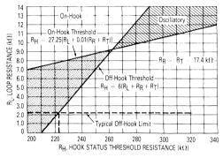
Figure 11 shows such a graph using 17.4 k $\Omega$  as the values for  $R_{P}$  and  $R_{T}$ . Note the oscillatory condition to the right of the crossing point. Selection of  $R_{H}$  in this region is usually not a problem since the majority of telephone lines do not fall into this resistance range.  $R_{H}$  always ties to  $V_{OB}$  and HST and will give reliable hook status information regardless of power supply voltages and  $\overline{PDI}$ .
