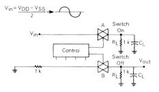
FIGURE 5 - CROSSTALK CONTROL TO OUTPUT
