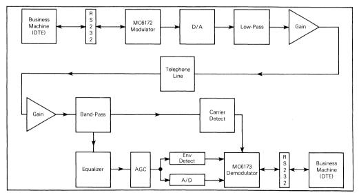
FIGURE 3-MC6172/6173 Modem Block Diagram
