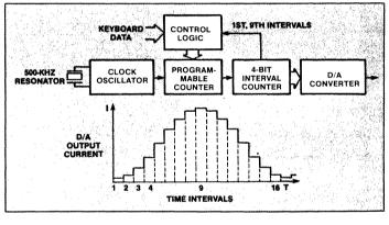
Fig. 2 The DTMF frequency synthesis technique.
