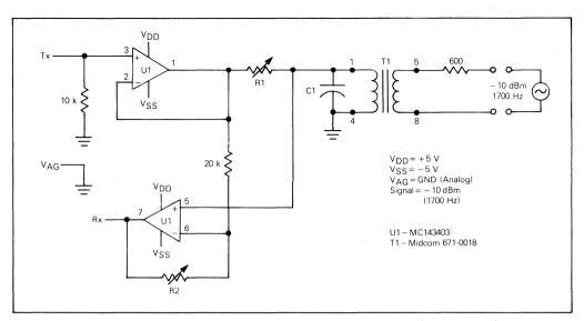
FIGURE 1 - Duplexer Circuit
