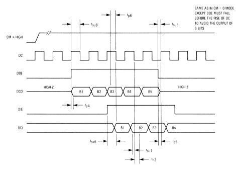
Figure 3D. Synchronous I/O, Variable Bit Length, Clock Mode High
