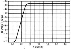
Figure 1. Equalization Amplifier Gain
