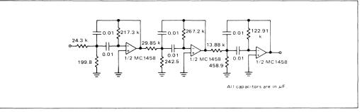
FIGURE 14a - Originate Filter Component Values
