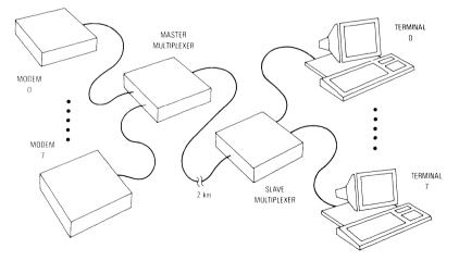
Figure 1. Typical Multiplexer Application
