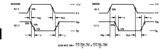
Figure 2. Switching Characteristics
