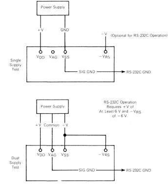
FIGURE 5 - Power Supply Set-Up
