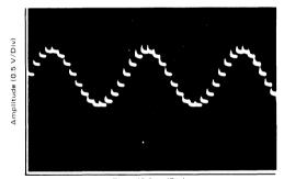
Time (0.2 ms/Div) FIGURE 9 — TRANSMIT CARRIER SINE WAVE
