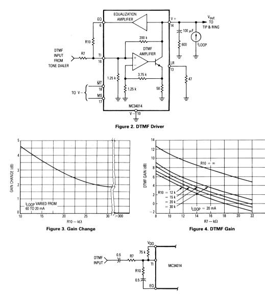
Figure 5. Alternate Biasing
