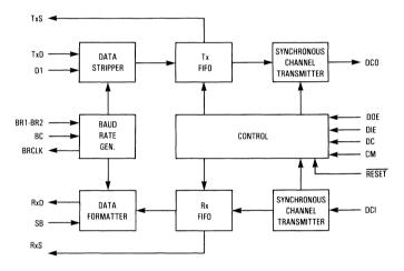
Figure 2. Block Diagram of the Data Set Interface
