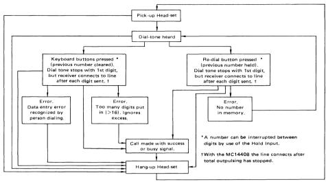
FIGURE 8 - KEYPAD TO PULSE DIALER FLOW DIAGRAM
