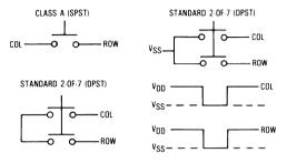
Figure 1. Keyboard Configurations
