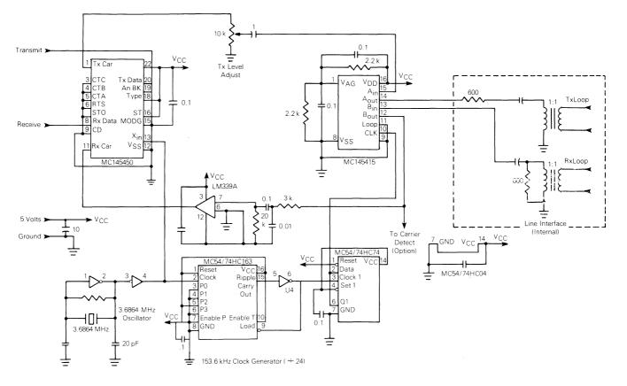
FIGURE 6 - TYPICAL 1200 BAUD 4 WIRE MODEM APPLICATION
