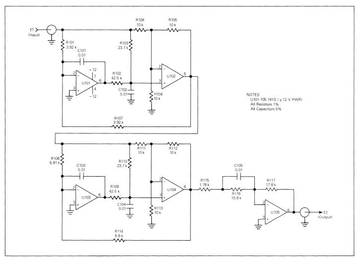
FIGURE 6 - 2400 BPS Modern System Equalizer Sub-Board
