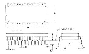
NOTES: 1. DIM "L" TO CENTER OF LEADS WHEN FORMED PARALLEL. 2. LEADS WITHIN 0.13 mm (0.005) RADIUS OF TRUE POSITION AT SEATING PLANE AT MAXIMUM MATERIAL CONDITION. (WHEN FORMED PARALLEL).
