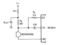
Figure 2. Alternate Biasing Scheme for Higher Voltage Microphones
