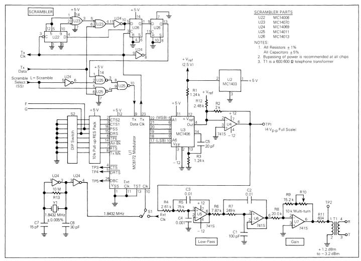
FIGURE 4 - 2400 BPS DPSK Modulator System
