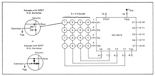
FIGURE 4 - TYPICAL KEYPAD INTERFACE APPLICATION
