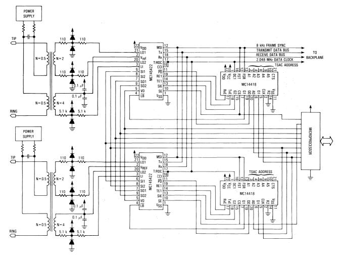
Figure 15. Typical Multichannel Digital Line Card
