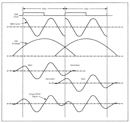
FIGURE 2-DPSK Waveforms
