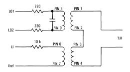
Figure 3. Transformer Configuration
