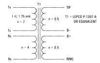
Figure 3. DLT Coupling Transformer
