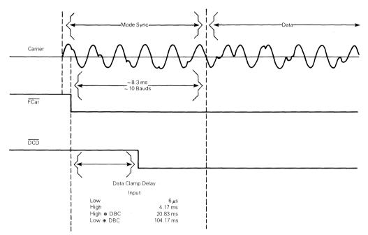
FIGURE 4 -- DEMODULATOR SYNC TIMING DIAGRAM
