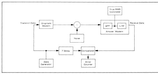
FIGURE 16 - Modem Test Equipment Configuration
