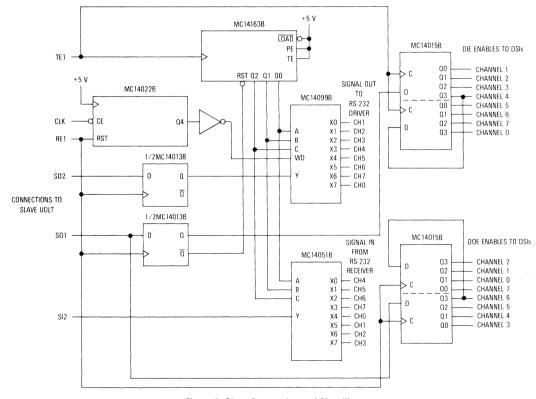
Figure 8. Slave Sequencing and Signalling
