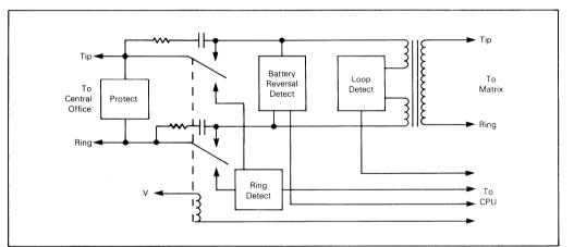
FIGURE 4A - Trunk Interface (Without Pulse Dialing)
