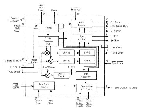
FIGURE 2 - DEMODULATOR BLOCK DIAGRAM
