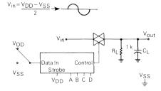
FIGURE 4 - CROSSTALK BETWEEN ANY TWO SWITCHES
