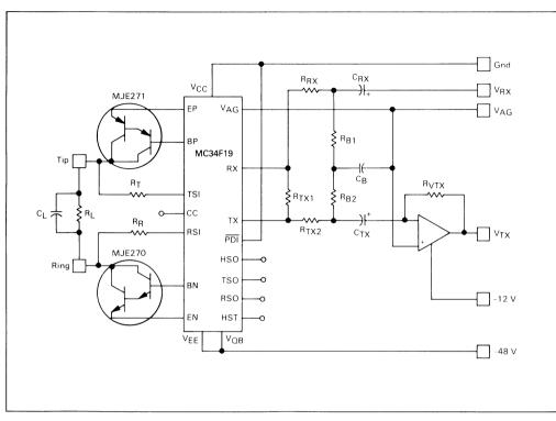
FIGURE 17 - BALANCE NETWORK FOR REACTIVE LINES
