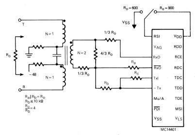
"T" Padded Transformer Hybrid Using MC14401
