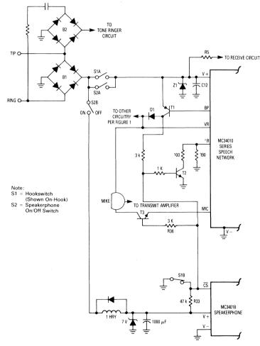
Figure 7. Microphone Muting — MC34010A Series
