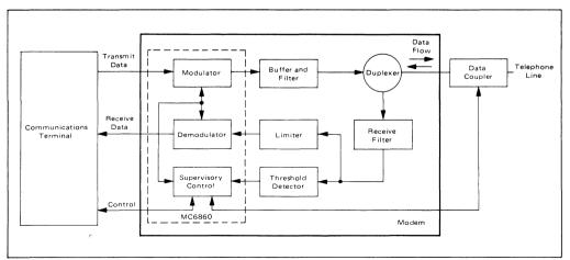
FIGURE 1 – Low-Speed Modem and Interconnections
