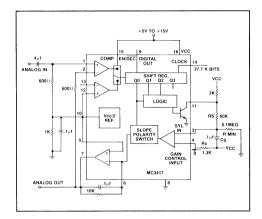
FIGURE 3 — BASIC CVSD ENCODER Single Pole Integration and a Single Pole Syllabic Filter Are Sufficient for Many Voice Channel Applications. Selection of External Components Tailors the Integrated Circuit to the Application.
