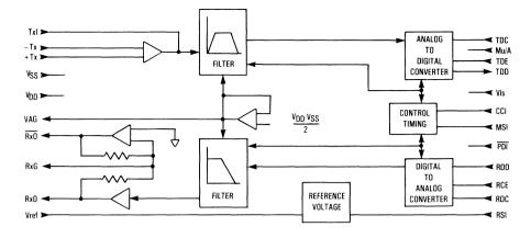
Figure 1. Block Diagram of the Mono-circuits
