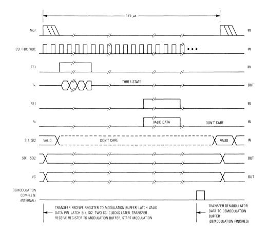
Figure 12. Master DLT Timing
