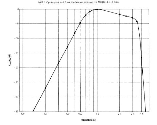
FIGURE 17 - TELEPHONY C-MESSAGE FILTER USING MC14414-1, -2 FILTER
