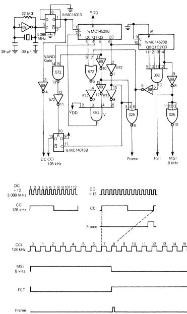
FIGURE 15 - CLOCK CIRCUIT AND TIMING FOR CODEC DATA CLOCKS AT 1.544  $\rm MHz$
