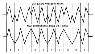
Figure 12. Modified Differential Phase Shift Keying
