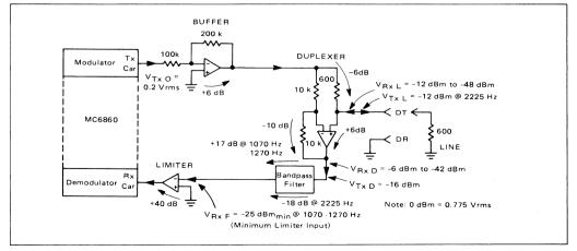
FIGURE 12 - System Level Constraints
