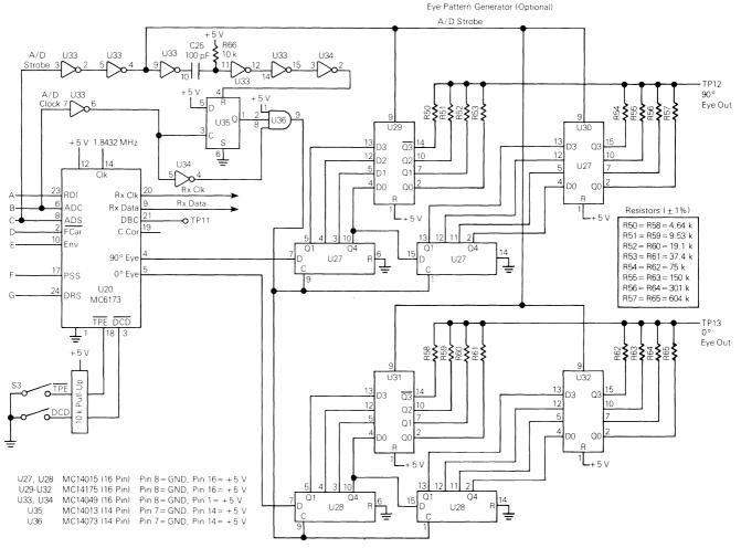
FIGURE 16 - 2400 BPS DPSK DEMODULATOR SYSTEM
