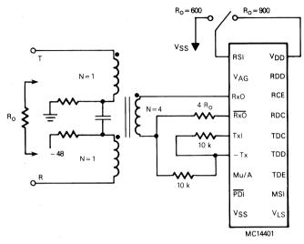
HYBRID INTERFACES TO MC14401 PCM CODEC FILTER MONO-CIRCUIT
