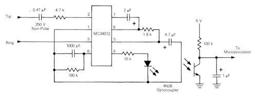
FIGURE 1 - Ring Detector Schematic
