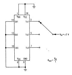
Figure 1. Power-Off Source Resistance (Drivers)
