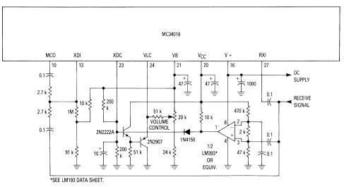
Figure 1. Receive-Idle Circuit
