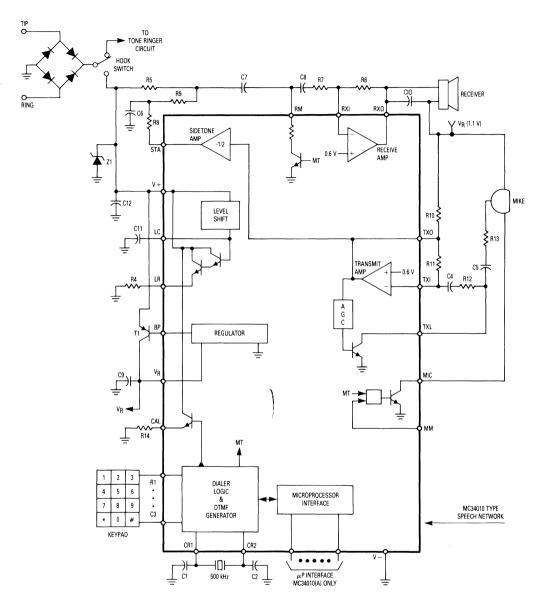
Figure 1. Basic MC34010 Type Telephone
