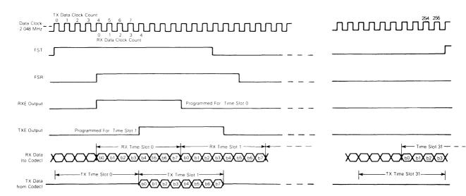
FIGURE 6 - DATA MULTIPLEX TIMING FOR 2.048 MHz
