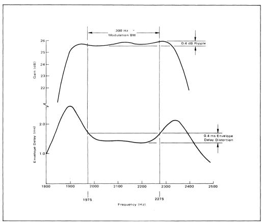
FIGURE 10 - Originate Bandpass Filter Characteristics
