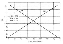
FIGURE 8 - LOG AMP TRANSFER CHARACTERISTICS
