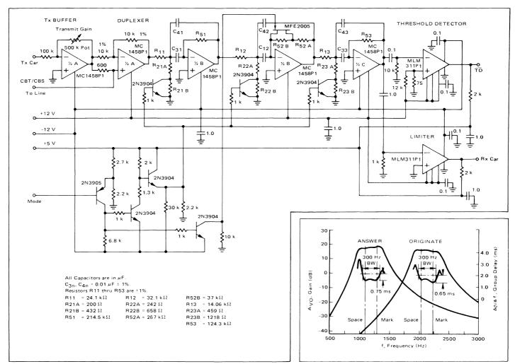
FIGURE 17a - Switchable Filter/Duplexer
