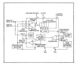
FIGURE 2 — CVSD BLOCK DIAGRAM A Delta Modulator Is Enclosed in a Digitally Controlled Gain Loop and Composes a Continuously Variable Slope Delta Modulator. A Bipolar/I<sup>2</sup>L Integrated Circuit Has Been Designed to Provide All the Active Circuitry Required.
