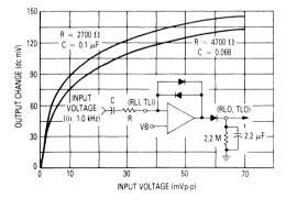
FIGURE 7 - LOG AMP TRANSFER CHARACTERISTICS
