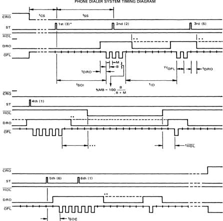
FIGURE 3 PHONE DIALER SYSTEM TIMING DIAGRAM
