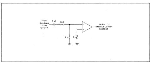
FIGURE 11 - Limiter Schematic
