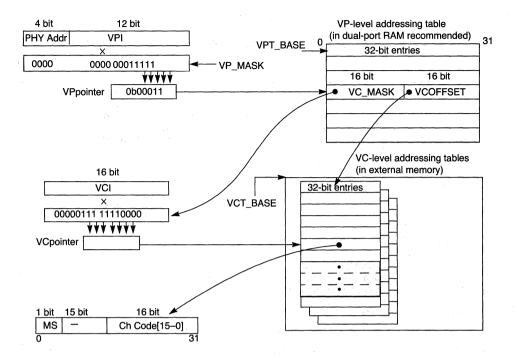
Figure 29-5. Address Compression Mechanism
