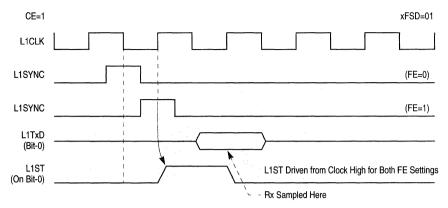
Figure 14-14 shows the effects of changing FE when CE = 1 with a 1-bit frame sync delay.
