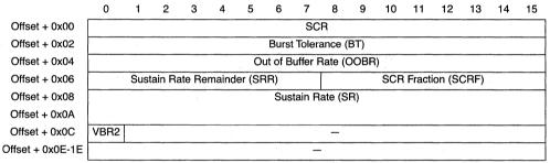
Figure 29-34. Transmit Connection Table Extension (TCTE)—VBR Protocol-Specific
