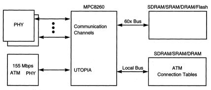
Figure 1-9. Basic System Configuration
