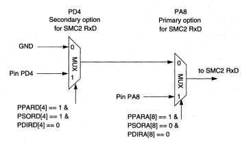
Figure 35-7. Primary and Secondary Option Programming
