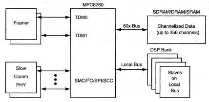
Figure 1-6. Cellular Base Station Configuration
