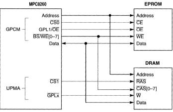
Figure 10-3. Simple System Configuration
