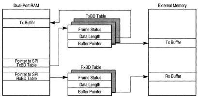
Figure 33-10. SPI Memory Structure
