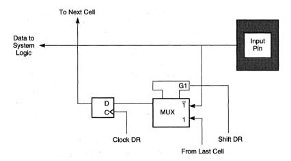
Figure 12-4. Observe-Only Input Pin Cell (I.Obs)
