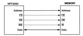
Figure 10-43. GPCM Memory Device Interface
