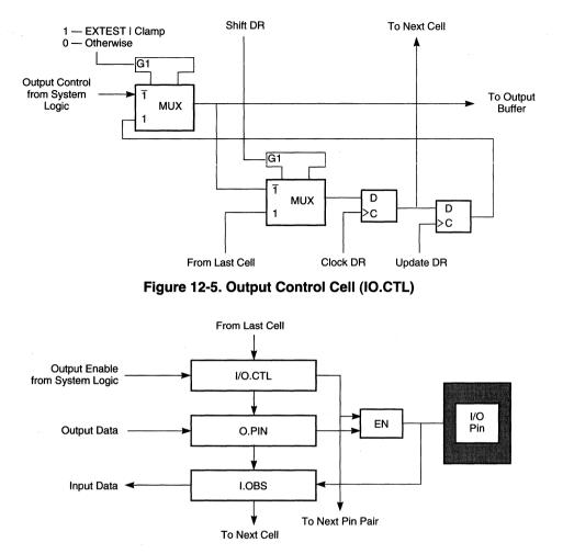
Figure 12-6. General Arrangement of Bidirectional Pin Cells
