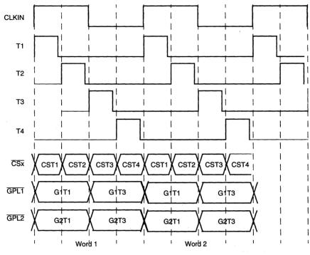
Figure 10-60. UPM Signals Timing Example
