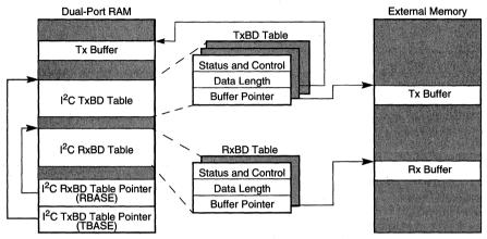
Figure 34-12. I<sup>2</sup>C Memory Structure
