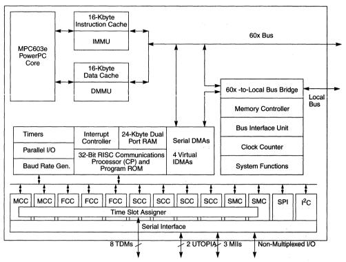
Figure 1-1. MPC8260 Block Diagram
