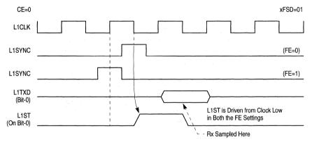
Figure 14-15. Falling Edge (FE) Effect When CE = 0 and xFSD = 01
