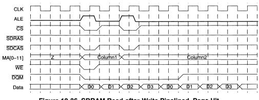
Figure 10-36. SDRAM Read-after-Write Pipelined, Page Hit
