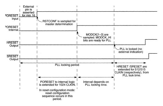
Figure 5-3 shows the power-on reset flow.
