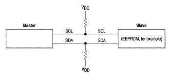
Figure 34-2. I<sup>2</sup>C Master/Slave General Configuration
