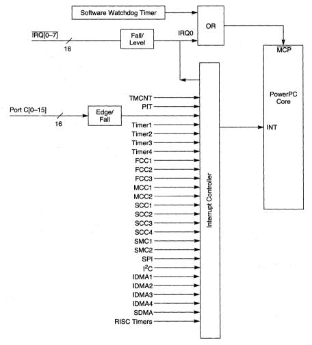
Figure 4-8. MPC8260 Interrupt Structure
