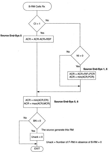
Figure 29-14. ABR Receive Flow
