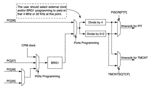
Figure 4-3. Timers Clock Generation
