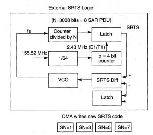
Figure 29-65. AAL1 SRTS Clock Recovery Using External Logic
