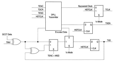
Figure 19-14. DPLL Transmitter Block Diagram
