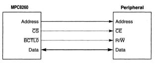
Figure 10-41. GPCM Peripheral Device Interface
