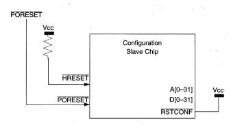
Figure 5-4. Single Chip with Default Configuration
