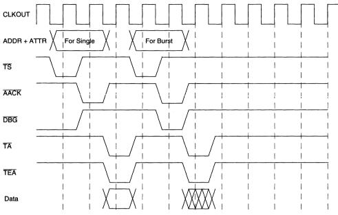
Figure 8-11. Data Tenure Terminated by Assertion of TEA
