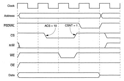
Figure 10-48. GPCM Relaxed-Timing Write (ACS = 10, SCY = 0, CSNT = 1, TRLX = 1)
