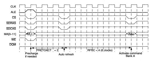
Figure 10-25. RFRC = 4 (6 Clock Cycles)
