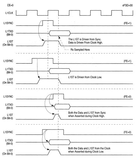
Figure 14-17 shows the effects of changing FE when CE = 0 with no frame sync delay.
