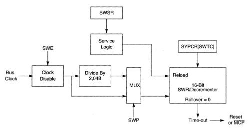
Figure 4-7. Software Watchdog Timer Block Diagram
