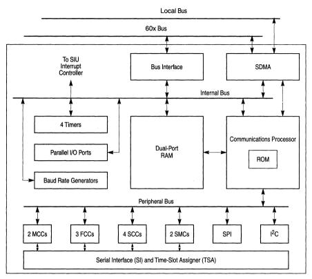
Figure 13-1. MPC8260 CPM Block Diagram
