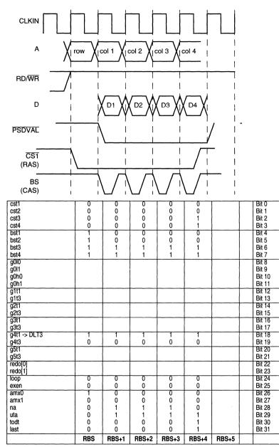
Figure 10-75. FPM DRAM Burst Read Access (Data Sampling on Falling Edge of CLKIN)
