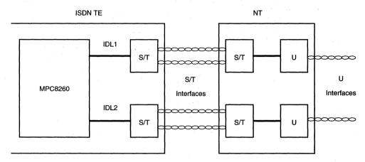
Figure 14-21. Dual IDL Bus Application Example
