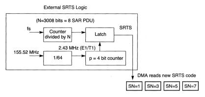
Figure 29-64. AAL1 SRTS Generation Using External Logic
