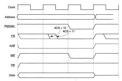
Figure 10-47. GPCM Relaxed-Timing Write (ACS = 1x, SCY = 0, CSNT = 0,TRLX = 1)
