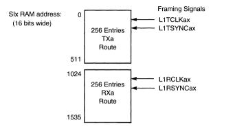
Figure 14-5. One TDM Channel with Static Frames and Independent Rx and Tx Routes
