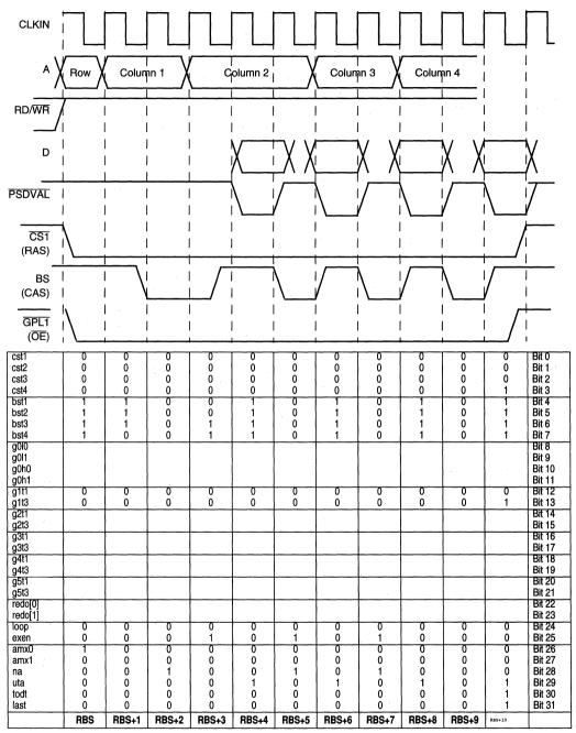
Figure 10-80. Burst Read Access to EDO DRAM
