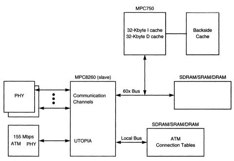
Figure 1-11. High-Performance System Microprocessor Configuration
