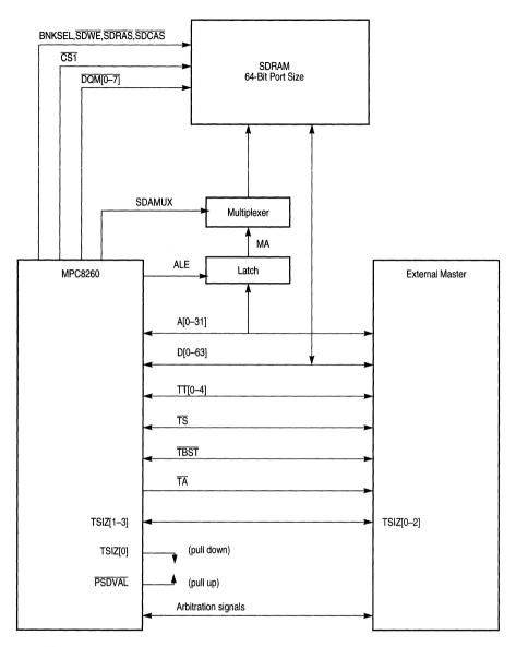
Figure 10-86. External Master Configuration with SDRAM Device
