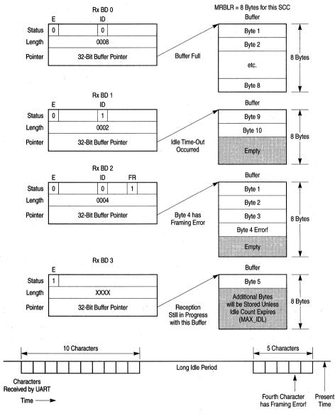
Figure 20-7. SCC UART Receiving using RxBDs
