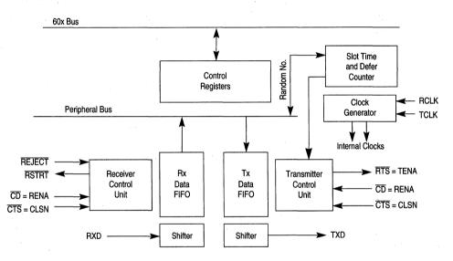
Figure 24-2. Ethernet Block Diagram
