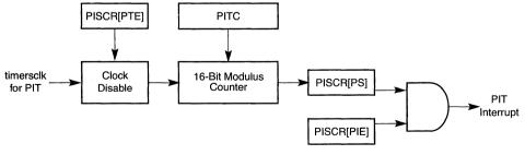
Figure 4-5. PIT Block Diagram
