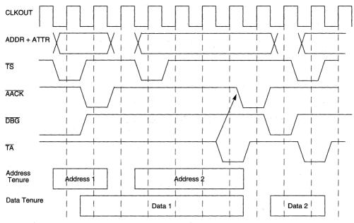
Figure 8-5. Address Pipelining
