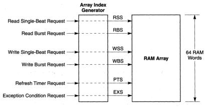
Figure 10-56. RAM Array Indexing
