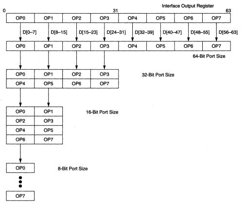
Figure 8-6. Interface to Different Port Size Devices
