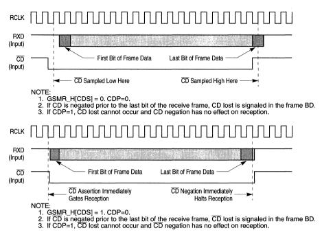
Figure 19-12. Using CD to Control Synchronous Protocol Reception
