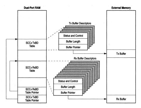
Figure 19-7. SCC BD and Buffer Memory Structure
