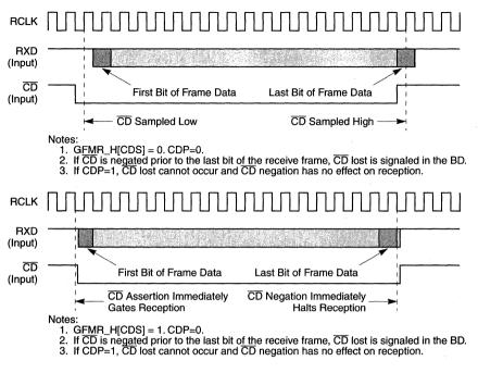
Figure 28-9. Using CD to Control Reception
