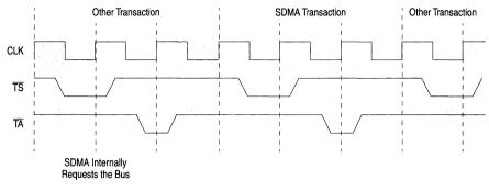
Figure 18-2. SDMA Bus Arbitration (Transaction Steal)
