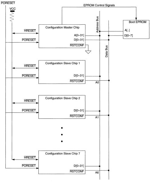
Figure 5-6. Configuring Multiple Chips
