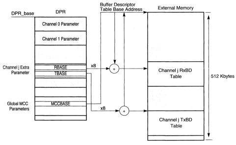
Figure 27-1. BD Structure for One MCC
