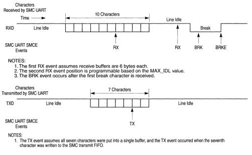
Figure 26-10. SMC UART Interrupts Example
