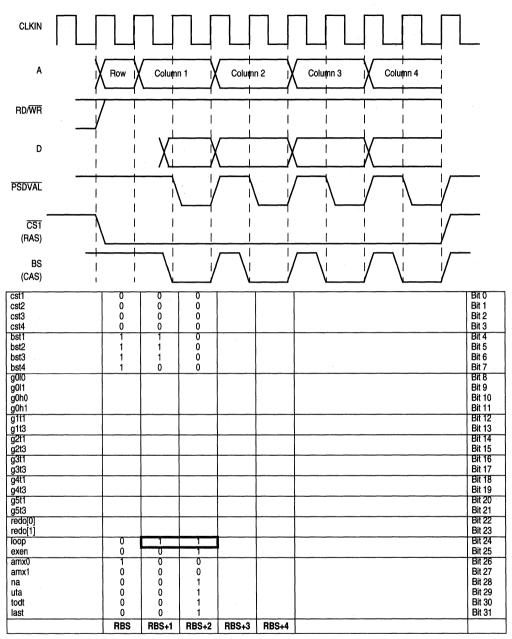
Figure 10-71. Burst Read Access to FPM DRAM (LOOP)
