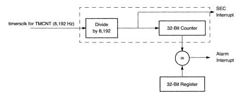
Figure 4-4. TMCNT Block Diagram
