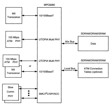
Figure 1-5. LAN-to-WAN Bridge Router Configuration
