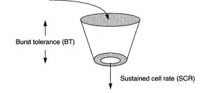
Figure 29-2. VBR Pacing Using the GCRA (Leaky Bucket Algorithm)
