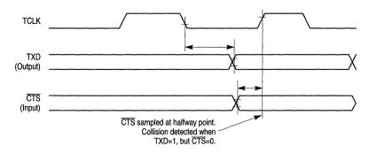
Figure 21-12. Detecting an HDLC Bus Collision
