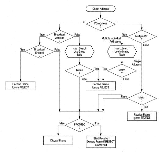
Figure 24-4. Ethernet Address Recognition Flowchart
