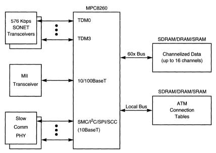
Figure 1-8. SONET Transmission Controller Configuration
