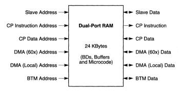
Figure 13-7. Dual-Port RAM Block Diagram
