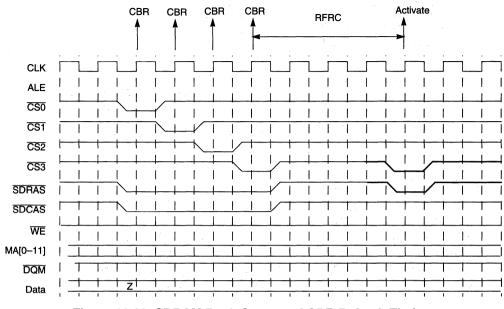
Figure 10-39. SDRAM Bank-Staggered CBR Refresh Timing
