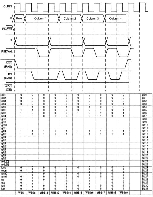
Figure 10-81. Burst Write Access to EDO DRAM
