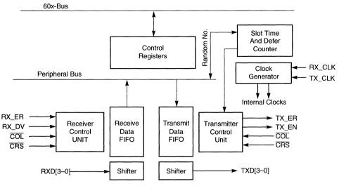
Figure 30-2. Ethernet Block Diagram
