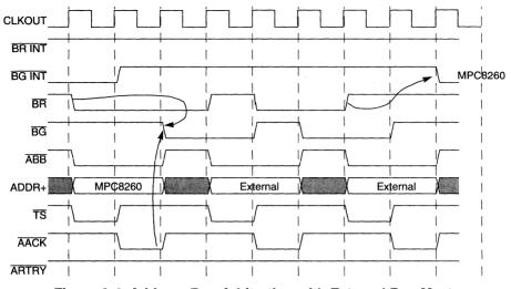
Figure 8-4. Address Bus Arbitration with External Bus Master
