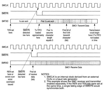
Figure 26-11. Synchronization with SMSYNx
