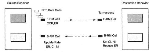
Figure 29-10. MPC8260's ABR Basic Model
