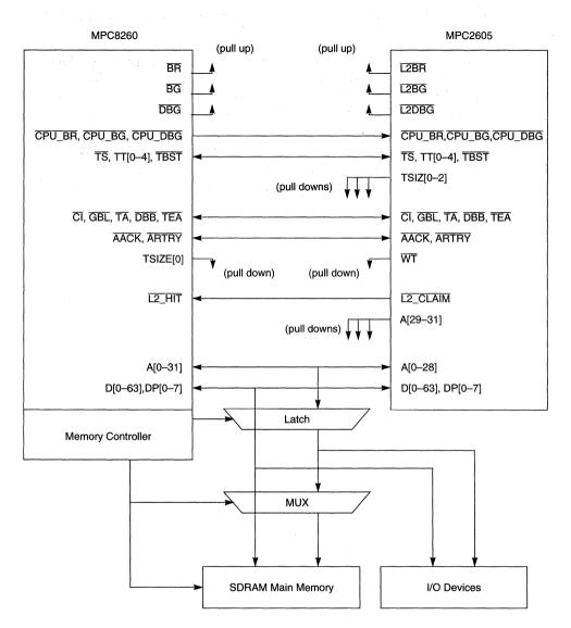
Figure 11-3. External L2 Cache in ECC/Parity Mode
