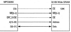
Figure 10-40. GPCM-to-SRAM Configuration
