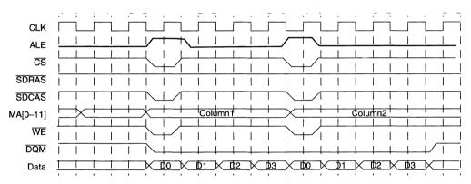
Figure 10-35. SDRAM Write-after-Write Pipelined, Page Hit
