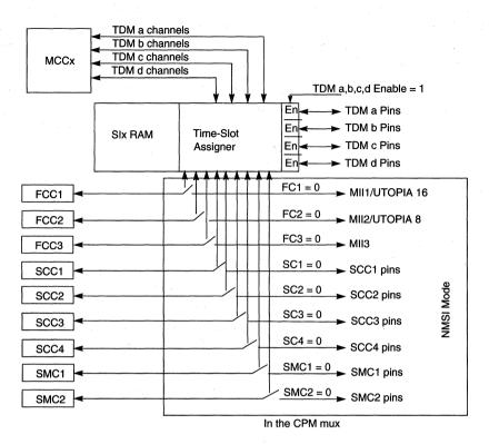
Figure 14-4. Enabling Connections to the TSA
