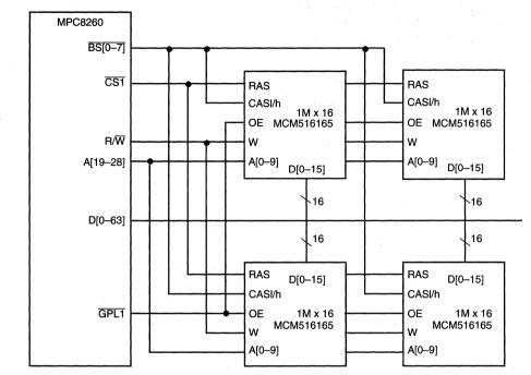
Figure 10-76. MPC8260/EDO Interface Connection to the 60x Bus
