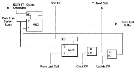
Figure 12-3. Output Pin Cell (O.Pin)
