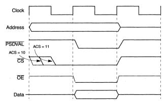
Figure 10-42. GPCM Peripheral Device Basic Timing (ACS = 1x and TRLX = 0)
