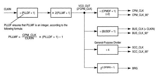
Figure 9-1. System PLL Block Diagram
