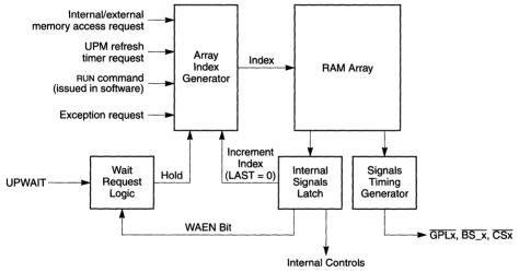
Figure 10-55. User-Programmable Machine Block Diagram
