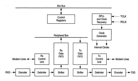
Figure 19-1. SCC Block Diagram
