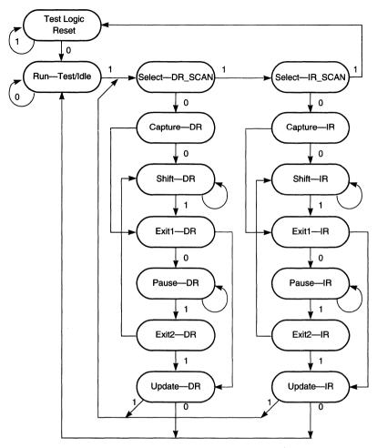
Figure 12-2. TAP Controller State Machine
