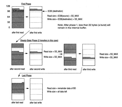
Figure 18-6 shows an example of the three IDMA transfer stages.
