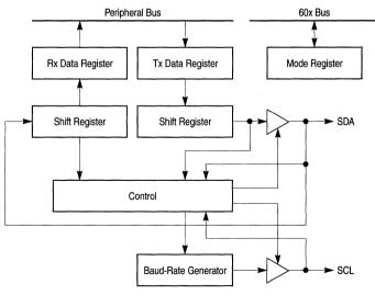
Figure 34-1. I<sup>2</sup>C Controller Block Diagram
