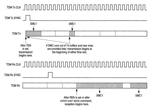
Figure 26-12. Synchronization with the TSA
