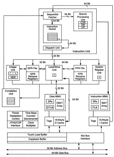
Figure 2-1. MPC8260 Integrated Processor Core Block Diagram
