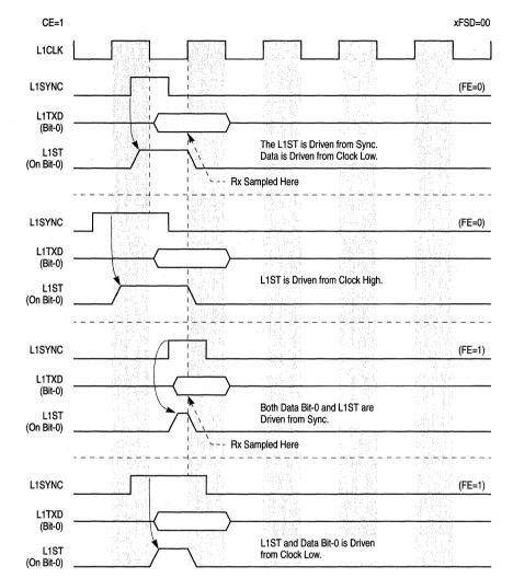
Figure 14-16 shows the effects of changing FE when CE = 1 with no frame sync delay.
