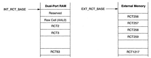
Figure 29-24. Example of a 1024-Entry Receive Connection Table
