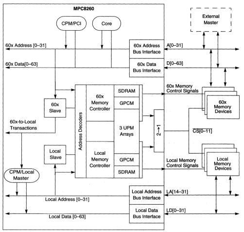
Figure 10-1. Dual-Bus Architecture
