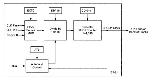
Figure 16-1. Baud-Rate Generator (BRG) Block Diagram
