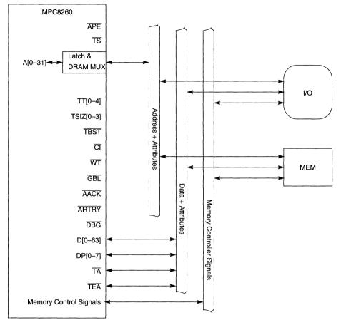
Figure 8-1. Single MPC8260 Bus Mode
