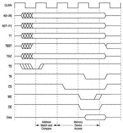
Figure 10-85. External Master Access (GPCM)
