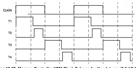
Figure 10-59. Memory Controller UPM Clock Scheme for Non-Integer (2.5:1/3.5:1) Clock Ratios
