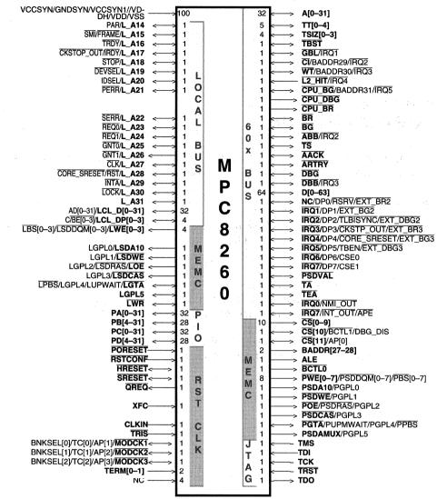
Figure 6-1. MPC8260 External Signals
