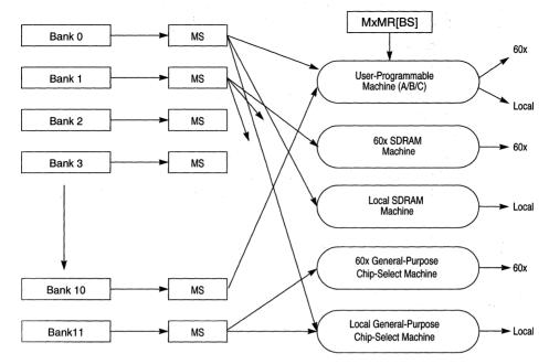
Figure 10-2. Memory Controller Machine Selection
