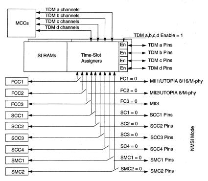
Figure 15-2. Enabling Connections to the TSA
