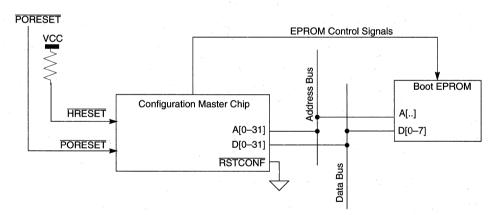
Figure 5-5. Configuring a Single Chip from EPROM
