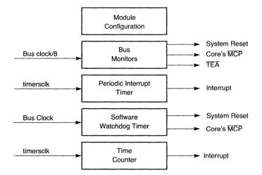
Figure 4-2 is a block diagram of the system configuration and protection logic.
