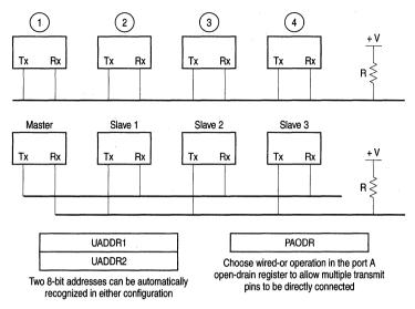
Figure 20-2. Two UART Multidrop Configurations
