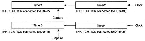
Figure 17-2. Timer Cascaded Mode Block Diagram
