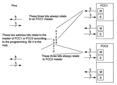
Figure 15-5. Connection of the Master Address
