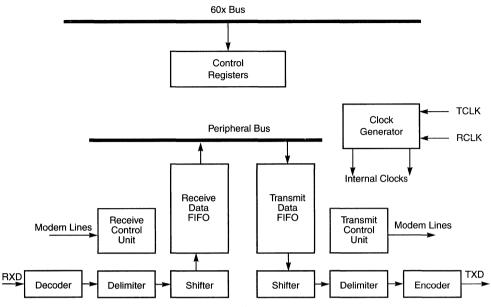
Figure 28-1. FCC Block Diagram
