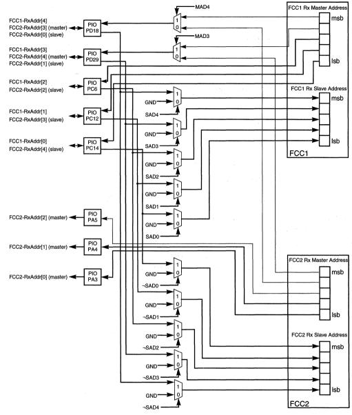
Figure 15-7. Multi-PHY Receive Address Multiplexing
