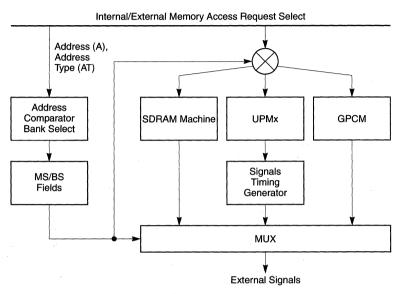
Figure 10-4. Basic Memory Controller Operation
