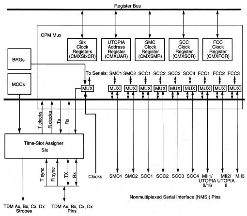
Figure 15-1. CPM Multiplexing Logic (CMX) Block Diagram
