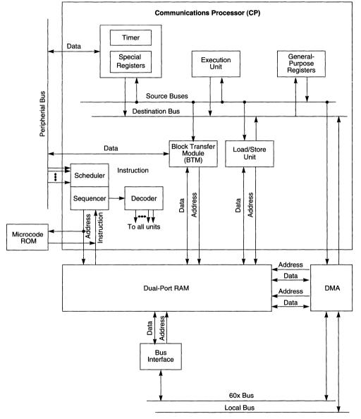
Figure 13-2 shows the CP block diagram.
