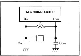
Fig.4.1.2 Oscillating Circuit Using a Crystal Resonator
