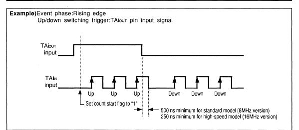
Fig.7.2.4 Recommended Waveform for Up/Down Switching Input and Event Input
