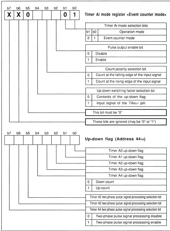
Fig 2.7.10 Event Counter Mode Related Registers Bit Structure
