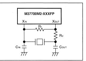
Fig.4.1.1 Oscillating Circuit Using a Ceramic Resonator
