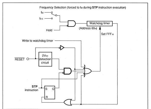
Fig.2.11.1 Watchdog Timer Block Diagram
