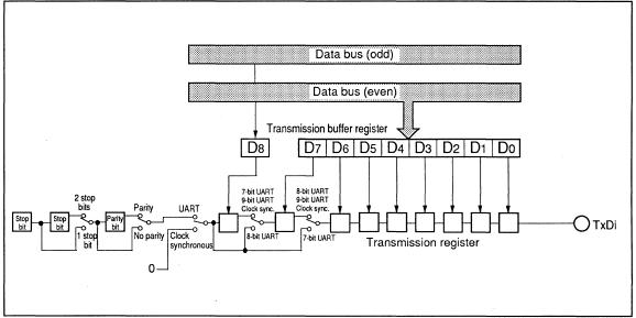
Fig.2.9.6 Serial I/O Transmission Block Diagram
