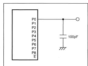
Fig.5.3.1 Testing Circuit for Ports P0~P8
