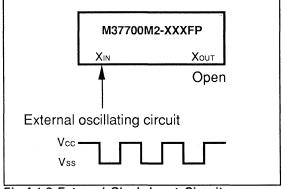
Fig.4.1.3 External Clock Input Circuit
