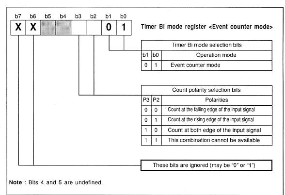
Fig.2.8.7 Timer Bi Mode Register Bit Configuration in Event Counter Mode
