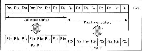
Fig.2.5.8 Data Bus (when BYTE="L")
