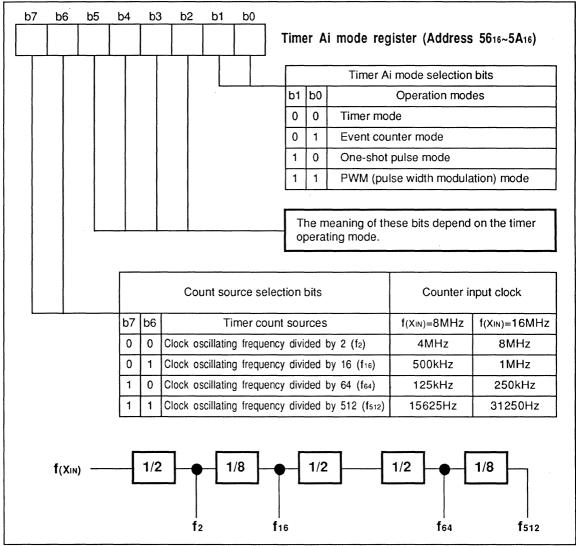
Fig.2.7.5 Timer Ai Mode Register Bit Structure
