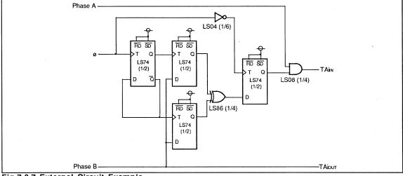
Fig.7.2.7 External Circuit Example
