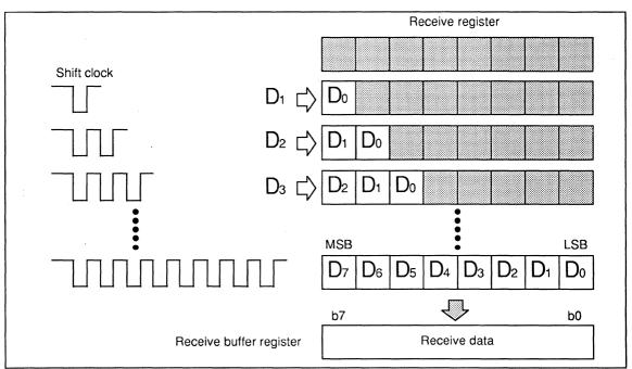
Fig.2.9.14 Serial I/O Receive Operation
