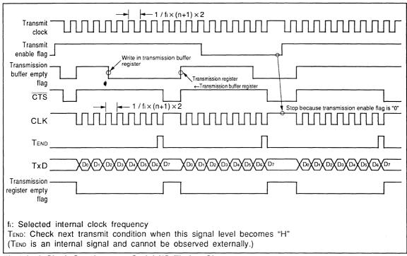
Fig.2.9.12 Clock Synchronous Serial I/O Timing Chart
