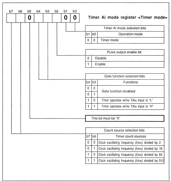
Fig.2.7.7 Timer Ai Mode Register Bit Structure in Timer Mode
