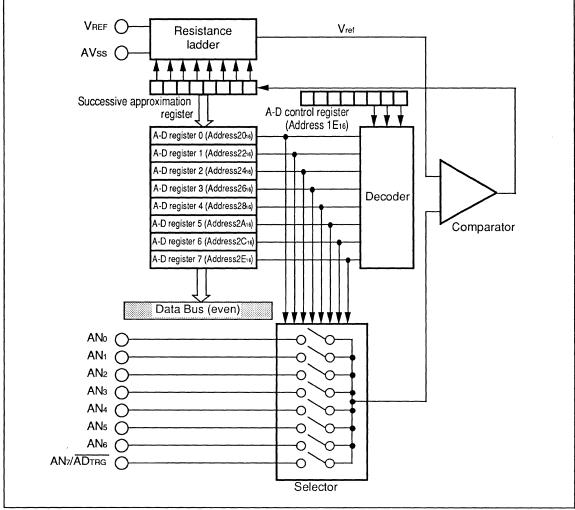
Fig.2.10.1 A-D Converter Block Diagram
