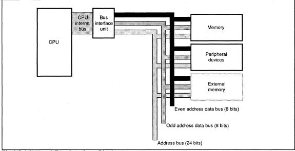
Fig.2.2.1 Internal Bus Interface Block
