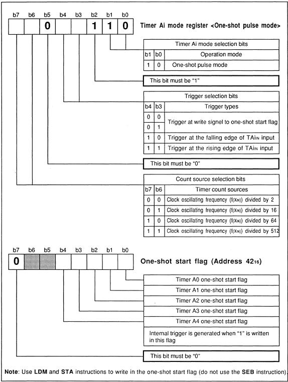
Fig.2.7.15 One-shot Pulse Mode Related Register Bit Structure
