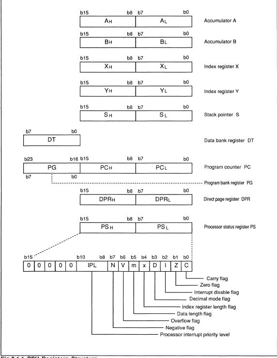
Fig.2.1.1 CPU Registers Structure
