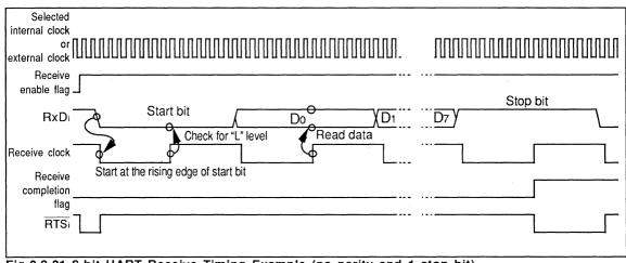
Fig.2.9.21 8-bit UART Receive Timing Example (no parity and 1 stop bit)
