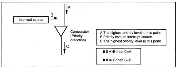
Fig.2.6.6 Interrupt Priority Detection Model
