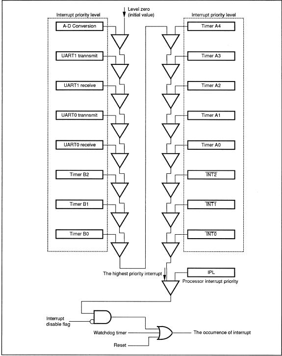
Fig.2.6.6 Interrupt Priority Detection Circuit
