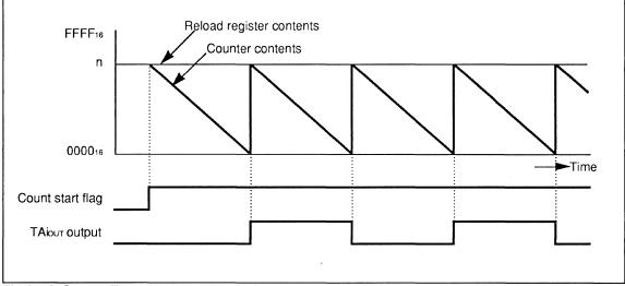
Fig.2.7.9 Output Example when Pulse Output Function is Selected
