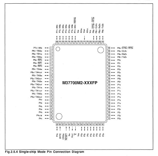
Port P4<sub>2</sub> can be programmed to output ø by setting the processor mode register (PMR). When the ø output selection bit in the processor mode register is set to enable, ø output starts at the rising edge of bus cycle  $\overline{E}$  that was pulled "L" to write "1" in the ø output selection bit.
