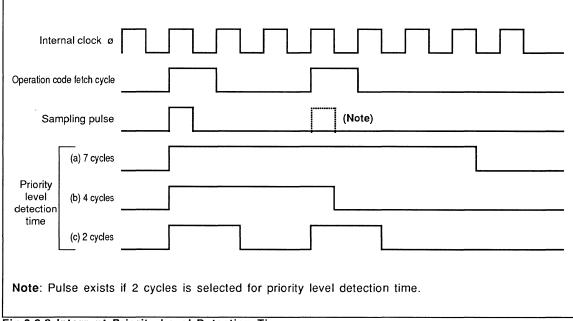
Fig.2.6.8 Interrupt Priority Level Detection Time
