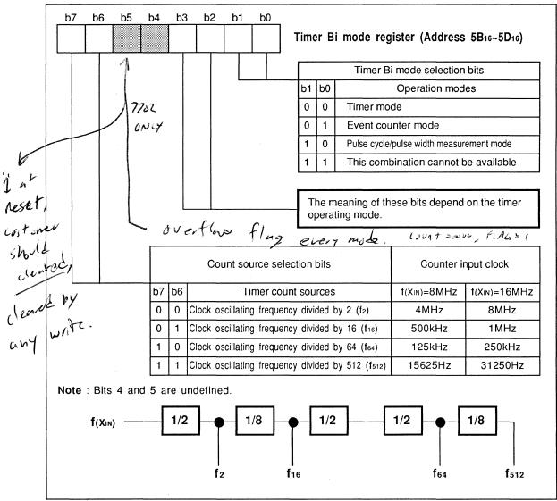
Fig.2.8.3 Timer Bi Mode Register Bit Structure
