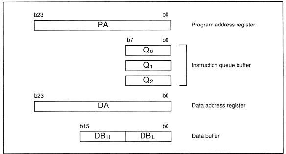
Fig.2.2.2 Bus Interface Unit Registers
