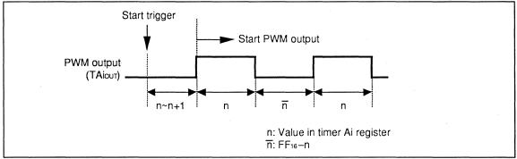
Fig.7.2.11 Pulse Output Start in 8-bit PWM Mode
