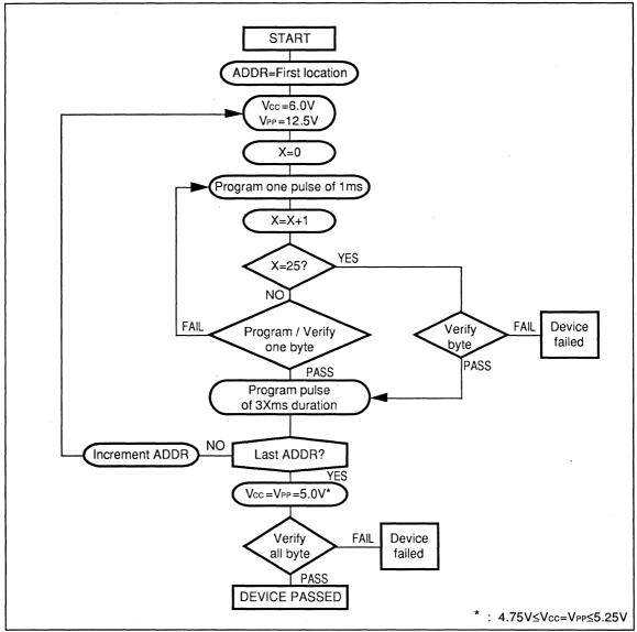
Fig.8.4.1 Fast Programming Algorithm Flow Chart
