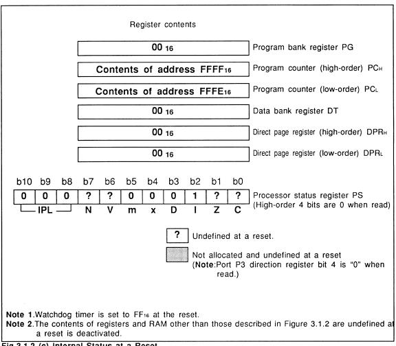
Fig.3.1.2 (c) Internal Status at a Reset
