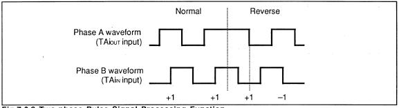
Fig.7.2.6 Two-phase Pulse Signal Processing Function
