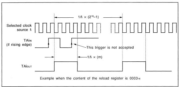
Fig.2.7.18 Output Waveform During 16-bit PWM Mode
