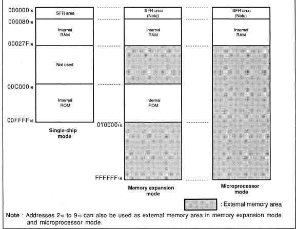
Fig.2.4.5 Memory Map in Each Processor Mode (M37700M2-XXXFP)
