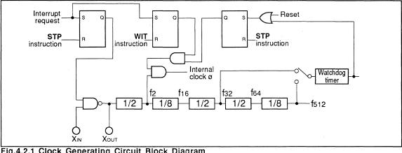
Fig.4.2.1 Clock Generating Circuit Block Diagram
