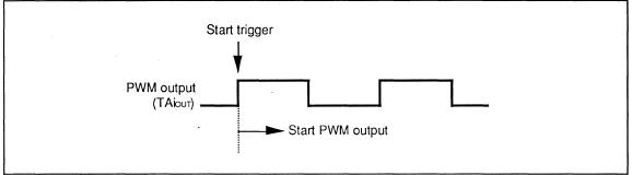
Fig.7.2.10 Pulse Output Start in 16-bit PWM Mode
