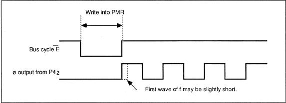
Fig.2.5.5 ø Output Start Timing
