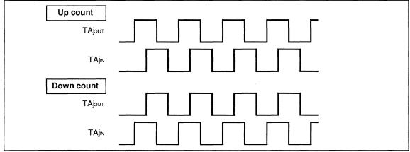
Fig.2.7.13 Two-Phase Pulse Signal Processing Function
