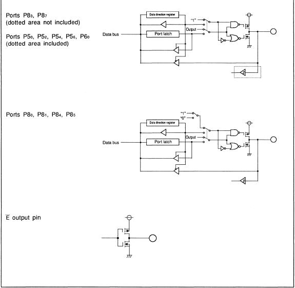
Fig 2.5.3 Port Peripheral Circuit (b)
