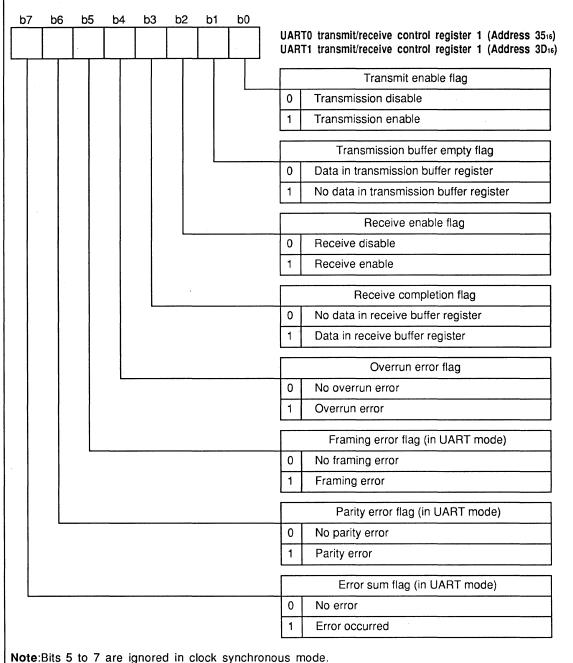
Each error flag is cleared when the content of the receive buffer register is read.
