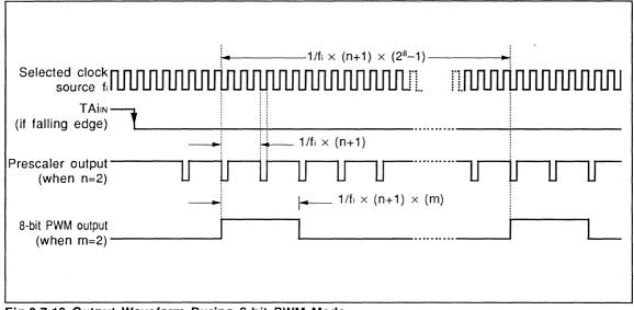
Fig.2.7.19 Output Waveform During 8-bit PWM Mode
