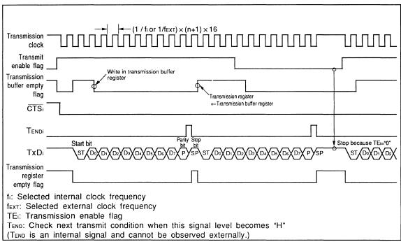
Fig.2.9.18 8-bit UART Transmission Timing Example (with parity and 1 stop bit)
