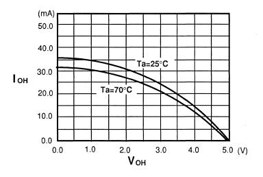
(2)Programmable I/O port (CMOS output) N channel IoL−VoL characteristics ● Supply voltage Vcc=5V
