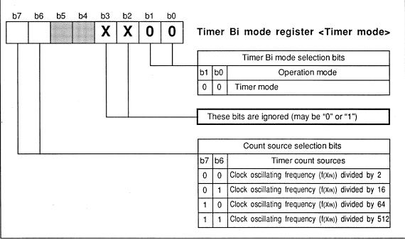
Fig.2.8.5 Timer Bi Mode Register Bit Configuration in Timer Mode
