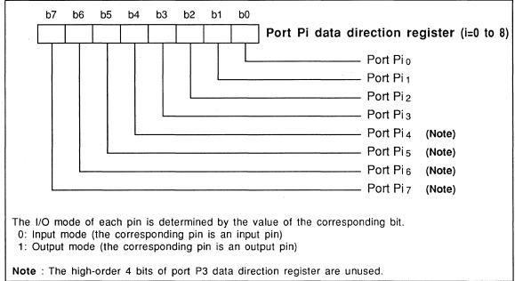
Fig.2.5.1 Relationship between the Port Data Direction register and Pins
