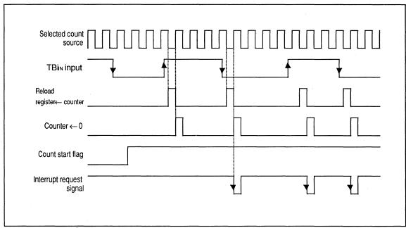
Fig.2.8.10 Timer Operation During Pulse Width Measurement Mode
