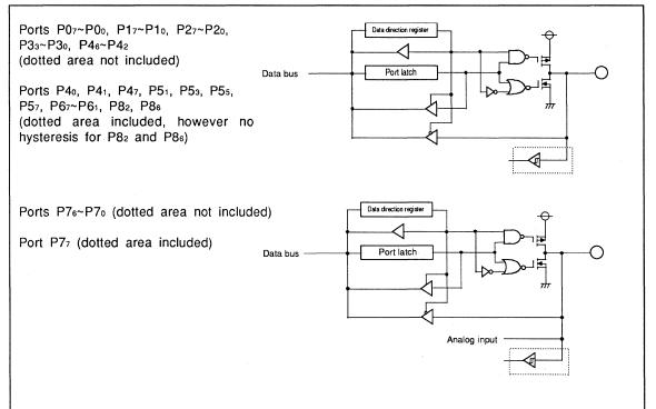
Fig 2.5.3 Port Peripheral Circuit (a)
