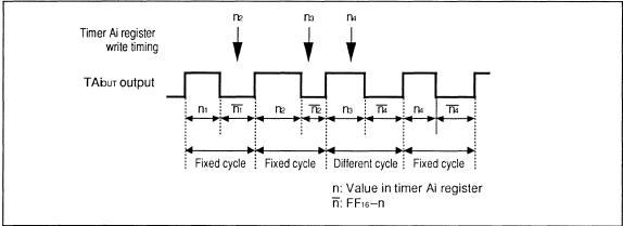
Fig.7.2.9 Output Pulse Cycle in PWM Mode
