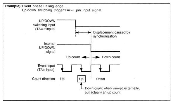
Fig.7.2.3 Displacement Caused by Up/Down Switching
