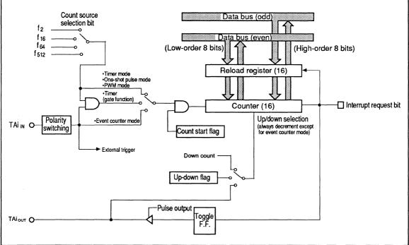
Fig.2.7.1 Timer Ai Block Diagram
