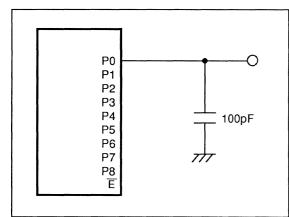
Fig.5.4.1 Testing Circuit for Ports P0~P8
