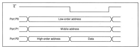
Fig.2.5.11 Bus Timing when External Bus Width is 8 Bits
