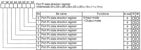
Note: The high-order 4 bits of port P3 data direction register are write prohibited and these bits will always return "0" when read.
