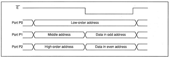
Fig.2.5.9 Bus Timing when External Bus Width is 16 Bits
