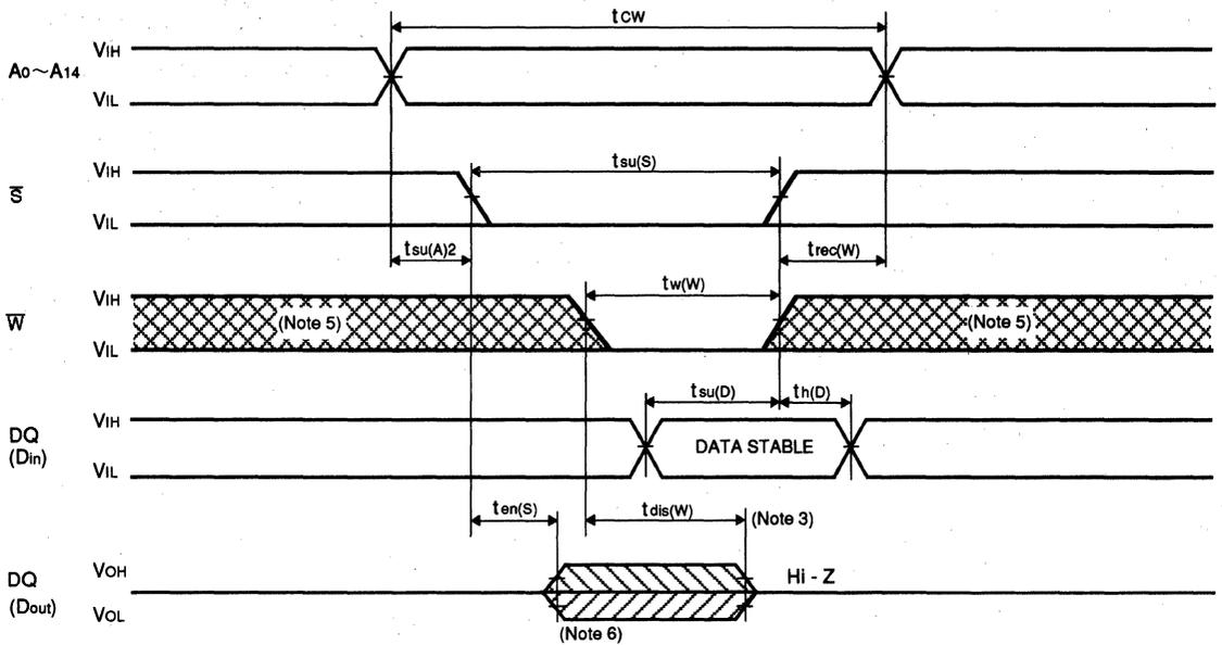
Note 6. When the falling edge of  $\bar{W}$  is simultaneous or prior to the falling edge of  $\bar{S}$ , the output is maintained in the high impedance.
