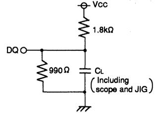
Fig.1 Output load
