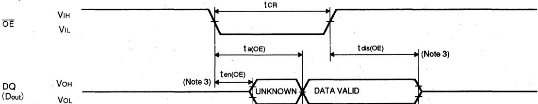
Note 4. Address and  $\bar{S}$  valid prior to  $\bar{OE}$  transition low by  $(t_a(A) - t_a(OE))$ ,  $(t_a(S) - t_a(OE))$ .
