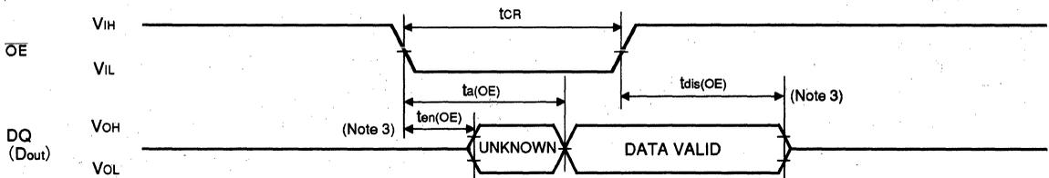
Note4. Address and  $\overline{S}$  valid prior to  $\overline{OE}$  transition low by  $(t_a(A) - t_a(OE))$ ,  $(t_a(S) - t_a(OE))$ .
