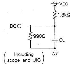
Fig. 1 Output load
