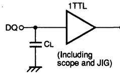
Fig.1 Output load
