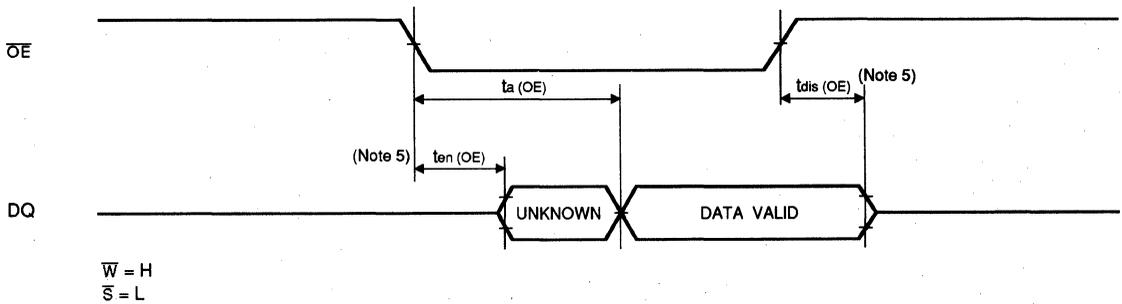
Note 6 : Addresses and  $\bar{S}$  valid prior to  $\bar{OE}$  transition low by  $(t_A(A) - t_A(OE))$ .  $(t_A(S) - t_A(OE))$
