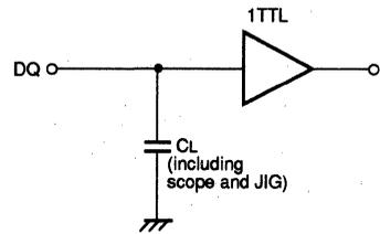
Fig.1 Output load
