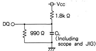
Fig.1 Output load
