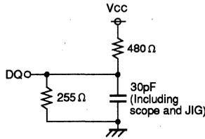
Fig.1 Output load
