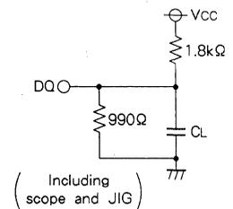
Fig. 1 Output load
