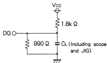
Fig. 1 Output load
