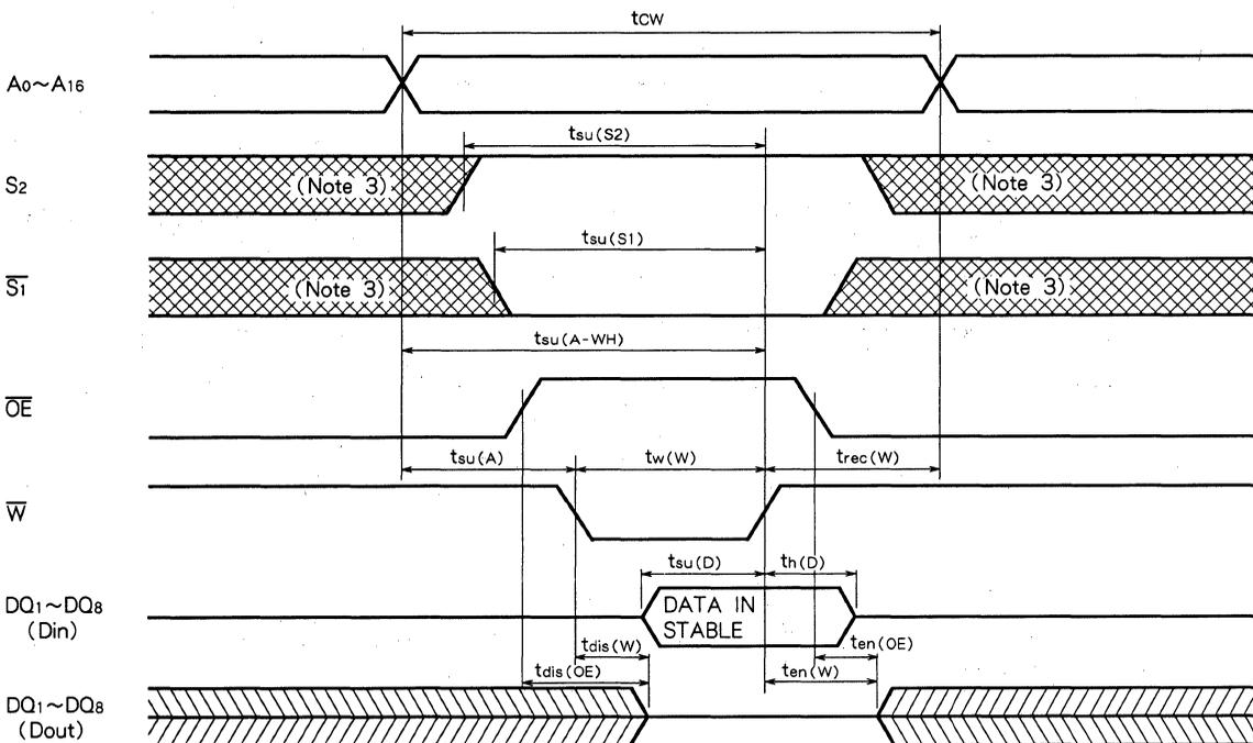
Write cycle ( $\overline{S1}$  control mode)
