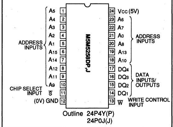
When  $\bar{S}$  is high, the chip is in the non-selectable state, disabling both reading and writing. In this case the output is in the floating (high-impedance) state, useful for OR-ties with other devices.
