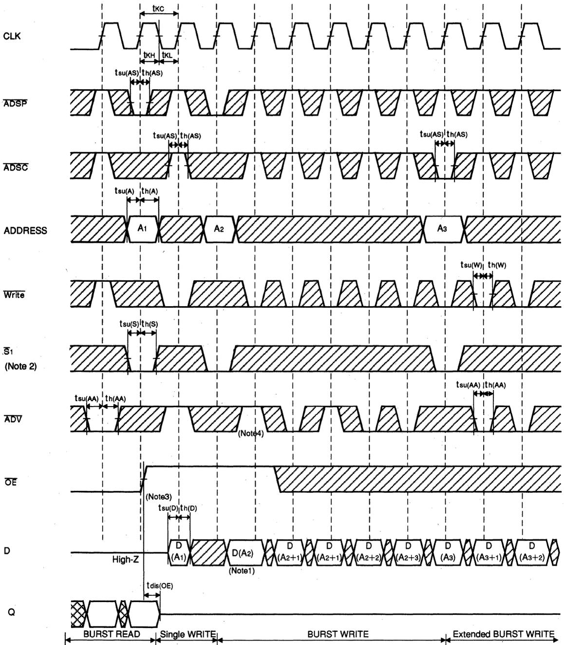
Note 1. Q(A2) refers to output from address A2. Q(A2+1) refers to output from the next internal burst address following A2.
