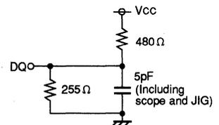
Fig.2 Output load for t<sub>en</sub>, t<sub>dis</sub>
