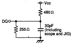
Fig.1 Output load
