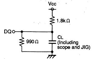
Fig.1 Output load
