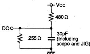
Fig.1 Output load
