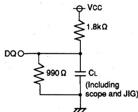
Fig.1 Output load
