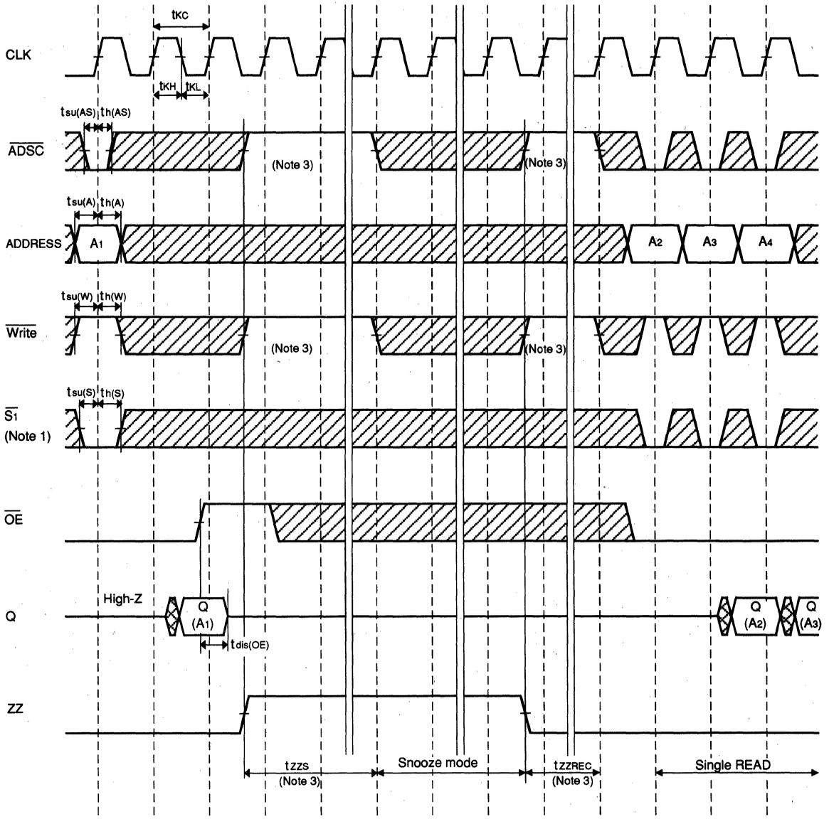
Note 1.  $\overline{S_2}$  and  $S_2$  have timing identical to  $\overline{S_1}$ . On this diagram, when  $\overline{S_1}$  is LOW,  $\overline{S_2}$  is LOW and  $S_2$  is HIGH.
