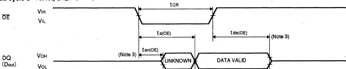
Note 4. Address and  $\bar{S}$  valid prior to  $\bar{OE}$  transition low by  $(t_{a(A)} - t_{a(OE)})$ ,  $(t_{a(S)} - t_{a(OE)})$ .
