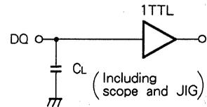
Fig.1 Output load
