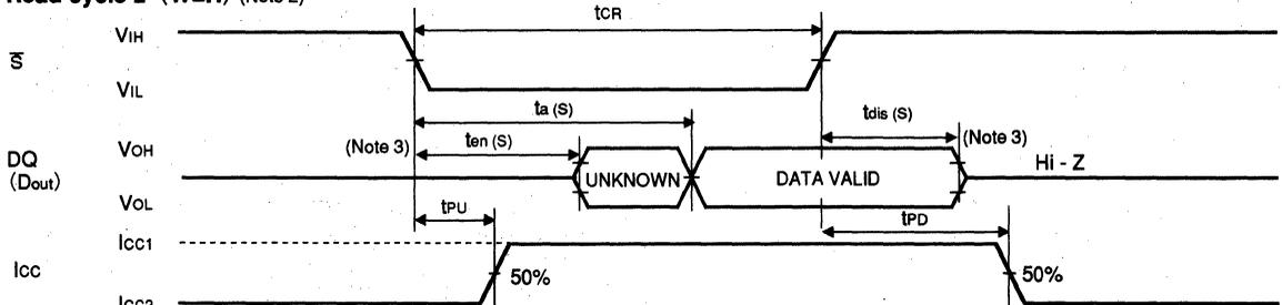
Note2. Address valid prior to or coincident with  $\overline{S}$  transition low.
