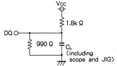
Fig.1 Output load
