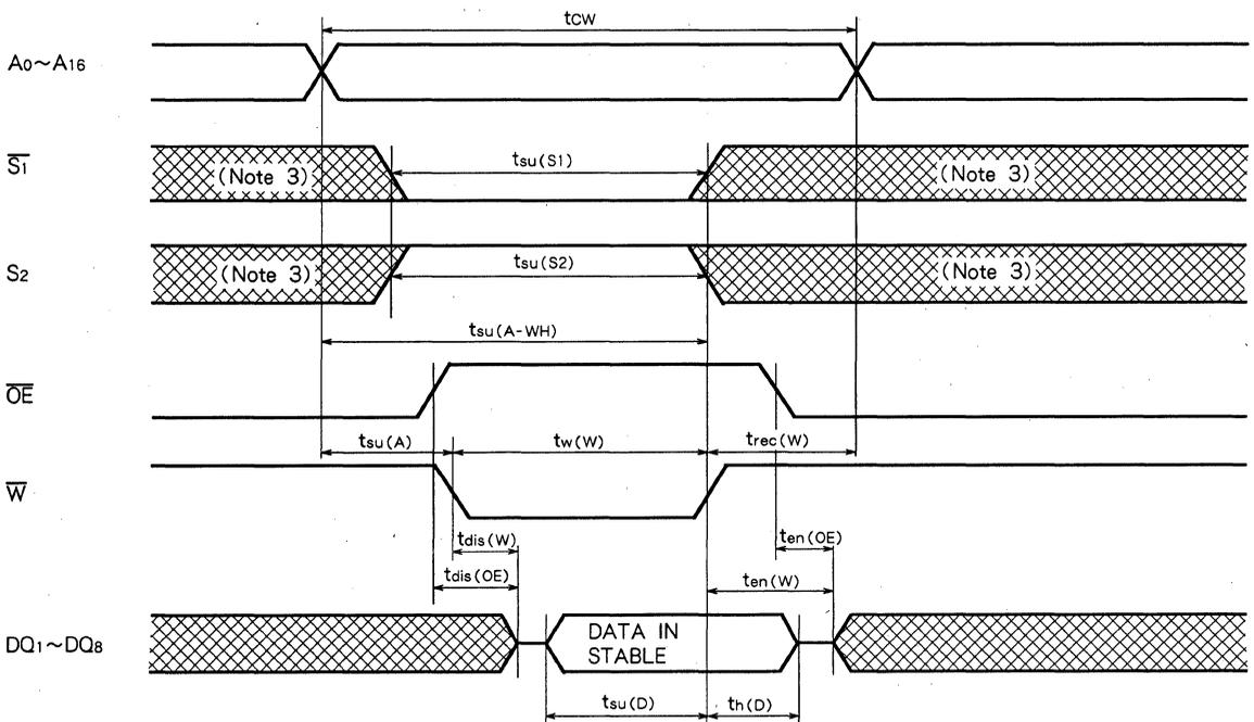
Write cycle ( $\overline{S1}$  control mode)
