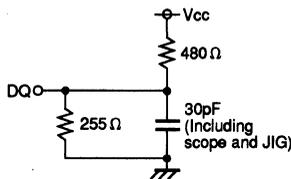
Fig.1 Output load
