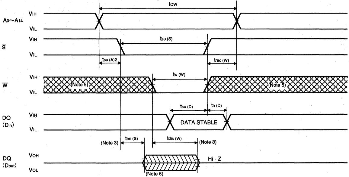
Note6. When the falling edge of  $\bar{W}$  is simultaneous or prior to the falling edge of  $\bar{S}$ , the output is maintained in the high impedance.
