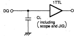
Fig.1 Output load
