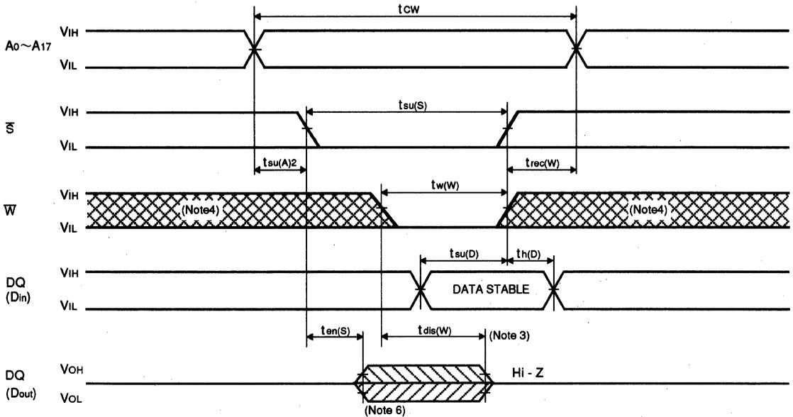
Note 5. When the falling edge of  $\bar{W}$  is simultaneous or prior to the falling edge of  $\bar{S}$ , the output is maintained in the high impedance.
