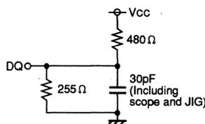
Fig.1 Output load
