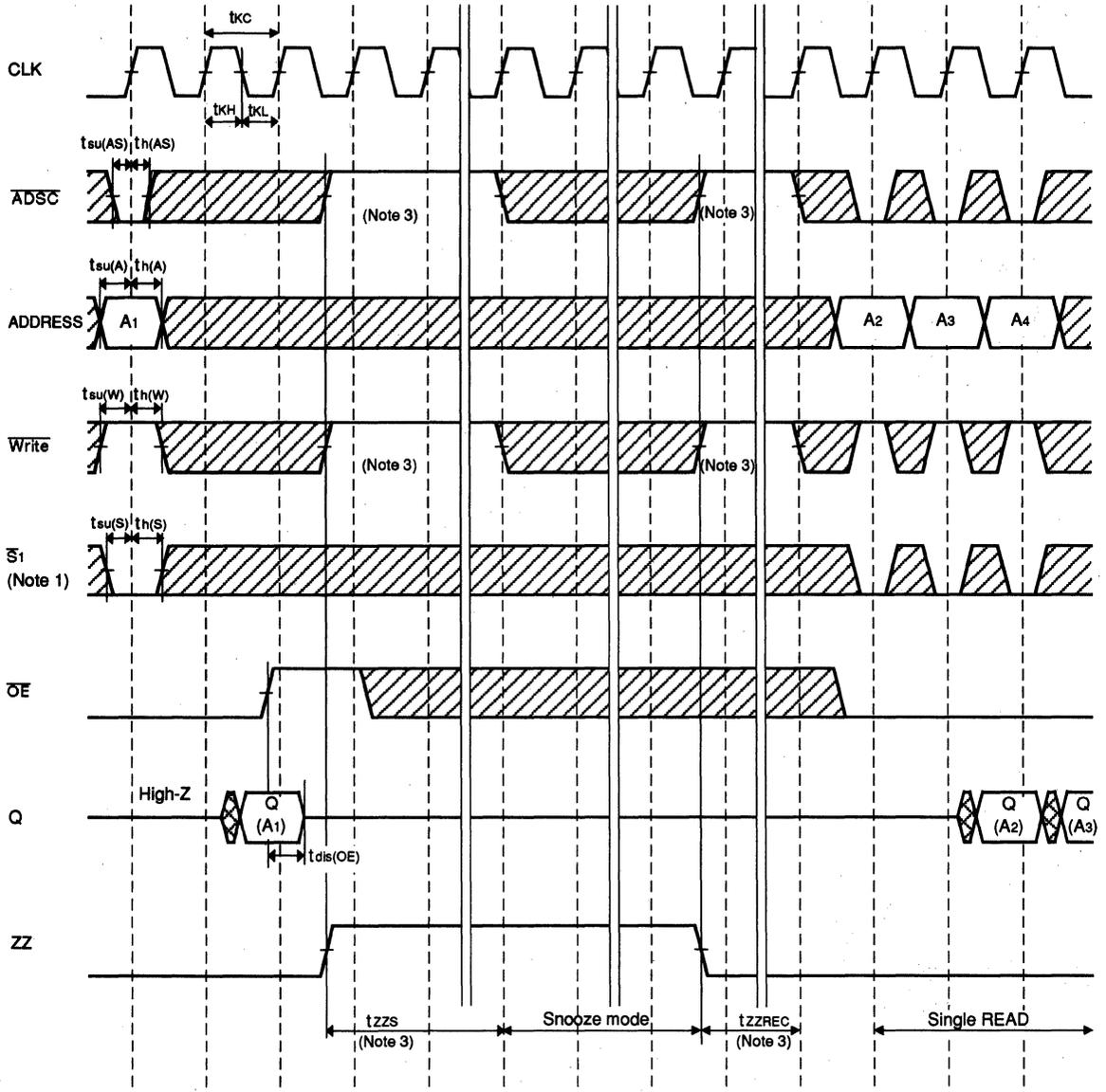
Note 1.  $\overline{S2}$  and  $S2$  have timing identical to  $\overline{S1}$ . On this diagram, when  $\overline{S1}$  is LOW,  $\overline{S2}$  is LOW and  $S2$  is HIGH. When  $\overline{S1}$  is HIGH,  $\overline{S2}$  is HIGH and  $S2$  is LOW.
