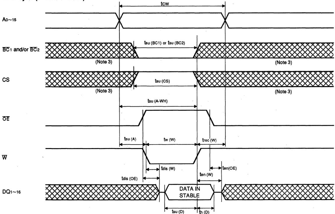
**Write cycle (  $\overline{BC}$  control mode)**
