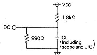
Fig. 1 Output load
