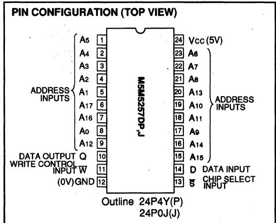
When  $\bar{S}$  is high, the chip is in the non-selectable state, disabling both reading and writing. In this case the output is in the floating (high-impedance) state, useful for OR- ties with other devices.
