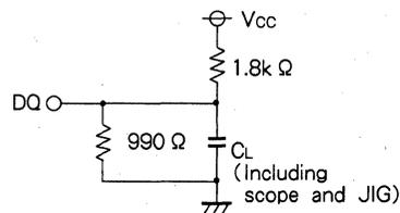
Fig.1 Output load
