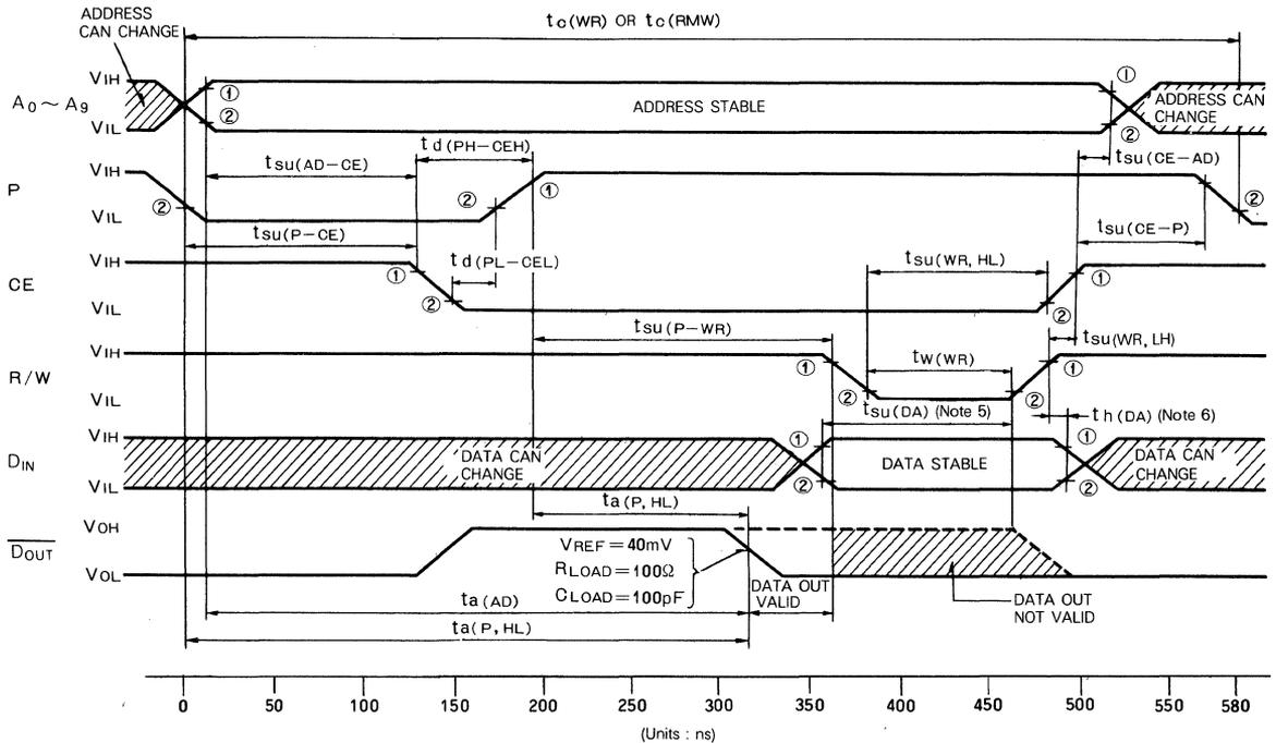
Note 3 : The reference level of point ① is  $V_{SS} - 2V$  . and point ② is  $V_{DD} + 2V$  .
