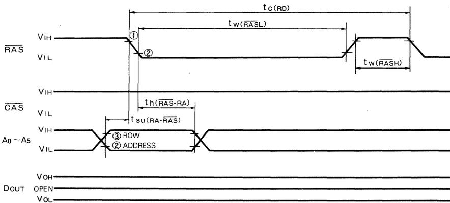
Note 3: Reference level for ①, ③ and ④ is 2.4V.
