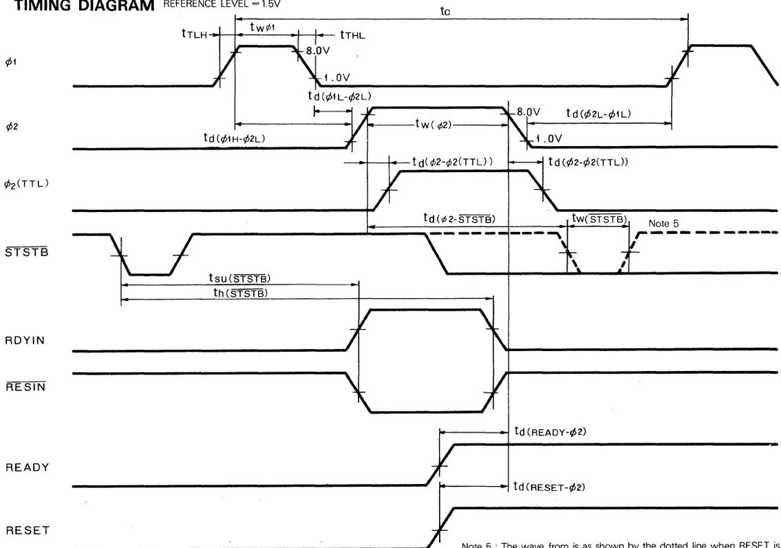
Note 5 : The wave from is as shown by the dotted line when RESET is low.
