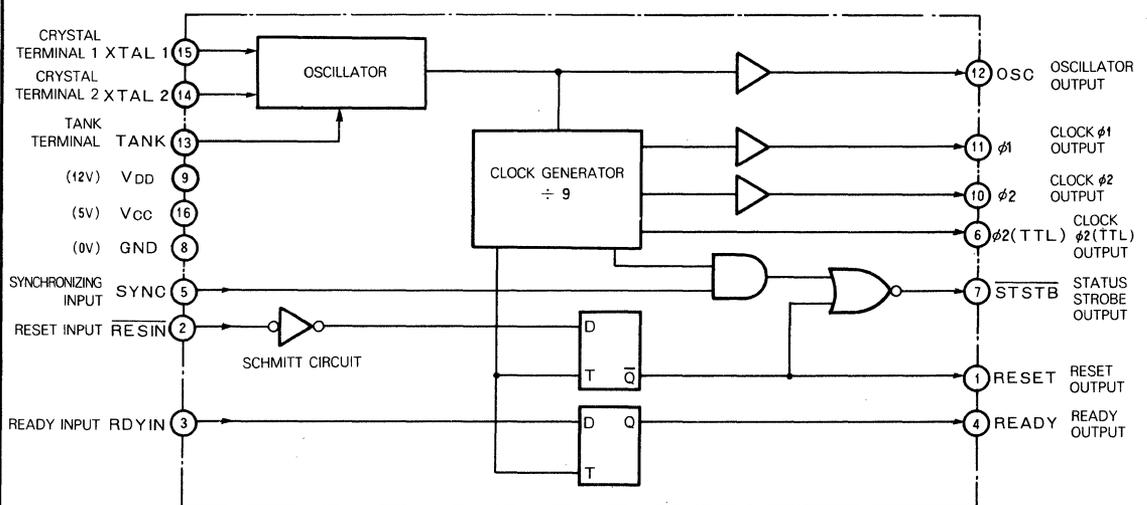
**CLOCK GENERATOR AND DRIVER FOR CPU M58710S**
