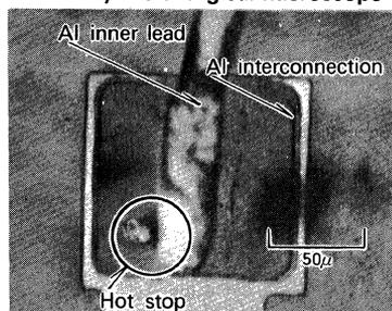
Fig.11 Enlargement of aluminum bridge in Fig. 10, analyzed by XMA-Al ka
