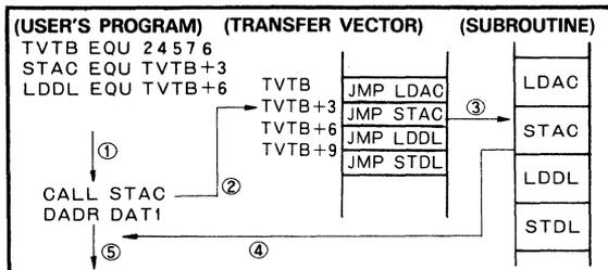
Note 1: The processing order is ①, ②, ③, ④ and ⑤. A transfer vector is used to set the entry address of each subroutine.
