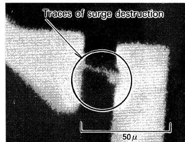
Fig. 14 Electromigration of aluminum interconnection, analyzed by SEM
