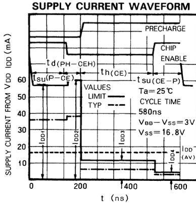
AVERAGE SUPPLY CURRENT FROM  $V_{DD}$
