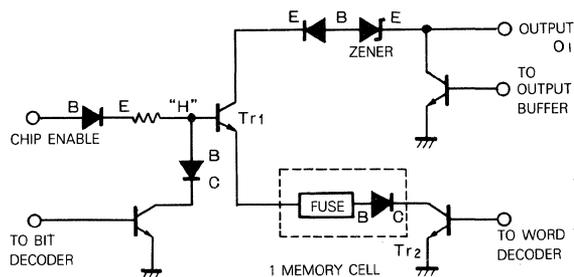
5. After programming is completed, apply an additional three programming pulses.
