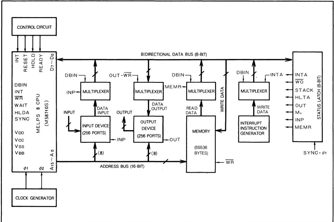
1. After the CPU receives the two phase clocks  $\phi_1$  and  $\phi_2$  from the clock generator and the external reset signal, the address bus provides the address to memory location zero.
