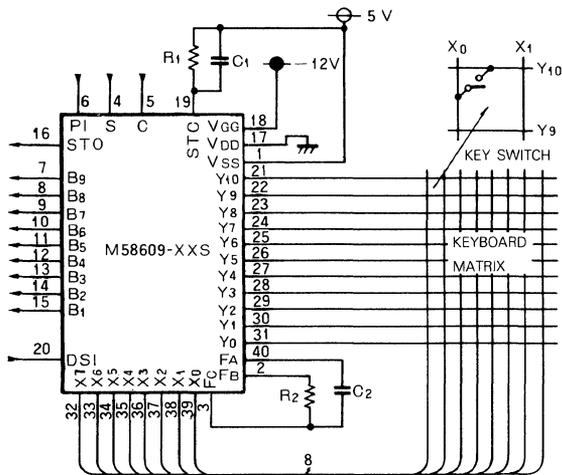
Note 4 : R<sub>1</sub> = 1.5MΩ, C<sub>1</sub> = 0.001μF provides approximately 1.5ms delay time.
