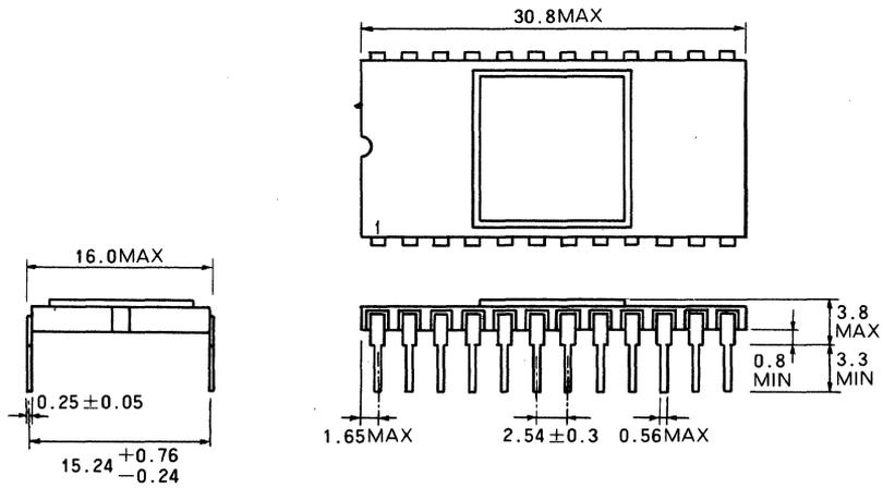
**TYPE 24S10 24-PIN METAL-SEALED CERAMIC DIL WITH QUARTZ LID**
