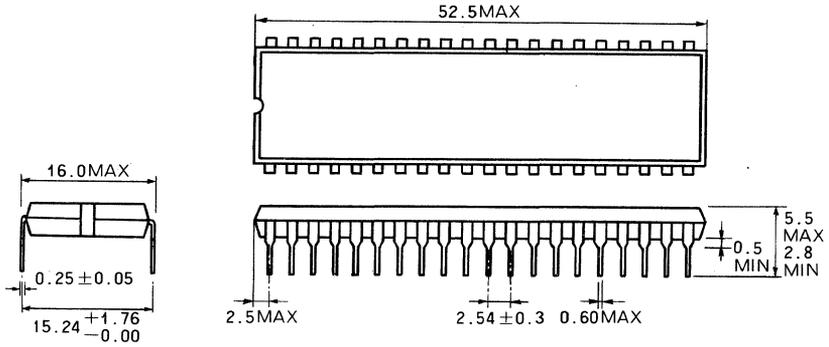
**TYPE 40B1 40-PIN RESIN-SEALED CERAMIC DIL**
