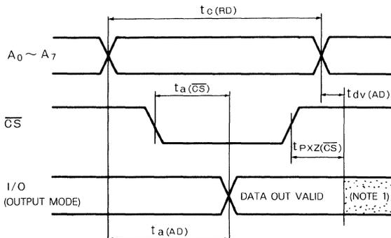
Note 1: In this period, the data out is valid for a definition of  $t_{dv}(AD)$  and is in the floating state for a definition of  $t_{PXZ}(\overline{CS})$
