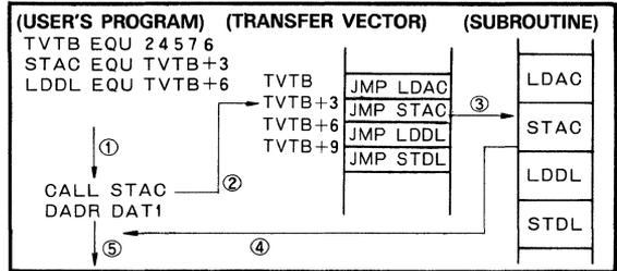
Note: The processing order is ①, ②, ③, ④, ⑤. A transfer vector is used to set the entry address of each subroutine.
