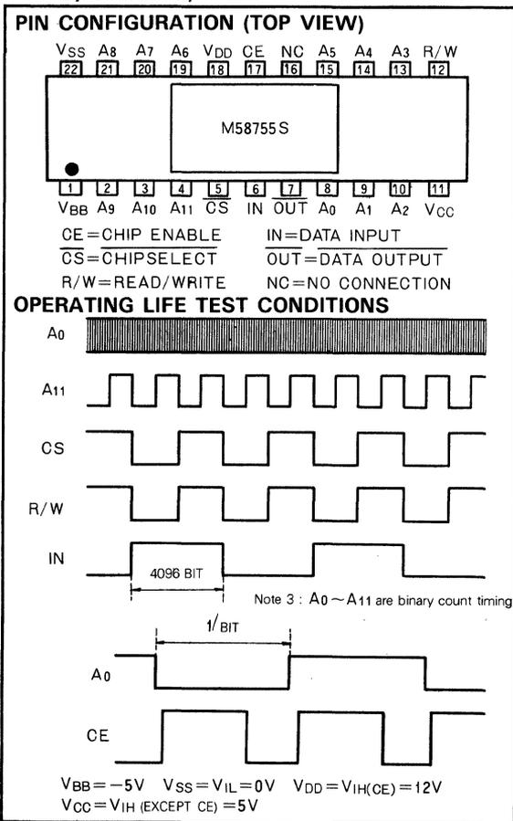
Fig. 7 DC biased test procedure (for M58751 1K-bit static RAM)
