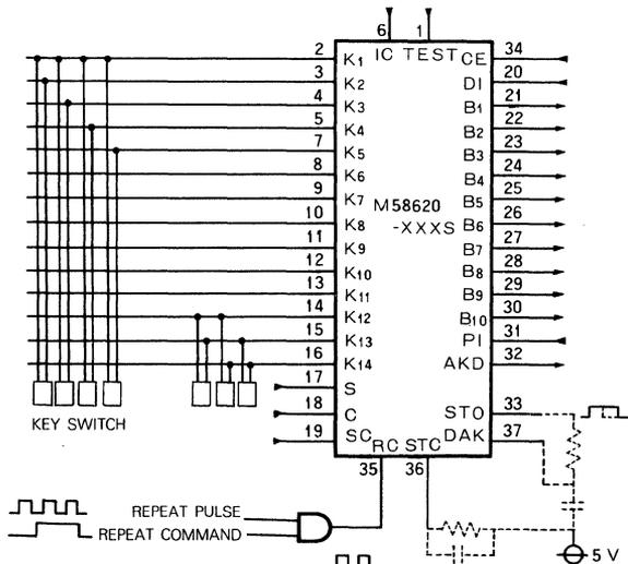
Use a key switch having outputs that are open-collector, or mutually separated by diodes.
