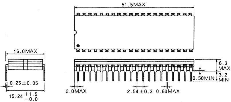
**TYPE 40S1 40-PIN METAL-SEALED CERAMIC DIL**
