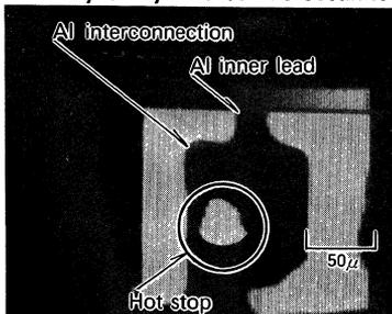
Fig. 8 Corrosion of vapor-deposited aluminum interconnection, analyzed by metallurgical microscope
