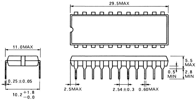
**TYPE 22S1 22-PIN METAL-SEALED CERAMIC DIL**
