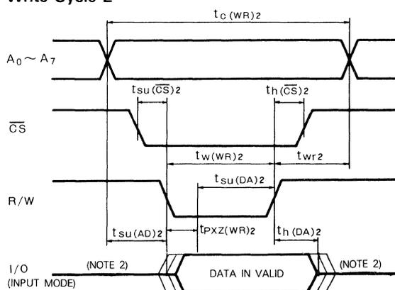
Note 2: The input signals from the external circuits should not be applied to the I/O terminals (keeping them three-state) for during this period the I/O terminals are in the output mode.
