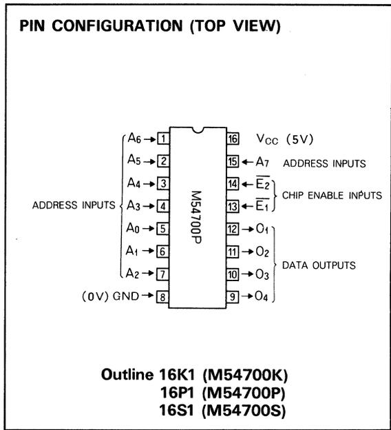
read out in parallel on data outputs  $O_1 \sim O_4$ . All inputs are TTL-compatible. An external decoder is not necessary. All outputs are open-collector outputs, so it is possible to AND-tie them to other ROMs and TTL devices. The AND-tie fanout of each output can accommodate up to 10 standard TTL loads. The chip enables  $\overline{E}_1$  and  $\overline{E}_2$  are used to inhibit data outputs  $O_1 \sim O_4$ .
