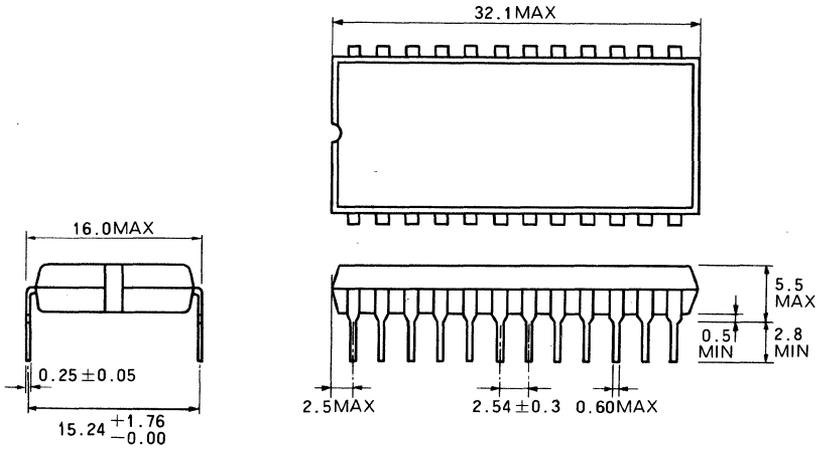
**TYPE 24S1 24-PIN METAL-SEALED CERAMIC DIL**
