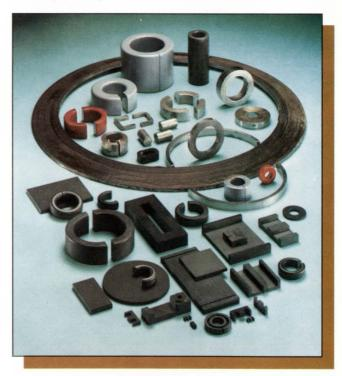
In addition to machined ferrites, components for custom applications include unusual core configurations, both cut and uncut, from strip as thin as 1/8 mil, or from stacking and bonding of stamped parts. Various shapes can also be pressed from powders and then sintered and/or annealed.
