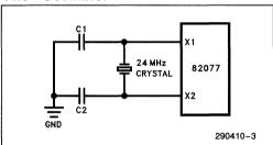
Figure 11-2. Crystal Oscillator Circuit
