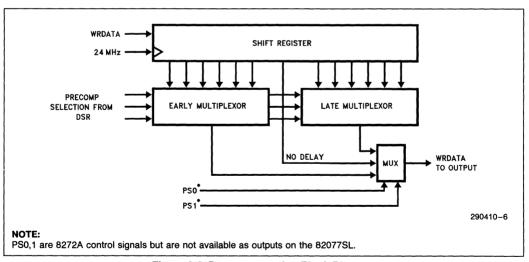
Figure 3-3. Precompensation Block Diagram
