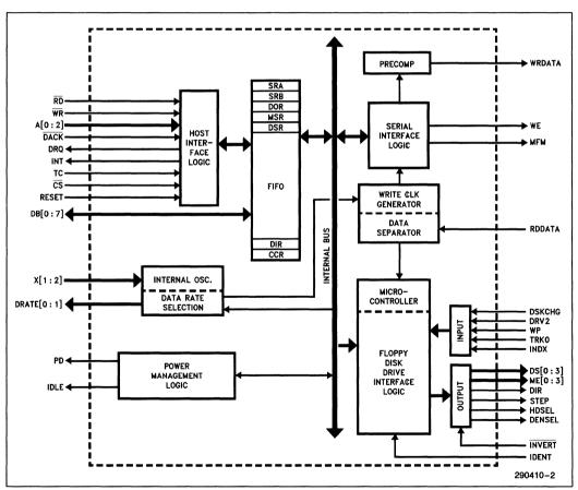
Figure 1-1, 82077SL Block Diagram
