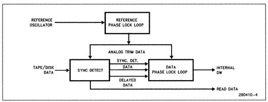
Figure 3-1. Data Separator Block Diagram
