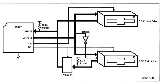
Figure 10-4. Combined 3.5" and 5.25" Drive Interface
