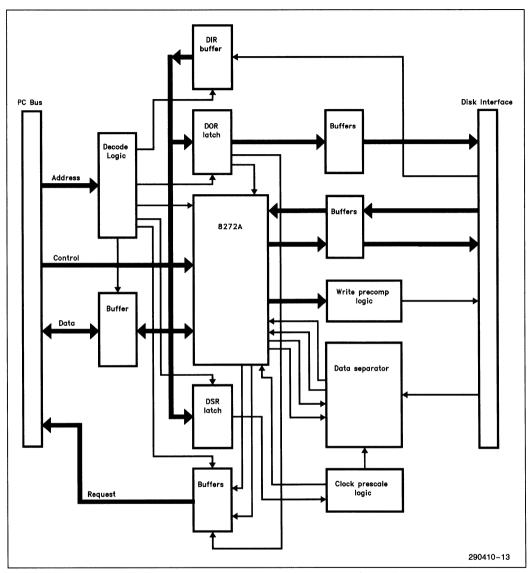
Figure 10-1. Standard IBM PC/AT Floppy Disk Controller
