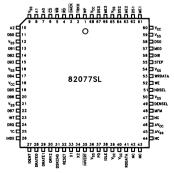
Figure 1. 82077SL Pinout
