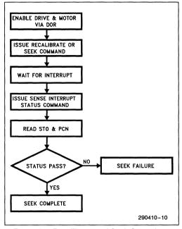
Figure 9-4. Recalibrate and Seek Operations
