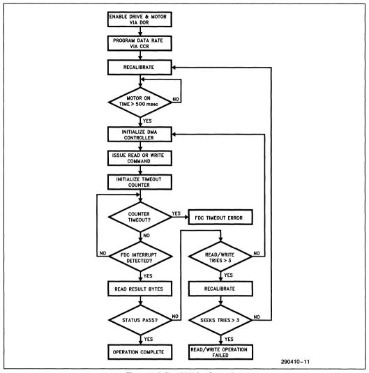
Figure 9-5. Read/Write Operation
