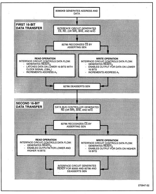
Figure 52. Operational Flow Diagram for 82786 Interface Circuit
