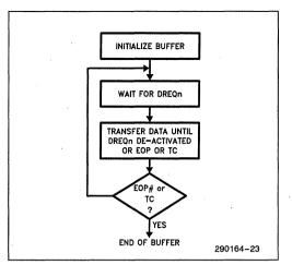
Figure 3-8. Buffer Transfer in Demand Transfer Mode
