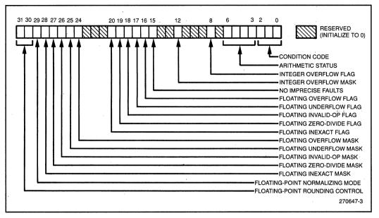
Figure 3. Arithmetic Controls
