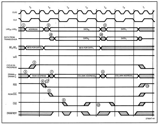
Figure 42. Timing Diagram for Two-word DRAM Write Transaction
