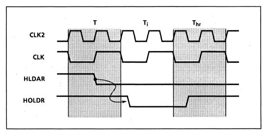
Figure 21. Forced Relinquishment Timing Diagram for an SMB
