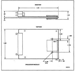
Figure 1: Processor Module
