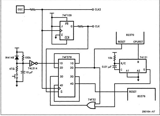
Figure 4-2. Interrupt Bank Block Diagram
