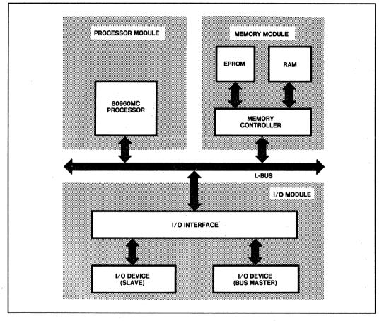
Figure 3. Basic 80960MC System Configuration
