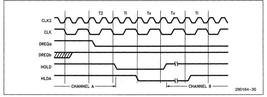
Figure 3-17. Switching between Active DMA Channels
