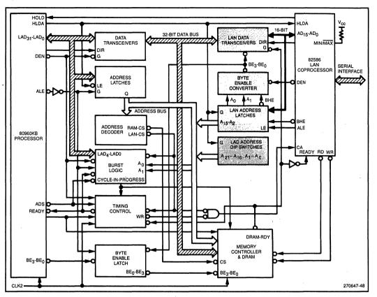
Figure 48. Block Diagram for LAN Controller
