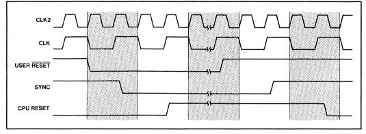
Figure 29. Diagram for RESET Timing Generation
