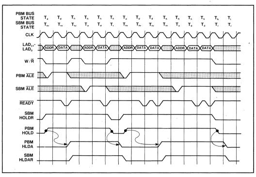
Figure 20. Example of a Bus Exchange Transaction
