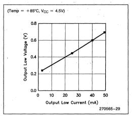
Figure 9. Worst Case Voltage vs Output Current on Open-Drain Pins
