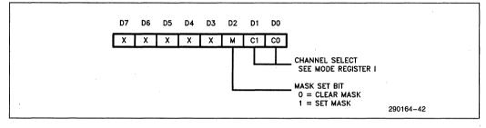
Mask Read/Write Register Group Channel Mask (read/write)
