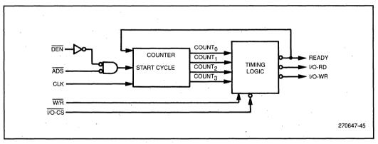
Figure 44. Timing Control Block Diagram
