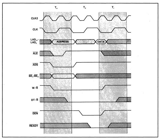
Figure 8. 80960MC Processor Read Transaction
