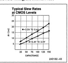
Figure 6.9. CMOS Level Slew Rates for Output Buffers
