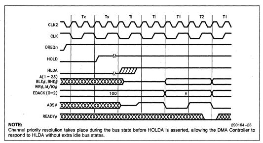
Figure 3-15. Beginning of a DMA process
