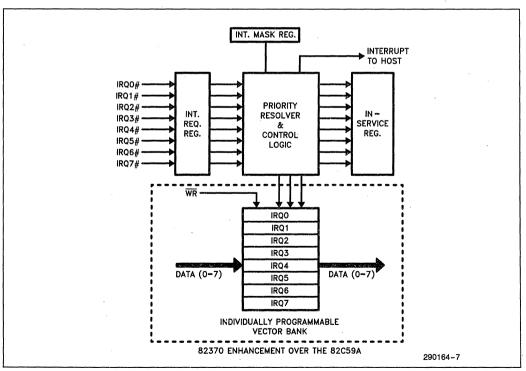
Figure 1-4. 82370 Interrupt Controller-Block Diagram
