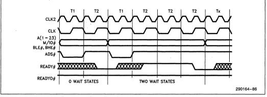
Figure 6-6. Early Termination of Bus Cycle By 'READY #'
