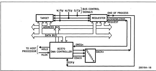
Figure 3-3. Requester, Target and DMA Controller Interconnection
