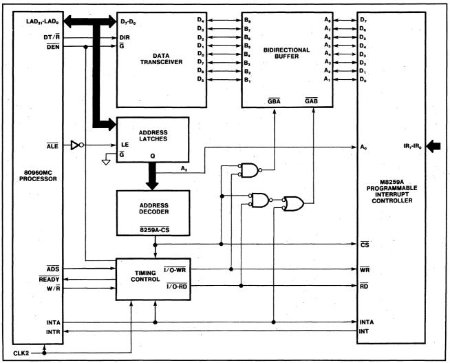
Figure 45. Block Diagram for M8259A Interface
