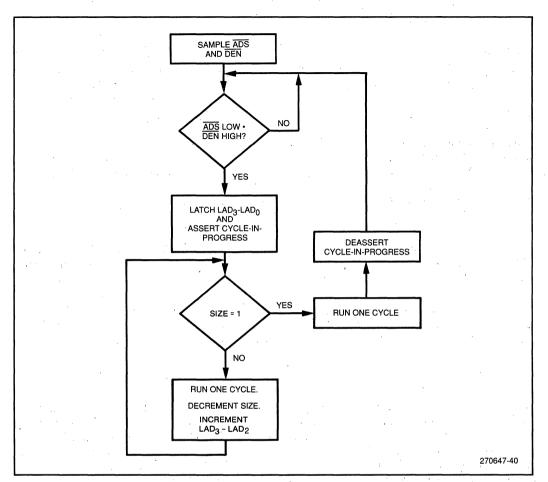
Figure 34. Burst Logic Flow Chart
