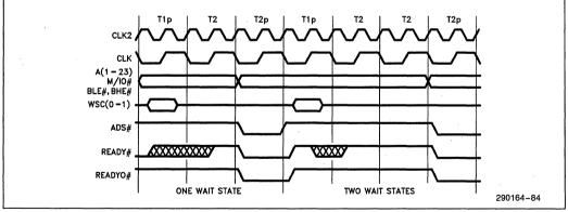
Figure 6-4. Wait States in Pipelined Cycles
