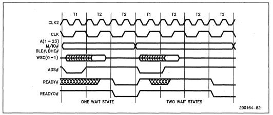
Figure 6-2. Wait States in Non-Pipelined Cycles
