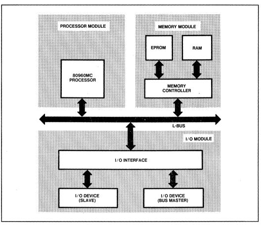
Figure 1. Basic 80960MC System Configuration
