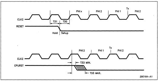
Figure 13-5. Reset Timing
