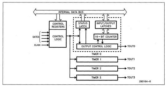
Figure 1-3. Programmable Interval Timers—Block Diagram
