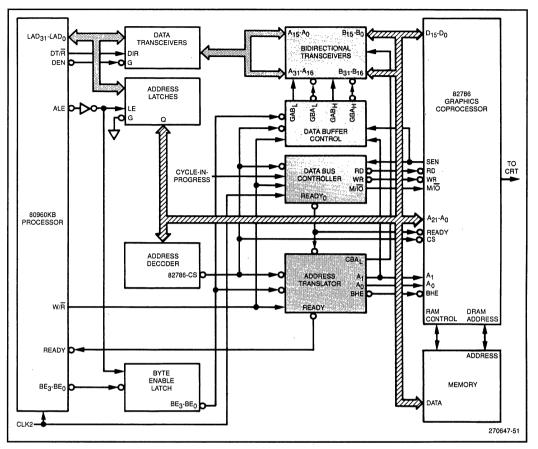
Figure 51. Block Diagram for 82786 Interface
