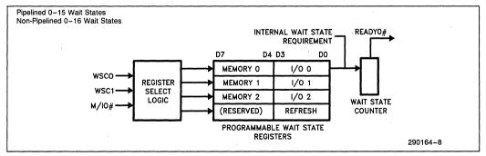
Figure 1-5. 82370 Wait State Generator—Block Diagram
