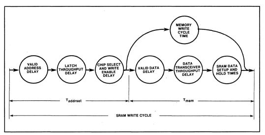
Figure 38. Critical Timing Path for SRAM Write Transaction
