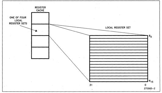
Figure 4. Multiple Register Sets Are Stored On-Chip
