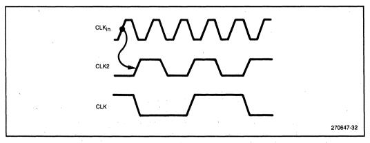
Figure 14. Clock Timing Waveforms
