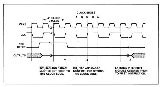
Figure 32. RESET Signal Timing Relationship
