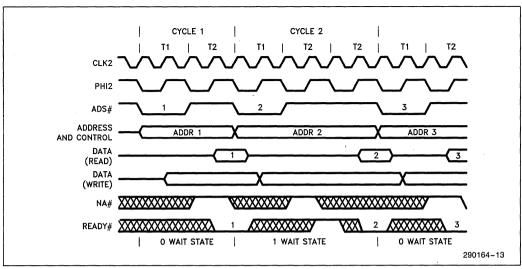
Figure 2-6. Non-Pipelined Bus Cycles
