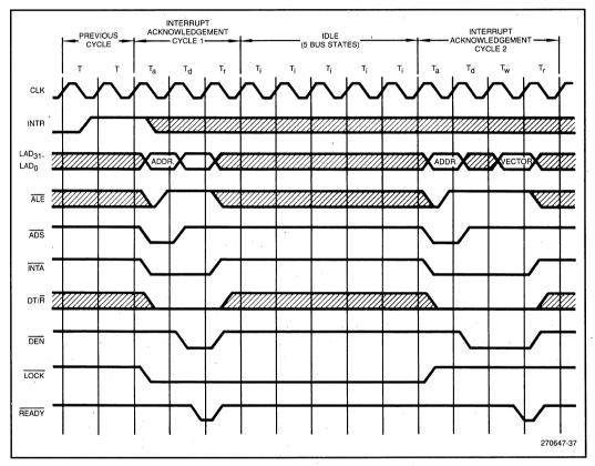
Figure 26. Timing Diagram for Interrupt Acknowledge Transaction
