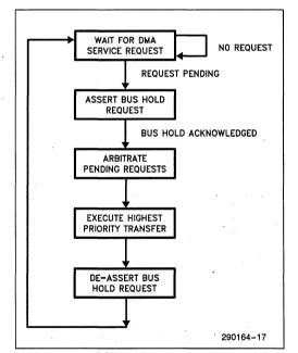
Figure 3-2. Flow of DMA Controller Operation
