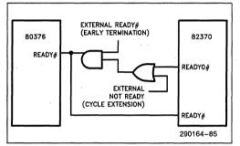
Figure 6-5. External 'READY' Control Logic
