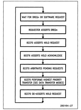
Figure 3-14. Bus Arbitration and DMA Sequence
