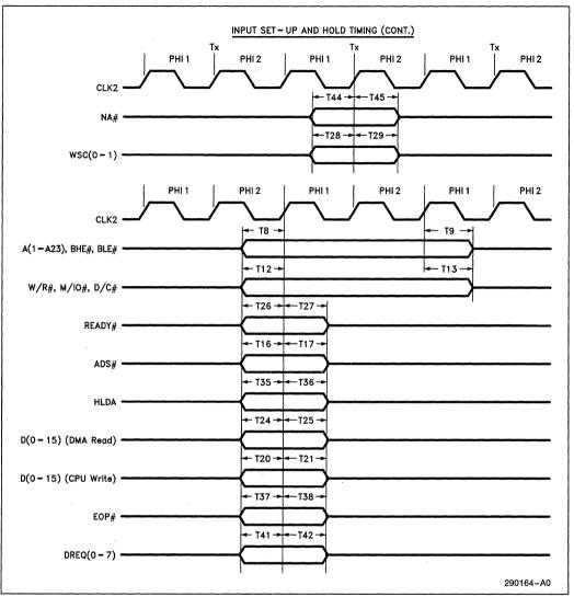
Figure 13-4. Input Setup and Hold Timing
