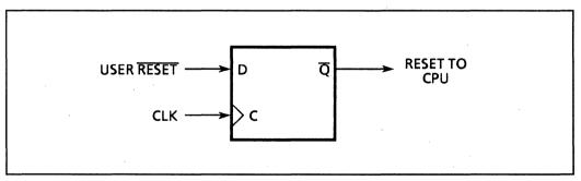
Figure 30. Synchronous RESET Circuit
