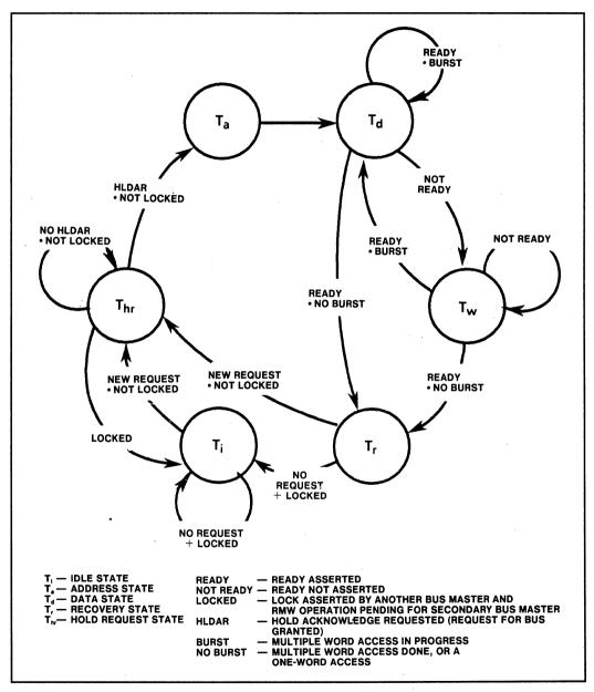
Figure 18. L-Bus States For Secondary Bus Master
