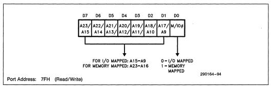
Figure 8-1. Relocation Register
