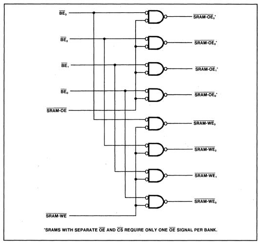
Figure 36. Logic Diagram for SRAM Interface
