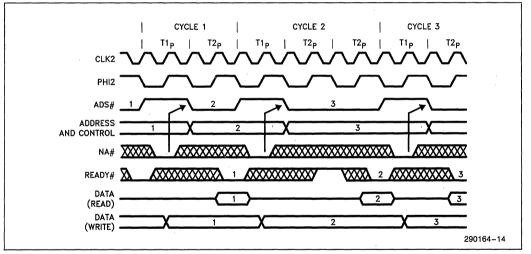
Figure 2-7. Pipelined Bus Cycles
