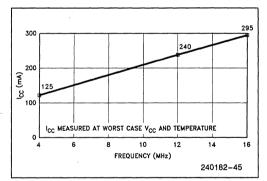
Figure 6.11. Typical I<sub>CC</sub> vs Frequency
