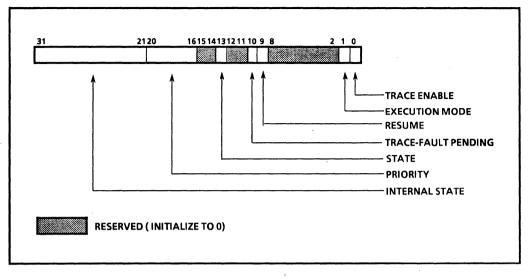
Figure A-4: Process Controls (Chapter 7)
