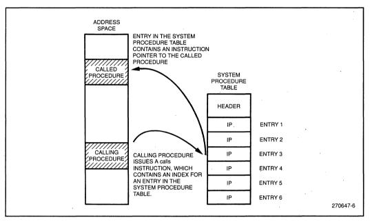
Figure 6. System Call Mechanism
