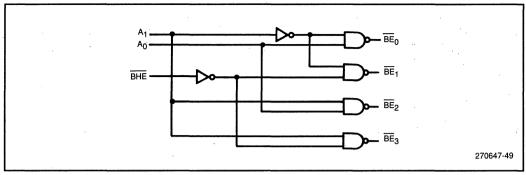
Figure 49. Byte Enable Generation Circuit
