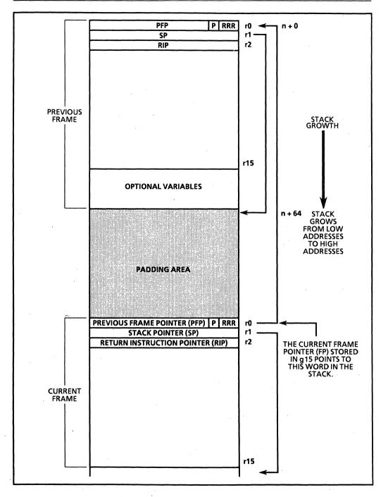
Figure A-3: Procedure Stack Structure (Chapter 4)
