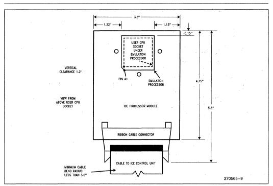
Figure 18. ICE-960KB Lateral Clearance Requirements
