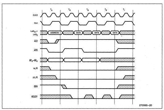
Figure 28. Burst Read Transaction
