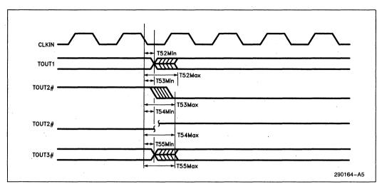
Figure 13-9. Timer Output Delays
