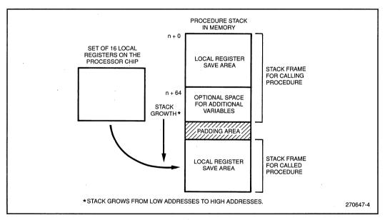
Figure 4. Local Registers and Procedure Stack
