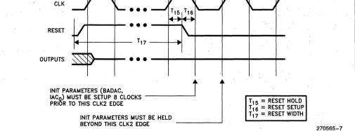
Figure 16. RESET Signal Timing
