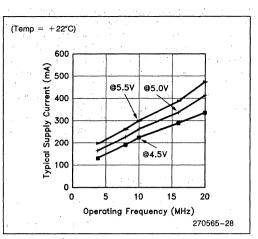
Figure 8. Typical Current vs Frequency
