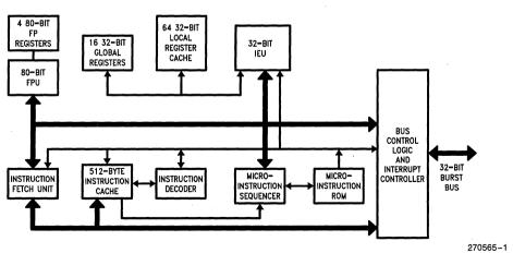
Figure 1. The 80960KB's Highly Parallel Microarchitecture
