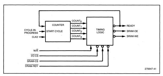
Figure 35. Timing Control Logic Block Diagram
