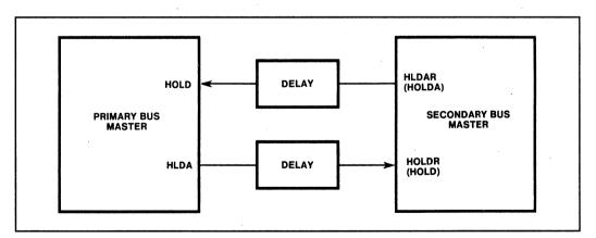
Figure 17. Arbitration Connection Between Two 80960MC Processors
