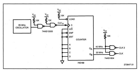
Figure 13. Clock Generation Circuit
