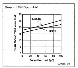
Figure 10. Capacitive Derating Curve
