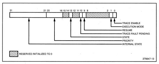
Figure 14. Process-Controls Word
