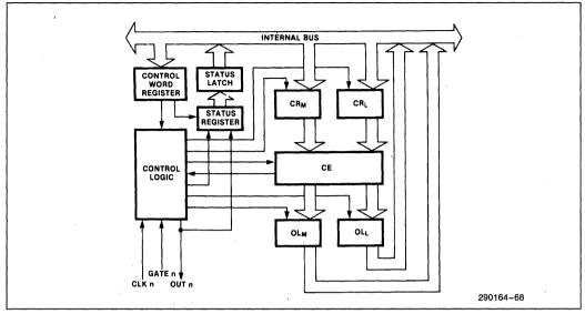
Figure 5-2. Internal Block Diagram of a Counter
