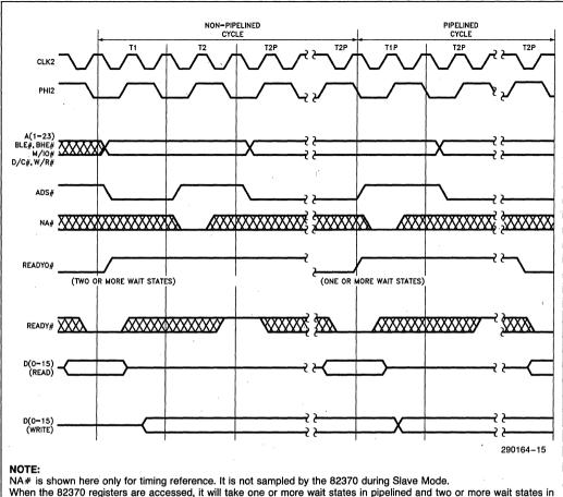
When the 82370 registers are accessed, it will take one or more wait states in non-pipelined cycle to complete the internal access.
