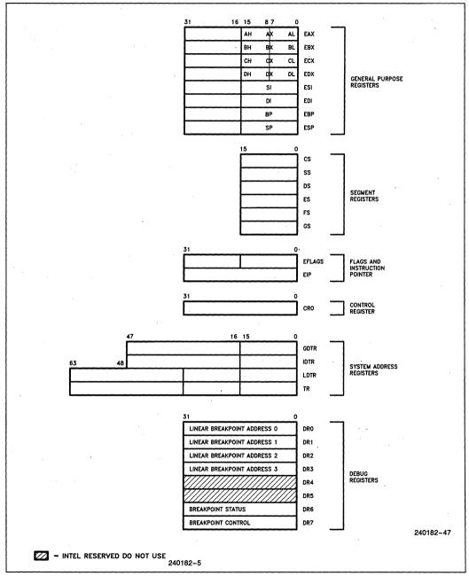
Figure 2.1. 80376 Base Architecture Registers
