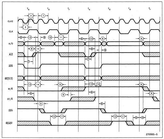
Figure 12. Timing Relationship of L-Bus Signals
