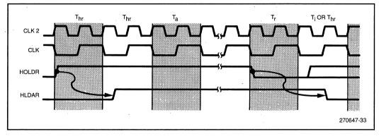
Figure 19. Arbitration Timing Diagram for an SBM
