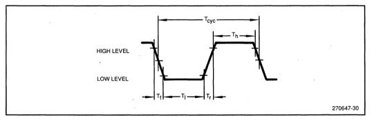
Figure 12. System Clock Pulse
