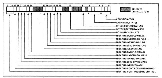
Figure A-1: Arithmetic Controls (Chapter 3)
