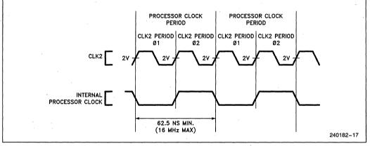
Figure 4.2. CLK2 Signal and Internal Processor Clock
