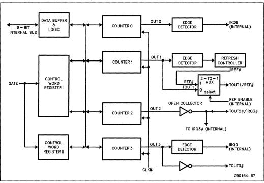
Figure 5-1. Block Diagram of Programmable Interval Timer
