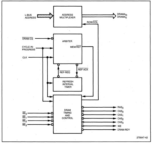
Figure 39. DRAM Controller Block Diagram
