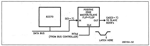
Figure 4-5. Slave Cascade Address Capturing
