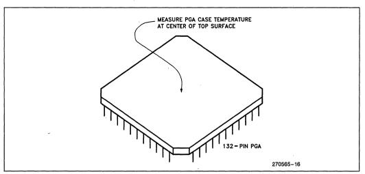
Figure 23. Measuring 80960KB PGA Case Temperature
