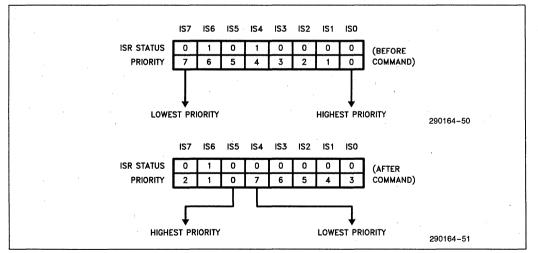
Figure 4-4. Rotate On Non-Specific EOI Command
