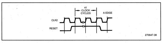
Figure 27. RESET Timing Diagram
