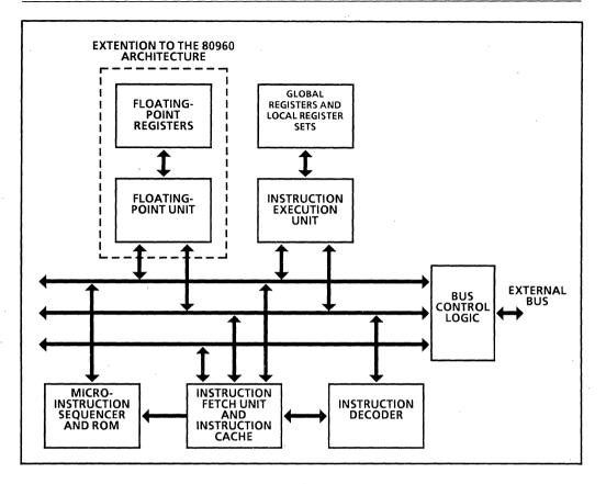
Figure C-1: Block Diagram of the 80960KB Processor
