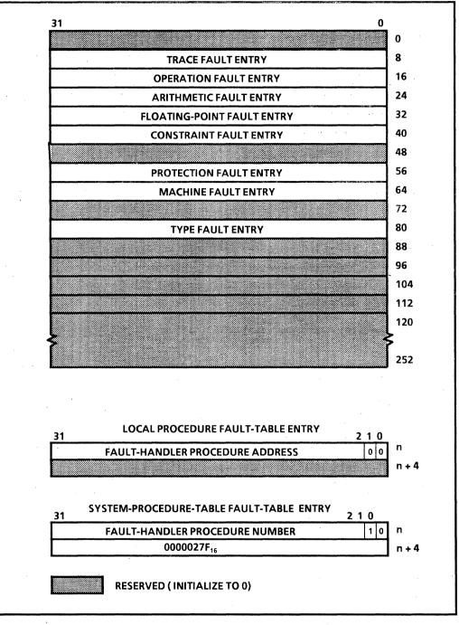
Figure A-10: Fault Table and Fault-Table Entries (Chapter 9)
