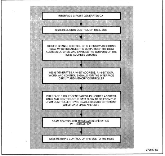
Figure 50. Operational Flow Diagram for 82586 Interface
