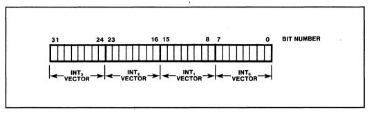
Figure 25. Interrupt Control Register
