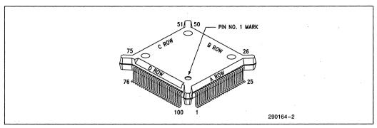
100 Pin Quad Flat-Pack Pin Out (Top View)
