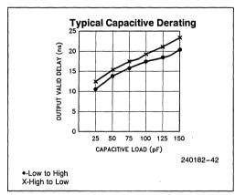
Figure 6.8. Capacitive Derating Curve
