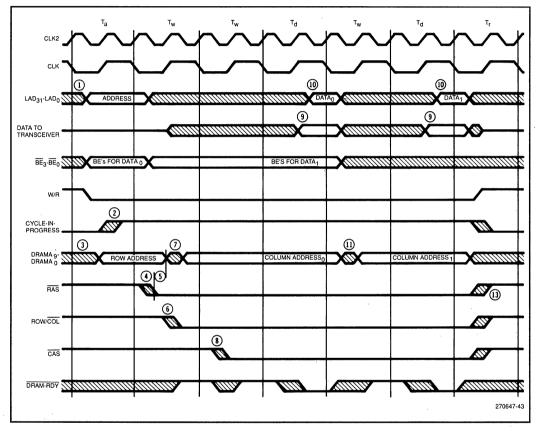
Figure 41. Timing Diagram for Two-word DRAM Read Transaction
