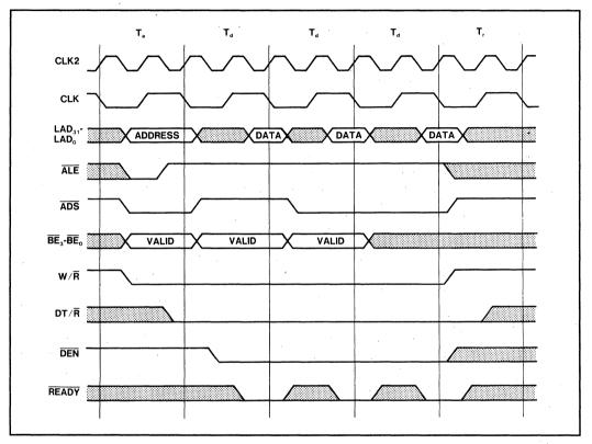
Figure 10. 80960MC Processor Burst Read Transaction
