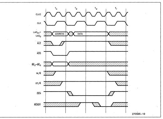
Figure 27. Write Transaction with One Wait State
