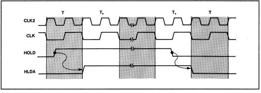
Figure 16. Arbitration Timing Diagram For A Bus Master
