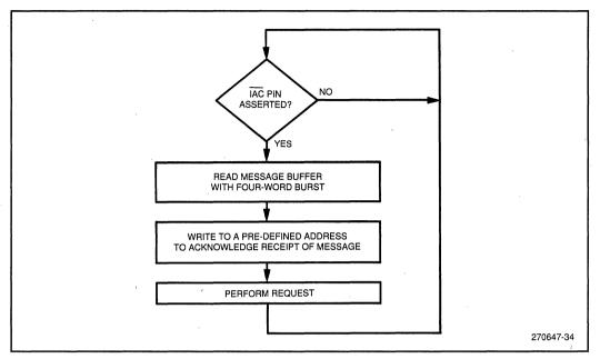
Figure 22. Example Flow Chart for an IAC Operation
