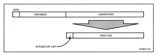
Figure 24. Binary Floating-Point Format
