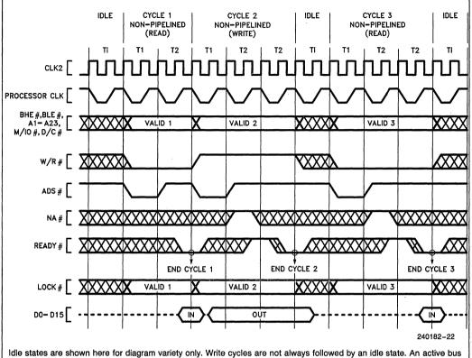
Idle states are shown here for diagram variety only. Write cycles are not always followed by an idle state. An active cycle can immediately follow the write cycle.
