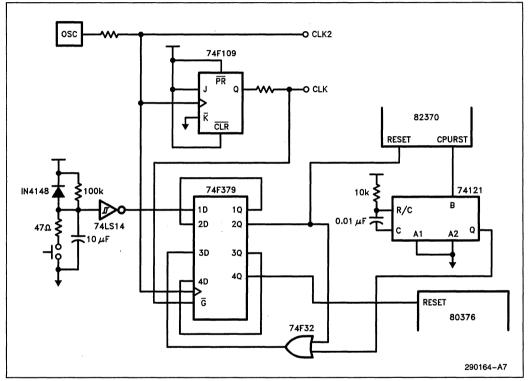
Figure D-1. Extending 82370 Reset Output
