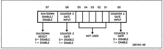
Figure 10-1. Internal Control Port
