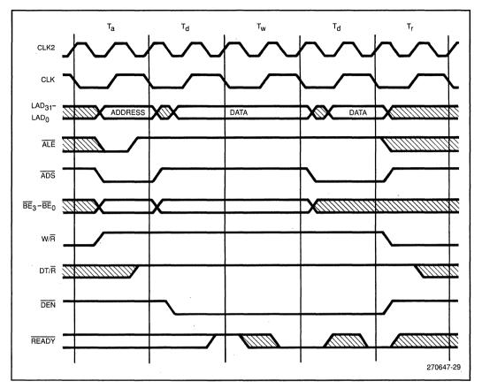
Figure 11. 80960KB Processor Burst Write Transaction
