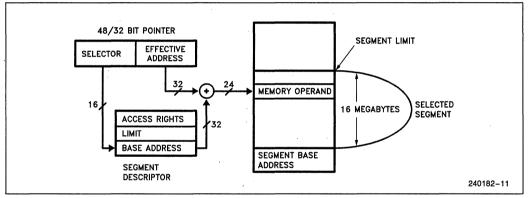
Figure 3.1. Address Calculation
