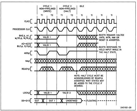
Figure 4.14. Example Halt Indication Cycle from Non-Pipelined Cycle
