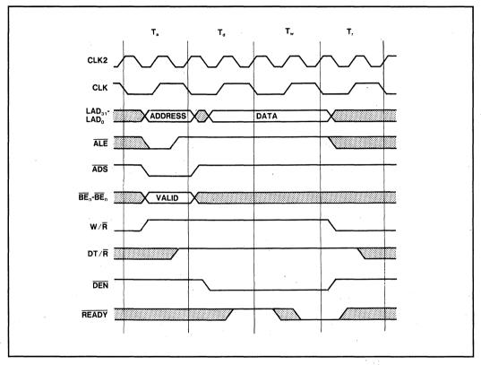
Figure 9. 80960MC Processor Write Transaction
