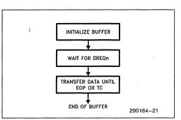
Figure 3-6. Buffer Transfer in Block Transfer Mode
