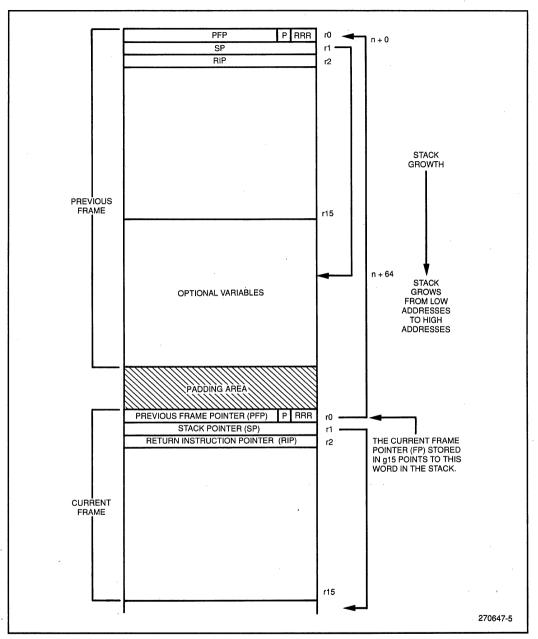
Figure 5. Procedure Stack Structure
