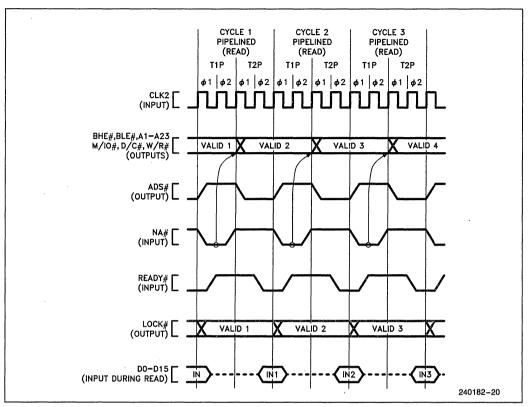
Figure 4.5. Fastest Read Cycles with Pipelined Timing
