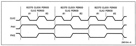
Figure 2-2. CLK2 and 82370 Internal Clock
