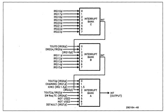
Figure 4-1. Interrupt Controller Block Diagram
