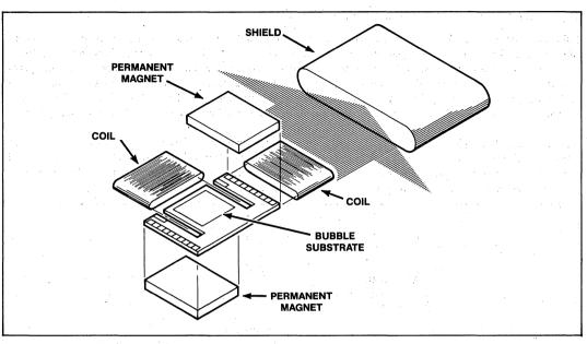
Figure 5. Magnetic Bubble Unit Assembly—Exploded View
