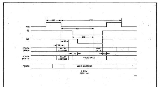
Figure 25. Asynchronous 8051 System Timing
