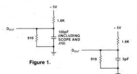
Figure 2. (FOR HIGH IMPEDANCE MEASUREMENTS ONLY)
