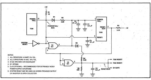
Figure 4. Recommended Power Fail Circuitry
