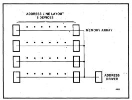
Figure 41. Recommended Address Line Routing
