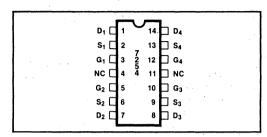
Figure 8. 7254 Pin Configuration
