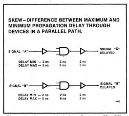
Figure 32. Skew — Variations Between Max/Min Propagation Delay
