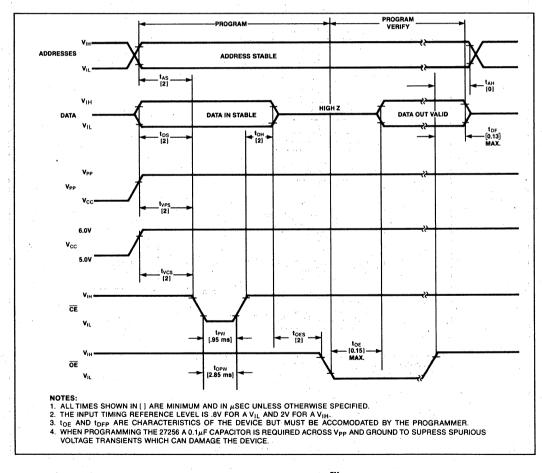
Figure 3. int<sub>e</sub>ligent Programming<sup>™</sup> Waveforms
