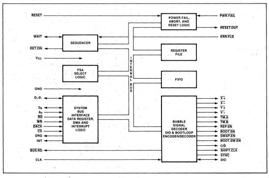
Figure 3. 7224 Bubble Memory Controller (BMC), Block Diagram
