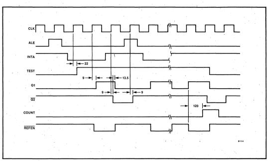
Figure 34. Burst Refresh Timing
