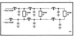
Figure 36. Equivalent Circuit for Distribution
