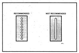
Figure 4. Recommended Voids for Multilayer PC Boards
