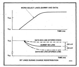
Figure 8. Sensing Voltage Waveforms
