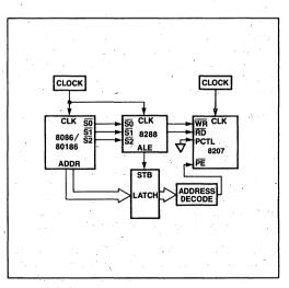
Slow-Cycle Asynchronous-Command Interface
