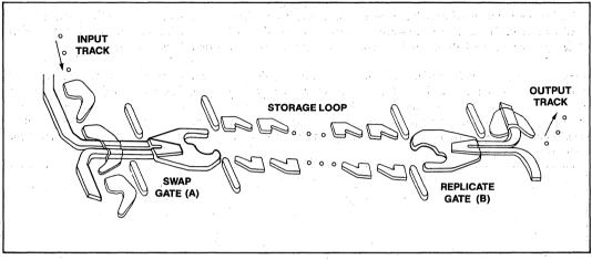
Figure 8. Swapping and Replication Configuration in Bubble Memory
