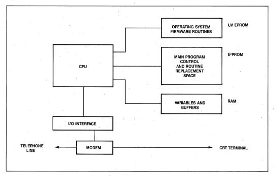
Figure 3. Partial Firmware Storage in E<sup>2</sup>PROM
