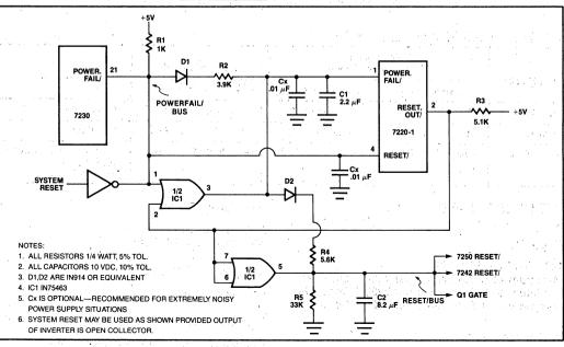
Figure 3. External Powerfail Circuit Solution
