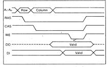
8. In all memory cycles, the row and column addresses are strobed to the RAMs by RAS and CAS. Sometime after the data out is valid, the control logic in Fig. 7b generates Write Enable (WE) to write the data back into the RAMs.
