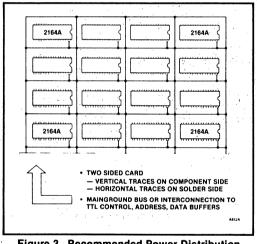
Figure 3. Recommended Power Distribution — Gridding
