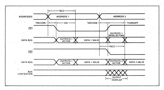
Figure 17. Single-Line Control and Bus Contention
