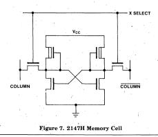
Figure 7 shows the standard six-transistor cell. Configured as a bi-stable flip-flop, the memory cell uses two transistors for loads and two for active devices so that the data is stored twice as true and compliment. The two remaining transistors enable data onto the internal I/O bus. Unlike the periphery, the cell is not powered down during deselect time to sustain data indefinitely.
