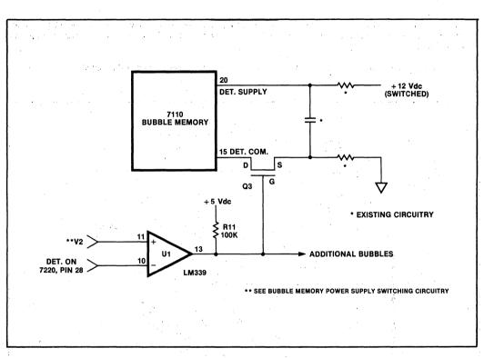
Figure 11. Bubble Memory Detector Power Supply Switching Circuitry
