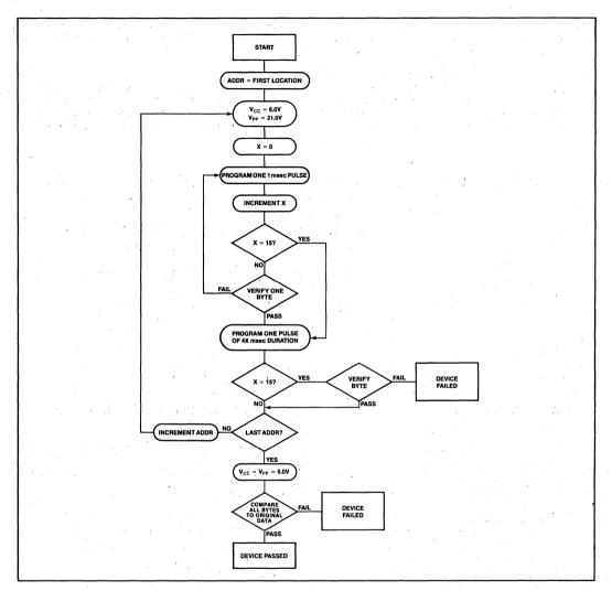
Figure 3. 2764 inteligent Programming<sup>™</sup> Flowchart
