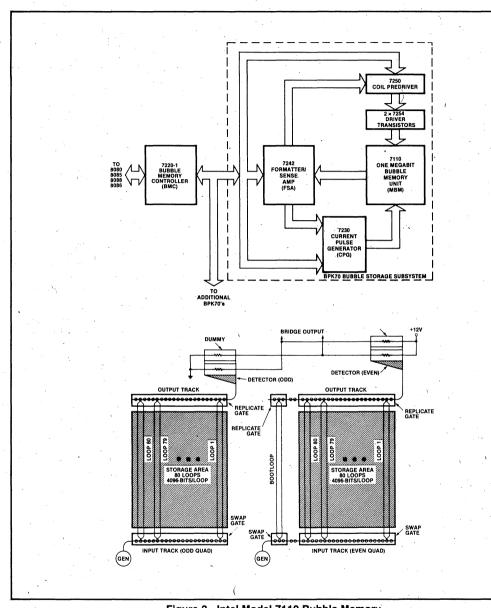
Figure 3. Intel Model 7110 Bubble Memory
