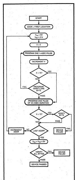
Intelligent programming algorithms, like the one for Intel's 27128 described by this flowchart, cut programming time by more than 80%.
