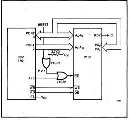
Figure 24. Asynchronous 8051 System
