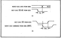
Fig 10 Required WE delay timing to memory
