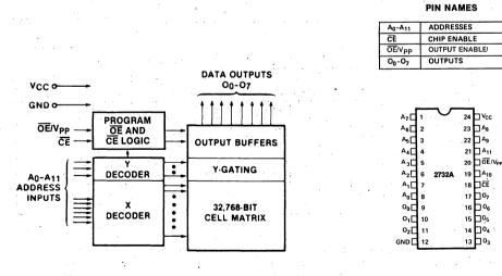
Figure 1. Block Diagram
