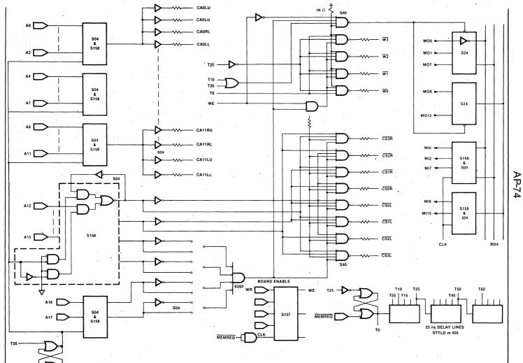
Figure 40. 16K X 16-Bit High Speed Static Memory
