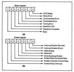
4. The status register bits (a) tell the host about any data errors, the state of the controller's readiness, or whether a command was completed properly or not. The register is updated every microsecond and indicates whether a data error was correctable or not, in addition to pointing out parity and timing errors. The enable register bits (b) specify several conditions, including interruption on an error, DMA enabling, and parity error interruption.
