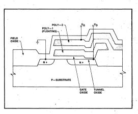
Figure 1. FLOTOX Device Structure Cross Section
