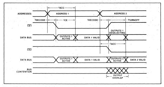
Figure 3. Single-Line Control and Bus Contention
