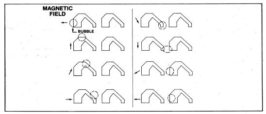
Figure 3. Bubble Propagation Under Asymmetric Chevrons
