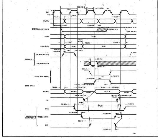
Figure 18. 8086 Bus Timing — Maximum Mode System (using 8288)
