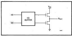
Figure 14. Simplified Output Buffer Circuit
