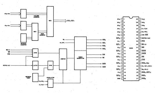
Figure 1. 8203 Block Diagram
