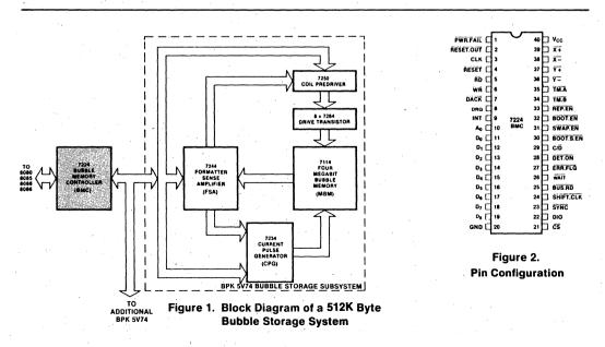
Intel Corporation Assumes No Responsibility for the Use of Any Circuitry Other Than Circuitry Embodied in an Intel Product. No Other Circuit Patent Licenses are Implied. © INTEL CORPORATION OCTOBER 1983 The BMC has an eight bit data bus plus parity bit. Word length expansion to 16 bit is possible by operating two controllers in parallel.
