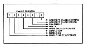
Figure 4. Enable Register Definition
