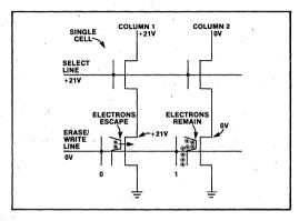
Figure 3b. Schematic of Memory Cell Operation During Write
