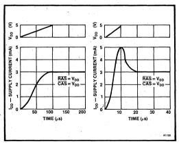
Figure 15. Typical I<sub>DD</sub> vs. V<sub>DD</sub> During Power Up
