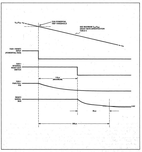
Figure 12. Power-down Timing (Revision 1)
