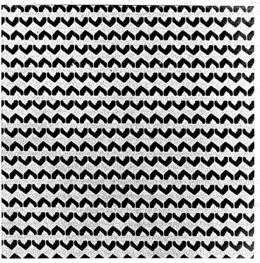
Photo 1. Asymmetric Chevrons Deposited on a Thin Film
