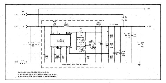
Figure 4. BPK 5V75 Voltage Regulator Circuit
