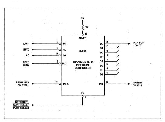
Figure 21. Interrupt Mode: 8259A in an 8088 System
