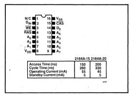
Figure 3. Intel® 2164A Pinout
