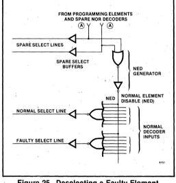
Figure 25. Deselecting a Faulty Element
