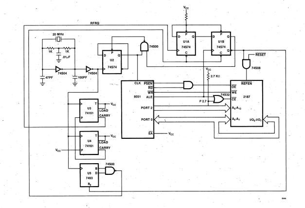
Figure 26. Synchronous 8051 System
