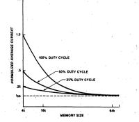
Figure 12. Average Current as a Function of Memory Size
