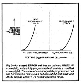
Finally, consider a device programmed for time  $t_2+T-t_0$ . In this case, charge added by the additional programming time T increases programming margin. The ZERO-to-ONE transition detected while increasing  $V_{CC}$  thus occurs when  $V_{CC}$  is greater than 5.25V, providing assurance of reliability.
