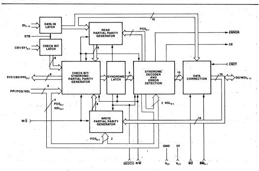
Figure 1. 8206 Block Diagram
