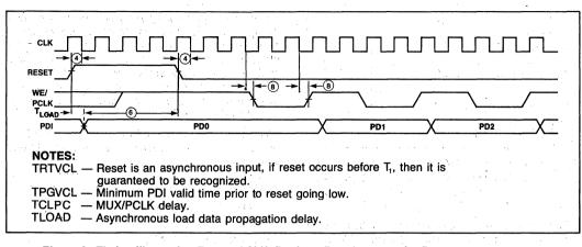
Figure 8. Timing Illustrating External Shift Register Requirements for Programming the 8207
