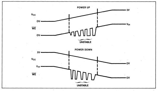
Figure 25. Typical TTL Driver Instability during V<sub>cc</sub> Power Transitions
