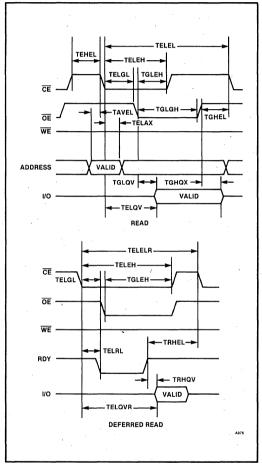
Figure 14. Read Cycle Timing
