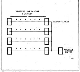
Figure 21. Recommended Address Line Routing
