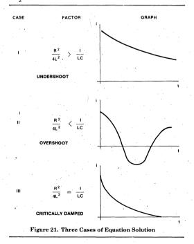
Dependent on the values of R, L and C, there are three cases shown in Figure 21. In case I, rise and fall times are excessively long. In case III, the current smoothly and clearly changes, while in case II, the current overshoots and rings. If ringing is severe enough, the voltage can cross the threshold voltage of the device as in Figure 22.
