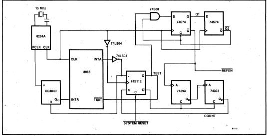
Figure 33. Burst Refresh Circuit
