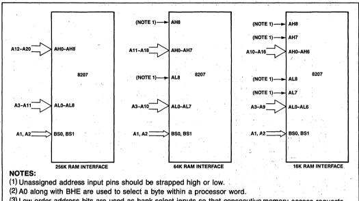
(3) Low order address bits are used as bank select inputs so that consecutive memory access requests are to alternate banks allowing bank interleaving of memory cycles.
