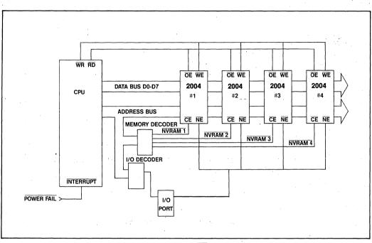
Figure 4. 2004 Array: Generating NE by I/O Output Port Bit
