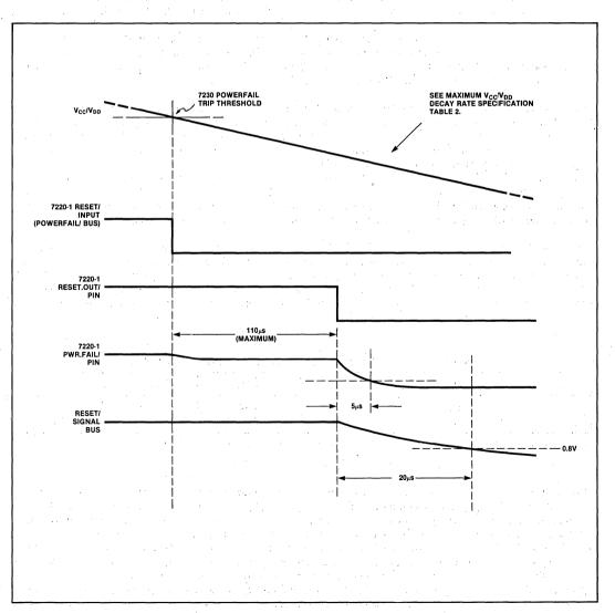
Figure 6. Power-down Timing for Powerfail Reset Circuit (Revision 2)
