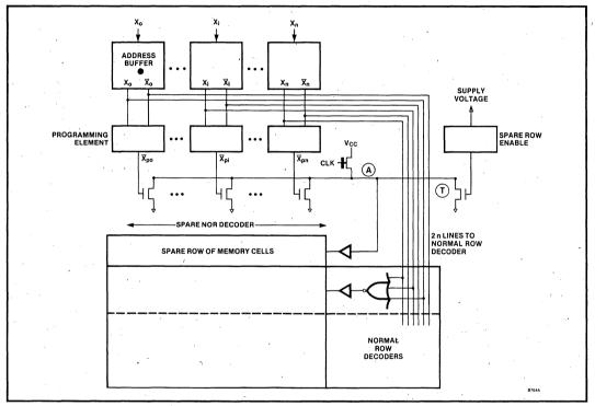
Figure 23. Block Diagram for a Spare Row
