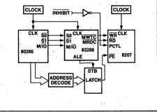
Fast-Cycle Asynchronous-Command Interface
