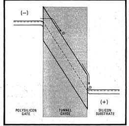
**2. Tunneling.** For a thin enough oxide, as shown here, under a field strength of  $10^7$  V/cm, Fowler-Nordheim tunneling predicts that a certain number of electrons will acquire enough energy to jump the forbidden gap and make it from the gate to the substrate.
