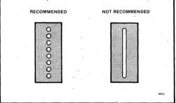
Figure 19. Recommended Voids for Multilayer PC Boards
