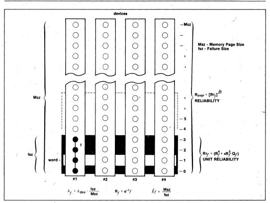
Figure 13. Single Failure Type Illustration
