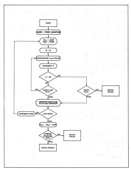
Figure 3. 2764A int<sub>e</sub>ligent Programming<sup>™</sup> Flowchart
