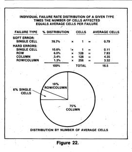
The illustration shows the statistical average cell failure for each type derived by taking the product of the component failure rate distribution times the number of cells affected. For the 2117 example device, the total average cell failure is 16.2 of which 11.8 are column and row failures.
