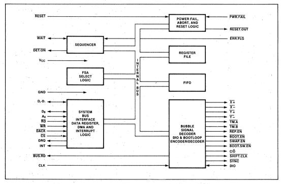
Figure 3. 7220 Bubble Memory Controller (BMC), Block Diagram
