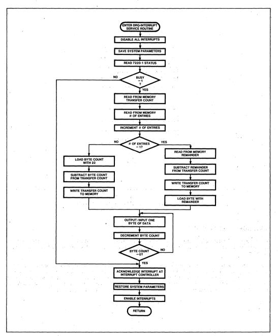
Figure 9. Interrupt-Driven Data Transfer Routine
