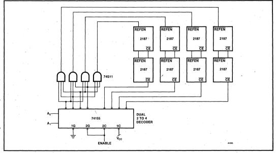
Figure 35. Synchronous Refresh Scheme
