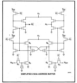
Figure 12. 2164A Simplified Address Buffer Circuitry
