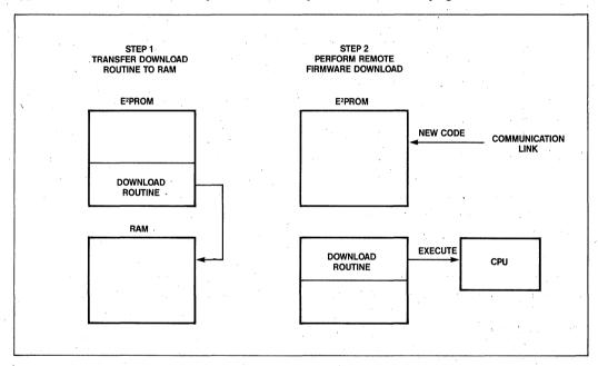
Figure 6. Remote Downloading to an E<sup>2</sup>PROM-only System with Download Routine in RAM
