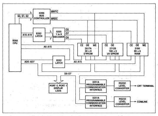
Figure 35. 2817A/8088 Applications Demo Board: Full Block Diagram
