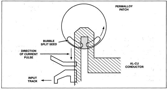
Figure 7. Seed Bubble and Bubble Generation
