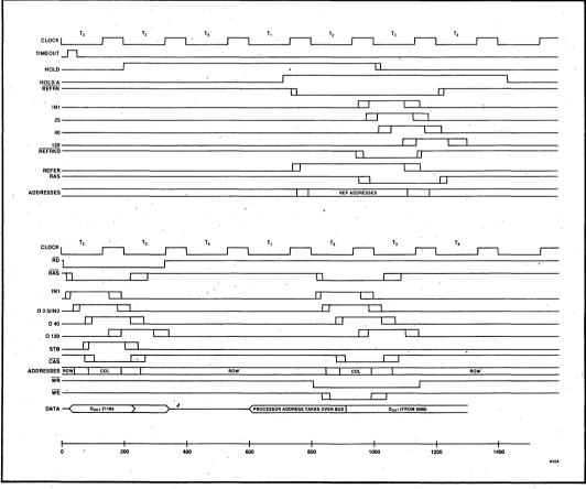
Figure 25. Timing Analysis Discrete Controller
