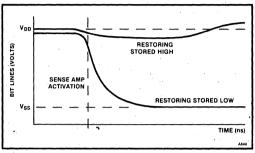
Figure 9. Bit/Sense Line Voltage
