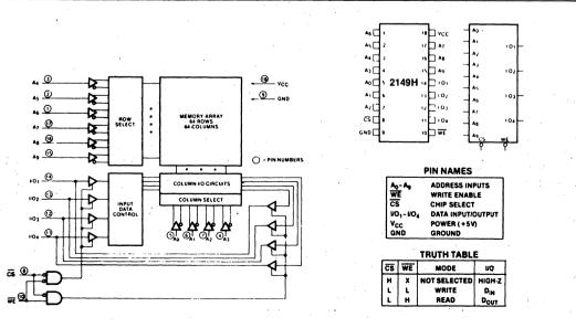
Figure 1. 2149H Block Diagram
