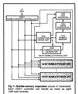
can control as many as eight bubble-memory modules, and with multiple BMCs, you can configure even larger systems (Fig 7). A memory module—providing expansion in increments of 128k bytes—consists of a 7110 bubble device, one 7230 current-pulse generator, one 7250 coil predriver, a 7242 formatter/sense amplifier and two 7254 drive-transistor packages.
