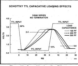
Figure 39. Capacitive Loading Effects
