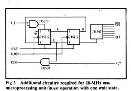
By adding a single AND gate to the 8086 interface (Fig 3) 2186 can be run in one wait state 10-MHz 8086 system. Upon going high, ALE causes the flipflop driving A to be set, forcing  $\overline{A}$  low. After a 1-gate delay, RDY1 is asserted. On the next falling edge of clock after ALE goes high, the flipflop driving A can now be reset on the next falling edge of clock, which occurs at the end of T2.
