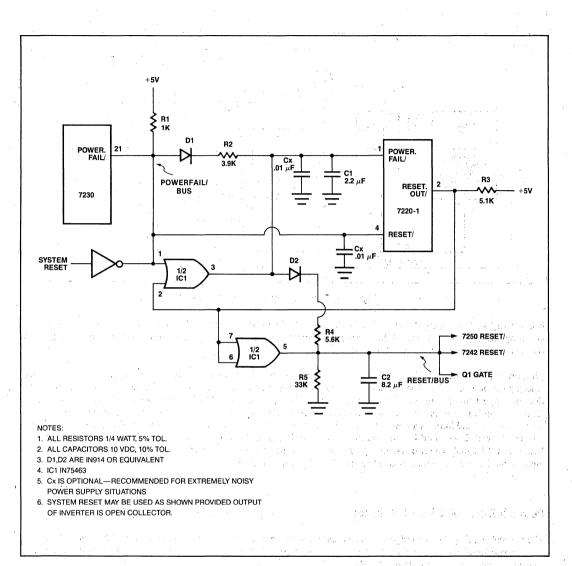
Figure 3. External Powerfail Circuit Solution
