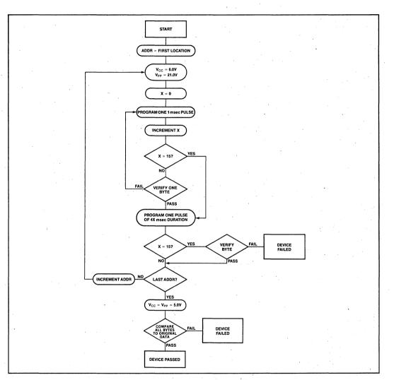
Figure 3. 27128 inteligent Programming<sup>™</sup> Flowchart
