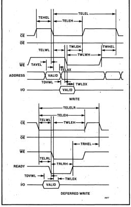
Figure 15. Write Cycle Timing
