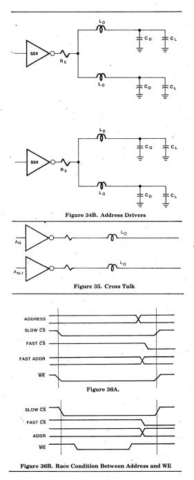
can sink 20 mA, inducing a transient in an adjacent trace. If the adjacent signal is switching to a one level, only  $400 \ \mu$ A of a source current from the driver is available. The induced current will generate a negative spike, driving the signal at a one leval negative. Additional time of 10 to 15 ns is required to recover and re-establish a stable one level. This may prevent stable address at the start of the cycle. Recall:
