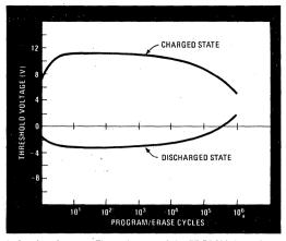
**4. Good endurance.** The endurance of the EE-PROM depends on the threshold-voltage difference between the charged and discharged states. Though repeated cycling degrades thresholds, the chip should stay within tolerable limits for  $10^4$  to  $10^6$  cycles.
