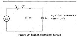
MOS RAM input is essentially capacitive. Simplifying the capacitance and writing the differential equation.
