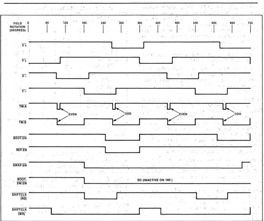
Figure 4. 7220 BMC Timing Diagram
