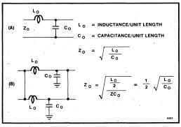
Figure 37. Transmission Line Characteristic Impedance
