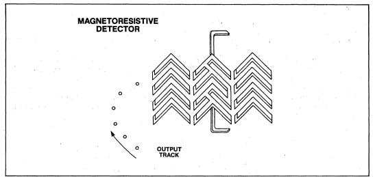
Figure 9. Bubble Detection
