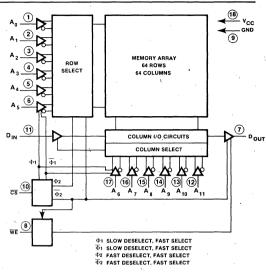
Figure 3. 2147H Block Diagram
