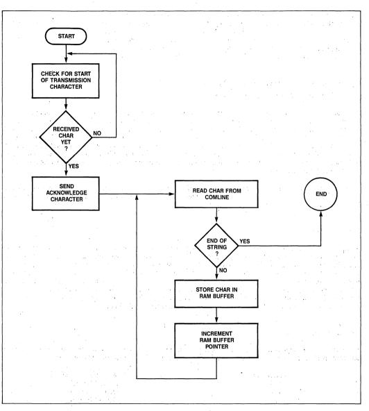
Figure 12. Data Transfer Software: Receiving System
