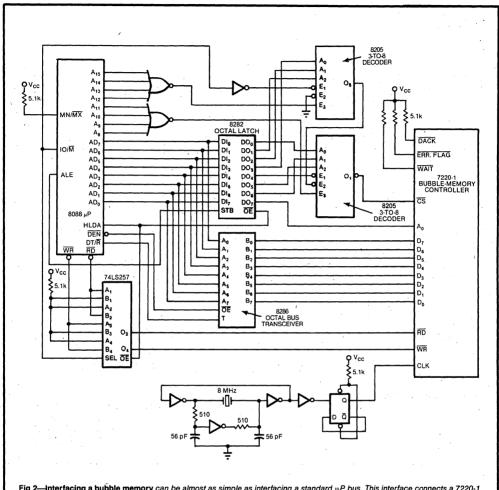
Fig 2—Interfacing a bubble memory can be almost as simple as interfacing a standard μP bus. This interface connects a 7220-1 bubble-memory controller with an 8088 μP.
