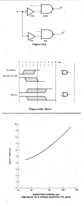
Figure 25. Capacitive Loading
