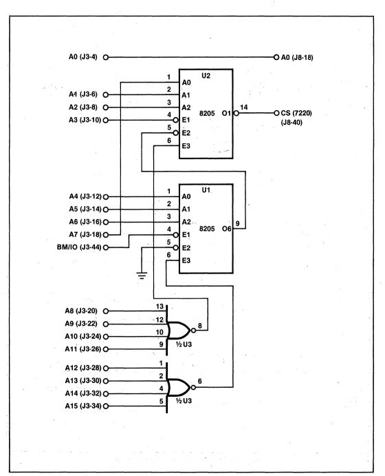
Figure 12. Address Decode Logic
