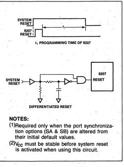
Figure 7. 8207 Differentiated Reset Circuit
