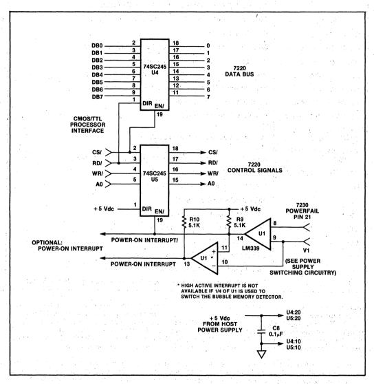
Figure 6. Bubble Memory Power Switch CMOS Bus Isolation Circuitry Polled Mode Only
