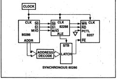
Fast-Cycle Synchronous-Command Interface
