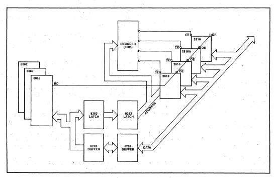
Figure 5. iAPX 86/2816A Read Architecture
