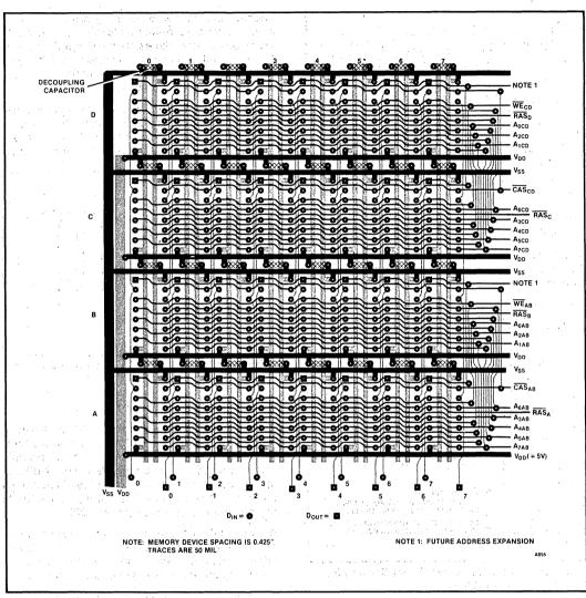
Figure 5. 2164A Memory Array PC Board Layout
