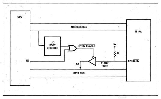
Figure 20. Polled Mode: Using an I/O Input Port to Poll the RDY/BUSY Output
