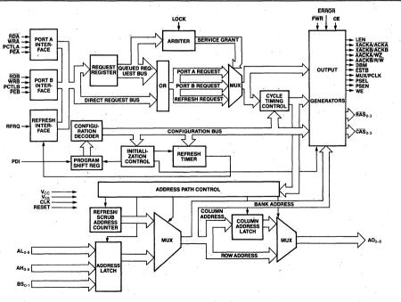
Figure 1. 8207 Block Diagram
