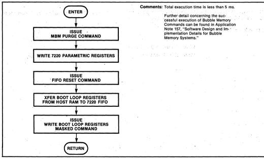
Figure 14. External Initialization Flowchart
