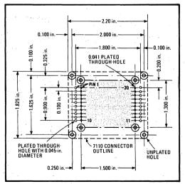
3. Four for one. If this pc board layout is followed, it is possible to plug either a socketed 7110, a leaded 4-Mb, or a leaded 1-Mb bubblememory package into this hole pattern. The socketed 7110 goes into the outer set of holes, while the newer packages fit the inner set.
