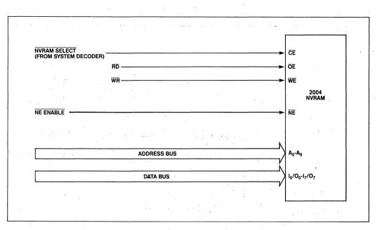
Figure 5. NVRAM System Interface
