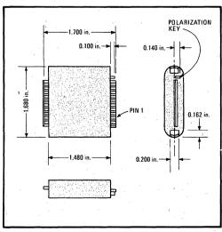
Leadless. The leadless package of this first-generation 1-megabit magnetic-bubble memory has a footprint of 2.20 by I.825 inches and an overall height of 0.430 in. when socketed. Thus boards cannot be spaced the standard 0.6 in. apart.
