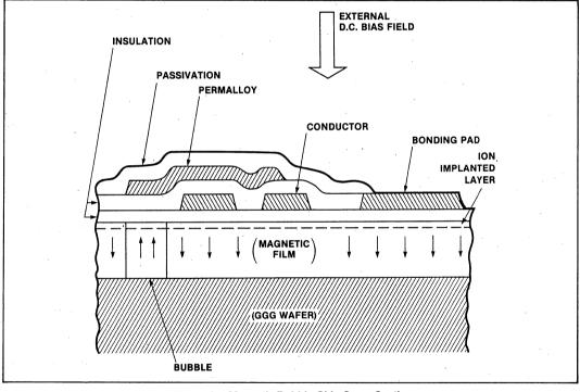
Figure 4. Magnetic Bubble Chip Cross Section
