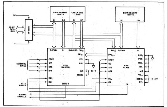
Figure 5. 32-Bit 8206 System Interface
