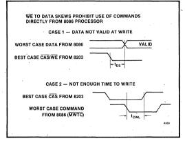
Figure 21. Write Cycle Problems
