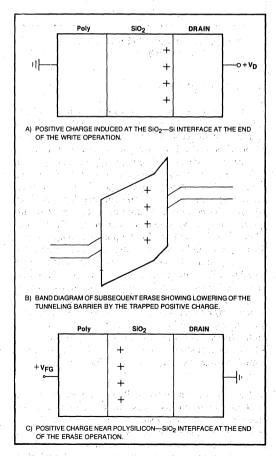
Figure 7. Threshold Window Widening
