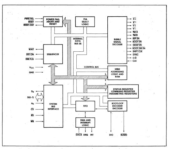
Figure 5. Block Diagram of the 7220 Bubble Memory Controller
