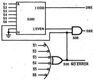
Figure 26. Double Error Decoder
