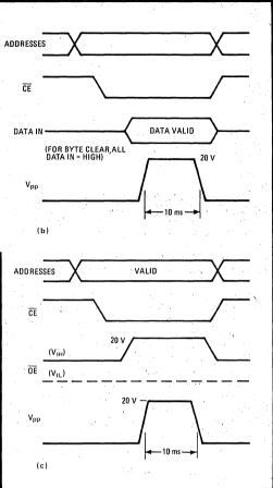
6. Timing. The Flotox memory's operating modes are shown for reading (a), writing or clearing of bytes (b), and chip clearing (c). Both writing and erasing require a 10-ms program-voltage pulse. The read mode is functionally identical to that of a 2716 E-PROM.
