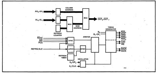
Figure 13. 8203 Dynamic RAM Controller Block Diagram
