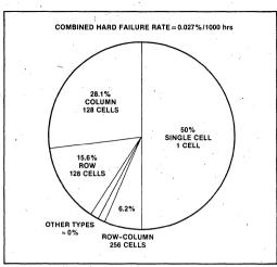
Figure 4. Failure Distribution — 2117 Example
