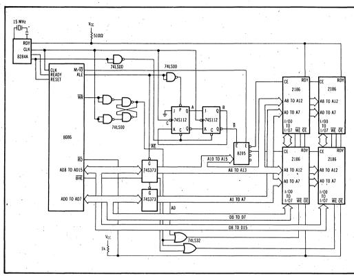
Fig 2 Schematic for iRAM use with 8086 microprocessing unit operation in minimum mode. NAND latch in processor's  $\overline{WR}$  line ensures adequate delay of data to iRAM as well as supplying trailing edge WR signal required by conventional SRAMS.
