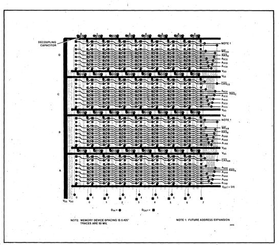
Figure 22. 2164A Memory Array PC Board Layout
