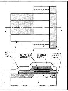
**1. Scaled.** Two-micrometer design rules squeeze the E-PROM cell down to 6 by 6  $\mu$ m. The active channel area, beneath the floating polysilicon gate, is just 1 by 1.2  $\mu$ m. The n<sup>+</sup> regions are 0.5  $\mu$ m deep.
