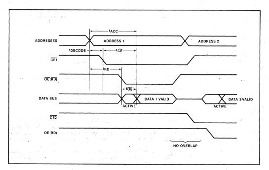
Figure 18. Two-Line Control Architecture
