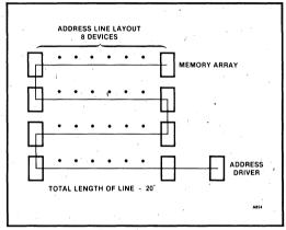
Figure 40. Unacceptable Address Line Routing (Serpentine)
