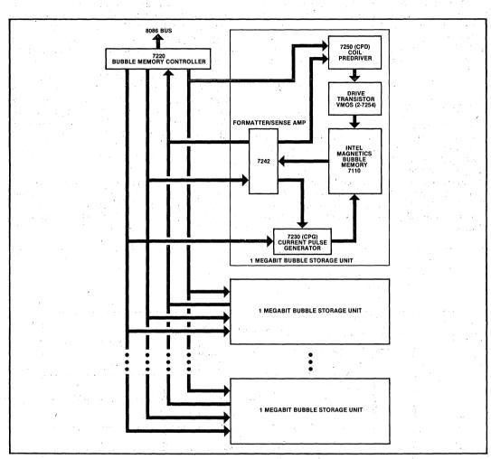
Figure 2. Bubble Memory System Expansion up to One Megabyte
