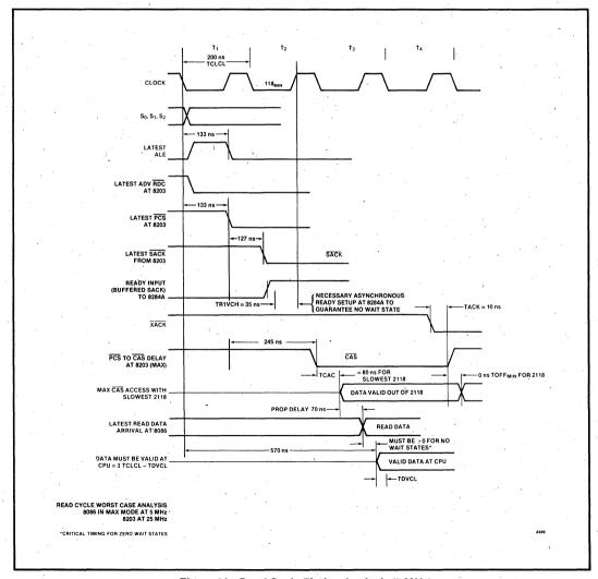
Figure 20. Read Cycle Timing Analysis (5 MHz)
