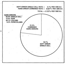
Figure 5. Combined Distribution of Failure Type
