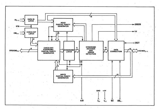
Figure 2. 8206-2 Block Diagram
