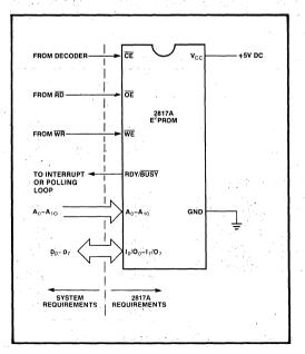
Figure 3. Simple 2817A Interface Requirements
