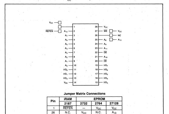
Figure 2. Universal Site Jumper Matrix — iRAM/EPROM Interchange
