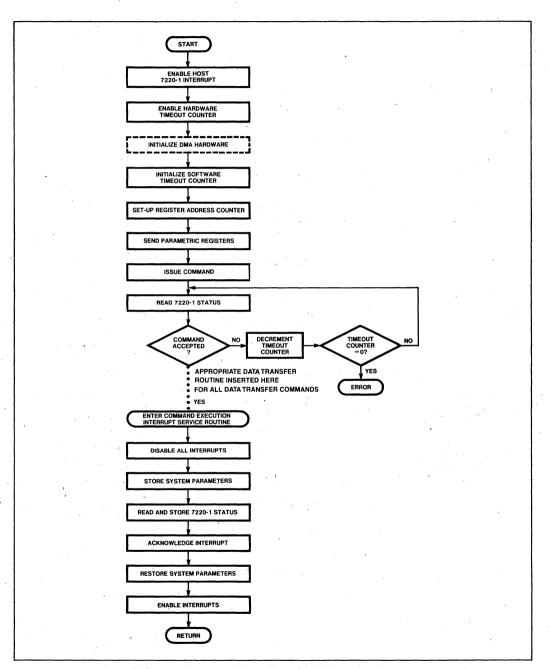
Figure 7. Interrupt-Driven Command Execution Routine
