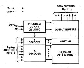
Figure 1. Block Diagram
