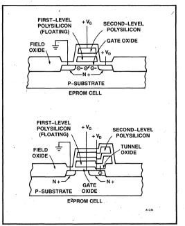
Figure 7. Double Poly Structure
