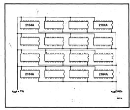
Figure 39. Unacceptable Power Distribution
