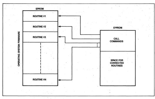
Figure 4. Firmware Patching: Operating System Memory Map
