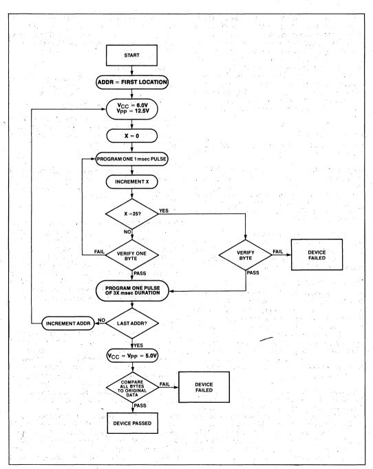
Figure 3. 27256 int<sub>e</sub>ligent Programming<sup>™</sup> Flowchart
