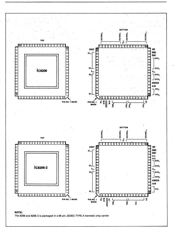
Figure 8. 8206 and 8206-2 Pinout Diagram
