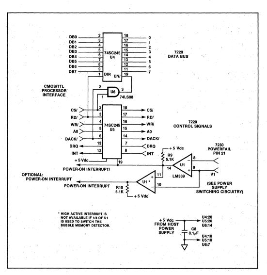
Figure 7. Bubble Memory Power Switch CMOS Bus Isolation Circuitry Polled/DMA Mode
