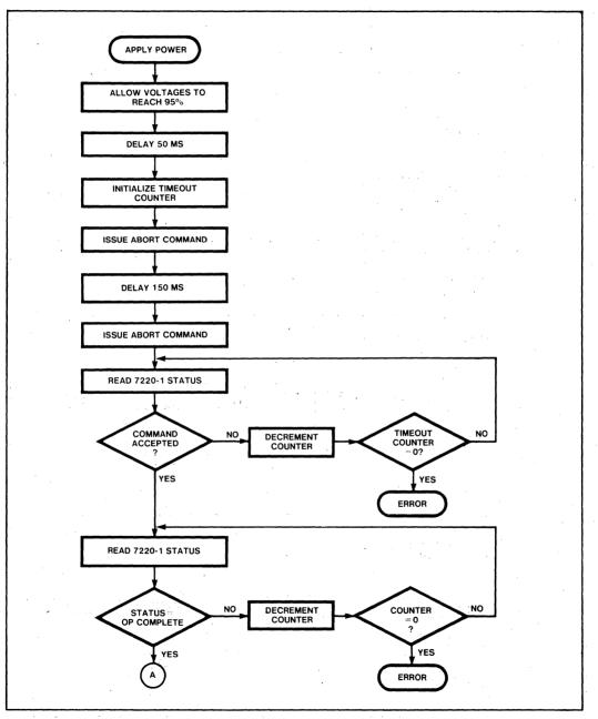
Figure 5. Power-Up Sequence (Polled Command Execution)
