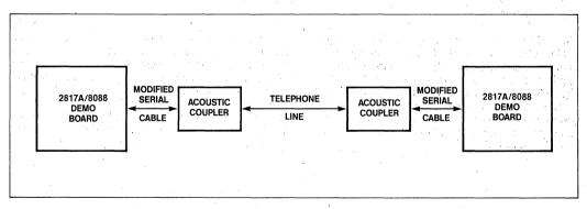
Figure 9. Remote Downloading over a Telephone Line using the 2817A/8088 Demo Board
