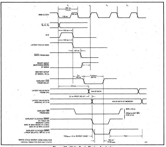
Figure 22. Write Cycle Timing Analysis
