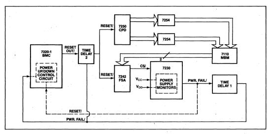
Figure 2. Block Diagram of Powerfail
