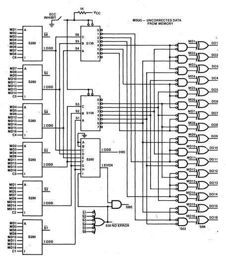
Figure 28. Complete Correction Circuit
