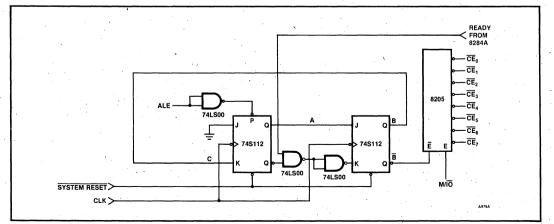
Figure 18. Interface Circuit No. 1
