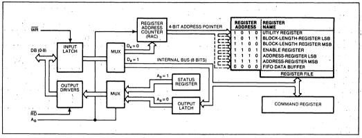
Figure 1. BMC Block Diagram
