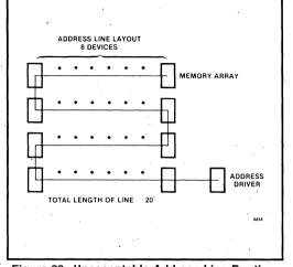
Figure 20. Unacceptable Address Line Routing (Serpentine)
