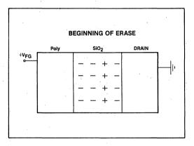
Figure 8. Negative Charges Trapped Uniformly Across Tunnel Oxide
