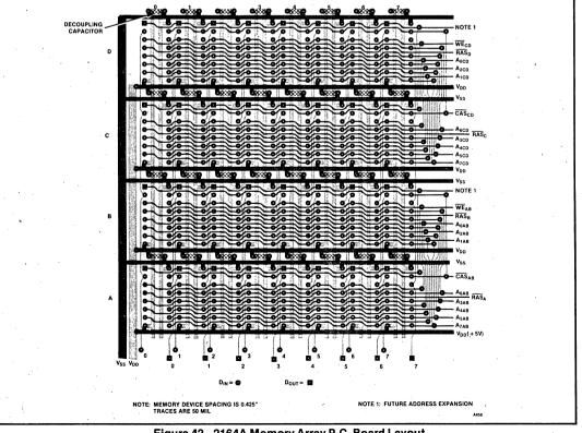
Figure 42. 2164A Memory Array P.C. Board Layout
