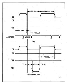
Figure 16. False Memory Cycle Timing
