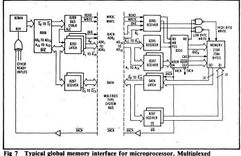
address/data bus serves as local bus and demultiplexed address/data bus serves as local bus. Minimum or maximum mode operation is possible.
