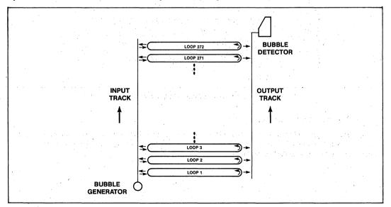
Figure 6. Block-Replicate Architecture
