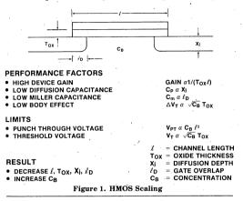
concentration. This has the additional advantage of balancing the threshold voltage which was decreased by scaling the oxide thickness for gain.
