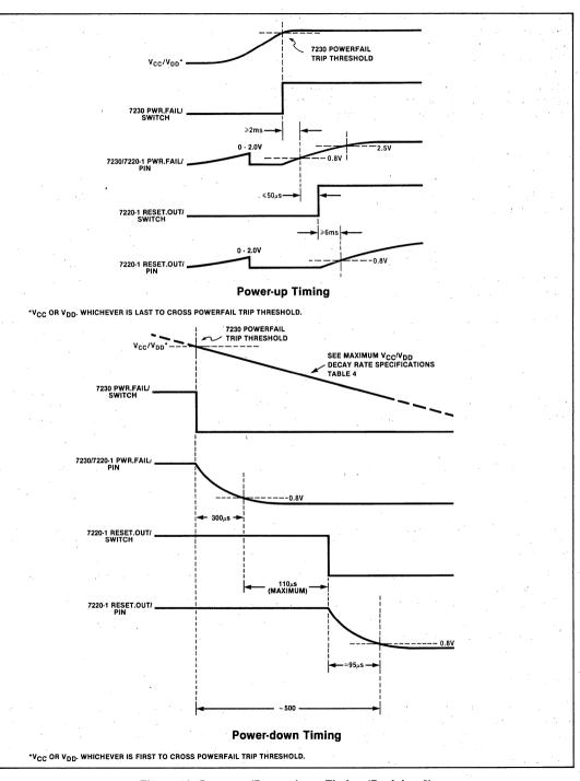
Figure 10. Power-up/Power-down Timing (Revision 0)
