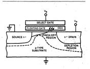
Information storage in an EPROM cell results from the transfer of charge to an MOS transistor's floating gate during the programming operation. the positive potential of the floating gate.
