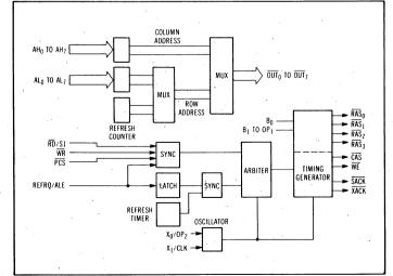
Fig 6 40-pin, 8203 DRAM controller includes arbiter that synchronizes refresh and memory cycle requests eliminating indecisive condition of Fig 5. Chip directly addresses 0.5M byte.
