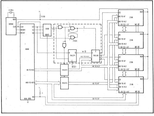
Fig 1 - Schematic for iRAM use with 8088 microprocessing unit running in maximum mode. To ensure proper startup, all iRAM control inputs must be inactive for 100  $\mu$ s after V<sub>CC</sub> reaches spec.
