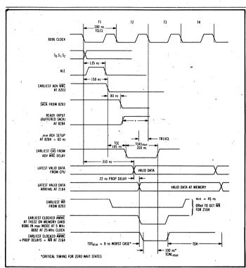
the 8203, WE falls a minimum of 8 ns after data are stable and valid at the memory. In addition, this ANDing guarantees a minimum  $t_{CWL}$  of 100 ns.
