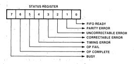
BUSY (when = 1) indicates that the BMC is in the process of executing a command. When equal to 0, BUSY indicates that the BMC is ready to receive a new command. In the case of Read Bubble Data, Read Bootloop, read Bootloop Register, or Read Corrected Data commands, BUSY may also indicate that the data has not been completely removed from the FIFO, and that DRQ is still active. BUSY will then drop as soon as DRQ does (after the user has finished reading the data remaining in the FIFO).
