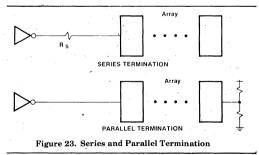
Series termination uses one resistor and consumes little power. Current through the resistor creates a voltage differential shifting the levels of input voltage to the devices slightly. This shift is usually insignificant because the 2147H has an extremely high input impedance.
