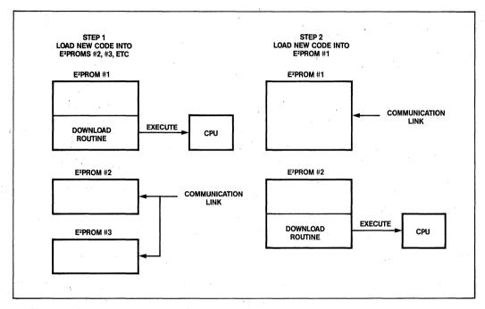
Figure 7. Remote Downloading to an E<sup>2</sup>PROM-only System with Downloading Routine in E<sup>2</sup>PROM
