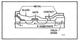
Figure 6. Completed Circuit (without passivation)
