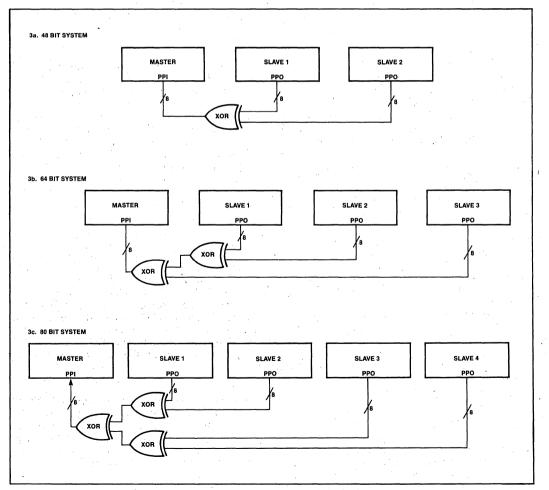
Figure 4. External Logic For Mult-Chip Systems
