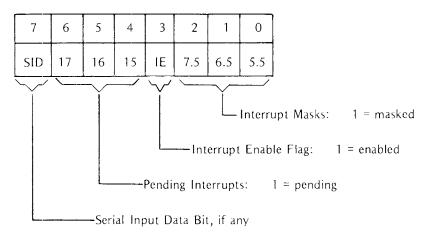
The mask and pending flags refer only to the RST5.5, RST6.5, and RST7.5 hardware interrupts. The IE flag refers to the entire interrupt system. Thus, the IE flag is identical in function and level to the INTE pin on the 8080. A 1 bit in this flag indicates that the entire interrupt system is enabled.
