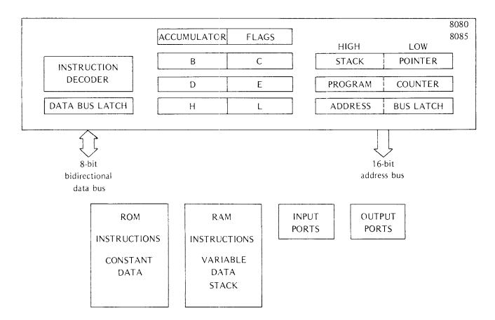
Figure 1-3. 8080/8085 Internal Registers
