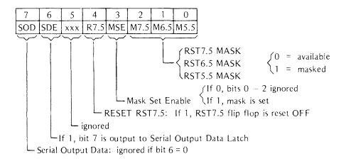
Accumulator bits 3 and 6 function as enable switches. If bit 3 is set ON (set to 1), the set mask function is enabled. Bits 0 through 2 then mask or leave available the corresponding RST interrupt. A 1 bit masks the interrupt making it unavailable; a 0 bit leaves the interrupt available. If bit 3 is set OFF (reset to 0), bits 0 through 2 have no effect. Use this option when you want to send a serial output bit without affecting the interrupt mask.
