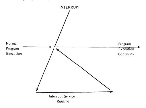
The 8080 contains a bit named INTE which may be set or reset by the instructions EI and DI described in Chapter 3. Whenever INTE is equal to 0, the entire interrupt handling system is disabled, and no interrupts will be accepted.
