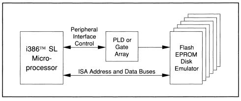
Figure 2-9. Dedicated Control Signals Simplify Flash EPROM Disk Emulator Systems
