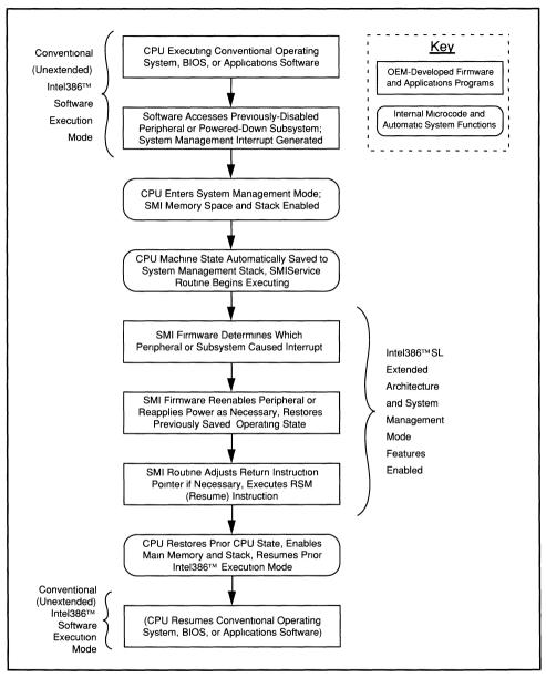
Figure 4-6. SMI Service Routine to Re-Enable Peripheral Power
