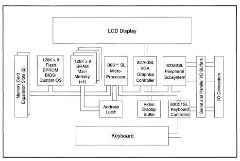
Figure 5-1. Ten-Chip Palm-Top PC Block Diagram
