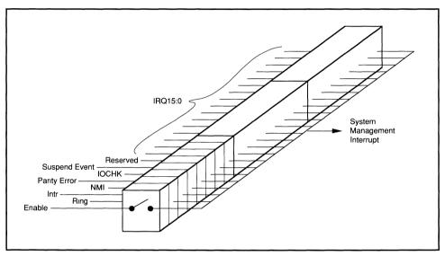
Figure 4-3. System Management Interrupt Requests and Mask Registers
