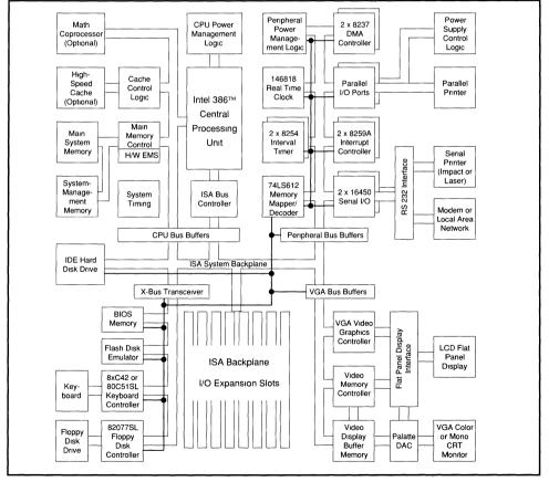
Figure 1-1. Industry-Standard PCs Contain a Common Set of System Functions and Peripherals
