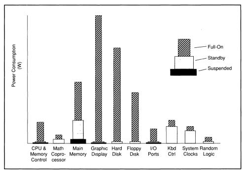
Figure 4-1. Lap-Top System Power Consumption Varies Greatly Depending on Operating Mode
