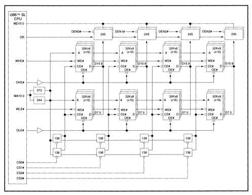
Figure 2-3. Typical Four-Bank, 4-Megabyte Buffered SRAM Memory Configuration
