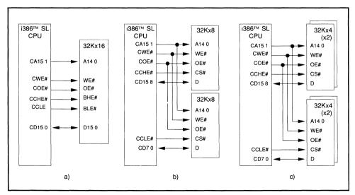
Figure 2-5. Optional High-Speed Caches Requires (a) One, (b) Two, or (c) Four External Chips
