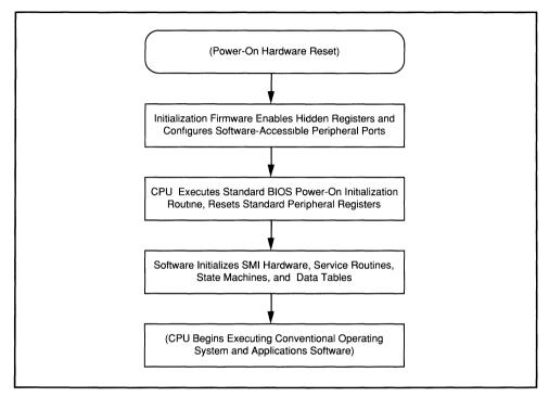
Figure 4-4. System Management Mode Initialization Sequence
