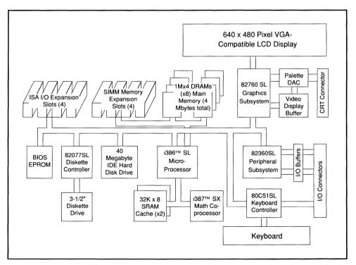
Figure 5-4. Lap-Top PC Block Diagram
