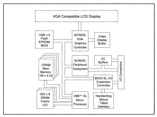
Figure 5-2. Note-Pad PC Block Diagram
