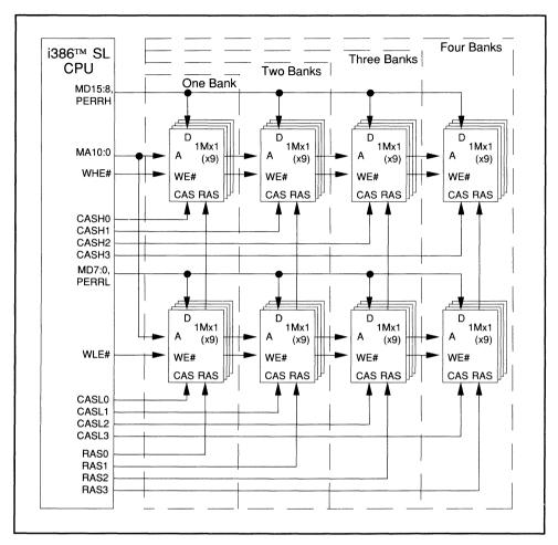
Figure 2-4. Four-Bank, 32-Megabyte Dynamic RAM Memory Configuration
