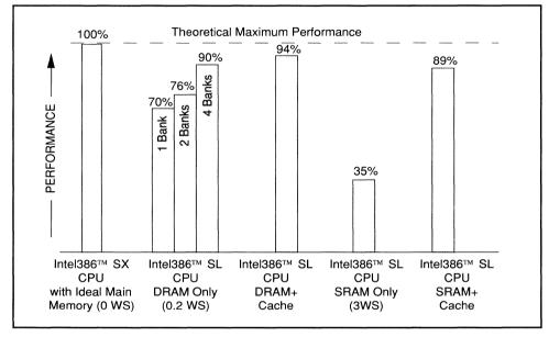
Figure 2-7. Adding Cache Memory Delivers Near-Ideal CPU Performance Levels
