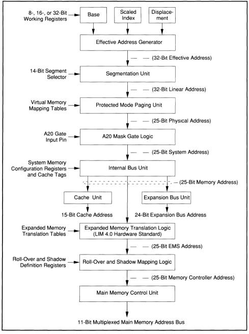
Figure 3-1. Intel386<sup>™</sup> SL Processor Memory Address Translation Logic Eliminates External Propagation Delays
