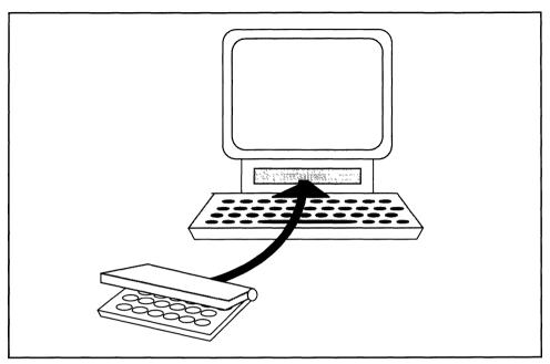
Figure 1-6. Stand-Alone Portable Module Acts as the Compute Engine of a Hybrid PC Design
