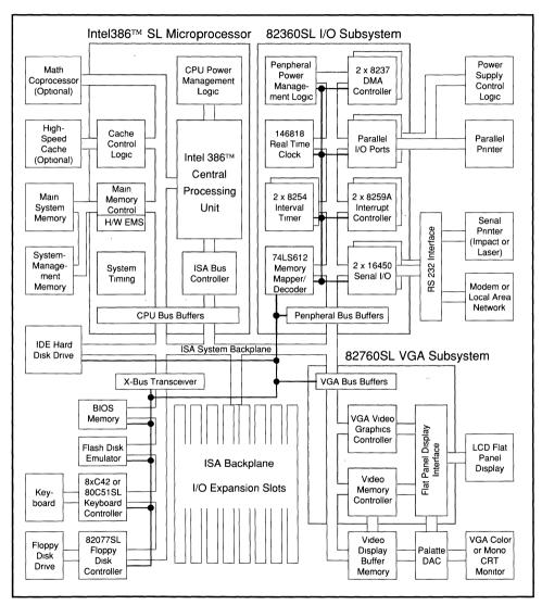
Figure 2-1. Intel 386<sup>™</sup> SL Microprocessor SuperSet Family Components Bring Together All Critical PC Functions
