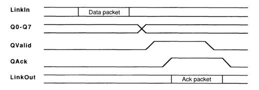
The link adaptor receives data from the serial link, presents it on **Q0-Q7**, and takes **QValid** high to commence the handshake. Receipt of the data is acknowledged on **QAck**, and the link adaptor then transmits an acknowledgement on the serial link. The link adaptor takes **QValid** low and the handshake is completed by taking **QAck** low.
