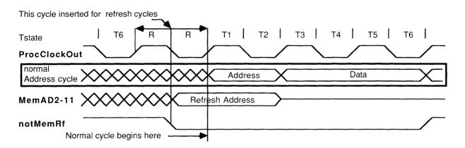
Refresh can be configured to be enabled or disabled. If Refresh is enabled, the interval between refresh cycles can be configured to be 18, 36, 54 or 72 periods of the input clock signal **ClockIn**.
