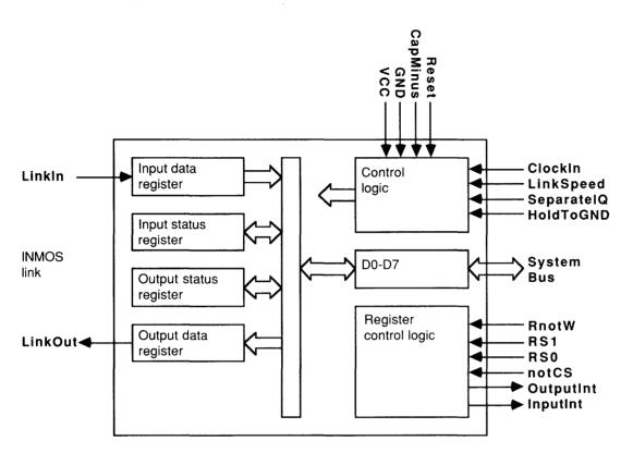
In mode 2 the link adaptor provides an interface between an INMOS serial link and a microprocessor system bus, via an 8-bit bi-directional interface.
