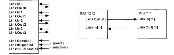
The T212 links wait until each full byte has been received before outputting the corresponding acknowledge packet. An acknowledge packet can be received at any time following the transmission of a data packet start bit.
