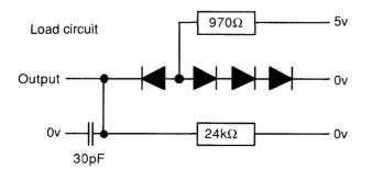
The load circuit approximates to two Schottky TTL loads, with total capacitance of 30 pF.
