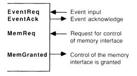
The two event signals, **EventReq** and **EventAck**, together provide a handshaken interface with an occam process executing in the processor.
