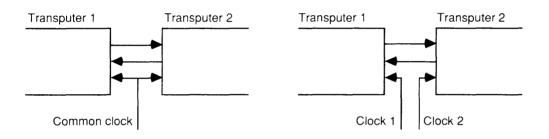
Link communication is not sensitive to clock phase. Thus, communication can be achieved between independently clocked systems as long as the communications frequency is the same.
