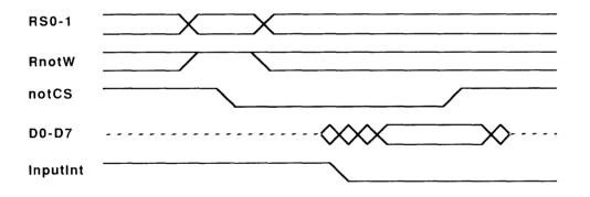
Write register timing diagram
