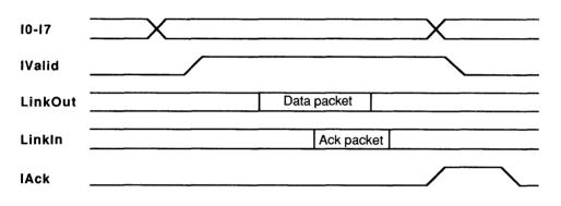
**IValid** and **IAck** provide a simple two wire handshake. Data is presented to the link adaptor on **I0-I7**, and **IValid** is taken high to commence the handshake. The link adaptor transmits the data through the serial link, and acknowledges receipt of the data on **IAck** when it has received the acknowledgment from the serial link. **IValid** is then taken low, and the link adaptor completes the handshake by taking **IAck** low.
