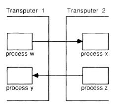
To provide synchonised communication, each message must be acknowledged. Consequently, a link requires at least one signal wire in each direction.
