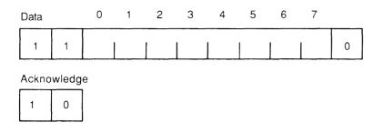
The links are designed to make the engineering of transputer systems straightforward. Board layout of two wire connections is easy to design and area efficient. All transputers will support a standard communications frequency of 10 Mbits/sec, regardless of processor performance. Thus transputers of different performance can be directly connected and future transputer systems will directly communicate with those of today.
