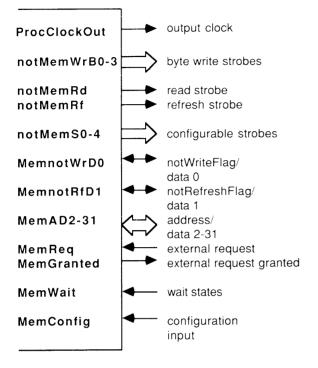
The memory interface uses a 32-bit wide multiplexed address/data bus and its controller may be configured, on reset, to suit a wide variety of different memory systems. One of 13 preset configurations may be selected or the configuration may be supplied externally.
