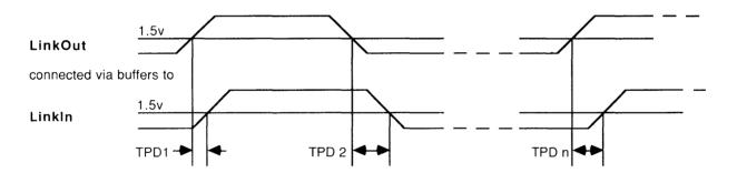
The absolute value of TPD is immaterial because data reception is asynchronous. However, TPD will vary from moment to moment because of ground noise, variation in the power supplies of buffers and the difference in the delay for rising and falling edges. This will vary the length of data bits reaching **LinkIn**. *Skew* is the difference between the maximum and minimum instantaneous values of TPD.
