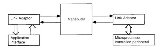
The third method is by memory mapping the peripheral onto the memory bus of a transputer. The peripheral is controlled by memory accesses issued as a result of **PORT** inputs and outputs. The application designer's peripheral device handler provides a standard occam channel interface to the rest of the application.
