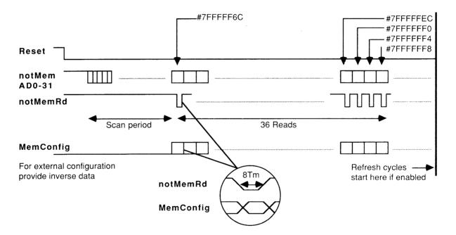
The following table gives, for each preset configuration, the **MemConfig** connection, the duration of each Tstate, the width of **notMemS1**, and the delay from the start of **T2** to the falling edge of **notMemS2-S4**. These times are all in periods **Tm**. The table also gives the number of periods of the input clock between refresh cycles, e.g. 72 periods of 200ns give a refresh interval of 14.4 microseconds.
