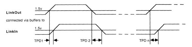
The absolute value of TPD is immaterial because data reception is asynchronous. However, TPD will vary from moment to moment because of ground noise, variation in the power supplies of buffers and the difference in the delay for rising and falling edges. This will vary the length of data bits reaching **LinkIn**. *Skew* is the difference between the maximum and minimum instantaneous values of TPD.
