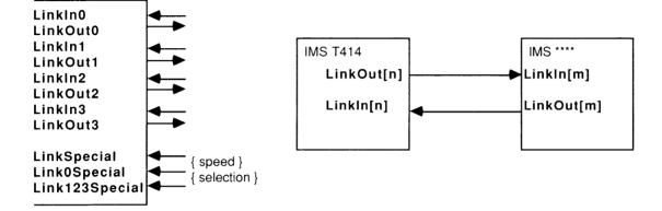
The T414 links wait until each full byte has been received before outputting the corresponding acknowledge packet. An acknowledge packet can be received at any time following the transmission of a data packet start bit.
