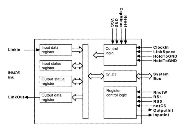
The C012 link adaptor provides an interface between an INMOS serial link and a microprocessor system bus, via an 8-bit bi-directional interface.
