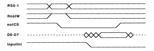
Write register timing diagram
