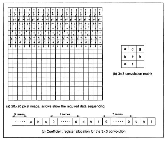
Figure 10.12 Improved version of the 3×3 image convolution/correlation with the IMS A100
