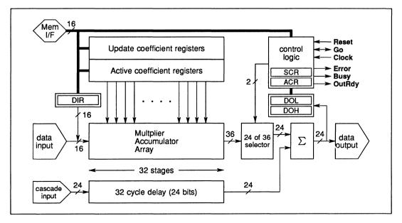
Figure 10.7 User's model of the IMS A100
