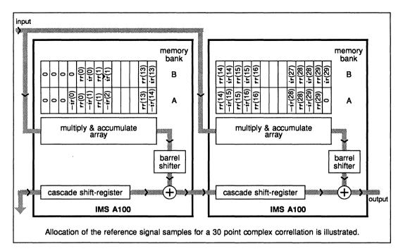
Figure 11.5 Cascading two IMS A100 devices to obtain a 31 point complex correlator
