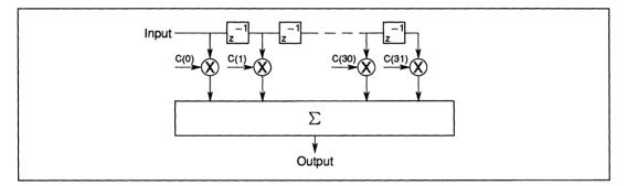
Figure 3.1 Canonical transversal filter architecture
