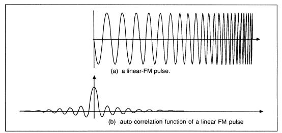
Figure 10.15 Pulse compression using a coded signal
