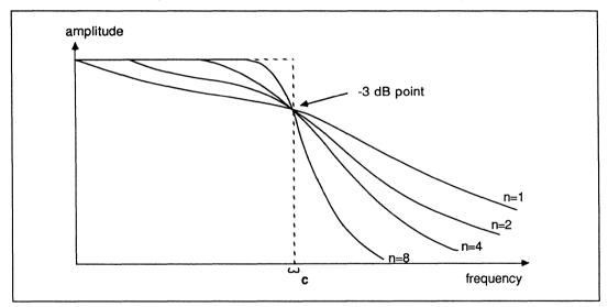
Figure 8.14 Frequency response of the Butterworth filter
