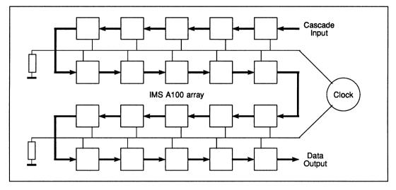
Figure 12.4 Clock distribution for large system
