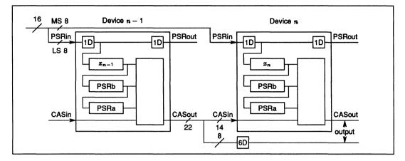
Figure 14.11 Alternative cascade if IMS A110s for increased data precision
