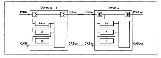
Figure 14.4 Direct data path connection for cascading IMS A110s
