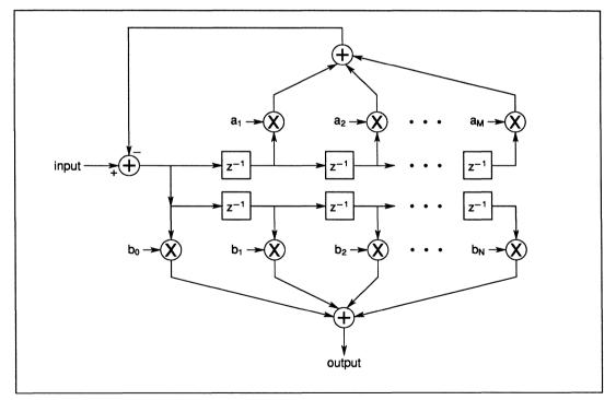
Figure 8.5 Recursive (IIR) digital filter structure
