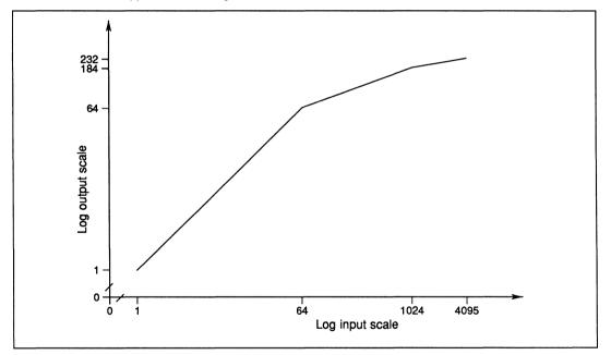
Figure 15.9 Typical dynamic range compression function
