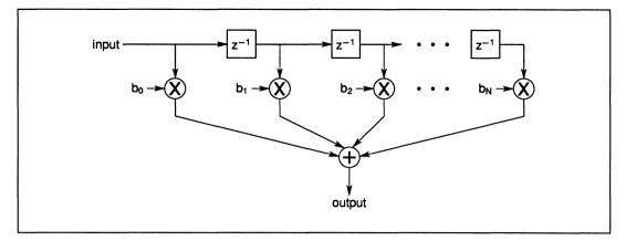
Figure 8.4 Nonrecursive digital filter structure
