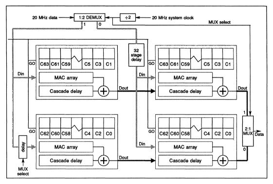
Figure 12.6 20 MHz system using cascade adders
