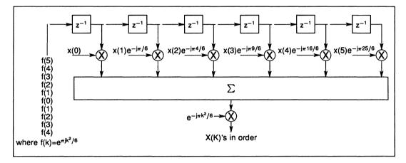
Figure 9.12 Schematic diagram for 6 point CZT using canonical transversal filter structure
