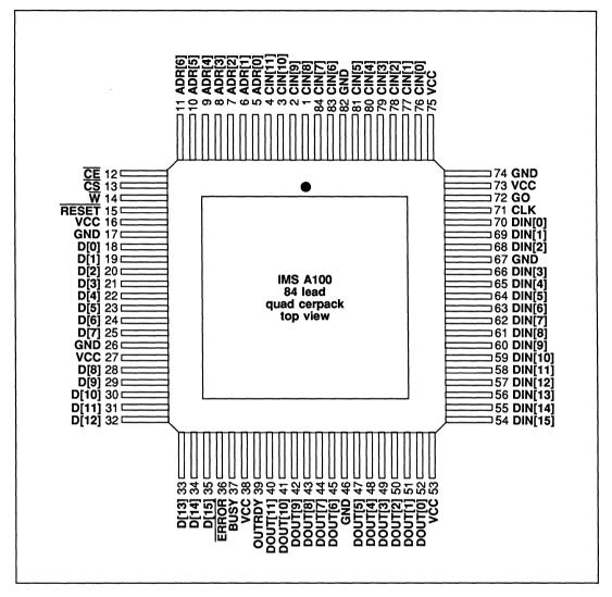
Figure 3.8 IMS A100 pin configuration
