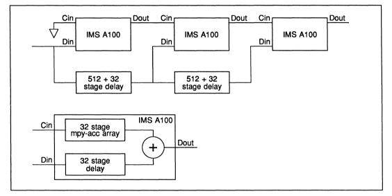
Figure 13.12 Hardware for real time image convolution
