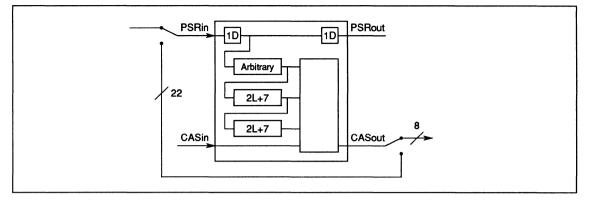
Figure 14.8 Multi-pass filtering by using feedback
