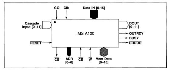
Figure 12.1 IMS A100 device schematic
