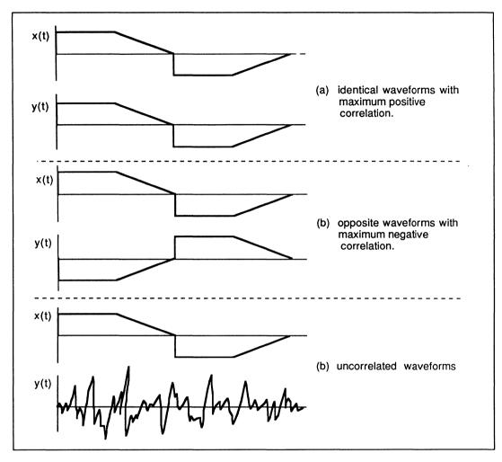
Figure 10.1 Illustration of correlation process
