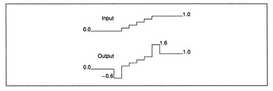
Figure 13.6 Effect of gradual edges on convolution output
