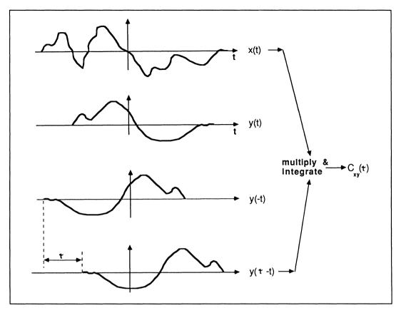
Figure 10.3 Illustrating the convolution process
