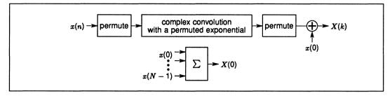
Figure 9.10 The principle of the prime number transform
