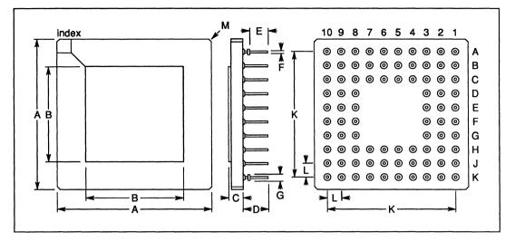
Figure 3.7 84 pin grid array package dimensions
