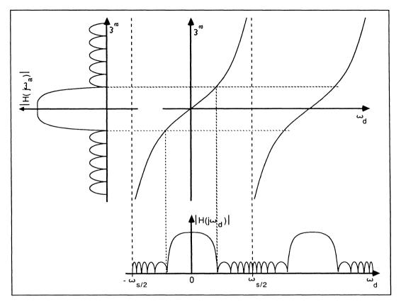
Figure 8.18 Graphical illustration of the bilinear z-transform
