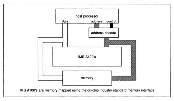
Figure 9.7 Schematic diagram of a simple IMS A100 based system
