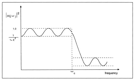
Figure 8.16 Frequency response for an elliptic filter
