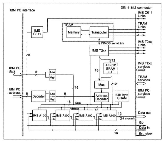
Figure 6.2 IMS B009 Detailed Block Diagram
