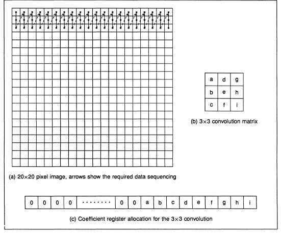
Figure 10.11 Example of a 3×3 image convolution/correlation with the IMS A100
