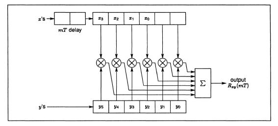
Figure 10.4 Schematic diagram for an ideal correlator hardware
