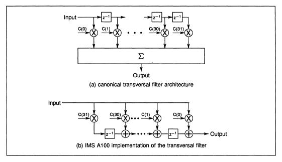
Figure 9.1 Transversal filter architecture
