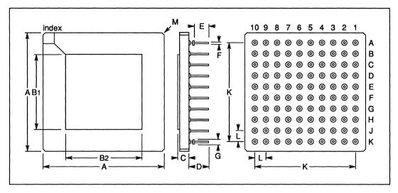
Figure 4.9 100 pin grid array package dimensions
