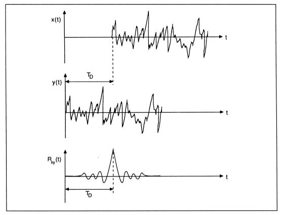
Figure 10.13 Delay estimation using correlation process
