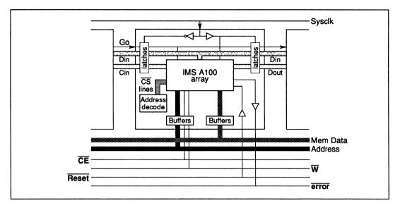
Figure 12.3 Placement of IMS A100 into large system
