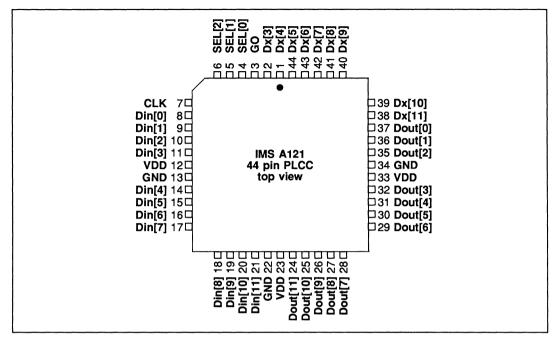
Figure 5.4 IMS A121 44 pin PLCC J-bend package pinout
