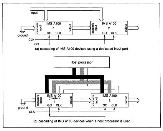
Figure 8.12 Cascading IMS A100 devices
