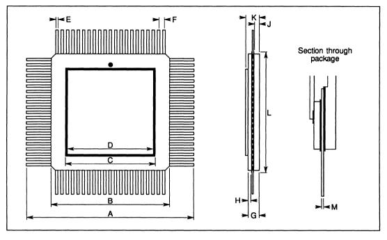
Figure 3.9 84 lead quad cerpack package dimensions
