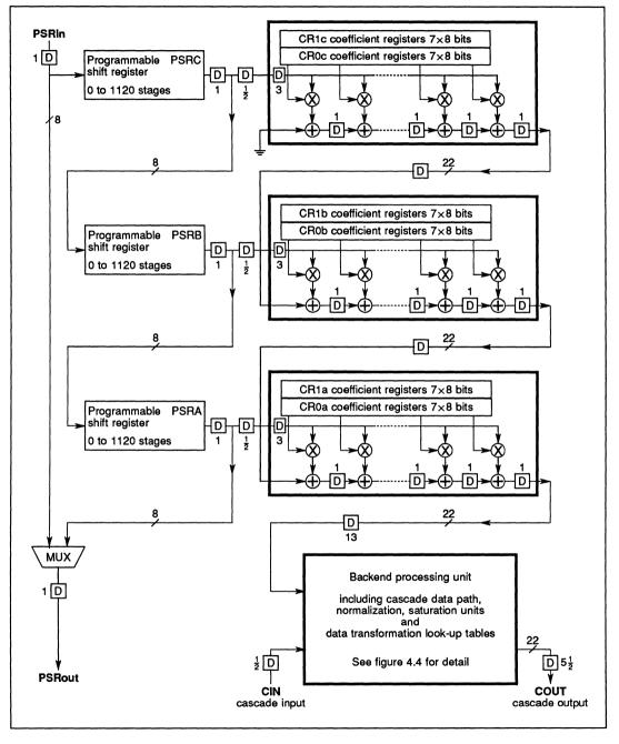
Figure 4.2 Synchronous functions of the IMS A110
