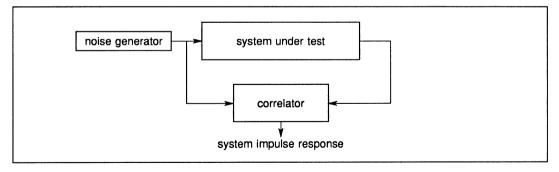
Figure 10.16 System identification using correlation
