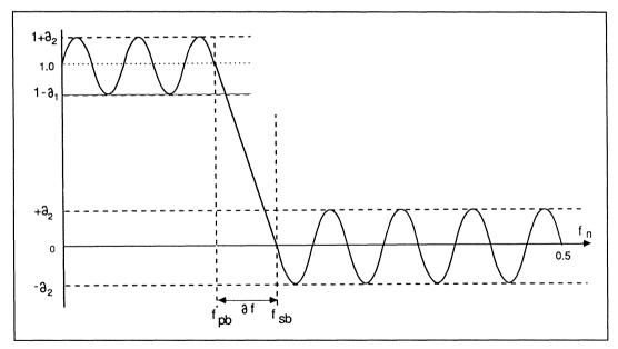
Figure 8.7 Specification parameters for a low pass filter. Similar parameters exist for high pass and band pass filters.
