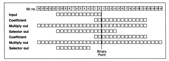
Figure 5.2 IDCT internal number format
