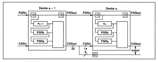
Figure 14.13 Alternative cascade if IMS A110s for increased coefficient precision
