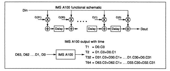
Figure 13.8 Illustration of IMS A100 pipelined calculation
