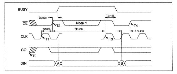
The bankswap timing diagram shows how successive data samples (A and B) can be processed by different sets of coefficients by causing a bankswap to occur between the input of sample A and sample B.
