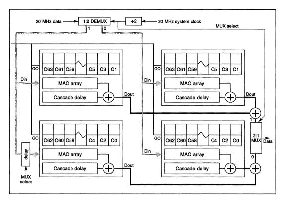
Figure 12.5 20 MHz system using external adders
