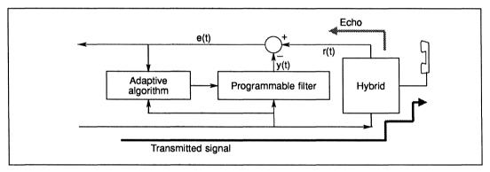
Figure 8.20 Application of adaptive filtering techniques to echo cancellation
