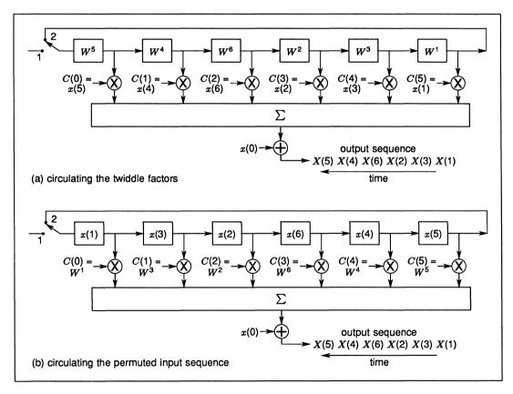
Figure 9.3 Prime number transform implementation based on the transversal filter structures
