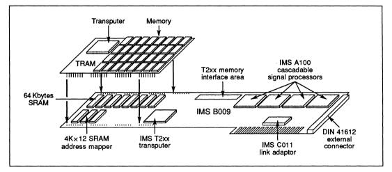
Figure 6.1 IMS B009 key components
