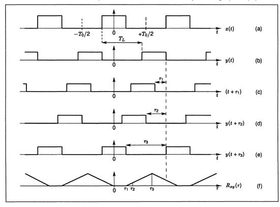
Figure 10.2 Graphical illustration of the correlation process
