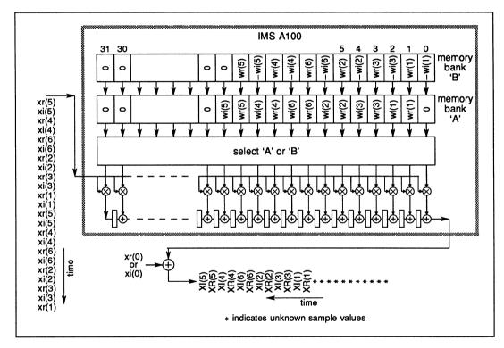
Figure 9.6 IMS A100 implementation of a 7 point complex DFT corresponding to the canonical transversal filter realization of figure 9.3b
