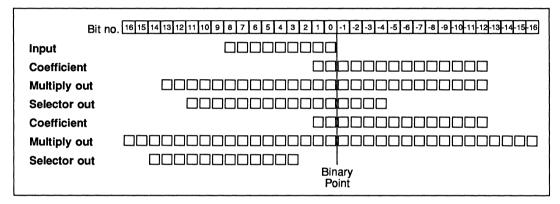
Figure 5.1 DCT internal number format
