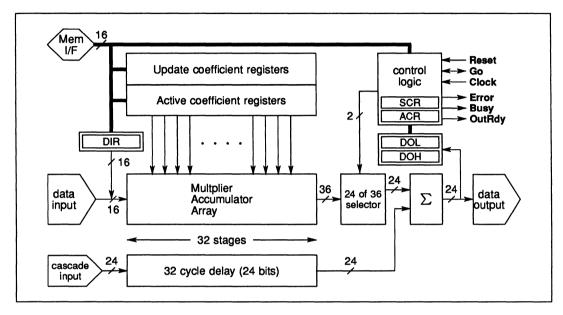
Figure 13.7 User's model of the IMS A100.
