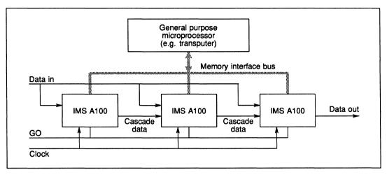
Figure 13.11 IMS A100 coefficient loading
