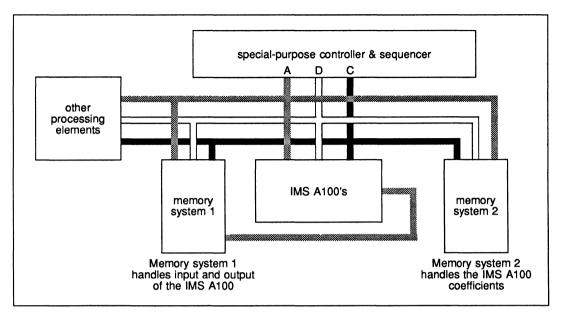
Figure 9.9 Schematic block diagram of a high performance involving a special purpose controller
