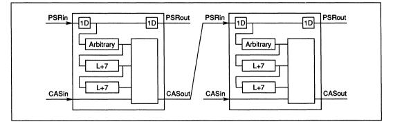
Figure 14.7 Cascading IMS A110s for multi-pass filtering
