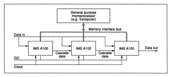
Figure 3.4 A simple IMS A100 based system
