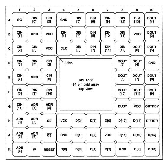
Figure 3.6 IMS A100 pin configuration
