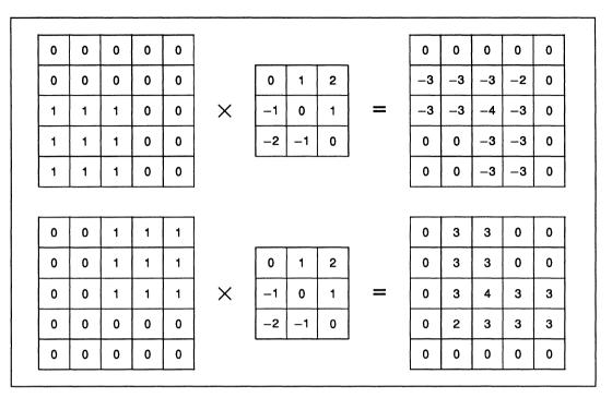
Figure 13.4 Illustration of edge detection
