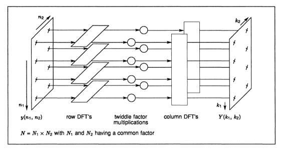
Figure 9.15 Mapping of an N point DFT into dimensions
