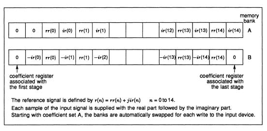
Figure 11.4 Example of reference signal allocation for a 15 point complex correlation using the IMS A100
