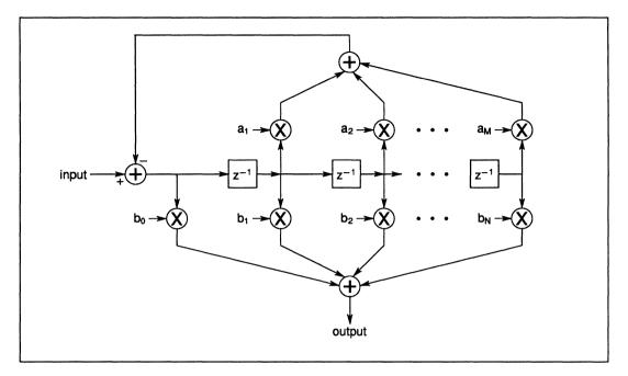
Figure 8.6 Alternative recursive (IIR) digital filter structure with reduced number of delay stages
