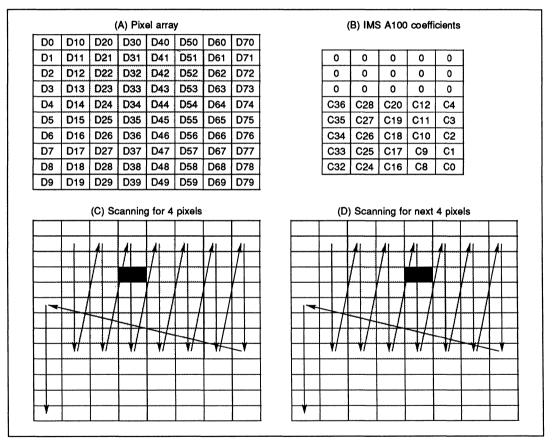
Figure 13.10 Pixel scanning and coefficient ordering - high performance
