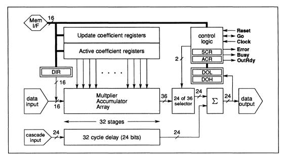
Figure 11.2 User's model of the IMS A100
