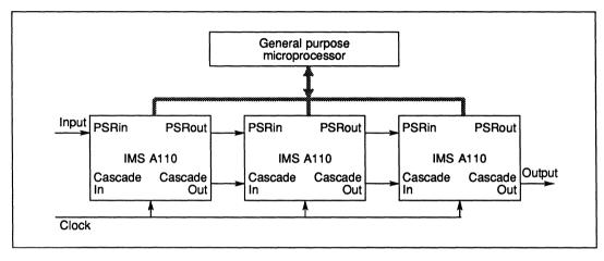
Figure 4.3 A typical IMS A110 based system
