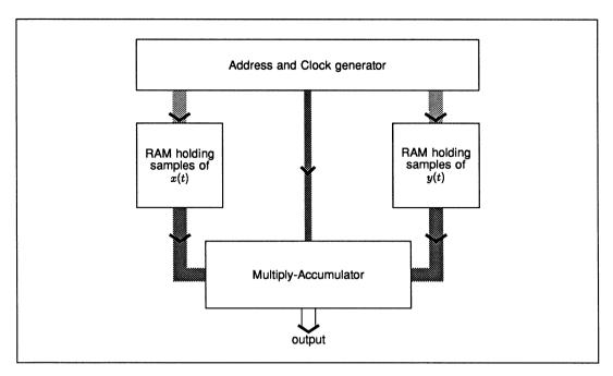
Figure 10.5 Block diagram of a conventional correlator/convolver
