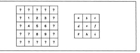
Figure 13.1 [3  $\times$  3] convolution on a [5  $\times$  5] image
