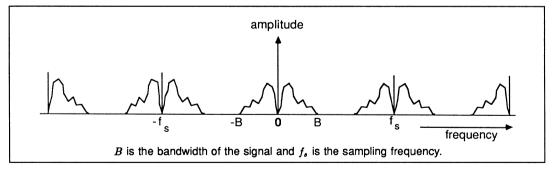
Figure 8.2 Spectrum of a sampled signal
