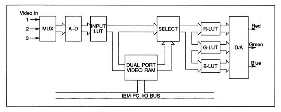
Figure 13.14 Frame grabber hardware support
