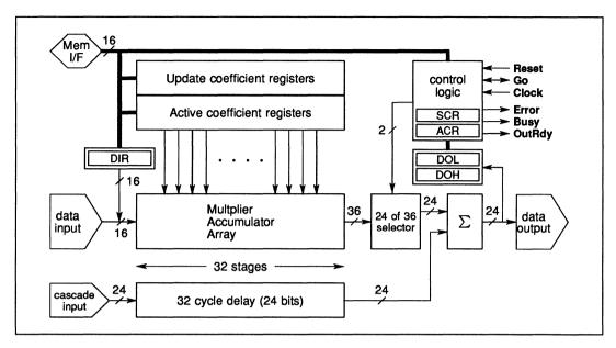
Figure 9.2 User's model of the IMS A100
