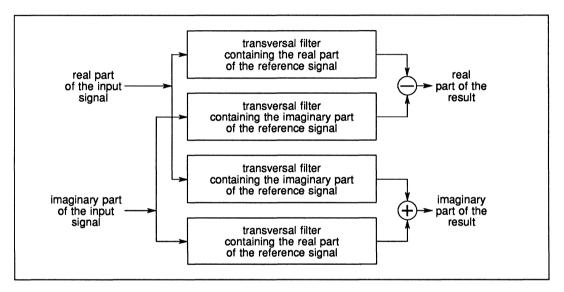
Figure 9.4 Conventional complex correlator/convolver involving four transversal filters
