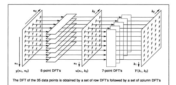
Figure 9.14 Schematic representation of equation 65 for  $N = N_1 \times N_2 = 7 \times 5$
