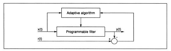
Figure 8.19 Basic structure of an adaptive filter
