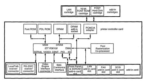
Figure 2. R36100-based Printer System
