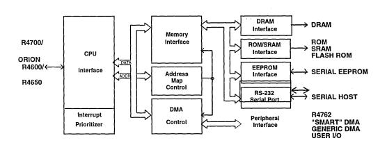
FIGURE 1: 4761 BLOCK DIAGRAM
