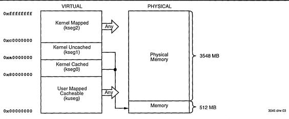
Figure 3. Virtual to Physical Mapping of Extended Architecture Versions
