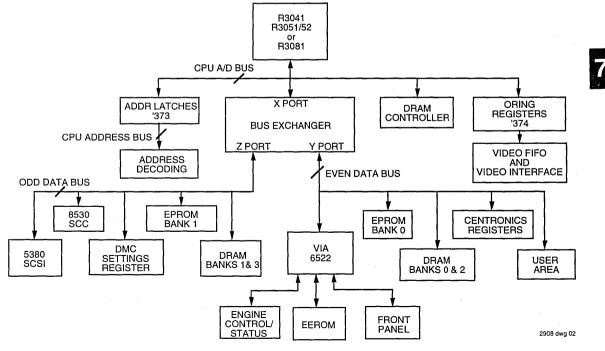
Figure 2. IDT79S389 High Level Schematics
