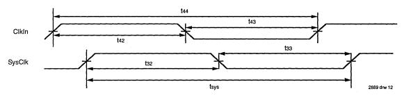
Figure 8 (a). R3081 Clocking (1x clock input mode, full frequency bus)
