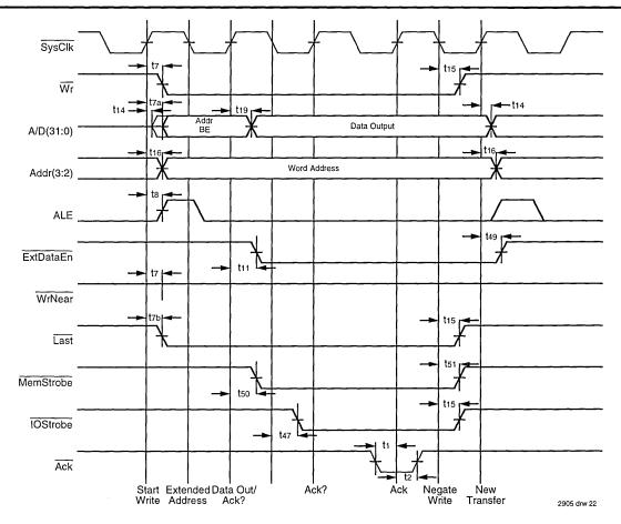
Figure 17. Basic Write to 32-bit Memory Port
