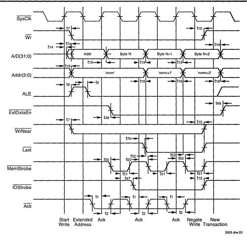
Figure 18. Trl-Byte Mini-burst Write to 8-bit Port
