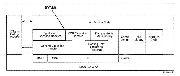
Figure 1. Schematic Representation of the modules in IDT/kit, showing how they control parts of the R3000 or R4000 CPU and connect to IDT/sim, IDT's debug monitor.
