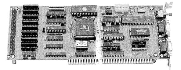
Figure 1. R3041 System Evaluation Board. Actual Size 4.2" x 10.0"
