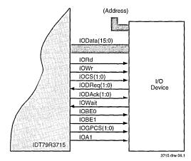
Figure 2.5 General Purpose I/O Device Interface
