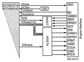
Figure 2.5: R3710/R3740 Engine Interface
