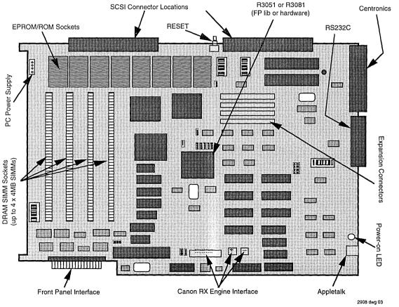
Figure 3. IDT79S389 Board Layout
