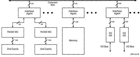
Figure 8. Multiprocessor System Using the R4400 MC
