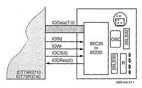
Figure 2.8: DMA-Supported AppleTalk I/O Port
