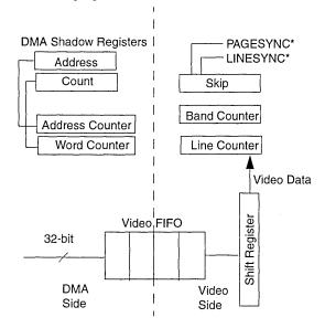
Figure 5.3 Video Block Diagram
