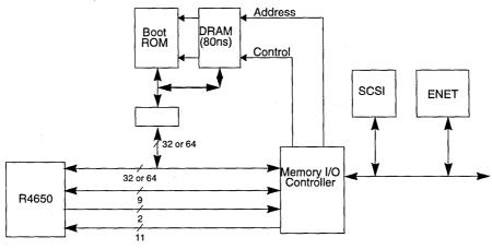
Figure 4: Typical R4650 System Architecture
