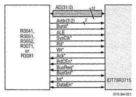
Figure 2.1 RISController to R3715 Interface
