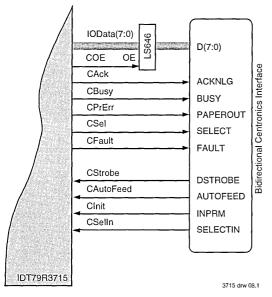
Figure 2.6 IEEE P1284 Bidirectional Centronics I/O Port
