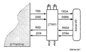
Figure 2.14: UART Serial Interface Implementation
