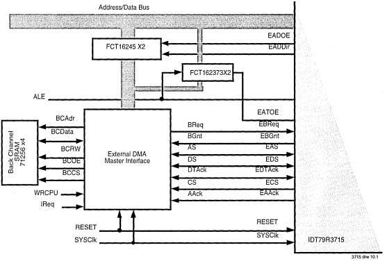
Figure 2.2 External DMA Master Coprocessor Implementation
