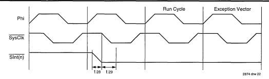
Figure 18. Synchronized Interrupt Input Timing
