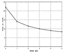
28 Pin SOJ Theta JA vs. Airflow
