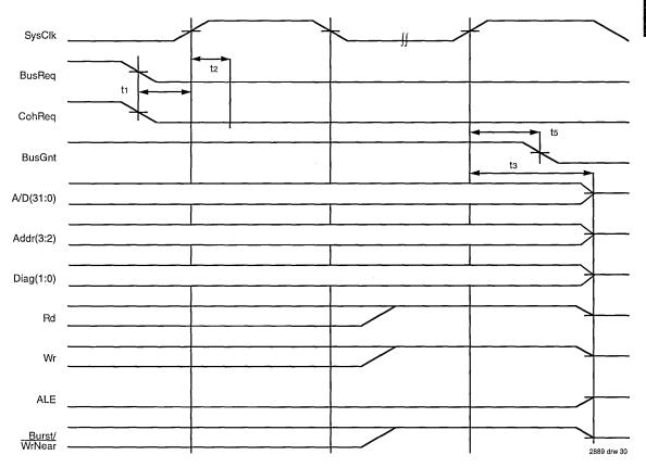
Figure 22. Coherent DMA Request
