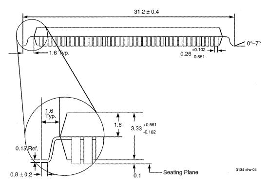
Figure 10.2 Expanded View of Figure 10.1 Detail
