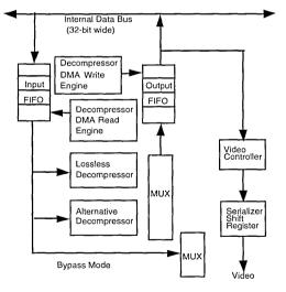
Figure 2.13.a: Decompressor Block Diagram
