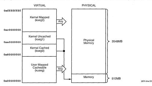
Figure 3. Virtual-to-Physical Mapping of Extended Architecture Versions
