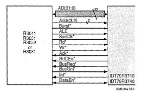
Figure 2.1: RISController to R3710/R3740 Interface
