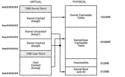
Figure 4. Virtual-to-Physical Mapping of Base Architecture Versions
