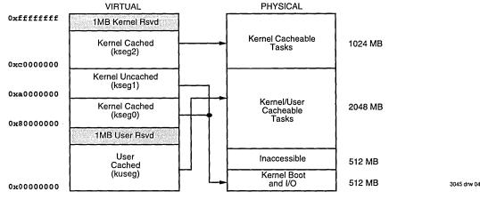
Figure 4. Virtual to Physical Mapping of Base Architecture Versions
