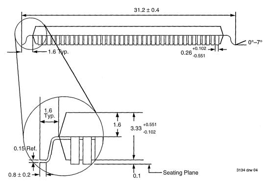
Figure 10.2: Expanded View
