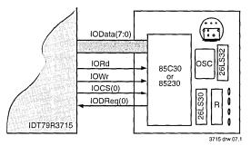
Figure 2.4 DMA-Supported AppleTalk I/O Port
