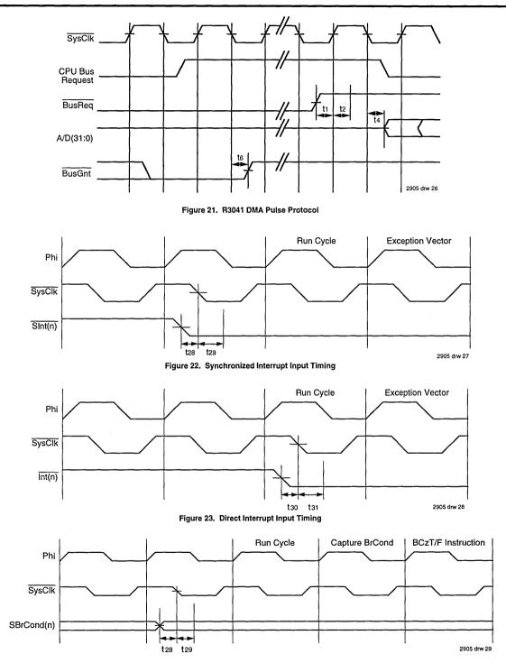
Figure 24. Synchronized Branch Condition Input Timing
