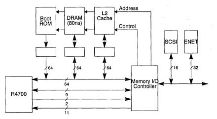
Figure 5: Typical Desktop System Block Diagram
