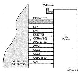
Figure 2.10: General Purpose I/O Device Interface
