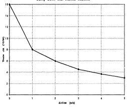
28 Pin Plastic Dip Theta JA vs. Airflow
