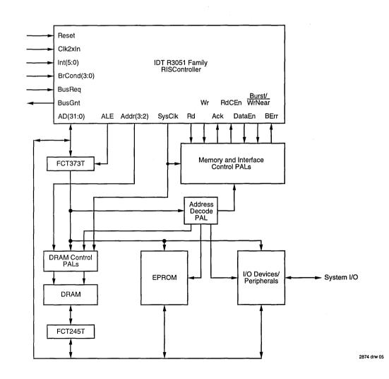
Figure 5. Typical R3051 Family Based System
