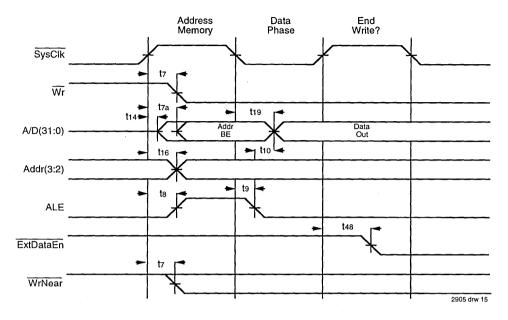
Figure 12(c). Start of Write Timing with Non-Extended Address Hold Option
