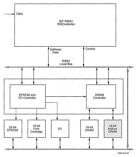
Figure 4. Typical R3041-Based Application
