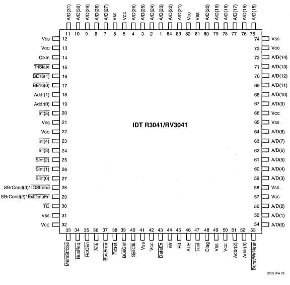
84-Pin PLCC/ Top View (Cavity Down)
