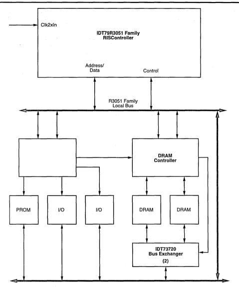
Figure 6. R3051 Family Chip Set Based System
