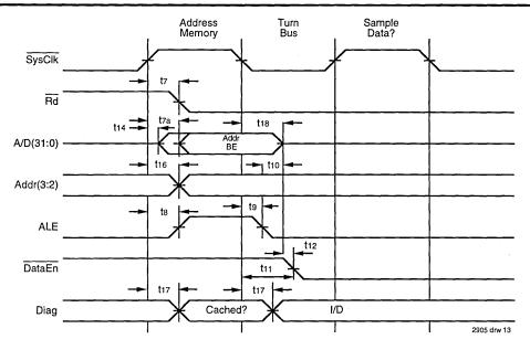
Figure 12(a). Start of Read Timing with Non-Extended Address Hold Option
