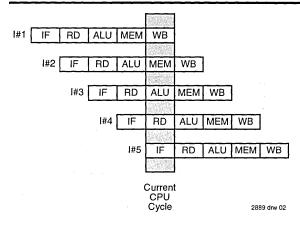
Figure 2. R3081 5-Stage Pipeline
