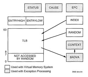
Figure 4. The System Coprocessor Registers
