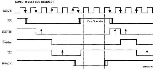
Figure 6. Bus Request Timing Diagram
