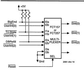
Figure 12. Reset Vector Circuit
