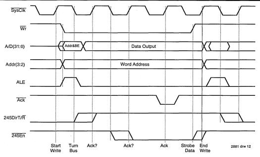
Figure 10b. Timing Diagram of FCT245 Enable and T/R Direction Controls for a Write
