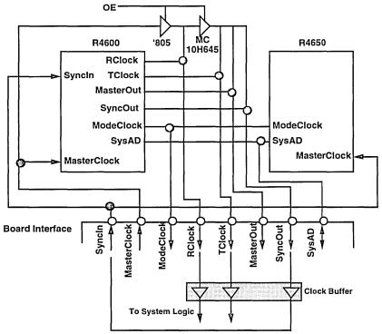
Figure 4. Single System With R4600 and R4650
