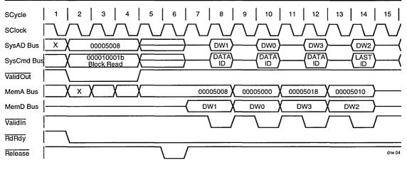
Figure 4. R4000 Block Read Cycle
