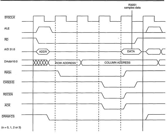
Figure 6. Single-Word Read Access Timing
