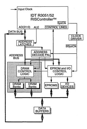
Figure 3. R3051 RISController Family-Based System
