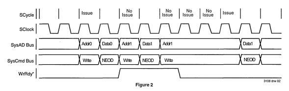
The Pipelined write protocol maintain the issue rules of the R4x00 compatible writes but eliminates the two unused cycles between back-to-back writes. The external system is there-
