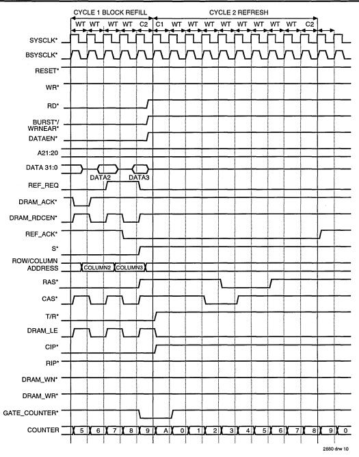
Figure 10. Refresh Arbitration and Refresh Timing Diagrams
