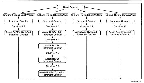
Figure 11. State Diagram of an Example Wait-State Controller for a Single Memory Type
