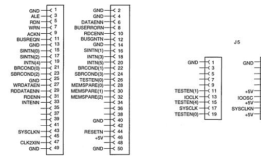
Figure 19. 50-Pin Connector
