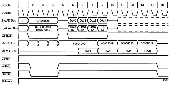
Figure 8. R4000 Write Block Cycle
