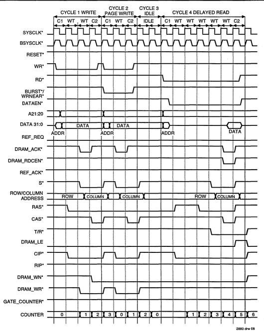
Figure 8. Delayed Single Read Timing Diagrams
