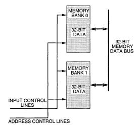
Figure 1b. Two-Bank Non-Interleaved System
