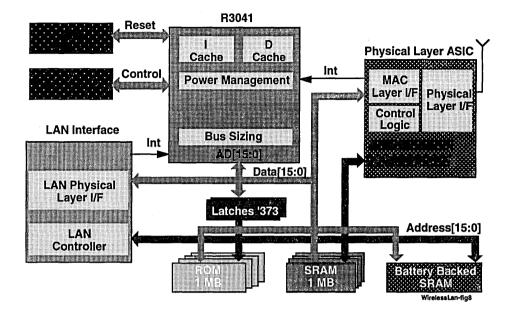
Figure 5. Access Point based on the R3041
