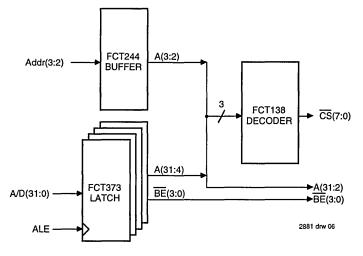
Figure 6. Address De-multiplexer and Decoder
