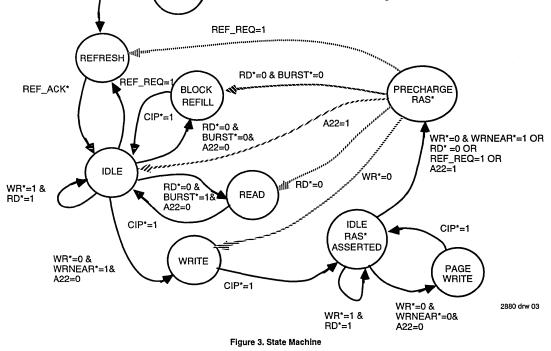
The state machine uses the Reset pulse to reset its internal states and to synchronize its operation to the R3051. During the RESET state, it also performs one refresh cycle before entering the IDLE state.
