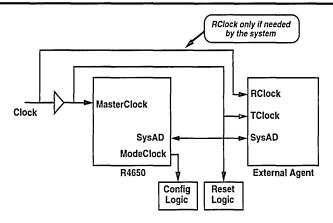
Figure 3. Generating R4600-Compatible Clocks
