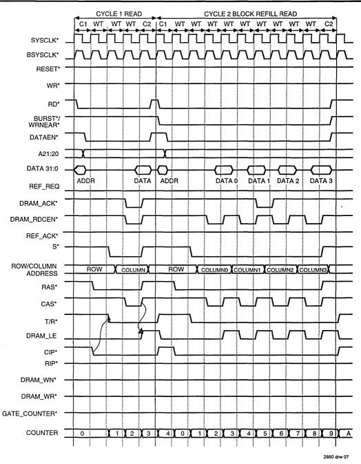
Figure 7. Single Read and Block Refill Read Timing Diagrams
