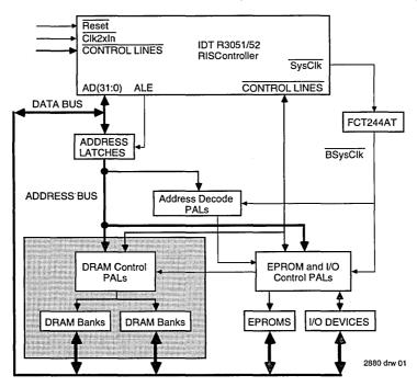
Figure 1. R3051 RISController Family Based System
