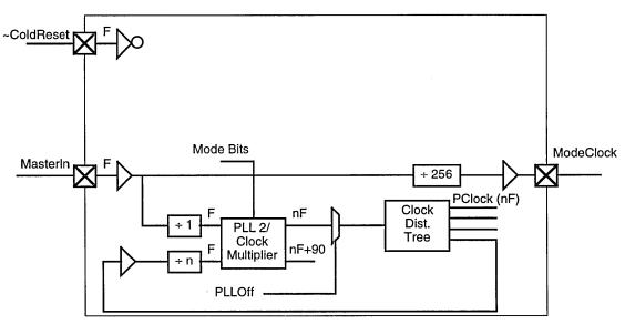
Figure 2. R4650 Clock Distribution Tree and PLL
