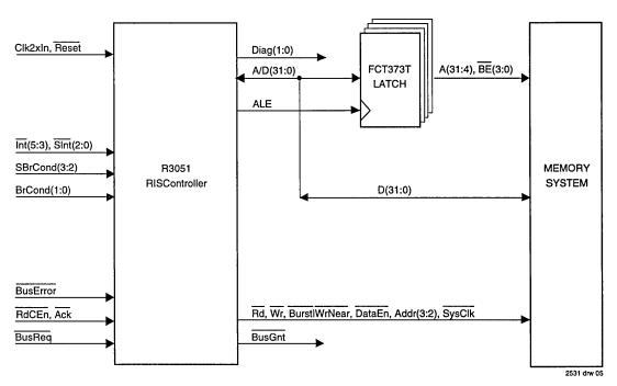
Figure 5. R3051 Memory System Connected Directly to the A/D Bus
