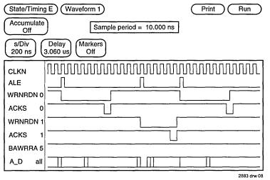
Figure 8. R3051 Timing Mode Waveform
