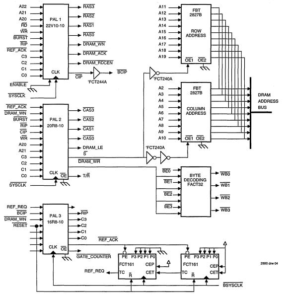
Figure 4. Control System and Address Path
