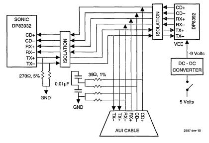
Figure 10. Physical Layer Interface Block Diagram
