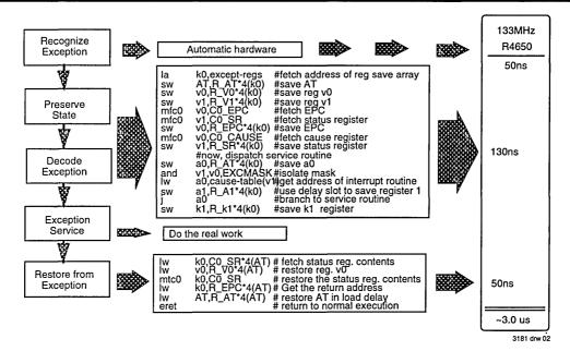
Figure 2. R4650 Interrupt Response Time Real-Time Interrupt Response
