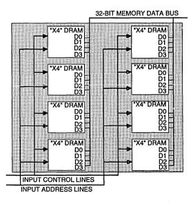
Figure 1a. Single-Bank Non-Interleaved System
