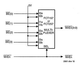
Figure 16. Gating Byte Enables into the Write Enables
