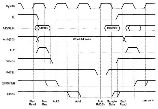
Figure 10a. Timing Diagram of FCT245 Enable and T/R Direction Controls for a Read
