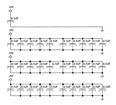
Figure 21. Decoupling Capacitors
