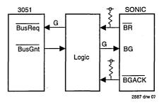
Figure 7. Bus Request Interface Block Diagram
