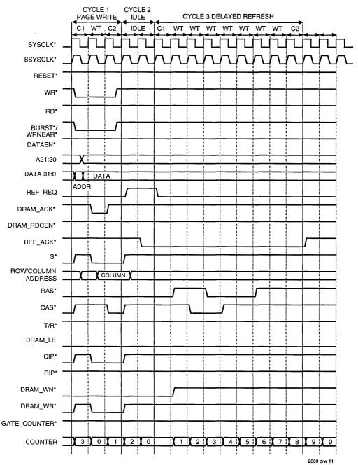
Figure 11. Delayed Refresh Timing Diagrams
