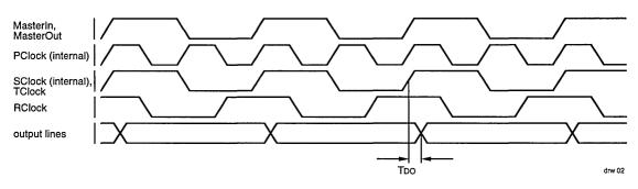
Figure 2. R4000 Clock Interface Timing (PClock to SClock divisor of 2)
