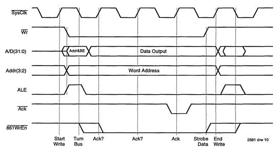
Figure 9b. Timing Diagram of FCT861 Write Direction Enable
