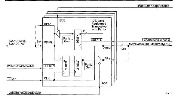
Figure 11. R4000 Integrated Read and Write Buffer
