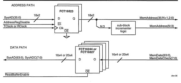
Figure 6. R4000 Single Level Read Buffer
