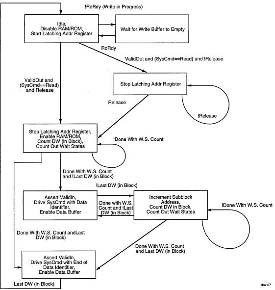
Figure 7. R4000 Read Interface State Machine
