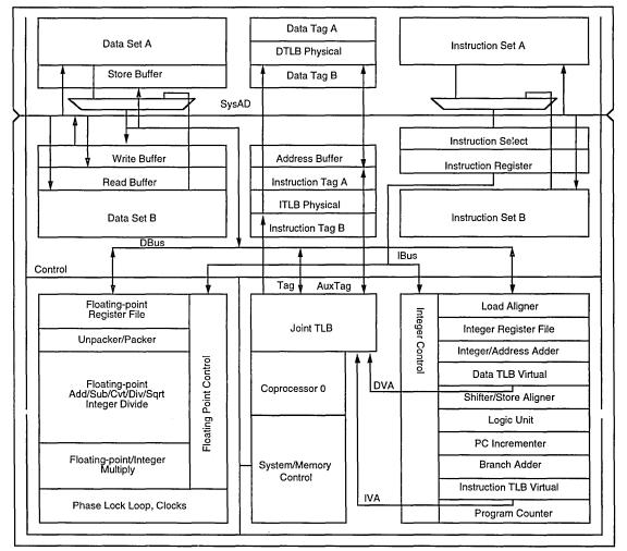
Figure 1. IDT Orion Block Diagram
