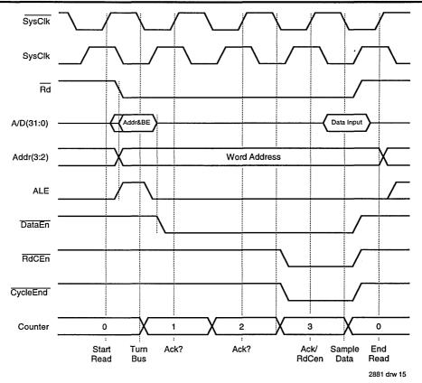
Figure 13. Timing Diagram of CycleEnd
