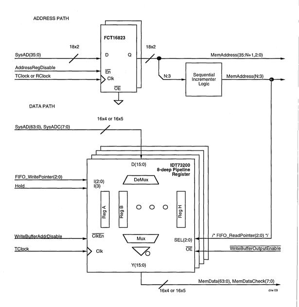
Figure 9. R4000 8-Level, 64-bit Wide Write Buffer
