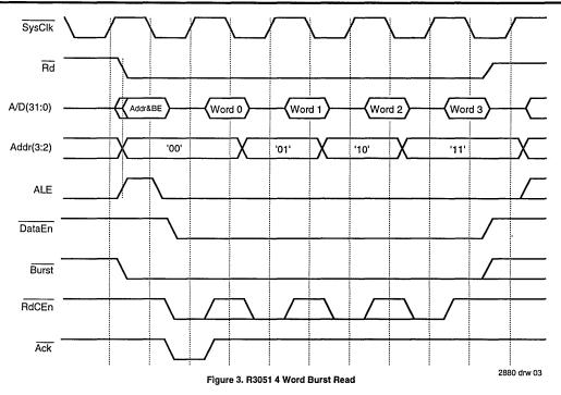
also designed to meet the address hold time of latches. As with all high speed processors, ALE should be considered a critical signal. Thus Printed Circuit Board routing should minimize ALE's trace length and crosstalk susceptibility.
