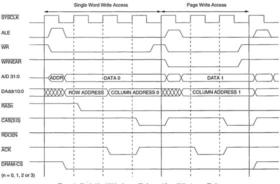
Figure 8. Single-Word Write Access Timing and Page Write Access Timing
