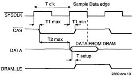
Figure 13. Read or Block Refill Access
