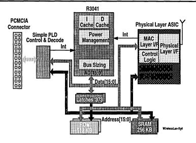
Figure 2. PCMCIA WLAN Adapter Based on the R3041 PCMCIA WLAN with the R3041
