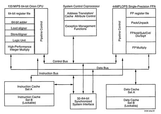
Figure 1. R4650 Block Diagram
