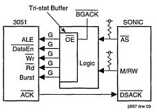
Figure 9. Master Interface Block Diagram
