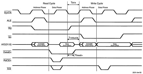
Figure 3. R3051 Read Cycle Followed by a Write Cycle
