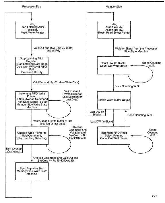
Figure 10. R4000 Write Buffer State Machine
