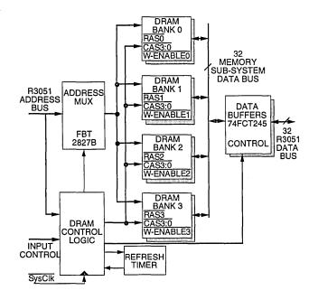
Figure 4. DRAM Memory Subsystem Architecture
