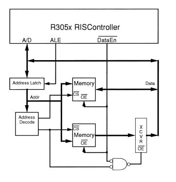
Figure 8.5. Use of DataEn as Output Enable Control
