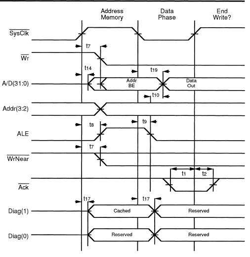
Figure 9.2. Memory Addressing and Start of Write
