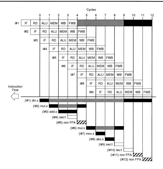
Figure 3.13. Overlapped Instructions in FPA Pipeline
