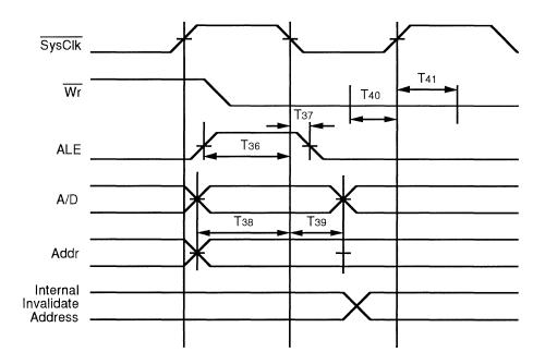
Figure 10.4. Capturing Write Target Address During Coherent DMA
