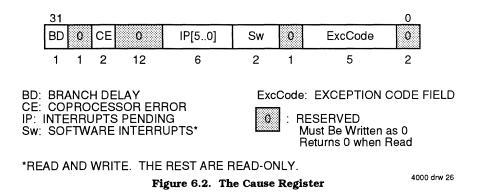
**SW** The Software interrupt bits can be thought of as the logical extension of the IP field. The SW interrupts can be written to force an interrupt to be pending to the processor, and are useful in the prioritization of exceptions. To set a software interrupt, a "1" is written to the appropriate SW bit, and a "0" will clear the pending interrupt. There are corresponding interrupt mask bits in the status register for these interrupts.
