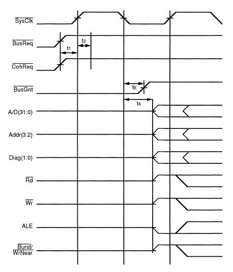
Figure 10.7. Terminating Coherent DMA
