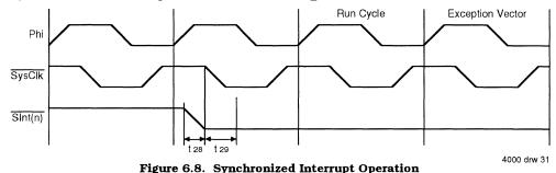
The other interrupts, Int(5:3), do not contain this synchronization logic, and thus have slightly better latency to the exception vector. However, the interrupting agent must guarantee that it always meets the interrupt input setup and hold time requirements of the processor. These inputs are useful for interrupting agents which operate off of the SysClk output of the processor. The operation of these interrupts is illustrated in Figure 6.9.
