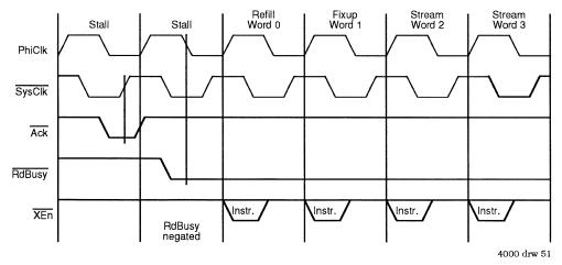
Figure 8.7. Instruction Streaming Example (Full Frequency Mode)
