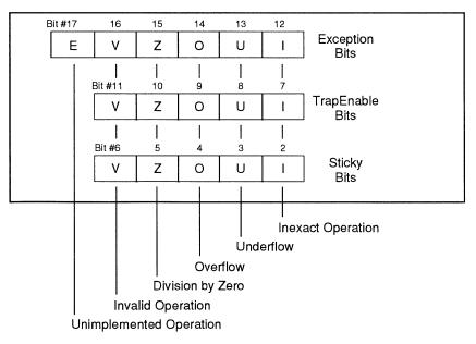
Figure 3.4. Control/Status Register Exception/Sticky/Trap Enable Bits
