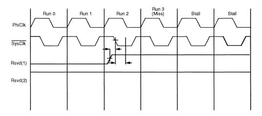
Figure 12.2. Forcing an Instruction Cache Miss in Debug Mode
