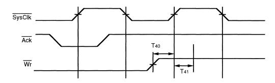
Figure 10.6. Terminating a Coherent Write Sequence
