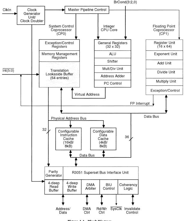
Figure 1.1. Block Diagram
