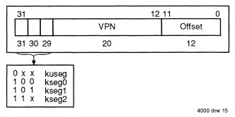
Figure 5.1. Virtual Address Format
