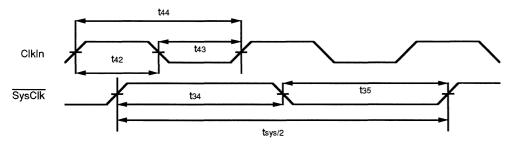
Figure 11.6 (b). R3081 Family Clocking (1x ClkIn, Half-Frequency Bus Mode)
