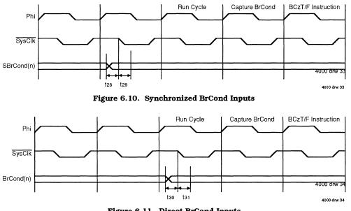
Figure 6.11. Direct BrCond Inputs
