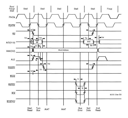
Figure 8.13. Single Word Read Terminated by Bus Error
