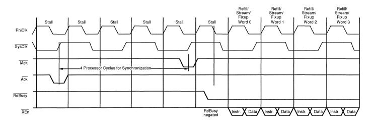
Figure 8.6(b). Internal Processor States on Burst Read (Half Frequency Mode)
