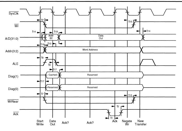
Figure 9.6. Write With Bus Wait Cycles
