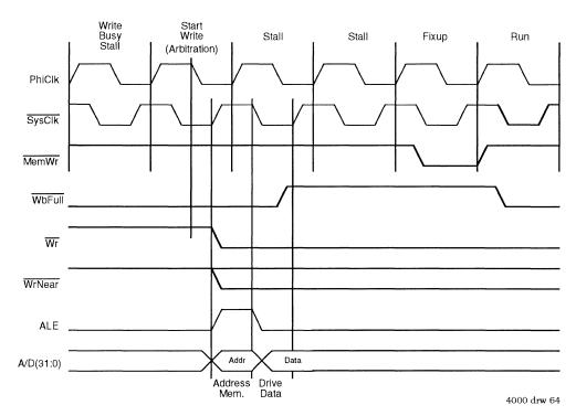
Figure 9.4. Write Buffer Full Operation
