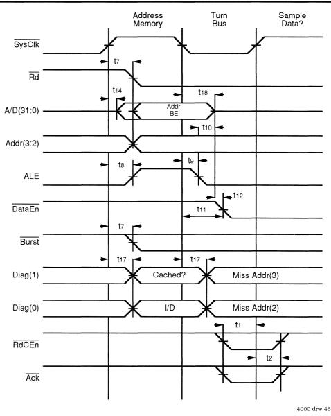
Figure 8.2. Start of Bus Read Operation
