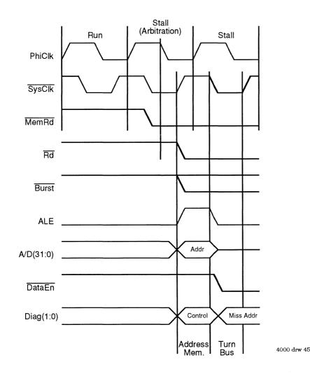
Figure 8.1(a). CPU Latency to Start of Read (Full Frequency Mode)
