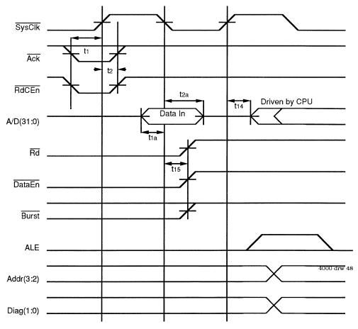
Figure 8.4. Read Cycle Termination
