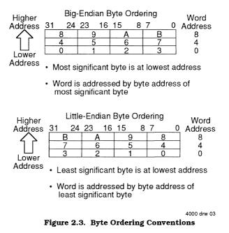
Figure 2.3 shows the ordering of bytes within words and the ordering of words within multiple word structures for the big-endian and little-endian conventions.
