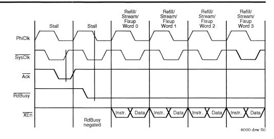
Figure 8.6(a). Internal Processor States on Burst Read (Full Frequency Mode)
