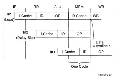
Figure 2.7. Load Delay
