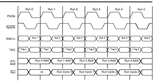
Figure 12.1 (a). R3051 Debug Mode Instruction Address Display (Full-Frequency Mode)
