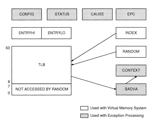
Figure 5.4. The System Coprocessor Registers
