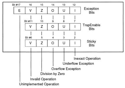
Figure 6.22. FPA Control/Status Register
