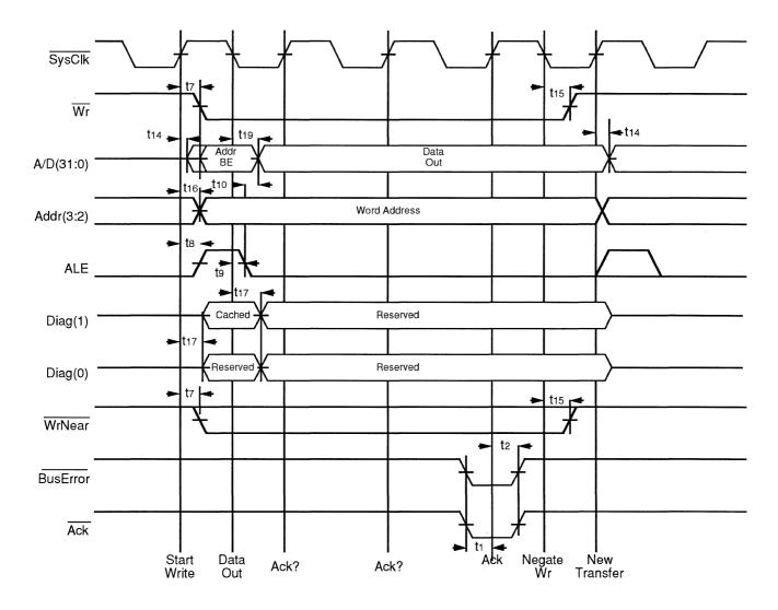
Figure 9.7. Bus Error on Write
