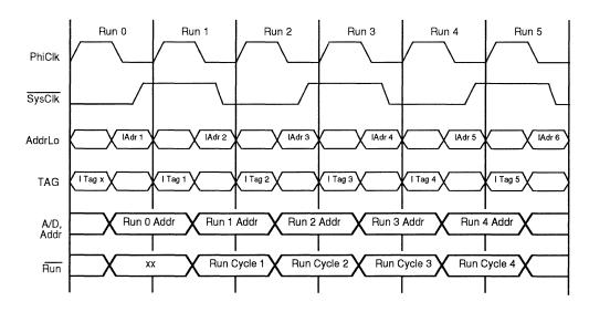
Figure 12.1 (b). R3051 Debug Mode Instruction Address Display (Half-Frequency Mode)
