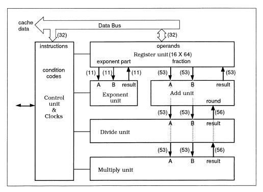
Figure 3.1. On-Chip FPA Functional Block Diagram
