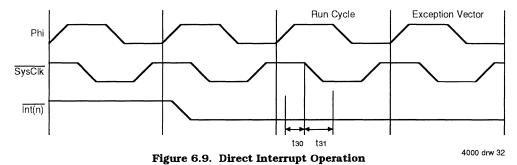
Note that one of the processor interrupt inputs will be used for the internal floating point unit, as determined by the Config register. The external input pin corresponding to the selected interrupt path for the floating point will be ignored. The system must provide a pull-up at the corresponding pin.
