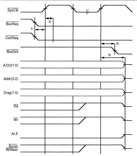
Figure 10.3. Requesting Coherent DMA
