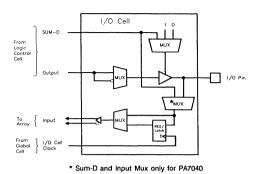
Figure 5. I/O Cell (IOC) for the PA7024 and PA7040
