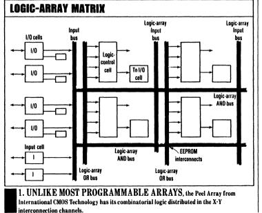
new family of electrically erasable. programmable logic circuits. The family solves some of the architectural limitations of past programmable chips by applying low-power CMOS circuitry and electrically erasable memory to a novel architecture.
