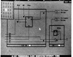
The PACE architectural editor graphically expands individual cells for detailed viewing and control of architecture and equations.
