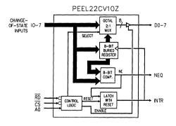
Figure 10. PEEL22CV10Z Change-of-State Detector functional block diagram
