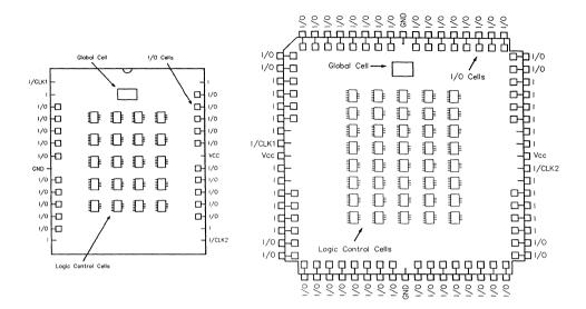
Figure 7. Pin/Block Diagrams for the PA7028 and PA7068
