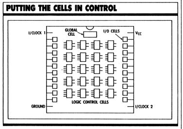
The PEEL family of programmable logic arrays combines I/O, logic-control, and a global cell in a new architecture.
