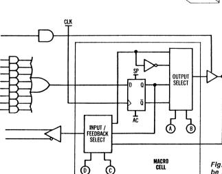
uct terms (AND gates) that are divided into groups of eight, each feeding into an OR function. Each OR function is directly associated with one of eight independent macrocells and I/O pins.
