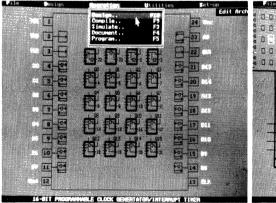
The PACE architectural editors "chip display" provides a global view of design allowing quick access to I/Os, registers, cells and equations.
