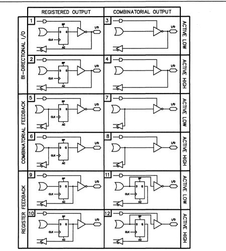
Figure 5. Equivalent Circuits for the Twelve Configurations of the PEEL18CV8 I/0 Macrocell.
