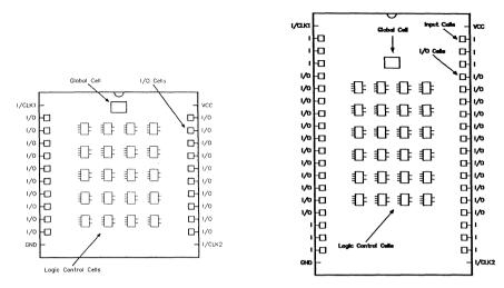
Figure 2: PEEL ARRAY pin/block diagrams for PA7024 and PA7040
