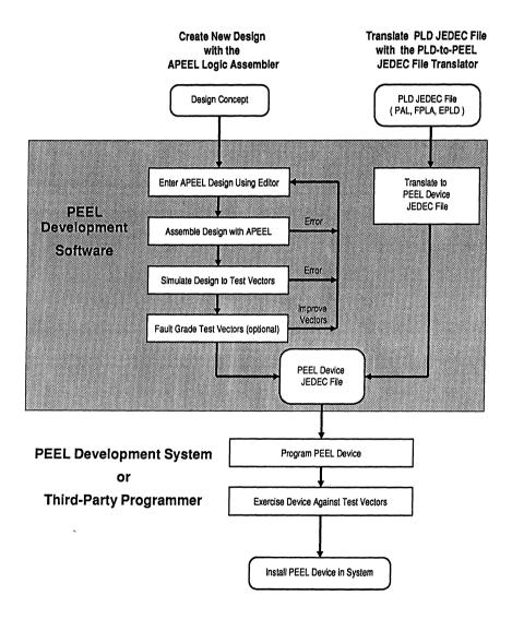
Figure 4. The PEEL Device Development Process
