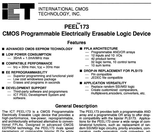
parameters of comparable bipolar PLDs while providing a dramatic improvement in active power consumption. The EE-reprogammability of the PEEL173 reduces development and field retrofit costs and enhances testability to ensure 100% field programmability and function. PEEL technology allows for low cost "windowless" packaging in a ceramic or plastic 24-pin, 300-mil DIP.
