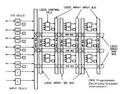
Figure 3. Distributed logic array matrix
