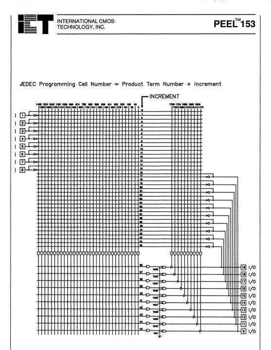
PEEL153 Logic Array Diagram
