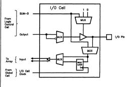
Figure 5. PA7040 I/O Cell (IOC)
