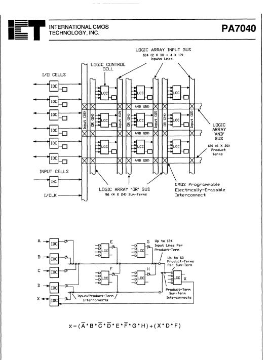
Figure 3. PA7040 Distributed logic array matrix (partial view) and illustration of a sum-of-products logic equation interconnected in the array
