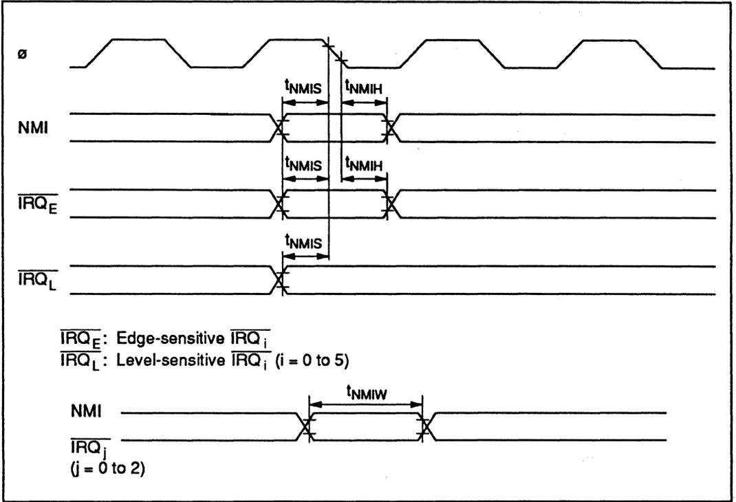
Figure 20-17 Interrupt Input Timing
