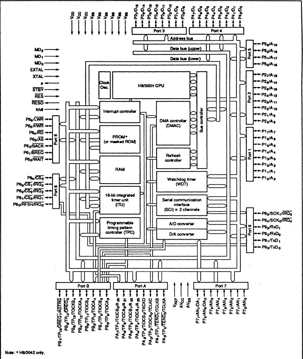
Figure 1-1 Block Diagram
