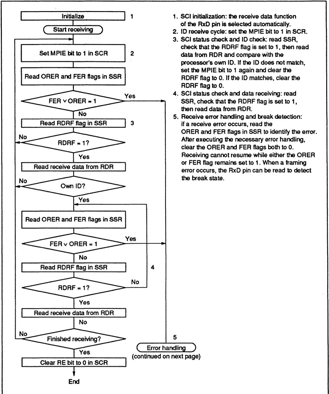
**Figure 13-12 Sample Flowchart for Receiving Multiprocessor Serial Data (1)**
