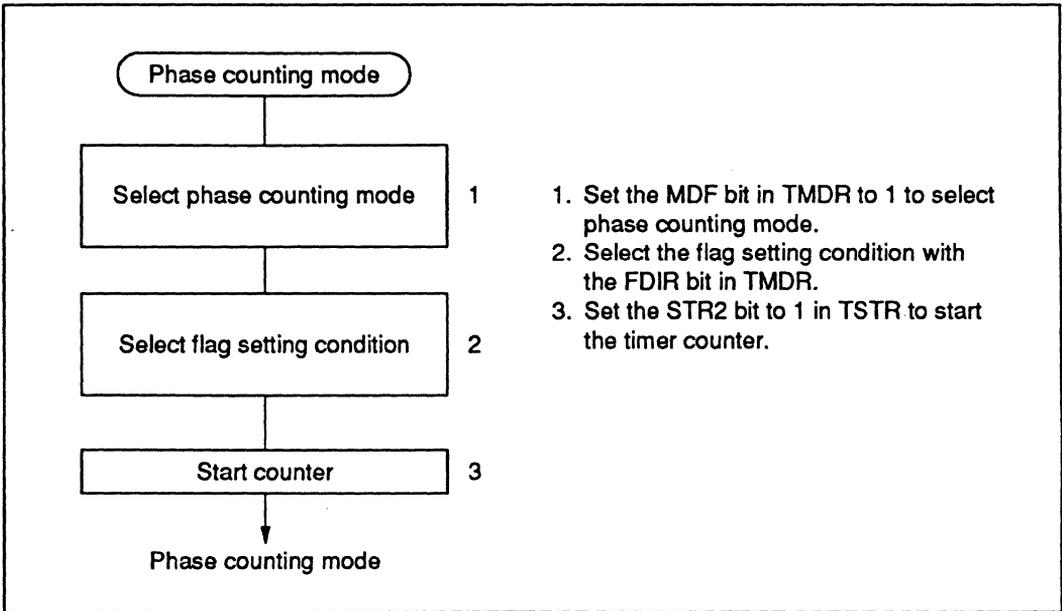
**Figure 10-43 Setup Procedure for Phase Counting Mode (Example)**
