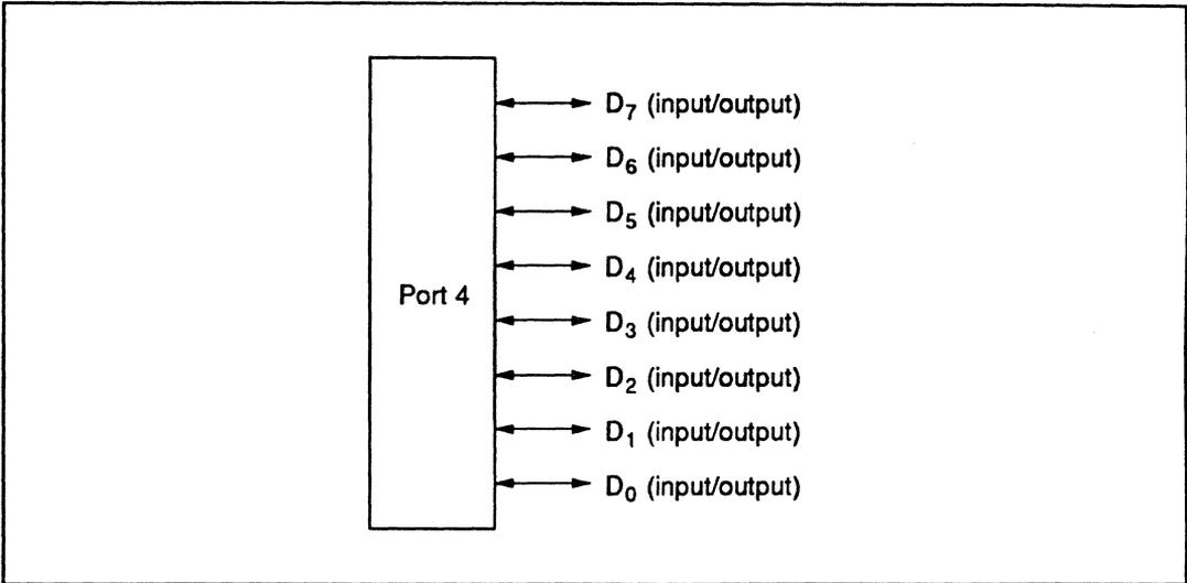
**Figure 9-14 Pin Functions in 16-Bit Bus Mode (Port 4)**
