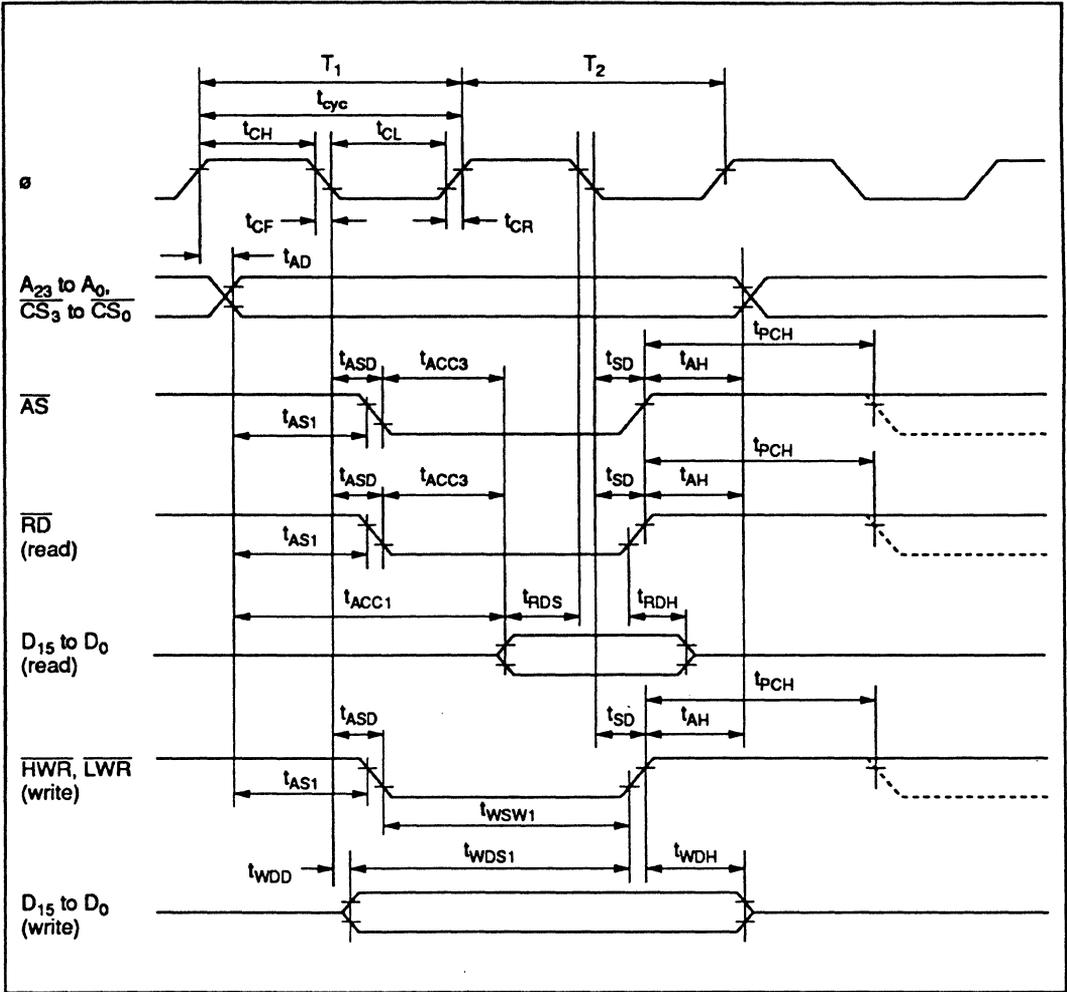
Figure 20-4 Basic Bus Cycle: Two-State Access
