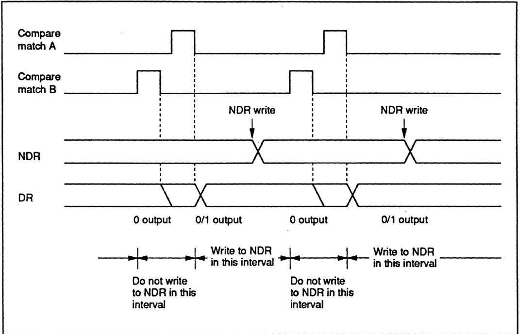
**Figure 11-10 Non-Overlapping Operation and NDR Write Timing**
