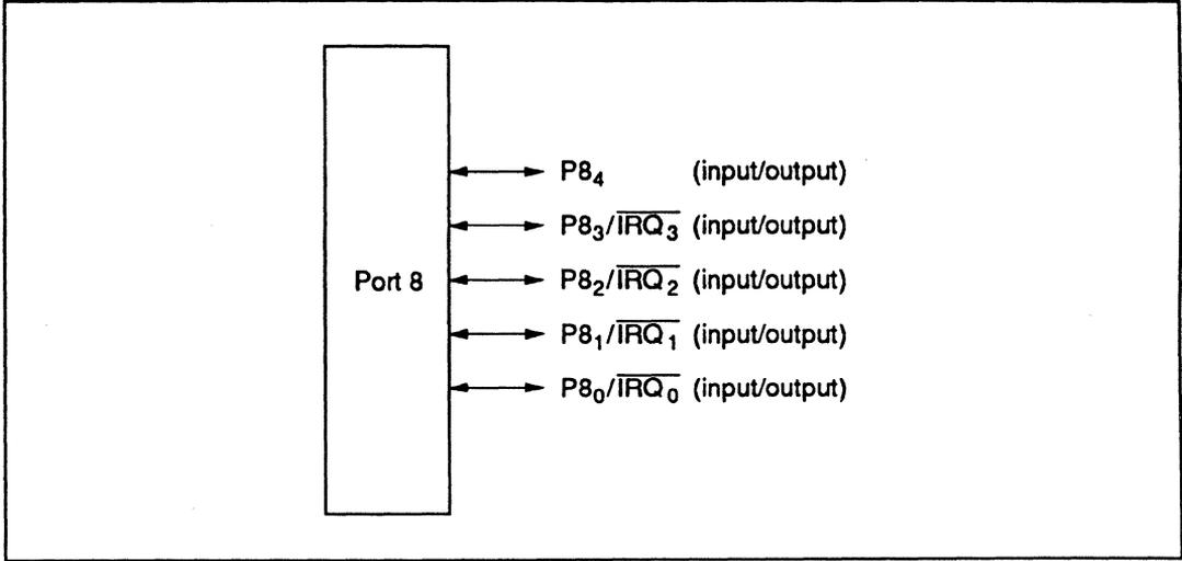
**Figure 9-26 Pin Functions in Modes 6 and 7 (Port 8)**
