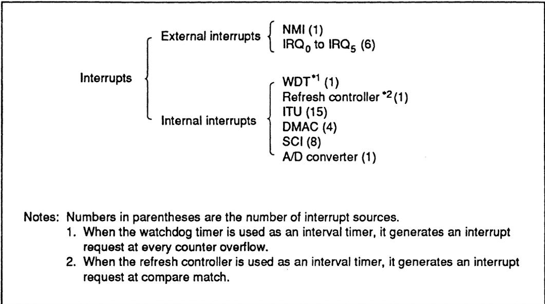
**Figure 4-5 Interrupt Sources and Number of Interrupts**
