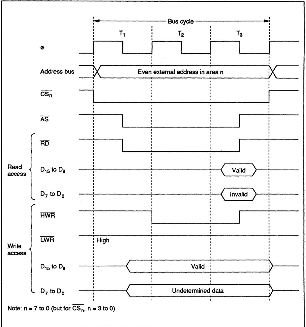
**Figure 6-6 Bus Control Signal Timing for 16-Bit, Three-State-Access Area (1)
