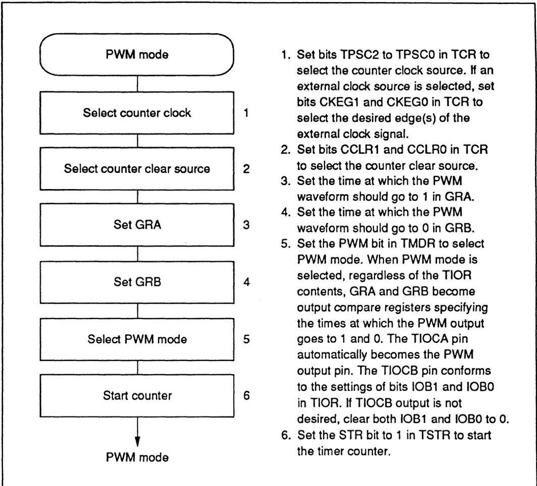
**Figure 10-28 Setup Procedure for PWM Mode (Example)**
