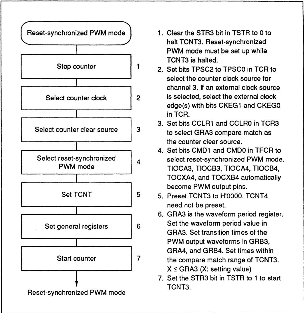
**Figure 10-31 Setup Procedure for Reset-Synchronized PWM Mode (Example)**
