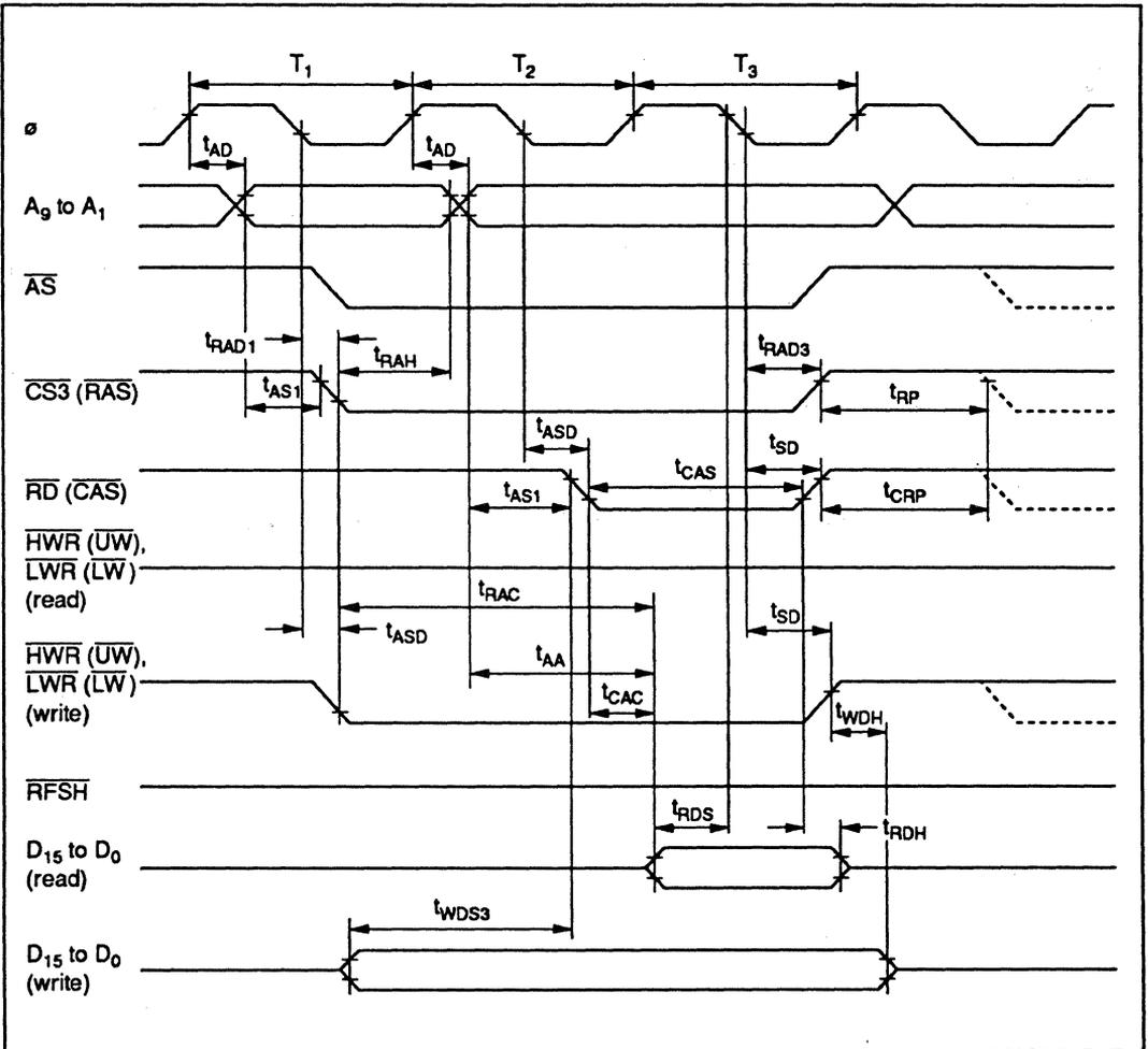
Figure 20-7 DRAM Bus Timing (Read/Write): Three-State Access
