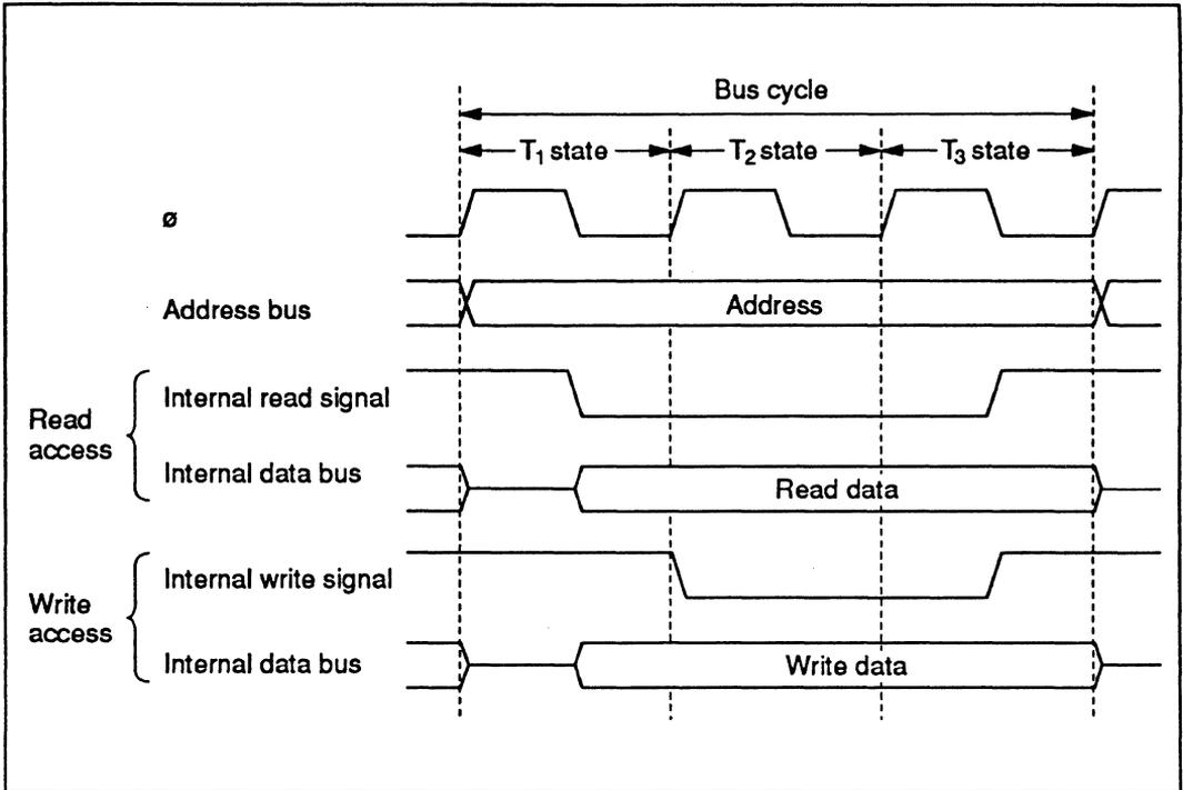
Figure 2-17 Access Cycle for On-Chip Supporting Modules
