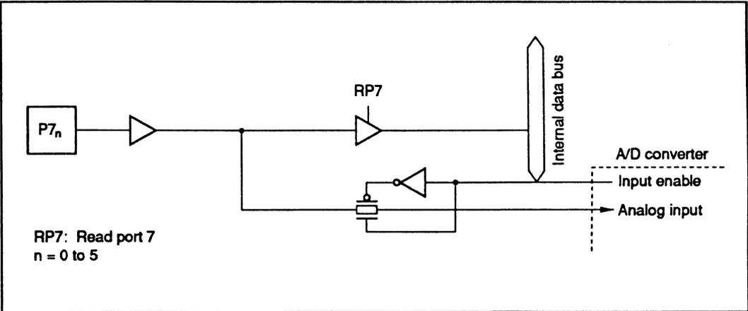
Figure C-7 (a) Port 7 Block Diagram (Pins P7<sub>0</sub> to P7<sub>5</sub>)
