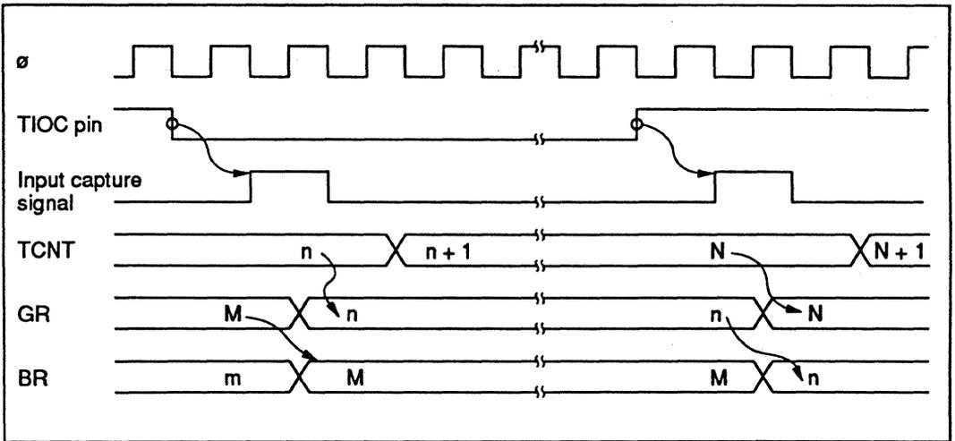
Figure 10-52 Input Capture and Buffer Transfer Timing (Example)
