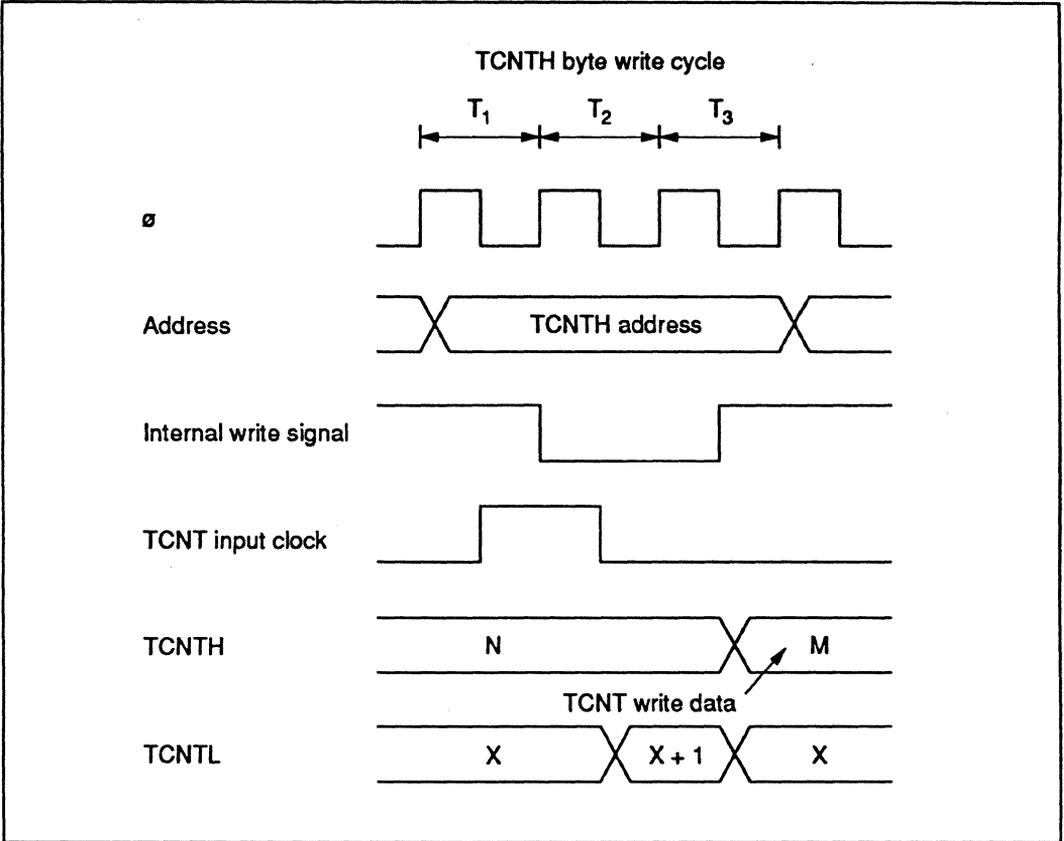
**Figure 10-63** Contention between TCNT Byte Write and Increment
