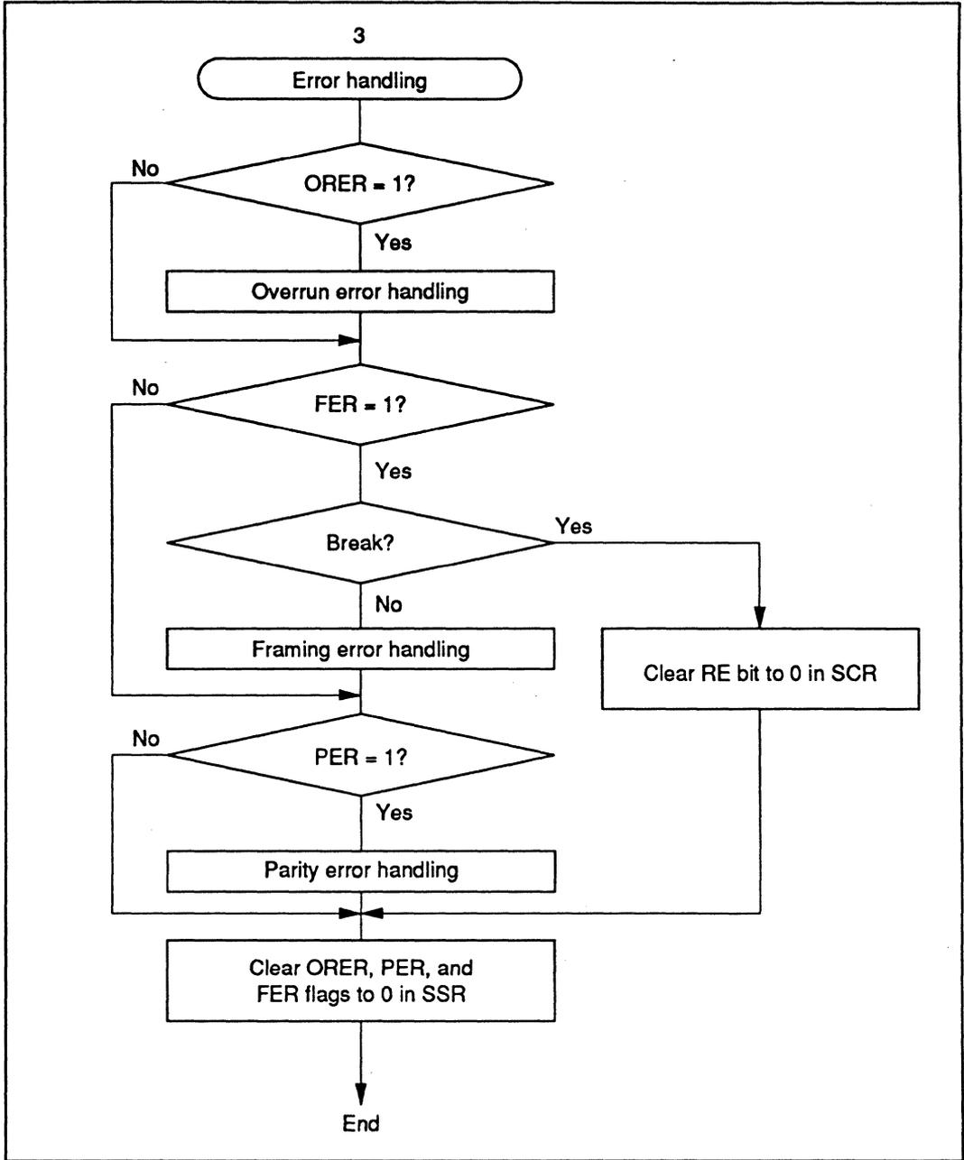
Figure 13-7 Sample Flowchart for Receiving Serial Data (2)
