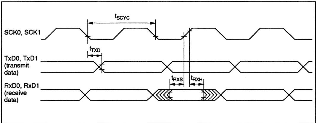
Figure 20-24 SCI Input/Output Timing in Synchronous Mode
