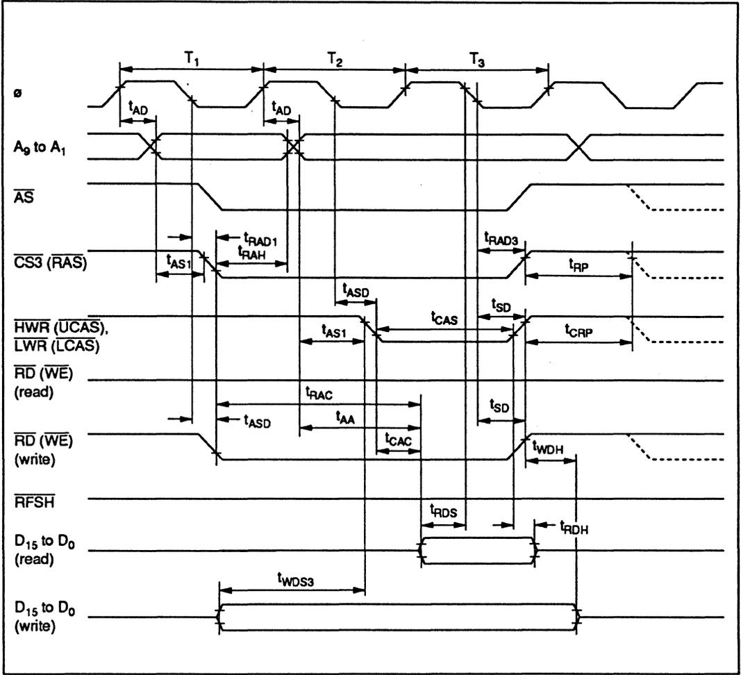
Figure 20-10 DRAM Bus Timing (Read/Write): Three-State Access
