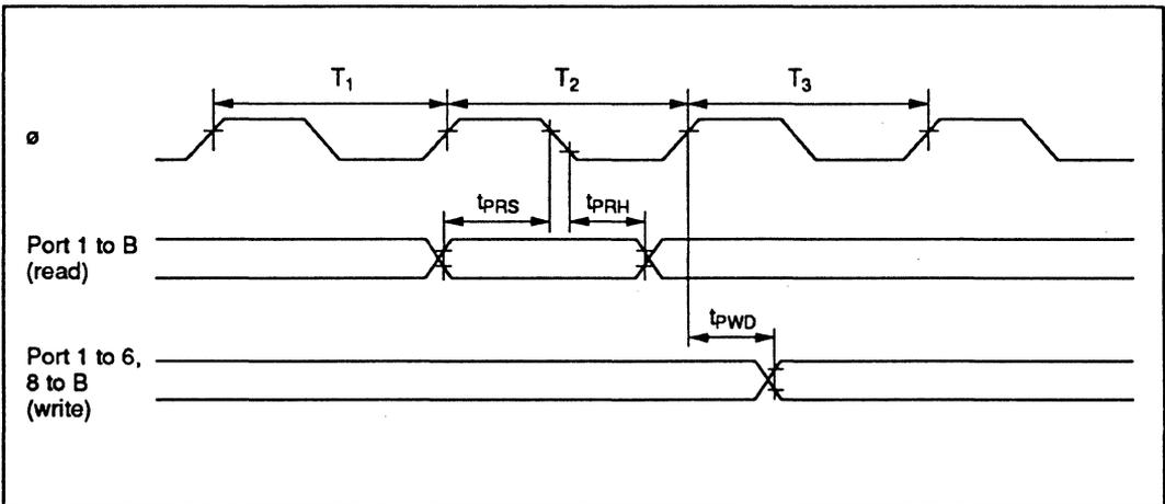
Figure 20-20 TPC and I/O Port Input/Output Timing
