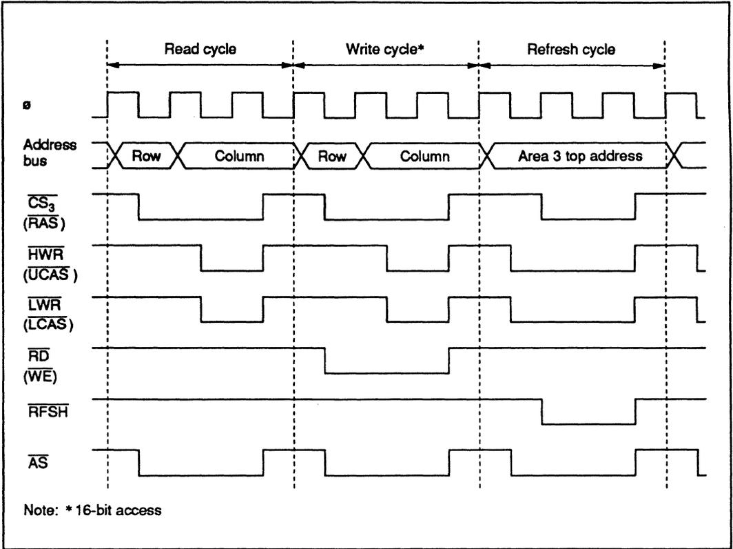
Figure 7-5 DRAM Control Signal Output Timing (2) (2CAS Mode)
