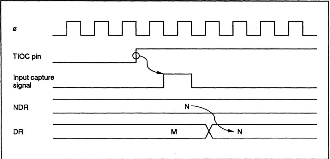
Figure 11-8 TPC Output Triggering by Input Capture (Example)
