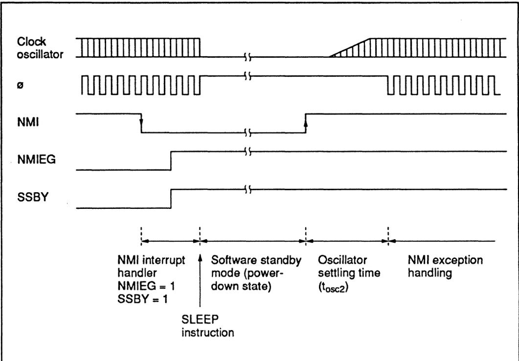
Figure 19-1 NMI Timing for Software Standby Mode (Example)
