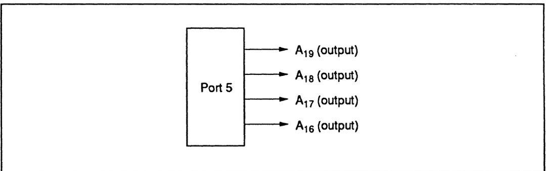
**Figure 9-17 Pin Functions in Modes 1 to 4 (Port 5)**
