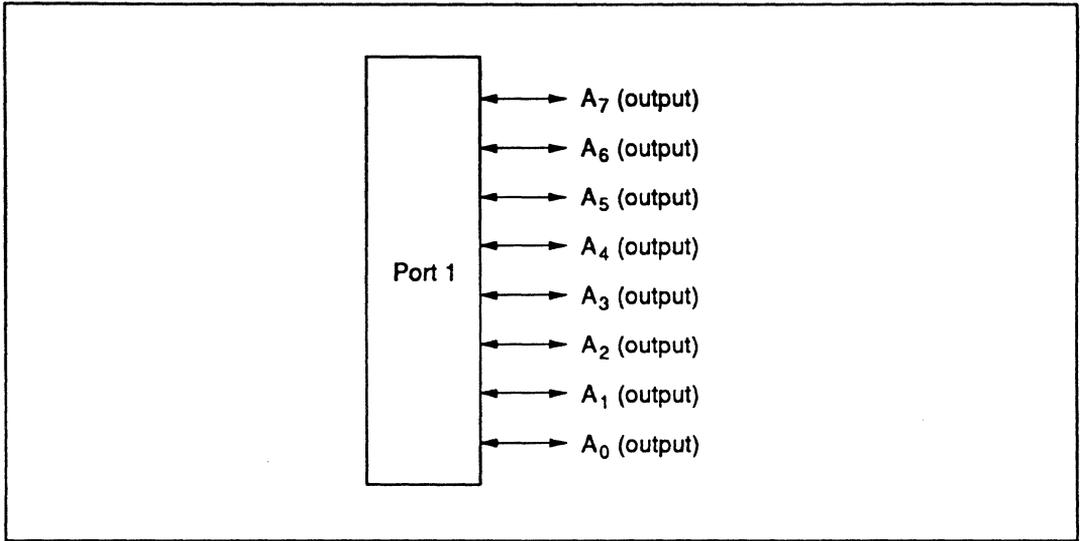
Figure 9-2 Pin Functions in Modes 1 to 4 (Port 1)
