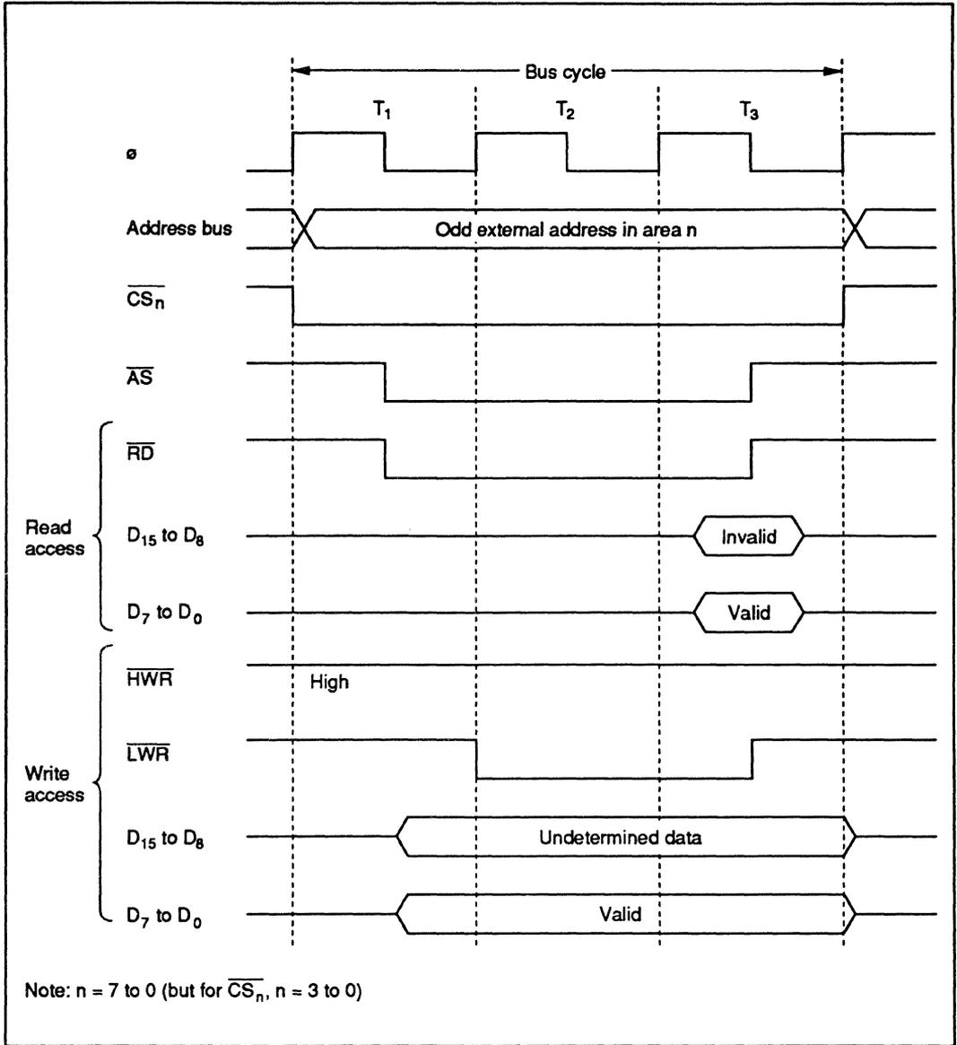
**Figure 6-7 Bus Control Signal Timing for 16-Bit, Three-State-Access Area (2)
