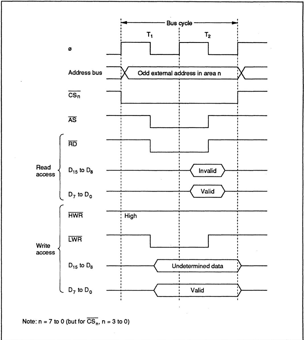
**Figure 6-10 Bus Control Signal Timing for 16-Bit, Two-State-Access Area (2)
