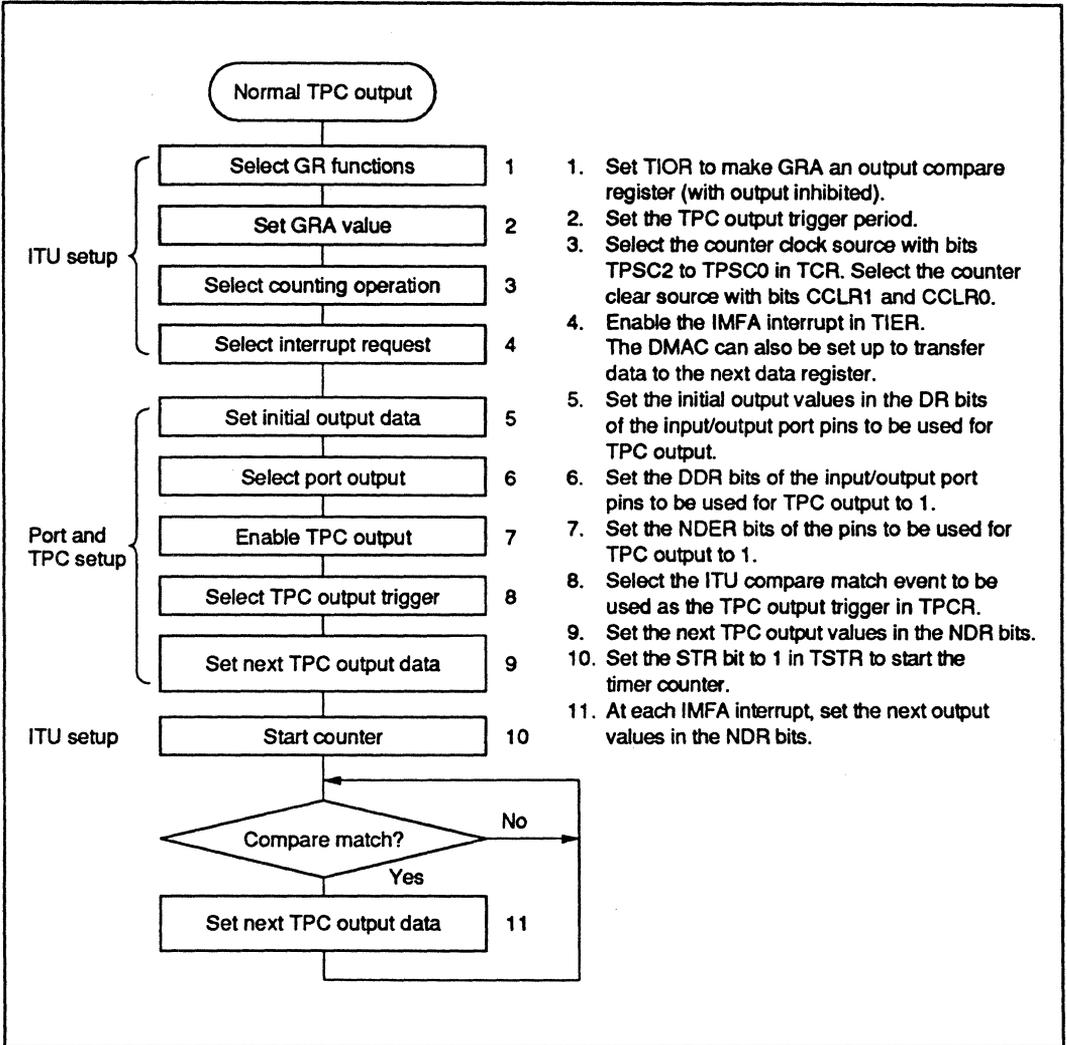
**Figure 11-4 Setup Procedure for Normal TPC Output (Example)**
