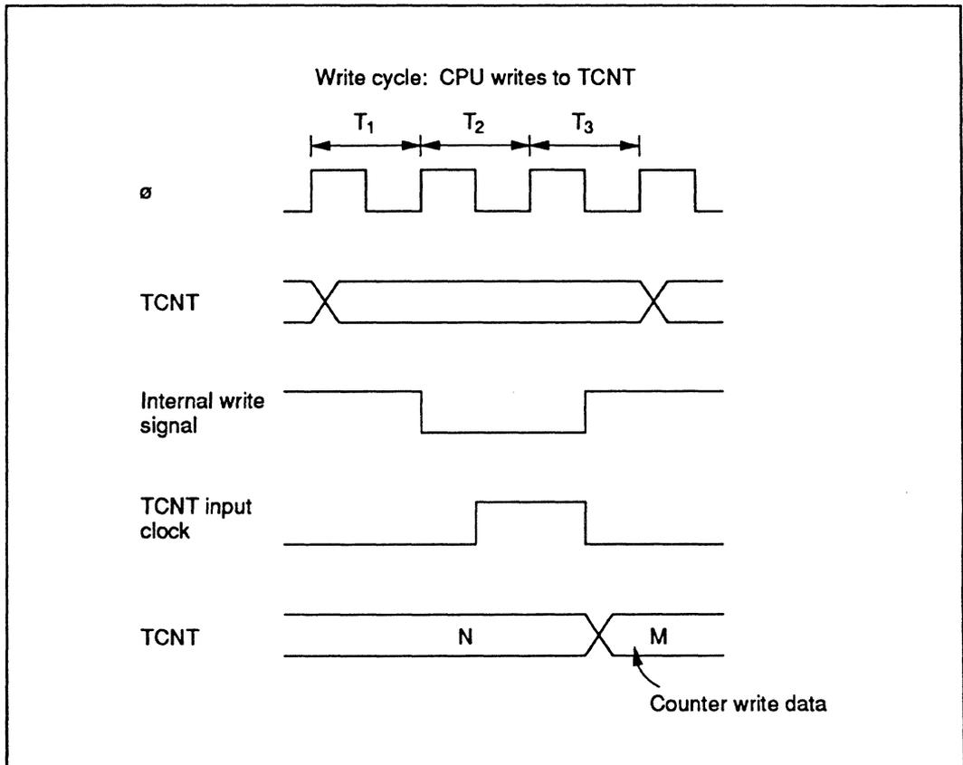
Figure 12-8 Contention between TCNT Write and Increment
