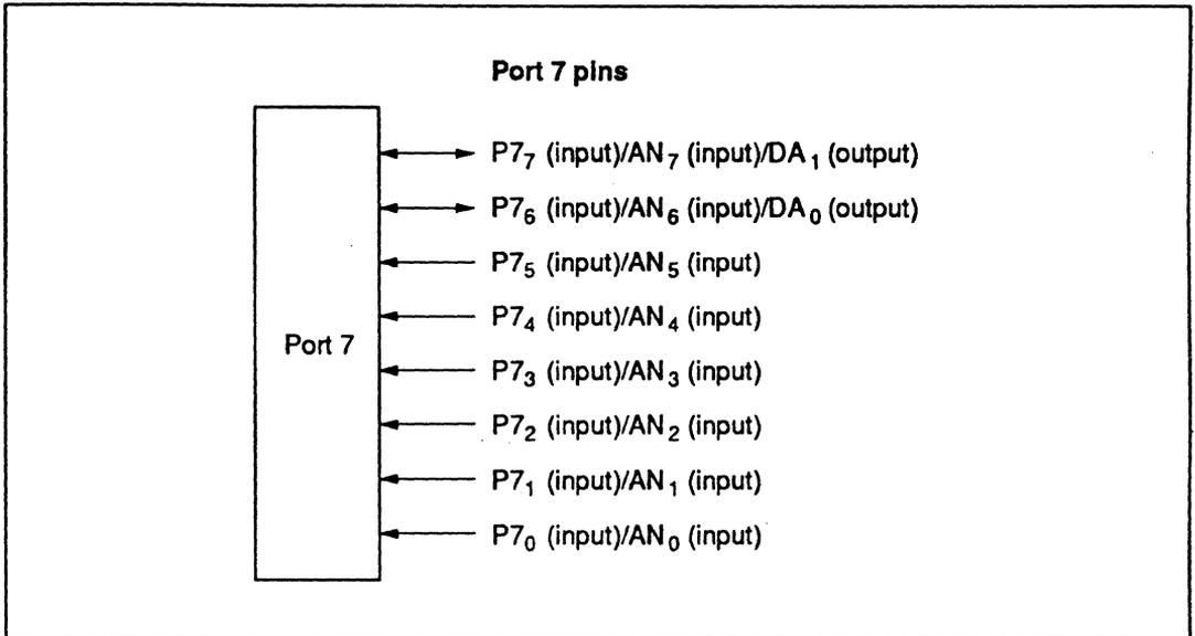
Figure 9-23 Port 7 Pin Configuration
