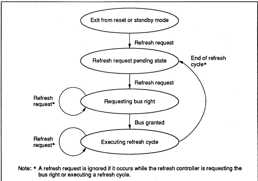
**Figure 7-3 State Transitions for Refresh Cycle Execution**
