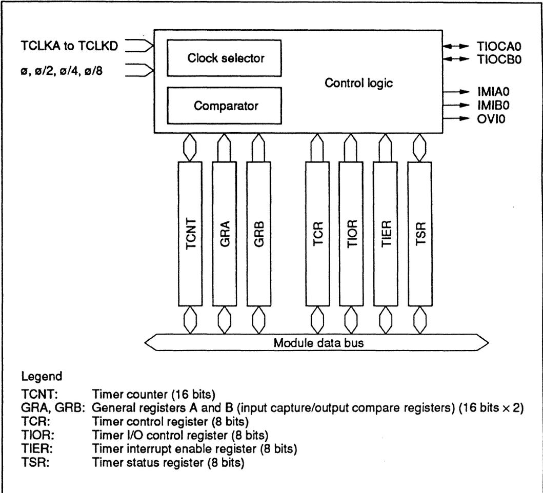
**Figure 10-2 Block Diagram of Channels 0 and 1 (for Channel 0)**
