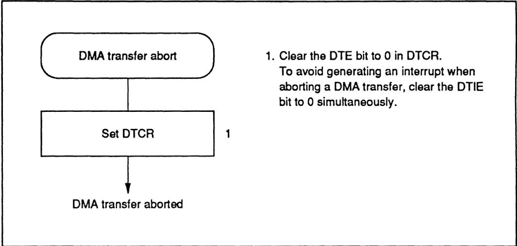
Figure 8-22 Procedure for Aborting a DMA Transfer
