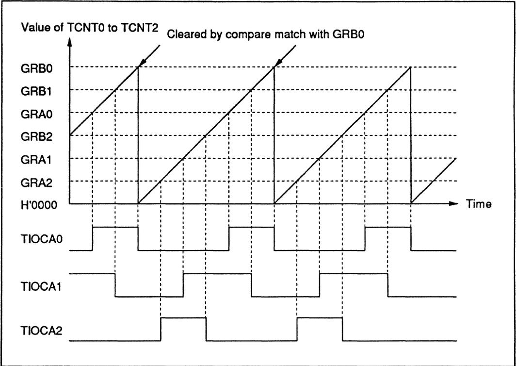
**Figure 10-27 Synchronization (Example)**
