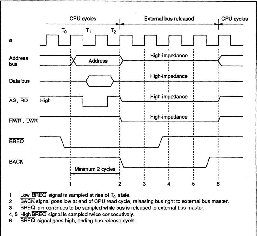
Figure 6-19 External-Bus-Released State (Two-State-Access Area, During Read Cycle)
