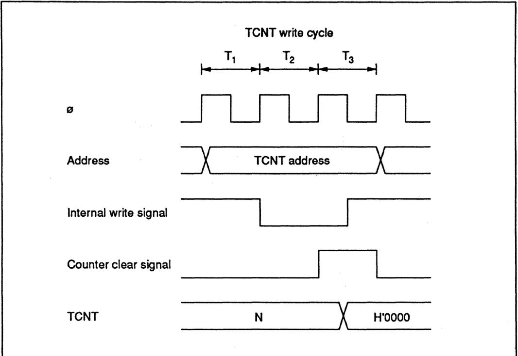
Figure 10-61 Contention between TCNT Write and Clear
