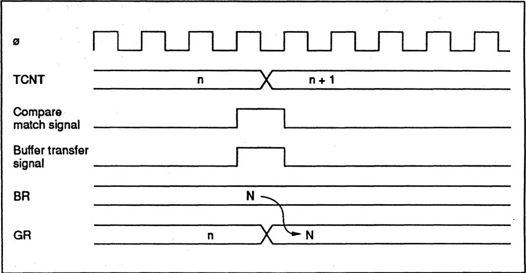
**Figure 10-50 Compare Match and Buffer Transfer Timing (Example)**
