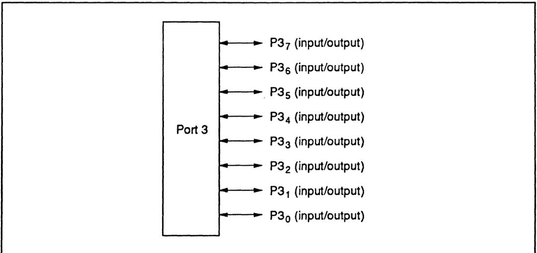
Figure 9-11 Pin Functions in Modes 6 and 7 (Port 3)
