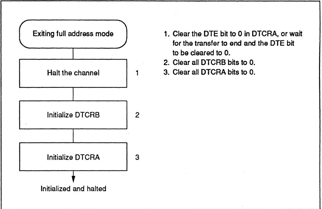
Figure 8-23 Procedure for Exiting Full Address Mode (Example)
