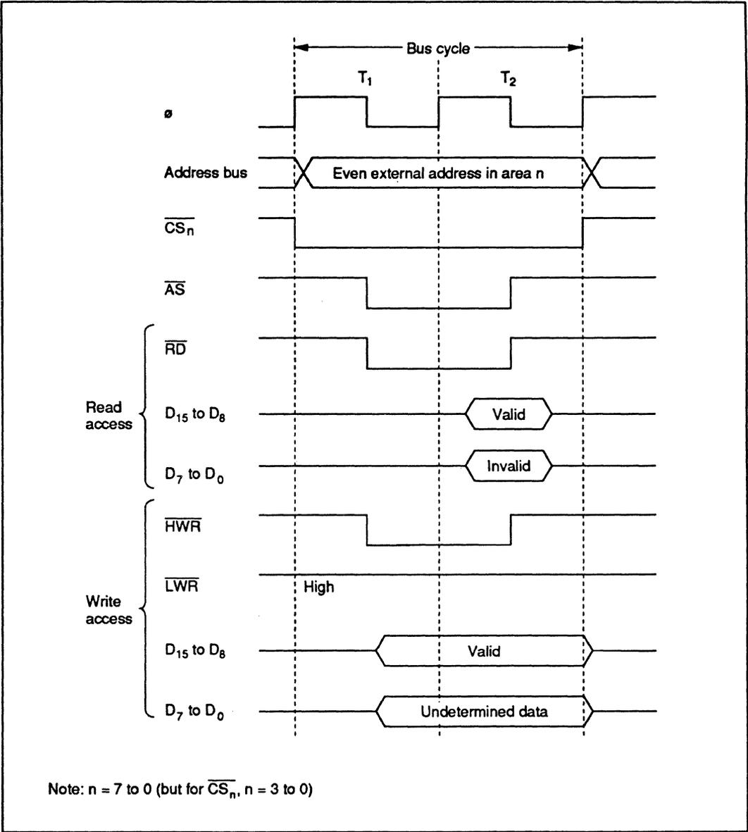
**Figure 6-9 Bus Control Signal Timing for 16-Bit, Two-State-Access Area (1)**
