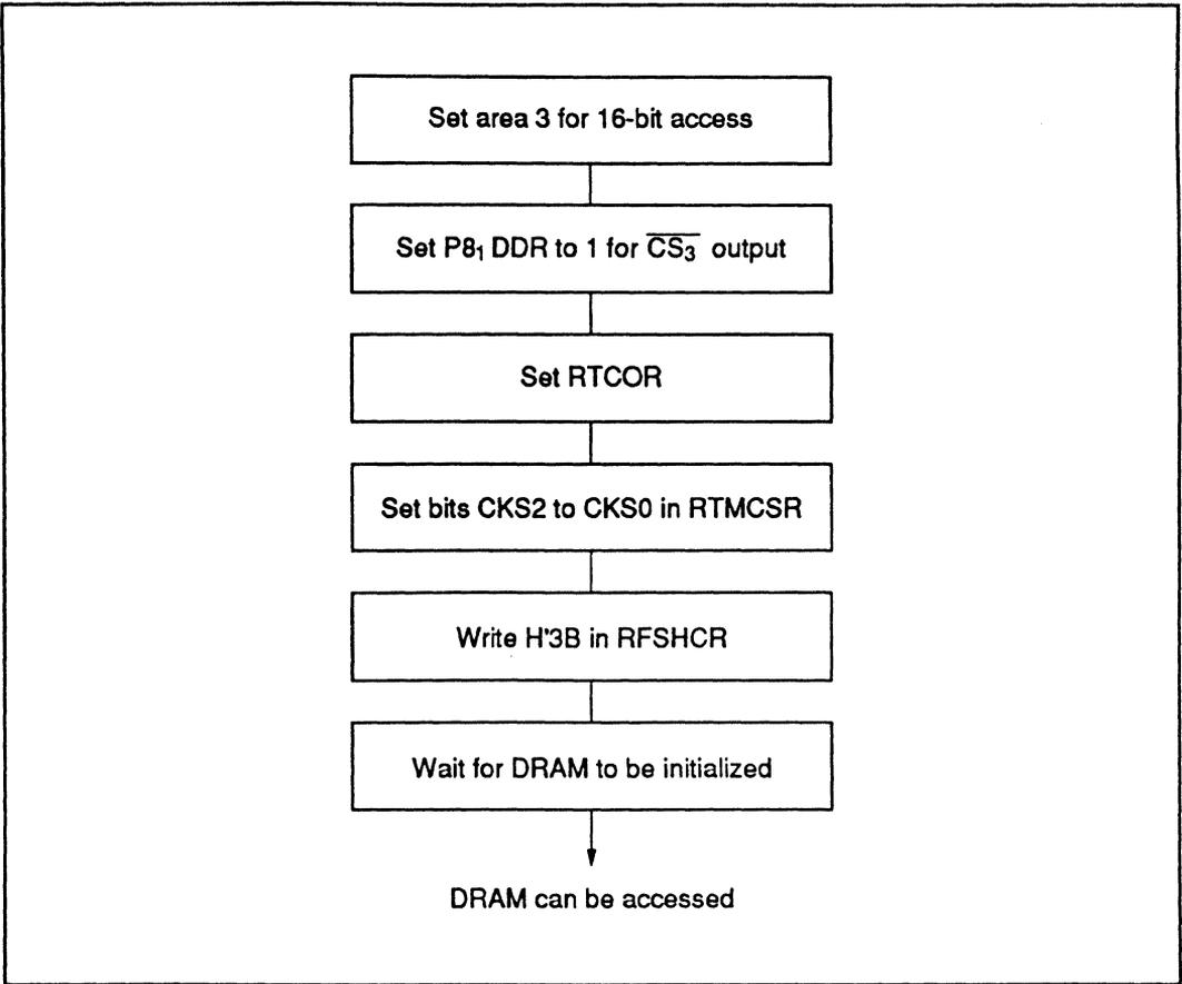
**Figure 7-12 Setup Procedure for  $\overline{2CAS}$  4-Mbit DRAM with 9-Bit Row Address and 9-Bit Column Address (16-Mbyte Mode)**
