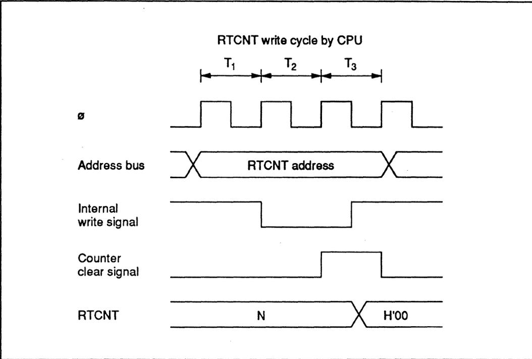
**Figure 7-20** Contention between RTCNT Write and Clear
