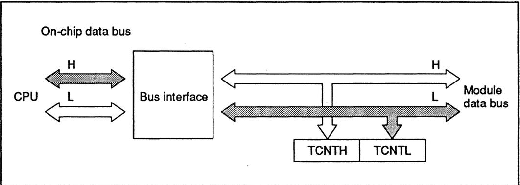
**Figure 10-9 Access to Timer Counter (CPU Writes to TCNT, Lower Byte)**
