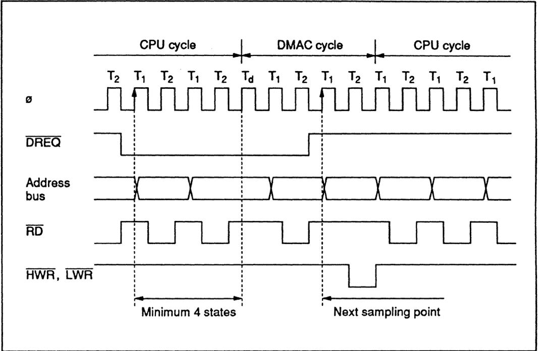
**Figure 8-17 Timing of DMAC Activation by Low  $\overline{DREQ}$  Level in Normal Mode**
