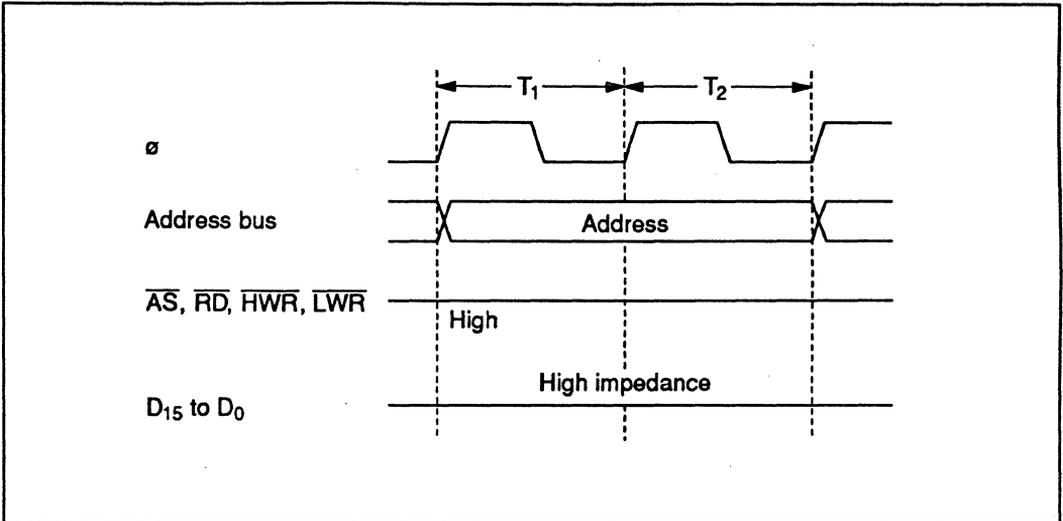
**Figure 2-16 Pin States during On-Chip Memory Access**
