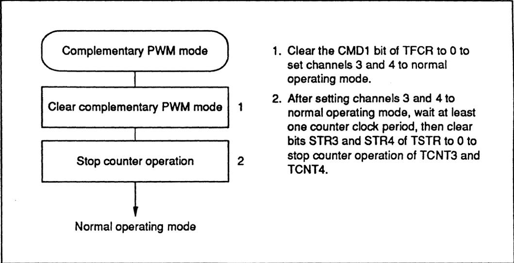
**Figure 10-34 Clearing Procedure for Complementary PWM Mode**
