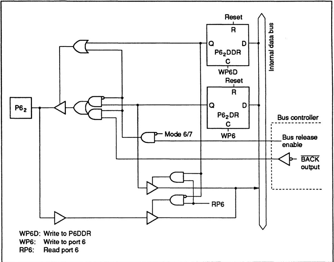
Figure C-6 (c) Port 6 Block Diagram (Pin P6<sub>2</sub>)
