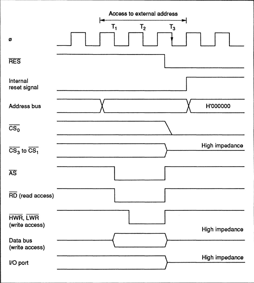
Figure D-3 Reset during Memory Access (Reset during T<sub>3</sub> State)
