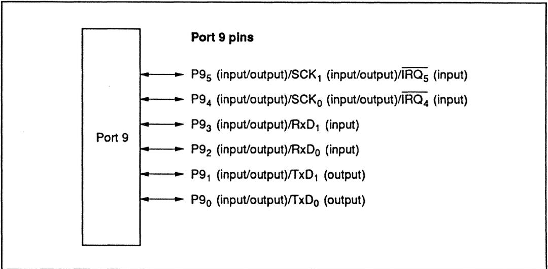
Figure 9-27 Port 9 Pin Configuration
