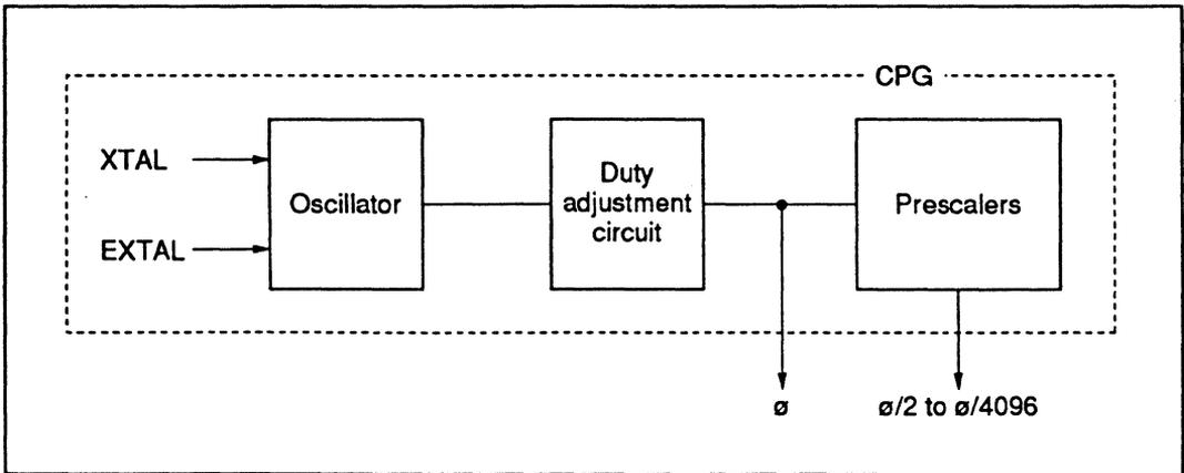
Figure 18-1 Block Diagram of Clock Pulse Generator
