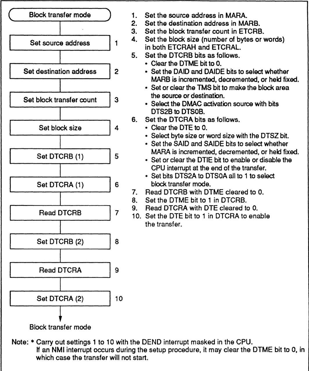
Figure 8-12 Block Transfer Mode Setup Procedure (Example)
