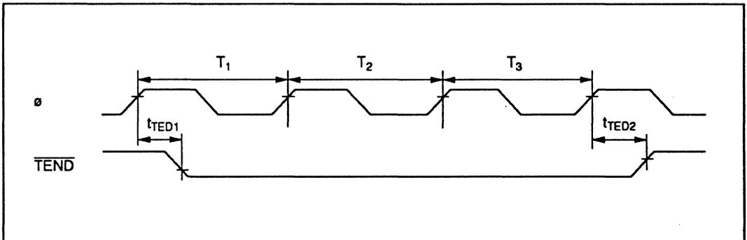
Figure 20-26 DMAC  $\overline{TEND}$  Output Timing for 3 State Access
