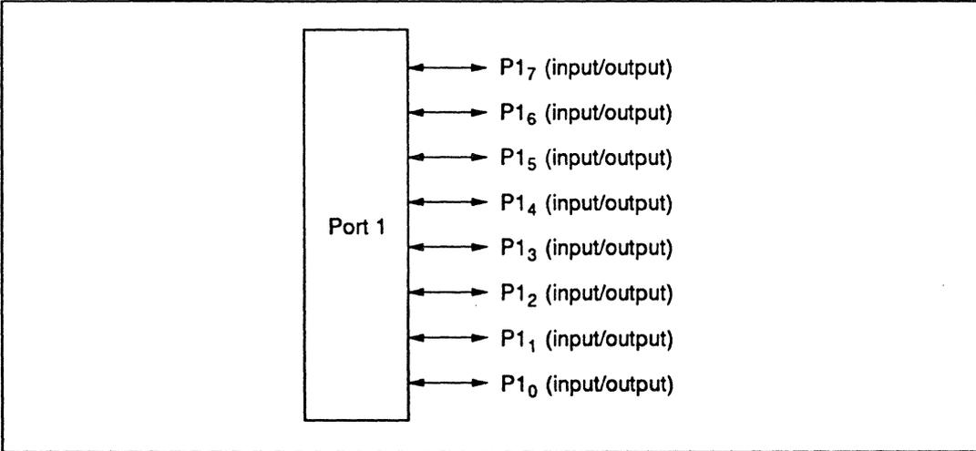
Figure 9-4 Pin Functions in Modes 6 and 7 (Port 1)
