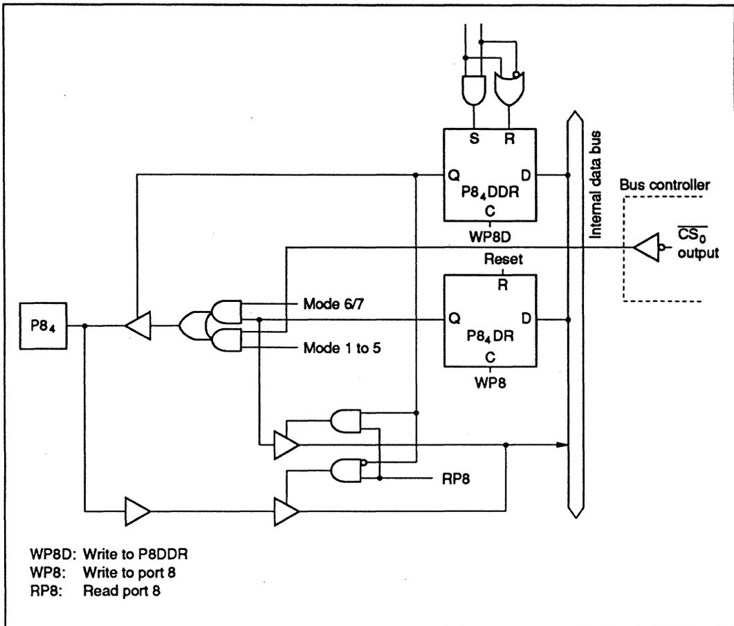
Figure C-8 (c) Port 8 Block Diagram (Pin P8<sub>4</sub>)
