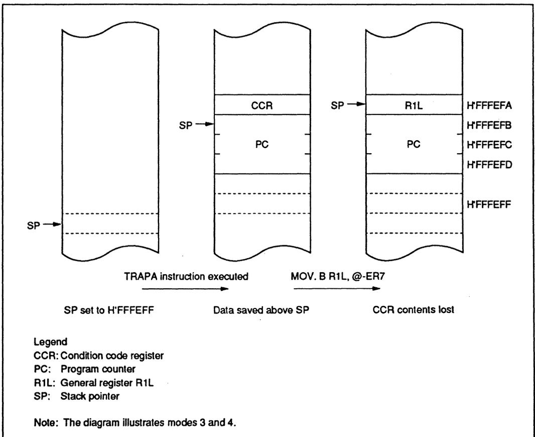
Figure 4-7 Operation when SP Value is Odd
