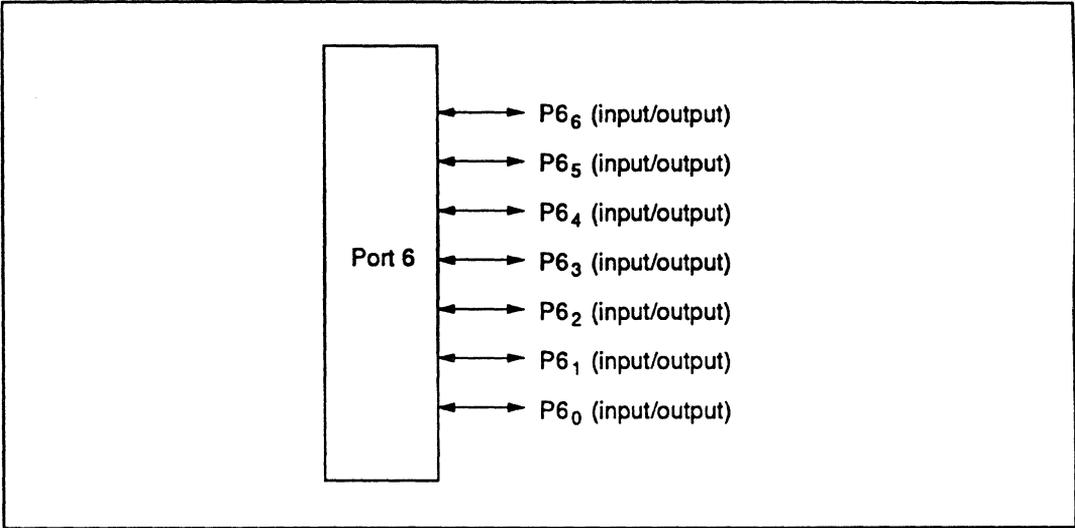
**Figure 9-22 Pin Functions in Modes 6 and 7 (Port 6)**
