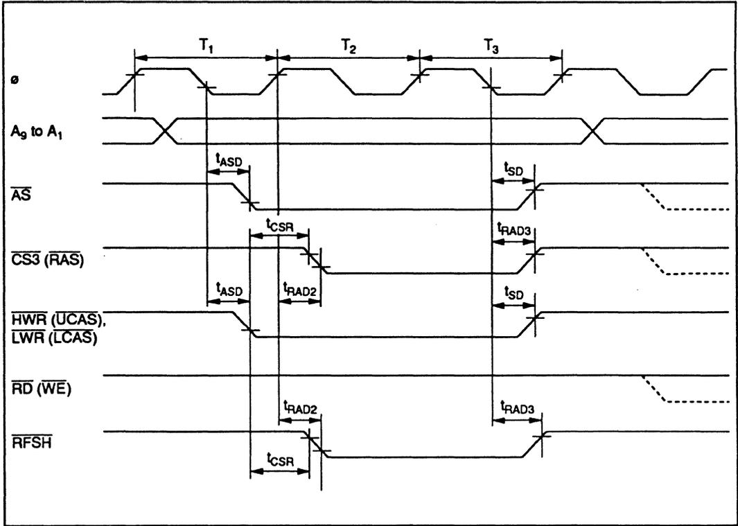
Figure 20-11 DRAM Bus Timing (Refresh Cycle): Three-State Access
