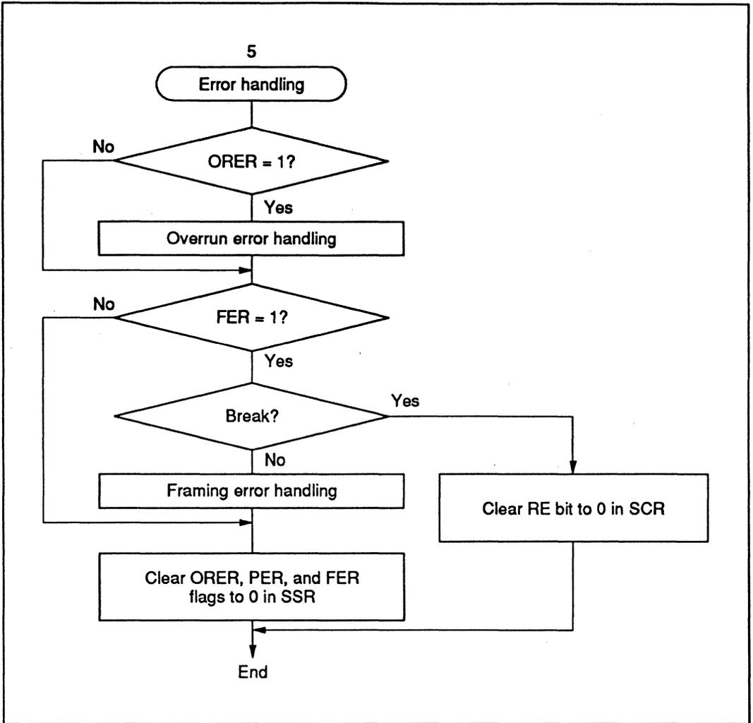
Figure 13-12 Sample Flowchart for Receiving Multiprocessor Serial Data (2)
