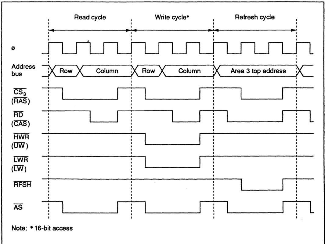
**Figure 7-5 DRAM Control Signal Output Timing (1) (2WE Mode)**
