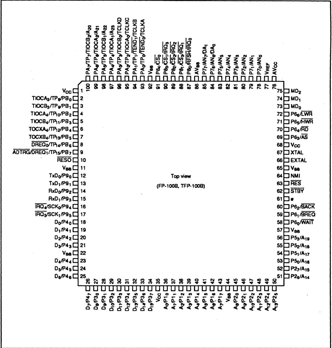
Figure 1-2 Pin Arrangement (FP-100B or TFP-100B, Top View)
