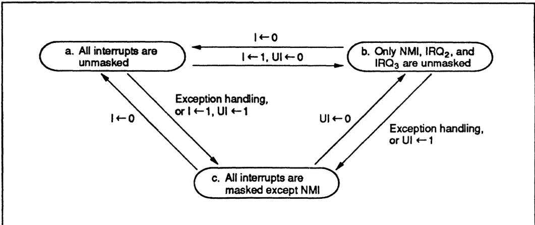
Figure 5-5 Interrupt Masking State Transitions (Example)
