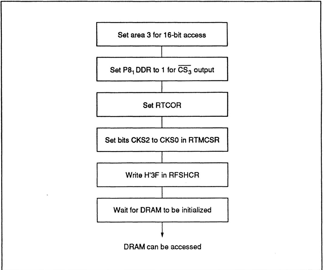
**Figure 7-14 Setup Procedure for Multiple  $2\overline{C\overline{A}S}$  4-Mbit DRAM Chips with 9-Bit Row Address and 9-Bit Column Address (16-Mbyte Mode)**
