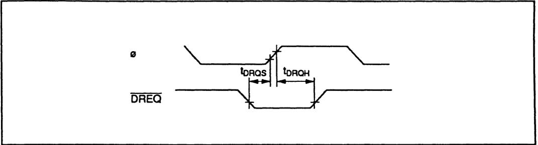
**Figure 20-27 DMAC  $\overline{DREQ}$  Input Timing**
