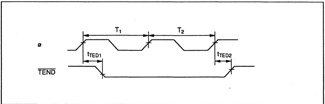
Figure 20-25 DMAC  $\overline{TEND}$  Output Timing for 2 State Access
