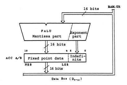
Fig. 5-1 Accumulator Input/Output Data
