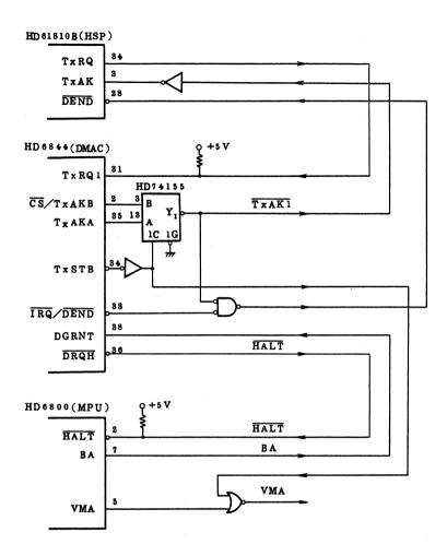
Fig. 6-6 Example of Connection between HSP and DMAC
