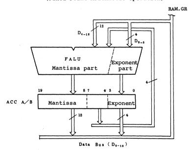
Fig. 5-2 Accumulator Input/Output Data (Floating Point Arithmetic Operation)
