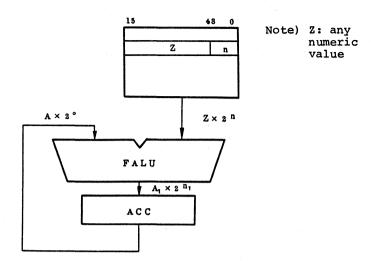
Fig. 3-6 Data Format Transformation Operation (From Fixed Point to Floating Point)
