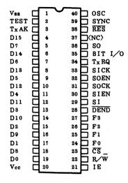
Fig. 2-1 Pin Arrangement (Top View)
