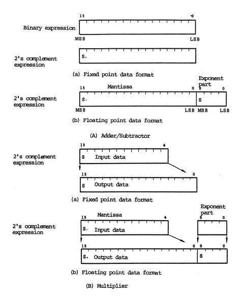
Fig. 3-2 Data Format of Operational Circuit
