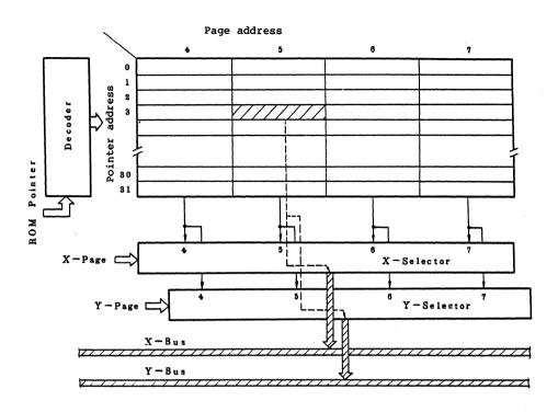
Fig. 4-4 Data ROM Access Method (Pointer Addressing Mode)
