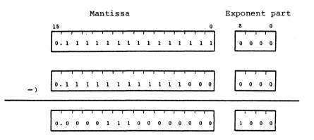
Fig. 3-4 Operation during Underflow
