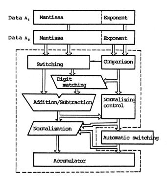
Fig. 3-3 Floating Point Adder/Subtractor Circuit
