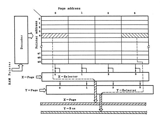
Fig. 4-3 Data RAM Access Method (Pointer Addressing Mode)
