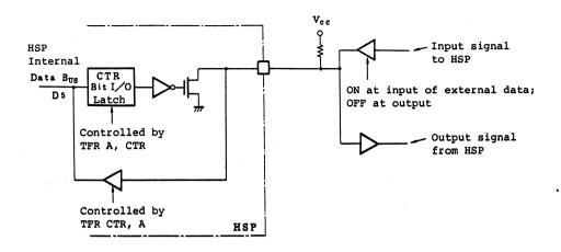
Fig. 6-7 Bit I/O Usage
