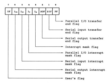
Fig. 5-5 Status Register Functions
