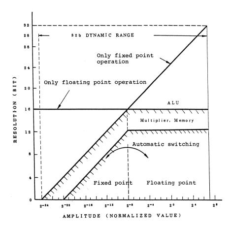
Fig. 3-1 Operation Accuracy of Signal Processing Application System
