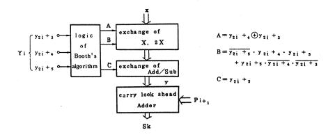
Fig. 3-8 Basic Multiplier Block Diagram
