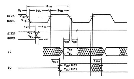
Fig. 9-2 Serial Input/Output Waveform
