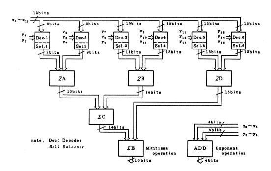
Fig. 3-9 Floating Point Multiplier Block Diagram
