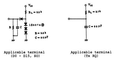
Fig. 9-5 Load Circuit (for Timing Test)
