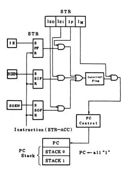
Fig. 6-4 Interrupt Circuit Configuration
