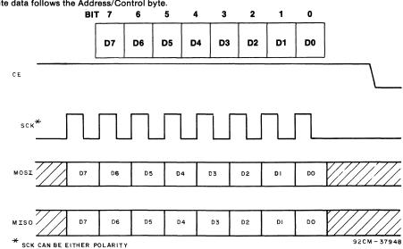
Fig. 10 - Read/Write data-transfer waveforms.
