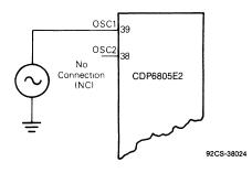
Fig. 10 - External clock connection.
