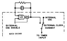
Fig. 14 - External Timer Oscillator Controls
