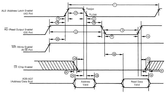
Fig. 3 — Bus-read timing competitor multiplexed bus.
