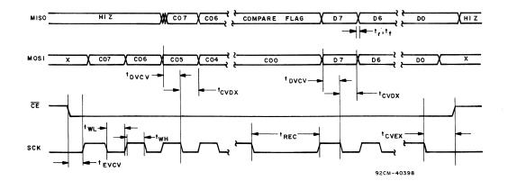
Fig. 8 - Write cycle timing waveforms.
