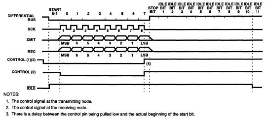
4. If the control pin is again puled low before the end of the stop bit, then the next start bit will begin at the end of the previous stop bit. FIGURE 3. SCK, CONTROL, AND IDLE SIGNALS DURING THE SPI MODE OF OPERATION
