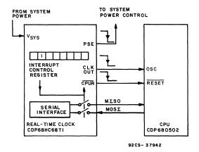
Fig. 4 - Power-down functional diagram.
