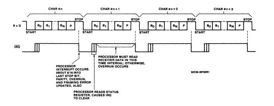
Fig. 9 - Continuous data receive.
