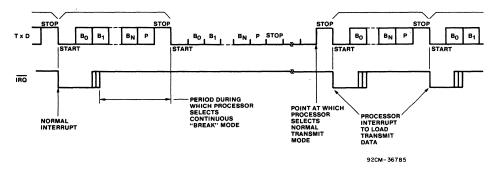
Fig. 18 - Transmit continuous "BREAK".
