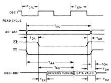
FIGURE 3. CONTROL TIMING DIAGRAM FOR THE CDP68EM05D2 EMULATOR.
