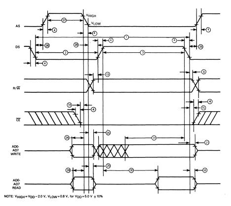
Fig. 2 — CDP6818 bus timing waveforms.
