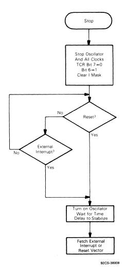
Fig. 16 - Stop function flowchart.
