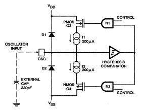
FIGURE 8. EQUIVALENT CIRCUIT FOR OSCILLATOR INPUT
