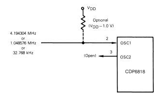
Fig. 10 — External Time-base connection.
