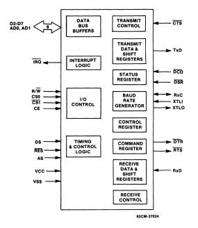
Fig. 1 - CDP6853 interface diagram.
