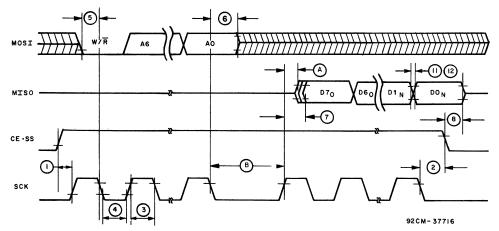
Fig. 8 - READ cycle timing waveforms.
