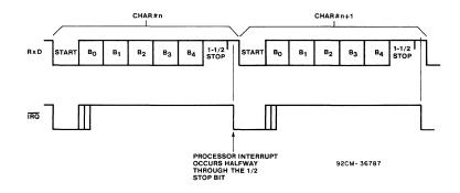
Fig. 17 - Timing with 1-1/2 stop bits.
