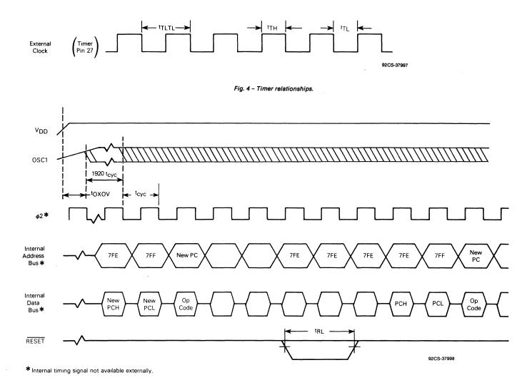
Fig. 5 – Power-on RESET and RESET.
