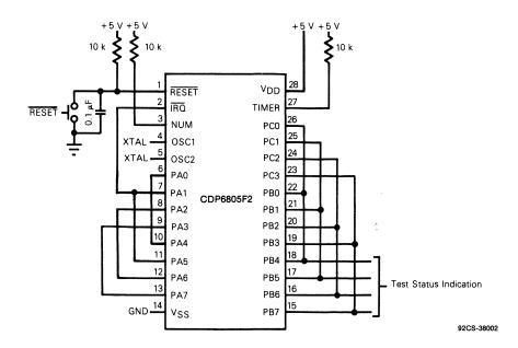
Fig. 10 - Self-check pinout configuration.
