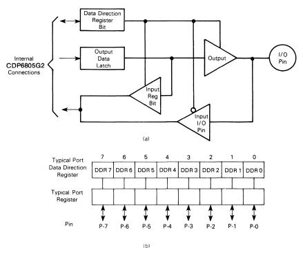
Fig. 9 – Typical port I/O circuitry.
