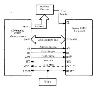
Fig. 20 - Connection to CMOS peripherals.
