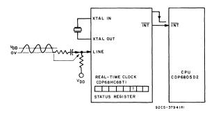
Fig. 3 - Power-sensing functional diagram.
