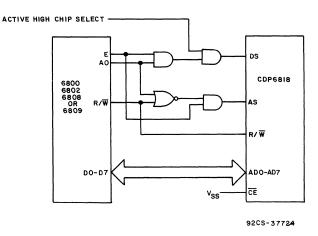
Fig. 21 — CDP6818 interfaced with Motorola type processors
