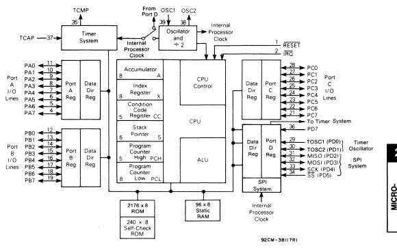
Fig. 1 — CDP68HC05D2 CMOS microcomputer block diagram.
