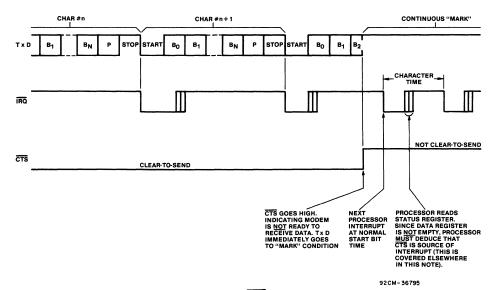
Fig. 11 - Effect of CTS on transmitter.
