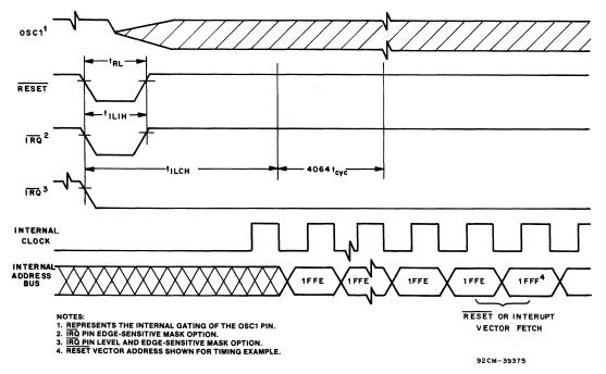
Fig. 25 - Stop Recovery Timing Diagram
