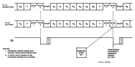
Fig. 16 - Framing error.
