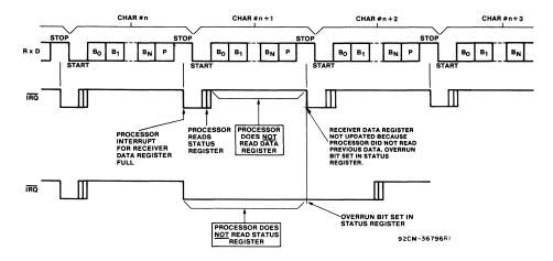
Fig. 11 - Effect of overrun on receiver.
