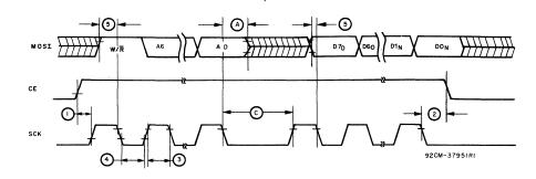
Fig. 14 - WRITE-cycle timing waveforms.
