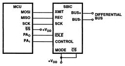
FIGURE 11. USING THE BUFFERED SPI MODE
