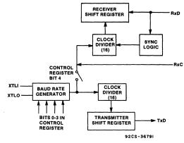
Fig. 6 - Transmitter receiver clock circuits.
