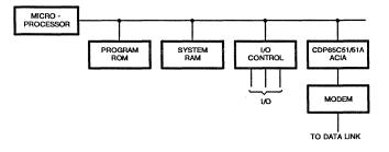
Fig. 20 - Simplified system diagram.
