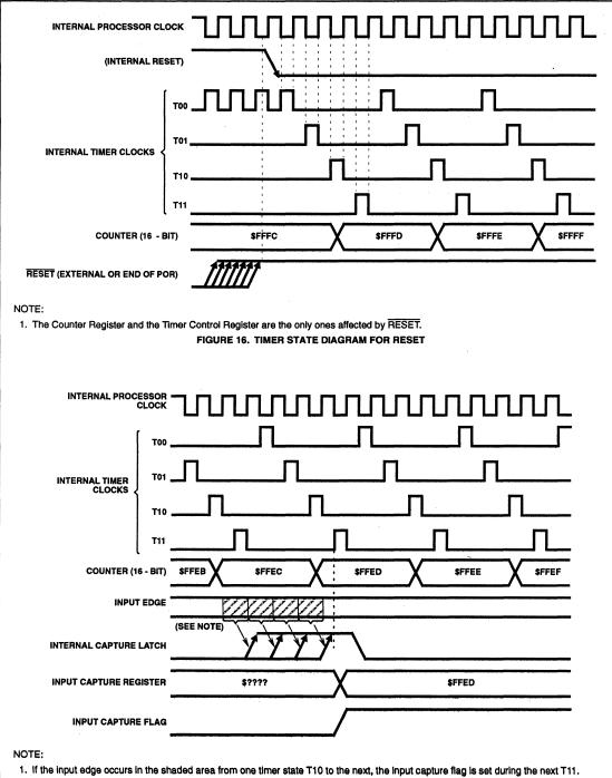
FIGURE 17. TIMER STATE DIAGRAM FOR INPUT CAPTURE
