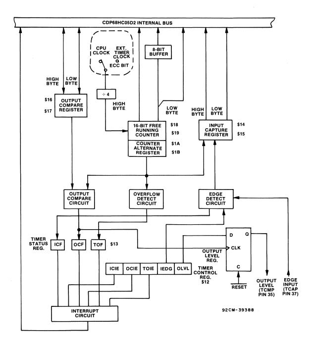
Fig. 15 - Programmable Timer Block Diagram
