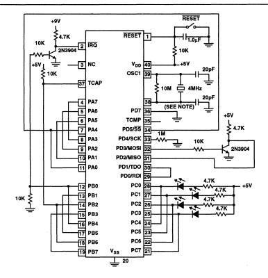
FIGURE 10. SELF-CHECK CIRCUIT SCHEMATIC DIAGRAM
