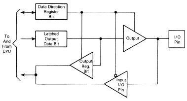
Fig. 8 - Typical port I/O circuitry.
