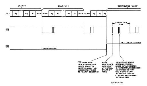
Fig. 10 - Effect of CTS on CDP65C51 transmitter
