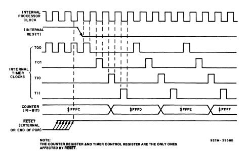
Fig. 16 - Timer State Timing Diagram For Reset
