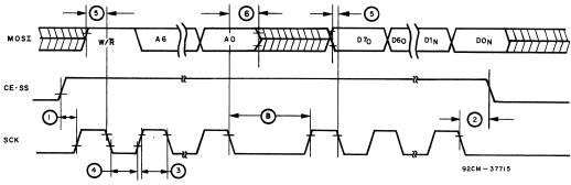
Fig. 7 - WRITE cycle timing waveforms.
