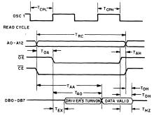
FIGURE 3. CONTROL TIMING DIAGRAM FOR THE CDP68EM05C4 EMULATOR.
