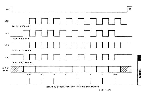
Fig. 21 - Data Clock Timing Diagram
