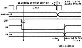
Fig. 4 - Receiver timing waveforms.
