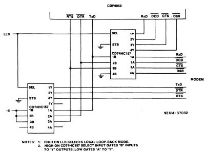
Fig. 22 - Loop-back circuit schematic.
