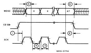
Fig. 6 - Page/Device byte timing waveforms.
