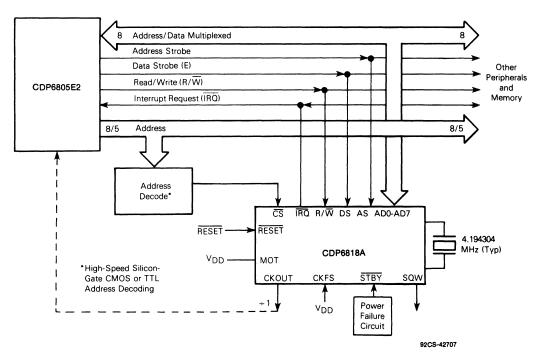
Fig. 16 - CDP6818A interfaced with Motorola compatible multiplexed bus microprocessors.
