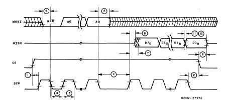
Fig. 15 - READ-cycle timing waveforms.
