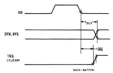
Fig. 26 - Transmit-timing waveforms with external clock.
