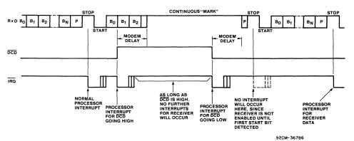
Fig. 17 - Effect of DCD on receiver.
