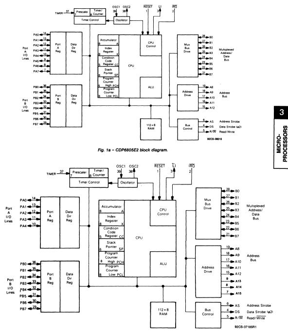
Fig. 1b - CDP6805E3 block diagram.
