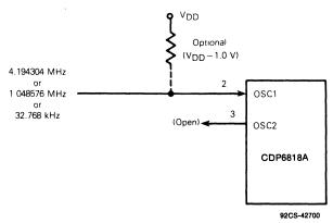
Fig. 9 - External time-base connection.
