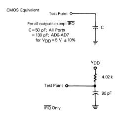
Fig. 2 - Equivalent test loads.
