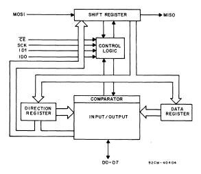
Fig. 1 - Single port I/O block diagram.
