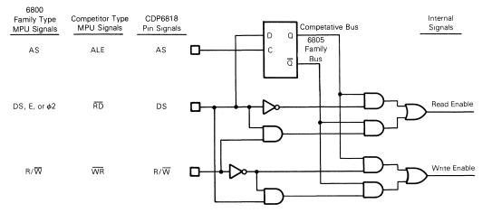
Fig. 9 — Functional diagram of MOTEL circuit.
