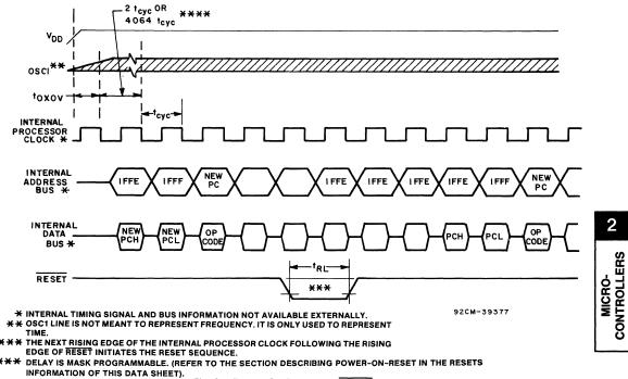
Fig. 8 - Power-On Reset and RESET
