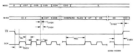
Fig. 9 - Read cycle timing waveforms.
