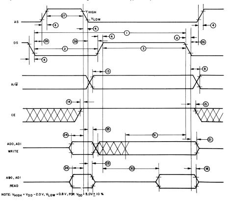
Fig. 23 - Bus timing waveforms of CDP6853.
