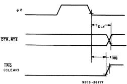
Fig. 24 - Interrupt and output timing waveforms.
