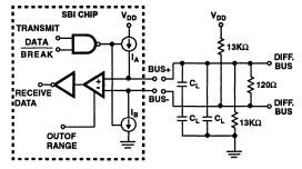
FIGURE 4. DIFFERENTIAL DRIVER/RECEIVER
