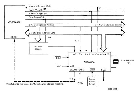
Fig. 18 - CDP6818A interfaced with CDP6805E2 CMOS multiplexed microprocessor with slow addressing decoding.
