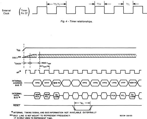
Fig. 5 - Power-on RESET and RESET.
