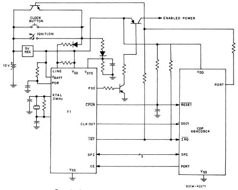
Example of an automotive system. The V<sub>SYS</sub> and LINE inputs can be used to sense the ignition turning on and off. An external switch is included to activate the system without turning on the ignition. Also, the CMOS CPU is not powered down with the system V<sub>DD</sub>, but is held in a low power reset mode during power down. When restoring power the CDP68HC68T1 will enable the CLK OUT pin and set the PSE and CPUR high.
