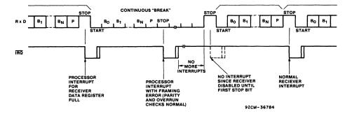
Fig. 19 - Receive continuous "BREAK".
