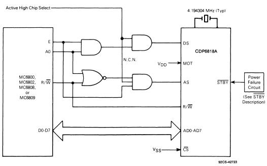
Fig. 20 - CDP6818A interfaced with Motorola Processors.
