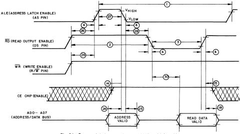
Fig. 24 - Bus-read timing waveforms of 8085 multiplexed bus.
