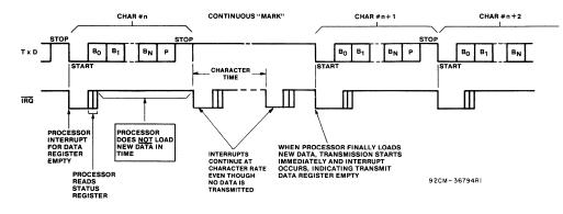
Fig. 9 - Transmit data register not loaded by processor.
