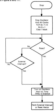
Fig. 17 - Stop function flowchart
