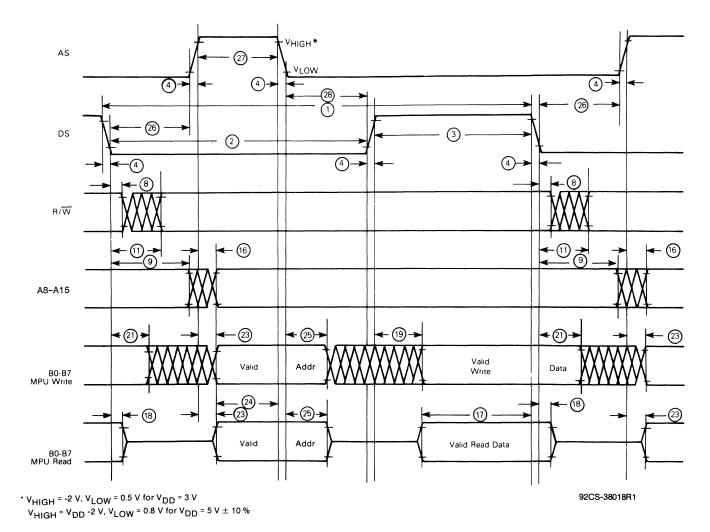
Fig. 4 – Bus timing waveforms.
