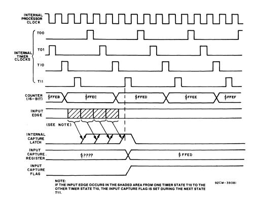
Fig. 17 - Timer State Timing Diagram For Input Capture
