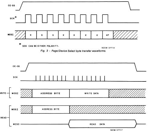
Fig. 4 - Single-byte transfer.
