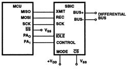
FIGURE 10. USING THE SPI MODE
