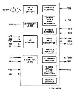
Fig. 1 - CDP65C51/51A interface diagram
