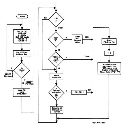
Fig. 14 - RESET and INTERRUPT processing flowchart.
