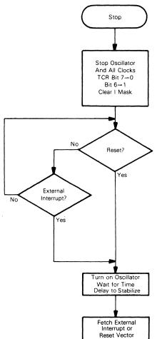
Fig. 16 - Stop function flowchart.
