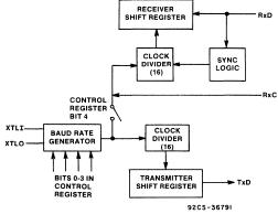
Fig. 7 - Transmitter receiver clock circuits.
