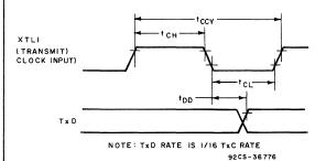
Fig. 23 - Transmit timing waveforms with external clock.
