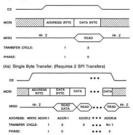
(4b) Multiple (N) byte Transfer. (Efficient Device Communication Requiring N+1 SPI Transfers)
