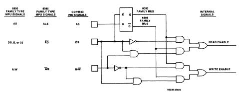
Fig. 2 – Functional diagram of MOTEL circuit.
