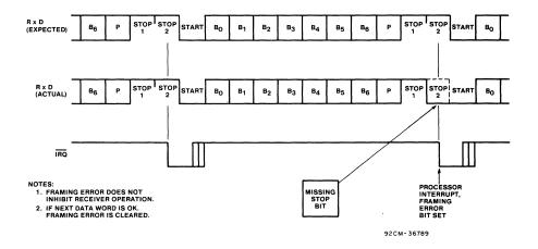
Fig. 15 - Framing error.
