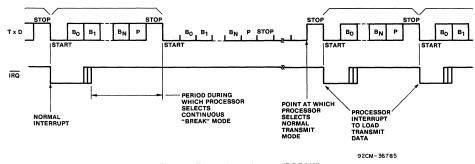
Fig. 19 - Transmit continuous "BREAK".
