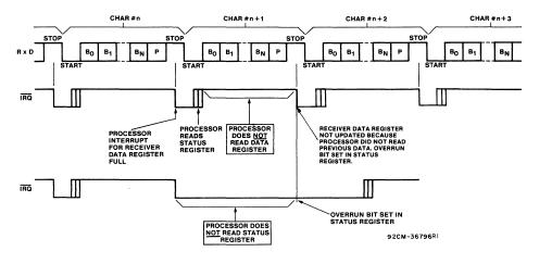
Fig. 12 - Effect of overrun on receiver.
