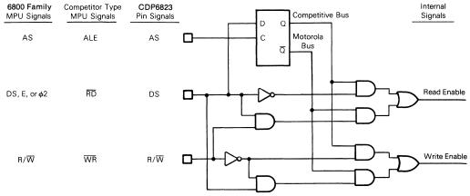
Fig. 7 - Functional diagram of MOTEL circuit.
