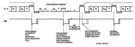
Fig. 20 - Receive continuous "BREAK".
