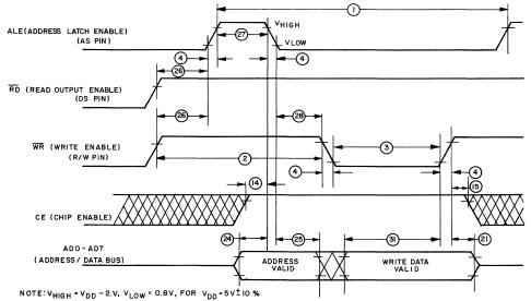
Fig. 25 – Bus-write timing waveforms of 8085 multiplexed bus.
