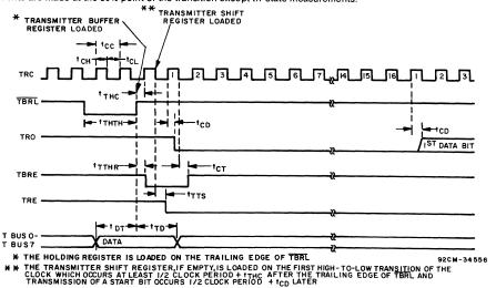
Fig. 7 - Transmitter timing waveforms.
