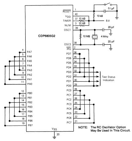
Fig. 10 - Self-check circuit.
