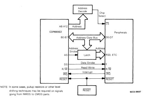
Fig. 21 - Connection to peripherals.
