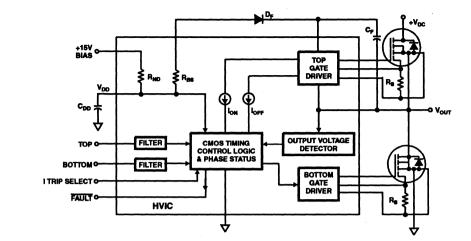
FIGURE 1. BLOCK DIAGRAM OF THE HVIC
