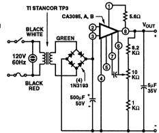
V<sub>OUT</sub> = 3.5V to 20V (0 to 90mA) Regulation = 0.2% (Line and Load) Ripple < 0.5mV at Full Load
