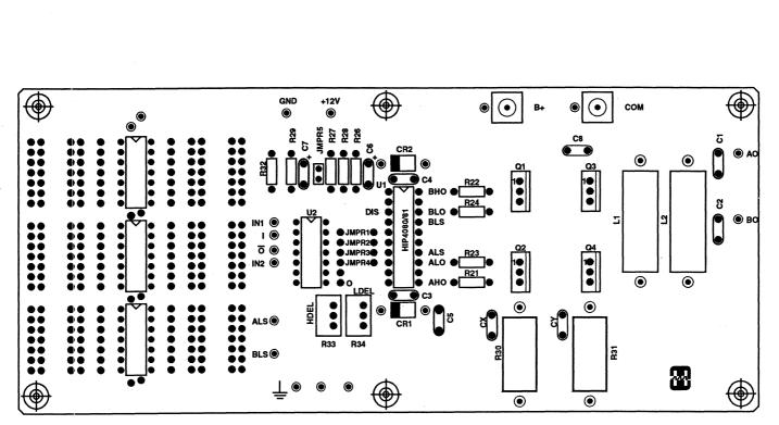
FIGURE 32. HIP4081A EVALUATION BOARD SILKSCREEN
