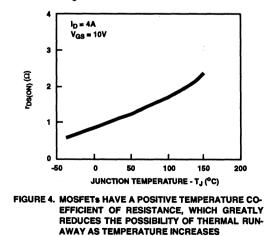
The positive temperature coefficient of resistance means that a MOSFET is inherently stable with temperature fluctuation, and provides its own protection against thermal runaway and second breakdown. Another benefit of this characteristic is that MOSFETs can be operated in parallel without fear that one device will rob current from the others. If any device begins to overheat, its resistance will increase, and its current will be directed away to cooler chips.
