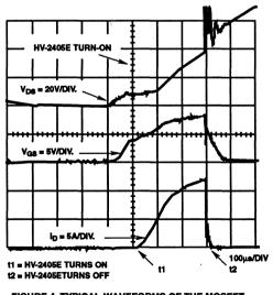
FIGURE 4. TYPICAL WAVEFORMS OF THE MOSFET (l<sub>OUT</sub> = 250mA)
