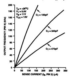
FIGURE 7. PULSE/FREQUENCY MODULATOR CHARACTERIS-TIC OF FREQUENCY vs. TIMING CAPACITOR CT AND SENSE CURRENT Is  $(T_A = +25^{\circ}C, V_1 = 5.9V,$  $V_5 = 11V, V_{CC} = 13V.)$
