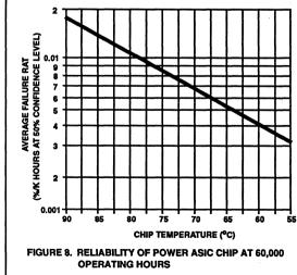
The improvement in reliability of the power ASIC chip, when the operating chip temperature is lowered in the application, is shown in Figure 8. For example, this shows that the reliability is improved 2 to 1 when using a chip temperature of  $+75^{\circ}$ C and 6 to 1 when using  $+55^{\circ}$ C instead of  $+90^{\circ}$ C.
