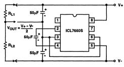
FIGURE 22. SPLITTING A SUPPLY IN HALF
