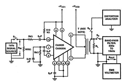
NOTE: Push-pull output transformer; load resistance (R<sub>L</sub>) should be selected to provide indicated collector-to-collector load impedance (R<sub>CC</sub>).
