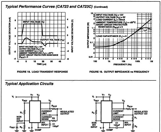
Circuit Performance Data: Regulated Output Voltage 5V Line Regulation ( $\Delta V_{|=} 3V$ ) 0.5mV Load Regulation ( $\Delta L_{|=} 50$ mA) 1.5mV Note: R3 = <u>R1 + R2</u> For Minimum Temperature Drift R1 + R2
