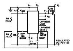
Circuit Performance Data: Line Regulation ( $\Delta V_1 = 3V$ ) 1mV Load Regulation ( $\Delta L_1 = 100mA$ ) 2mV Note: For Applications Employing the TO-5 Style Package and Where  $V_Z$  Is Required, An External; 6.2V Zener Diode Should be Connected in Series with  $V_0$  (Terminal 6).
