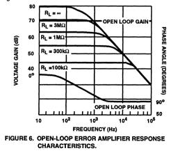
The output amplifier terminal is also used to compensate the system for ac stability. The frequency response and phase shift curves are shown in Figure 7. The uncompensated amplifier has a single pole at approximately 250Hz and a unity gain cross-over at 3MHz.
