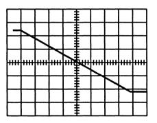
Horizontal: 0.5V/Div. Vertical:  $50\mu$ A/Div. I<sub>ABC</sub> = 100 $\mu$ A, Diode Current = 1mA
