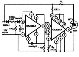
FIGURE 22. VOLTAGE REGULATOR FOR SENSOR AND ZERO-VOLTAGE SWITCH
