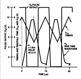
FIGURE 10. SIGNAL WAVEFORMS OF THE CIRCUIT OF FIGURE 4 (WITH 10.5pF TEST-PROBE LOADING). ( $C_T$  = 240pF, R<sub>3</sub> APPROXIMATELY 39kΩ, F<sub>(MAX)</sub> = 200kHz.)
