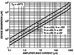
FIGURE 4. DEVICE DISSIPATION vs AMPLIFIER BIAS CUR-RENT (I<sub>ABC</sub>, TERMINAL 5)
