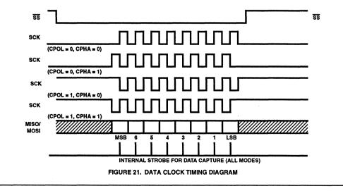
status flag in the serial peripheral status register (location \$0B) description for further information on the effects that the SS input and CPHA control bit have on the I/O data register. A high level SS signal forces the MISO (master in slave out) line to the high-impedance state. Also, SCK and the MOSI (master out slave in) line are ignored by a slave device when its SS signal is high.
