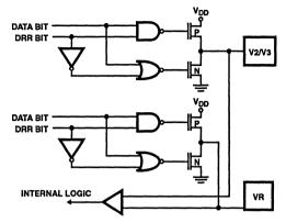
FIGURE 7. ANALOG INPUT I/O PINS
