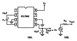
FIGURE 16. SIMPLE NEGATIVE CONVERTER AND ITS OUTPUT EQUIVALENT
