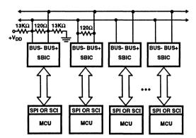
NOTE: Hardware configuration for a network consisting of 3 or more MCU's. Notice that the bus utilizes no more than 1 set of 13K bias resistors and no more than two  $120\Omega$  termination resistors.
