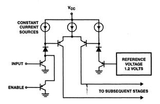
FIGURE 2. CA3262A EQUIVALENT SCHEMATIC OF ONE INPUT STAGE
