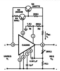
FIGURE 12. HIGH OUTPUT CURRENT VOLTAGE REGULATOR WITH "FOLDBACK" CURRENT LIMITING
