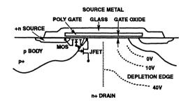
FIGURE 6. CROSS SECTION OF POWER MOSFET
