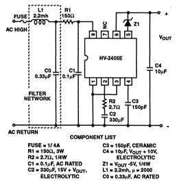
FIGURE 8. IMBEDDED SUPPLY WITH EMI FILTER (IOUT S 30mA)
