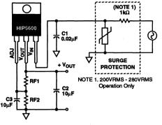
FIGURE 13. AC/DC CONVERTER
