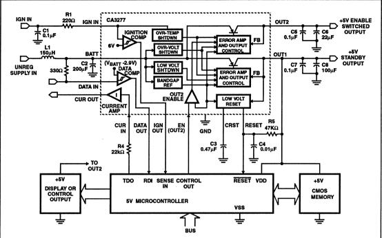
NOTE: DATA IN and CUR OUT are remote/host Serial Data Communication Buffers. Typical Remote Source Impedance for DATA IN is 1kΩ. Typical Remote Load for CUR OUT is 250Ω.
