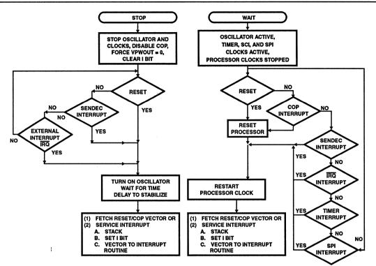
FIGURE 14. STOP AND WAIT FLOW DIAGRAM
