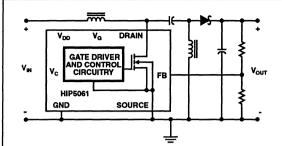
FIGURE 39A. SEPIC (FAIL-SAFE BUCK) CONVERTER
