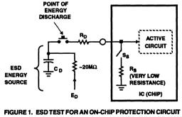
GURE 1. ESD TEST FOR AN ON-CHIP PROTECTION CIRCUIT USING THE MIL-STD-883, METHOD 3015.7 (HUMAN BODY MODEL) 11
