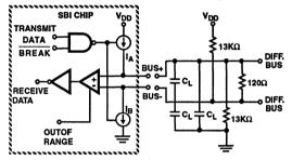
FIGURE 4. DIFFERENTIAL DRIVER/RECEIVER
