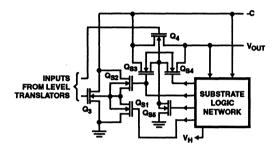
FIGURE 5. THE SUBSTRATE LOGIC NETWORK
