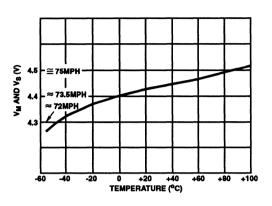
FIGURE 22. TYPICAL CHARACTERISTIC OF THE F/V CON-VERTER OUTPUT, Vg, AND D/A OUTPUT, Vg, TRACKING vs TEMPERATURE IN THE CIRCUIT OF FIGURE 2
