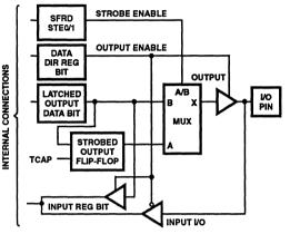
FIGURE 6. STROBED OUTPUT BLOCK DIAGRAM (PD0, PD STE0 and STE1 are not affected by RESET.
