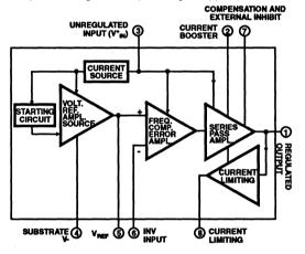
FIGURE 1. BLOCK DIAGRAM OF CA3085 SERIES
