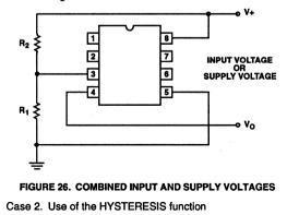
The disadvantage of the simple detection circuits is that there is a small but finite input range where the outputs are neither totally 'ON' nor totally 'OFF'. The principle behind hysteresis is to provide positive feedback to the input trip point such that there is a voltage difference between the input voltage necessary to turn the outputs ON and OFF.
