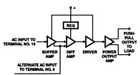
FIGURE 2. FUNCTIONAL BLOCK DIAGRAM OF THE CA3020 AND CA3020A
