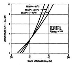
FIGURE 3. TRANSFER CHARACTERISTIC
