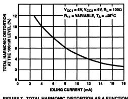
FIGURE 7. TOTAL HARMONIC DISTORTION AS A FUNCTION OF I<sub>CC2</sub> IDLING CURRENT FOR A SUPPLY VOLT-AGE OF 6V AND AN OUTPUT OF 100mW
