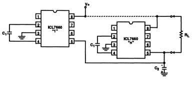
FIGURE 13. PARALLELING DEVICES
