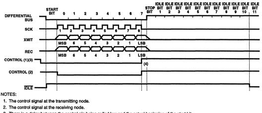
3. There is a delay between the control pin being pulled low and the actual beginning of the start bit.
