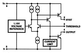
FIGURE 1. ICL8211 FUNCTIONAL DIAGRAM
