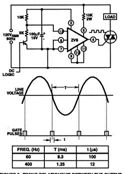
FIGURE 6. TIMING RELATIONSHIP BETWEEN THE OUTPUT PULSES OF THE ZERO-VOLTAGE SWITCH AND THE AC LINE VOLTAGE
