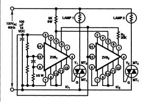
FIGURE 50. SYNCHRONOUS LIGHT FLASHER
