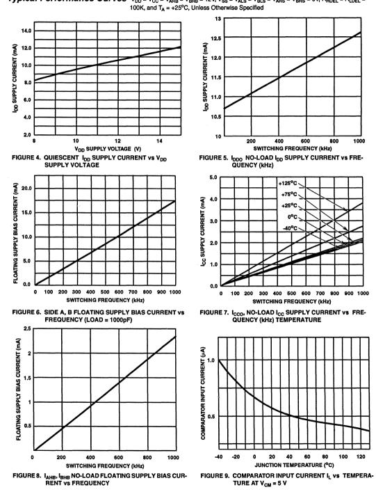
Typical Performance Curves V<sub>DD</sub> = V<sub>CC</sub> = V<sub>AHB</sub> = V<sub>BHB</sub> = 12V, V<sub>SS</sub> = V<sub>ALS</sub> = V<sub>BLS</sub> = V<sub>BHS</sub> = 0V, R<sub>HDEL</sub> = R<sub>LDEL</sub> =
