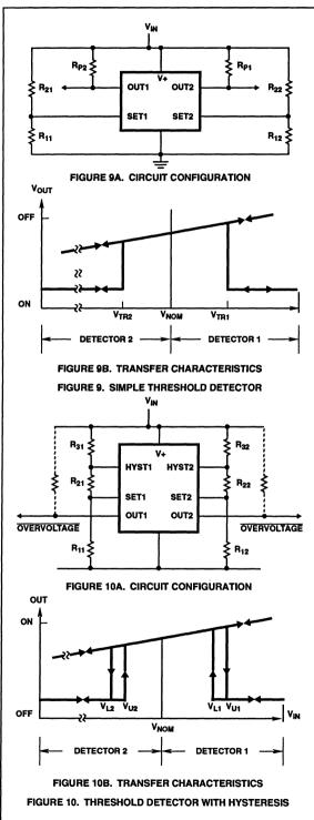
Either detector may be used alone, as well as both together, in any of the circuits shown here.
