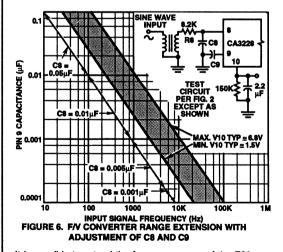
It is possible to extend the frequency range of the F/V converter to frequencies as low as 10Hz and as high as 500kHz. However, the loop stability of the lower frequencies may be difficult to control. Higher values become very dependent on stray capacitance, causing some loss of output linearity where the internal circuit becomes bandwidth limited.
