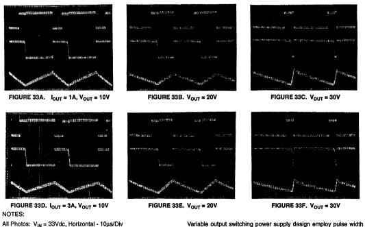
Variable output switching power supply design employ pulse width modulation techniques to achieve high performance. Note that "on" times of Q1 and the CA1524 are more dependent on the circuit's output voltage than by the output current to the load.
