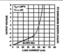
FIGURE 7. OUTPUT CHARACTERISTICS
