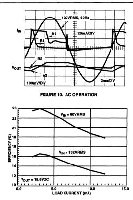
FIGURE 11. EFFICIENCY AS A FUNCTION OF LOAD CURRENT
