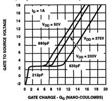
FIGURE 9. MOSFET GATE DYNAMIC CHARACTERISTICS
