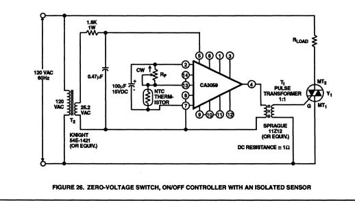
increase when temperature is low since it was assumed that the sensor has a negative temperature coefficient. The potential at the noninverting terminal, being greater than that at the inverting terminal at the amplifier, causes the multivibrator to oscillate at approximately 10kHz. The oscillations are transformer coupled through a current limiting resistor to the gate of the thyristor, and trigger it into conduction.
