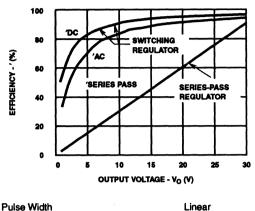
Modulator (PWM) Switching Regulator Linear Series-Pass Regulator
