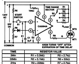
$R4 = 44M\Omega$ FIGURE 23. PRESETTABLE ANALOG TIMER
