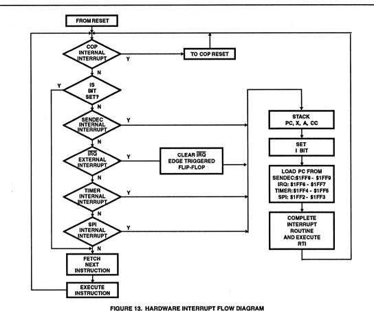
FIGURE 13. HARDWARE INTERNOFT FLOW DIA
