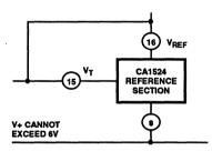
NOTE: V+ Should Be in the 5V Range And Must Not Exceed 6V
