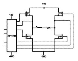
FIGURE 1. HIP4081 SIMPLIFIED APPLICATION DIAGRAM
