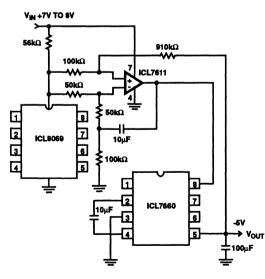
FIGURE 22. REGULATED OUTPUT INVERTER
