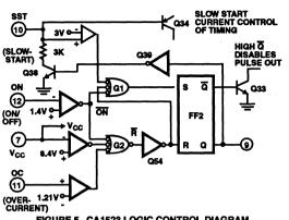
FIGURE 5. CA1523 LOGIC CONTROL DIAGRAM
