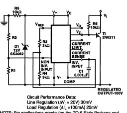
NOTE: For applications employing the TO-5 Style Package and where  $V_Z$  is required, an external 6.2V zener diode should be connected in series with  $V_O$  (terminal 6)
