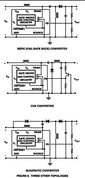
It should be noted that when the Cuk topology is implemented, a transistor current source is used to convert the negative output voltage of the Cuk converter to a current that is level shifted to the FB terminal on the HIP5061.
