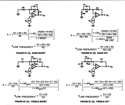
FIGURE B1. FOUR OPERATIONAL AMPLIFIER CIRCUIT CONFIGURATIONS AND THE GAIN EXPRESSIONS FOR EACH
