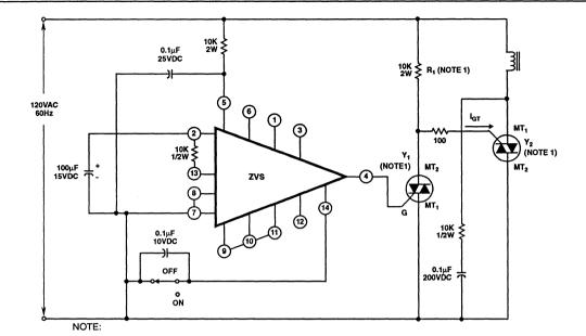
1. If Y<sub>2</sub>, For Example, is a 40A TRIAC, then R<sub>1</sub> must be Decreased to Supply Sufficient I<sub>GT</sub> for Y<sub>2</sub>.
