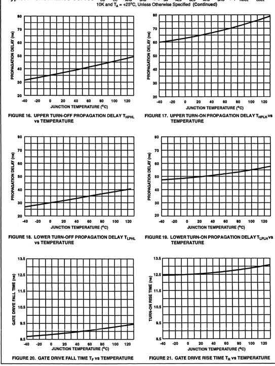
**Typical Performance Curves**  $V_{DD} = V_{CC} = V_{AHB} = V_{BHB} = 12V$ ,  $V_{SS} = V_{ALS} = V_{BLS} = V_{AHS} = 0V$ ,  $R_{HDEL} = R_{LDEL} = 10K$  and  $T_A = +25^{\circ}$ C, Unless Otherwise Specified (Continued)
