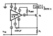
$\mathbf{Q}_1$ : Any N-P-N Silicon Transistor that can handle a 2A Load Current such as 2N3772 or Equivalent NOTE
