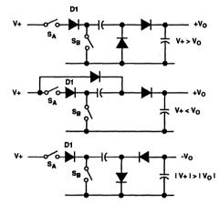
NOTE: Diode D1 Is Necessary To Prevent Reverse Emitter-Base Breakdown of Transistor Switch S<sub>4</sub>.
