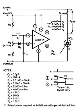
Potentiometer required for initial time set to permit device inter connecting. Time variation with temperature < 0.3%/°C.</li>
