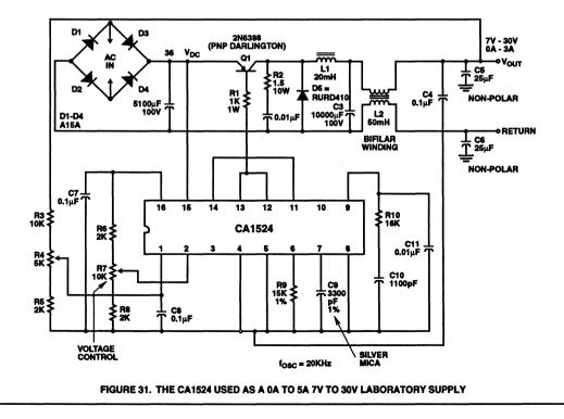
Although most switching regulator designs and applications imply a fixed output voltage, the CA1524 Series can be applied to a variable-output-voltage power supply.
