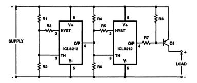
FIGURE 20. POWER SUPPLY WINDOW DETECTOR
