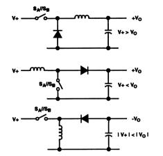
FIGURE 18. SINGLE-ENDED INDUCTOR CIRCUITS WHERE THE TWO OUTPUTS ARE CONNECTED IN PARALLEL (I.e.; SA/SB)
