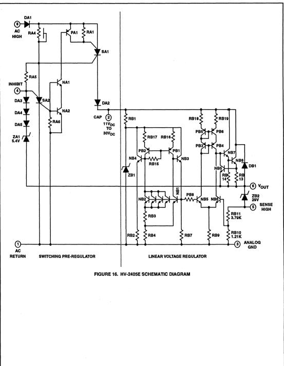
Assume that SA1 is on and the current path is from pin 8 to pin 2. If a small current is pulled out of the base of SA2s pnp (point 1, Figure 17A) SA2 will turn on. When SA2 turns on the collector current of SA1s pnp no longer provides base drive to its npn and SA1 turns off. Figure 17(B) shows the current relationships for both SCRs.
