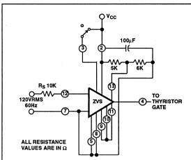
FIGURE 8. OPERATION OF THE ZERO-VOLTAGE SWITCH FROM AN EXTERNAL DC POWER SUPPLY CON-NECTED BETWEEN TERMINALS 2 AND 7.
