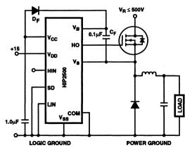
FIGURE 1. DOUBLE FORWARD CONVERTER SCHEMATIC
