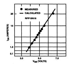
FIGURE 6. DRAIN CURRENT VS GATE VOLTAGE (NOTE SQUARE ROOT SCALE) - MEASURED CURVE VS CALCULATED POINTS.
