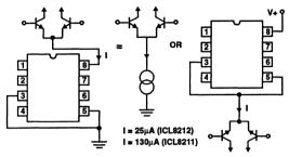
FIGURE 32. CONSTANT CURRENT SOURCE APPLICATIONS
