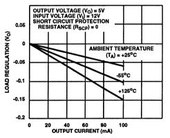
FIGURE 3. LOAD REGULATION WITHOUT CURRENT LIMIT-ING
