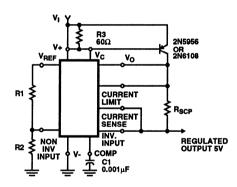
Circuit Performance Data: Line Regulation ( $\Delta V_I = 3V$ ) 0.5mV Load Regulation ( $\Delta I_L = 1A$ ) 5mV
