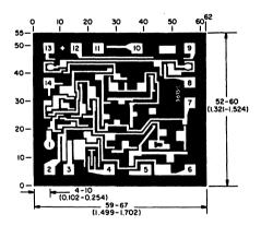
Dimensions in parentheses are in millimeters and are derived from the basic inch dimensions as indicated. Grid gradations are in mils  $(10^{-3} \text{ inch})$ .
