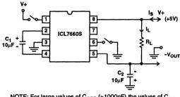
NOTE: For large values of  $C_{OSC}$  (>1000pF) the values of  $C_1$ and  $C_2$  should be increased to 100 $\mu$ F
