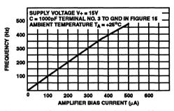
FIGURE 16. FREQUENCY AS A FUNCTION OF  $I_{ABC}$  FOR C = 1000pF FOR CIRCUIT IN FIGURE 15
