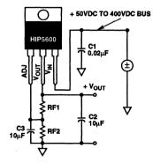
FIGURE 12. DC/DC CONVERTER
