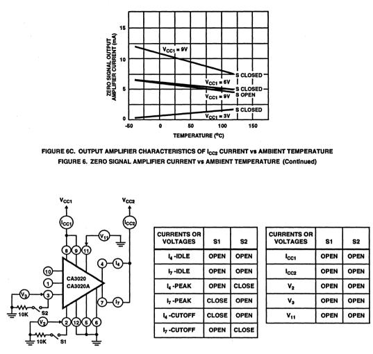
FIGURE 7. STATIC CURRENT AND VOLTAGE TEST CIRCUIT
