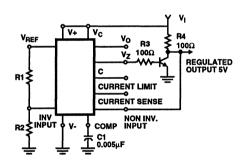
Circuit Performance Data: Line Regulation ( $\Delta V_I = 10V$ ) 0.5mV Load Regulation ( $\Delta I_L = 100$ mA) 1.5mV NOTE: For applications employing the TO-5 Style Package and where V<sub>Z</sub> is required, an external 6.2V zener diode should be connected in series with V<sub>Q</sub> (terminal 6).
