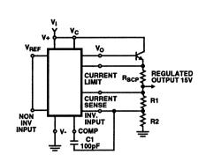
Circuit Performance Data: Line Regulation ( $\Delta V_I = 3V$ ) 1.5mV Load Regulation ( $\Delta I_L = 1A$ ) 15mV
