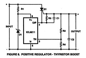
A word of warning, however. Thyristor data sheets do not generally specify individually the gain of the PNP portion of the thyristor, on which the circuit relies. It must therefore either be very conservatively designed or some screening or guarantee of the PNP gain be provided.
