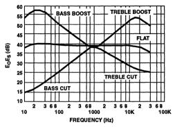
FIGURE 16. THE MEASURED RESPONSE OF THE AMPLIFIER AT EXTREMES OF TONE CONTROL ROTATION
