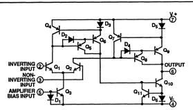
FIGURE 23. SCHEMATIC DIAGRAM OF THE CA3080
