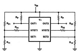
FIGURE 11. AN ALTERNATIVE HYSTERESIS CIRCUIT
