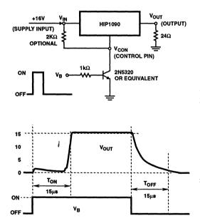
FIGURE 3. TYPICAL ON-OFF SWITCHING CHARACTERISTIC OF THE HIP1090 USING AN NPN TRANSISTOR TO SWITCH THE  $\rm V_{CON}$  INPUT TERMINAL
