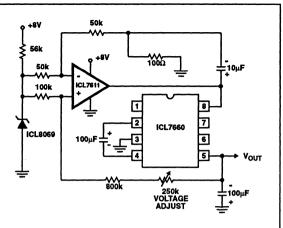
FIGURE 22. REGULATING THE OUTPUT VOLTAGE
