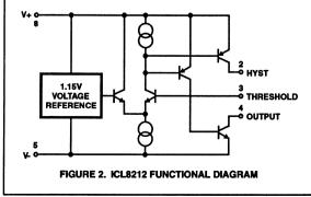
For a detailed circuit description of the ICL8211/ICL8212 refer to the data sheet. For large volume applications the ICL8211/ICL8212 may be customized by the use of metal mask options to include setting resistors or to vary the output options, or even to adapt the circuit as a temperature sensing element.
