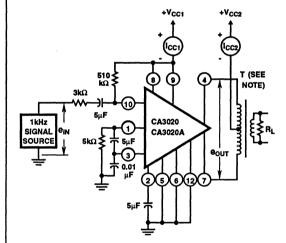
NOTE: Push-pull output transformer; load resistance (Rt) should be selected to provide indicated collector-to-collector load impedance (R<sub>CC</sub>).
