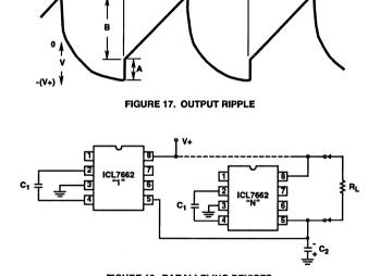
FIGURE 18. PARALLELING DEVICES
