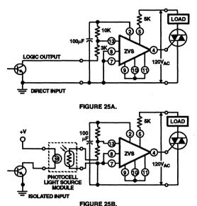
FIGURE 25. BASIC INTERFACING TECHNIQUES: A. DIRECT IN-PUT; B. ISOLATED INPUT
