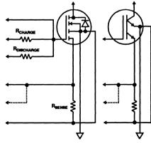
FIGURE 3. POWER-OUTPUT SECTION INTERFACING WITH CURRENT SENSING MOSFET OF IGT.
