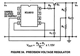
This regulator may be used with lower input voltages than most other commercially available regulators and also consumes less power for a given output control current than any commercial regulator. Applications would therefore include battery operated equipment especially those operating at low voltages.
