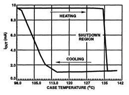
FIGURE 9. THERMAL HYSTERESIS CURVE
