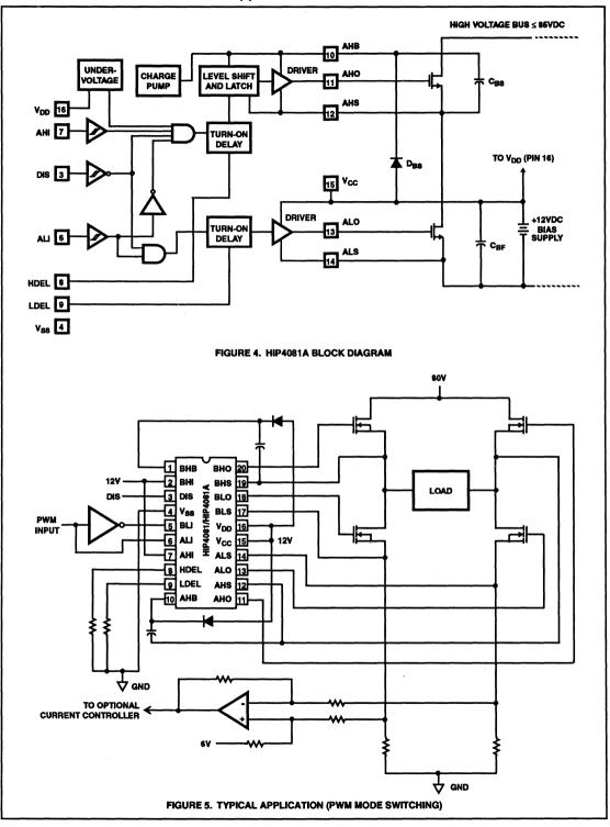
The Level-Translation circuit communicate "on" and "off" pulses from the Propagation Delay sub-circuit to the upper logic and gate drive sub-circuits which "float" at the potential of the upper power MOSFET source connections. This voltage can be as much as 85V when the bias supply voltage is only 10V (the sum of the bias supply voltage and bus voltages must not exceed 95VDC).
