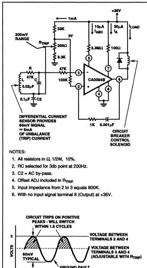
FIGURE 32. GROUND FAULT INTERRUPTER (GFI) AND WAVE-FORM PERTINENT TO GROUND FAULT DETECTOR
