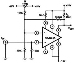
FIGURE 5. CLASS A AMPLIFIER -280mW CAPABILITY INTO A RESISTIVE LOAD
