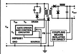
FIGURE 9. FORWARD CONVERTER
