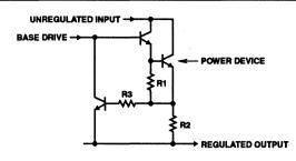
FIGURE 14. STANDARD CURRENT LIMIT
