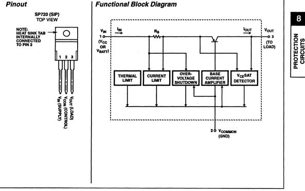
CAUTION: These devices are sensitive to electrostatic discharge. Users should follow proper I.C. Handling Procedures. Copyright @ Harris Corporation 1993
