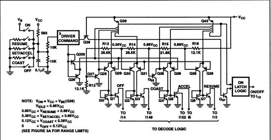
FIGURE 3. DRIVER COMMAND INPUT COMPARATOR CIRCUIT AND LOGIC OUTPUT TO COMMAND DECODE
