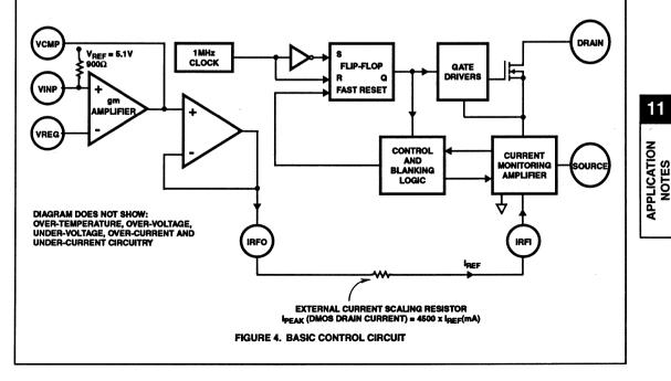
As the output voltage decays below the reference voltage, 1MHz switching starts again. The resulting burst mode maintains the required regulator voltage under very light load conditions.
