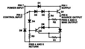
FIGURE 1. MOSFET DRIVER SCHEMATIC
