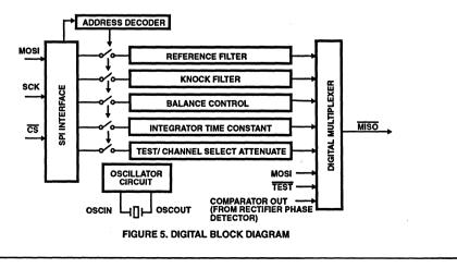
The digital block diagram shows the programming flow of the chip. An eight bit word is received at the  $\overline{\text{MISO}}$  port. Data is shifted in by the SCK clock when the chip is enabled by the  $\overline{\text{CS}}$  pin. The word is decoded by the address decoding circuit, and the information is directed to one of 5 registers. These registers control:
