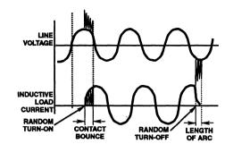
FIGURE 43. TRANSIENTS GENERATED BY RELAY CONTACT BOUNCE AND NONZERO TURN OFF OF INDUC-TIVE LOAD.
