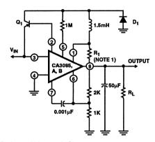
All Resistance Values are in Ohms D<sub>1</sub>: 1N4001 or Equivalent Q<sub>1</sub>: 2N5322 or Equivalent
