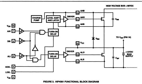
comes along to set the latch to the opposite state. Very reliable operation can be obtained with pulse widths of approximately 80ns. At a switching frequency of even 1.0MHz, with an 80VDC bus potential, the power developed by the leveltranslation circuit will be less than 0.08W.
