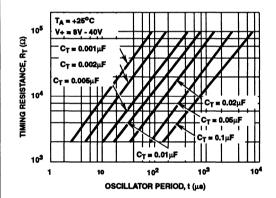
FIGURE 10. TYPICAL OSCILLATOR PERIOD AS A FUNCTION OF  $R_T$  AND  $C_T$
