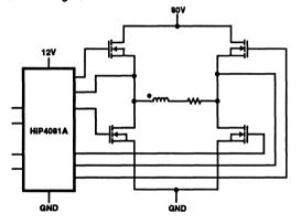
FIGURE 1. HIP4081A SIMPLIFIED APPLICATION DIAGRAM
