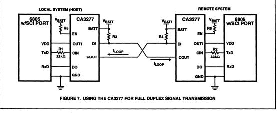
can be used to transmit and receive data. A data rate of 9600 baud should be easily attainable in most applications and could potentially be much higher where line impedances are low and a twisted pair, shielded cable is used. The shield should be tied to the system with the lowest source ground impedance.
