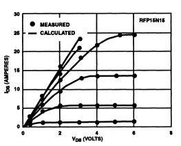
FIGURE 7. DRAIN CURRENT VS DRAIN VOLTAGE FOR CON-STANT VALUES OF GATE VOLTAGE - MEASURED CURVES VS CALCULATED POINTS.
