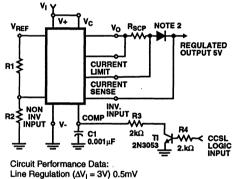
Load Regulation ( $\Delta L = 50$ mA) 1.5mV Short Circuit Current 20mA
