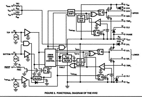
through caused by high voltage, high-speed switching. These features aid in providing predictable operation of the floating upper rail driver section, which is capable of slewing over 10,000 volts per µs.
