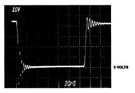
FIGURE 5. DMOS TRANSISTOR DRAIN VOLTAGE DURING CONDUCTION.
