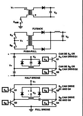
FIGURE 19. TRANSFORMER-COUPLED OUTPUTS
