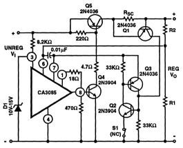
FIGURE 16. HIGH-VOLTAGE REGULATOR INCORPORATING CURRENT "SNAP-BACK" PROTECTION
