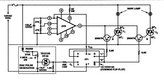
FIGURE 49. SYNCHRONOUS SWITCHING TRAFFIC FLASHER
