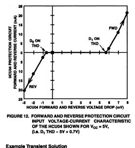
Based on the circuit of Figure 10, negative and positive ESD discharge circuit models of the SP720 and HCU04 are shown in Figure 13A and 13B. The negative ESD voltage is taken as the worse case condition because a positive ESD voltage will discharge to the  $V_{CC}$  power supply and the positive offset voltage will reduce the forward current. Using the negative
