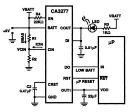
FIGURE 6. EXAMPLE OF A LOW BATTERY FAULT INDICATOR CIRCUIT 11
