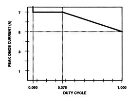
FIGURE 3. PEAK DMOS TRANSISTOR DRAIN CURRENT VS DUTY CYCLE
