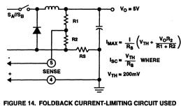
TO REDUCE POWER DISSIPATION UNDER SHORTED OUTPUT CONDITIONS
