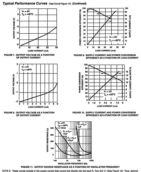
NOTE 6. These curves include in the supply current that current fed directly into the load R<sub>L</sub> from the V+ (See Figure 12). Thus, approximately half the supply current goes directly to the positive side of the load, and the other half, through the ICL7660S, to the negative side of the load. Ideally,  $V_{OUT} \simeq 2V_{IN}$ ,  $I_S \simeq 2I_L$ , so  $V_{IN} \times I_S \simeq V_{OUT} \times I_L$ .
