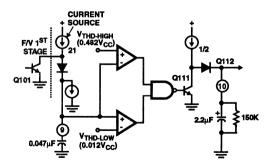
FIGURE 8. F/V CONVERTER COMPARATOR STAGE
