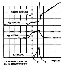
FIGURE 3. TYPICAL WAVEFORMS OF THE MOSFET (I<sub>OUT</sub> = 50mA)
