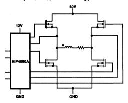
FIGURE 1. HIP4080A SIMPLIFIED APPLICATION DIAGRAM
