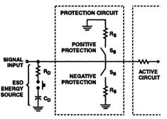
FIGURE 3. ESD AND TRANSIENT PROTECTION CIRCUIT
