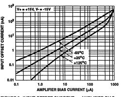
FIGURE 2. INPUT OFFSET CURRENT vs AMPLIFIER BIAS CURRENT (I\_{ABC}, TERMINAL 5)
