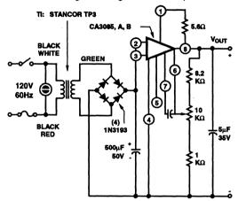
FIGURE 3. BASIC POWER SUPPLY
