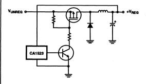
FIGURE 2C. BUCK CONVERTER REGULATOR
