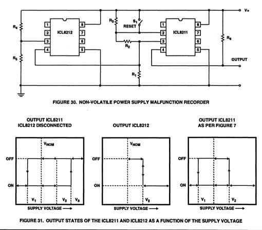
Since there is no internal compensation in the ICL8212 it is necessary to use a large capacitor across the output to prevent oscillation.
