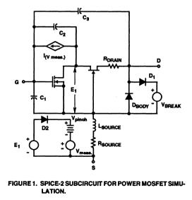
NOTE: If the JFET source voltage,  $E_1$ , is very low relative to its  $V_{\text{PINCH}}$  voltage, the JFET is in a highly conductive state, tightly coupling  $C_2$  to the JFET drain. However, as the voltage  $E_1$  approaches  $V_{\text{PINCH}}$ , the JFET operates in a constant-current mode, thereby permitting a much faster drain slew rate, which is determined primarily by  $C_3$ .
