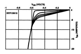
FIGURE 8. THIRD-QUADRANT DRAIN CURRENT VS DRAIN VOLTAGE WITH CONSTANT POSITIVE GATE VOLTAGE (CALCULATED).
