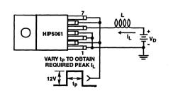
FIGURE 1. UNCLAMPED ENERGY TEST CIRCUIT
