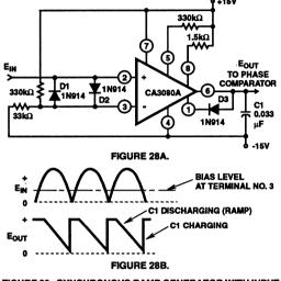
FIGURE 28. SYNCHRONOUS RAMP GENERATOR WITH INPUT AND OUTPUT WAVEFORMS
