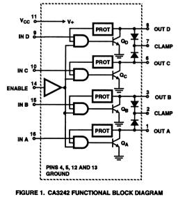
Proper application will protect the CA3242E during turn-off under shorted load conditions. Observations of wide ranging conditions have been done to test the shutdown behavior and has revealed several pitfalls that should be addressed to assure safe shutdown. One should be aware that a forced short circuit test condition may be considerably more severe than a normal application shorted load. In either case, two problems arise that affect the severity of the overload during shutdown. These are:
