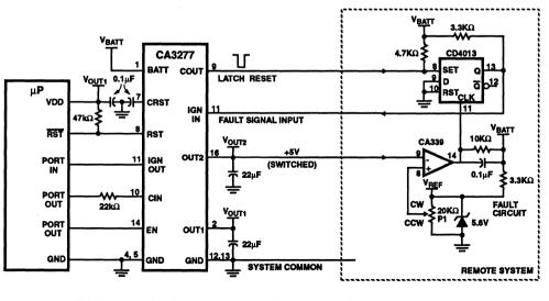
FIGURE 2. REMOTE SINGLE BIT COMMUNICATION AND LOGIC LEVEL TRANSLATION
