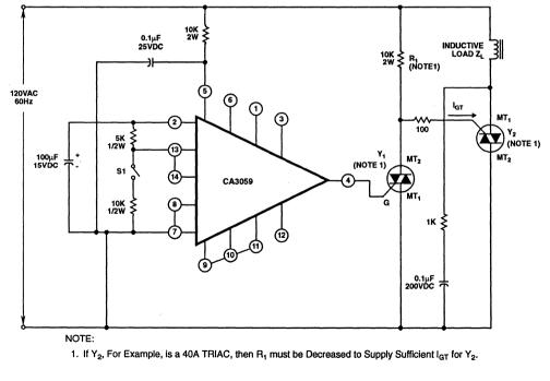
FIGURE 52. ZERO-VOLTAGE SWITCH TRANSIENT FREE SWITCH CONTROLLER IN WHICH POWER IS APPLIED TO THE LOAD WHEN THE SWITCH IS CLOSED
