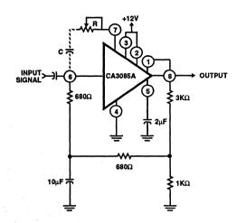
FIGURE 23. GENERAL-PURPOSE AMPLIFIER USING CA3085A
