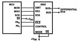
FIGURE 11. USING THE BUFFERED SPI MODE
