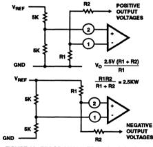
FIGURE 13. ERROR AMPLIFIER BIASING CIRCUITS
