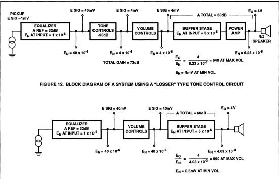
FIGURE 13. A SYSTEM IN WHICH TONE CONTROLS ARE IMPLICIT IN THE FEEDBACK CIRCUIT OF THE POWER AMPLIFIER
