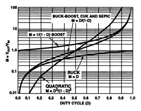
FIGURE 12. VOLTAGE TRANSFER AS A FUNCTION OF DUTY CYCLE FOR VARIOUS TOPOLOGIES 11
