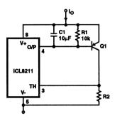
FIGURE 13. PROGRAMMABLE CURRENT SOURCE
