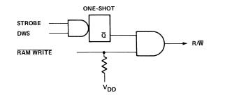
The one-shot is needed to adjust the DMA WRITE pulse width to the particular RAM requirements.
