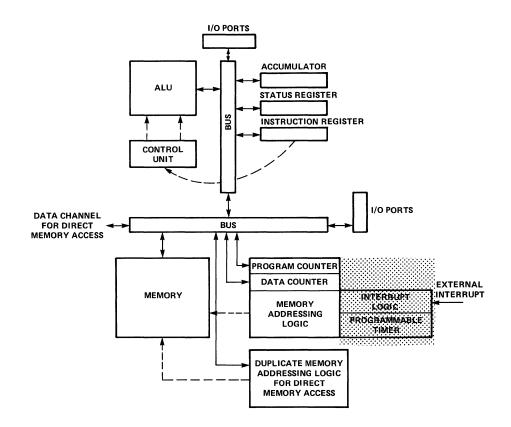
Figure 1-13. 3861 Peripheral Input/Output Device Logic
