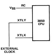
Figure 2-6. External Mode Clock Generation
