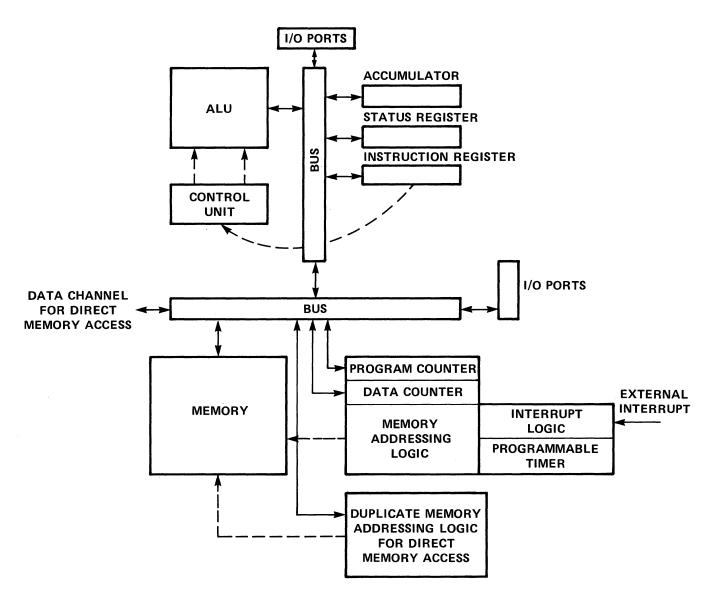
Figure 1-8. Functional Logic of a Complete Microcomputer System
