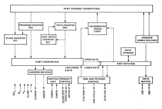
Figure 4-1. Logic Organization and Pins for the 3852 DMI
