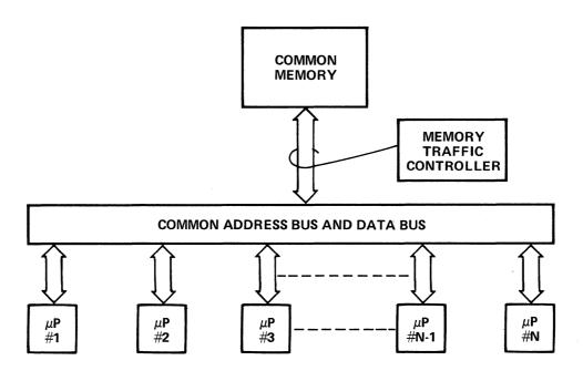
Figure 14-5. Microprocessor Network with Common Memory
