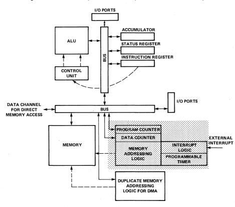
Figure 1-12. 3853 Static Memory Interface Device Logic
