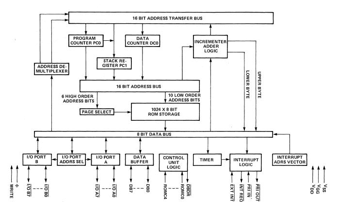
Figure 3-1. Logical Organization and Pins for the 3851 PSU
