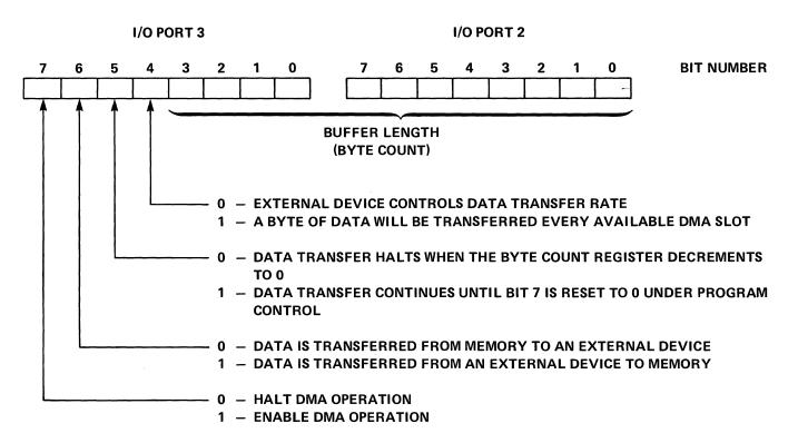
Figure 6-2. How PORT2 and PORT3 are Used to Control DMA Operations
