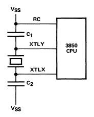
Figure 2-5. Crystal Mode Clock Generation
