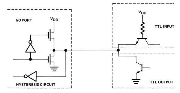
Figure 3-4. Standard Pull-up Configuration
