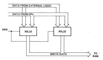
The 83L22 devices are low power quad two-input multiplexers. Each is four bits wide. DWS is used to select between the two data sources.
