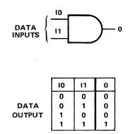
Figure 1-1. A Very Elementary Logic Device
