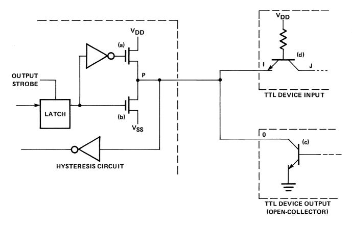
Figure 2-12. An F8 I/O Port Bit
