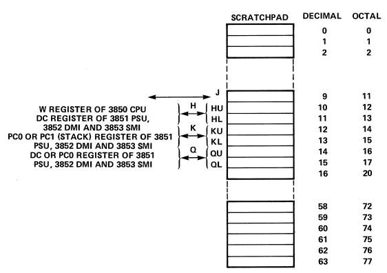
Figure 2-3. The 3850 CPU Scratchpad Registers
