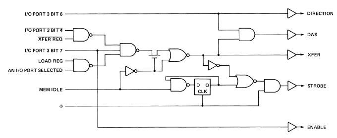
Figure 6-4. DMA Control Signals Output by the 3854 DMA Device
