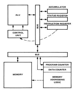
Figure 1-5. A Simple CPU with Memory
