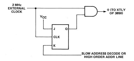
Figure 12-7. Modifying Clock Period under Hardware Control
