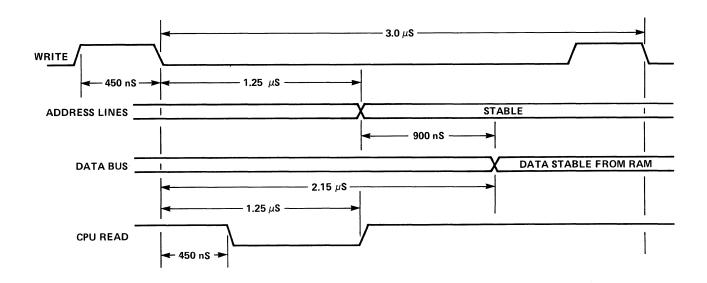
Figure 5-7. 3853 SMI Timing Signals Output during a Long Cycle Memory Read, with Address Out of Data Counter
