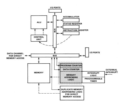
Figure 1-11. 3852 Dynamic Memory Interface Device Logic
