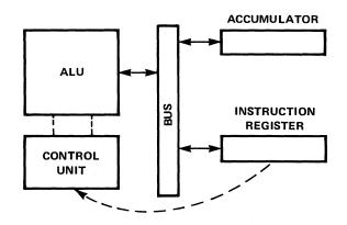
Figure 1-4. An Elementary Central Processing Unit
