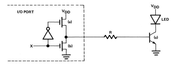
Figure 3-6. Driver Pull-up Configuration
