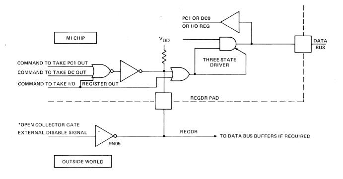
Figure 5-3. REGDR Controls Data Bus Drivers
