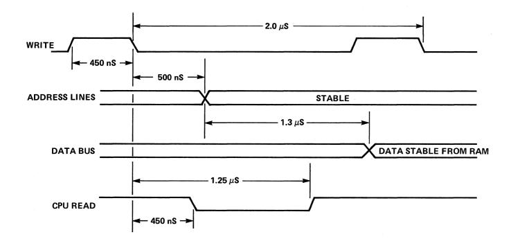
Figure 5-5. 3853 SMI Timing Signals Output during a Short Cycle Memory Read Using PCO
