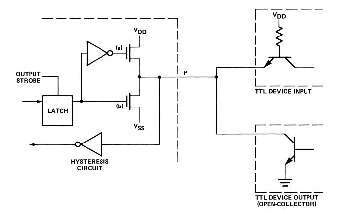
Figure 7-5. An F8 I/O Port Bit
