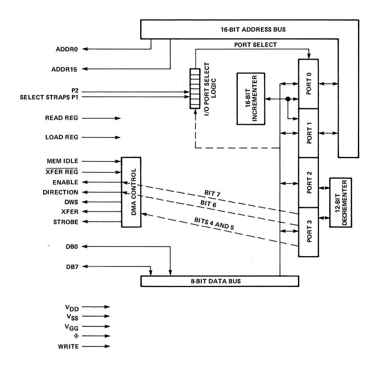
Figure 6-1, Logic Organization and Pins for the 3854 DMA Device
