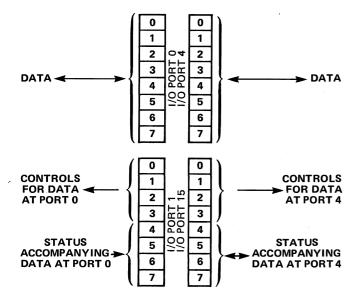
Figure 11-2. I/O Ports Divided into Two Subsystems for a Two-Device F8 Configuration
