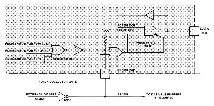
Figure 12-3. REGDR Controls Data Bus Drivers
