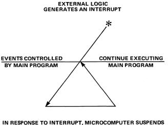
IN RESPONSE TO INTERRUPT, MICROCOMPUTER SUSPENDS MAIN PROGRAM AND EXECUTES A SPECIAL INTERRUPT SERVICE ROUTINE
