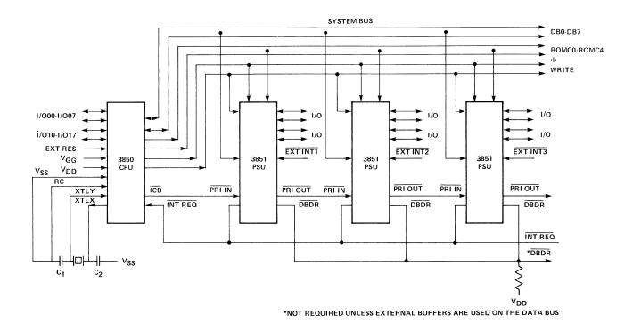
Figure 11-6. A Multi PSU F8 Configuration
