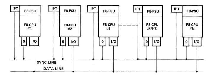
Figure 14-4. F8 Microprocessor Network using a Symetrically Connected Two-Wire System
