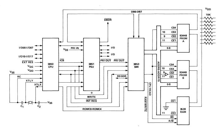
Figure 12-2. Interfacing ROM and RAM using a 3853 SMI
