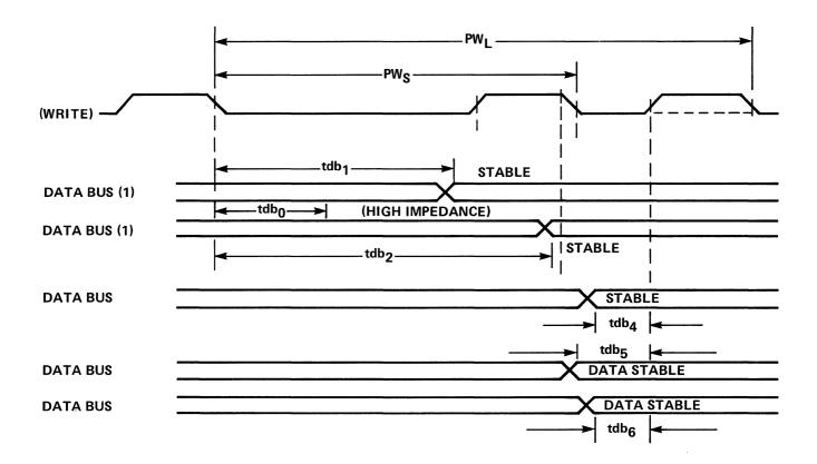
1. Timing for CPU outputting data onto the data bus.
