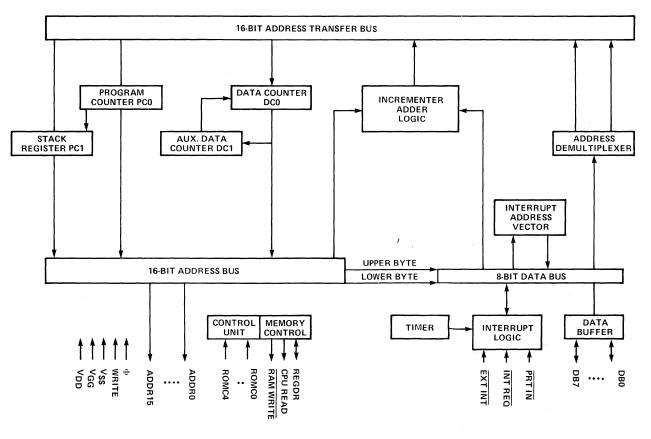
Figure 5-1. Logic Organization and Pins for the 3853 SMI
