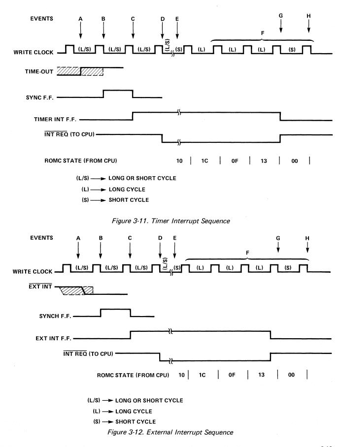
3-19 RBS0 5-1-76 Figure 3-10 is a conceptual logic diagram of the PSU's interrupt logic. Between the EXT INT input or the time-out input and the output INT REQ, there are 3 flip-flops. EXT INT and the time-out interrupt input each have a synchronizing flip-flop and edge detect logic.
