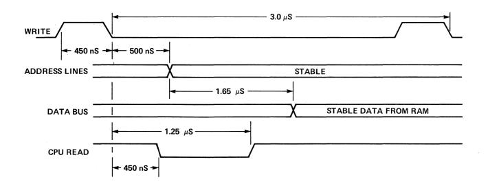
Figure 5-6. 3853 SMI Timing Signals Output during a Long Cycle Memory Read, with Address Out of Program Counter
