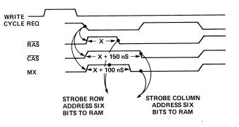
X is the address set-up time for the DMI, and has a worst case, maximum value of 400 nS.
