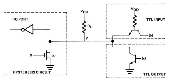
Figure 3-5. Open Drain Configuration
