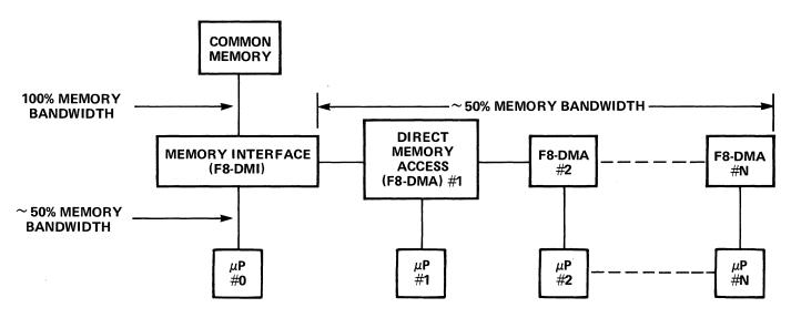
Figure 14-6. Multiprocessor Network using F8-DMI and F8-DMA Chips
