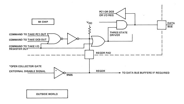
Figure 4-3. REGDR Controls Data Bus Drivers
