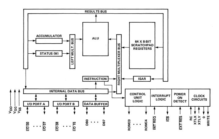
Figure 2-1. Logical Organization and Pins for the 3850 CPU
