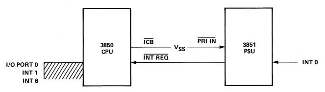
Figure 11-4. Handling Multiple Interrupts in a Two-Device F8 Configuration
