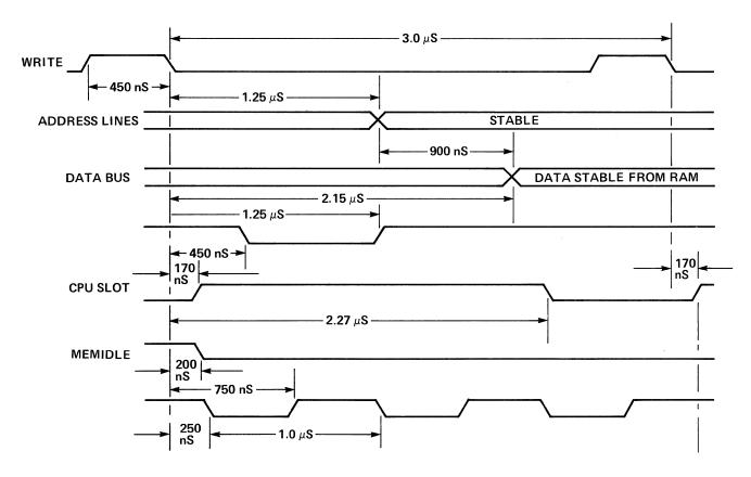
Figure 4-7. 3852 DMI Timing Signals Output during a Long Cycle Memory Read, with Address Out of Data Counter
