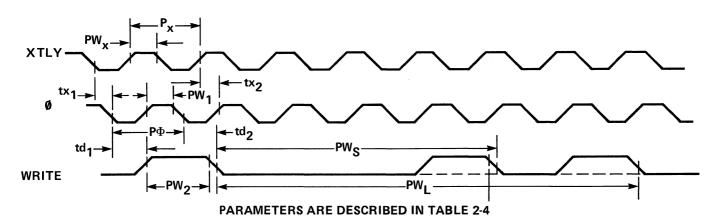
Figure 2-8. Timing Signal Specifications
