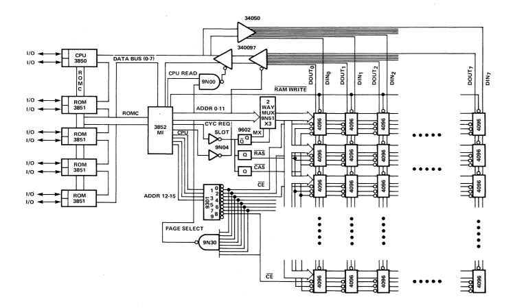
Figure 12-5. 4K ROM and 32K RAM Configuration using 4096 Devices
