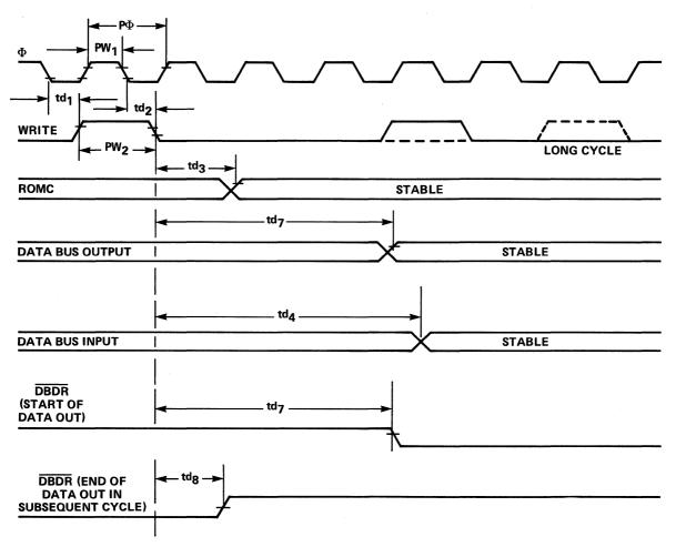
Figure 7-3. 3861 PIO Data Bus Timing
