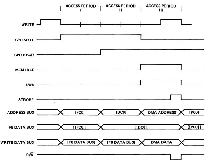
Figure 13-2. DMA Timing during a Typical Cycle
