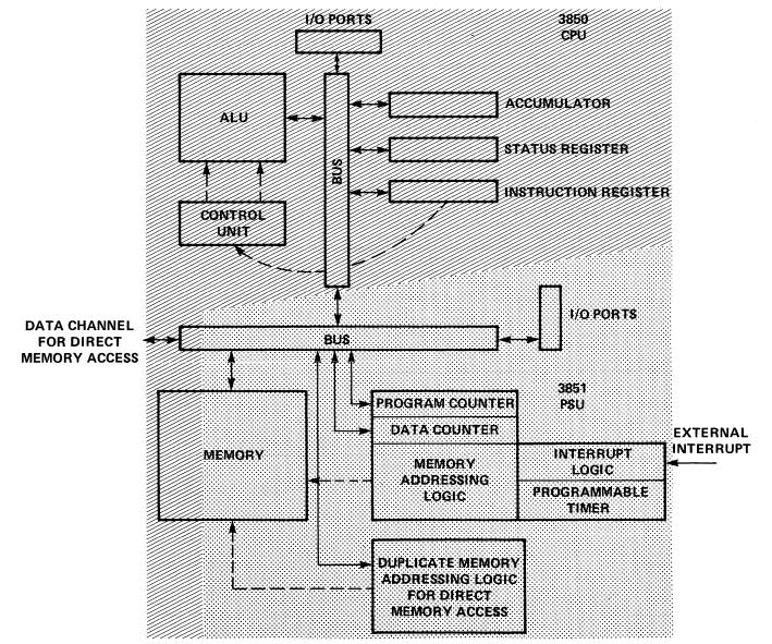
Figure 1-10. A Two-Device Configuration Consisting of a 3850 CPU and a 3851 PSU
