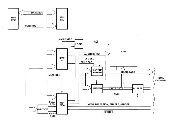
Figure 13-1. A Typical DMA Configuration
