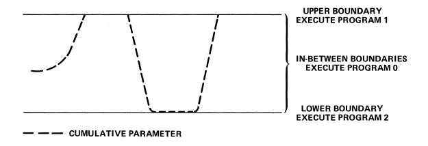
Figure 12-8. Bang-Bang Control Logic
