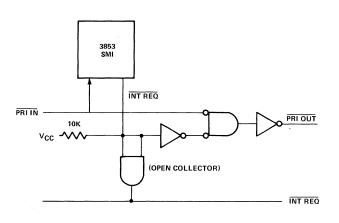
Second, the 3853 SMI interrupt address vector consists of two programmable I/O ports. The interrupt address vector is set under program control, rather than being a mask option, as it is with the 3851 PSU. Even though the 3853 SMI interrupt address vector is programmable, bit 7 is still set to 0 for a timer interrupt, or to 1 for an external interrupt, as described for the 3851 PSU.
