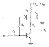
Fig. 1 (b) Zener Diode Biasing Circuit (as per reference 1)
