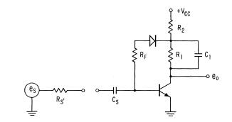
Fig. 2 An alternative method of Low-Frequency Compensation
