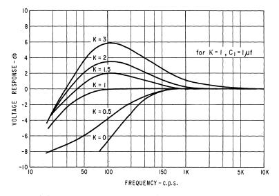
Fig. 4 Various responses showing the effect of different k's
