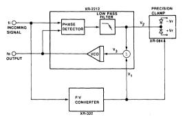
Figure 1. Tracking PLL Block Diagram.
