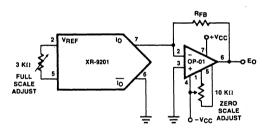
Figure 13. Full Scale and Zero Scale Adjustment
