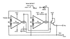
Figure 25. Peak Detector and Hold Circuit
