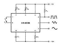
Figure 1. Generalized Test Circuit
