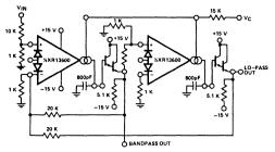
Figure 14. Voltage Controlled State Variable Filter
