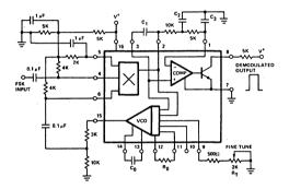
Figure 3. Circuit Connection for FSK Demodulation (Single Supply)
