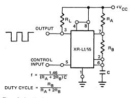
Figure 1. Monostable (One-Shot) Circuit
