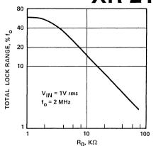
Figure 7. Total Lock Range,  $\pm \Delta f_L,$  versus VCO Gain Control Resistor,  $R_D$
