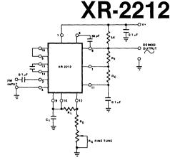
Figure 10. Circuit Connection for FM Demodulation
