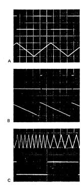
Figure 15. Output Waveforms: (a) Squarewave and Triangle Outputs (b) Pulse and Sawtooth Outputs (c) Frequency-Shift Keyed Output Top: FSK Output With  $f_2 = 2f_1$ Bottom: Keying Logic Input
