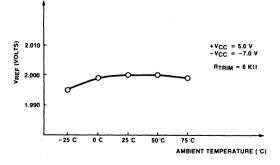
Figure 7. VREF vs. Temperature
