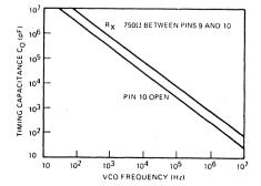
Figure 7. VCO Free Running Frequency vs Timing Capacitor
