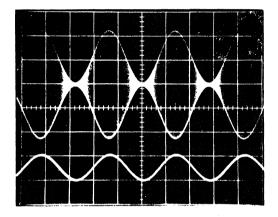
Figure 22-1. Double Sideband AM Output Waveform  $f_{carrier}=3.688\ \text{MHz}\ f_{mod}=1\ \text{kHz}\ (90\%\ \text{modulation})$
