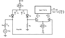
Figure 3. Equivalent VCA Input Circuit
