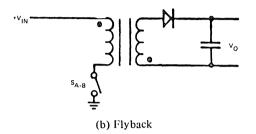
Figure 11. Push-Pull and Flyback Connections for Transformer-Coupled Outputs
