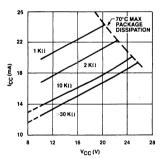
Figure 3. Supply Current versus Supply Voltage, Timing, R.
