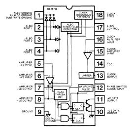
peater IC. It contains all the active circuitry to implement one side of a PCM, repeater operating on either pulp or plastic insulated cables. Repeater to repeater spacing on either type of cable is 6300 ft. max.
