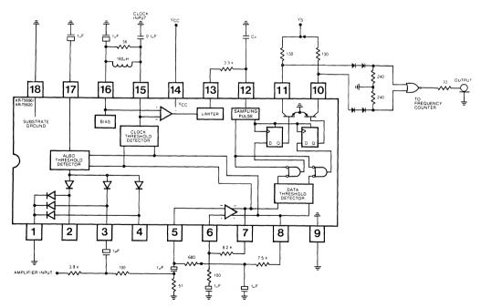
Figure 4. Sampling Pulse Test Circuit
