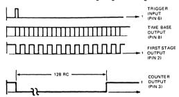
Figure 7. Timing Diagram of Output Waveforms
