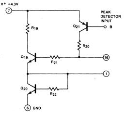
Figure 9. Automatic Line Build-Out (ALBO) Section.
