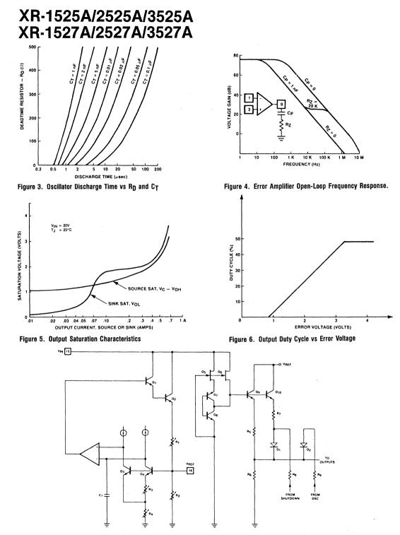
Figure 7. Equivalent Schematic of Voltage Reference Section
