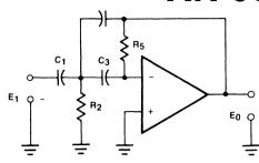
Figure 4. Network Function for the High-Pass Filter.
