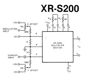
Figure 7. Double Sideband Amplitude Modulation Using XR-S200 Multiplier Section
