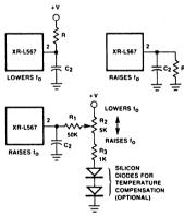
Figure 7. Detection Band Skew Adjustment
