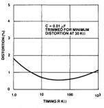
Figure 6. Trimmed Distortion versus Timing Resistor.
