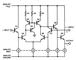
Figure 6. Circuit Diagram of Preamplifier Section.
