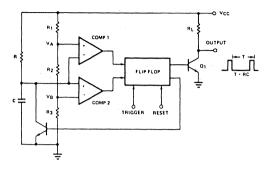
Figure 4. Simplified Schematic of a Time-Base Oscillator Circuit
