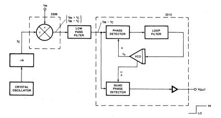
Figure 1. Functional Diagram of Narrow Band Tone Decoder.
