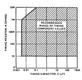
Figure 8. Recommended Range of Timing Component Values.
