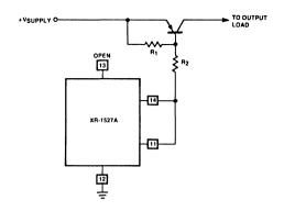
Figure 12. Single-Ended Output for XR-1527A
