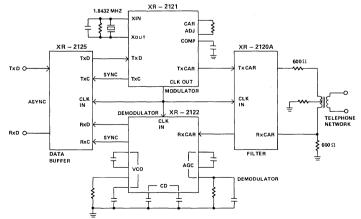
Figure 2. Complete 1200/300 BPS Modem Signal Processor
