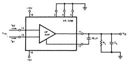
Figure 5. Test Circuit for Op Amp DC Parameters
