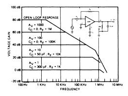
Figure 10. Amplifier Section Frequency Response
