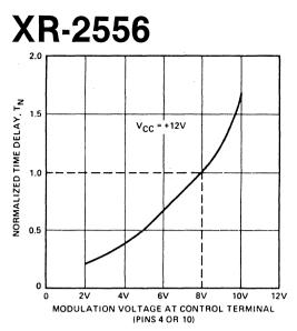
Figure 19. Normalized Time Delay vs. Modulation Voltage
