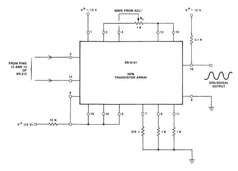
ADJUST Rq FOR MINIMUM HARMONIC DISTORTION.
