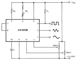
Figure 3. Connection to Achieve Minimum Sine-Wave Distortion.
