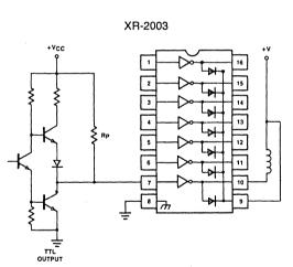
Figure 9. Use of Pull-up Resistors to Increase Drive Current
