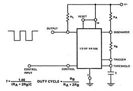
Figure 2. Astable (Free-Running) Circuit
