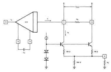
Figure 6. XR-210 Current Controlled Oscillator.
