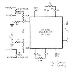
Figure 8. Multiplier Section as Frequency Doubler
