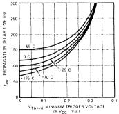
Figure 14. Propagation Delay vs. Trigger Voltage
