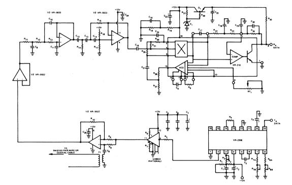
Figure 6. Complete Schematic for 100 Kilobaud FSK Modem
