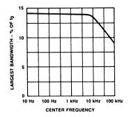
Figure 9. Largest Detection Bandwidth Versus Operating Frequency
