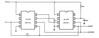
Figure 4. Cascaded Operation of Two XR-2243 Timer Circuits
