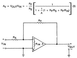
Figure 2. Basic Feedback Configuration Using an Operational Amplifier With Finite Input Impedance and Gain
