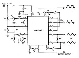
Figure 1. Test Circuit for Single-Supply Operation
