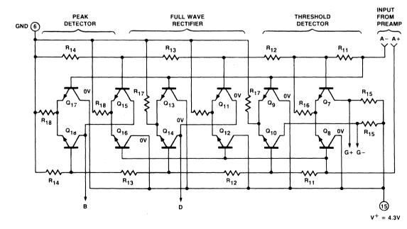
Figure 8. Circuit Diagram of Threshold-Detector, Full-Wave Rectifier and Peak-Detector Sections.
