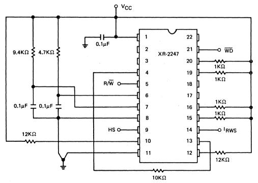
Figure 4. Test Circuit for AC Switching Characteristics
