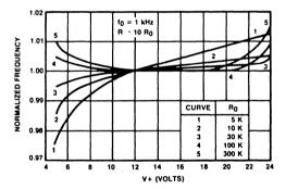
Figure 7. Typical fo vs Power Supply Characteristics
