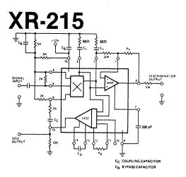
Figure 24. Circuit Connection For Tracking Filter Applications
