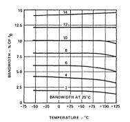
Figure 8. Bandwidth Variation with Temperature
