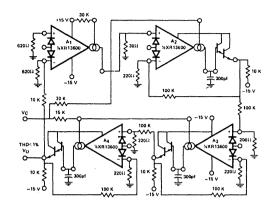
Figure 17. Sinusoidal VCO Using Two XR-13600 Circuits
