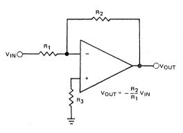
Figure 1. Inverting Amplifier
