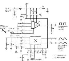
Figure 21. Waveform Generator Typical Circuit Connection Diagram
