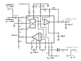
Figure 18. Time-Multiplexing XR-215 Between Two Simultaneous FM Channels
