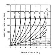
Figure 7. Bandwidth Versus Input Signal Amplitude (C<sub>2</sub> in  $\mu$ F)
