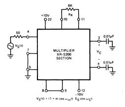
Figure 9. Synchronous AM Detector
