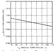
Figure 13. Delay Time vs. Temperature
