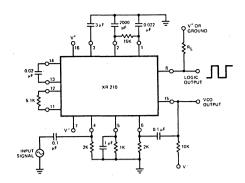
Figure 2. Test Circuit for Split Supply Operation
