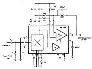
Figure 18. Synchronous AM Detector.
