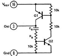
Figure 12. Recommended External Circuitry for Long Duration Blanking Pulse Generation (Method 3 of Deadband Control. Note: For 5  $\mu$ sec blanking, choose  $C_B = 200 \ \rho$ F,  $R_B = 10 \ K\Omega$ )
