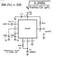
Figure 1. XR-L567 Test Circuit
