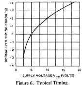
Accuracy as a Function of Supply Voltage
