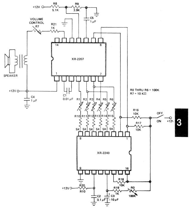
Figure 3. Circuit Connection Diagram for the Music Synthesizer.
