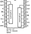
XR-C504 is a buffered version of the XR-C503 flip-flop array. Both flip-flops contain Schottkybipolar input and output buffers (see page 26). The two flip-flops share a common injector which is internally connected to V<sup>+</sup> = 5V, the I<sup>2</sup>L gates are biased at approximately 50  $\mu$ A gate and are positive edge triggered.
