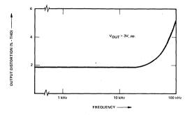
Figure 8. Output Distortion vs Frequency.
