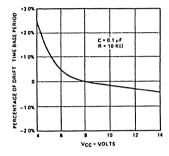
Figure 11. Power Supply Drift
