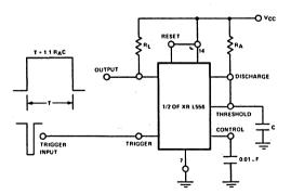
Figure 1. Monostable (One-Shot) Circuit
