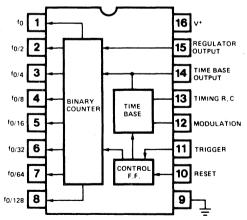
Figure 2. Functional Block Diagram of XR-2240 Counter/ Timer.
