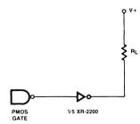
Figure 3. Circuit Connection for Driving Non-Inductive Loads
