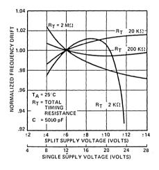
Figure 6. Frequency Drift vs. Supply Voltage
