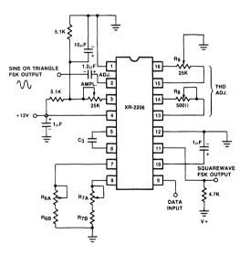
Figure 1. The XR-2206 Sinusoidal FSK Generator.
