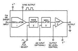
Figure 1. Basically, a waveform generator consists of four sections. Each section can be built readily in monolithic form with established IC technology.
