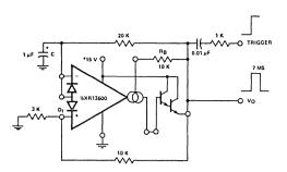
Figure 19. Timer With Zero Stand-By Power
