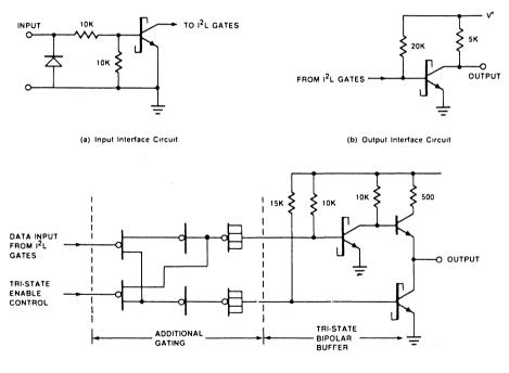
(c) Tri-State Output Interface Circuit
