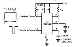
Figure 3. Monostable (One-Shot) Circuit
