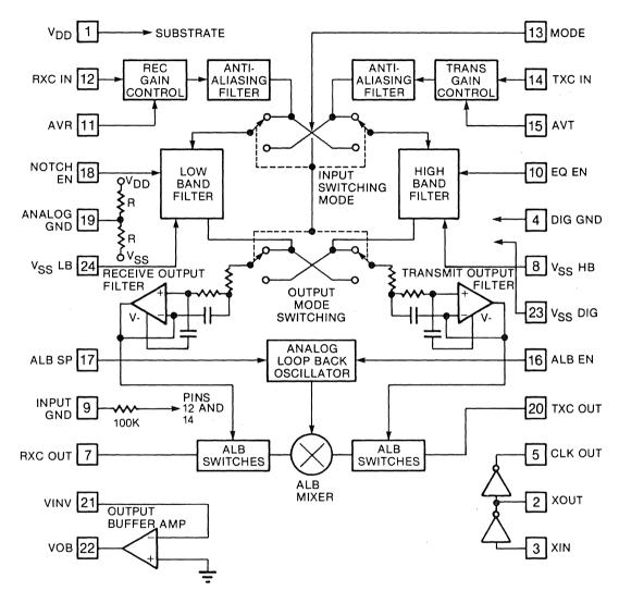
EQUIVALENT SCHEMATIC DIAGRAM
