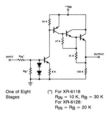
EQUIVALENT SCHEMATIC DIAGRAM
