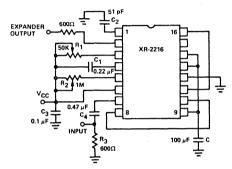
Figure 3. External Connections for Operation Expander
