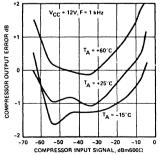
Figure 5. XR-2216 Compressor Output Error vs. Input Signal Amplitude
