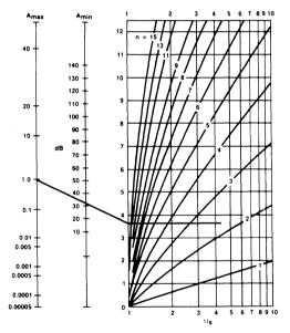
Figure 1. Nomograph to Select Desired Response.
