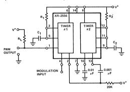
Figure 29. Pulse-Width Modulation With Internal Clock
