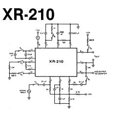
Figure 1. Test Circuits for Single Supply Operation
