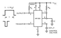
Figure 1. Monostable (One-Shot) Circuit
