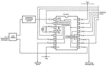
Figure 1. Typical Connection of the XR-14412 in a Complete Modem System
