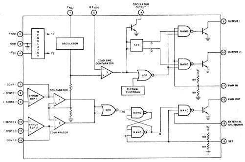
Figure 1. Equivalent Schematic Diagram
