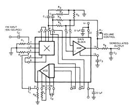
Figure 17. Circuit Connection for FM Detection
