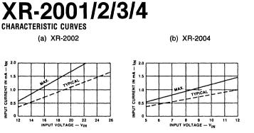
Figure 1. Input Current as a Function of Input Voltages
