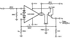
Figure 11. Voltage Controlled Low-Pass Filter
