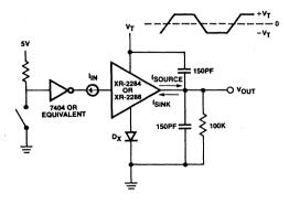
Figure 1. Generalized Test Circuit
