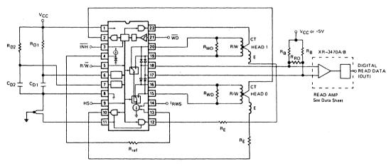
Figure 5. Typical Dual Head Floppy Disk System
