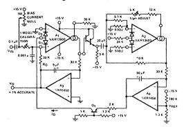
Figure 27. True RMS Converter Circuit
