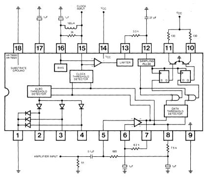
Figure 3. A.C. Parameter Test Circuit
