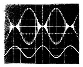
Figure 7-1. AM Modulation, 95% AM,  $\rm f_{C}$  = 50 kHz,  $\rm f_{M}$  = 1 kHz
