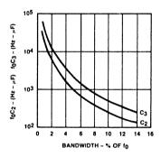
Figure 10. Detection Bandwidth as a Function of  $C_2$  and  $C_3$
