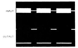
Response to 100 mV rms tone burst. R<sub>1</sub> = 100 ohms.
