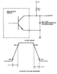
Figure 1. Common-Emitter Configuration
