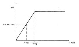
Figure 10. Differentiator Response for Cn and R
