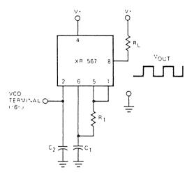
Figure 23. Precision Oscillator to Switch 100 mA Loads
