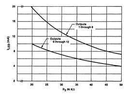
Figure 4. Output Drive Current as a Function of Current Setting Resistor, R<sub>2</sub>
