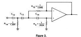
After calculating  $\mathsf{R}_X$  remember for single supply operation the op amp must be biased at 1/2 V<sub>CC</sub>; therefore take twice the calculated value for  $\mathsf{R}_X$  and configure as shown in Figure 4.
