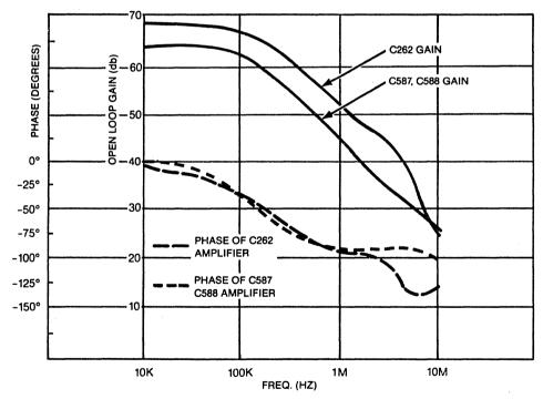
Figure 1. Bode Plot of C262 and C587/C588 Amplifiers
