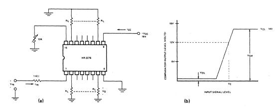
Figure 1. Basic Test Circuit: (a) Circuit Connection, (b) Output Waveform.
