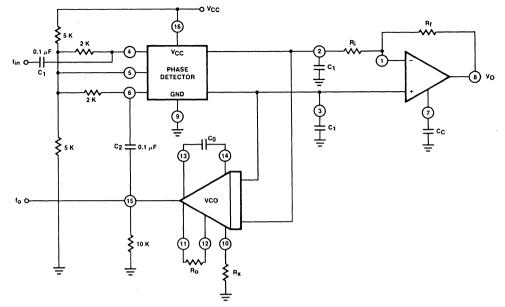
Figure 2. XR-215 with External Components.
