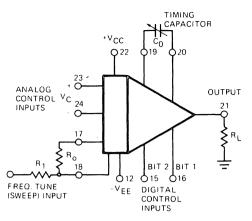
Figure 11. XR-S200 Oscillator Section
