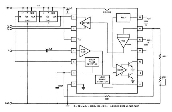
Figure 5. Frequency Synthesizer
