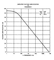
Figure 6. Amplifier Voltage Amplification vs Frequency
