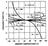
Figure 8. Frequency Drift versus Temperature.
