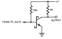
(b) Output Interface Circuit Figure 12. Tyipcal Bipolar I/O Interface Circuits.
