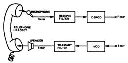
Figure 14. Acoustical Coupling
