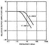
Figure 8. Small-Signal Frequency Response for the Multiplier Section. (Output Measured at Pin 15—See Fig. 4).
