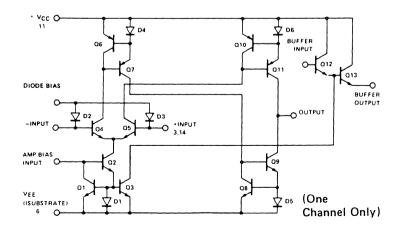
EQUIVALENT SCHEMATIC DIAGRAM
