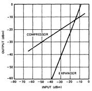
Figure 2. Transfer Characteristics of Compressor a Expander Circuits
