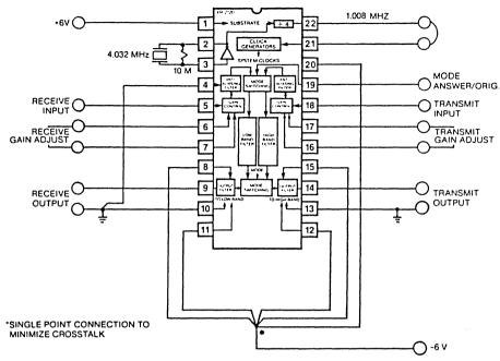
Figure 1. Typical Split Supply Connection.
