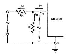
Figure 12. Frequency Sweep Operation
