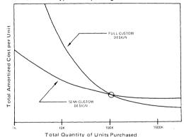
Figure 15. A Comparison of Relative Cost Advantages of Semi-Custom and Full Custom LSI Products. (NOTE: Amortized cost per unit includes the development cost.)
