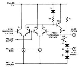
Figure 7. Circuit Diagram of the Peak-Detector and the ALBO Sections.
