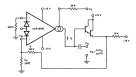
Figure 8. Voltage Controlled Resistor, Single-Ended
