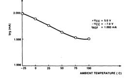
Figure 8. IFS vs. Temperature
