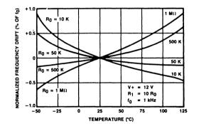
Figure 8. Typical Center Frequency Drift vs Temperature
