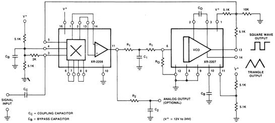
Figure 3. Circuit Interconnections for Single Supply Operation.
