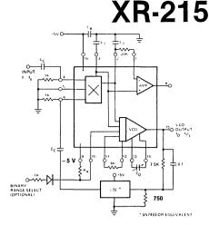
Figure 22. Circuit Connection For Frequency Synthesis
