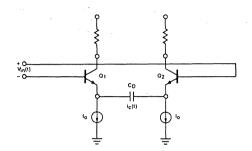
Figure 9. Simplified Active Differentiator Section
