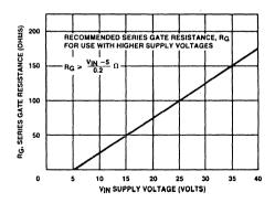
Figure 6. SCR Trigger—Series Gate Resistance (R<sub>G</sub>) vs. Input Voltage
