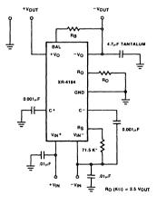
For Best Tracking Temperature Coefficient of Ro Should Be Same As For RS Adjust Ro for "Vs = 6 V (15 Kii) then Adjust Rg for \*Vs = 12 V (20 Kii)
