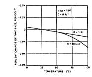
Figure 14. Temperature Drift of Time-Base Period, T
