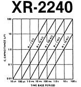
Figure 9. Time-Base Period, T, as a Function of External RC
