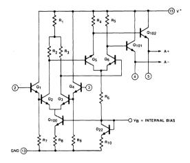
Figure 7. Circuit Diagram of Preamplifier Section.
