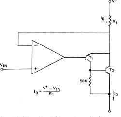
Figure 13. Voltage-Controlled Current-Source Circuit
