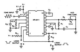
Figure 11. Circuit Connection for Tone Detection
