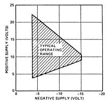
Figure 3. Typical Operating Range For Split Supply Voltage
