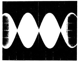
Figure 22-2. Suppressed Carrier AM Output Waveform  $f_{carrier} = 3.688 \text{ MHz} f_{mod} = 1 \text{ kHz}$
