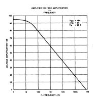
Figure 6. Amplifier Voltage Amplification vs Frequency
