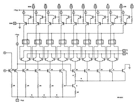
Figure 3A. Equivalent Circuit of Data Latches and Current Switches
