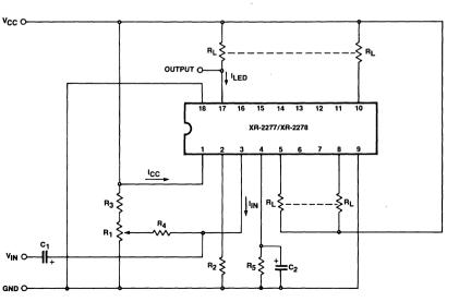
$R_1 = 500\Omega$  $R_2 = 27K\Omega$  $R_3 = 330K\Omega$  $R_4 = 10K\Omega$  $R_5 = 10K\Omega$  $C_1 = 2.2 \mu F$  $C_2 = 10\mu F$  $R_L = 200\Omega$
