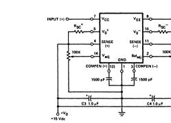
C1 and C2 should be located as close to the device as possible. A 0.1 µF ceramic capacitor may be required on the input lines if the device is located an appreciable distance from the rectifier filter capacitors. C3 and C4 may be increased to improve load transient response and to reduck the output noise voltage. At low temperature operation, it may be necessary to bypass C4 with a 0.1 µF ceramic disc capacitors.
