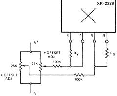
Figure 13. Offset Adjustment
