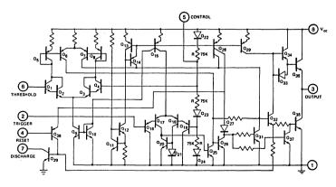
EQUIVALENT SCHEMATIC DIAGRAM
