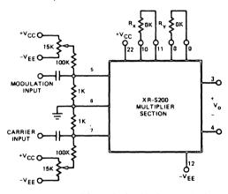
Figure 6. Suppressed Carrier Modulation Using XR-S200 Multiplier Section
