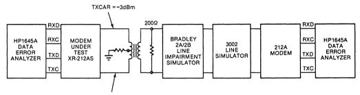
CONDITIONS: RXCAR = -40 dBM, NOISE LEVEL = -52 dBM (S/N = 12 dB), HIGH SPEED MODE (1200 BPS) DETURN LOSS = -4 dB 511 DATA DATTERN
