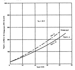
Figure 6. Output Saturation Voltage vs Load Current
