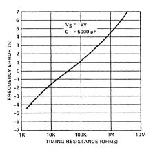
Figure 5. Frequency Accuracy vs. Timing Resistance
