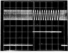
Figure 26. Input and Output Waveforms for FSK Decoding Top: Input FSK Signal (f<sub>2</sub> = 3f<sub>1</sub>) Bottom: Demodulated Output
