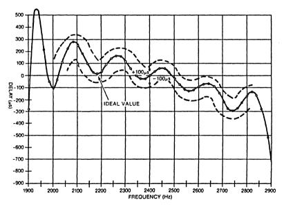
Figure 8. High Band Group Delay Characteristics
