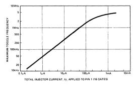
Figure 6. Typical Maximum Toggle Frequency vs. Injector Current Characteristics for XR-C409 Frequency Divider Section
