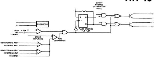
EQUIVALENT SCHEMATIC DIAGRAM
