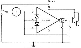
LEAKAGE CURRENT TEST CIRCUIT
