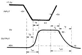
Figure 3. AC Test Waveforms
