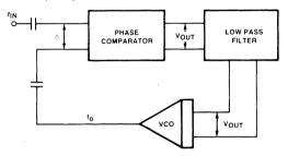
Figure 1. Phase Locked Loop Functional Diagram.
