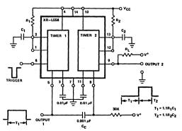
Figure 16. Sequential Timing
