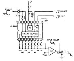
Figure 26. Staircase Generator
