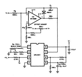
Figure 4. Precision Voltage-to-Frequency Converter
