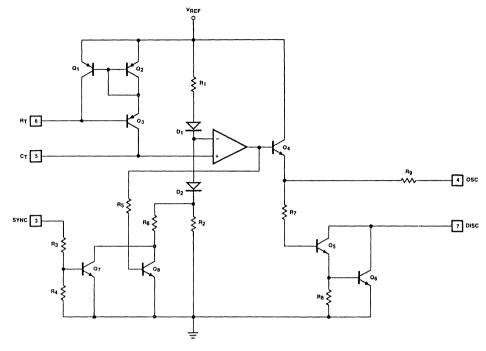
Figure 8. Equivalent Schematic of the Oscillator Section
