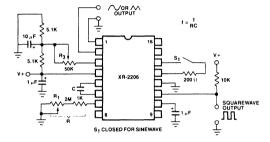
Figure 10. Circuit for Sine Wave Generation without External Adjustment. (See Figure 2 for Choice of R<sub>3</sub>).
