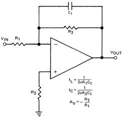
Figure 9. A Simple Low-Pass Filter Circuit
