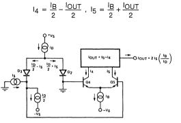
Figure 1. Linearizing Diodes
