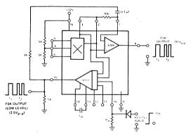
Figure 21. Circuit Connection For FSK Generation
