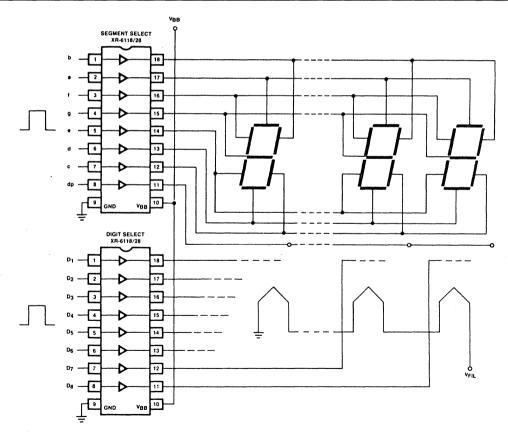
Figure 2. Typical Multiplexed Fluorescent Display Drive Application
