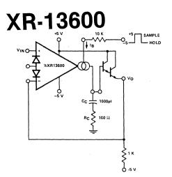
Figure 24. Sample-Hold Circuit
