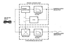
Figure 2. The Basic Phase-Locked Loop AM Detector.
