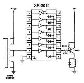
Figure 8. Buffer for Higher Current Loads
