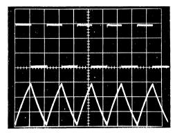
Figure 22. Oscillator Output Waveform Available From CCO Section.
