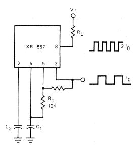
Figure 25. Oscillator with Double Frequency Output
