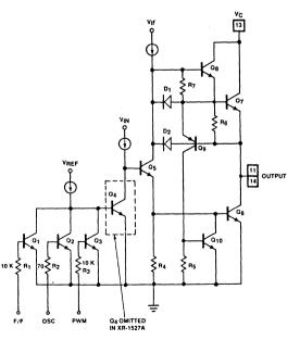
Figure 10. Equivalent Schematic of Output Drivers
