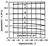
Figure 12. Bandwidth Variation With Temperature
