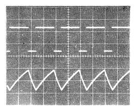
Figure 16. Astable Waveforms Top: Output Waveform Bottom: Waveform Across Timing Capacitor
