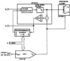
Figure 5. Wide Range Synthesizer Block Diagram.
