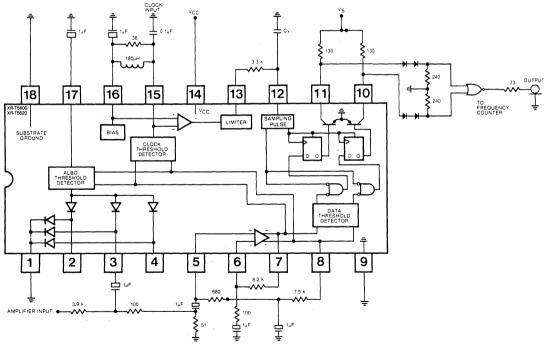
Figure 4. Sampling Pulse Test Circuit
