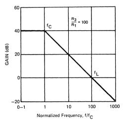
Figure 10. Frequency Response of the Simple Low-Pass Filter
