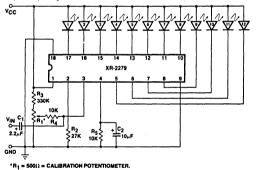
Figure 5. Circuit Connection for Moving-Dot Display Generation
