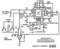
Figure 2. Linearity Test Circuit
