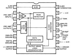
Figure 3. Package Diagram of XR-C277 Monolithic PCM Repeater
