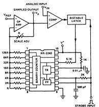
Figure 27. Digital Sample and Hold Circuit
