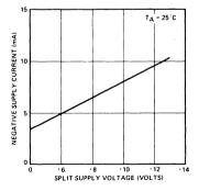
Figure 19. Negative Supply Current, I<sup>—</sup> (Measured at Pin 12) vs. Supply Voltage
