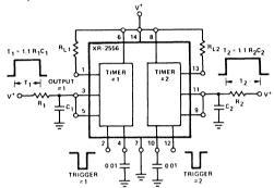
Figure 20. Generation of Two Independent Time Delays
