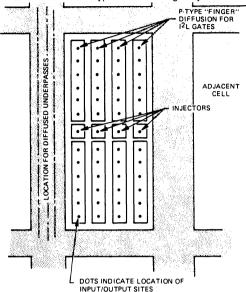
Figure 5. Basic 8-Gate Cell Before Customization.
