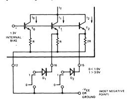
Figure 15. Explanation of VCO Digital Controls
