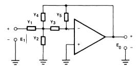
Figure 3. Multiple Feedback Connection with Noninverting Input Grounded.
