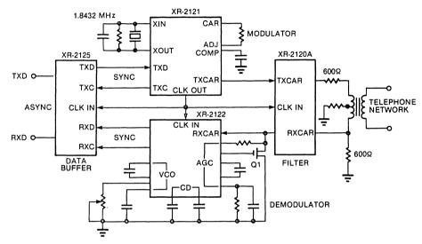
Figure 3. Complete Modem Signal Processor
