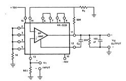
Figure 6. Op Amp AC Test Circuit
