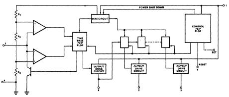
Figure 1. Simplified Circuit Schematic
