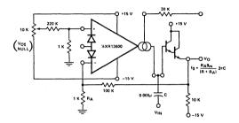
Figure 12. Voltage Controlled High-Pass Filter
