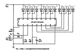
Figure 6. Circuit Connection for Bar-Graph Display Generation
