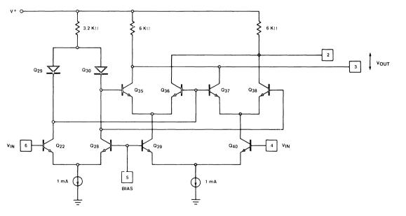
Figure 2. XR-210/XR-215 Phase Comparator.
