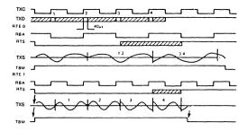
Figure 1. Timing Diagram of the Transmitter
