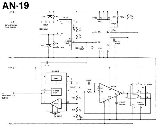
P1 = > ADJUST SO POSITIVE PORTION OF fi IS EQUAL TO  $^{1}_{2}$  OF THE CLOCK PERIOD P2 = > ADJUST FOR 90 PHASE SHIFT BETWEEN ft and fo WITH fi = fCLK
