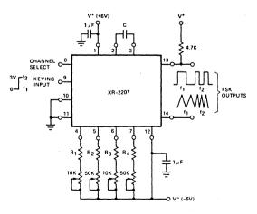
Figure 16. Multi-Channel FSK Generation
