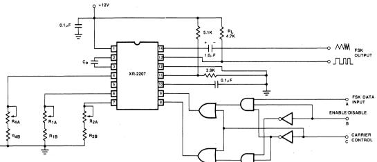
Figure 4. Three-State FSK Transmitter Using the XR-2207.
