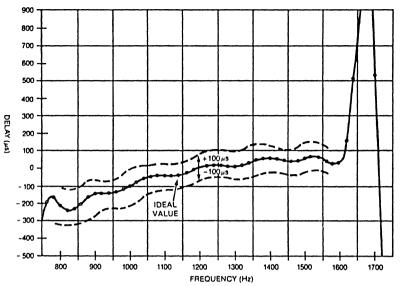
Figure 7. Low Band Group Delay Characteristics
