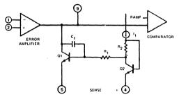
Figure 7. Current Limiting Circuitry of the XR-1524
