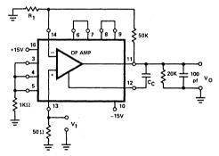
Figure 6. Op Amp AC Test Circuit
