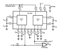
Figure 23. Connection for Decoding Dual-Tone Encoded Input Signals
