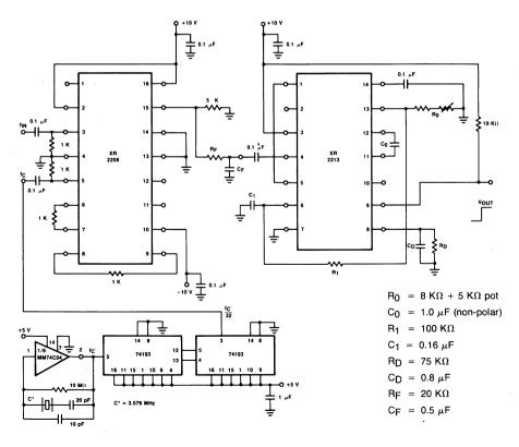
Figure 3. Circuit Schematic of Narrow Band Tone Decoder.
