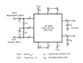
Figure 4. XR-S200 Multiplier Section as a Phase Comparator
