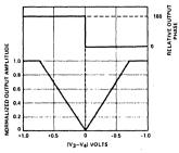
Figure 5. Modular Section Phase and Amplitude Transfer Characteristics
