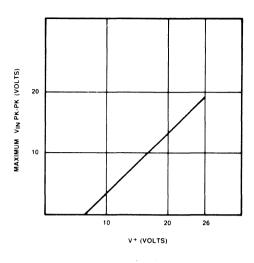
Figure 10. Maximum Input Voltage vs. Supply Voltage.
