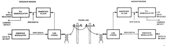
Figure 1. Block Diagram of FSK Modem System.
