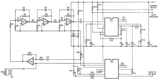
Figure 2. Complete FSK Modem Using XR-2211 and XR-2206.
