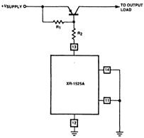
Figure 11. Single-Ended Output for XR-1525A
