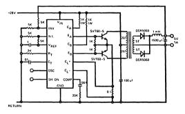
Figure 17. A High-Current DC-DC Converter with Push-Pull Outputs (Vin = +28V, V\_0 = +5V, I\_0  $\leq$  5A)
