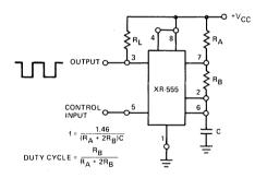
Figure 2. Astable (Free-Running) Circuit
