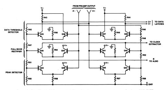
Figure 9. Data-Threshold Detector, Full-Wave Rectifier and The Peak Detector Sections of XR-C277
