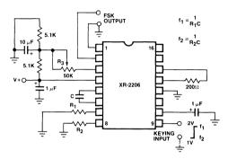
Figure 12. Sinusoidal FSK Generator.
