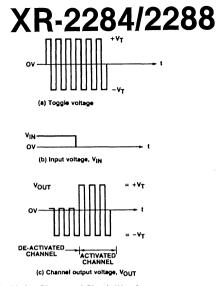
Figure 3. Timing Diagram of Circuit Waveforms
