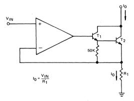
Figure 12. Voltage-Controlled Current-Sink Circuit
