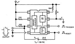
Figure 8. Circuit Connection for Timing Applications (Switch S<sub>1</sub> Open for Astable Operations, Closed for Monostable Operations)
