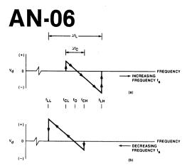
Figure 2. Frequency to Voltage Transfer Characteristics of a PLL System; (a) Increasing Input Frequency; (b) Decreasing Input Frequency.
