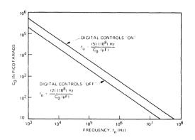
Figure 12. VCO Frequency as a Function of Timing Capacitor, C<sub>0</sub>
