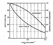
Figure 6. Duty-Cycle and Frequency Variation as a Function of Resistor  ${\rm R}_B$  Connected Across Pins 13 and 14
