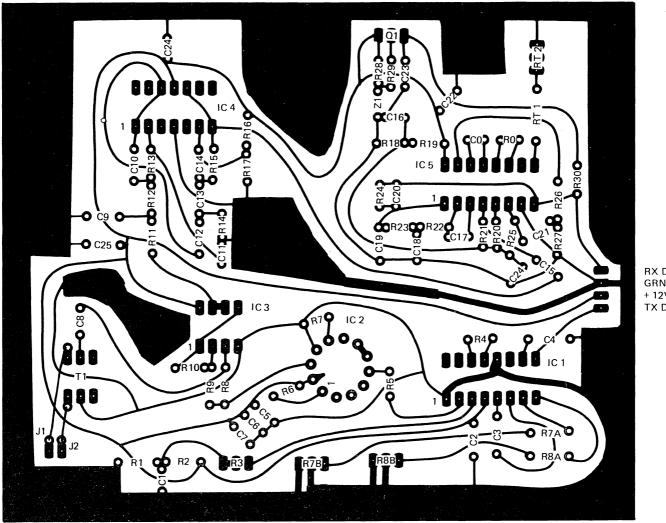
Figure 7. P.C. Board Layout for 100 Kilobaud FSK Modem-Component Side
