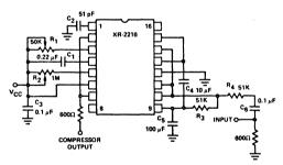
Figure 4. External Connections for Compressor Operation
