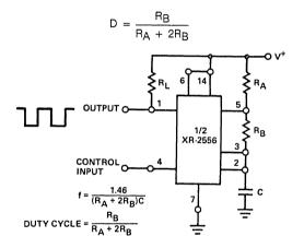
Figure 15. Astable (Free-Running) Circuit
