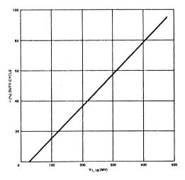
Figure 2. Modulation Duty Cycle vs Error Voltage
