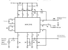
Figure 3. Test Circuit For Split-Supply Operation
