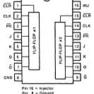
XR-C505 contains two independent J-K flip-flops which share a common injector. Both the inputs and outputs are comprised of unbuffered I<sup>2</sup>L gates. Both flip-flops are positive edge triggered.
