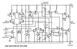
EQUIVALENT SCHEMATIC DIAGRAM
