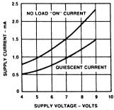
Figure 8. Supply Current Versus Supply Voltage
