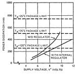
Figure 5. Internal Power Dissipation vs. Supply Voltage. Both Units Activated,  $R_L = 20 \text{ k}$
