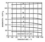
Figure 13. Bandwidth Variation With Temperature
