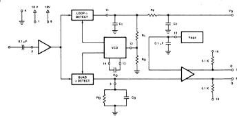
Figure 4. F/V Circuit Diagram.
