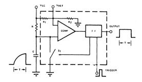
Figure 1. Exponential-Ramp Type Timing Circuit
