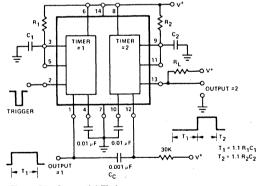
Figure 21. Sequential Timing
