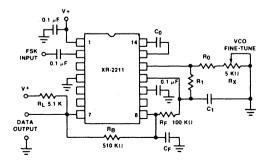
Figure 9. Circuit Connection for FSK Decoding
