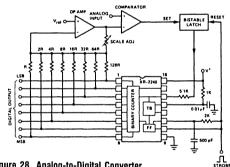
Figure 28. Analog-to-Digital Converter
