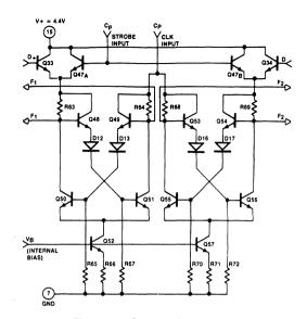
Figure 11. Data-Latch Section of XR-C277
