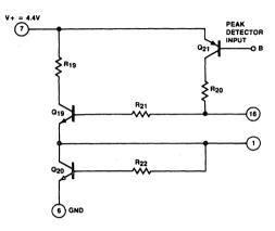
Figure 8. Automatic Line Build-Out (ALBO) Section
