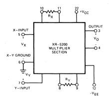
Figure 2. XR-S200 Multiplier Section
