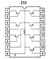
NOTE: 5 Small & 2 Large Vertical PNP's. Resistance shown is substrate resistance between middle and edge of die.
