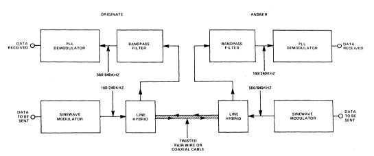
Figure 1. Block Diagram of High Speed FSK Modem System
