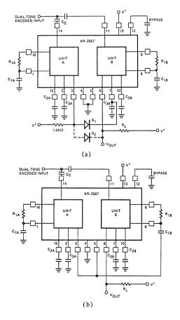
Figure 24. Additional Dual-Tone Decoding Circuits
