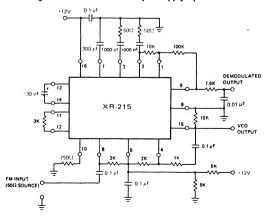
Figure 4. Test Circuit For FM Demodulation
