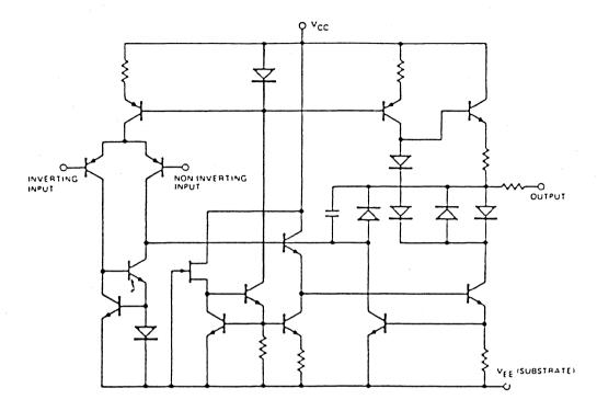
EQUIVALENT SCHEMATIC DIAGRAM
