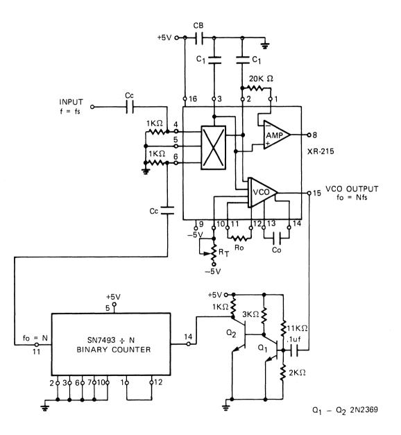
Figure 3. High Frequency Synthesis Circuit.
