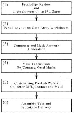
Figure 13. Sequence of Steps Associated with a Semi-Custom LSI Development Cycle.
