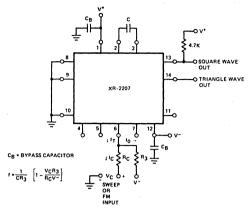
Figure 12. Frequency Sweep Operation
