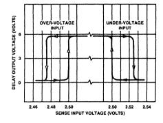
Figure 4. Over-Voltage and Under-Voltage Comparator Hysteresis
