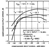
Figure 7. XR-2216 Compandor Tracking Error vs. Input Signal
