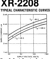
Figure 7. Supply Current vs Supply Voltage
