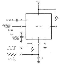
Figure 3. XR-567 Connection Diagram
