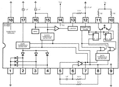
Figure 2. D.C. Parameter Test Circuit
