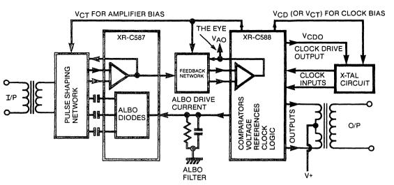
Figure 2. Block Diagram of C587/C588 Interconnected
