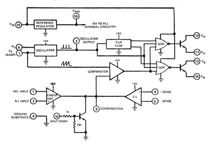
Figure 1. Detailed System Block Diagram of XR-1524
