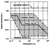
Figure 4. R versus Oscillation Frequency.
