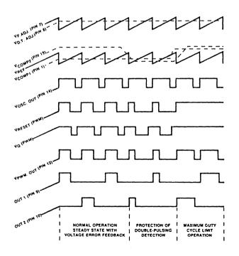
Figure 10. Timing Waveform Diagram
