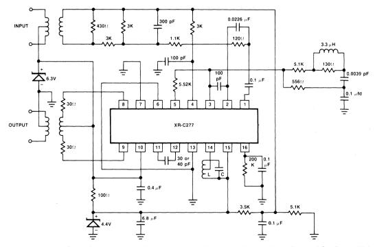
Figure 6. Typical Circuit Connection of XR-C277 in 1.544 MHz T-1 Repeater System. (Note: Set L and C to Form a High Q Tank Resonant at 1.544 MHz. It is Recommended that Q∂100, and C ≈ pF for most applications).
