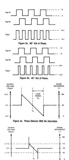
Figure 4b. Phase Detector With Saturation.
