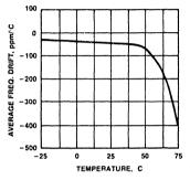
Figure 15. Typical Center Frequency Drift With Temperature (V  $^+~=~$  5V, R  $_1~=~$  80 kΩ, f  $_0~=~$  1 kHz)
