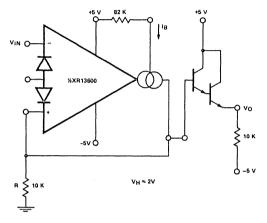
Figure 22. Schmitt Trigger
