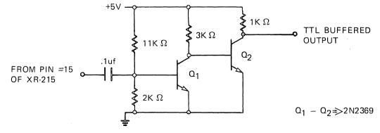
Figure 2. Common Emitter Buffer Circuit.
