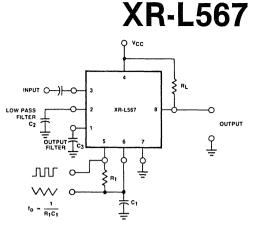
Figure 2. XR-L567 Generalized Connection Diagram
