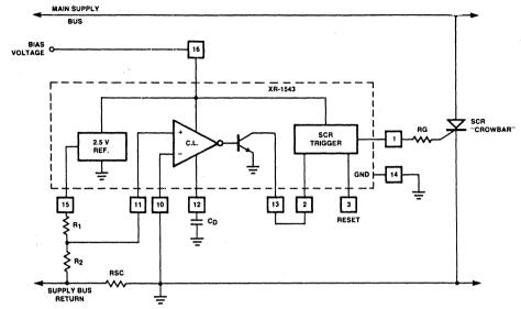
Figure 11. XR-1543-Over Current Shutdown Circuitry
