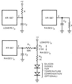
Figure 16. Connections to Reposition Detection Band
