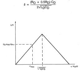
Figure 11. Differentiator Response with RD, CD, and L
