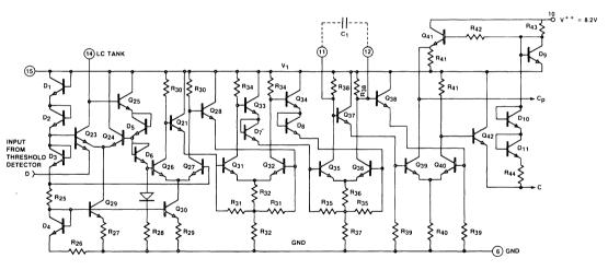
Figure 10. Circuit Diagram of Clock Extractor Section.
