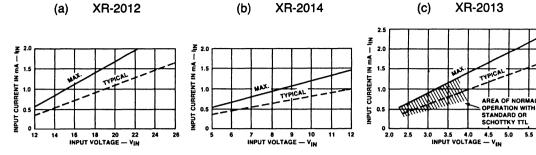
Figure 1. Input Current as a Function of Input Voltages
