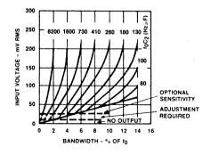
Figure 11. Bandwidth Versus Input Signal Amplitude (C2 in  $\mu$ F)
