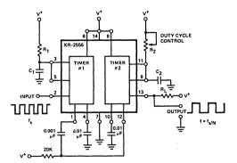
Figure 24. Frequency Divider and Pulse-Shaper
