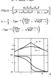
Band Reject  $H(s) = \frac{(s^2 + \omega \sigma^2)H\sigma}{s^2 + \omega \sigma \sigma s + \omega \sigma^2}$
