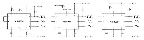
Figure 2. Possible Connections for the External Timing Resistors.
