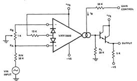
Figure 2. Voltage Controlled Amplifier (VCA) Circuit
