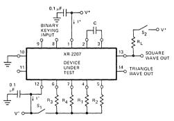
Figure 1. Test Circuit For Split Supply Operation
