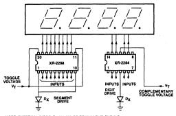
NOTE: EXTERNAL DIODE, D<sub>X</sub> (IN4002 OR EQUIVALENT) SHOULD BE SEPARATE FOR DIGIT AND SEGMENT SIDES
