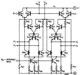
Figure 11. Data Output Latches (Logic Section).
