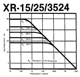
Figure 5. Error Amplifier Frequency Response as a Function of External Resistor, RL, at Pin 9
