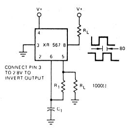
Figure 24. Oscillator with Quadrature Output
