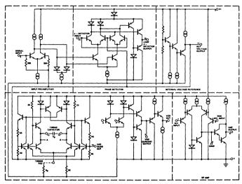
Figure 3. Simplified Circuit Schematic of XR-2212
