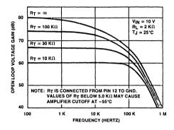
Figure 3. Current Limiting Amplifier Gain vs. Threshold Setting Resistor (R<sub>T</sub>
