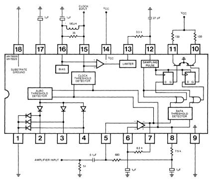
Figure 3. A.C. Parameter Test Circuit
