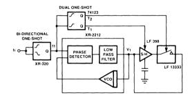
Figure 2. Clock Regenerator Block Diagram.
