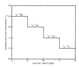
Figure 13. VCO Digital Tuning Characteristics
