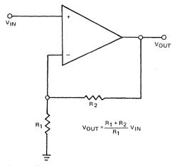
Figure 2. Non-Inverting Amplifier
