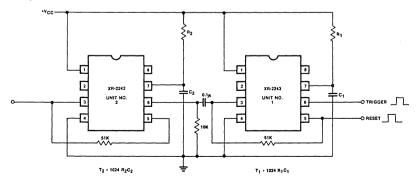
Figure 5. Sequential Timing Using XR-2243 Timer Circuits
