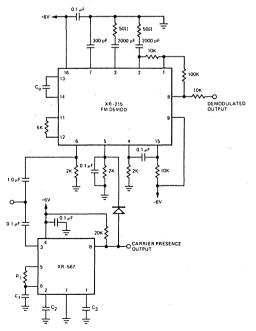
Figure 20. Narrow Band FM Demodulator with Carrier Detect
