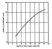
Figure 7. Supply Current vs. Supply Voltage in Reset Condition (Supply Current Under Trigger Condition is  $\approx 0.7 \text{ mA less}$ )
