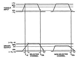
Figure 2. Typical Timing Waveforms
