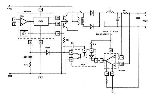
Figure 12. XR-1543 - DC Converter with Isolated Current Limiting
