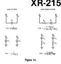
and 3. The low-pass filter components can be connected either between pins 2 and 3 or, from each pin to ground. Typical filter configurations and corresponding filter transfer functions are shown in Figure 14 where R<sub>1</sub> (6 k $\Omega$ ) is the internal impedance at pins 2 and 3.
