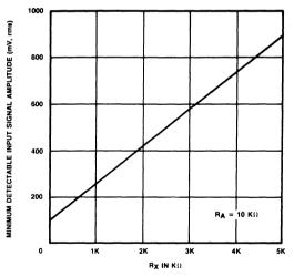
Figure 7. Minimum Detectable Input Carrier Level, as a Function of Multiplier Gain Setting Resistor, R<sub>X</sub>.
