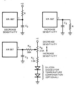
Figure 14. Optional Sensitivity Connections
