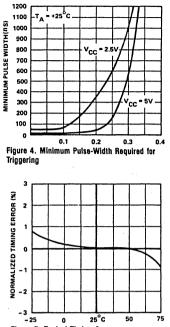
Figure 7. Typical Timing Accuracy as a Function of Temperature ( $V_{CC} = 51V$ ,  $R_A = 100K\Omega$ ,  $C = 0.01 \mu F$ )
