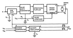
Figure 5. Steering Servo System
