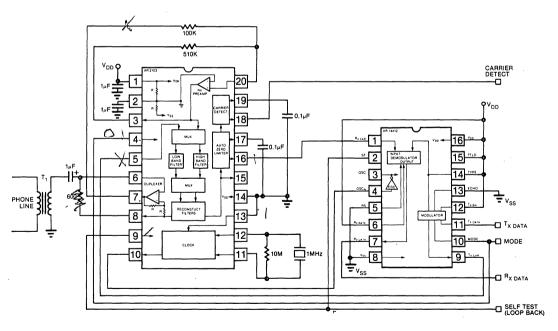
Figure 4. Bell 103 Compatible Modem
