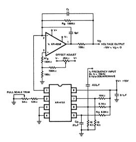
Figure 6. Precision Frequency-to-Voltage Converter
