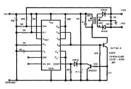
Figure 15. A Low-Current DC-DC Converter Using Flyback Principle (Vout =  $\pm$  15V, Vin = +5V, IL  $\leq$  20 mA)
