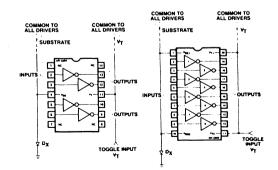
Figure 4. Generalized Connection Diagram XR-2284 and XR-2288.
