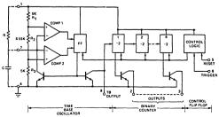
EQUIVALENT SCHEMATIC DIAGRAM
