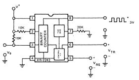
Figure 3. Generalized Test Circuit
