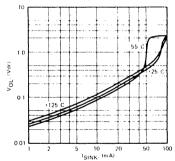
Figure 11. Low Output Voltage  $V_{CC} = 15 Vdc$
