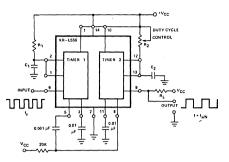
Figure 18. Frequency Divider and Pulse-Shaper
