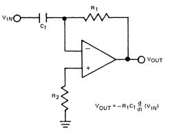
Figure 6. Basic Differentiator Connection
