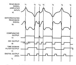
Figure 7a-f. Waveforms Through the XR-3470A/3470B
