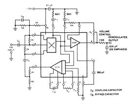
Figure 15. Circuit Connection for FM Demodulation
