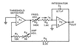
Figure 15. A Simple Triangle Wave Oscillator
