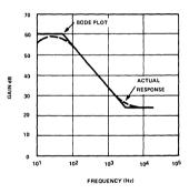
BODE PLOT OF NAB EQUALIZATION AND THE RESPONSE REALIZED IN THE ACTUAL CIRCUIT USING THE XR-5533
