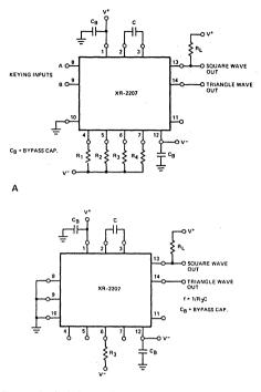
Figure 10. Split-Supply Operation: (a) General (b) Fixed Frequency
