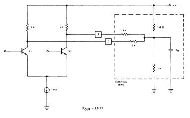
Figure 5. External Resistor Bias Network.
