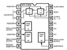
Figure 1. Package Terminals for XR-C409 Test IC.
