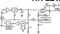
Figure 2. Generalized Circuit Connection for FM Detection, Signal Tracking or Frequency Synthesis
