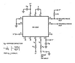
Figure 13. Alternate Frequency Sweep Operation
