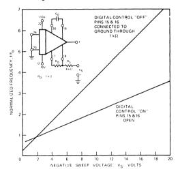
Figure 14. Voltage Sweep Characteristics
