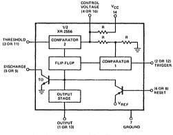
Figure 2. Functional Diagram of One Timer Section
