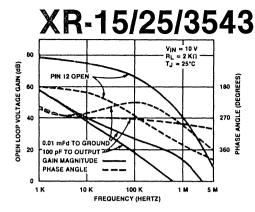
Figure 2. Current Limiting Amplifier—Frequency Response
