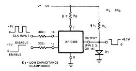
Figure 4. Test Circuit for Frequency Divider Section.
