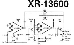
Figure 21. Phase-Locked Loop
