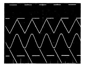
Figure 21-1. Basic Waveforms Available from XR-S200
