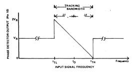
Figure 9. Phase Detector Output Voltage (Pin 10) as a Function of Input Signal Frequency. Note: Output Voltage is Referenced to Internal Reference Voltage V<sub>R</sub> at Pin 11
