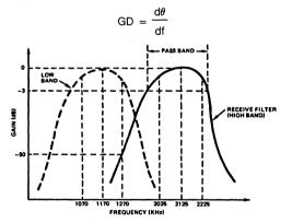
Figure 12. 103 FSK Receive Filter
