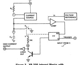
Figure 3. XR-320 Internal Blocks with External Components.
