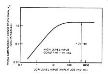
Figure 8. Phase Comparator Conversion Gain, K<sub>d</sub>, versus Input Amplitude
