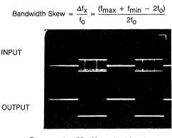
Response to 100 mV rms tone burst.  $R_L = 1K$  ohms
