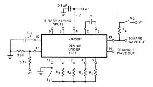
Figure 2. Test Circuit For Single Supply Operation
