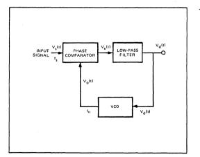
Figure 1. The basic phase locked loop consists of three functional blocks: a phase comparator, a low pass filter and a voltage-controlled oscillator.
