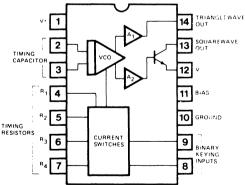
Figure 1. Functional Block Diagram of XR-2207 Oscillator Circuit.
