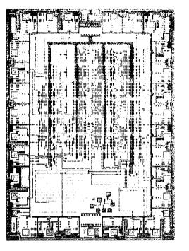
Figure 14. Photo-Micrograph of a Typical Semi-Custom  $\ensuremath{I^2L}$  LSI Chip.
