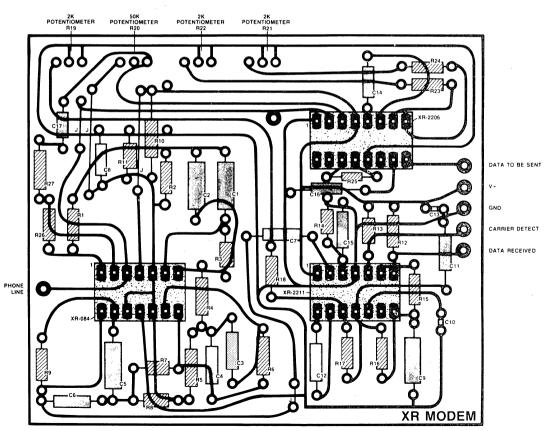
Figure 3. XR Modem Foil Side Shown (Not to Scale).
