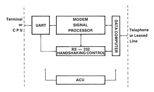
Figure 1. Modem Block Diagram
