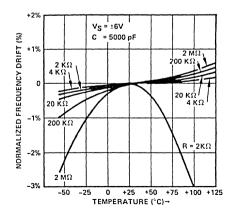
Figure 7. Normalized Frequency Drift With Temperature
