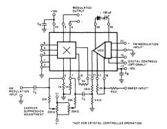
Figure 22. Circuit Connection for AM/FM or Crystal-Controlled AM Generator Application
