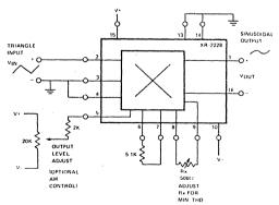
Figure 19. Triangle-to-Sinewave Converter
