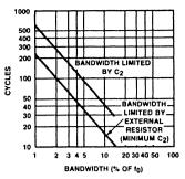
Figure 13. Greatest Number of Cycles Before Output
