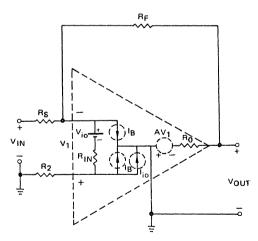
Figure 3. Equivalent Circuit of a Practical Operational Amplifier Showing the Effects of Finite Input Impedance, Current and Voltage Offsets
