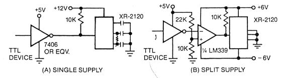
Figure 5. TTL Interfacing of Digital Inputs
