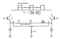
Figure 12. Nulling Network to Minimize Peak Shift (PS)
