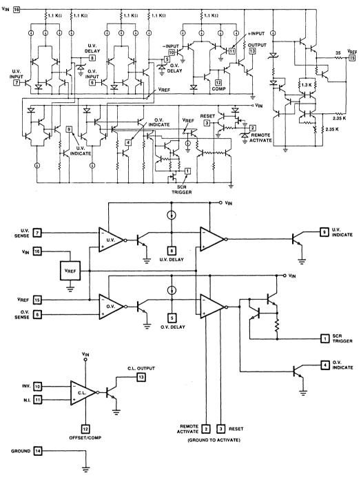
Figure 7. XR-1543 Block Diagram
