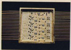
With custom hybrids, your only limitation is your imagination. You'll be amazed by the variety and number of parts that we can put in a package. In our unique facility, our craftsmen produce thin film and thick film hybrid microcircuits ranging from simple multiple-chip circuits to complex multi-layered assemblies.
