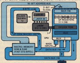
Diagram shows 16-bit minicomputer constructed from 3000-Series parts. Although slices are only two bits wide, they include a large number of parallel paths for high processing throughput.
