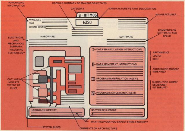
Legend diagram for EDN's µP files with the various "information spaces" called out and explained. The information is purposely equally divided into a hardware half and a software half to emphasize the "two-sided" nature of these SP/GP/DC-type products. (SP/GP/DC stands for stored program, general-purpose digital computer.)
