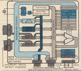
HARDWARE SUPPORT: Special 64-pin device for prototyping 660X's ROM can carry "KIM" or "TIM" monitors, so users can develop stand-alone prototyping stations. Besides 650X parallelbus support chips, 660X will have serial-bus peripheral devices
