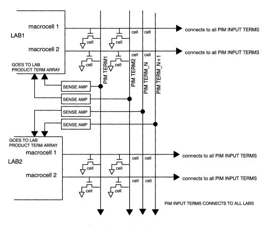
Figure 3. Array-Based Interconnect
