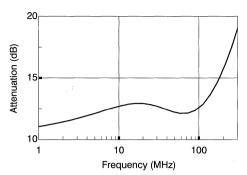
Figure 12. Combined Cable and Equalizer Attenuation
