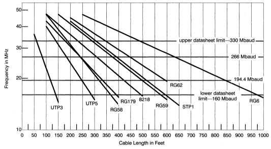
Figure 5. Maximum Data-Rate versus Distance Comparison
