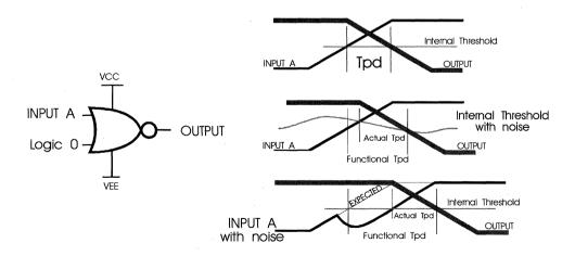
Figure 3. Delay Through a Logic Gate Changes with Injected Noise
