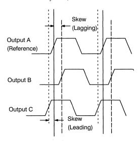
Figure 5. Graphical Representation of Skew
