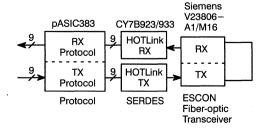
Figure 5. Design Example Structure
