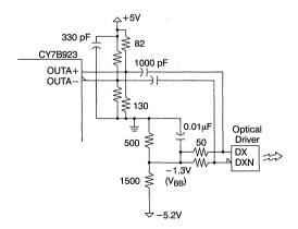
Figure 30. HOTLink Transmitter-to-Negative-Referenced ECL Optical Module
