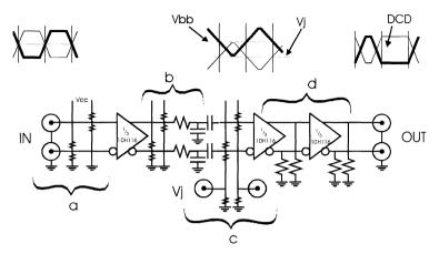
Figure 49. Duty Cycle Distortion Jitter Generator Schematic
