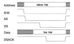
Figure 4. 680x0-Compatible Write Cycle
