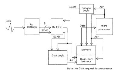
Figure 5. Dual-Ported Configuration
