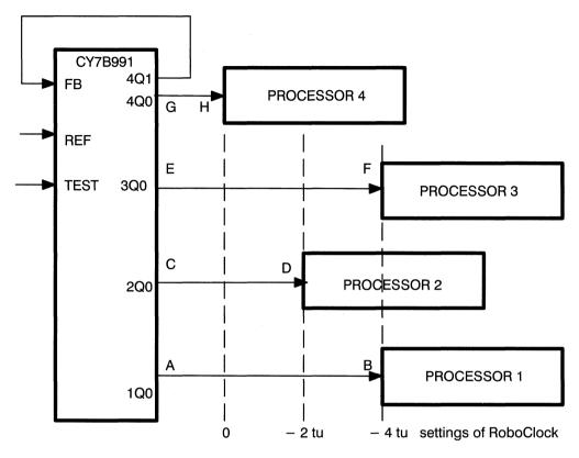
Figure 3. One RoboClock Driving Multiple Processors
