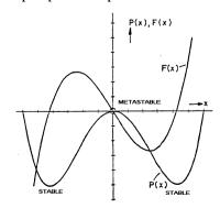
Figure 9. Energy/Force Function of a Bistable System
