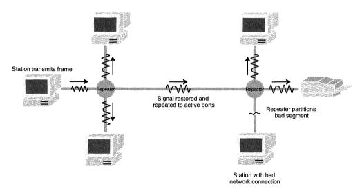
Figure 1. Ethernet Network Built with Repeaters
