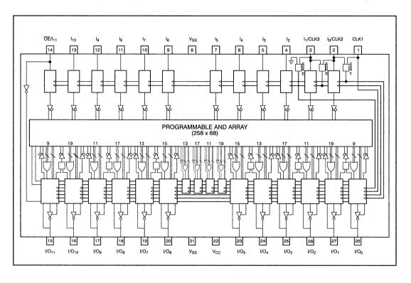
Figure 1. CY7C335 Block Diagram
