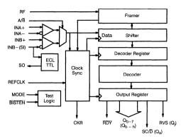
Figure 3. CY7B933 Receiver Logic Block Diagram
