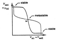
Figure 11. Energy Transfer Diagram of Simple RS Flip-Flop
