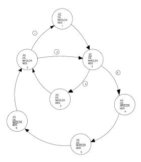
Figure 7. 680x0 Bus Cycle State Machine
