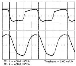
Figure 34. Thévenin Bias, Direct-Coupled, No Cable, 93Ω Load
