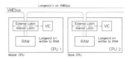
Figure 4. Block Transfer Read Cycle
