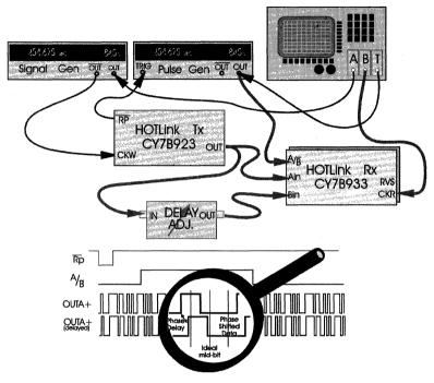
Figure 39. Set-Up to Measure HOTLink Phase Acquisition Characteristics
