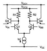
Figure 5. Buffered ECL Switch
