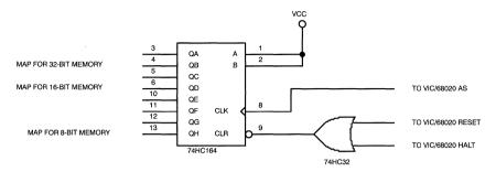
Figure 1. ROM Remapping Circuit
