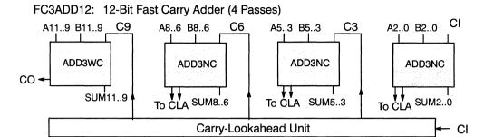
Figure 8. 12-Bit Full Carry-Lookahead Adder using ADD3WC and ADD3NC
