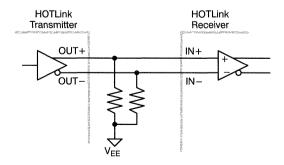
Figure 18. Differential Connection
