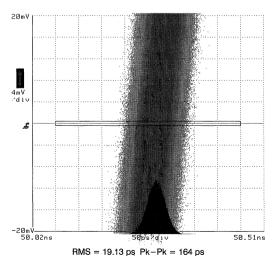
Figure 16. HOTLink Transmitter OUTA± Rj vs. CKW
