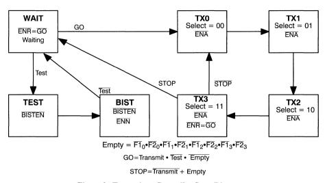
Figure 2. Transmitter Controller State Diagram
