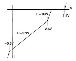
Figure 23. Output HIGH Linearized V-I Curve
