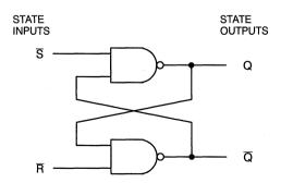
Figure 1. SR Latch, Asynchronous State Machine Example
