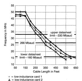
Figure 3. RG59 Test Results, Linear Frequency Scale
