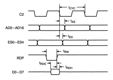
Figure 2. Expansion Bus Read Waveform
