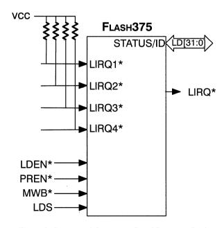
Figure 8. Inputs and Outputs to Local Interrupt Logic
