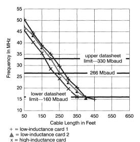
Figure 2. RG58 Test Results, Linear Frequency Scale
