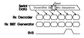
Figure 9. RVS Indicates Errors in Received Sequence
