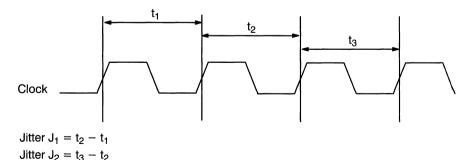
Figure 2. Cycle-Cycle Jitter
