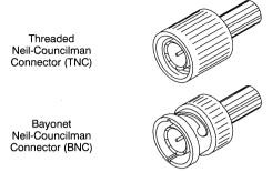
Figure 78. TNC/BNC Cable Connectors
