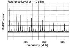
Figure 50. 0000011111 (K28.7) Pattern Spectral Characteristics
