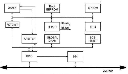
Figure 2. Typical VMEbus Design
