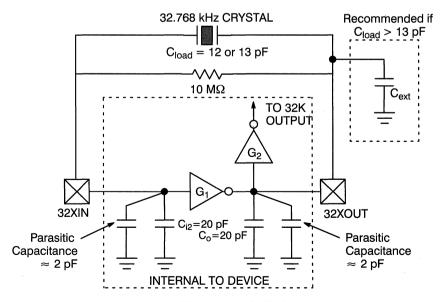
Figure 4. Using a 32.768 kHz Crystal
