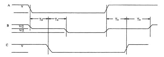
Figure 15. Series Damping Timing
