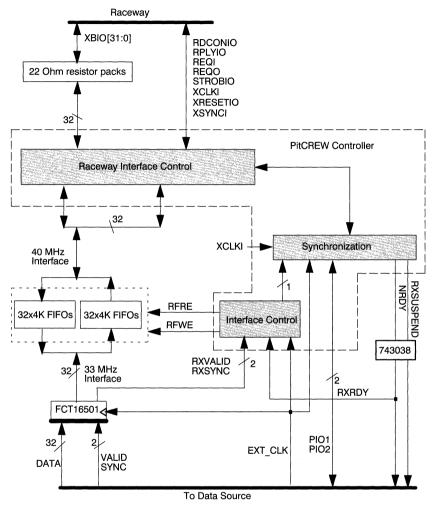
Figure 2. Architecture of a Sample Input Interface Using PitCREW
