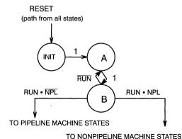
Figure 3. CPU Inactive States
