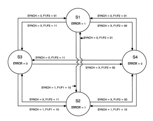
Figure 18. Metastability Testing State Diagram
