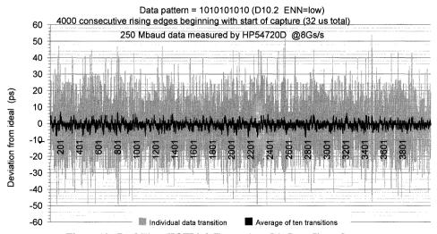
Figure 19. Real-Time HOTLink Transmitter Bit-Rate Jitter Output
