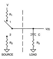
Figure 18. Lumped Load; AC Termination
