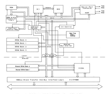
Figure 5. CY7C611A/VIC64 VMEbus Board Block Diagram
