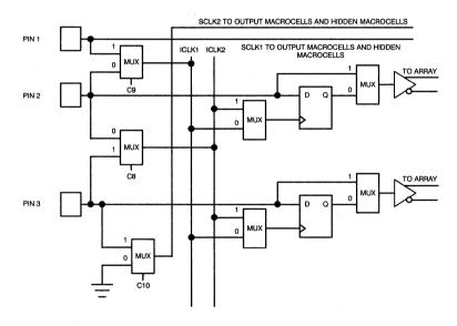
Figure 5. CY7C335 Input Clocking Scheme
