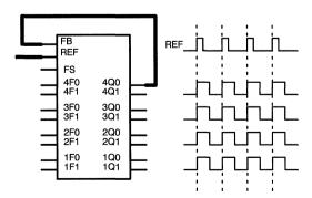
Figure 33. Low-Skew Clock Buffer
