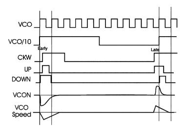
Figure 7. Phase/Frequency Corrections in Multiplier PLL
