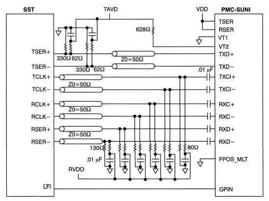
Figure 5. High Performance SST to PMC SUNI Interface
