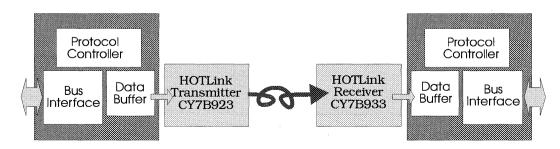
Figure 1. Typical Data-Communication Link using HOTLink
