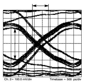
Figure 37. Eye Diagram, Thévenin Bias, Direct-Coupled, with  $50\Omega$  Cable
