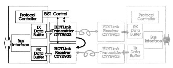
Figure 5. Local Loop Back Testing
