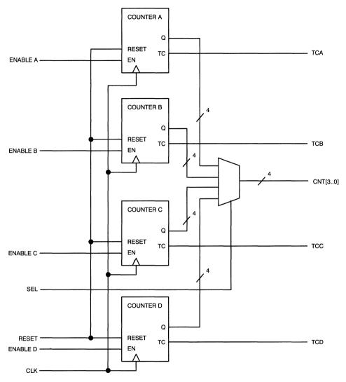
Figure 2. Multiplexed Quad Counter Design
