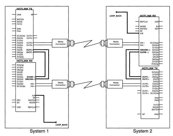
Figure 8. Example HOTLink Loop-Back System Connection
