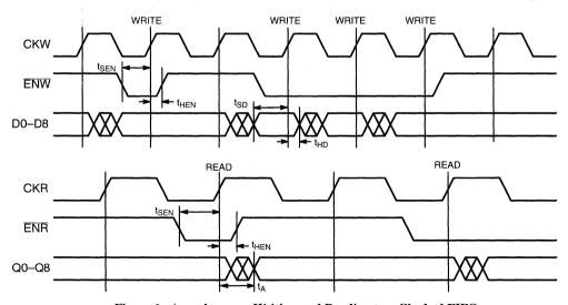
Figure 1. Asynchronous Writing and Reading to a Clocked FIFO
