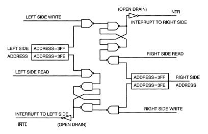
Figure 2. Interrupt Logic
