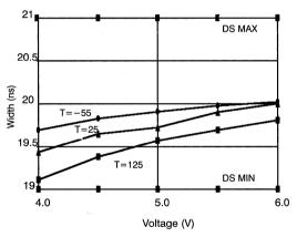
Figure 64. Pulse Width High vs. Voltage over Temperature
