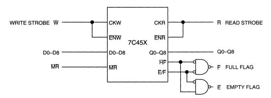
Figure 8. Using a Clocked FIFO Like a Standard FIFO
