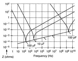
Figure 64. Capacitor Impedance vs. Frequency
