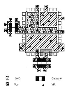
Figure 7. Sample RoboClock Layout
