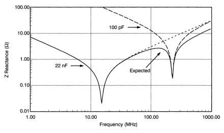
Figure 3. Expected Impedance of "Real" Capacitors
