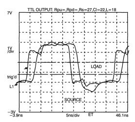
Figure 27. Series Terminated, 22-pF Load
