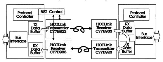
Figure 6. Long Loop Back Testing
