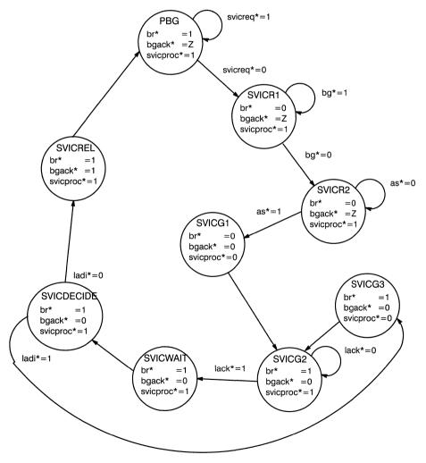
Figure 8. State Diagram of SVIC to 68020 Arbiter
