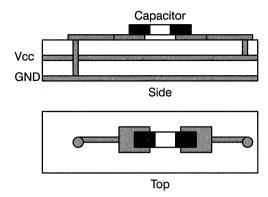
Figure 5. Typical Capacitor Layout
