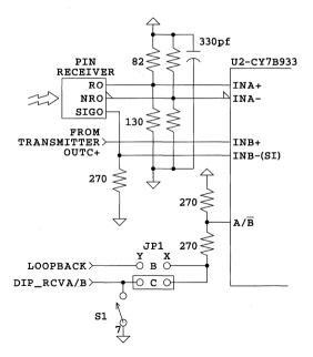
Figure 10. Optical-to-HOTLink Receiver Serial Interface
