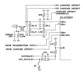
Figure 11. Copper-to-HOTLink Receiver Serial Interface
