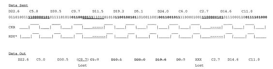
Figure 14. Illustration of Receiver Behavior during Reframe Clock Stretch
