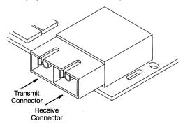
Figure 20. U4 Fiber-Optic Module Connectors
