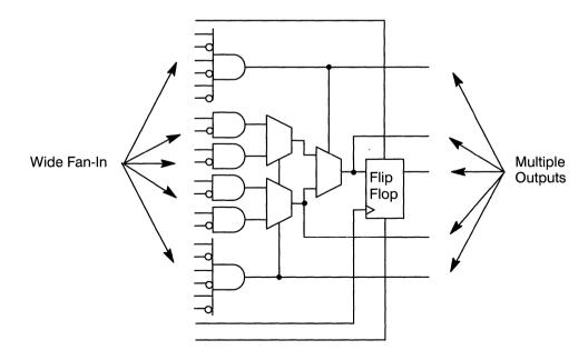
Figure 4. An Optimal Logic Cell
