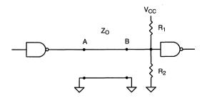
Figure 16. Pull-Up/Pull-Down
