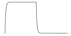
Figure 53. Synthesized K28.7 Waveform
