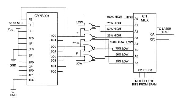
Figure 5. Simplified Laser Modulation Diagram
