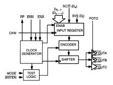
Figure 1. CY7B923 HOTLink Transmitter Logic Block Diagram
