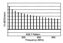
Figure 54. FFT Spectrum of Synthesized K28.7 Pattern
