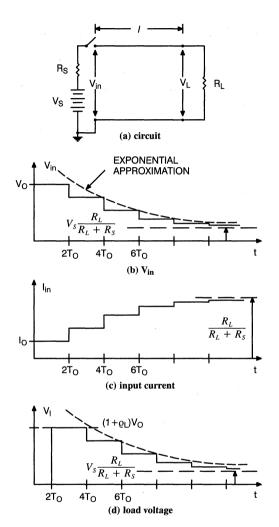
Figure 10. Step Function Applied to Line Mismatched on Both Ends; Shown for Negative Values of  $\rho_S$  and  $\rho_L$
