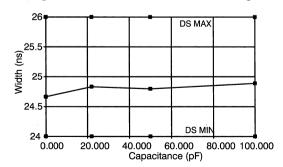
Figure 62. Pulse Width High vs. Capacitance  $t_{REF} = 50$ ns
