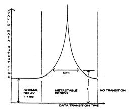
Figure 6. Output Propagation vs. Data Transition
