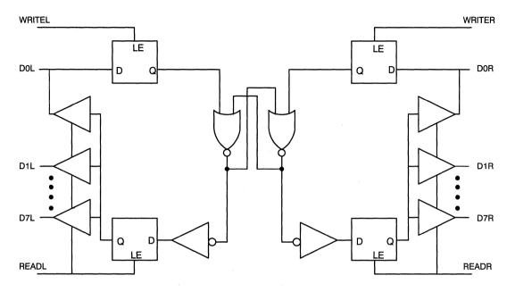
Figure 5. Semaphore Latch Cell
