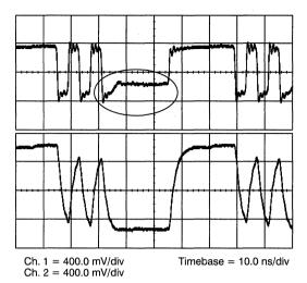
Figure 57. Dual Transformer, Series Secondaries,  $50\Omega$  Resistive Load
