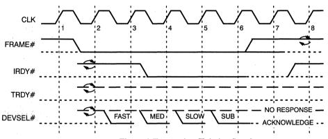
**Figure 6. Transaction Claiming Speed**
