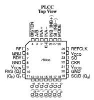
Figure 57. CY7B933 HOTLink Receiver Pin Configuration
