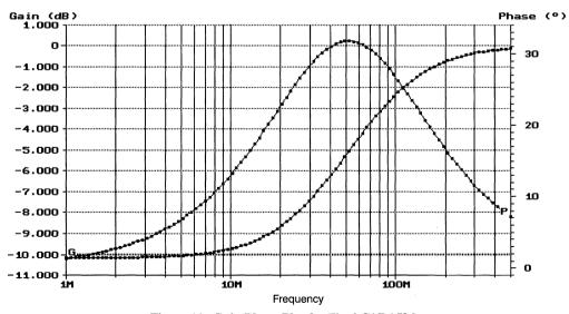
Figure 11. Gain Phase Plot for Final C1/L1 Values
