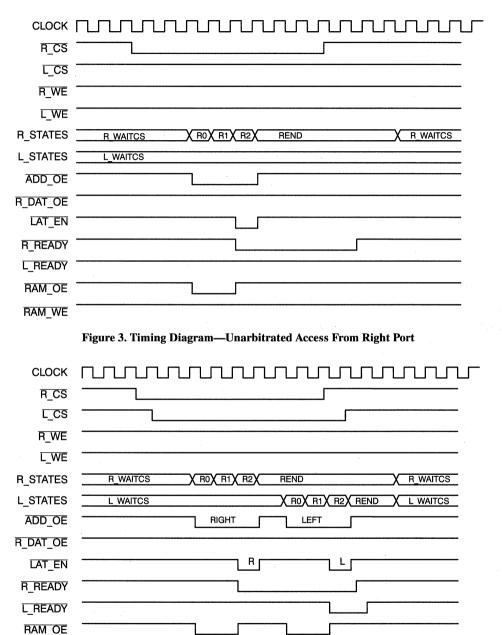
Figure 4. Timing Diagram—Right Port Access Before Left Port
