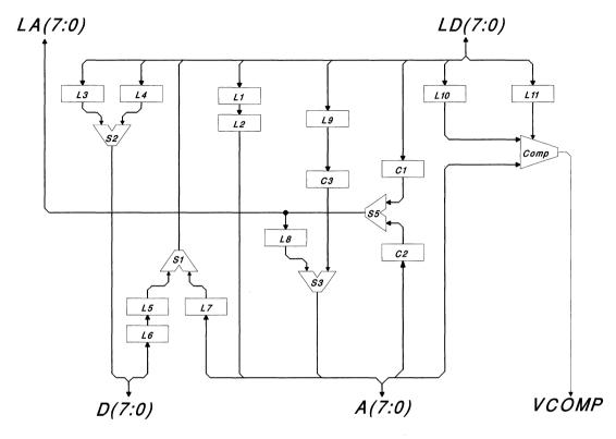
Figure 2. CY7C964 Byte-Width Mode II Block Diagram
