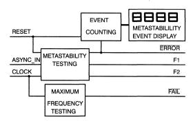
Figure 20. Metastability Test Board Block Diagram
