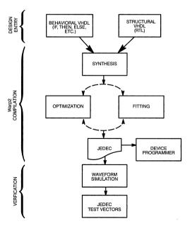
Figure 6. Warp2 Design Flow
