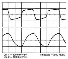
Figure 32. Thévenin Bias, Direct-Coupled, No Cable,  $50\Omega$  Load
