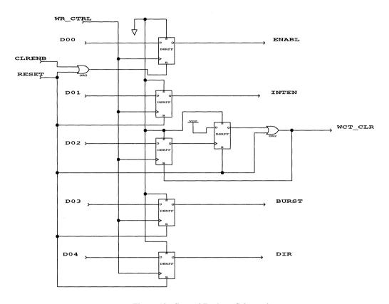
Figure 10. Control Register Schematic
