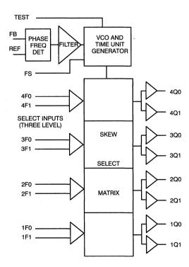
Figure 2. RoboClock Block Diagram
