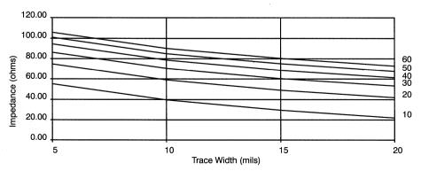
Figure 12. Impedance vs. Trace Width over Dielectric Thickness (Strip Line)
