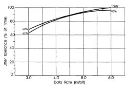
Figure 33. Data-Dependent-Jitter Tolerance as a Function of Data Rate
