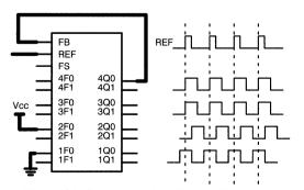
Figure 35. Programmable Phase Adjustment
