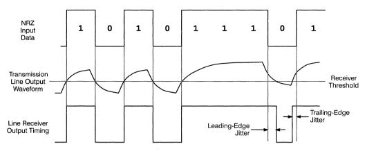
Figure 40. Long Time Constant Transmission Line Response
