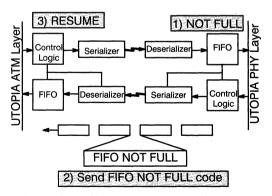
Figure 14. FIFO State Updating, FIFO Not Full
