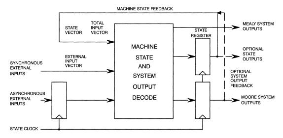
Figure 2. Synchronous State Machine Block Diagram
