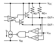
Figure 18. HOTLink Transmitter ECL Output
