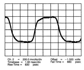
Figure 4. Properly Terminated ECL Waveform
