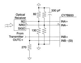
Figure 36. PECL Optical Module-to-HOTLink Receiver
