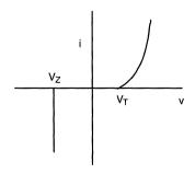
Figure 2. Zener Diode Characteristic
