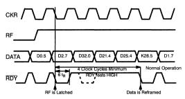
Figure 3. RDY During Framing in Encoded Mode
