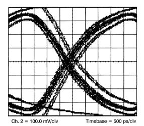
Figure 39. Eye Diagram, Thévenin Bias, Direct-Coupled, with 75Ω Cable
