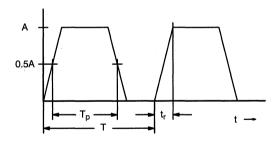
Figure 5. Periodic Pulse Waveform
