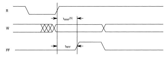
Figure 11. Write Bubble-Through Timing Violation
