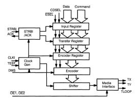
Figure 5. TAXI-275 Transmitter Block Diagram
