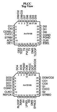
Figure 7. Am79168 and Am79169 Pin Configurations
