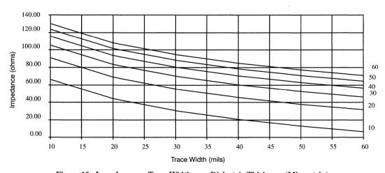
Figure 10. Impedance vs. Trace Width over Dielectric Thickness (Microstrip)
