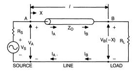
Figure 3. Ideal Transmission Line Loaded and Driven
