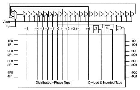
Figure 6. Distributed-Phase Clock Oscillator and Output Adjust Matrix
