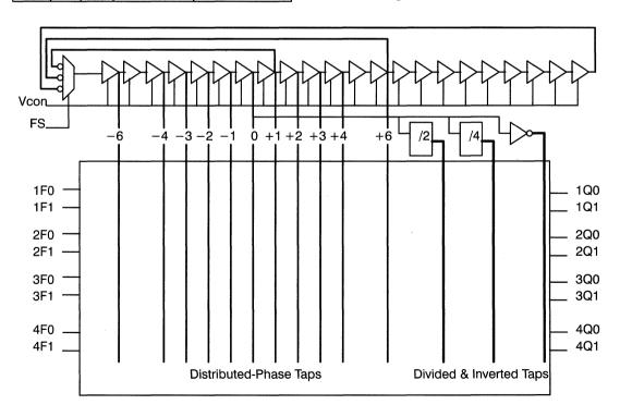
Figure 29. Distributed-Phase Clock Oscillator and Output Adjust Matrix
