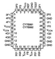
Figure 1. PLCC and LCC Pin Configuration
