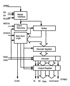
Figure 6. TAXI-275 Receiver Block Diagram
