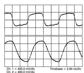
Figure 33. Thévenin Bias, Direct-Coupled, No Cable, 75Ω Load
