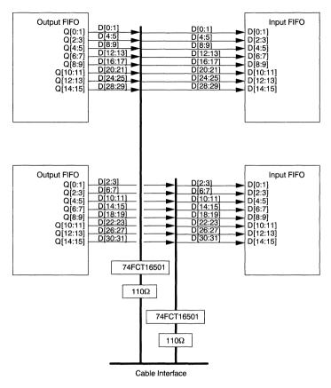
Figure 4. Example—Connecting the FIFOs to a Cable Interface
