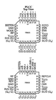
Figure 4. CY7B923 and CY7B933 Pin Configurations
