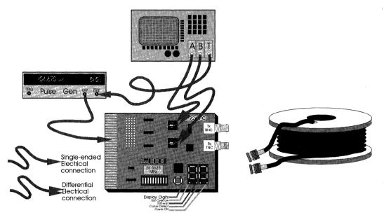
Figure 52. Coax Test Bed to Test for Deterministic Jitter
