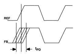
Figure 43. Propagation Delay
