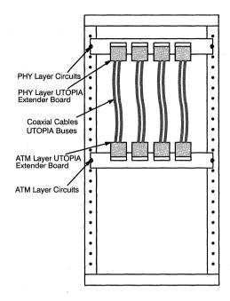
Figure 11. UTOPIA Extender in a Rack Mount Switch
