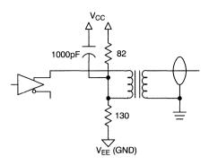
Figure 53. Single Driver, Direct-Coupled, High-Frequency Bypass
