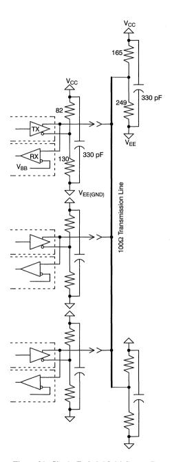
Figure 21. Single-Ended, Multi-Source Bus
