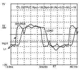
Figure 20.  $50\Omega$  Parallel Termination, 50-pF Load
