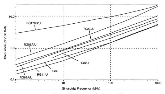
Figure 77. Coaxial Cable Attenuation Characteristics
