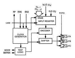
Figure 2a. CY7B923 Transmitter Logic Block Diagram
