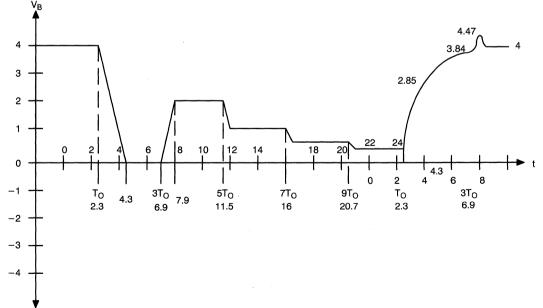
Figure 22b. Unterminated Line Example;  $V_B(t)$
