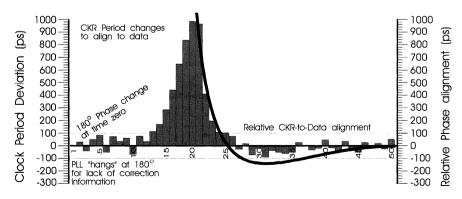
Figure 41. Phase Hop Timing with Exactly 180-Degree Phase Difference
