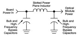
Figure 68. Optical Module Power  $\pi$ -Filter
