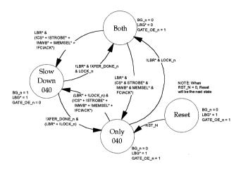
Figure 9. Bus Arbitration State Machine
