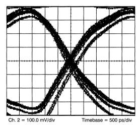
Figure 44. DDJ Measurement
