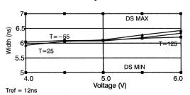
Figure 65. Pulse Width High vs. Voltage over Temperature
