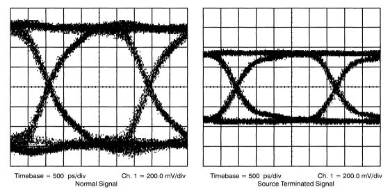
Figure 8. Error-Free, 363-Mbit/second Signal at the Driver End of a 300-Foot RG59 Cable
