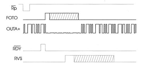
Figure 13. Missing-Transition Test Timing Diagram
