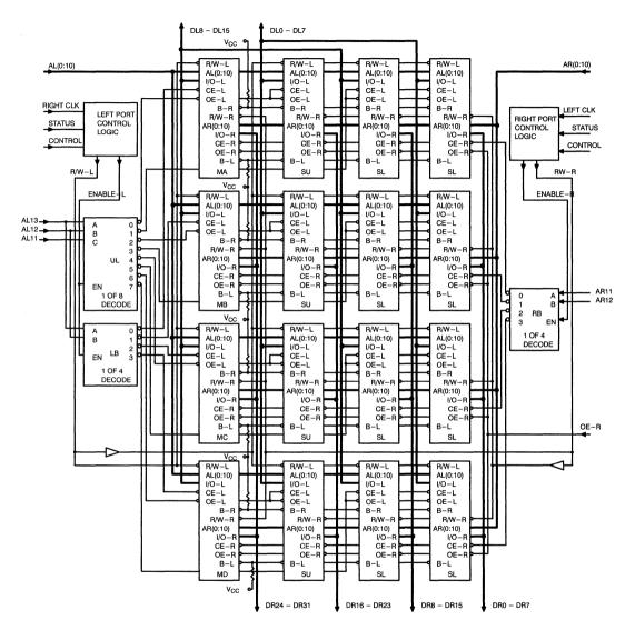
Figure 9. Logic Diagram for Dual-Port Example
