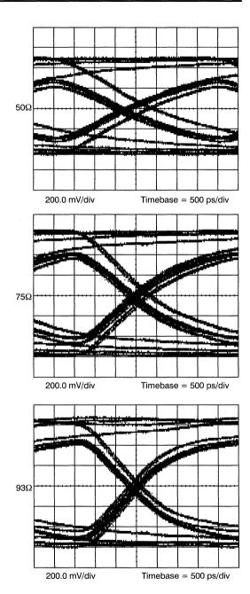
Figure 48. Eye Diagrams, Shunt-Bias, Direct-Coupled, with Cable
