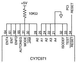
Figure 6. Configuration Pins
