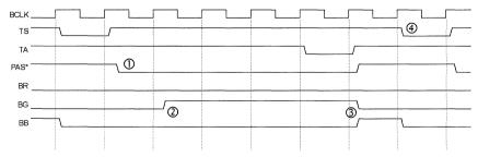
Figure 2. Arbitration Used to Eliminate Contention
