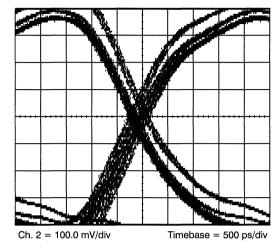
Figure 41. Eye Diagram, Thévenin Bias, Direct-Coupled, with 93Ω Cable
