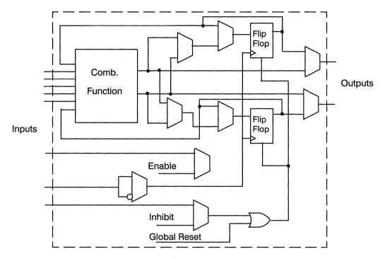
Figure 2. Coarse-Grain Logic Cell
