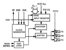
Figure 2. CY7B923 Transmitter Logic Diagram
