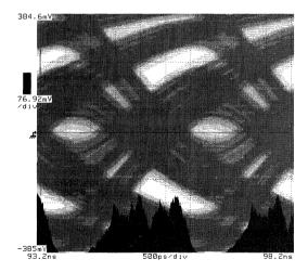
Figure 35. BIST data at 370 Mbaud after 250 ft. of RG-59 coax (BER<4.5x10<sup>-11</sup> with <700 ps eye opening)
