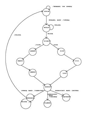
Figure 14. DMA Control State Machine
