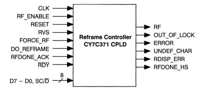
Figure 2. Controller Inputs and Outputs
