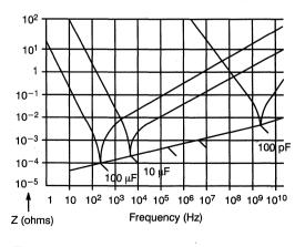
Figure 4. Capacitor Impedance Versus Frequency
