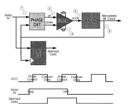
Figure 8. Receive-PLL Block Diagram
