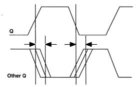
Figure 49. t<sub>SKEW2</sub> and t<sub>SKEW4</sub> Measurement
