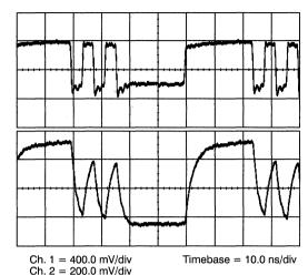
Figure 59. Single Driver, Direct Coupled,  $25\Omega$  Resistive Load
