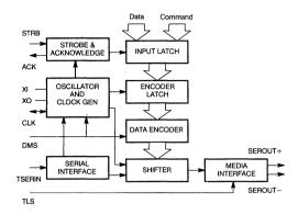
Figure 2. Am7968 Logic Diagram
