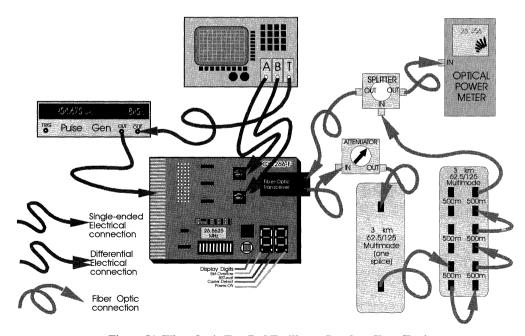
Figure 51. Fiber-Optic Test Bed Facilitates Random-Jitter Testing
