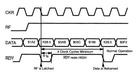
Figure 6. RDY During Framing in Bypass Mode
