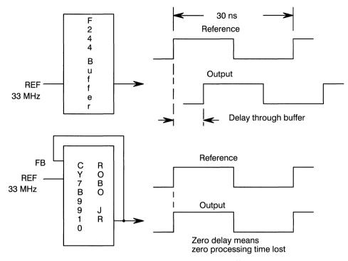
Figure 3. Zero Propagation Delay Buffer
