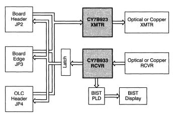
Figure 1. HOTLink Evaluation Board Block Diagram
