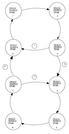
Figure 6. Clock-Generation State Machine
