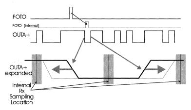
Figure 30. Technique to Measure Static Alignment
