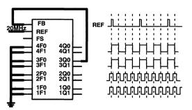
Figure 47. Multi-Function Clock Buffer
