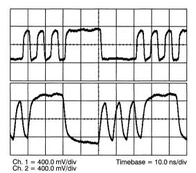
Figure 40. Thévenin Bias, Direct-Coupled, with 93Ω Cable
