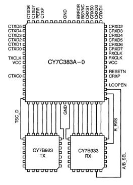
Figure 12. HOTLink/pASIC Pinout and Interconnect
