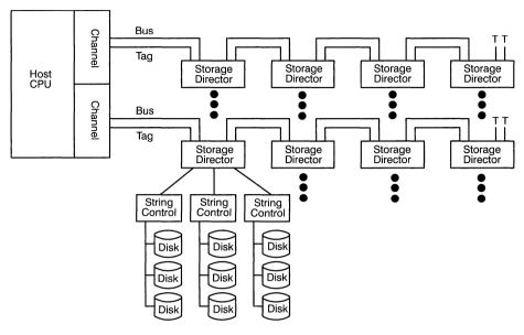
Figure 1. Block-Multiplexer Channel Subsystem
