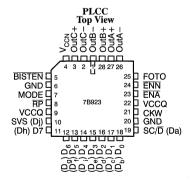
Figure 56. CY7B923 HOTLink Transmitter Pin Configuration
