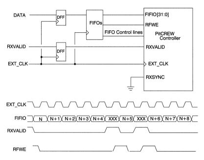
Figure 7. Input Data Qualification with RXVALID
