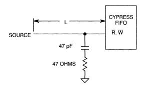
Figure 8. Recommended Termination Network
