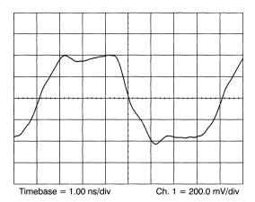
Figure 45. DCD Measurement
