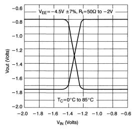
Figure 13. 100K ECL Transfer Functions
