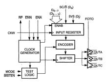
Figure 3. CY7B923 Transmitter Logic Diagram
