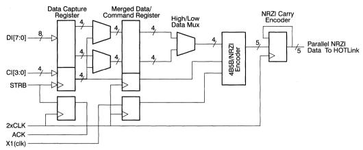
Figure 6. 4B/5B/NRZI Encoder PLD Block Diagram
