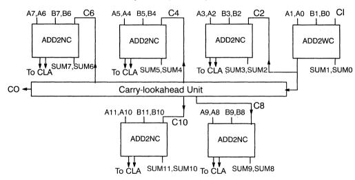
Figure 7. 12-Bit Full Carry-Lookahead Adder Using ADD2WC and ADD2NC
