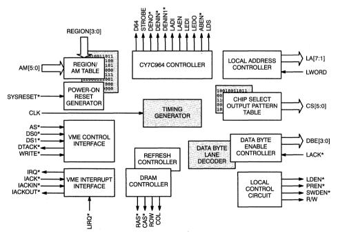
Figure 1. Internal Block Diagram of the CY7C960
