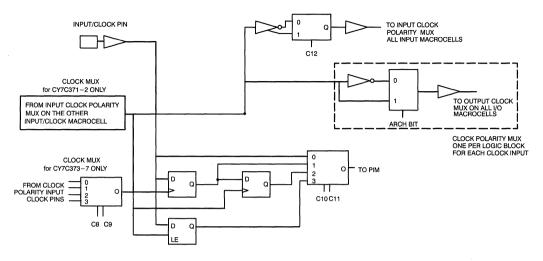
Figure 9. Input/Clock Pins
