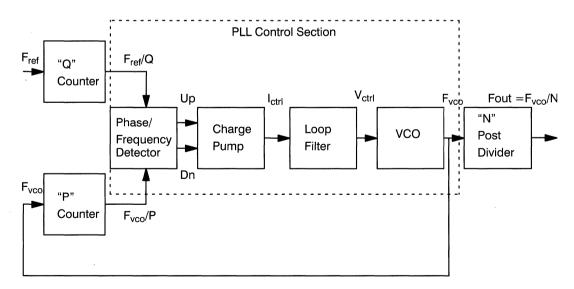
Figure 1. Block Diagram of a Phase-Locked Loop
