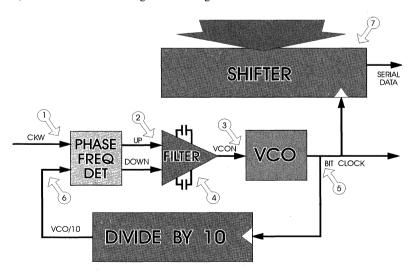
Figure 6. Clock Multiplier PLL Noise Injection Points
