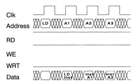
Figure 2. CY7C611A Load Single Operation
