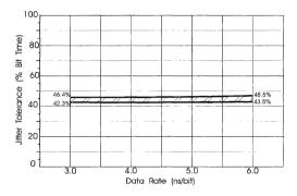
Figure 32. Duty-Cycle-Distortion Jitter Tolerance as a Function of Data Rate
