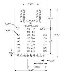
Figure 71. Standard Optical Module Footprint
