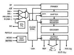
Figure 2b. CY7B933 Receiver Logic Block Diagram
