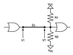
Figure 28. Thévenin Equivalent Parallel Termination
