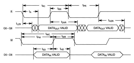
Figure 1. Asynchronous Read and Write Timing
