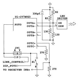
Figure 8. HOTLink Transmitter-to-Optical Serial Interface
