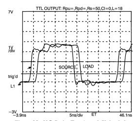
Figure 25. 50Ω Series Terminated, Unloaded
