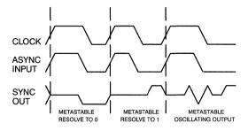
Figure 3. Possible Metastable States of Synchronizer
