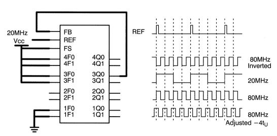
Figure 41. Multi-Function Clock Buffer
