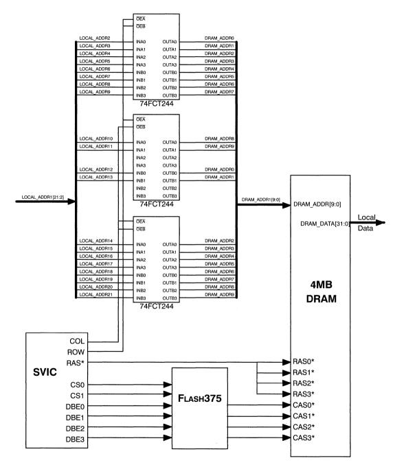
Figure 5. DRAM Interface Logic Example
