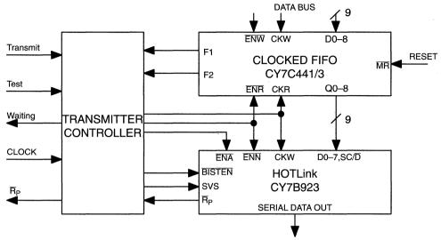
Figure 1. Transmitter Interface Block Diagram
