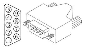
Figure 79. STP Cable Connector and Connector Pinout
