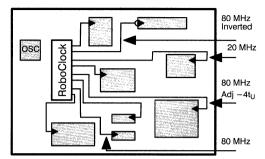
Figure 42. Multi-Function Clock Buffer Application
