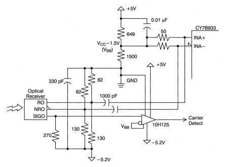
Figure 37. Negative-Referenced Optical Module-to-HOTLink Receiver
