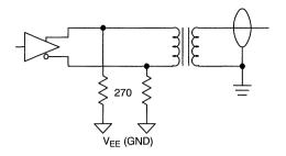
Figure 47. Shunt Bias, Direct-Coupled
