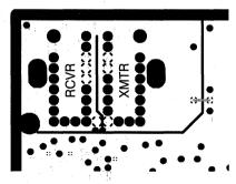
Figure 69. Fiber-Optic Module Slotted Power Plane
