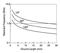
Figure 7. Scope Probe Resonant Frequency
