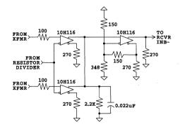
Figure 12. Copper Interface Carrier-Detect
