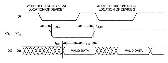
Figure 5. Write Expansion Timing
