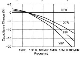
Figure 61. Capacitance vs. Frequency
