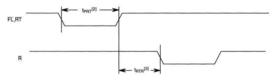
Figure 7. Retransmit Timing
