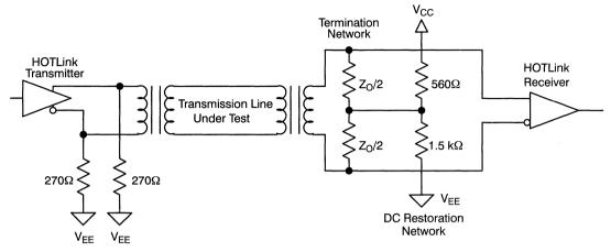
Figure 1. Cable Test Configuration
