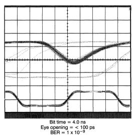
Figure 38. Random Jitter out of Fiber-Optic Link Triggered by RVS & Bit Clock
