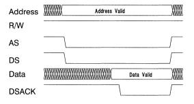
Figure 3. 680x0-Compatible Read Cycle
