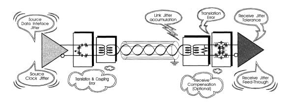
Figure 1. Link Jitter Budget Depends on Link Components
