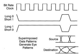
Figure 42. Eye Pattern Generation Waveforms
