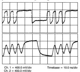
Figure 36. Thévenin Bias, Direct-Coupled, with  $50\Omega$  Cable
