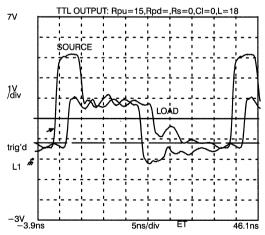
Figure 17. Unloaded 15 $\Omega$  Parallel Termination
