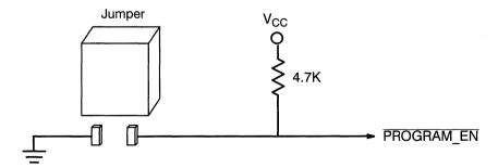
Figure 3. Install Jumper for Programming
