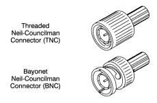
Figure 22. TNC/BNC Cable Connectors
