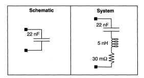
Figure 2. The "Real" Schematic
