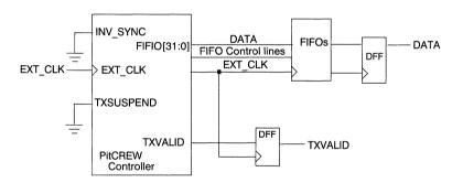
Figure 9. Basic Output Interface
