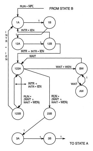
Figure 5. Pipelined States
