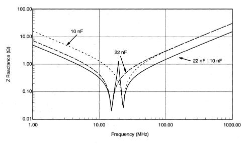
Figure 7. Real Z vs. f for Parallel 22-nF and 10-nF Capacitors
