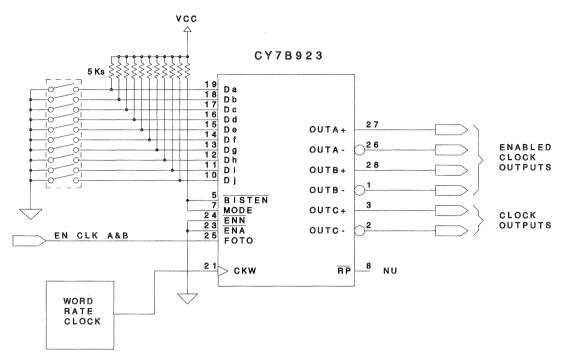
Figure 2. CY7B923 Clock Generator Test Circuit
