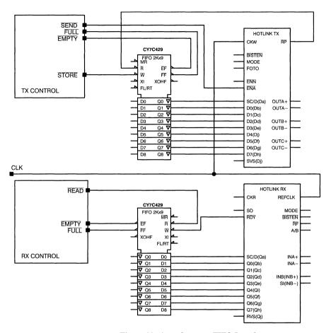
Figure 11. Asynchronous FIFO Interface
