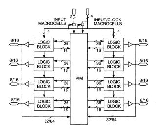
Figure 5. CY7C374/5 Block Diagram
