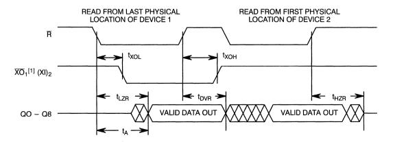
Figure 6. Read Expansion Timing
