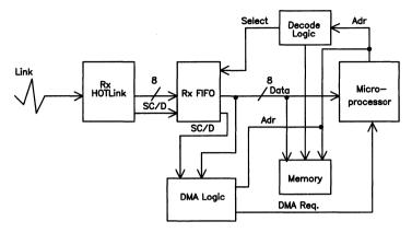
Figure 4. DMA Configuration
