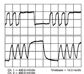
Figure 38. Thévenin Bias, Direct-Coupled, with 75 $\Omega$  Cable
