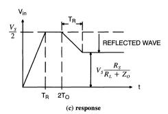
Figure 8. Effect of Rise Time on Response of Mismatched Line with  $R_L < Z_O$
