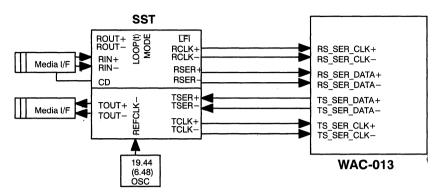
Figure 8. SST to IgT WAC-013 Connection Diagram
