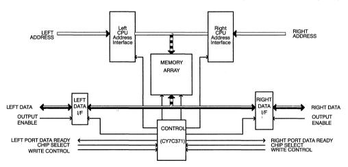
Figure 1. Dual-Port Memory Array Block Diagram
