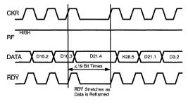
Figure 8. RDY and CKR Stretching (Encoded Mode)
