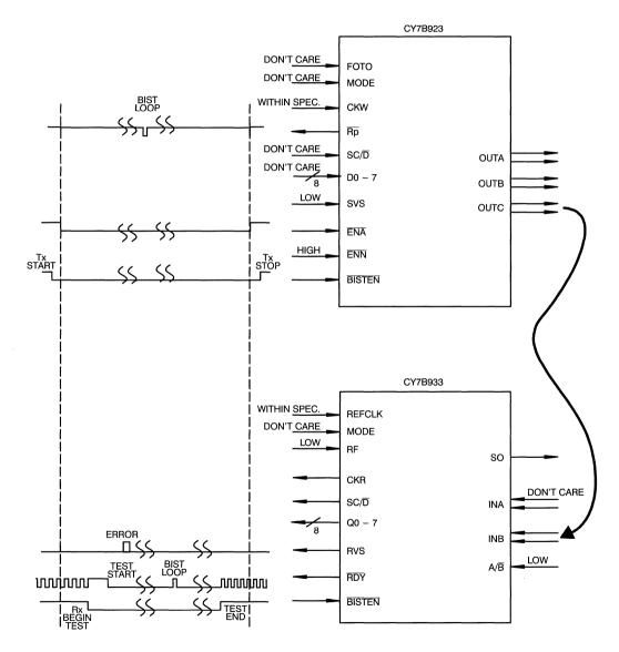
Figure 10. Built-In Self-Test
