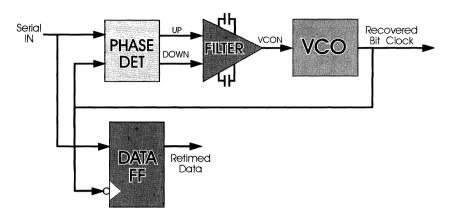
Figure 29. HOTLink Receiver PLL Block Diagram
