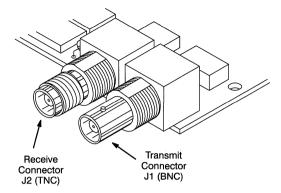
Figure 21. J1 and J2 Coaxial Board Connectors
