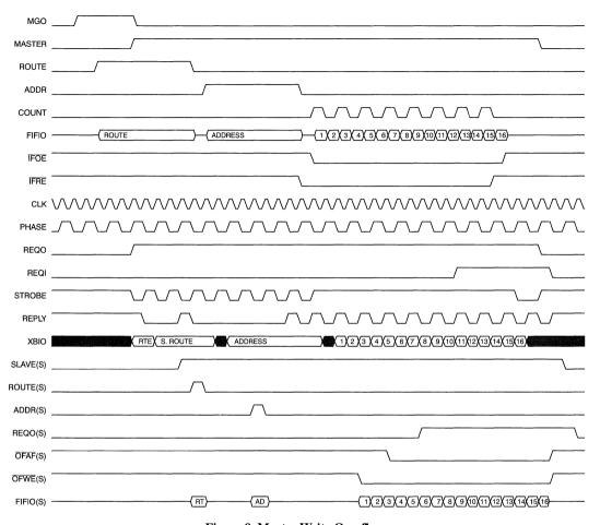
Figure 8. Master Write Overflow
