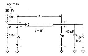
Figure 20. Equivalent Circuit for Cypress PAL Driving
