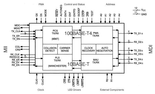
Figure 3. CY7C971 Block Diagram
