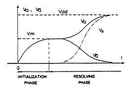
Figure 8. Two Phases of Metastability
