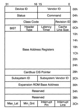
Figure 3. Type 00h Configuration Space Header
