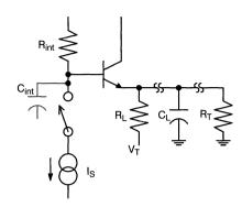
Figure 24. ECL Output Driver with Loading
