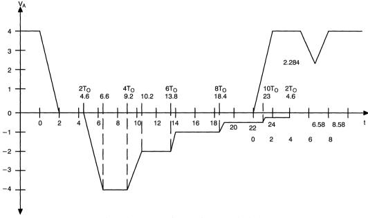
Figure 22a. Unterminated Line Example;  $V_A(t)$
