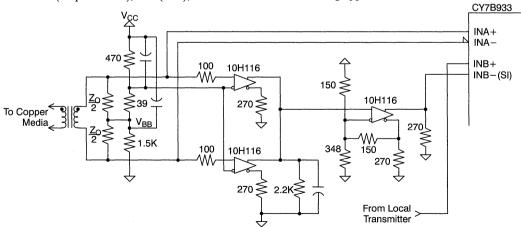
Figure 38. Copper Interface Signal Detect Circuit
