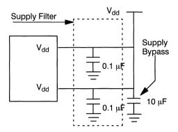
Figure 9. Power Supply Noise Filter Circuit
