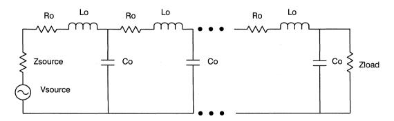
Figure 8. Simplified PCB Trace Model
