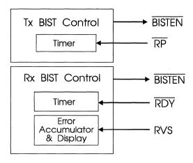
Figure 7. Control Functions for Built-In Self-Test
