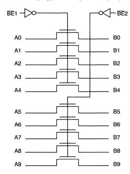
Figure 1. Configuration of the Bus Switch
