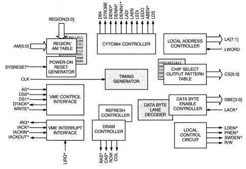
Figure 1. SVIC Block Diagram
