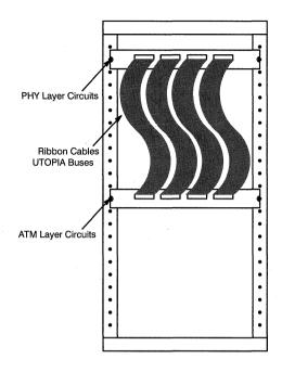
Figure 5. UTOPIA in a Rack Mount Switch
