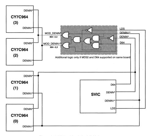
Figure 4. Additional Logic for MD32 Support
