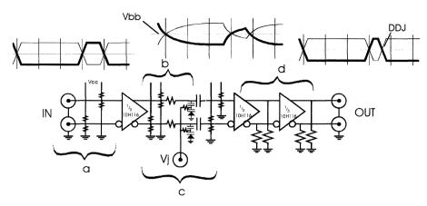
Figure 50. Data Dependent Jitter Generator Schematic
