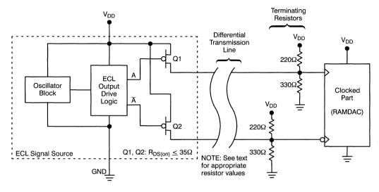
Figure 1. Differential ECL Output Driver
