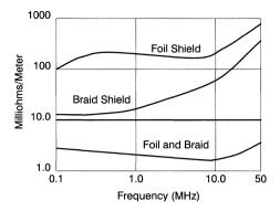
Figure 15. Shield Transfer Impedance
