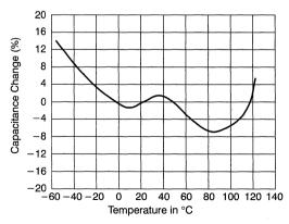
Figure 59. Capacitance vs. Temperature for X7R Dielectrics
