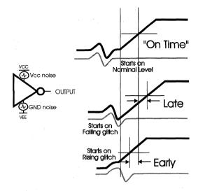
Figure 2. Power Supply Glitches Affect I/O Actual Timing
