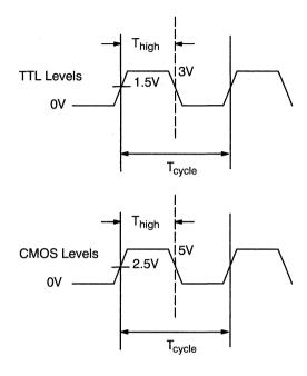
Figure 6. CMOS/TTL Duty Cycle Measurement
