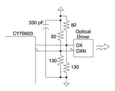
Figure 29. HOTLink Transmitter-to-PECL Optical Module
