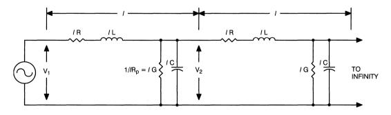
Figure 1. Transmission Line Model
