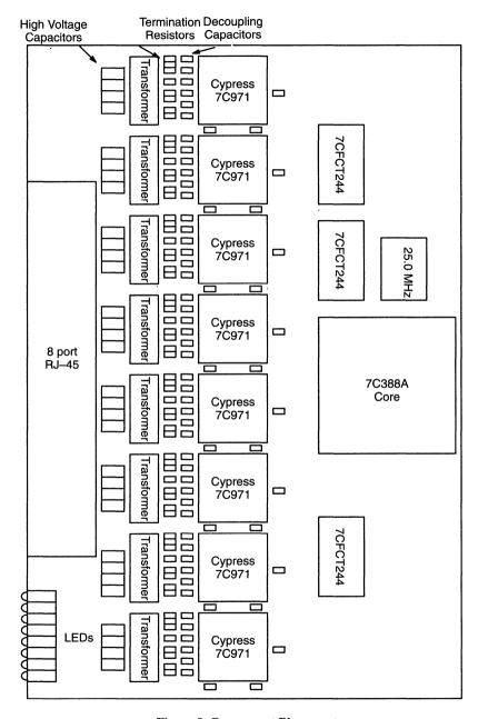
Figure 8. Component Placement
