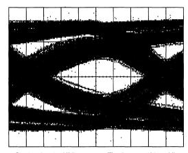
Ch. 1 = 200.0 mV/div Timebase = 500 ps/div Figure 2. Eye Pattern with Forced Noise
