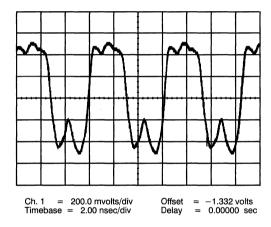
Figure 3. Improperly Terminated Waveform
