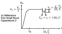
Figure 7. Reflections from Small Discontinuities with a Finite Rise Time Pulse
