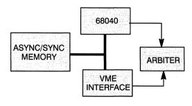
Figure 4. Single Memory Bank Architecture
