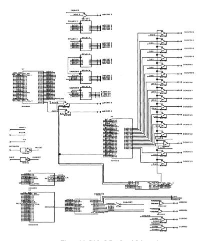
Figure 16. DMAC Top-Level Schematic
