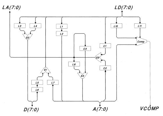
Figure 1. CY7C964 Byte-Width Mode I Block Diagram
