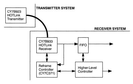
Figure 1. Block Diagram
