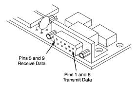
Figure 23. STP P1 Board Connector
