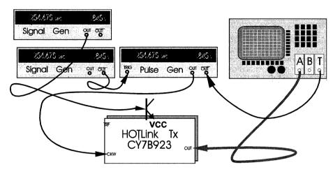
Figure 25. HOTLink Transmitter V<sub>CC</sub> Coupled Jitter Set-Up
