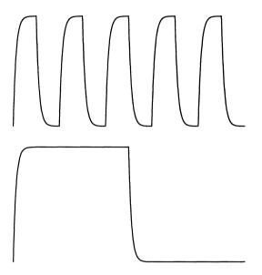
Figure 3. Synthesized D21.5 and K28.7 Waveforms
