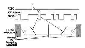
Figure 11. Example of Error Free Window Testing
