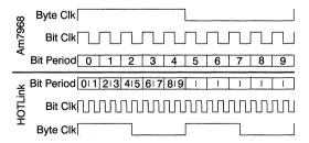
Figure 5. Am7968 vs CY7B923 Bit Timing
