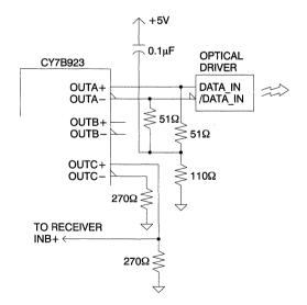
Figure 7. HOTLink Transmitter-to-Optical Serial Interface
