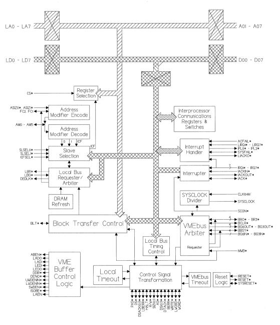
Figure 1. VIC068A Functional Block Diagram
