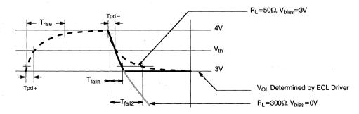
Figure 26. Expanded Detail of Falling Edge Rate Comparison
