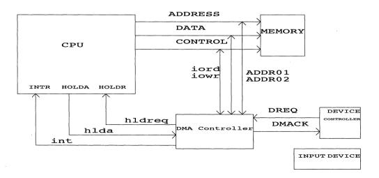
Figure 7. DMA Controller Controlling an Input Device
