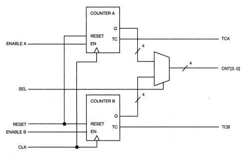
Figure 1. Multiplexed Dual Counter Design
