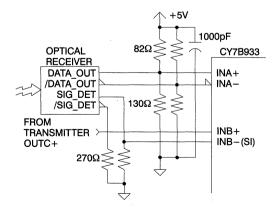
Figure 8. Optical-to-HOTLink Receiver Serial Interface
