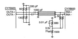
Figure 23. Capacitive-Coupled, Copper Interface
