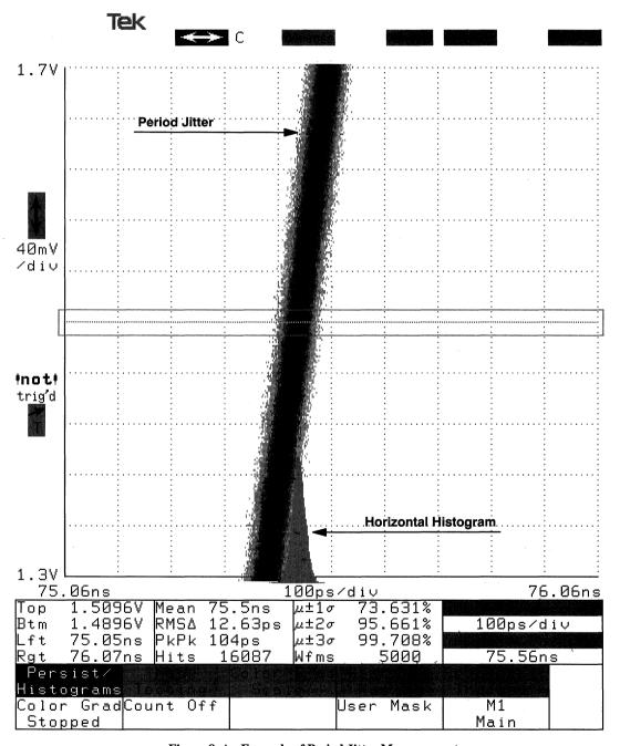
Figure 8. An Example of Period Jitter Measurement
