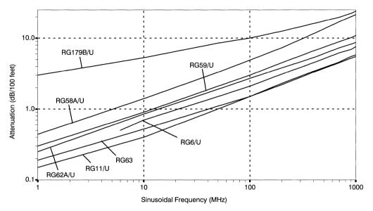
Figure 2. Coaxial Cable Attenuation Characteristics
