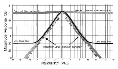
Figure 11. V<sub>CC</sub> Noise Injection Transfer Function
