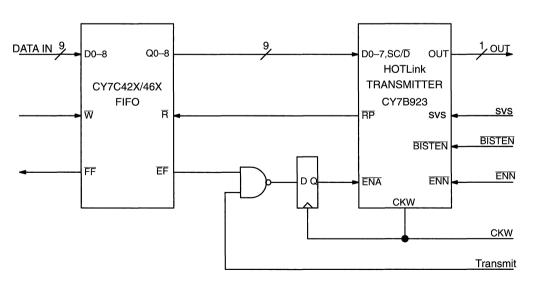
Figure 1. Transmitter Interface Diagram
