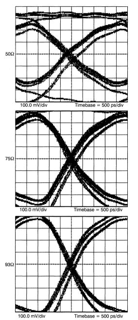
Figure 44. Eye Diagrams, Thévenin Bias, AC-Coupled, with Cable
