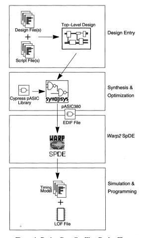
Figure 4. Design Compiler-Warp Design Flow
