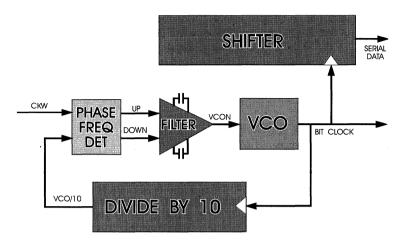
Figure 13. HOTLink Transmitter PLL Block Diagram
