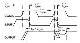
Figure 5. Triggering Modes of a Simple Flip-Flop
