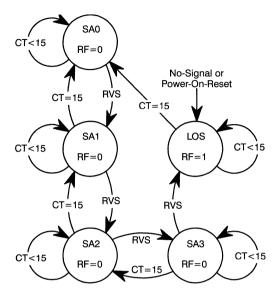
Figure 3. Synchronization State Machine
