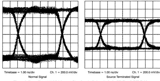
Figure 6. Error-Free, 173-Mbit/second Signal at the Driver End of a 550-Foot RG59 Cable
