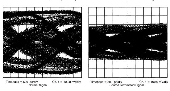
Figure 9. Error-Free, 363-Mbit/second Signal at the Receiver End of a 300-Foot RG59 Cable
