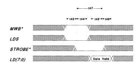
Figure 5. Mask Register Load Cycle
