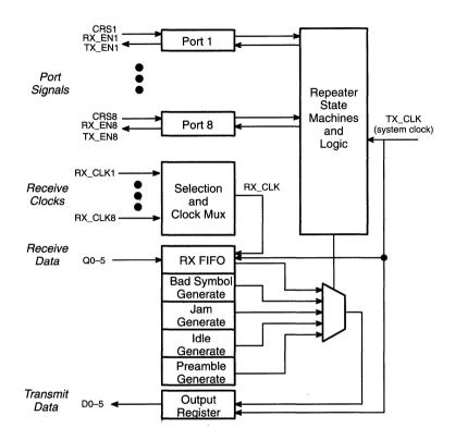
Figure 9. Core Logic
