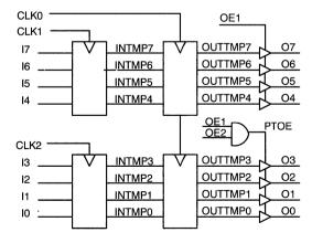
Figure 7. Pipelined Buffer Block Diagram
