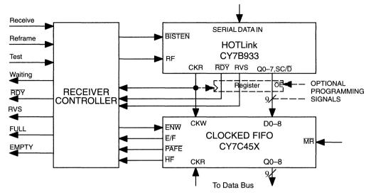
Figure 4. Receiver Interface Block Diagram
