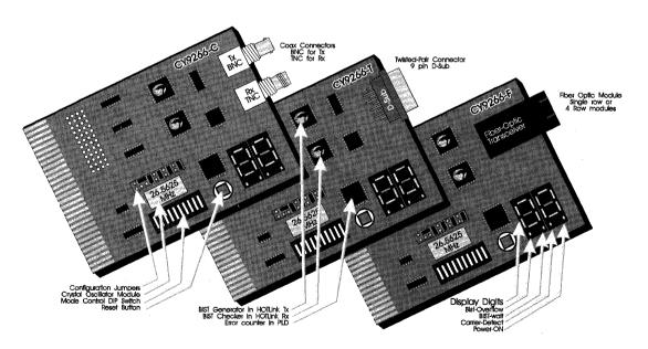
Figure 53. HOTLink Evaluation Boards Form the Core of a Comprehensive Evaluation System
