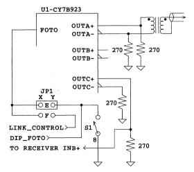
Figure 9. HOTLink Transmitter to Copper Serial Interface
