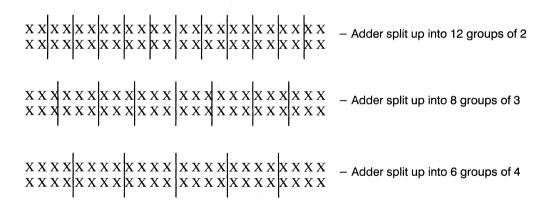
Figure 13. Three Different Carry-Lookahead Schemes to Implement a 24-Bit Adder
