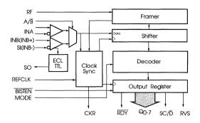
Figure 3. HOTLink Receiver Block Diagram
