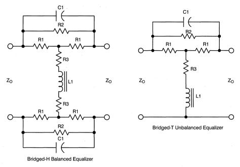
Figure 9. Constant Impedance Equalizer Circuits
