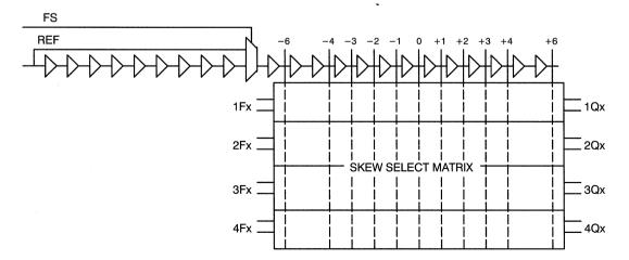
Figure 3. RoboClock Test Mode
