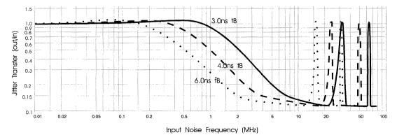
Figure 23. HOTLink Transmitter Jitter Transfer Function
