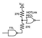
Figure 35. TTL-to-HOTLink PECL Interface
