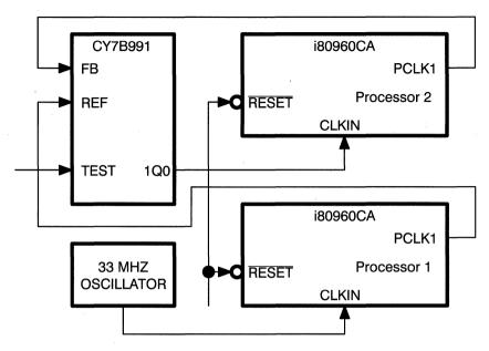
Figure 1. Clock Connections for Synchronization
