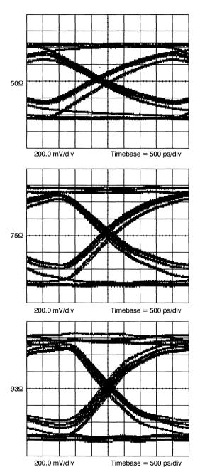
Figure 50. Eye Diagrams, Shunt Bias, AC-Coupled, with Cable
