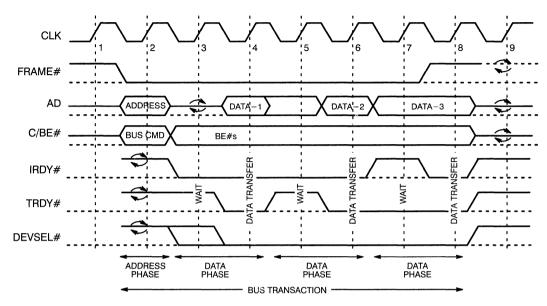
Figure 4. Read Transaction Waveform
