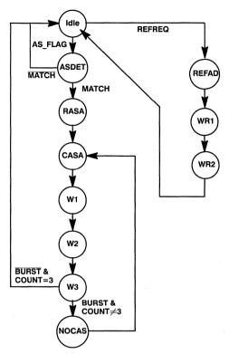
Figure 4. Controller State Machine State
