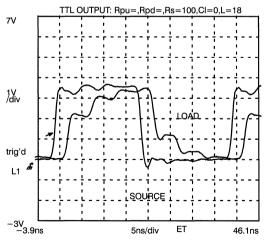
Figure 24.  $100\Omega$  Series Terminated, Unloaded
