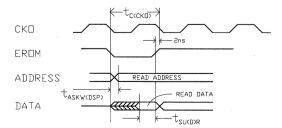
Figure 2. DSP1616 External Program Memory Timing
