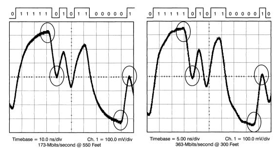
Figure 10. Error-Free, K28.5 Character at Maximum Data Rate
