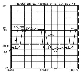
Figure 19. 50Ω Parallel Termination, 22-pF Load
