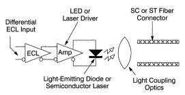
Figure 67. Fiber-Optic Emitter Module Block Diagram
