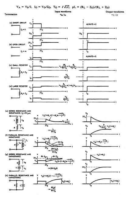
Figure 4. Step Function Response of Figure 3 for Various Terminations
