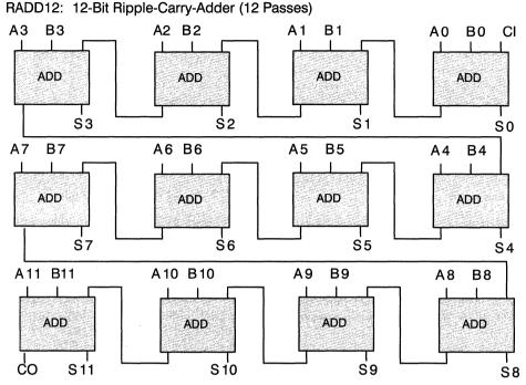
Figure 2. Block Diagram of a 12-Bit Ripple Carry Adder
