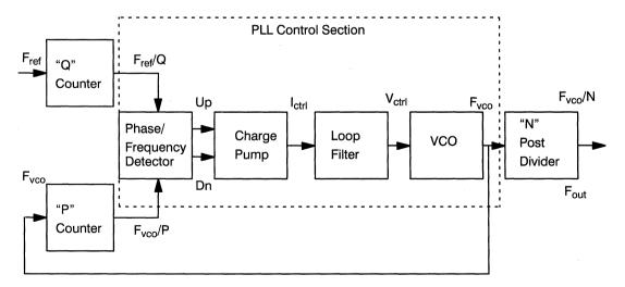
Figure 1. Block Diagram of a Phase Locked Loop
