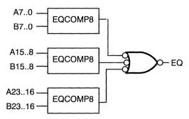
Figure 15. Block Diagram of a 24-Bit Equality Compare
