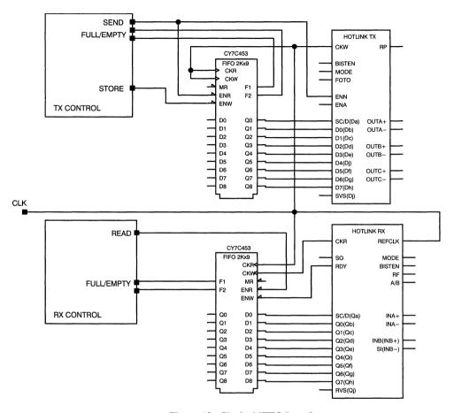
Figure 12. Clocked FIFO Interface
