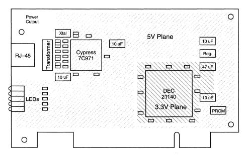
Figure 7. Power Plane and Component Placement
