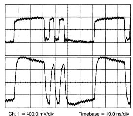
Figure 54. Single Driver, Direct-Coupled, High-Frequency Bypass,  $50\Omega$  Resistive Load
