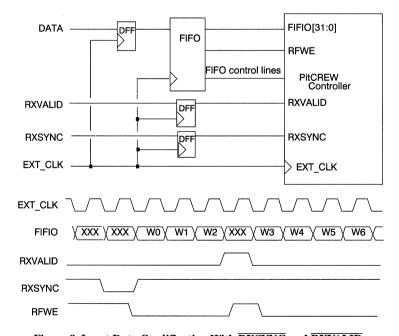
Figure 8. Input Data Qualification With RXSYNC and RXVALID
