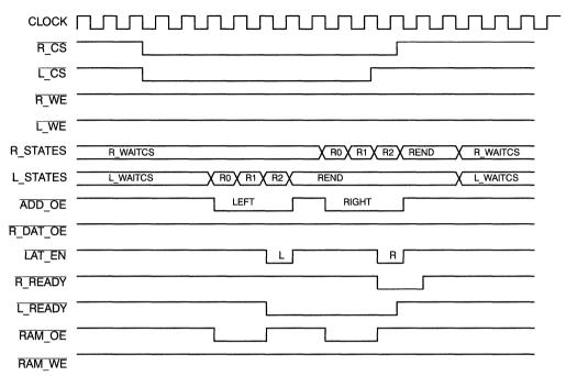
Figure 5. Timing Diagram—Simultaneous Access
