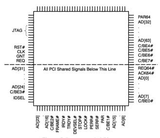
Figure 7. Recommended Pinout
