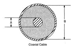
Figure 12. Coaxial Cable Critical Dimensions
