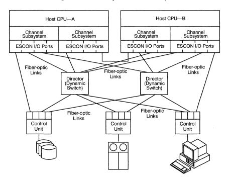
Figure 2. ESCON Channel Subsystem
