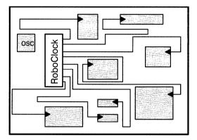
Figure 34. RoboClock in Low Skew Buffer Application
