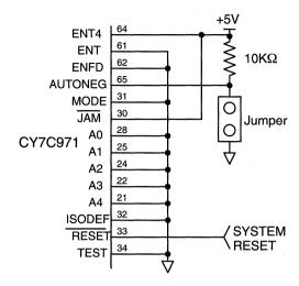
Figure 7. Configuration Pins
