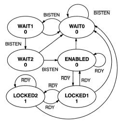
Figure 17. BIST State Machine Bubble Diagram
