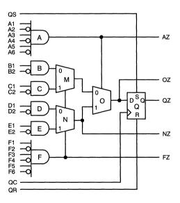
Figure 12. pASIC380 Internal Logic Cell
