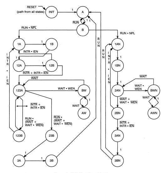
Figure 6. CPU Clock State Machine
