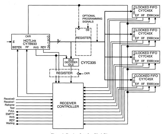
Figure 4. Receiver Interface Block Diagram
