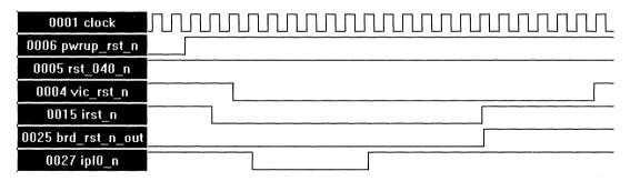
Figure 6. Power-Up or Pushbutton Reset
