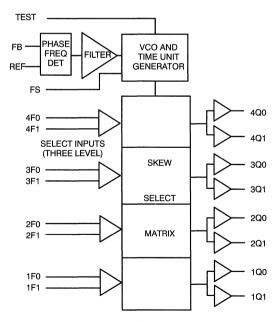
Figure 1. Logic Block Diagram
