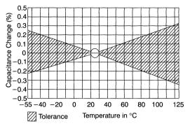
Figure 62. Capacitance vs. Temperature for NP0/C0G Dielectrics
