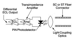
Figure 70. Fiber-Optic Detector Module Block Diagram
