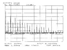
Figure 4. Frequency Components of an 80-MHz Clock Signal
