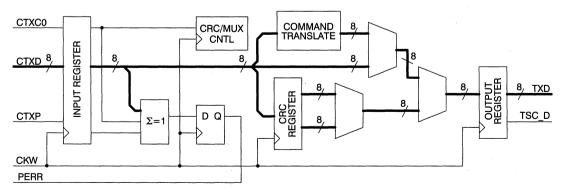
Figure 9. pASIC Transmit Path Block Diagram
