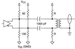
Figure 45. Transformer Core Saturation Test Fixture
