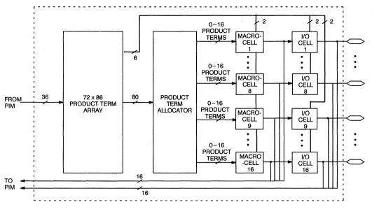
Figure 7. Logic Block for CY7C371, CY7C373, CY7C375, and CY7C377 (I/O Intensive)
