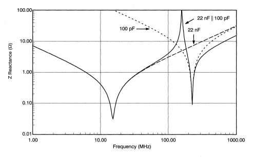
Figure 5. Real Z vs. f for Parallel 22-nF and 100-pF Capacitors
