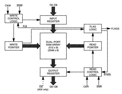
Figure 2. Clocked FIFO Data Path
