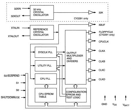
Figure 1. Block Diagram of CY2291/2
