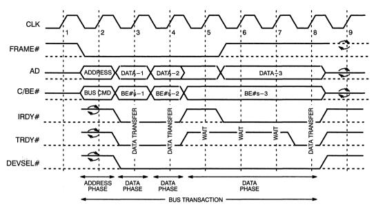
Figure 5. Write Transaction Waveform
