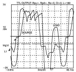
Figure 14. Unterminated Transmission Line
