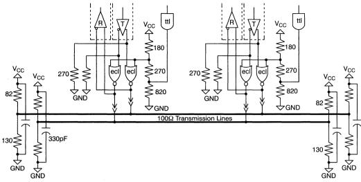
Figure 22. Differential, Multi-Source Bus
