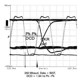
Figure 46. CKR Output Jitter as DCD Corrupted Data is Being Received
