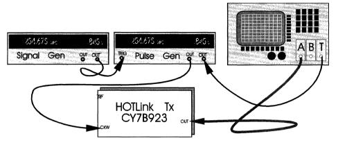
Figure 14. HOTLink Transmitter Random Jitter Set-Up
