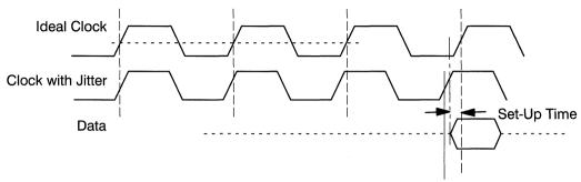
Figure 5. Application for Period Jitter Measurement
