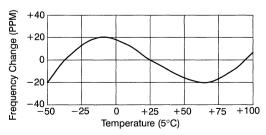
Figure 55. Oscillator Temperature Stability
