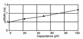
Figure 59. Fall Time vs. Capacitance
