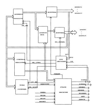
Figure 8. DMAC Block Diagram
