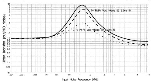
Figure 26. HOTLink Transmitter V<sub>CC</sub> Coupled Jitter Transfer Characteristic
