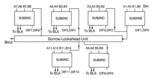
Figure 12. 12-Bit Fast Borrow Subtracter Built using SUB2WB and SUB2NC
