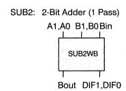
Figure 11. Block Diagram of a 2-Bit Subtracter with a Borrow-Out
