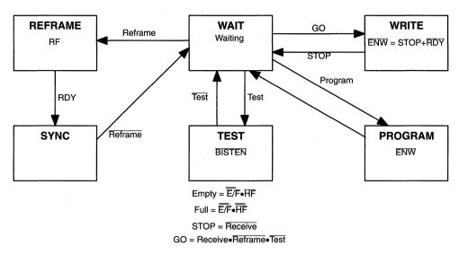
Figure 5. Receiver Controller State Diagram
