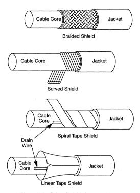
Figure 14. Cable Shield Constructions
