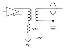
Figure 35. Thévenin Bias Equivalent Circuit
