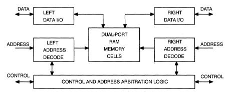
Figure 1. Dual-Port RAM Block Diagram
