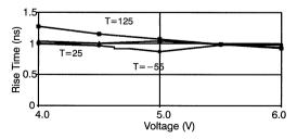
Figure 57. Rise Time vs. Voltage over Temperature
