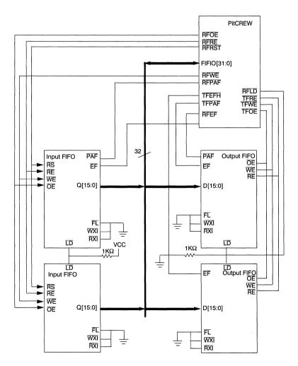
Figure 5. Connecting the FIFOs to the PitCREW Controller
