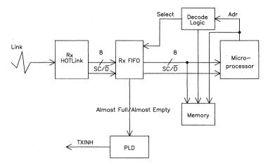
Figure 3. Receiver Flow Control
