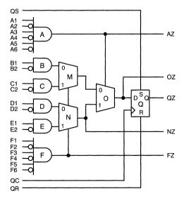
Figure 6. pASIC380 Internal Logic Cell
