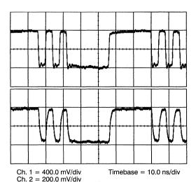
Figure 52. Single Driver, Direct-Coupled,  $50\Omega$  Resistive Load
