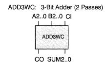
Figure 5. A 3-Bit Full Adder with a Carry-Out
