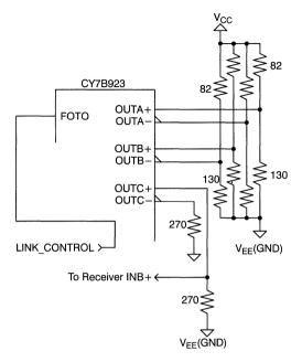
Figure 27. Baseline Test Configuration
