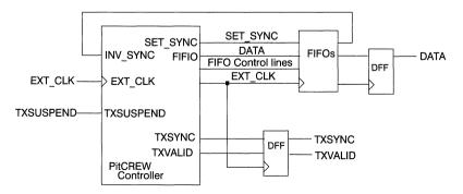
Figure 10. Output Interface with TXSUSPEND and TXSYNC
