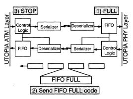
Figure 13. FIFO State Updating, FIFO Full
