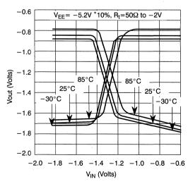
Figure 11. 10K ECL Transfer Functions
