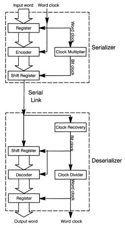
Figure 7. Architecture of a Serial Link
