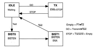
Figure 2. Transmitter Controller State Diagram
