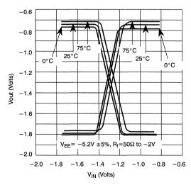
Figure 12. 10KH ECL Transfer Functions
