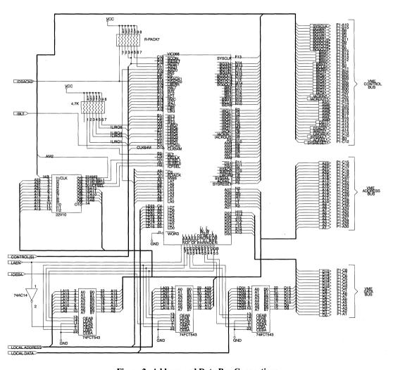
Figure 2. Address and Data Bus Connections
