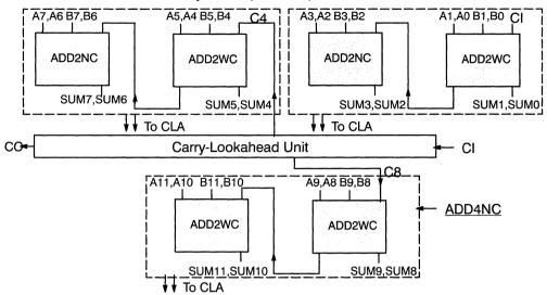
Figure 9. 12-Bit Full Carry-Lookahead Adder using ADD4NC
