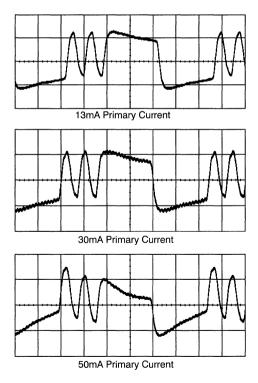
Figure 46. Transformer Core Saturation Test
