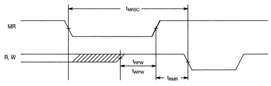
Figure 9. Master Reset Timing
