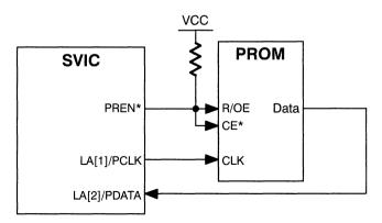
Figure 10. Connection of SVIC to Serial PROM
