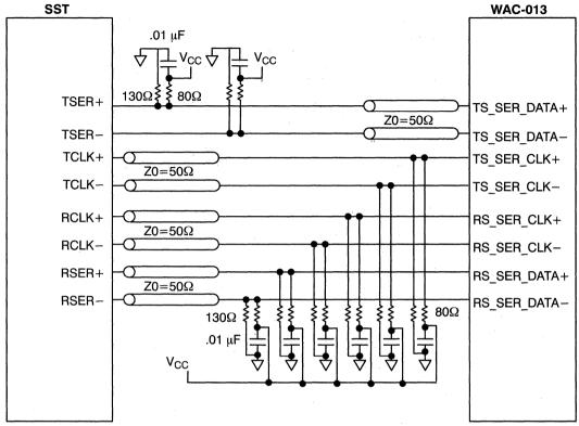
Figure 9. High Performance SST to WAC-013 Interface
