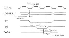
Figure 6. Motorola DSP56000 External Program Memory Timing
