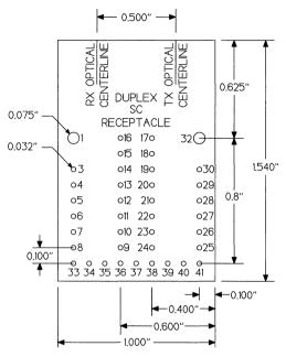
Figure 18. Optical Module, Top View Dimensions
