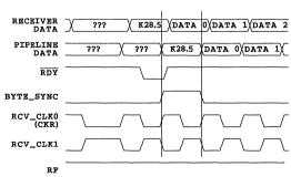
Figure 14. Receiver Data Timing, Bypass Mode, RF HIGH
