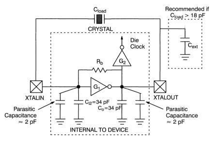
Figure 3. Using a Crystal as Reference
