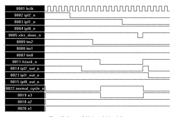
Figure 17. Interrupt Initiation and Acknowledge
