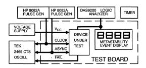
Figure 22. Metastability Test Set-Up
