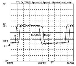
Figure 18.  $50\Omega$  Parallel Termination, Unloaded
