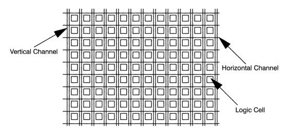
Figure 1. Global FPGA Architecture
