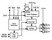
Figure 2. CY7B923 Transmitter Logic Block Diagram
