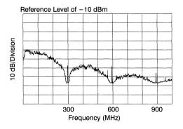
Figure 48. BIST Pattern Spectral Characteristics
