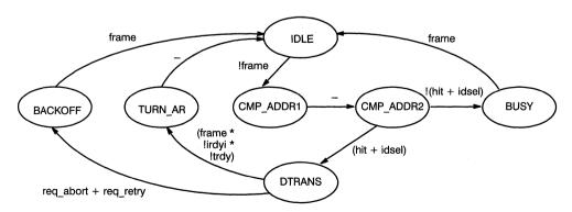
Figure 9. PCI Interface State Machine
