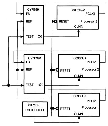
Figure 2. Clock Connections for Synchronization of Three Processors
