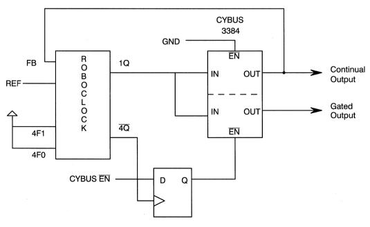
Figure 5. Gated RoboClock
