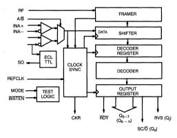
Figure 3. CY7B933 Receiver Logic Diagram
