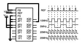
Figure 40. Frequency Divider and Multiplier
