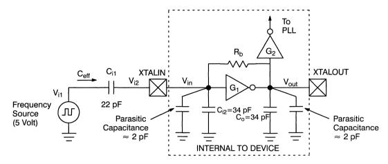
Figure 5. Using an External Driver as Reference
