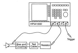
Figure 30. Test Set-Up
