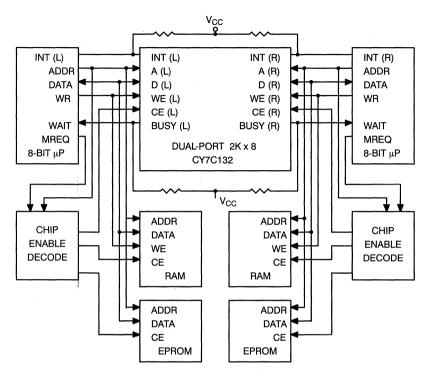
Figure 7. Typical 8-Bit Microprocessor
