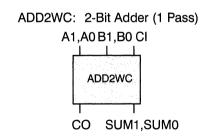
Figure 3. A 2-Bit Full Adder with a Carry-Out
