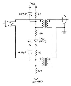
Figure 56. Dual Transformer, Series Secondaries
