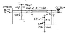
Figure 32. Capacitive-Coupled, Copper Interface
