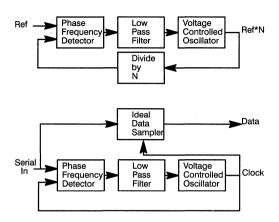
Figure 8. Multiplication and Clock/Data Recovery PLLs
