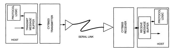
Figure 1. HOTLink System Connections
