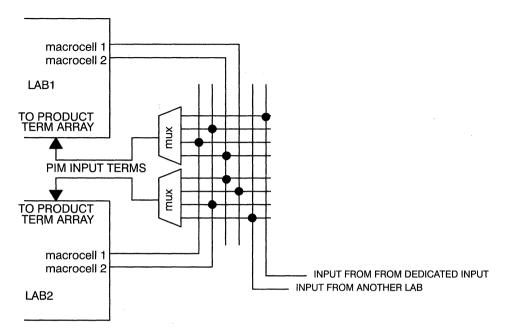
Figure 4. Mux Based Interconnect
