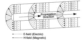
Figure 1. Electric and Magnetic Fields for TEM Mode in a Coaxial Transmission Line
