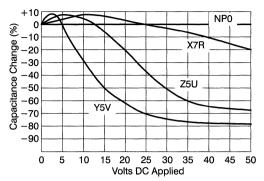
Figure 60. Capacitance vs. DC Voltage
