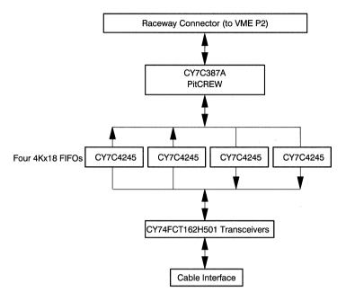
Figure 1. Components of a Sample I/O Interface
