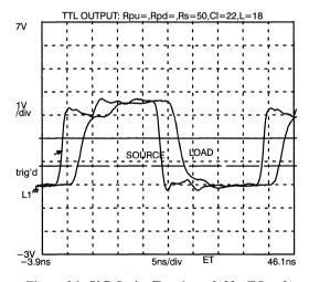
Figure 26.  $50\Omega$  Series Terminated, 22-pF Load
