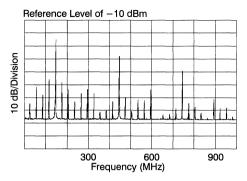
Figure 49. 0101 (D21.5) Pattern Spectral Characteristics
