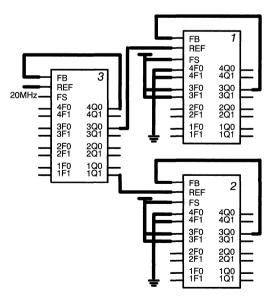
Figure 51. Devices in Parallel and Serial
