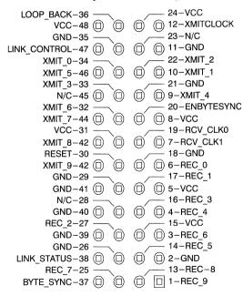
Figure 4. JP4 Pin Numbering, Top Side of Board View (Pins Are On the Bottom)
