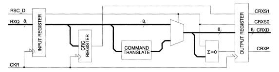
Figure 10. pASIC Receive Path Block Diagram
