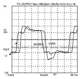
Figure 16. Unloaded  $100\Omega$  Parallel Termination
