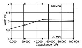
Figure 63. Pulse Width High vs. Capacitance  $t_{REF} = 12ns$
