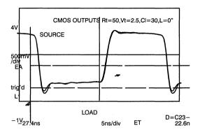
Figure 45. Lumped Load with Datasheet Load
