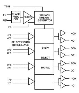
Figure 1. Logic Block Diagram
