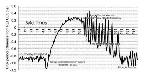
Figure 43. Frequency Acquisition from/to +3.0% Changes CKR Period
