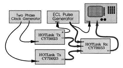
Figure 15. Receiver Phase Tolerance Test Setup
