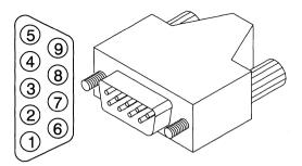
Figure 24. STP Cable Connector and Connector Pinout
