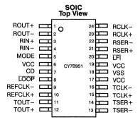
Figure 2. SST Pinout
