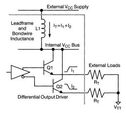
Figure 23. Loaded Differential Driver
