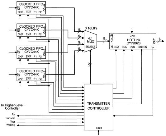
Figure 1. Transmitter Interface Block Diagram
