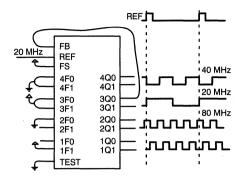
Figure 32. Frequency Multiplier with Phase Adjustment
