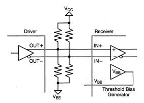
Figure 15. Differential Connection
