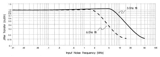
Figure 45. HOTLink Receiver Jitter Transfer Function (BIST Data)
