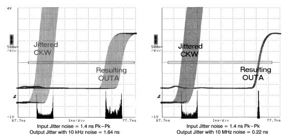
Figure 24. Serial Output Jitter Varies as a Function of Input Noise Frequency
