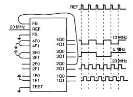
Figure 31. Frequency Divider Connections
