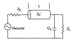
Figure 13. Simplified Transmission Line
