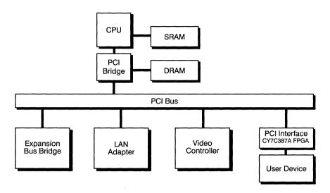
Figure 1. PCI Architecture
