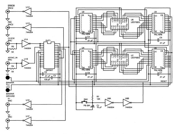
Figure 21. Metastability Test Board Schematic
