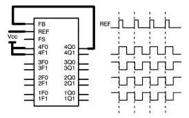
Figure 37. Inverted Output Clock Driver
