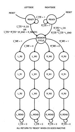
Figure 2. Memory Control Function State Machine
