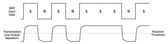
Figure 39. Short Time Constant Transmission Line Response
