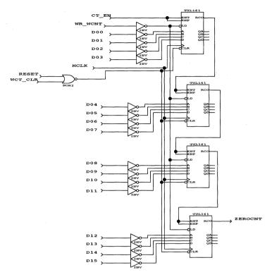
Figure 12. Word Counter Implemented in Warp3 Schematic Capture Tool
