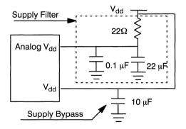
Figure 10. Power Supply Noise Filter Circuit
