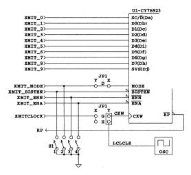
Figure 7. Transmitter Parallel Interface
