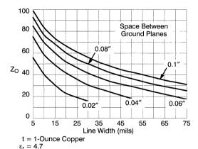
Figure 10. Calculated Impedance vs. Trace Width for Stripline Transmission Lines
