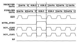
Figure 15. Receiver Data Timing, Decode Mode, RF LOW
