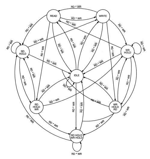
Figure 1. FIFO Dipstick State Machine Bubble Chart
