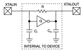
Figure 2. On-Chip Crystal Oscillator Circuitry
