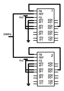
Figure 50. Part-to-Part Skew Example
