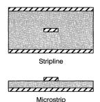
Figure 6. Circuit Board Transmission Lines
