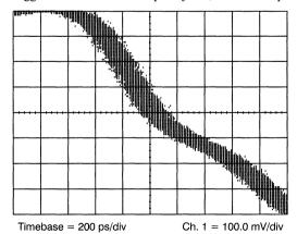
Figure 46. RJ Measurement
