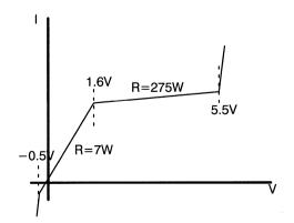
Figure 22. Output LOW Linearized V-I Curve
