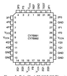
Figure 2. RoboClock PLCC/LCC Pinout
